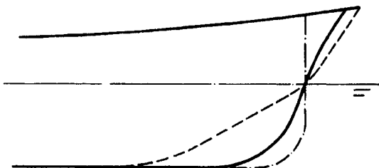
Figure 2.4 Various bulbless bow forms. — Conventional form; - - - Maier bow of 1930s; - · - · Vertical stem, in use from mid-nineteenth century to around 1930
