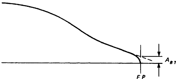
Figure 2.15 Bulb with projecting length. Theoretical bulb section area of the forward perpendicular
