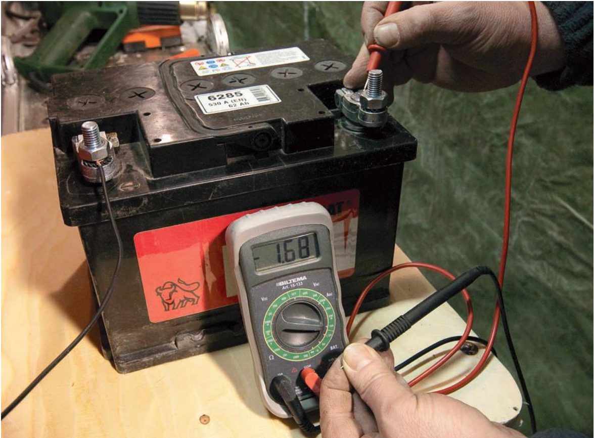
To check current you need to put the multimeter in series with the circuit to test - here I used the battery to test the amperage of a filament bulb lamp (out of picture).
