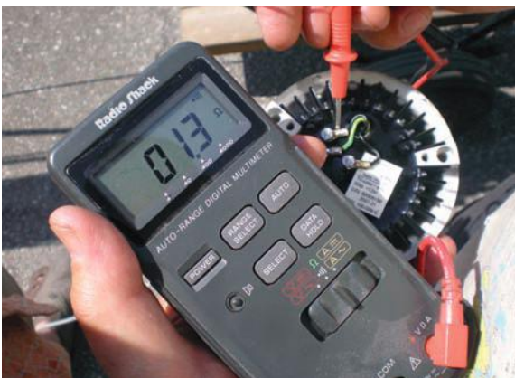
To check which cable went to the lamp, I used the multimeter to identify the circuit with the least resistance. In the same way, you can check whether a lightbulb works – if there's high resistance it's broken, if there's low resistance, it's not.
