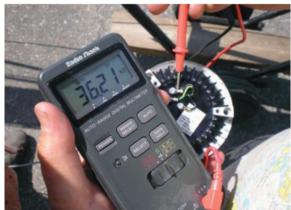
To check which cable went to the lamp, I used the multimeter to identify the circuit with the least resistance. In the same way, you can check whether a lightbulb works – if there's high resistance it's broken, if there's low resistance, it's not.
