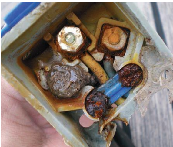
I discovered that the 240 V intake plug had at some point been short circuited – could have caused a nasty accident. The owners at the time must have been extremely lucky that a fire didn't break out as a result.
