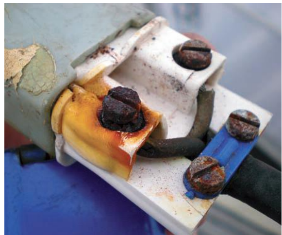
I discovered that the 240 V intake plug had at some point been short circuited – could have caused a nasty accident. The owners at the time must have been extremely lucky that a fire didn't break out as a result.
