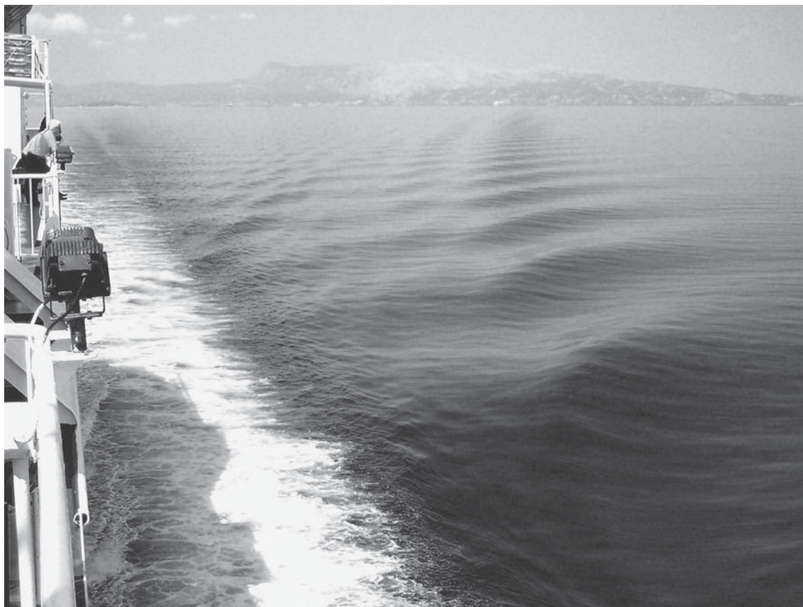
Figure 5.14 A ship wave pattern displaying some clearly defined rays at the outside of the Kelvin wedges from bow, shoulder, and stern.
