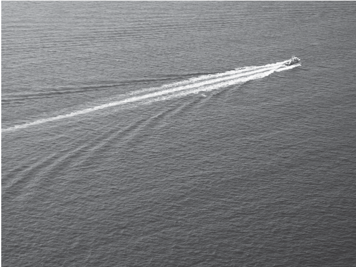
Figure 11.40 Wave pattern at high Froude number. Transverse waves nearly absent; no Kelvin angle visible; only sharply diverging waves.
