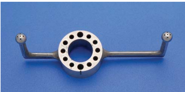
Figure 8.7 Rake for wake measurements containing two five-hole pitot tubes. (Photo: Sven Wessling. Courtesy of SSPA.)
