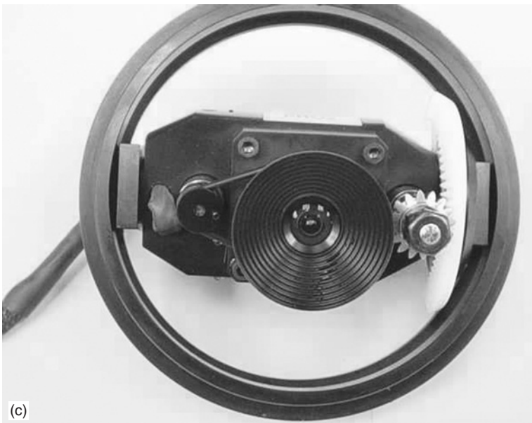
Figure 10.53 Typical arrangement – CCD camera system mounted to ring with tilting mechanism.
