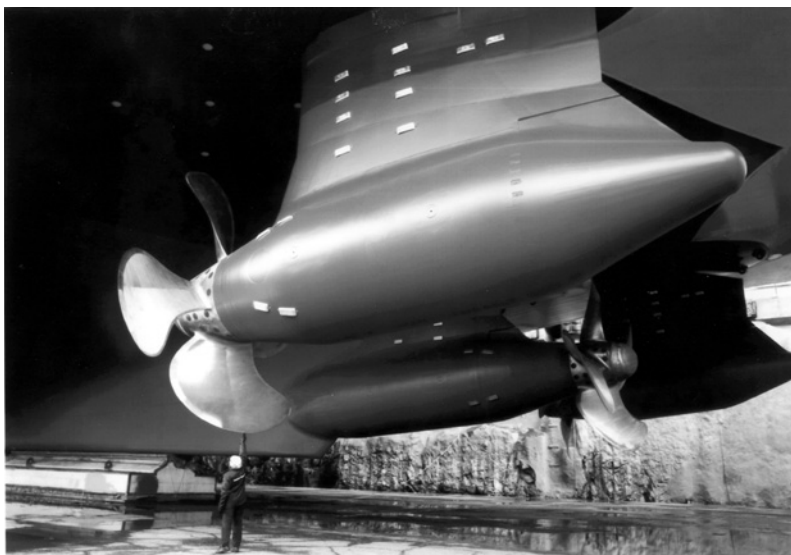
Figure 6.37 Three 14 000kW Azipod propulsors power Royal Caribbean Cruises' Voyager-class liners.
