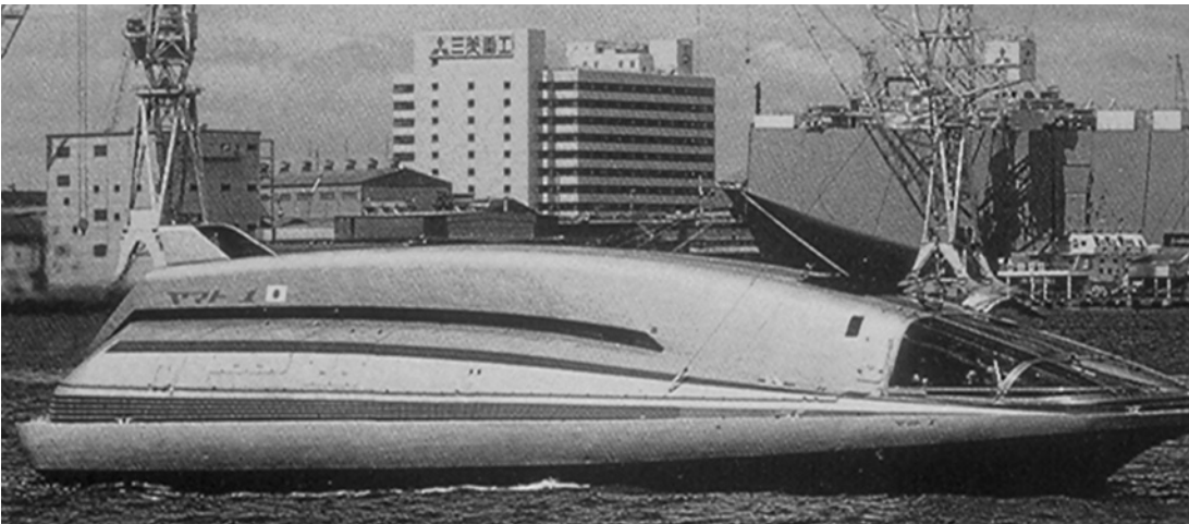
Figure 6.19 Yamato 1 : Experimental magnetohydrodynamic propulsion craft.
