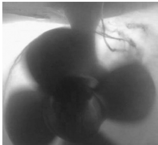
Figure 5.74 Example of a propeller–hull vortex emanating from a podded propulsion unit.
