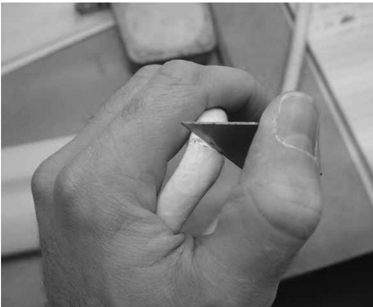
Figure 10.60 Slicing is conducted by peeling back the conductors of the tether.
