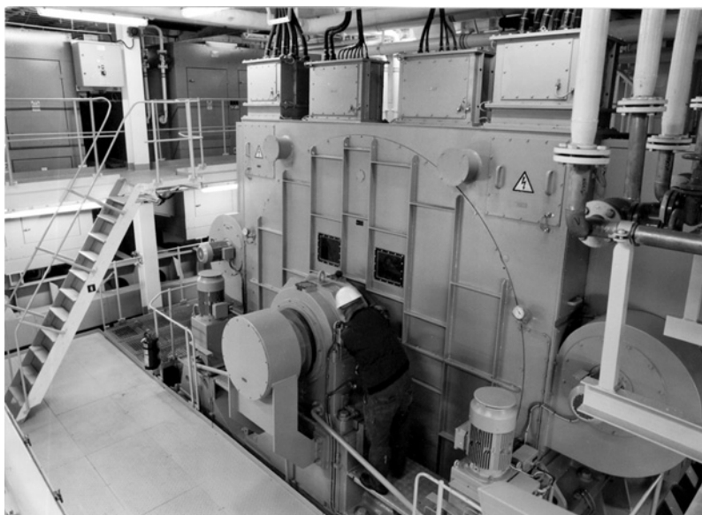
Figure 6.34 One of two 15 000kW STN Atlas propulsion motors installed on the cruise liner Costa Victoria .
