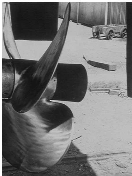
Figure 5.105 Truncated fairwater cone fitted to a high-speed patrol vessel.
