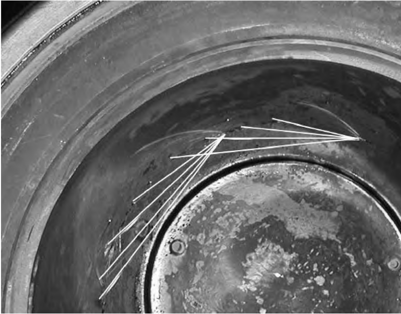
FIGURE 12.31 Arrangement of multiple lube oil jets in the cylinder liner, indicating the pattern of distribution with Wärtsilä's pulse jet lubricating system
