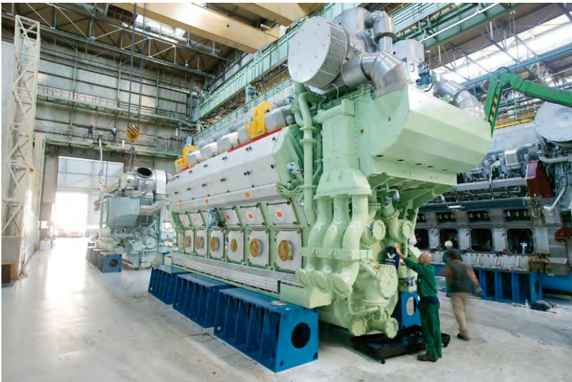
FIGURE 2.5 Wärtsilä 50DF engine in V12 cylinder form for LNG carrier propulsion
