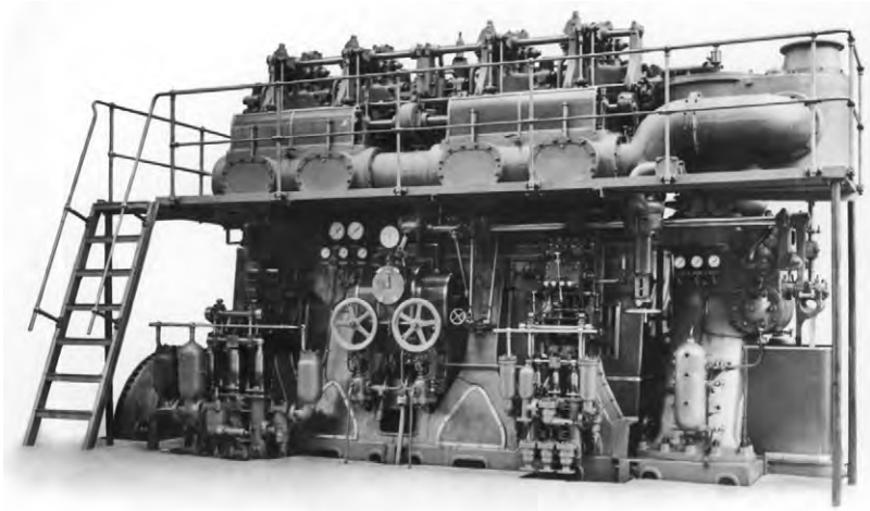
FIGURE I.5 One of the two Sulzer 4S47 engines installed in the Monte Penedo (1912)
