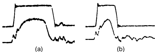
FIGURE 8.6 Fuel line pressure (lower line) and needle lift diagrams. (a) At high load. (b) At low load (Delphi Bryce)
