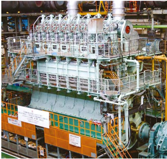
FIGURE 11.20 Mitsubishi's first production eco-engine on test in 2005, an eight-cylinder 60LSII model subsequently installed in a pure car/truck carrier
