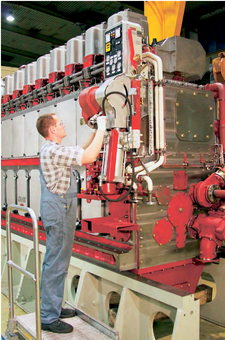
FIGURE 21.10 Mounting a flexible camshaft technology (FCT) unit on an MaK low emission engine
