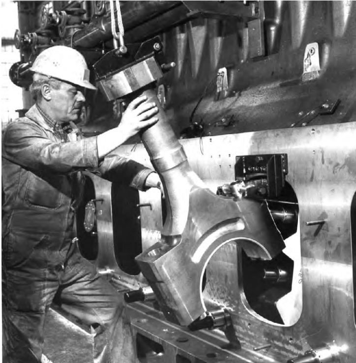
FIGURE 22.13 A low piston dismantling height is achieved by the joint in the upper part of the connecting rod shaft (L58/64, L48/60 and L40/54 engines)
