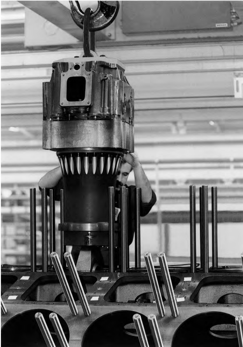
FIGURE 30.19 All the cylinder components of the MTU Series 8000 engine are combined in a functional module termed a ‘power unit’ for ease of withdrawal and replacement
