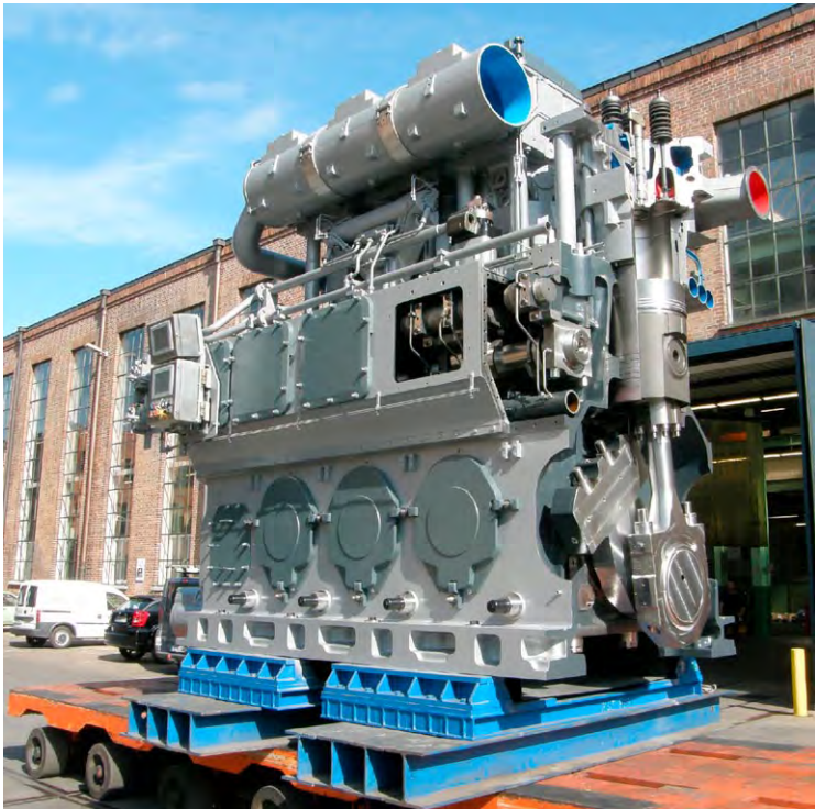
FIGURE 22.37 A 48/60CR engine with a cylinder unit exposed for an exhibition
