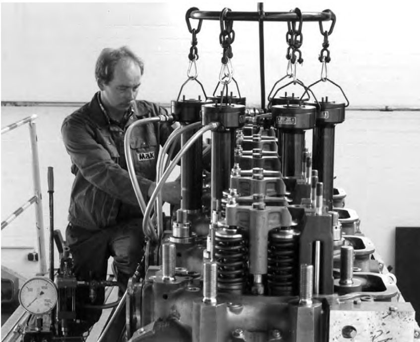
FIGURE 21.5 A six-element hydraulic tool is used to secure or release the M32 cylinder head nuts
