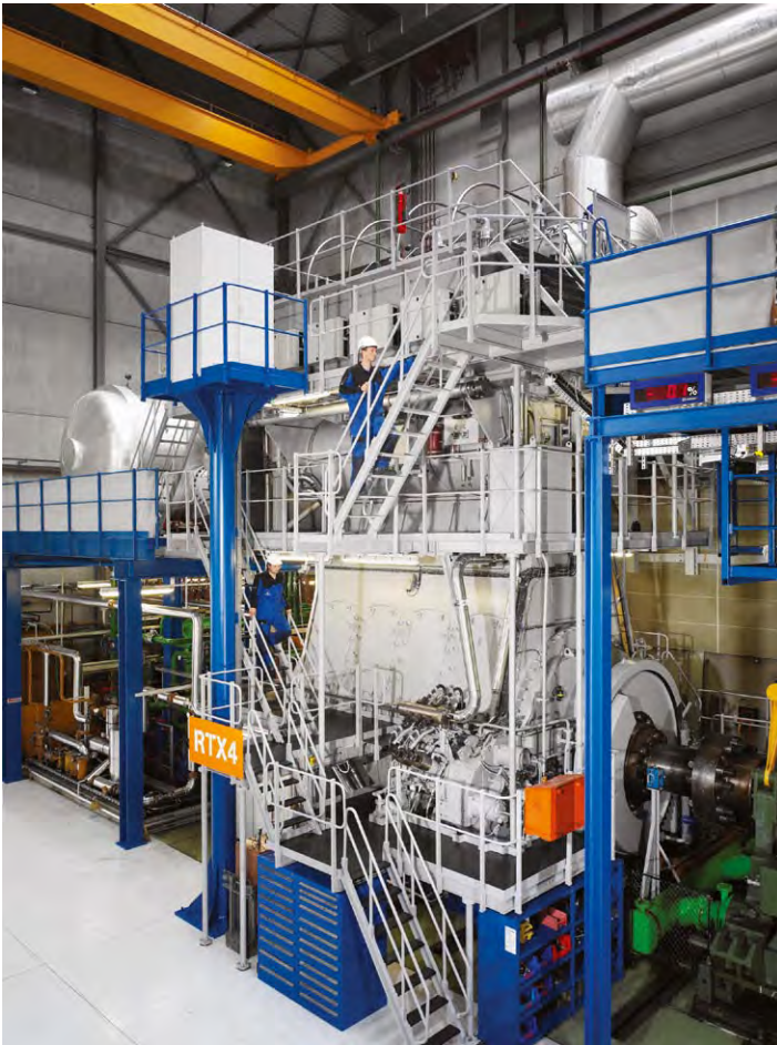
FIGURE 9.4 Wärtsilä's RTX-4 research engine in the Diesel Technology Centre at Winterthur in Switzerland
