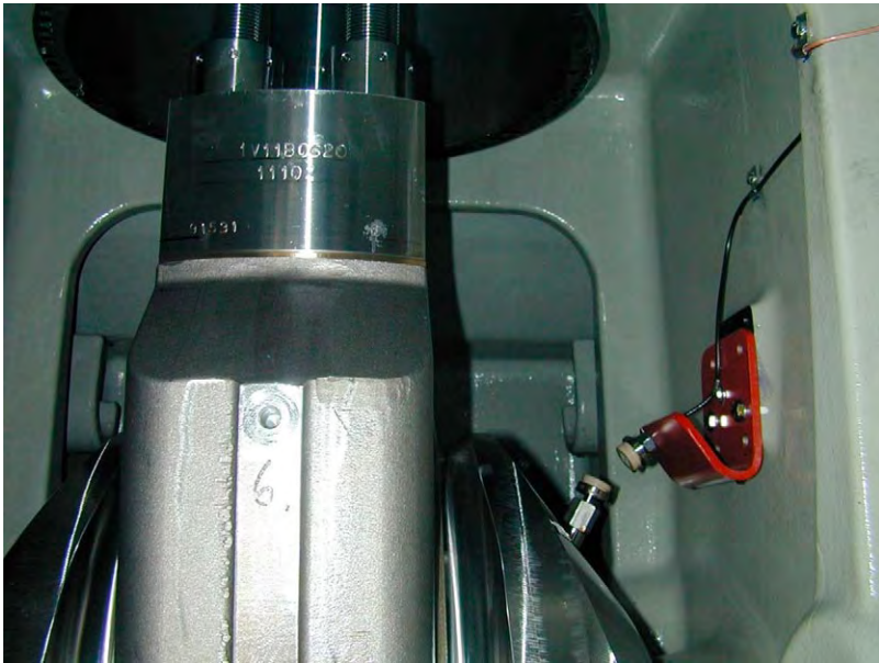
FIGURE 32.1 Continuous big end bearing temperature monitoring is performed by Kongsberg Maritime's Sentry system on Wärtsilä's 46F medium-speed engine
