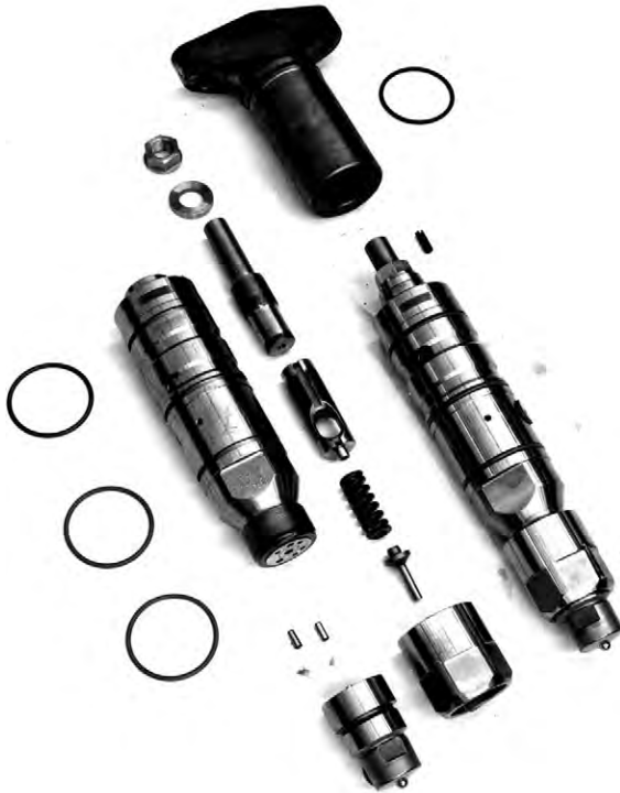
FIGURE 22.16 Main components of L58/64 engine fuel injection valve
