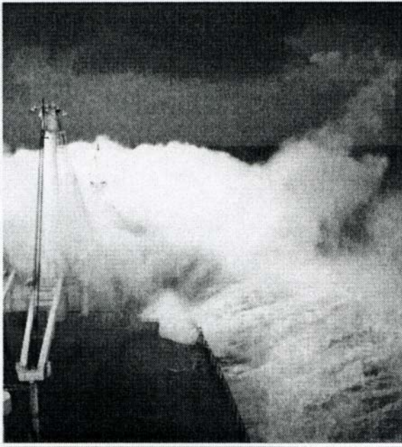
Figure 4.16 Bow flare slamming in heavy sea. Photograph by Lauritzen Group.
