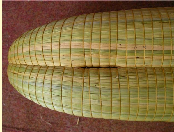
Fig. 10. an upturned model shows how the two hulls are joined together. The smaller inner cylinder is not seen.
