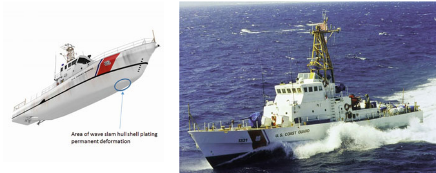
Fig. 12.12 Island-class patrol vessel with annotation for location of slam damage
