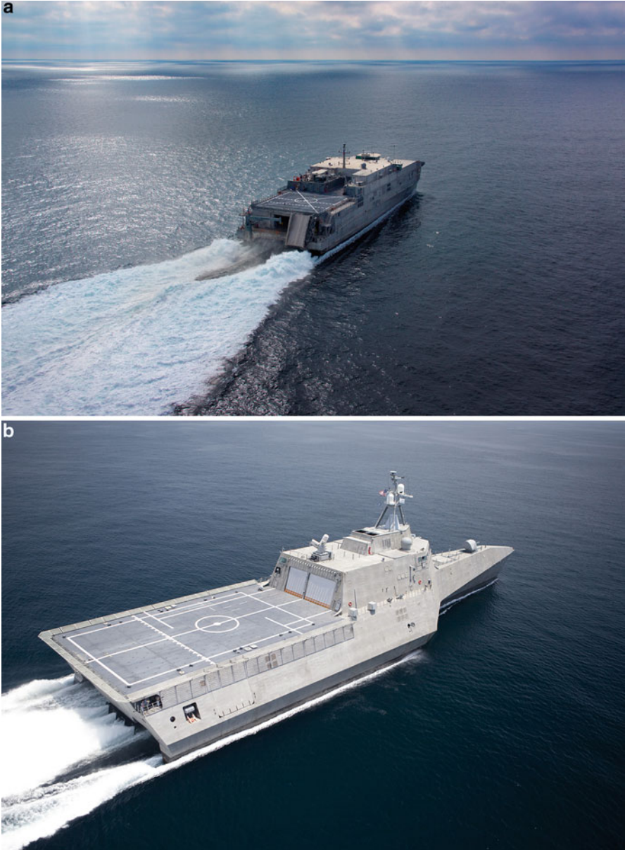
Fig. 1.15 (a) US military catamaran JHSV-1 on trials; (b) US military trimaran LCS-2 USS Independence at speed
