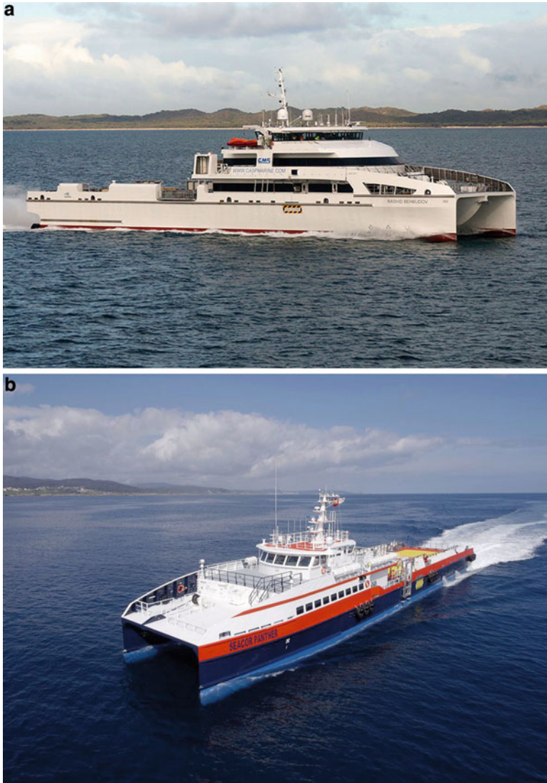
Fig. 10.14 SSTH high-speed supply vessels: (a) Caspian Marine Services 70-m vessel; (b) Seacor Marine 57-m vessel
