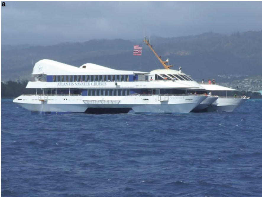
Fig. 9.11 SWATH Navatek 1 : (a) the vessel; (b) profile and general arrangement
