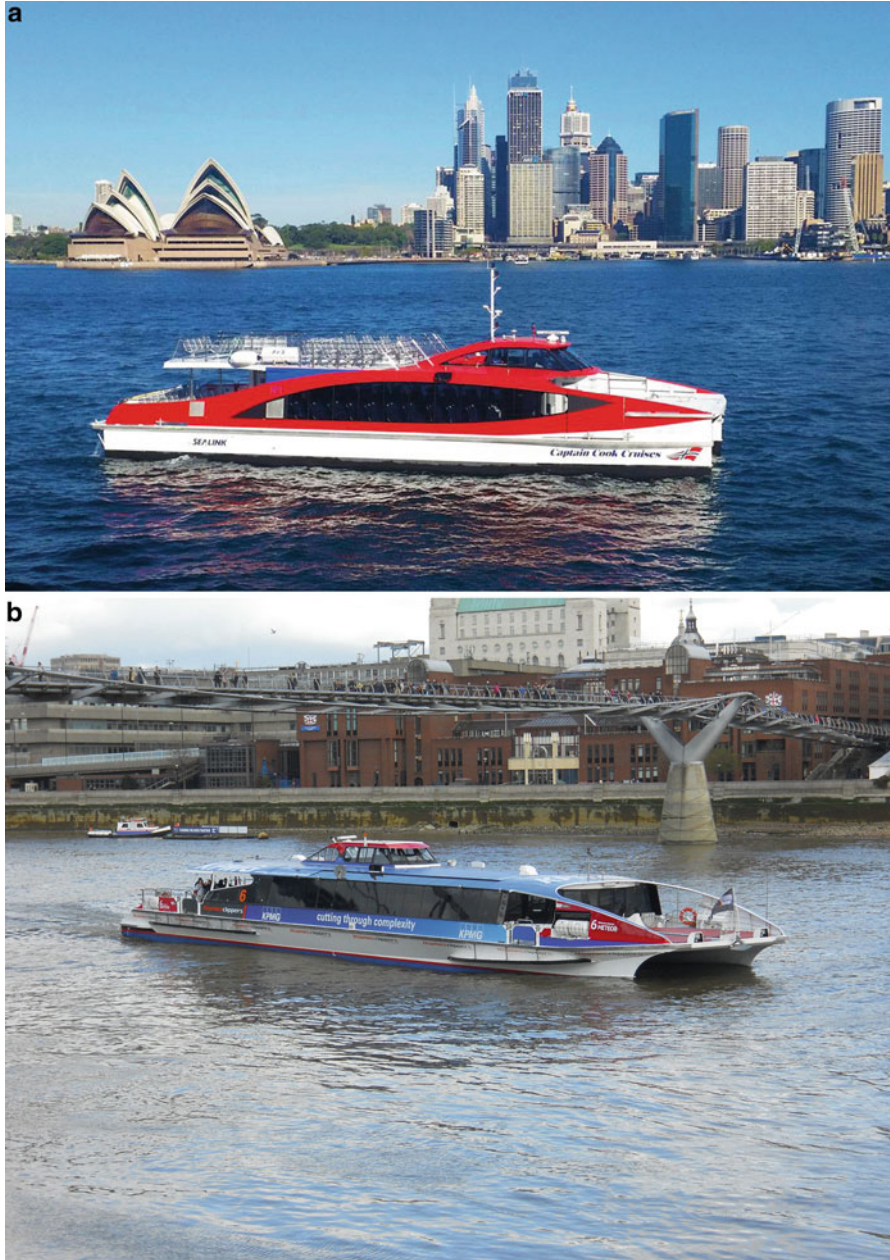
Fig. 13.13 (a) River bus with open upper deck (Sydney); (b) Thames River bus with closed passenger cabin on single-level deck
