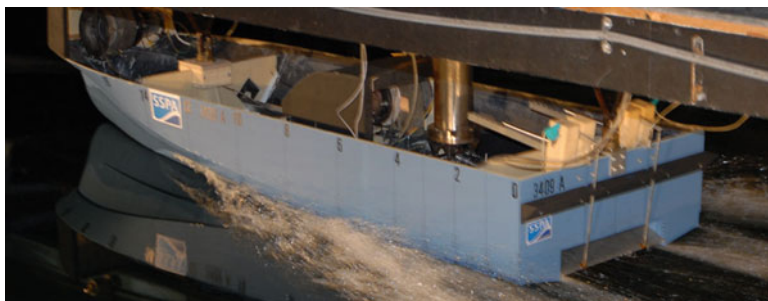
Fig. 10.37 ASV monohull model test showing flattened wake
