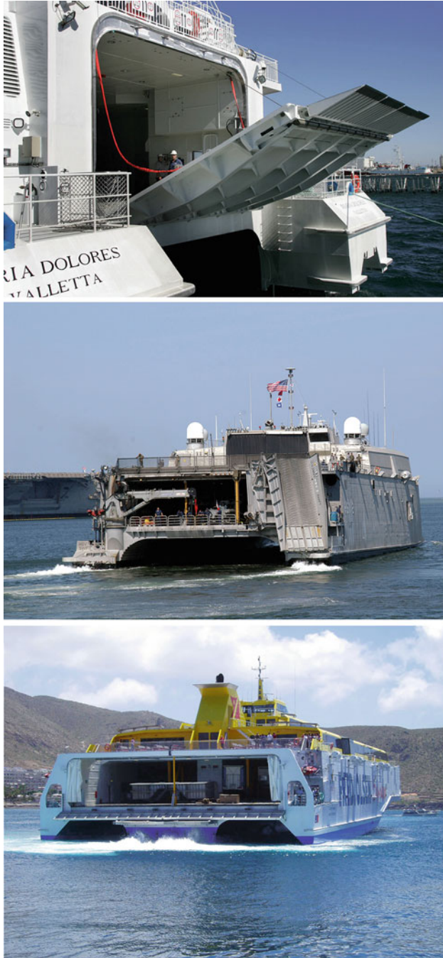
Fig. 13.10 (a) Austal ferry Maria Dolores stern ramp; (b) USN HSV2 rear ramp and crane; (c) trimaran Fred Olsen Benchijigua leaving Los Cristianos with stern simple closure and folding barrier
