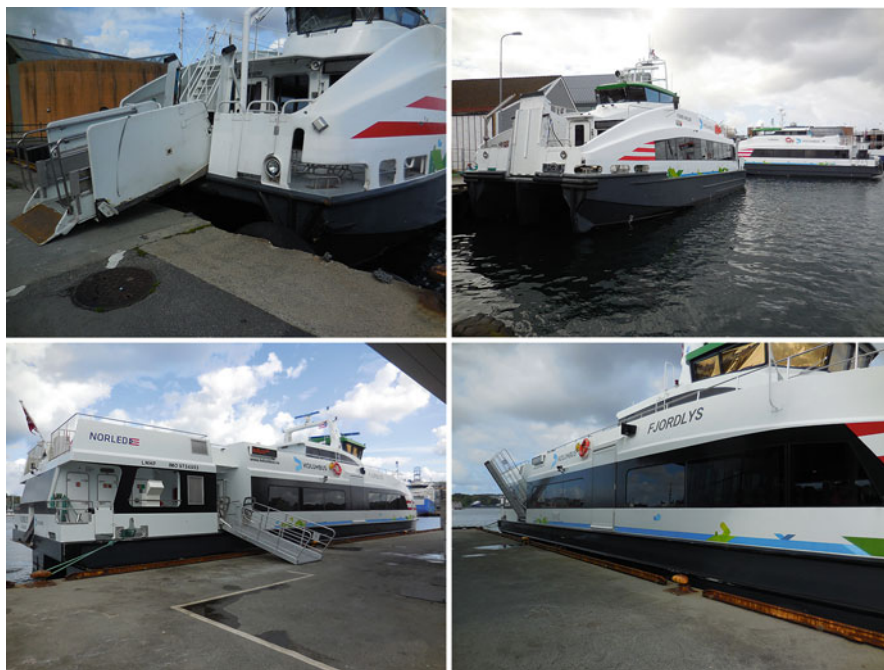
Fig. 13.9 Hydraulic ramp illustrations – showing bow ramp down and up, and rear ramp down and up
