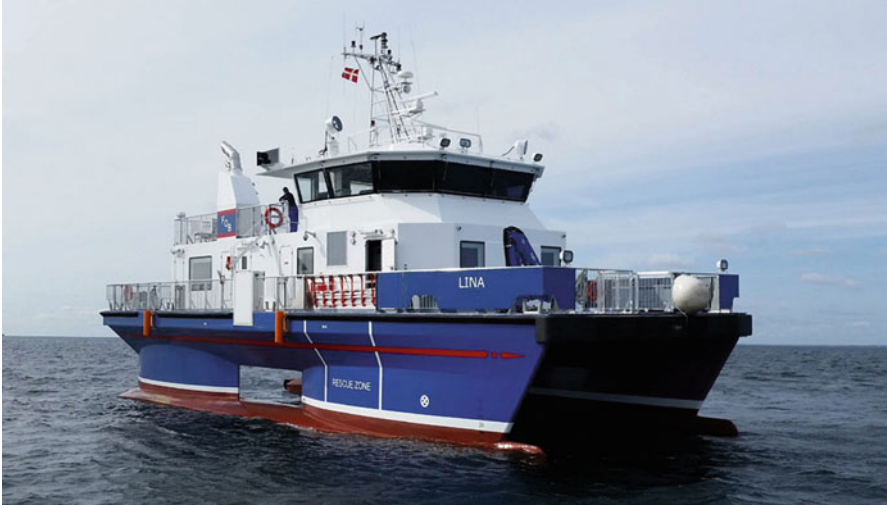
Fig. 9.36 Danish Yachts 27-m wind farm service SWATH vessel Lina operated by Odfjell
