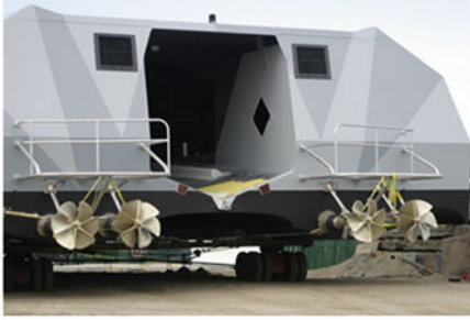
Twin disc installation in M80
