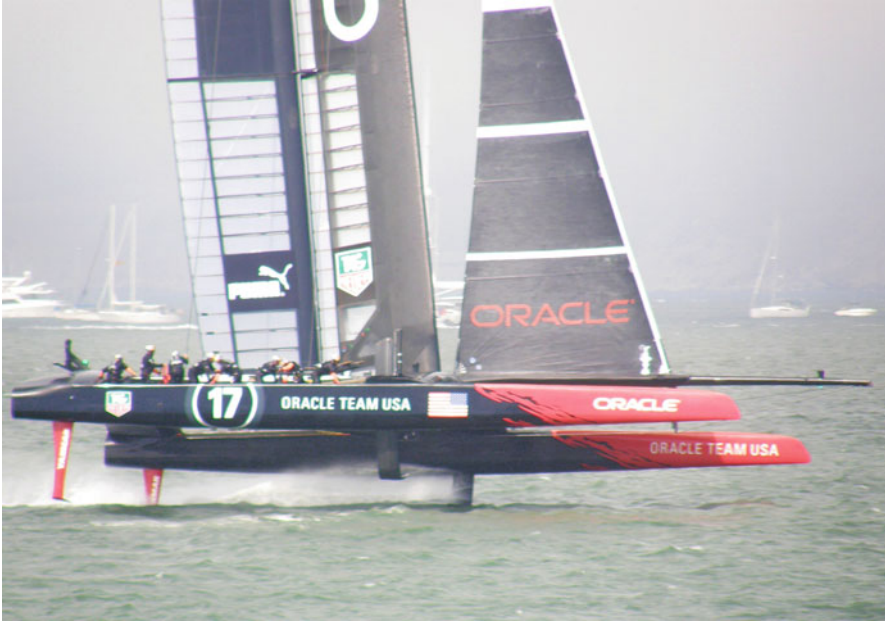
Fig. 1.3 Example of fast sailing catamaran on hydrofoils, America's Cup catamarans in 2013
