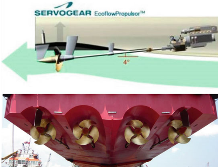
Fig. 11.9 (a) Servogear propeller flow diagram; (b) stern view of quadruple installation
