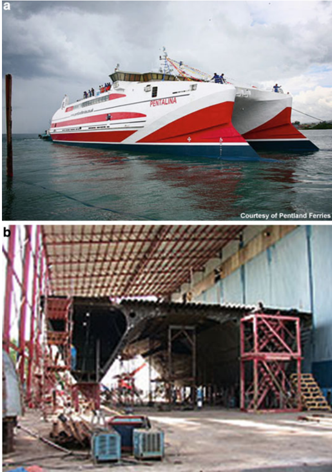
Fig. 9.32 FBM Pentalina RoRo ferry: (a) the vessel; (b) inset steel hull construction showing above water cross section
