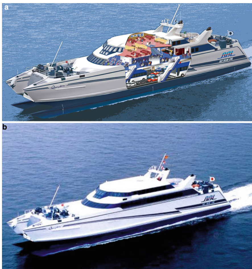
Fig. 10.12 Ocean Arrow SSTH ferry: (a) cutaway; (b) at speed; (c) general arrangement
