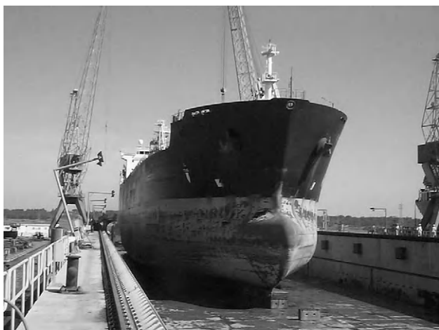
Figure 2.1 A vessel in dry dock sitting on keel blocks undergoing repairs
