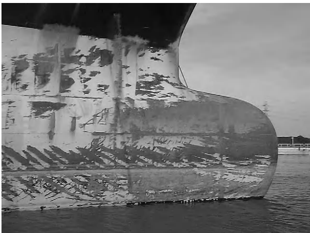
Figure 2.2 A vessel showing a high degree of paint damage
