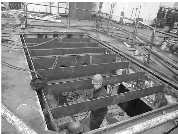
Figure 3.2 Repair of damage to ship's deck plating
