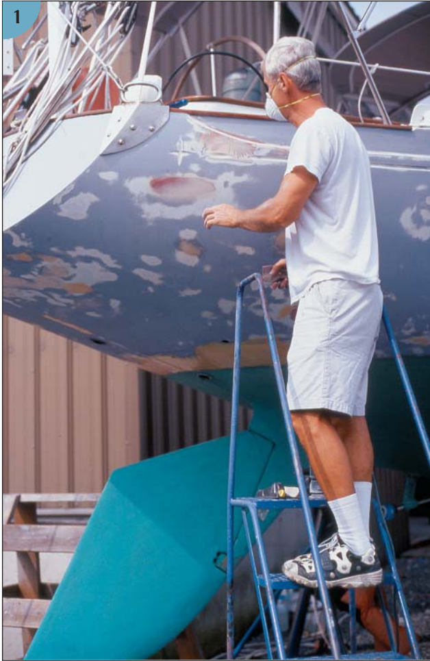
Preparing a hull before painting is critical. This hull is being faired with thickened epoxy prior to sanding and priming (1, 2).
