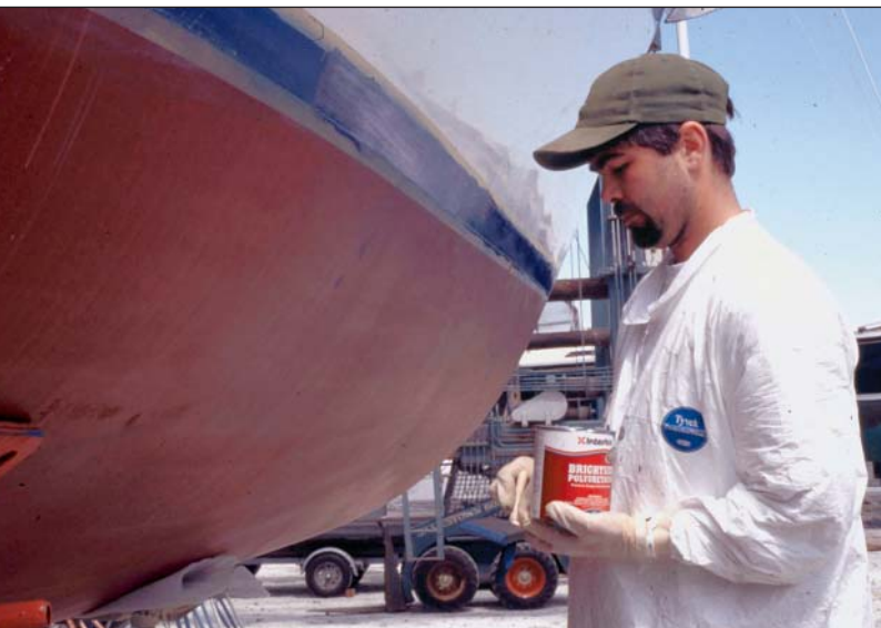
Painting a boottop with Brightside, a single-part modified urethane paint. Notice how the top and bottom of the stripe are masked off. Nothing beats a two-part polyurethane for a topside paint, but two-part paints are hard to mix properly in the small quantities required for jobs such as a boottop. Single-part paints are convenient for such jobs.
