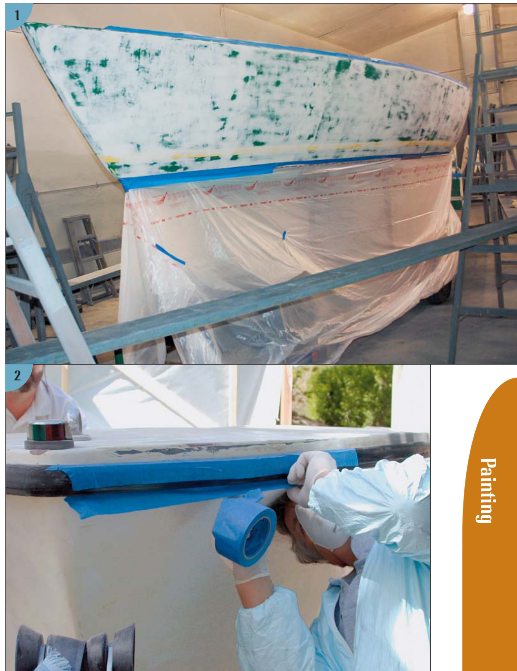
(1) The primed hull of the J/24 has been sanded and the boottop has been masked. (2) Here a rubrail is being masked off on a different boat.
