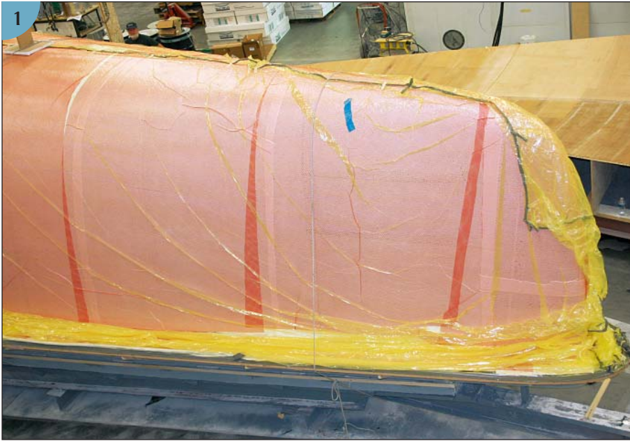
(1) The bow of a yacht under a vacuum bag. (2) This WEST System vacuum-bagging kit contains a venturi vacuum generator, release fabric, bleeder cloth, vacuum membrane, vacuum gauge, tubing, and manual. It costs about $200 (2009). (3) This close-up shows the resin (small dots) coming through the bleeder cloth under the plastic vacuum bag cover.
