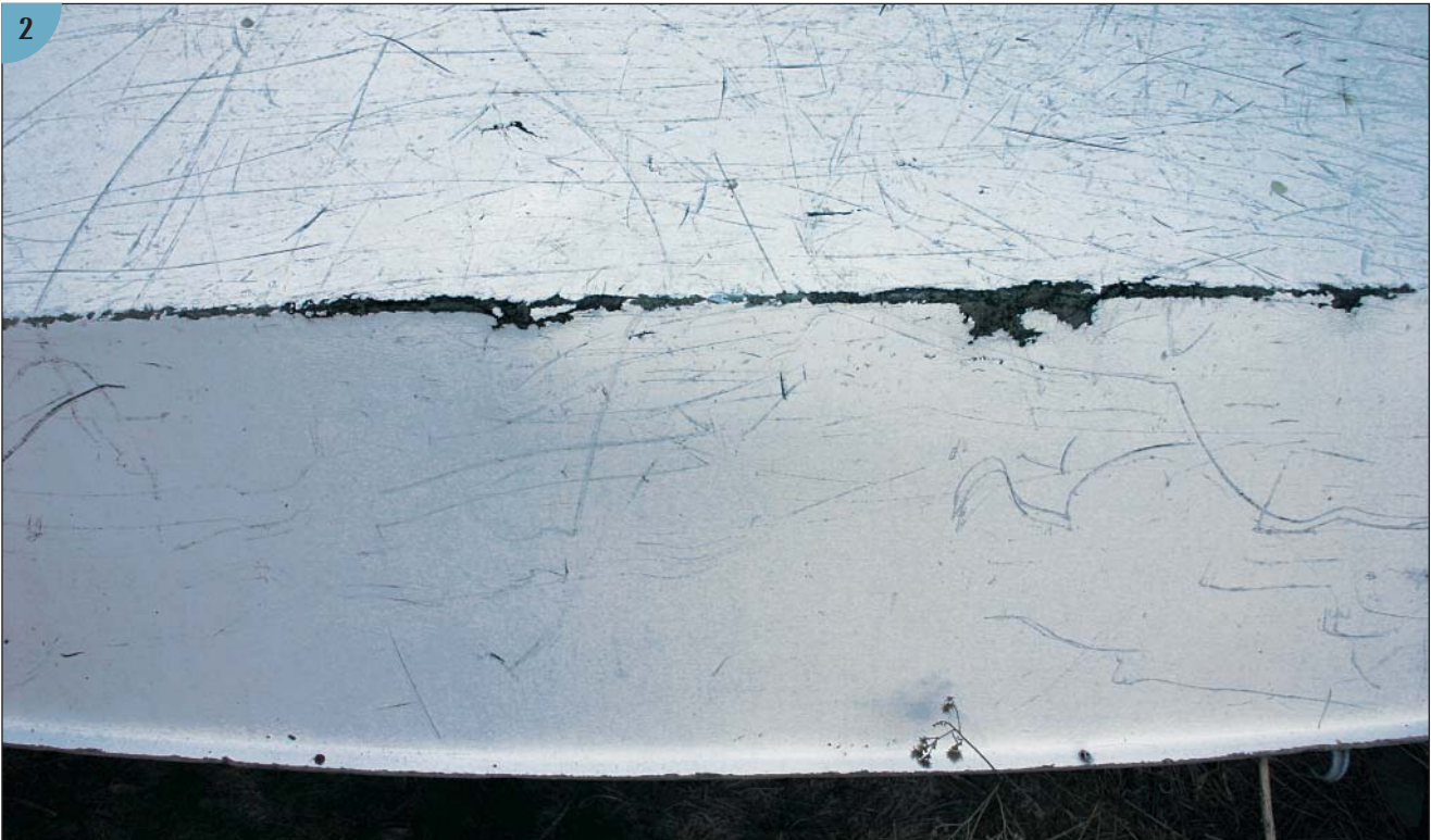
(2) This photo shows impact damage to the chine. This is another small dinghy that has suffered from being dragged either on board or over a beach or dock. The chine is torn
