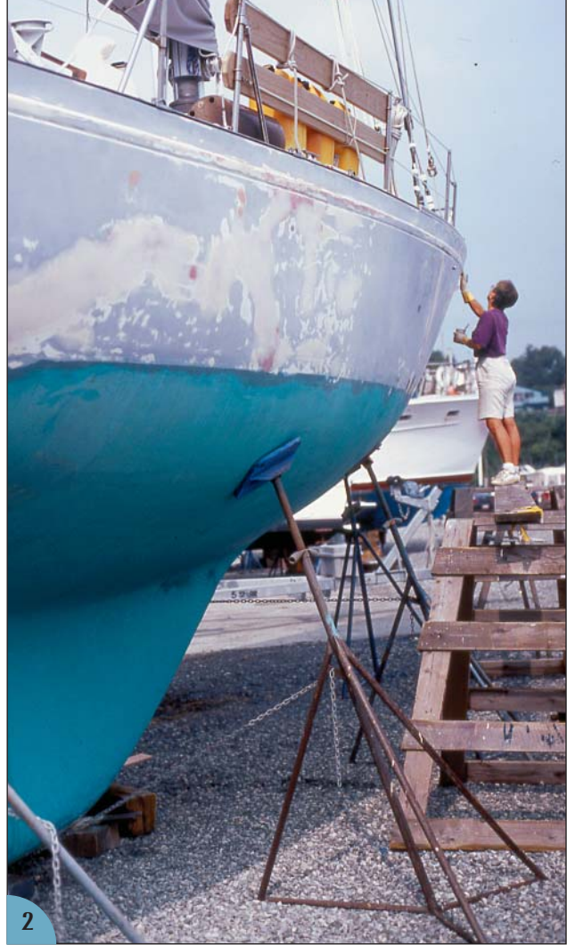
Preparing a hull before painting is critical. This hull is being faired with thickened epoxy prior to sanding and priming (1, 2).
