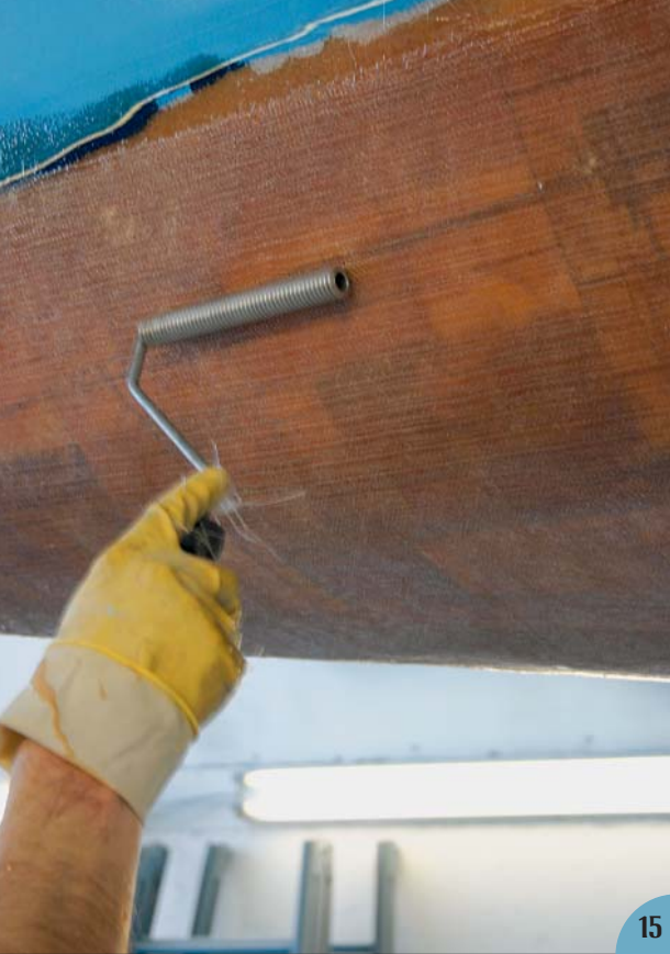
(15) More layers followed, and they rolled each one carefully to eliminate air pockets.
