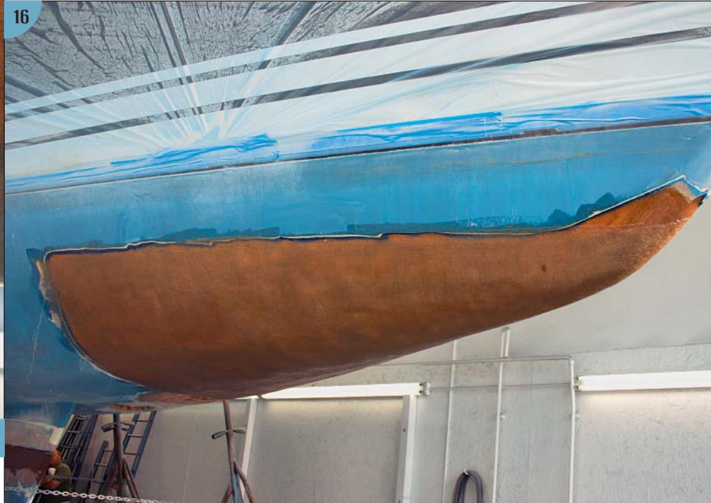
(16) After curing at 80°F, the repair was ready for fairing and finishing.
