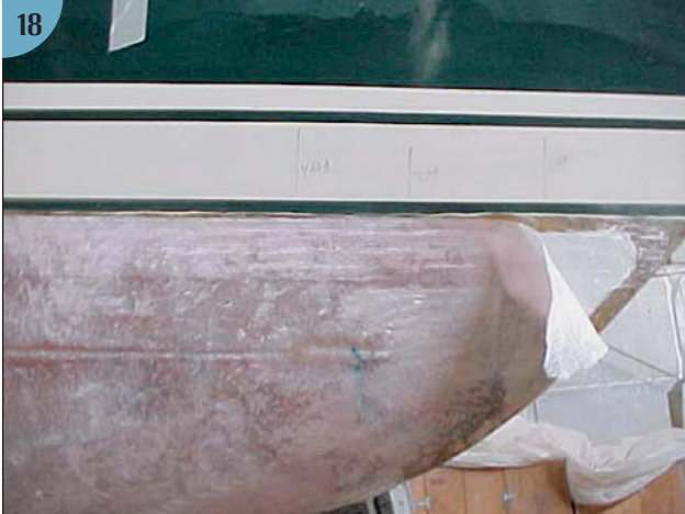
(20) The exterior of the hull underbody is given a barrier coat of Interprotect epoxy resin to provide an additional guard against water penetration.
