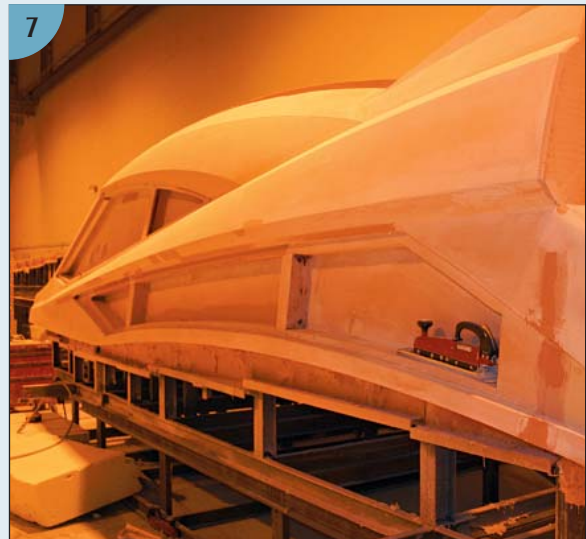
(5, 6, 7) The router at the D. L. Blount Associates production facility in Norfolk, Virginia, runs for two shifts a day to keep up with the workload. These parts for a large fiberglass yacht show some of the complex shapes that can be molded with a computer-controlled router. Note how the steps in photo 6 are cut into the bulkhead. (Courtesy D. L. Blount Associates)
