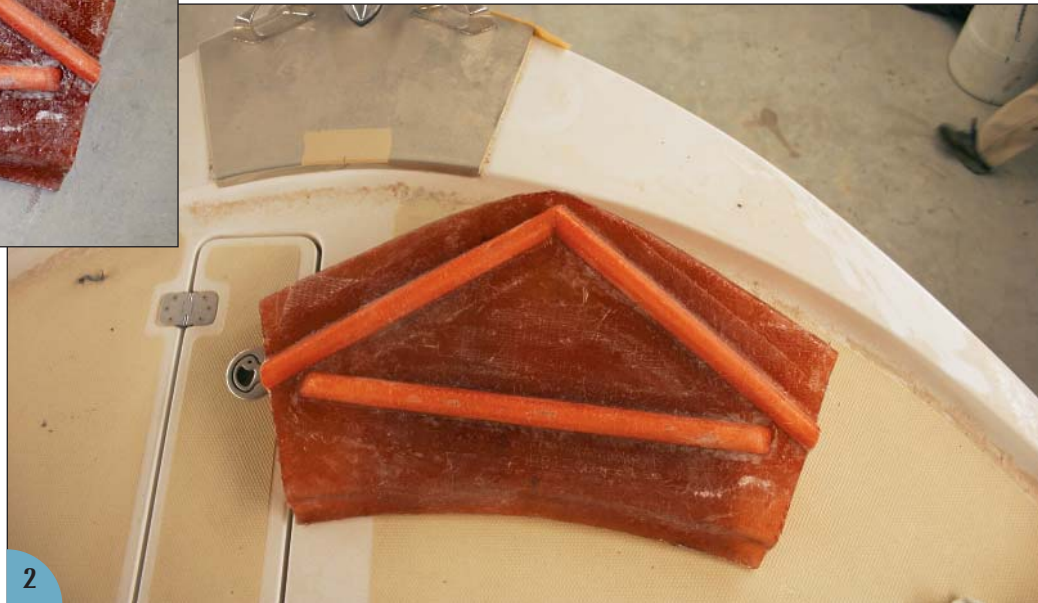
(1) This splash is a bow template used by the builder of a production boat to locate the bolt layout for the stemhead. (2) The template next to the stemhead that was prepared from it.
