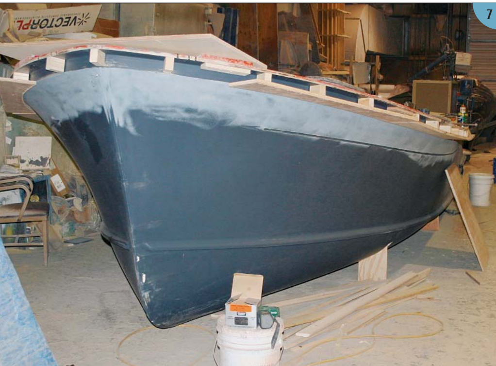
(7) The hull plug after it has been turned upright and removed from the mold. Here the flange along the top is being worked on to ensure a tight hull/deck joint.
