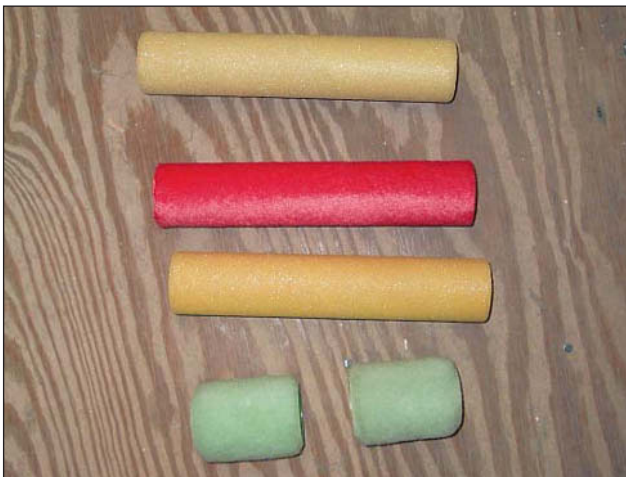
Various rollers used to apply topcoats. The foam rollers shown here are designed for marine paints and will not fall apart. The nylon rollers (pale green) are best used for nonskid.
