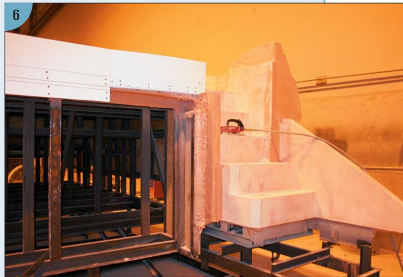
(4) Here a router bit is cutting foam. To the right you can see a stream of chips coming off the bit.
