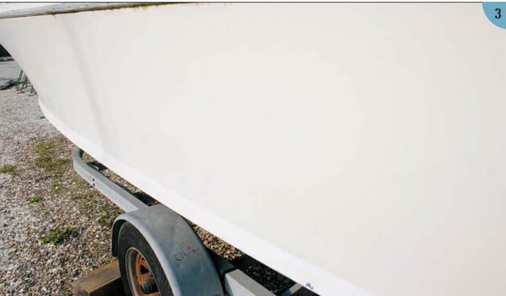
(3) This gelcoat looks as if it hasn't been polished or waxed in years. If the owner continues to neglect it, it could end up looking like the gelcoat in the preceding photos. Restoring it will require aggressive compounding with an abrasive rubbing compound (see the buffing compound sidebar on page 72), followed by waxing and polishing.
