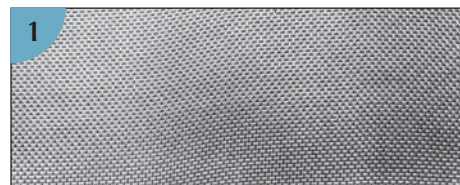
(1) Fiberglass cloth. (Reprinted with permission from The Modern Cruising Sailboat by Charles J. Doane)
