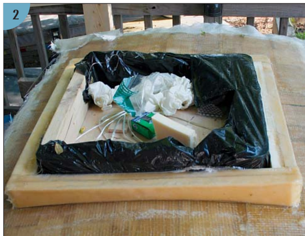
balsa core. (We butted this deck core against the wooden frame you see in photo 1.) On top of the balsa we laminated an outer skin of 1\frac{1}{2} -ounce CSM followed by 24-ounce woven roving and another layer of 1\frac{1}{2} -ounce CSM. We then erected the foam core for the new hatch boss against the outside of the wooden frame, removed the frame, and laminated two layers of 6-ounce cloth over the entire part, encapsulating the foam boss core.
