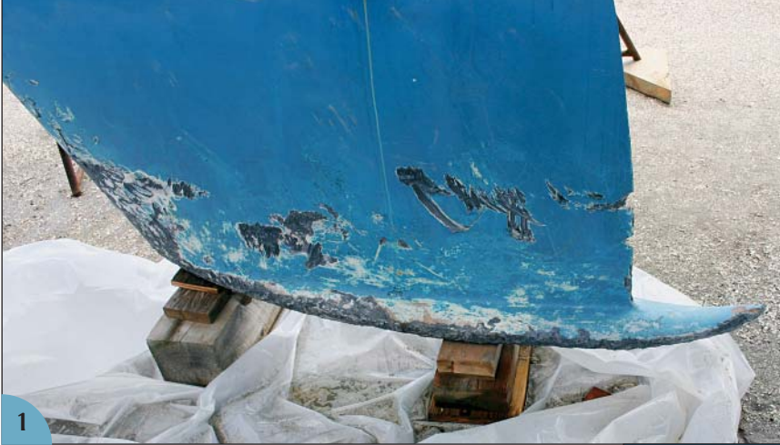
(1, 2) Damage to the keel on this sailboat shows that it has gone aground heavily and spent some time on the rocks. Damage this extensive suggests that the entire interior needs to be checked carefully. (The repairs to this boat are discussed in Chapter 7.)
