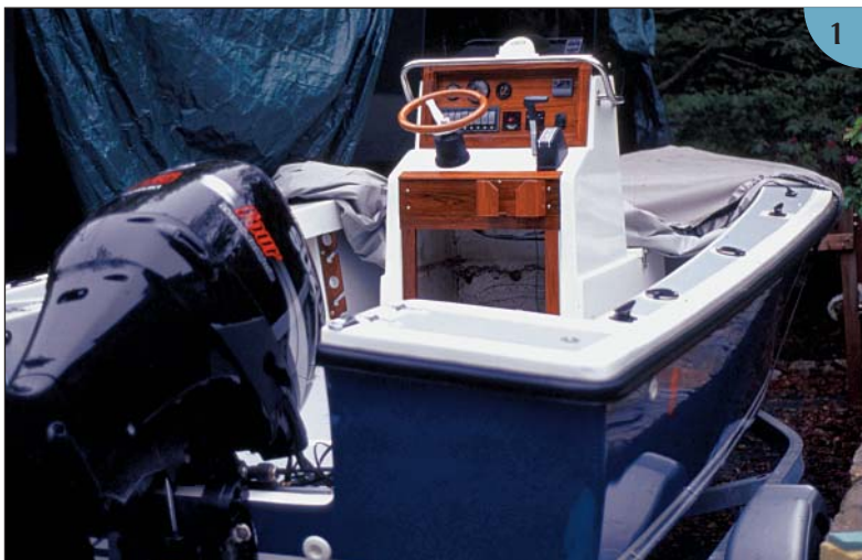
(1) The cutout transom in my project boat. This outboard has a 20-inch shaft. When the boat is coming off a plane or backing down, water can flood the cockpit. I first raised the engine to its maximum position and measured carefully around it. (2) This photo was shot when I had fitted but not yet trimmed the well guard.
