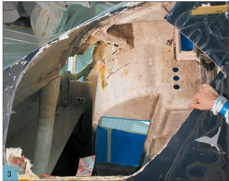
(1) The grounding damage on this boat runs along the starboard side of the hull, but the major damage occurred near the transom where the boat lay on the rocks. The hull there was completely stove in, and the laminate had to be cut away completely. (2) The rudder was also extensively damaged, and the stock was bent. (3) The cutaway portion of the hull shows how much of it was damaged. The yard had to cut deep into the transom and remove part of the deck.
