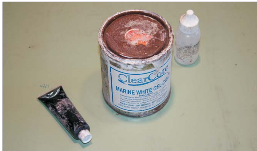
You can purchase small cans of resin (in this case, gelcoat resin) suitable for most small repair jobs at your local chandlery or marine products distributor. Be sure to measure out the resin carefully in order to get a good, strong bond. The bottle to the right rear of this photo contains MEKP, while the tube in the lower left contains a black coloring agent. It only took one or two drips of the black pigment to turn white gelcoat from this can the right shade of gray to repair the 420 shown in Chapter 4.
