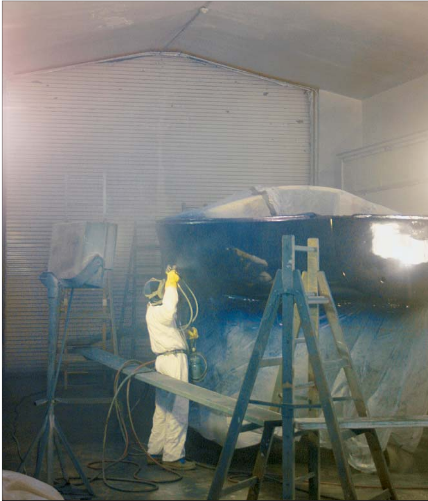
Spraying a topcoat in a dedicated enclosed space called a spray booth. Even though the spray booth fans are running full tilt, there is still enough overspray to cloud the booth. The photographer was wearing a respirator when taking this picture, and you should not go into a spray booth without one.
