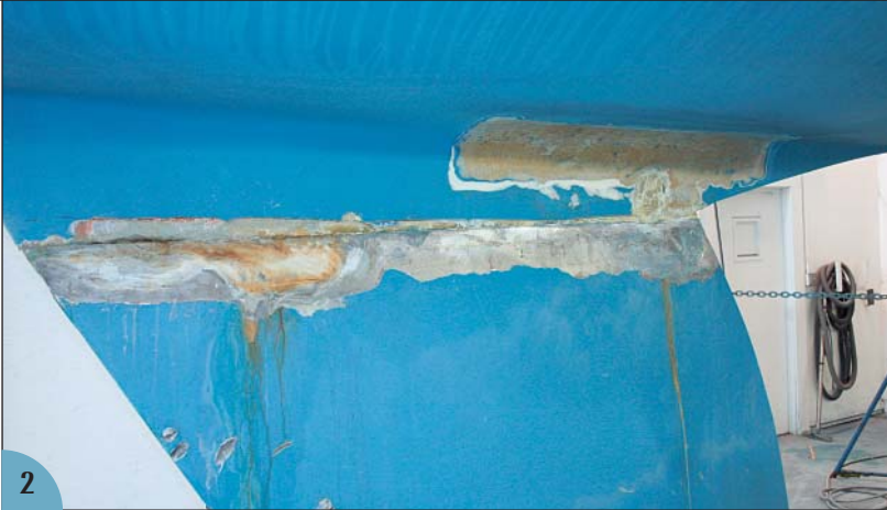
(1, 2) Damage to the keel on this sailboat shows that it has gone aground heavily and spent some time on the rocks. Damage this extensive suggests that the entire interior needs to be checked carefully. (The repairs to this boat are discussed in Chapter 7.)
