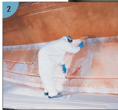
(1) Spraying gelcoat into a mold to form the polished exterior surface of a hull. (2) Rolling resin over fiberglass. (Courtesy Ranger Boats)
