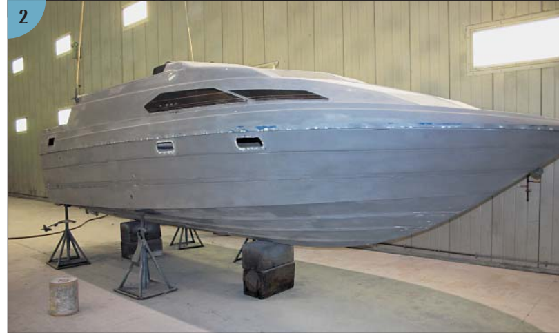
(1) Sanding a primed hull and deck to prepare them for the topcoat. (2) A boat primed and ready for a topcoat.
