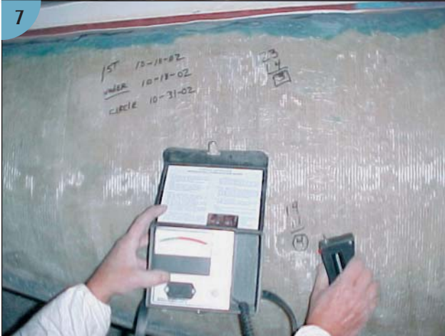
(4) A hull being peeled, exposing blister craters. (5) The laminate has been fully peeled, but moisture is still present in the cored hull. (6) A second peel exposes wet core, which will have to be replaced. (7) Moisture levels in the core are carefully measured to ensure that the core is dry enough for a new outer skin. (8) The peeling of this keel has exposed areas of delamination. (9) This hull has been peeled to its core, which is in very poor condition and will need to be replaced. After being peeled, a hull needs to dry out. (10) Powerful heaters like this infrared one help the process along.
