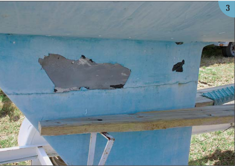
(3) The severe cracking between the hull sump and the keel on this sailboat suggests that it may have gone aground. The boat should be checked for interior damage.
