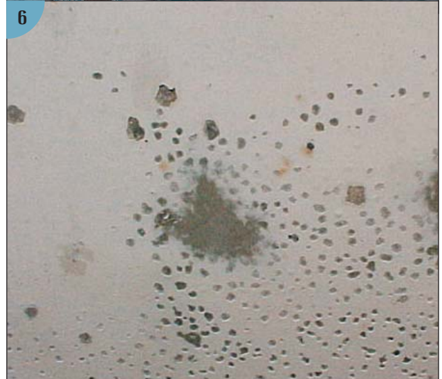
(1) These representative examples of osmotic blistering caused by water penetration into the outer laminate of a hull include blisters after a hull has been peeled, water penetration via blisters into a peeled hull's core (2), which will need to be dried out or replaced, and other examples of blisters (3, 4, 5, 6). (All images courtesy Jamestown Boat Yard.)
