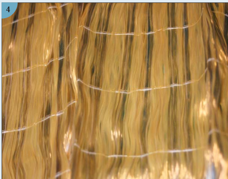
(4) Unidirectional Kevlar combined with S glass makes this high-strength, impact-absorbent material. The Kevlar is light brown, and the S glass is silvery. The thin lines crossing the material are the glue lines that hold the scrim together.
