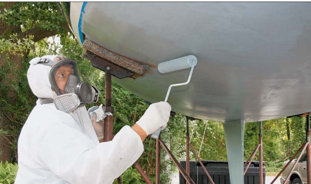
Rolling Interprotect onto a hull. Interprotect is an epoxy resin that helps keep water from infiltrating into the fiberglass hull skin through the gelcoat.
