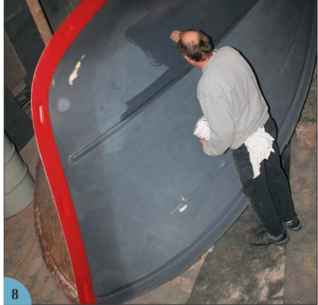
(8) This is a two-part mold because of the boat's tumblehome. The mold has been split apart, and the boat will be craned out ready to be fitted out with the cockpit and interior. A bow-to-stern flange is set up along the plug's fore-and-aft centerline to divide the two halves of what will be a two-part hull mold. This permits the two mold halves to be pulled sideways off the plug (rather than having to be lifted vertically off the plug, as would need to be done with a one-part mold) and then be mated along the flange. This is useful when overhead space is limited, and also when a boat has tumblehome in its topsides (as this boat does in its stern sections), which would prevent the hull from being removed from a single-piece mold.
