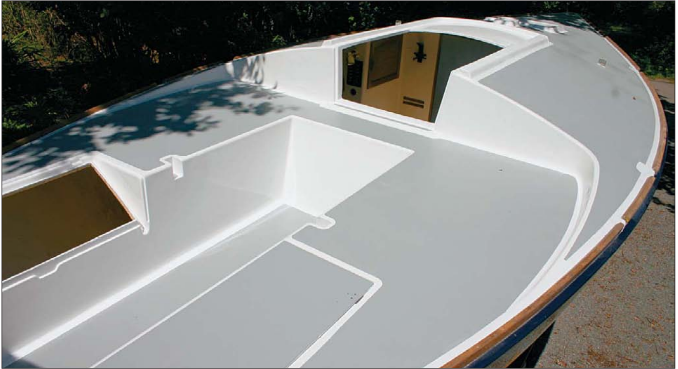
The deck of my son's J/24 freshly painted with Interlux's Interdeck gray nonskid and white Perfection. A good paint job can increase the appearance and value of your boat far beyond anything else you can do.
