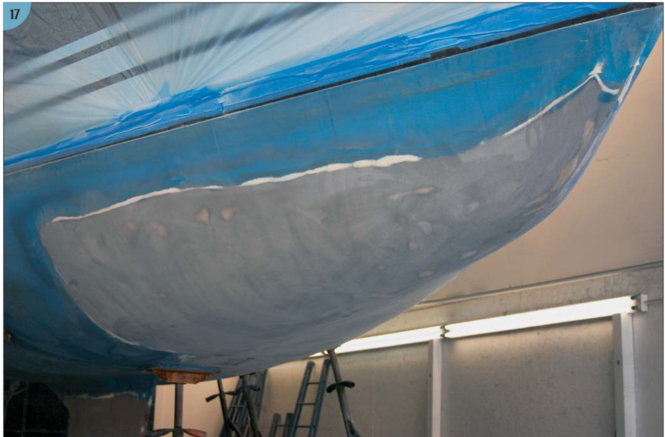
(17) They smoothed the hull with fairing compound, which shows as a gray layer.
