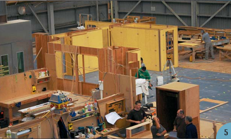
(3, 4) Furniture for a yacht being built off-site. These joinery pieces will be carried to the vessel and installed after the boat is built. (5) The SMI plant in New Zealand
