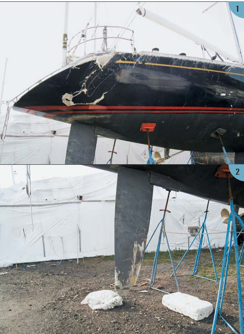
(1) The grounding damage on this boat runs along the starboard side of the hull, but the major damage occurred near the transom where the boat lay on the rocks. The hull there was completely stove in, and the laminate had to be cut away completely. (2) The rudder was also extensively damaged, and the stock was bent. (3) The cutaway portion of the hull shows how much of it was damaged. The yard had to cut deep into the transom and remove part of the deck.
