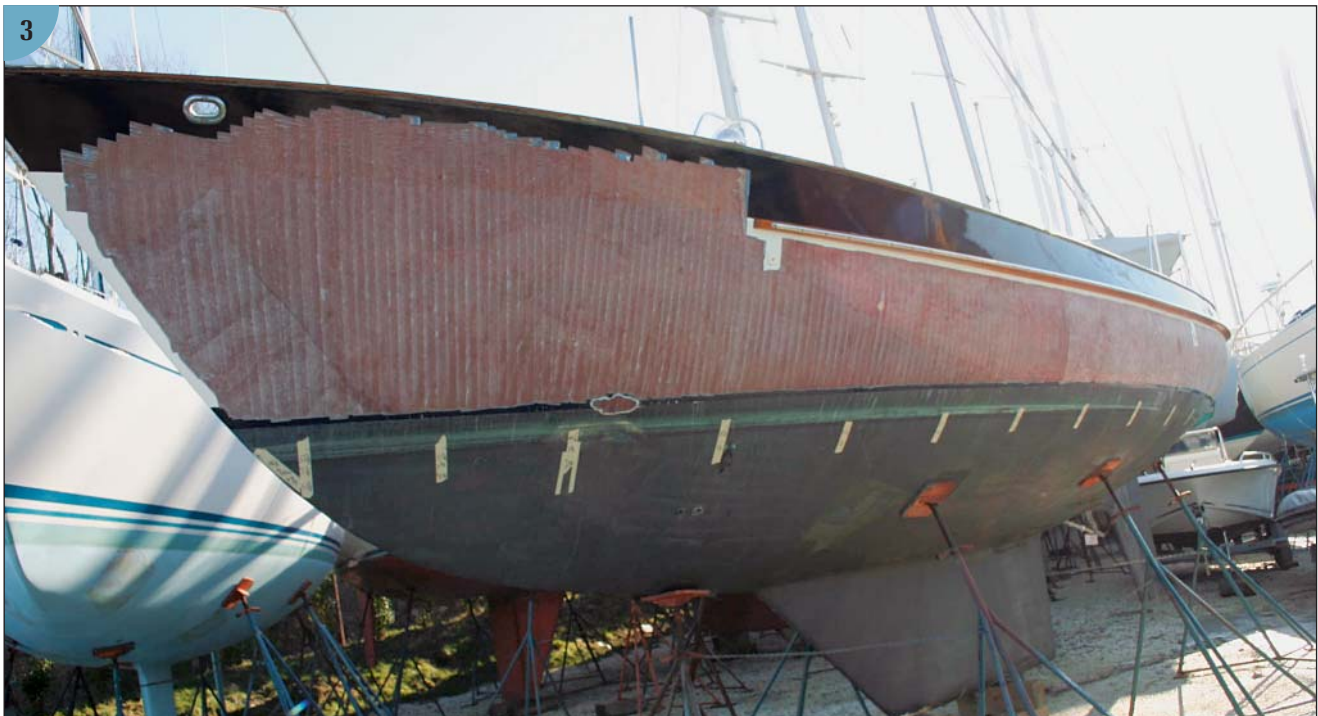
(1, 2) A blistered Valiant 40 hull after a professional peeling. (3) The extent of the work on the topsides.
