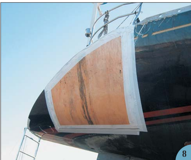
(8) After cutting back the hull and grinding scarfs into the edges of the opening, the yard fastened several layers of thin plywood over the hole to allow new laminate to be glassed up from the inside. Laminating that repair in the confined space between the hull side and the cockpit tub must have been an unpleasant job.
