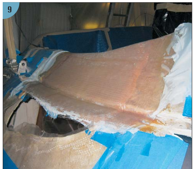
(9) The cutaway portion of the transom had to be laid up again using the same technique as on the hull side, leaving this small hole (between the top of the swept-back transom and the aft rim of the cockpit coaming above it) to be finished.
