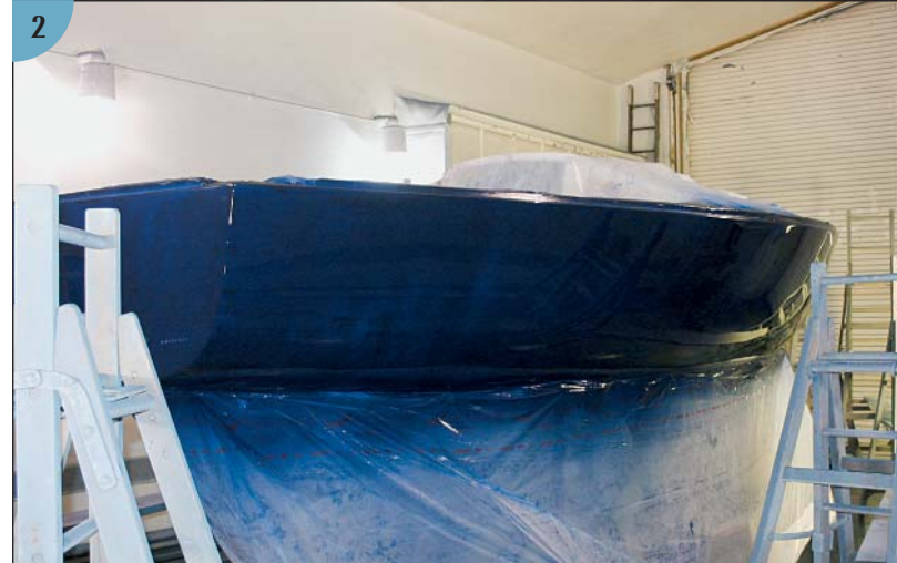
(1) The hull after being sprayed with its first coat of Perfection. Note the high-gloss finish and the shine of the Perfection paint. (2) The finished hull.
