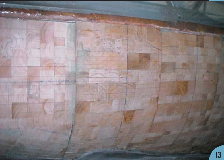
(11, 12, 13) Core replacement can be limited or more general, depending on the need. (14) Vacuum bagging a replacement core in place to eliminate voids. With a hand layup you can expect about 15% to 20% voids in a laminate, but vacuum bagging can reduce the void content to under 2%, which reduces the potential for renewed hull blistering down the road. (15) Testing the vacuum sealing bag for leaks.
