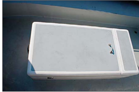
The nonskid gelcoat on this engine box was applied with a foam roller over the existing gelcoat. Often the gelcoat is pigmented to make it stand out from the white gelcoat around its perimeter.
