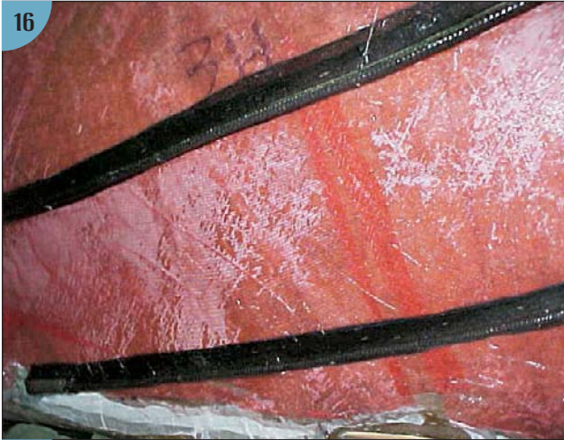
(16) The vacuum bag in place with the vacuum lines running along the hull underbody. With the new core in place, the hull laminate is laid up using woven roving and CSM. (17) A worker sprays CSM on the core. (18) The outer skin laminate is laid up over the chopped strand and will then be vacuum bagged. (19) A worker sands the newly laminated hull.
