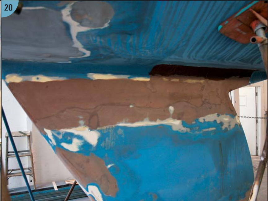
(20) They also refaired the top of the keel to its original contours, and refilled and refaired the hull-to-keel joint.
