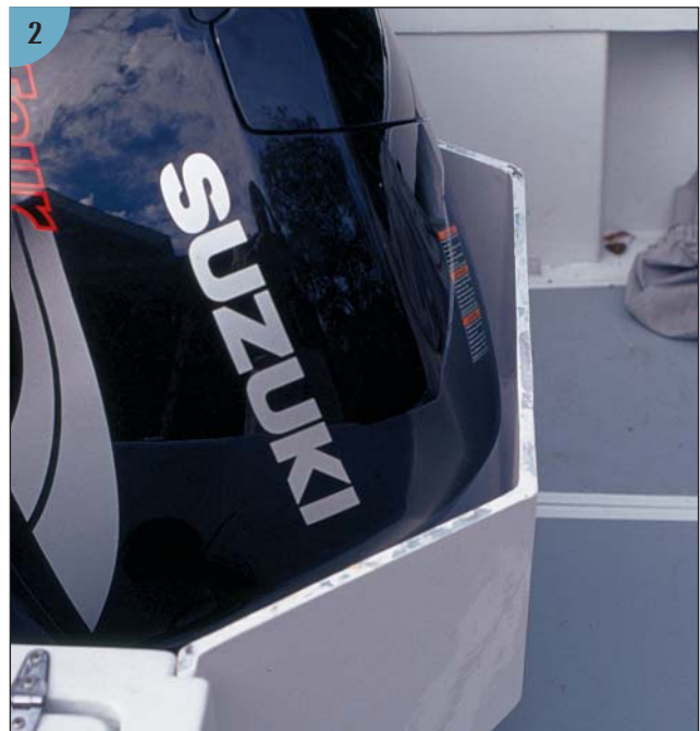
(1) The cutout transom in my project boat. This outboard has a 20-inch shaft. When the boat is coming off a plane or backing down, water can flood the cockpit. I first raised the engine to its maximum position and measured carefully around it. (2) This photo was shot when I had fitted but not yet trimmed the well guard.
