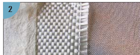
(2) From left, mat, woven roving, and cloth. (Reprinted with permission from Maintain and Improve Your Powerboat by Paul Esterle)
