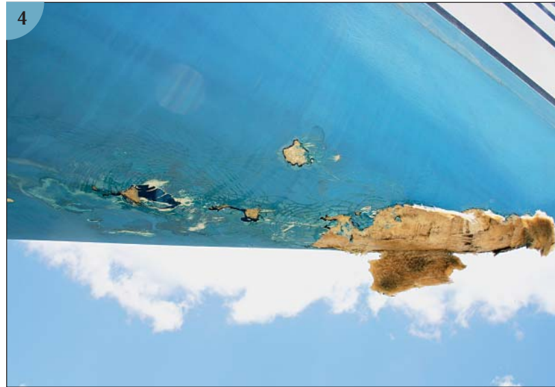
(4) More impact damage, here on the bow of a boat that went onto the rocks. Much of this damage punched through the outer laminate and into the core.
