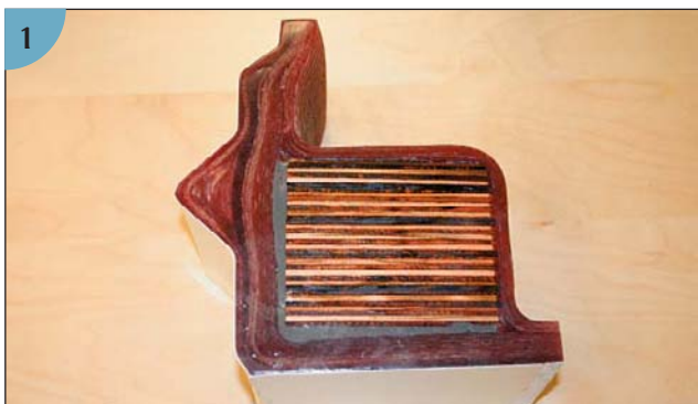
(1) This sectioned Volvo IPS system stern gland shows how it is laminated. The leftward-pointing knuckle is extremely hard to laminate properly, even for a skilled technician, because the fiberglass fabric tends to lift away from and bridge tight
