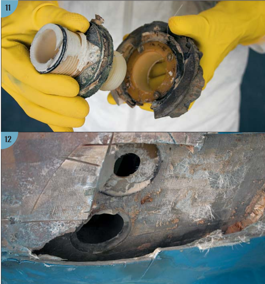
During hull repair, they removed the speedometer through-hull and found that the core around it had rotted. (11) When the instrument had been installed, some material had been squirted into the void, but this material had merely hardened to a rocklike consistency and allowed water to seep into the core, requiring the removal and replacement of an additional core section. (12) With the new core in place, they began laminating the new fiberglass.
