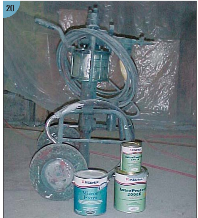
(20) The exterior of the hull underbody is given a barrier coat of Interprotect epoxy resin to provide an additional guard against water penetration.
