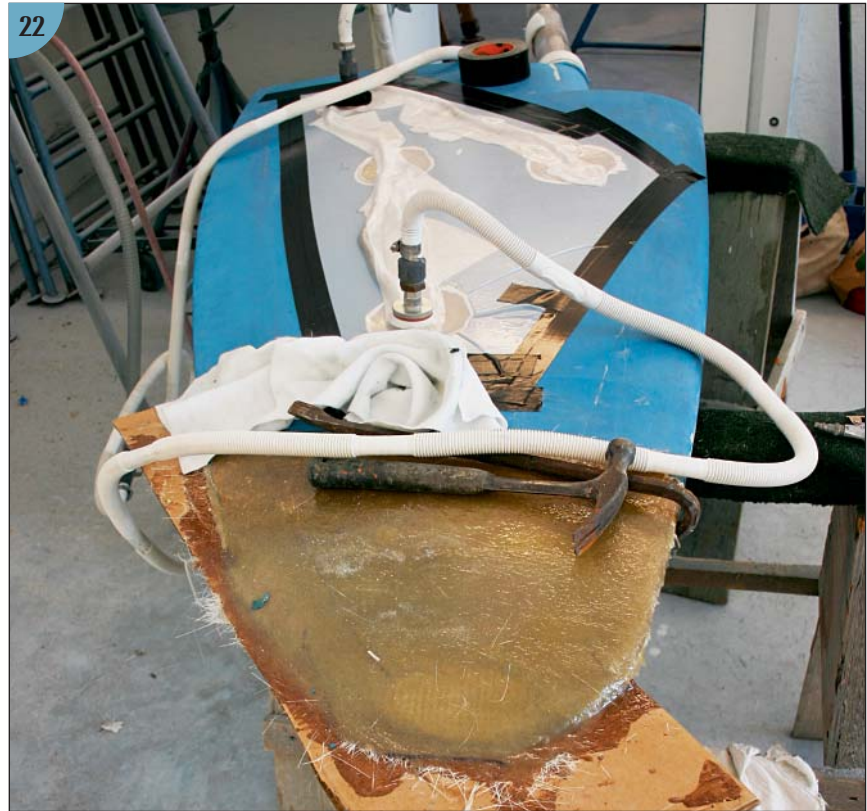
(22) Here they are vacuum bagging the rudder repair to make sure that the laminate is strong in this crucial part of the boat.
