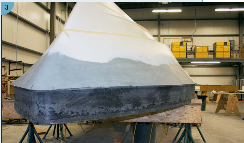
(3) A carbon fiber hull under construction. This entire hull and deck weighs under 600 pounds. With a hull this light, you can use smaller engines, carry less fuel, and achieve a much higher performance.
