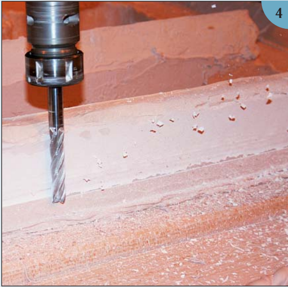
(4) Here a router bit is cutting foam. To the right you can see a stream of chips coming off the bit.
