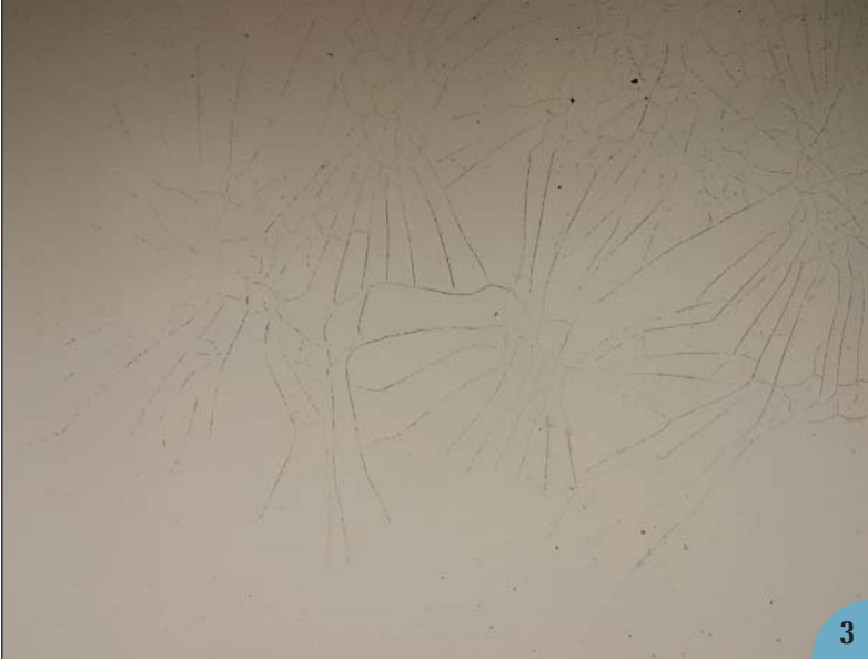
(3) Impact damage on the topside of a single-skin hull. Note the four separate star patterns suggesting four hard impacts, which may have occurred at different times. This damage needs to be fixed as soon as possible so that water cannot penetrate beneath the gelcoat, which can lead to delamination or blistering. If this were a cored hull, you would need to worry about saturation of the core or delamination of the core-to-skin bond.
