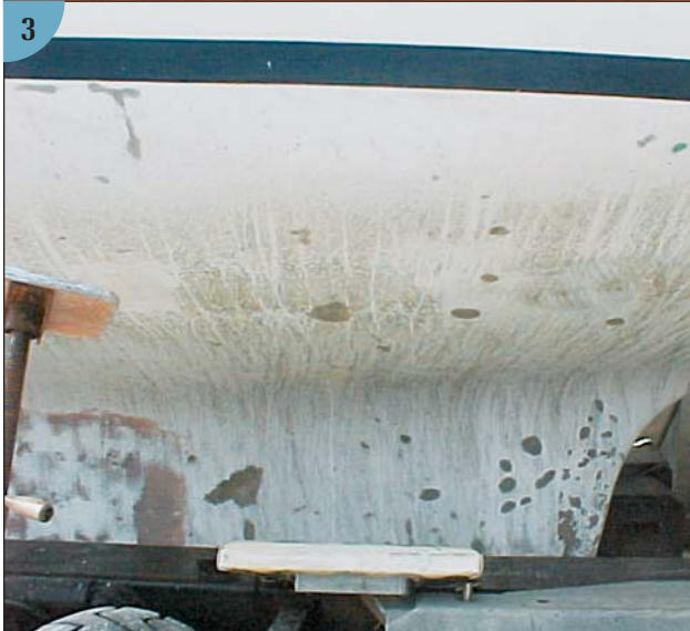
(1) These representative examples of osmotic blistering caused by water penetration into the outer laminate of a hull include blisters after a hull has been peeled, water penetration via blisters into a peeled hull's core (2), which will need to be dried out or replaced, and other examples of blisters (3, 4, 5, 6). (All images courtesy Jamestown Boat Yard.)
