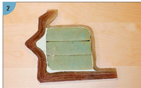
corners rather than conform to them. (2) A section through a foam-cored version of the same gland. Using shaped foam provides a more uniform laminate topology and reduces the possibility of voids in this critical part.
