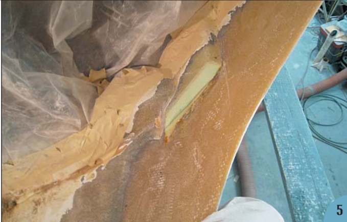
(4, 5, 6, 7) These photos taken from inside the hull show how much of the stern and transom was cut away. Note that edges of the cutaway section have been ground back into scarfs several inches wide.
