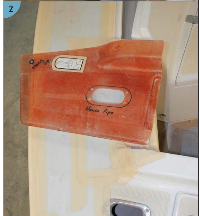
(1) Another template made by a production builder. (2) This one shows where the stern chock hole is to be cut. Any template, or splash, you might need to mold a missing piece could be fabricated in the same way.
