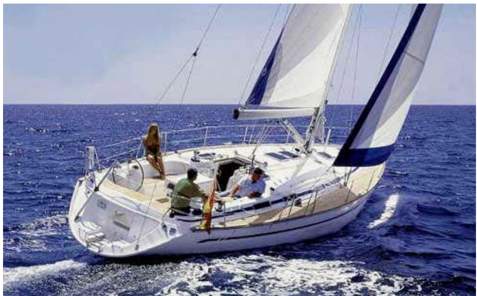
Note how the waterline of this sailboat is canoe shaped in spite of the transom stern.
