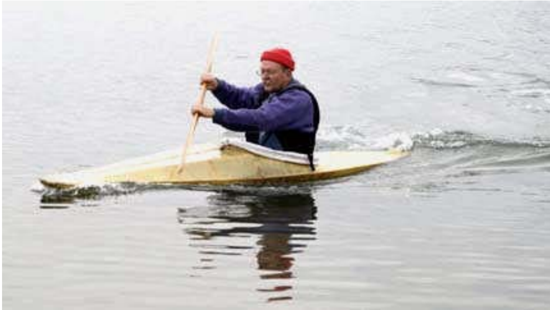
Note how both the bow and the stern create waves as this displacement hull moves through the water.
