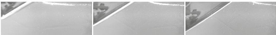
Figure 10. Evolution of the water entry of a wedge (W) ( \beta = 30^\circ ) entering the water at \approx 4.2 m/s at 25, 40, and 55 ms from the impact.
