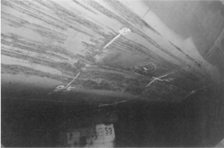
Fig. 5.6.1 Dent of bottom shell by grounding
