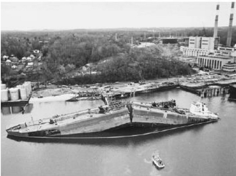
Fig. 10.1.1 Jack-knifed failure of Liberty Ship
