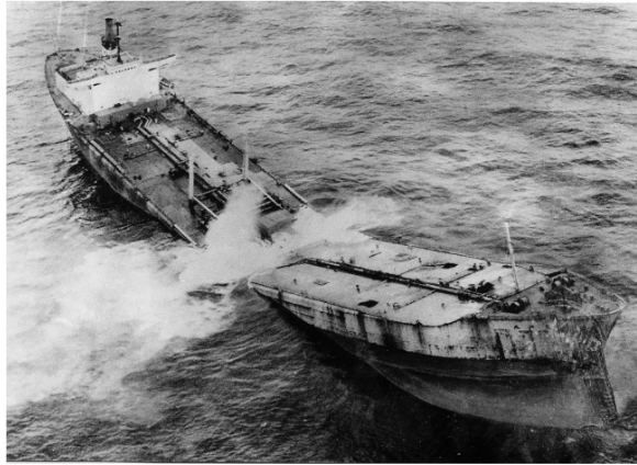
Fig. 2.1 Example of damage on longitudinal members
