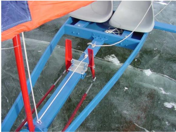
In this shot you can see the foot pedal assembly and seat mounting rails. The center post mounting bracket should be noted also. In the updated version we no longer use the plastic seats. We sit right down on the floor and use a small back rest for our shoulders.
