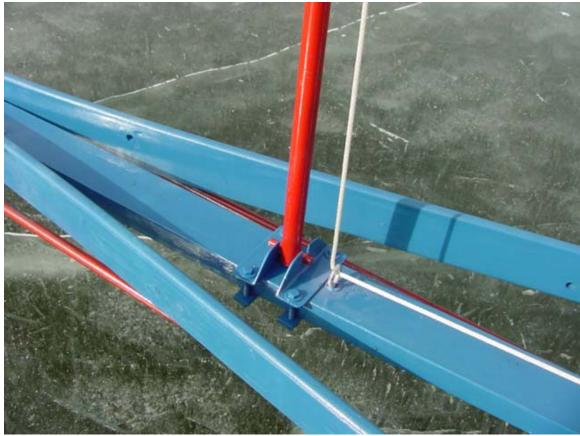
Here is the mast step and the end of the mast. Make sure to mount the 2 mast step brackets far enough apart to allow the mast some freedom of movement. I have about a ½"wider gap then the diameter of the mast. Also notice that I rounded the edges of all my lumber to keep it from splintering as easily.
