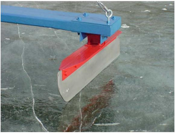
Rear Runner Assembly and Axle mounting on the end of the Beam.
