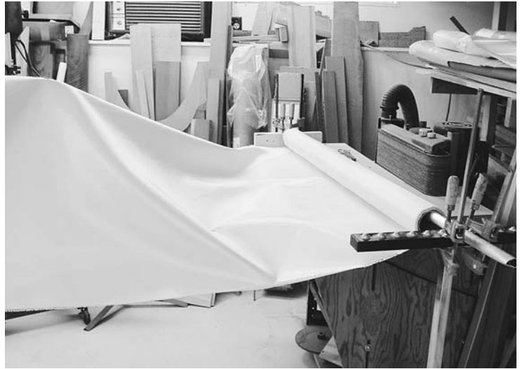
FIGURE 9.1. Kevlar fabric is being unrolled onto the form from a makeshift holder for the fabric that was supplied rolled on a cardboard tube. Here the roll is shown placed on a scrap metal tube, which is clamped to a bench and a roller stand.
