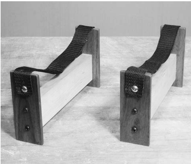
FIGURE 10.18. Two miniature sling stands were made to display my Dragonfly model. The wood parts are scraps of walnut and pine. The slings are cut from the light nylon web material of a recycled fanny pack. Thin leather or ribbon material would work just as well.
