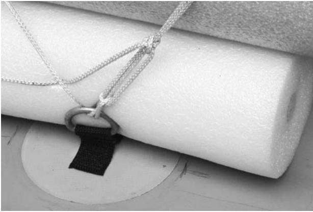
FIGURE 15.17. D-ring and foam cylinder flotation installed in a Royalex hull.
