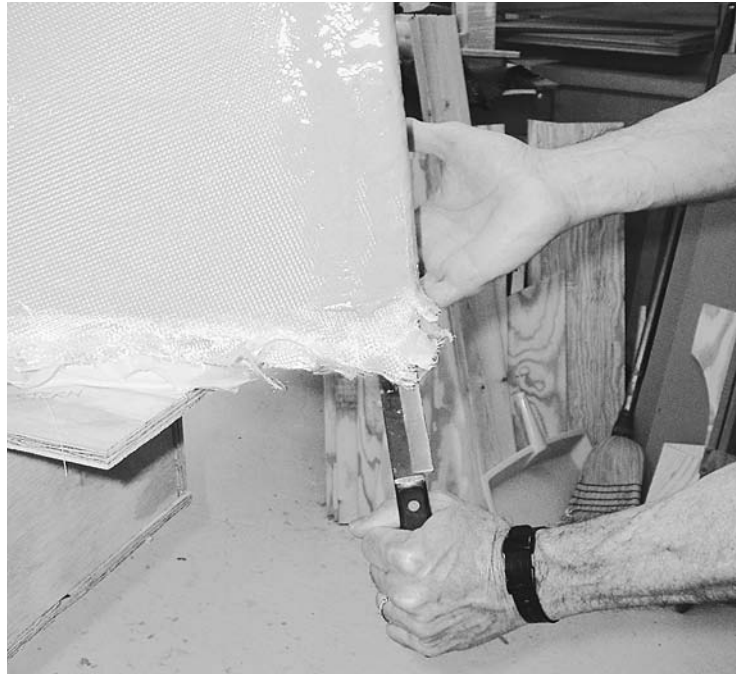
FIGURE 9.8. Use a long knife or thin metal ruler to pry between peel ply and tape to release the laminate from the ends of the form. The ends may stick, and it could take a long time to release them. Be persistent; keep working with the long knife. It may help to tap or drive the ends of the hull upward off the form with a mallet or hammer. Place a block of wood under the end and tap, or whack, as necessary. If all else fails, it is possible to saw the ends apart to remove the hull. The ends can be rejoined with fiberglass and epoxy and reinforced on the inside later. However, persistence is usually rewarded, and I've never found it necessary to saw the ends.
