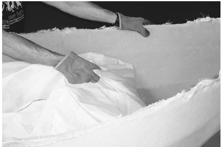
FIGURE 9.11. The polyester fabric is peeled from the interior of the hull. This takes some effort, but the polyester will pull free. Use heavy leather gloves for protection from the sharp Kevlar edge, which is made sawlike when hardened by the epoxy. Pretend there is a shark in your canoe, or a monster muskellunge if you prefer. After the peel ply is removed, be certain to mark the station and cut-line scribes with a marker or a pencil to make them easier to locate.
