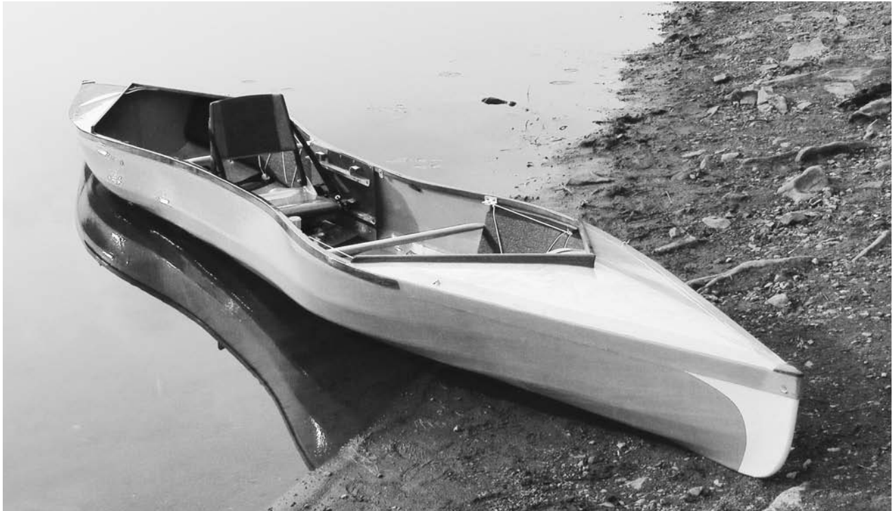
FIGURE 6.1. Wasp is a partially decked solo canoe made using the fabric form process.
