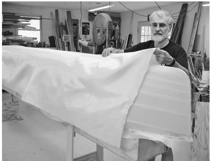
FIGURE 9.2. The Kevlar fabric is draped carefully onto the form.
