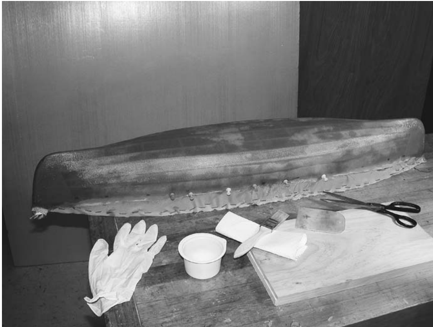
FIGURE 10.14. Fiberglass is laminated over the form just as for a full-size canoe. Marks for the gunwale trim line can be seen through the fiberglass. These were made with marker on the peel ply fabric at each station after shrinking and before laminating. The wrinkles in the fabric at the mounting board are outside the hull area beyond the gunwale trim line, so they will cause no difficulty. Pushpins hold the fiberglass tightly to stringers along the sides at the gunwales to ensure that the hull laminate conforms to the tumblehome of the form.
