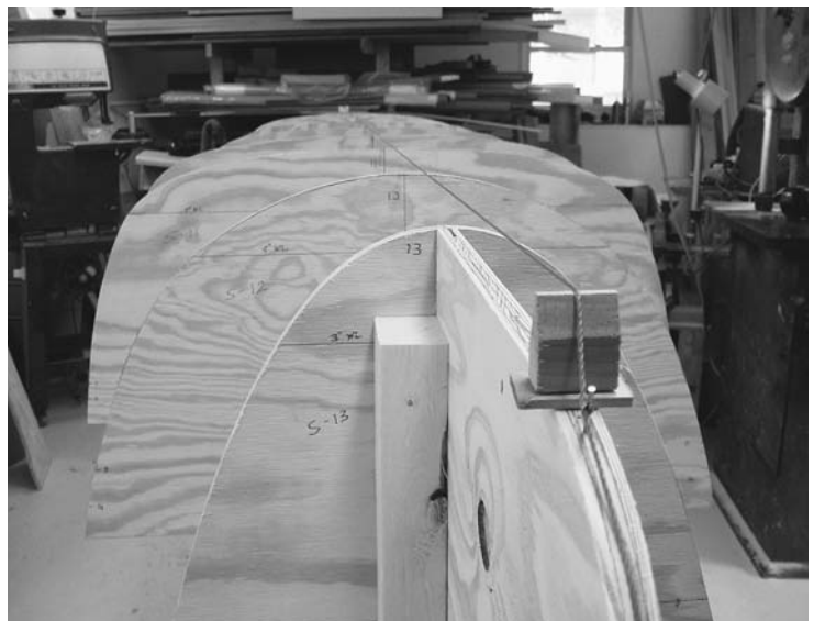
FIGURE 6.5. A string is stretched end to end to align the stations.
