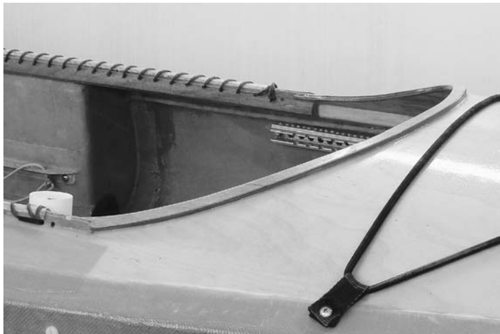
FIGURE 12.15. A curved and arched coaming is formed from plywood.
