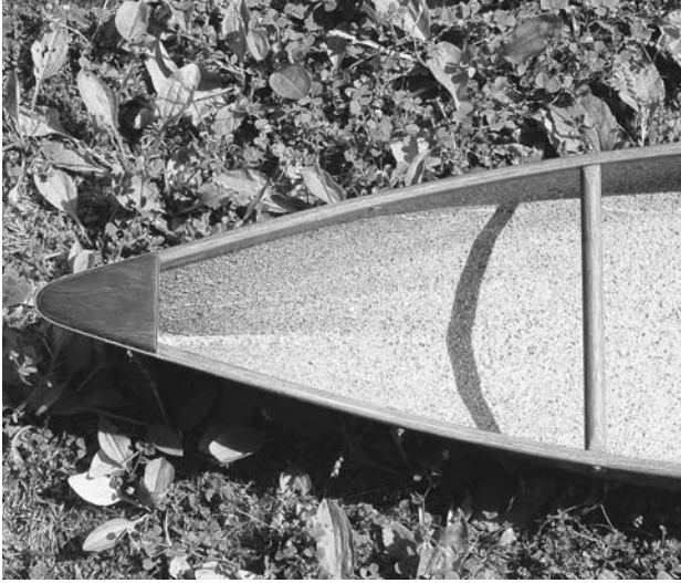
FIGURE 10.20. To avoid any sanding on the inside, the interior of this model was sprayed with a textured paint. You can find textured paints in convenient spray cans at local hardware stores. Masking tape must be used to protect the gunwales and hull exterior from overspray. The end decks were carved from scraps of rosewood veneer. One-quarter-inch mahogany dowels make scale-size thwarts.
