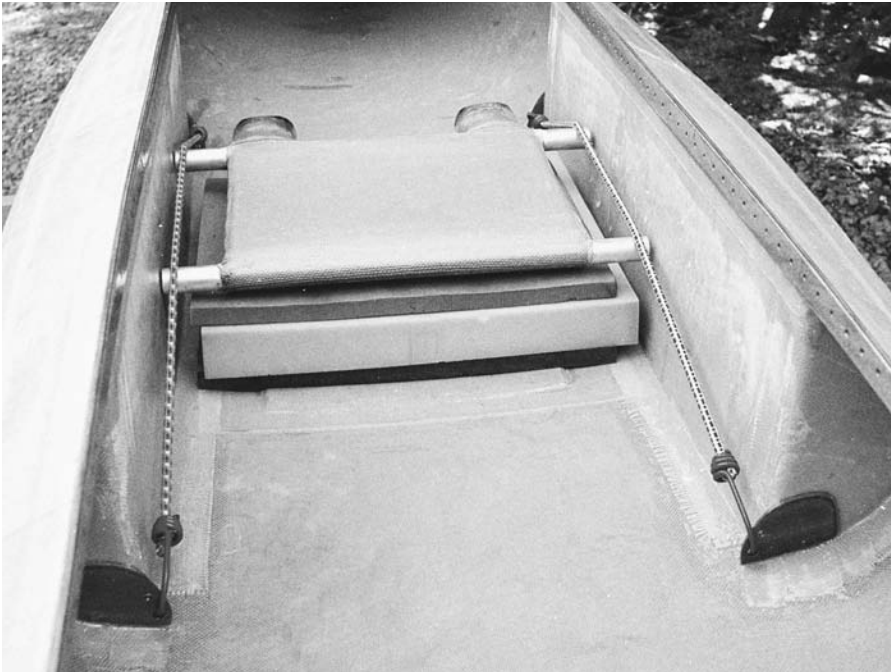
FIGURE 12.18. Plywood hard points are bonded in place near the floor to accommodate ropes for securing gear or bungee cords to hold a movable seat.
