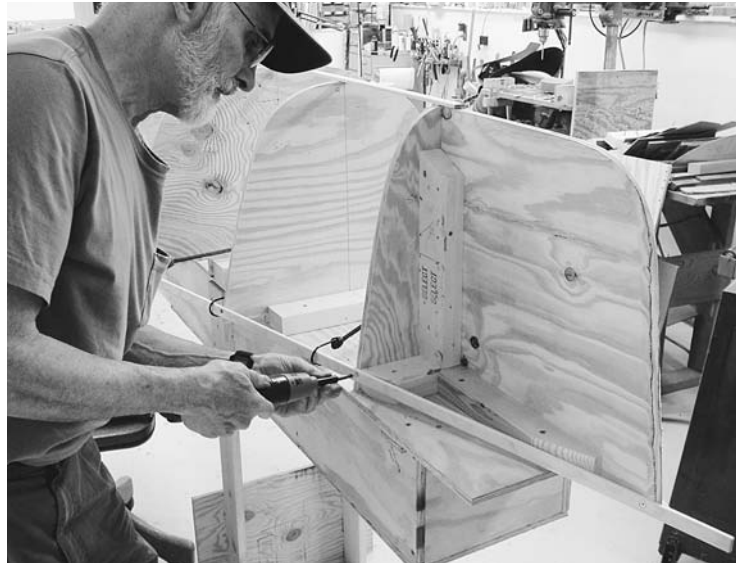
FIGURE 6.8. Attaching the stringers.
