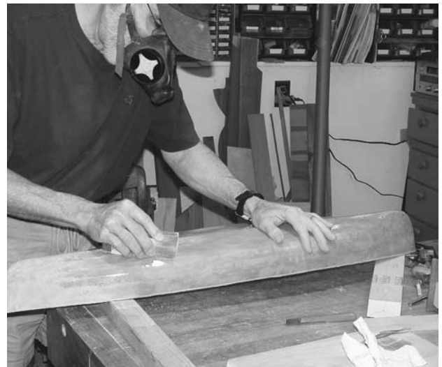
FIGURE 10.15. The hull surface need not be finished any further. It is reasonable to complete the model in a simple manner and save your labors for a full-size boat. However, I've decided on a smooth painted exterior finish for my model Dragonfly. After trimming the hull to the gunwale line, a padded sanding block and 60-grit sandpaper start the smoothing process on the hull exterior. If you desire a really good-looking model, any low spots and pinholes can be built up level with layers of epoxy thickened with microfibers or Microlight filler. Sand the exterior with progressively finer sandpapers, finishing with 220-grit paper.
