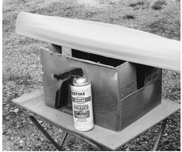
FIGURE 10.21. A coat of primer on the exterior makes it easier to achieve a very smooth finish. Since I chose to spray, the interior was covered with paper and the natural wood gunwales were protected with masking tape. The primer is sanded with 320-grit paper before adding the color coats.
