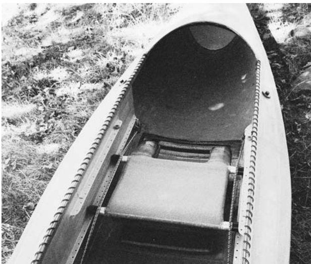
FIGURE 12.21. In the seat position, the combination seat and yoke can be moved forward and aft to trim the balance of the boat through a wide range. Although bungee cords are pictured, spring clips were later added to hold the seat and to speed switching from portaging to paddling. The spring clips are described in Chapter 14.
