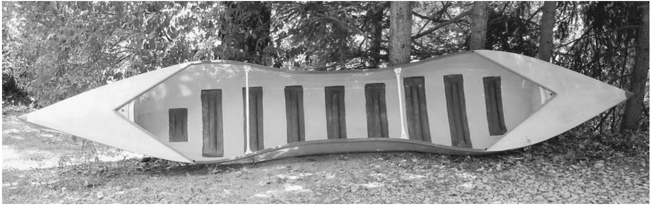
FIGURE 11.26. The rib locations for Wasp are visible here. The bow is to the left.
