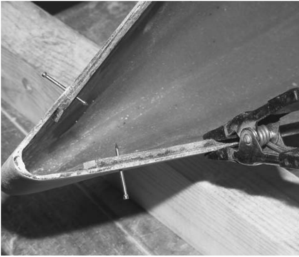
FIGURE 10.16. Wood gunwale strips are bonded to the fiberglass. Small wire nails or tacks in predrilled holes hold the gunwale strips in place on the hull for epoxy bonding. Without nails to keep the parts lined up, they will slide out of place before the epoxy sets.
