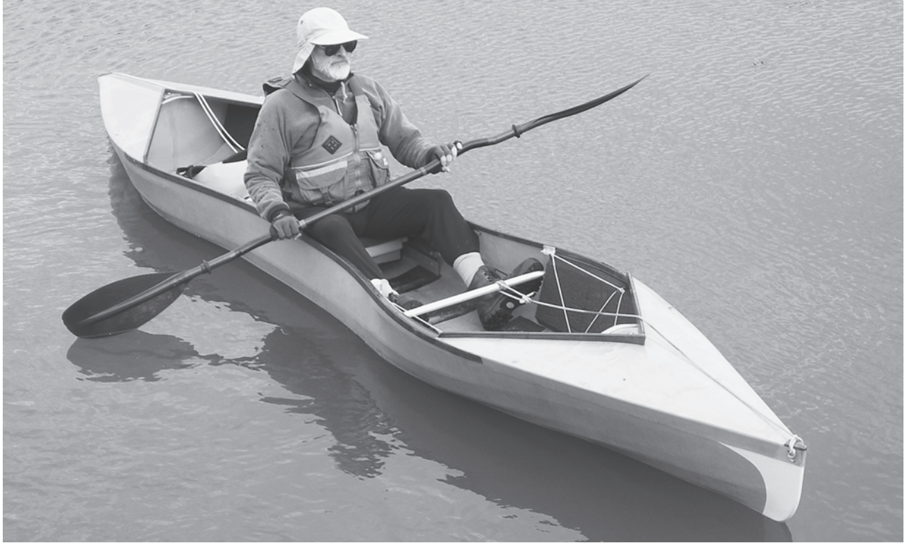
FIGURE 11.28. Wasp is fully outfitted and on the water. The ends of Wasp have received a coating of epoxy, silica filler, and white pigment for extra abrasion resistance. I expect to paddle Wasp where there are submerged rocks and stumps, and the extra coating should lengthen the intervals between touch-up work and repairs on these high-wear areas. Wasp is now ready for adventures! Photo by Carrie Rizzetta.
