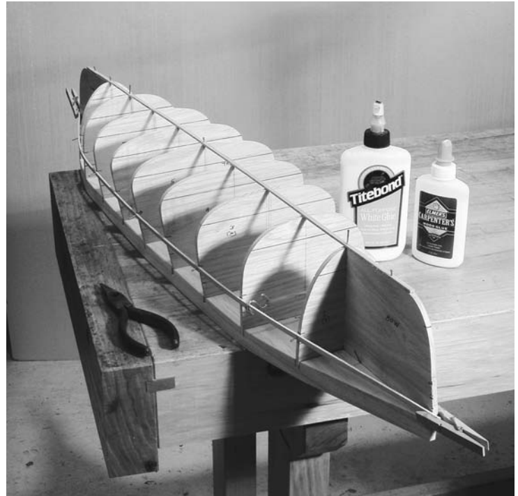
FIGURE 10.5. The mounting board is cut to shape, and the station forms and end forms are glued in place. The first stringers are attached at the keel line and near the sheerline or gunwale location. Clothespins make convenient little spring clamps.
