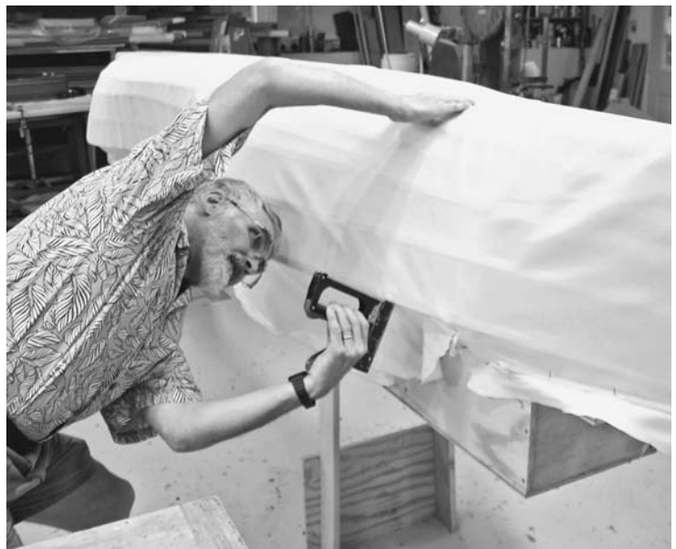
FIGURE 8.4. The fabric is stretched and stapled to the form.
