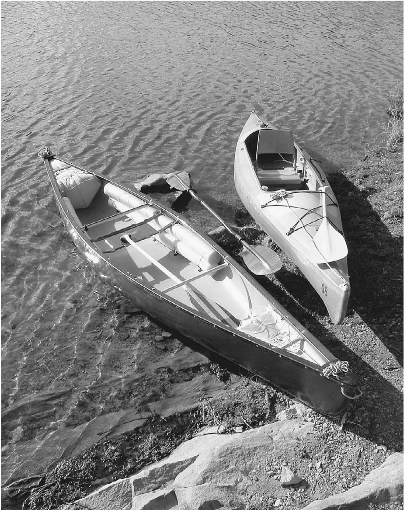
FIGURE 15.1. On the left is a factory-made, Royalex-hull solo canoe with inflatable flotation bags in the ends and foam flotation in the sides. On the right is Kayoo, a lightweight kayak/decked canoe with flotation chambers built in.
