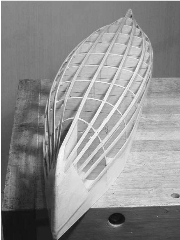
FIGURE 10.9. The ends, stringers, and sides of the mounting board are covered with plastic tape so that epoxy will not stick.
