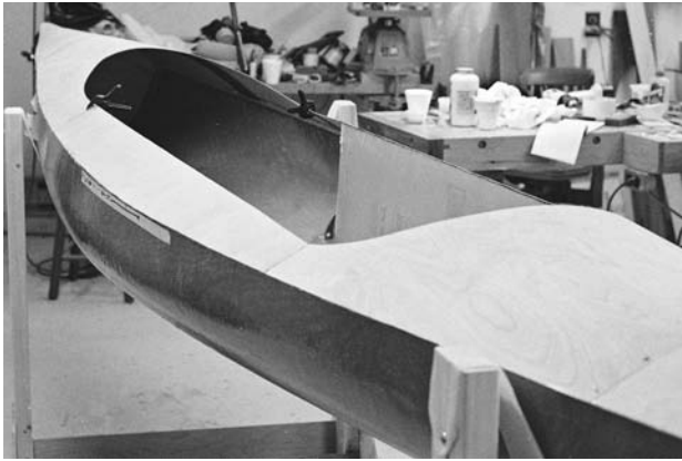
FIGURE 12.12. All deck sections are bonded in place.
