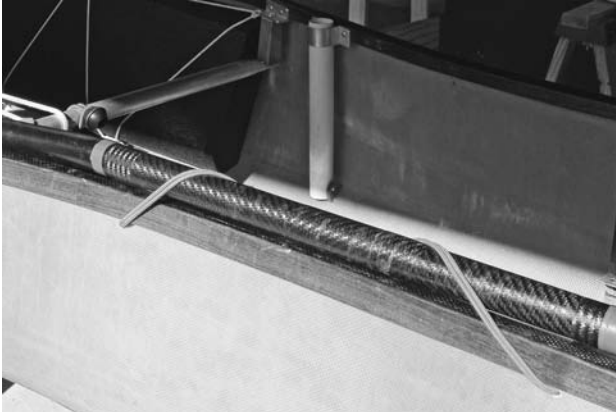
FIGURE 14.5. A paddle shaft is held to the gunwale of Wasp with a bungee paddle keeper.
