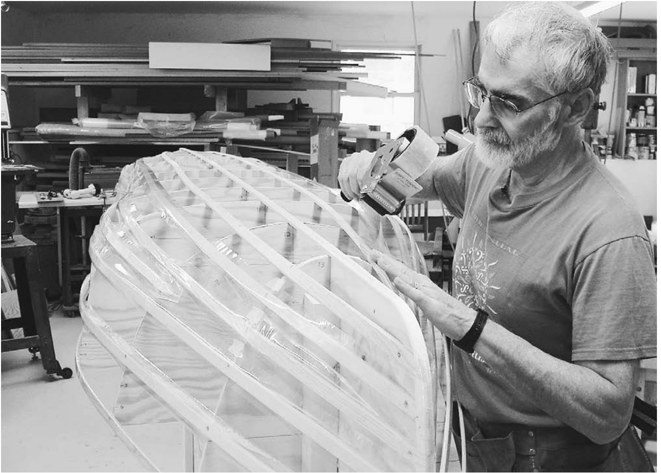
FIGURE 8.1. The stringers and exposed portions of the form are covered with clear plastic package-sealing tape.
