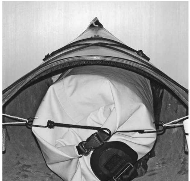
FIGURE 12.23. Bow tie-in points are just forward of the foot rests.
