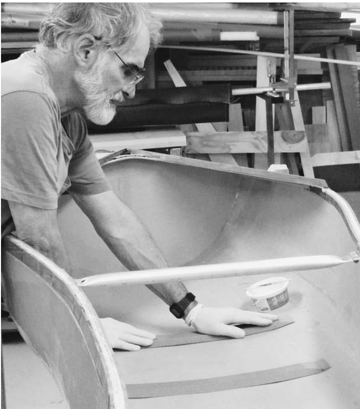
FIGURE 11.21. Bonding foam ribs into the hull.
