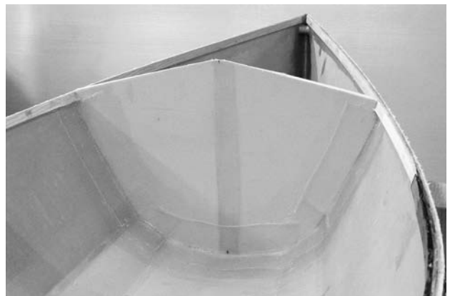
FIGURE 11.10. The bulkhead is bonded in place.
