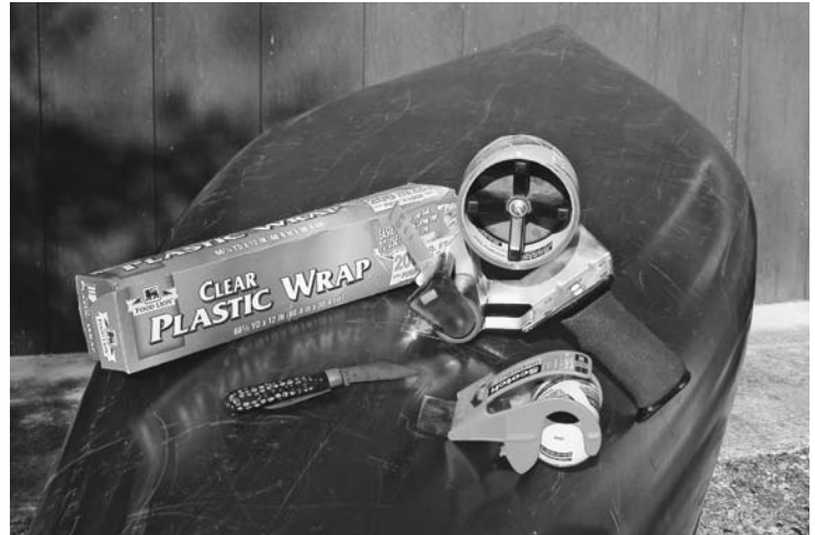
FIGURE 7.3. Package-sealing tape and plastic wrap will protect the canoe that is used for a form, enabling the new laminated hull to be easily removed. This 15-foot canoe made of Royalex is more than 20 pounds heavier than the Kevlar canoe laminated on top of it.
