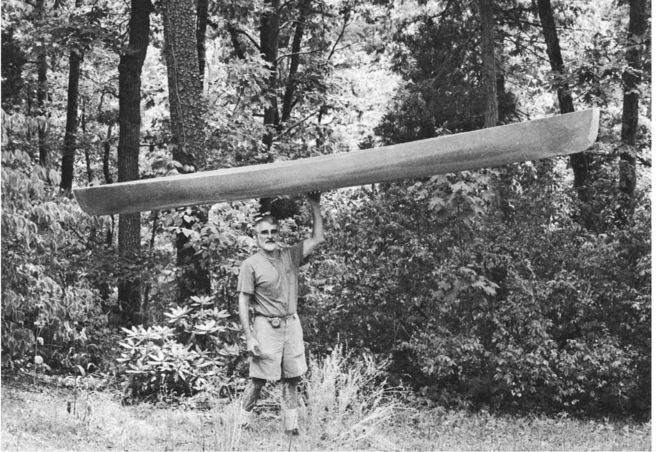
FIGURE 1.2. A light boat starts with a light hull. This strong hull, laminated with Kevlar and carbon fiber, is 14½ feet long and weighs 11.8 pounds.
