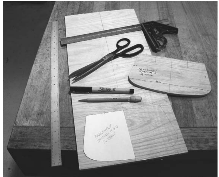
FIGURE 10.1. Tracing station templates for the Dragonfly model.
