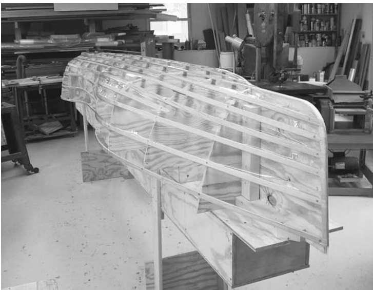
FIGURE 8.2. The form now has release tape in place.
