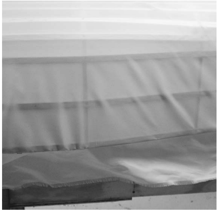
FIGURE 8.5. Any wrinkles in the fabric are distributed over as wide an area as possible.
