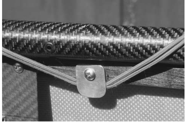
FIGURE 14.6. A hook to hold the bungee is screwed to the inside of the gunwale and pointed down so that it will not catch on clothing or cause injury. This one was cut from 1/16-by-1-inch aluminum bar stock and filed and sanded smooth. The wide end and surface are safer than smaller metal hooks. Hardware and building supply stores often stock a selection of aluminum bar stock and extrusions.
