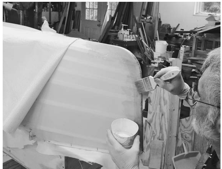
FIGURE 9.3. To begin the laminating process, fiberglass and epoxy are applied to the ends.
