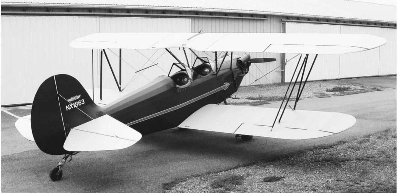
FIGURE 2.1. Although it looks like an antique, this experimental Hatz biplane was built in 2000 by Gordon Hockman of Shenandoah Junction, West Virginia. It exhibits the fabric on wood frame and metal tube frame aircraft construction that is the inspiration and basis for building fabric form canoe hulls. The turtle deck behind the cockpit most clearly shows the construction of fabric over wood stringers. This method of building aircraft goes back to the Wright brothers and the classic biplanes of World War I and the 1920s. It is a time-proven process, and some new aircraft are still built this way. The author crafted the cockpit woodwork and performed the test flights.
