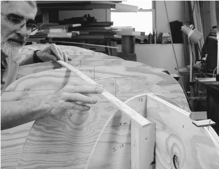
FIGURE 6.6. Use a wood strip to check the curve between stations. The curve of the hull should be smooth, gradual, uniform, and symmetrical side to side.
