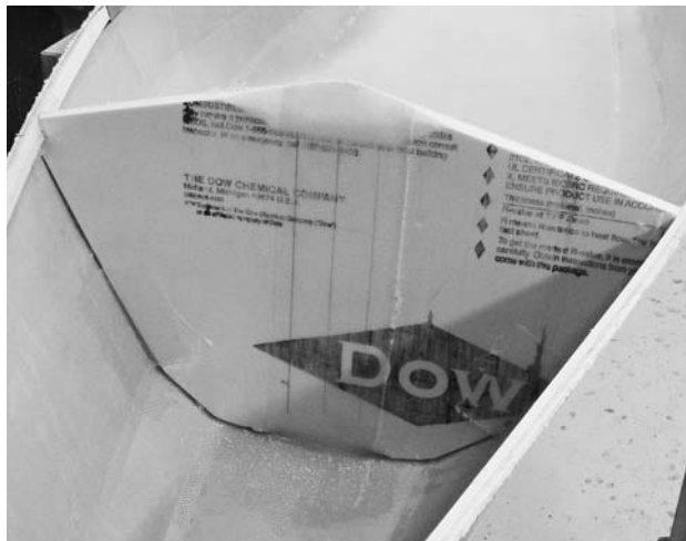
FIGURE 11.11. The back side of the bulkhead is reinforced. If the bulkhead is rather large, as it is likely to be if it is 25 to 30 inches from the end, then it should be reinforced on the inside. Here a layer of heavy fiberglass tape 4 inches wide has been applied vertically to the middle of a bulkhead and lapped onto the hull at the bottom. Scraps of fiberglass also reinforce the joint at each side. This may be hard to see as the fiberglass is almost clear when wet with epoxy.
