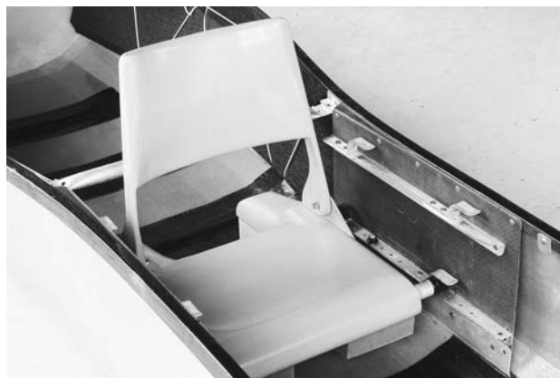
FIGURE 14.16. The combination seat and portage yoke is in sitting position on the lower rails.
