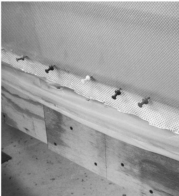
FIGURE 9.5. If the design has any tumblehome, thumbtacks may be used to force the epoxy-saturated Kevlar to conform to the required shape.
