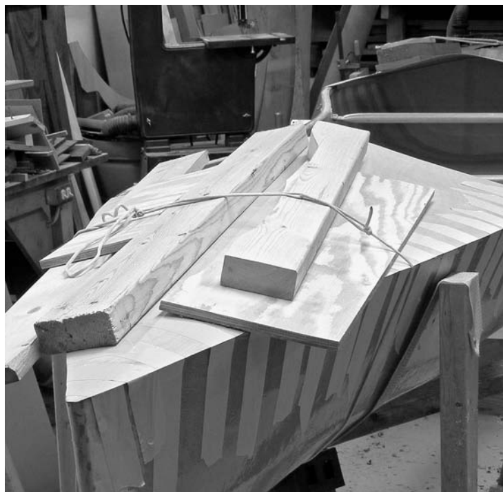
FIGURE 11.14. The deck is held in place with masking tape, rope, and wood scraps while the epoxy cures.
