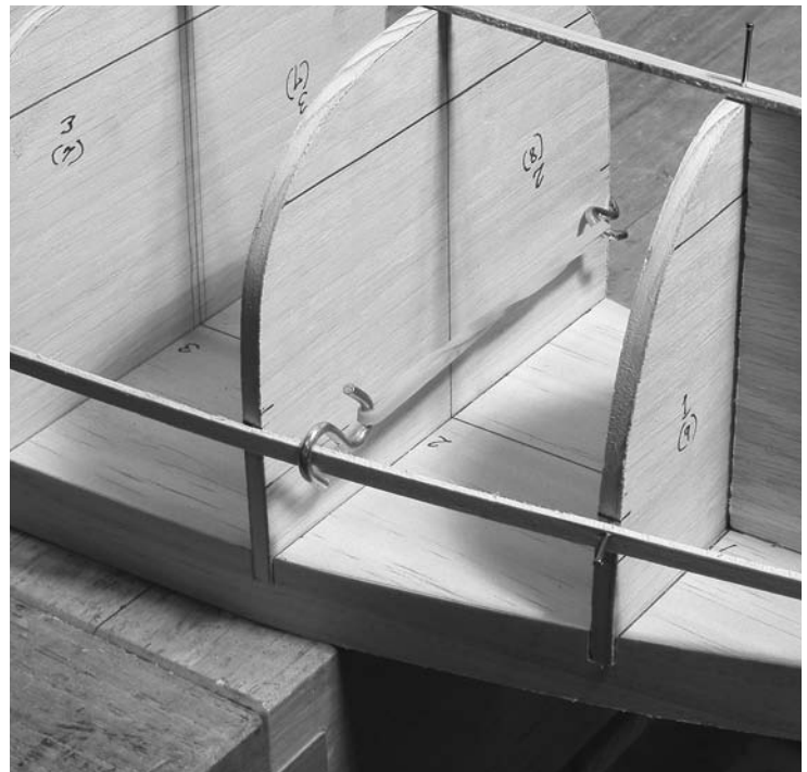
FIGURE 10.6. Rubber bands and S-hooks make miniature bungee cords to hold stringers.
