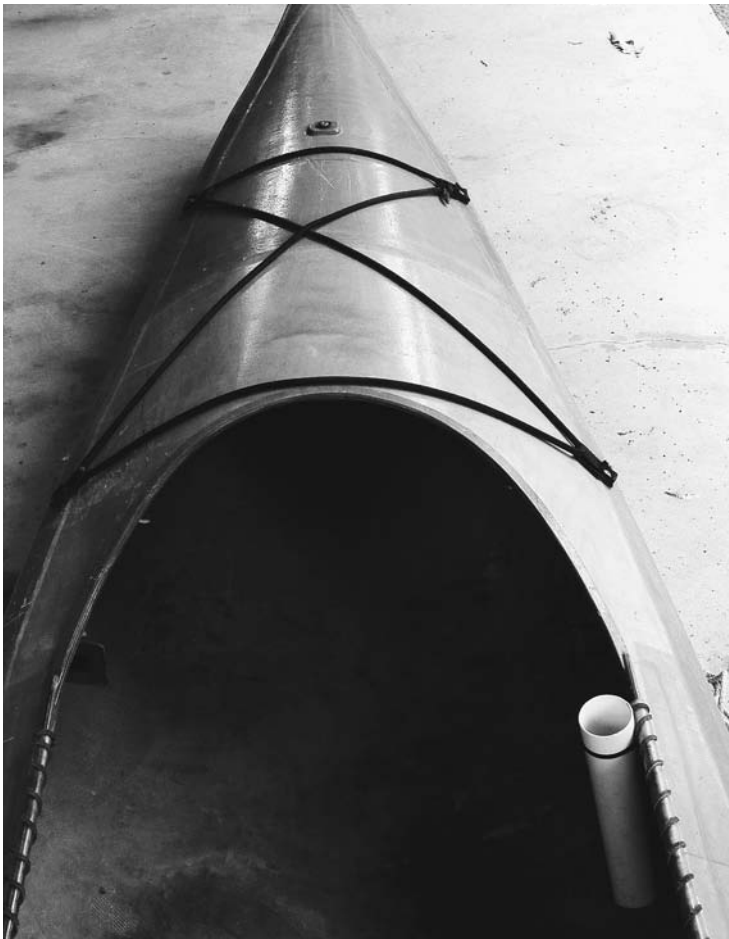
FIGURE 11.18. A curved and arched deck coaming on Kayoo.
