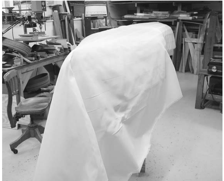
FIGURE 8.3. A 2.7-ounce polyester fabric is draped over the form.
