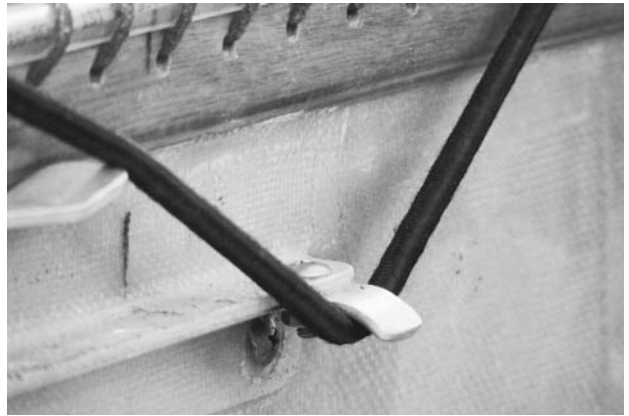
FIGURE 14.8. On Kayoo an aluminum bungee hook is screwed to one of the rails that support the combination seat and portage yoke. Make sure that you mount a hook so that it will not catch on clothing or cause injury.
