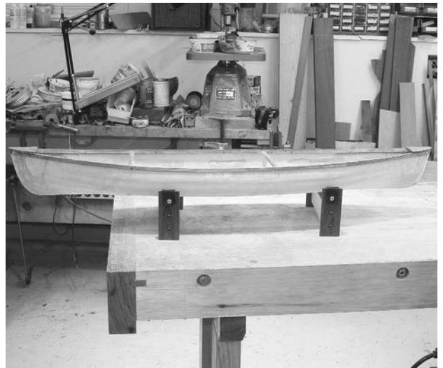
FIGURE 10.19. The exterior fiberglass is sanded and ready for paint.
