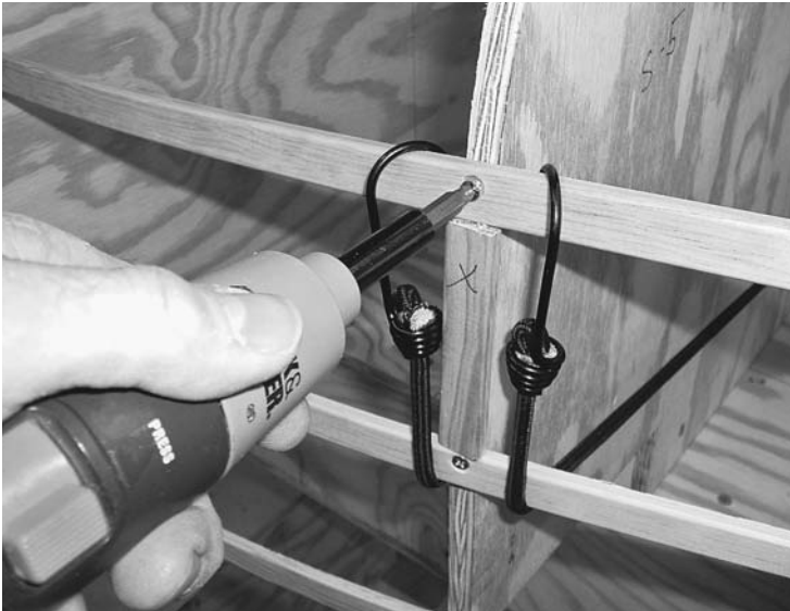
FIGURE 6.10. Bungee cords hold one strip in place against a station form and against a spacer block (marked with an "X") while the strip is screwed in place.
