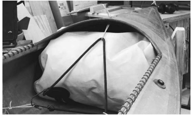
FIGURE 12.22. Cavernous volume under the rear deck accommodates portage packs or large dry bags. Tie-in points allow gear to be easily secured against possible capsizing. Although most dry bags are not intended for full submersion, they can provide extra flotation long enough for most capsize emergencies. And some flotation bags are designed to double as dry bags. The extra flotation floats a swamped boat higher in the water and reduces the bailing required after self-rescue reentry.
