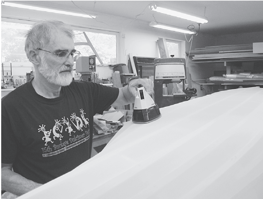
FIGURE 8.9. The fabric is shrunk taut with a warm clothes iron.
