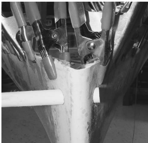
FIGURE 11.6. A piece of plastic pipe is fitted in place to seal and reinforce the line hole.
