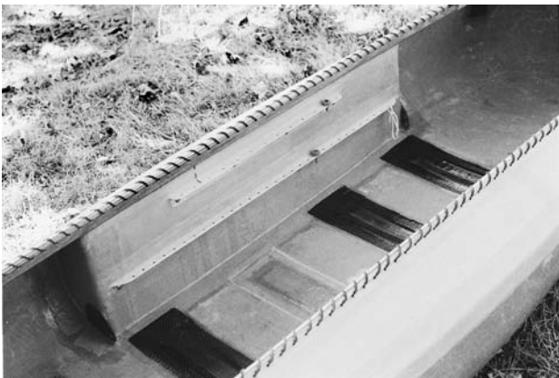
FIGURE 12.19. Rails attached to Kayoo's side chambers will support a combination seat and portage yoke as described in Chapter 14. The aluminum angle rails are held to the side chamber walls with stainless steel sheet metal screws and then bonded to the walls with a layer of fiberglass and epoxy from the top and bottom to ensure structural strength and watertight flotation chambers. The Wasp prototype lacks built-in side chambers. Instead, it has removable panels to support the rails, which are installed with machine screws. (See Figure 14.15.)
