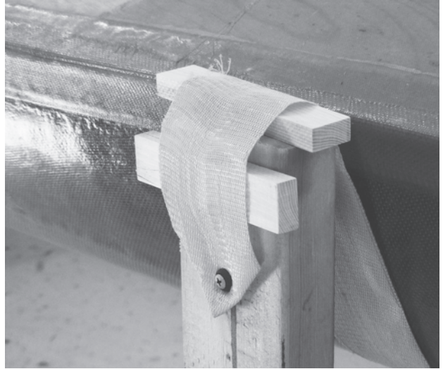
FIGURE 9.15. Blocks can be placed under the web to adjust the stand height.
