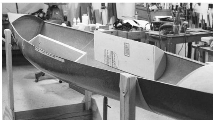
FIGURE 12.10. Side flotation chambers are test-fitted into the hull.
