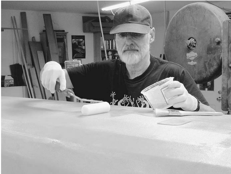
FIGURE 9.7. Additional coats of epoxy are applied with brush or roller to seal the hull and fill the weave of the fabric. Note once more that I should be wearing a respirator.
