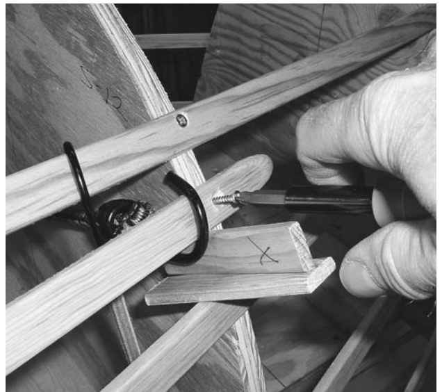
FIGURE 6.13. A short strip may be needed wherever there is a sharp turn of the hull. This is one end of the strip shown in Figure 6.14.
