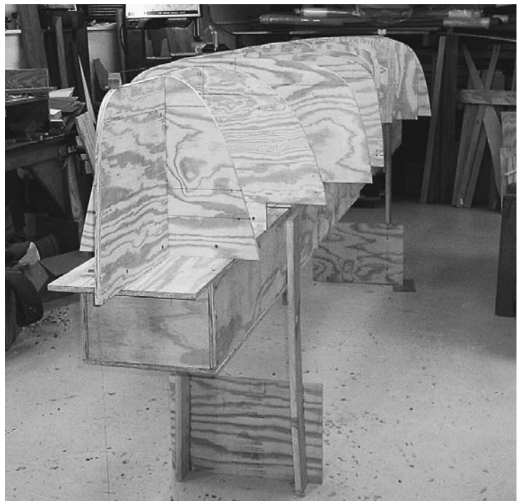
FIGURE 6.3. Stations are assembled to the strongback.
