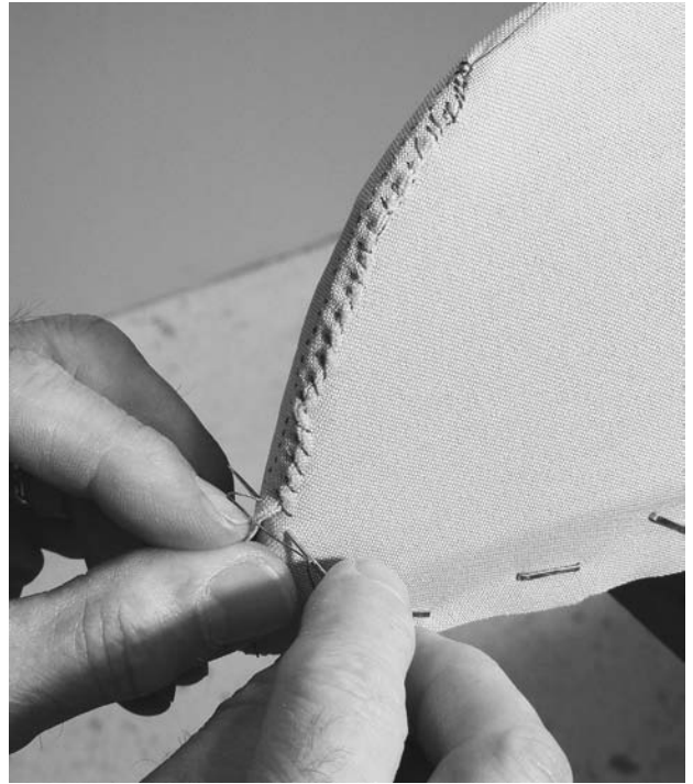
FIGURE 10.13. The fabric is trimmed to within about ¼ inch of the end stitches. The remaining ¼-inch flap of fabric is folded to one side and sewn to lay flat.
