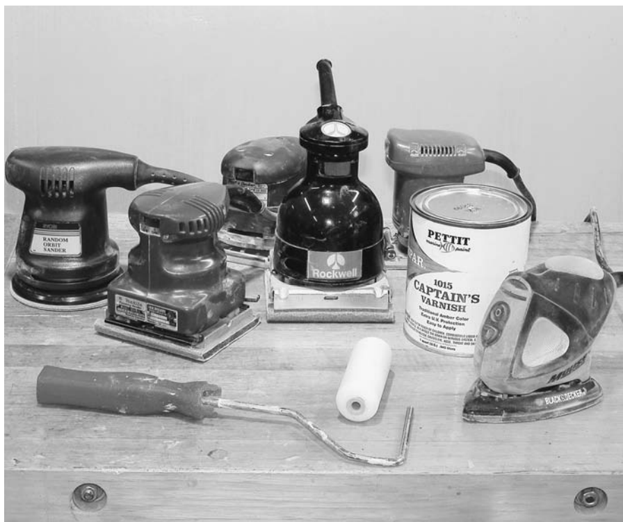
FIGURE 13.3. It is possible to do a lot of damage with power sanders! It can be difficult to avoid wavy surfaces with power sanders, so it is often best to do the rough shaping and coarse sanding by hand with sanding boards and blocks. However, lightweight palm-size sanders are great for coarse sanding before filler is applied and for fine sanding and finish work. On the left is a random orbit sander, which is good for fast removal of material. The wedge-shaped sander on the right will sand into corners and curves inside the hull. The others are palm sanders, which are versatile, easy to use, and excellent for final sanding with fine sandpaper.
