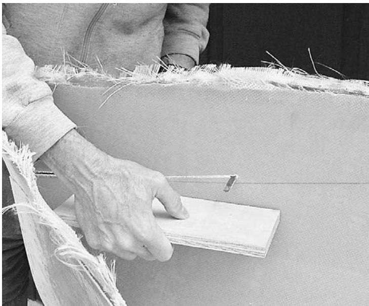
FIGURE 9.13. Trimming the hull with a saber saw.
