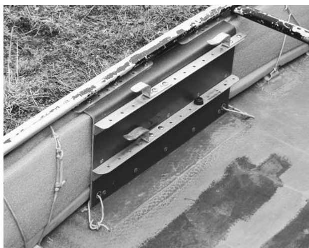
FIGURE 14.20. An old Kevlar solo canoe has been fitted with a combination seat/yoke mount similar to the ones in Wasp and Kayoo. The side wall is \frac{1}{8} -inch-thick Kevlar 18 inches long laminated over two sides of a 2 \times 10 as a form to provide the right-angle shoulder bend at the top. The attachment to the hull at the bottom is similar to the attachment in Wasp described earlier. At the top, the Kevlar side wall is screwed to aluminum angle brackets, which are in turn screwed to the gunwale. The side wall also helps hold foam side flotation (as described in Chapter 15). The rope loops at the bottom provide places to tie ropes or hook bungee cords for securing camping and safety gear.
