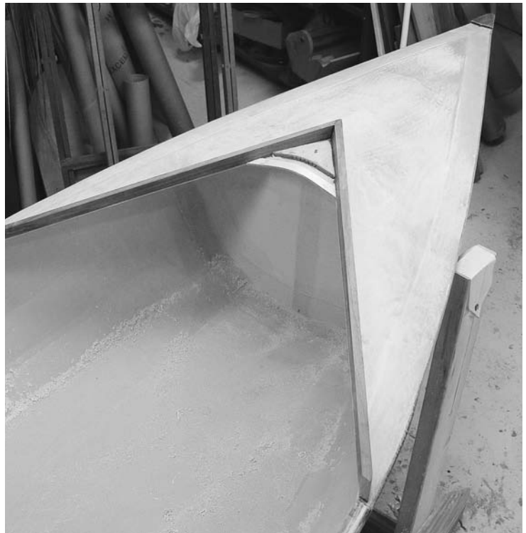
FIGURE 11.17. Here is the deck termination above the bulkhead at the cockpit opening.
