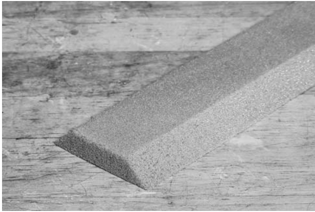
FIGURE 11.22. A foam rib with beveled sides.
