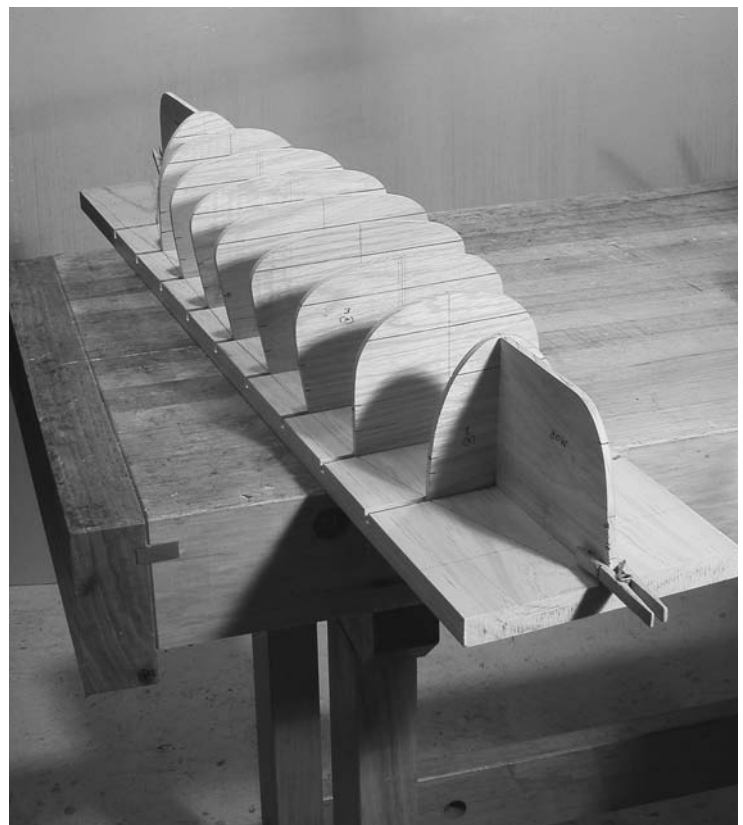
FIGURE 10.4. The station forms and end forms are test-fitted on the mounting board.
