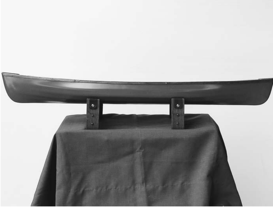
FIGURE 10.23. After the paint dries, only a few finishing touches remain. For the finished model shown here, the wood gunwales, end decks, and thwarts were given a hand-rubbed oil finish for a non-glossy, natural wood look. Varnish or lacquer will provide a gloss finish, if you prefer.
