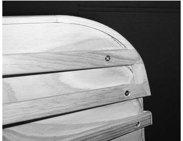
FIGURE 6.16. Filler pieces at the stems are cut to fit and are glued lightly in place. Additional filler pieces will be added until the gaps between all the strips are filled at the ends. The ends must be smooth and continuous or the hull will not release from the form.
