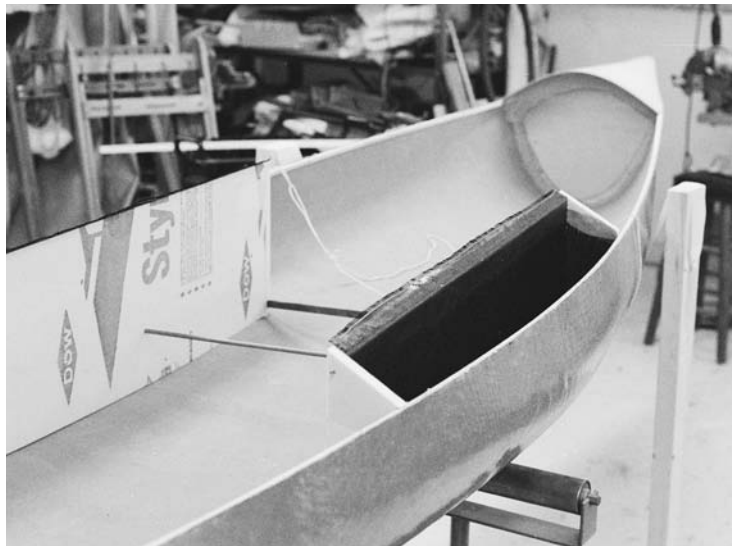
FIGURE 12.11. These side chambers are being reinforced on the inside with carbon fiber. Fiberglass could also be used. The cloth must lap onto the hull at the bottom and roll onto the exposed edge of the foam panels at the top. This will ensure a stronger bond and a more watertight seal to the plywood deck covers that will be installed later.
