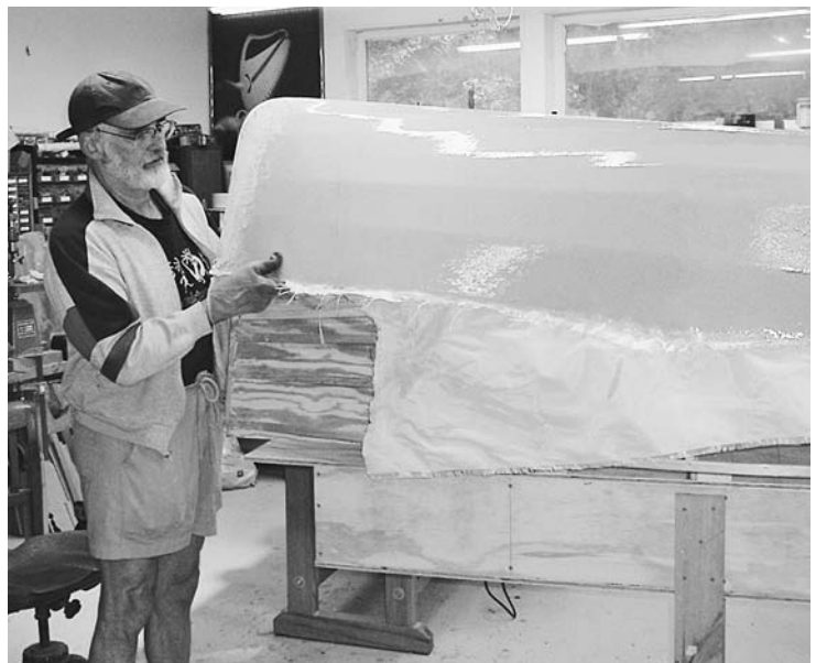
FIGURE 9.9. Lift the hull from the form, end first. Wear leather gloves.
