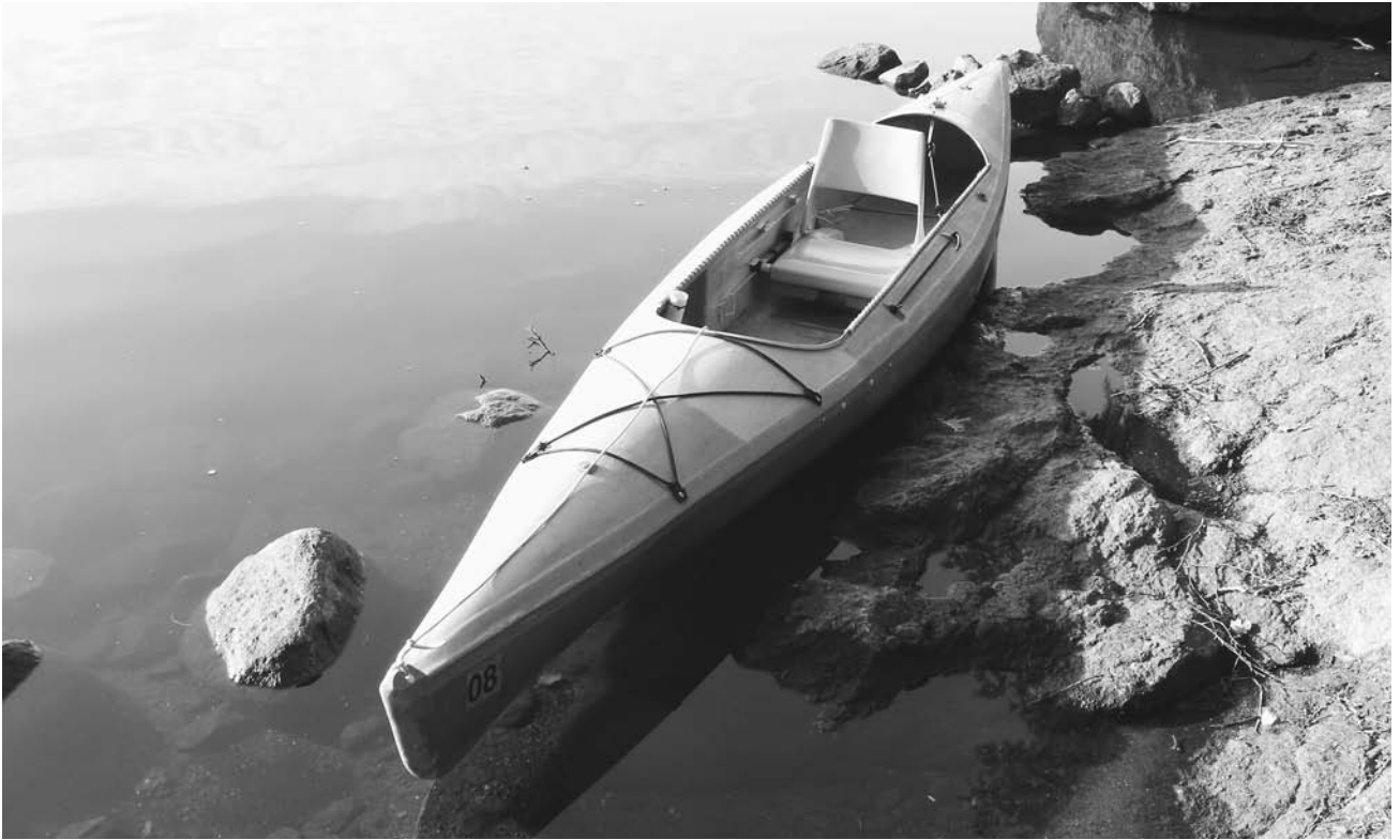
FIGURE 16.9. Kayoo with deck rigging and a combination seat and portage yoke with a folding backrest.
