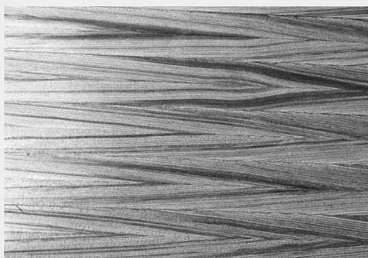
Figure 6-28. Flipping over every other strip creates an alternating pattern. Since the grain varies across the width of the original board, the grain will vary across the span of the strips.
