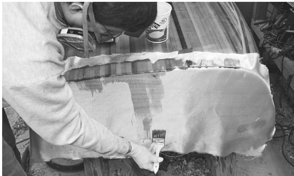
Figure 11-23. The glass on the transom extends a couple of inches onto the strips. Note the use of blue tape to make a clean edge. The end grain of the strips absorbs a lot of resin, so either keep adding more or do a seal coat before starting the glass coat.
