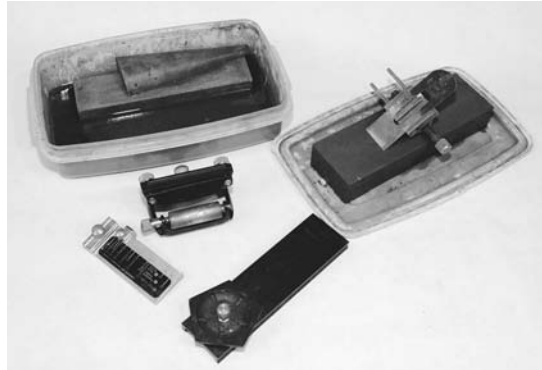
Figure 3-1. Sharp tools make just about everything quicker, easier, and more precise. You can do a good job sharpening your tools with sandpaper stuck to a piece of glass, or use waterstones as shown. The little jig that holds the plane blade on the right will shorten the time spent sharpening, or you can use the more sophisticated jigs shown below the stones.
