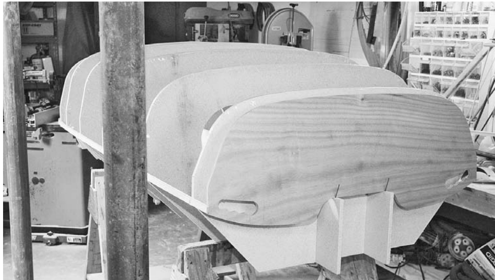
Figure 11-10. The Coot has transoms (flat ends) at both ends. The transoms have been pre-coated with epoxy to protect them from glue drips and other abuse. This strongback has supports to hold the transoms in the correct position.
