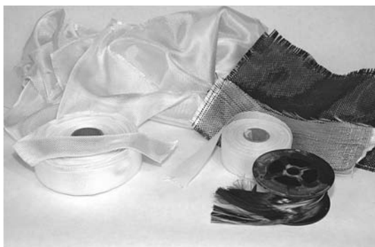
Figure 2-5. Reinforcing fabrics are available in a variety of materials. The white fabrics on the left are fiberglass, which becomes clear when saturated with resin. The black carbon fiber (top right) stays black. Woven tapes of different widths (middle right) are available for reinforcing and joining parts. The spool on the lower right contains carbon fiber “tow,” an unwoven roll of fibers that can be used to make reinforcing ribs.
