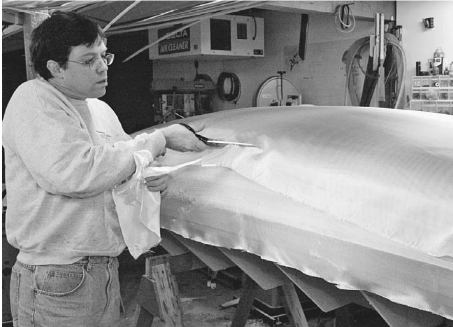
Figure 11-18. The Coot is too wide to span with one piece of cloth. For a light layup, you can overlap two layers along the centerline, but I wanted some added durability, so I overlapped two layers of 6-ounce cloth across the whole bottom. Trim the cloth so it follows the line of the strips. This helps hide any irregularity that may result.
