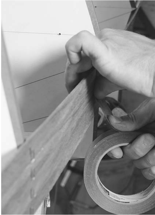
Figure 6-16. A smooth finish in the completed boat starts with a smooth joint between strips. Cove-and-bead strips are pretty much self-aligning but may need some help staying tight between the forms. I've taken to running a length of tape over the strip down onto the previous strips. This is usually enough to pull the joint together, and with square-edged strips the tape will help hold the strips even with each other. Ideally there should be no steps detectable from strip to strip. With standard carpenter's glue the glue sets up quickly enough that the tape may be removed in a few minutes.
