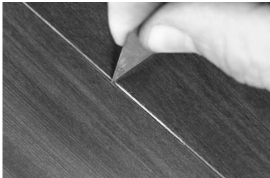
Figure 13-45. It is very hard to create a crisp edge with stain because it soaks under masking tape very easily. You can stain right over any transition, then scrape off the stain. Here I stained the whole boat and then scraped the stain off the maple feature line with a modified utility knife blade.
