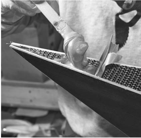
Figure 13-64. Make a dam to contain an end-pour. Strips of tape would do the job, but here I cut a piece of an old squeegee. Add as many microballoons to the epoxy as it can contain and still move a bit. Fill in behind the dam until the epoxy is even with the top of the sheer. Clean up the top surface with a rasp after the epoxy has cured. If you prefer, you can install a piece of wood instead of the epoxy; just be sure that all the grain is very well sealed so it doesn't absorb water and rot.
