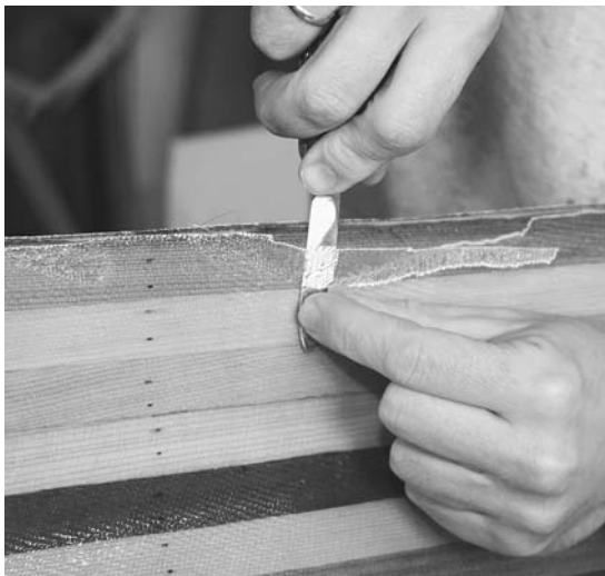
Figure 9-25. You may get a bubble in the glass. This will most likely be along the gunwale/sheer. Usually you can just shave off the lifted glass by holding a knife tight against the surface. Try to get it as flush as possible, then sand the edge so it doesn't jut up. If the gap is under a gunwale or will get another layer of glass later on, wait until then and just cover it with the gunwale or lay the new layer of glass directly over the area. If this is not an option you may patch over it with an oversized scrap.
