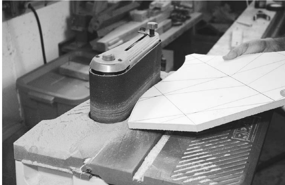
Figure 4-5. If you don't trust your hands to cut out forms exactly on your first try, cut them oversize and then sand down to the line. Here I'm also beveling the edge of the form.
