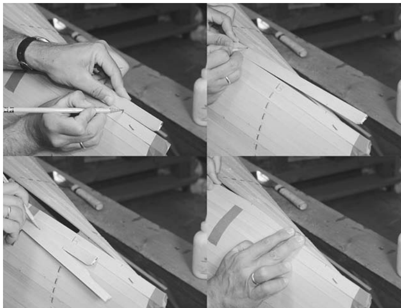
Figure 12-18. Now it is time to close up the bottom. Fit strips into the bottom gap by marking both the length and where the upper edge of the strip crosses the gap. Connect these two points and then trim to that line.
