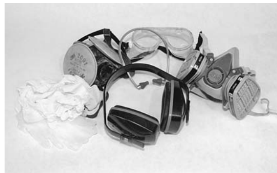
Figure 3-15. Although many of the materials used in strip building may seem benign, there are risks. You should strongly consider wearing hearing and eye protection whenever you run power tools. Wood sawdust is considered carcinogenic; a good dust mask (upper left) will keep it out of your lungs. Even though epoxy does not smell much, an organic vapor respirator (upper right) is highly recommended. You also don't want to get epoxy on your skin, so wear gloves.
