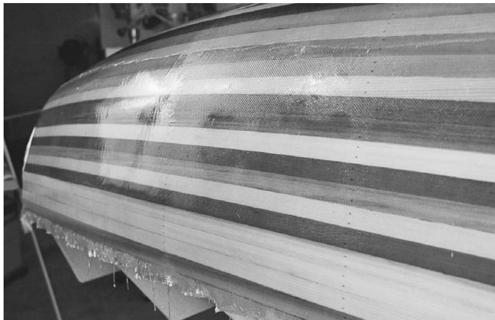
Figure 9-27. The fill coat fills up the fabric texture (right) to create a smooth finish (left). There are several methods for doing this: some are quicker but open you up to making a mess; others are more controlled but time consuming. I brush on the epoxy using the same crisscross technique I use to apply varnish.
