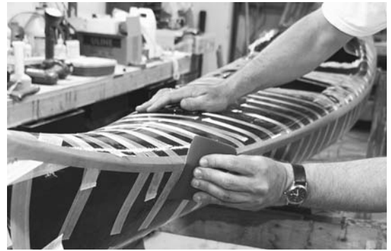
Figure 9-33. Apply tape across the seam every 4 to 6 inches to be sure the seam does not pop while you are working on it. When the seam is aligned and secure, apply a strip of masking tape along the seam to keep the epoxy in. Burnish down the tape so there is no room for epoxy to collect.
