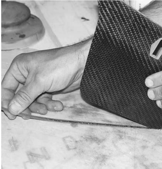
Figure 13-58. Bend a thin strip of mahogany around the edge of the cheek plate to cover any edge grain that was not sealed by epoxy. Dots of CA glue hold the edging to the cheek plate, which should be pre-sprayed with accelerant. Press the edge down against the worktable as you work around the edge to help keep the thin strip from breaking.
