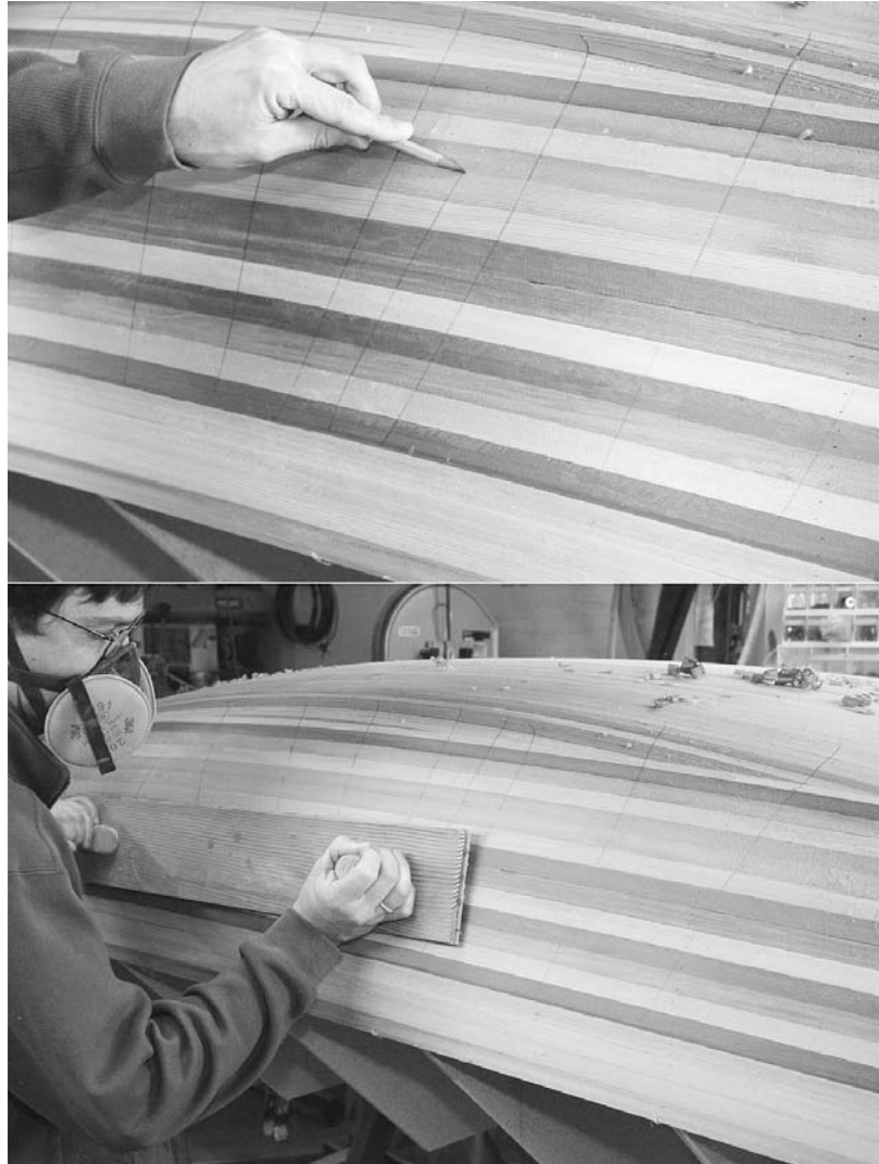
Figure 11-17. To get a fair, consistent surface you want to sand everything to approximately the same degree. You can provide sanding guides by scribbling on the surface with a soft pencil. Do not press hard, and use the side of the pencil point so you don't create grooves in the wood.
