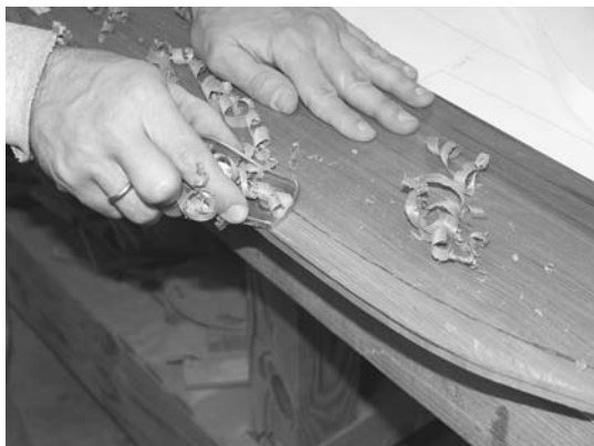
Figure 13-16. The inner stem of the kayak has a gradual curve that can be cut out of a solid piece of wood. Here the stem pattern is traced on western red cedar planed to 1/2 inch thickness. Cut the outer edge on a band saw and then plane both sides to form a bevel back to the back edge line. The result should be a V-shaped edge.
