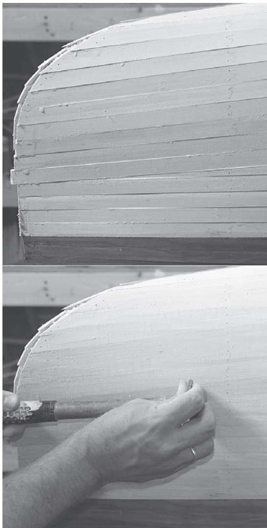
Figure 7-1. Although the scraper is really good at removing glue drips, it can also do a lot of fairing pretty quickly. The scraper needs to be held firmly so it does not chatter and skip.
