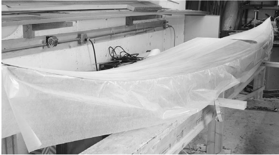
Figure 7-17. With a decked boat you could remove the hull or deck while sanding, staining, or glassing the other half, but often the safest place for it is on the forms. Inserting waxed paper at the sheerline will protect the bottom half as you work on the top.
