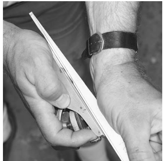
Figure 6-23. Tapers can be planed into the ends of strips using a push or pull stroke. With a sharp plane you may be able to accurately shape some long tapers without support, but as they get longer you may want to back up the strip with another scrap piece.
