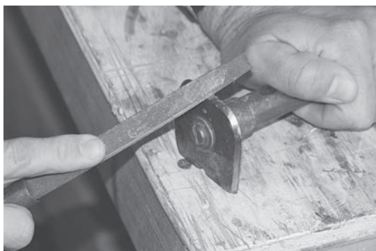
Figure 7-3. A sharp scraper will work much better than a dull one. Use a fine metal file to keep a good edge on it. This scraper has been modified with a variety of different radii and a flat section to conform to various shapes. The outside of most boats would probably do well with just a flat edge, but the inside often has some tight turns.
