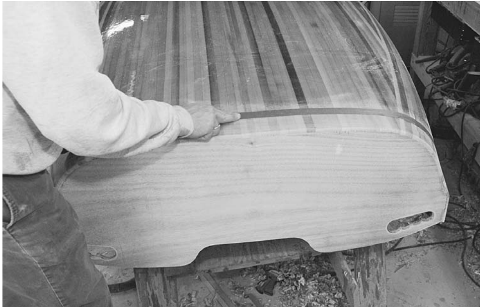
Figure 9-26. After the main body of the deck or hull has been covered with glass, you can come back and cover bits that were hard to deal with on the first go-round, such as transoms and stems. With this transom, I first applied a fill coat to the body of the hull, let that cure, then masked off the stern area before applying a layer of fiberglass to the transom.
