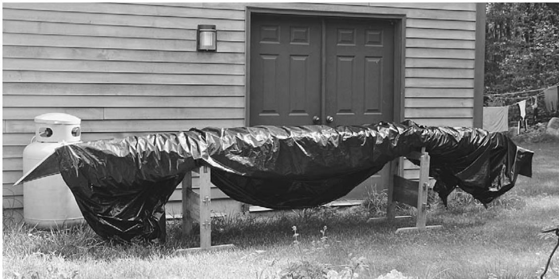
Figure 10-1. Epoxy takes a long time to fully cure even after it is hard to the touch. It continues to get harder as days and weeks proceed. This continued curing could cause the fabric texture to print through. To help reduce this effect and to harden the epoxy prior to sanding, I will often “cook” the boat out in the sun on a warm day. Even on a cool day, wrapping the boat in black plastic can make the boat quite warm. This accelerates the final cure.
