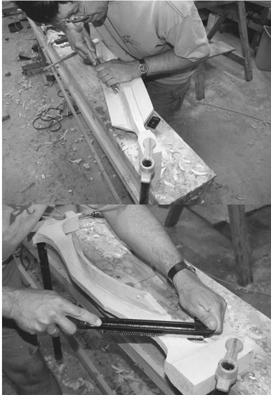
Figure 12-34. I cut the backrest from 2-inch-thick Sitka spruce. The top and bottom pieces were cut as nested pieces from the same piece of wood on a band saw with the table set at an angle. The glued up pieces were shaped with rasps and microplanes.
