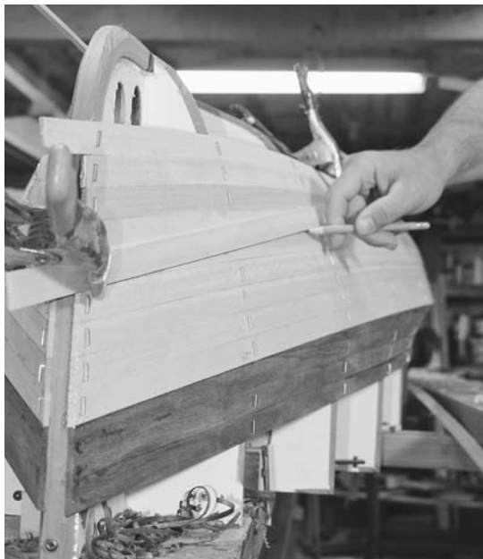
Figure 6-37. To eliminate the buckling, lay another strip over the existing strips in such a way that a minimum amount of force is needed to hold it in place, i.e., almost all the bend is the "easy" way. Clamp the strip in place and then trace the edge onto the existing strips.
