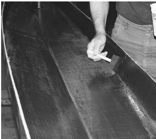
Figure 13-66. All epoxied surfaces should eventually get a coat of varnish or other UV-protective coating. For closed boats you may want to apply this finish to the inside before joining the deck and hull. A satin or matte finish looks good if you leave the fabric texture because it tends to tone down the appearance of the texture whereas a gloss finish highlights the texture.
