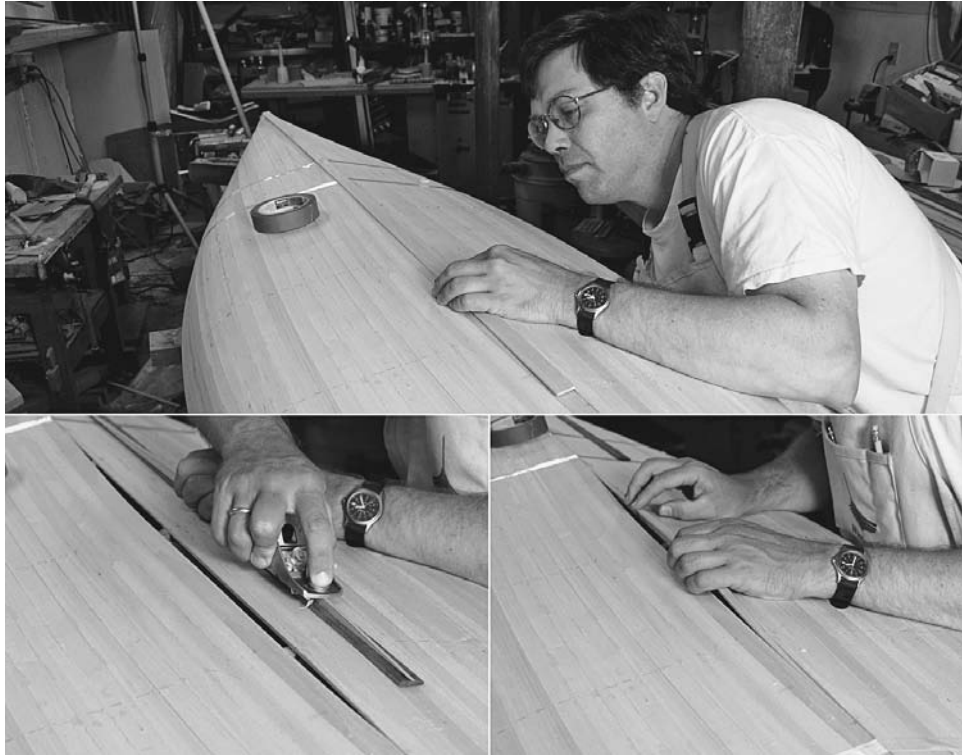
Figure 12-20. Eventually there will be a last strip. Make the edges of the second to last strip, and maybe the third to last strip, square so that you don't need to try to fit the ends down into long holes created by a cove. Place a strip over the hole and reach in underneath to trace the shape of the hole on the underside. Without moving the strip, also mark the location of the ends of the gap on the strip. Bend a scrap strip over the marks you made to indicate the approximate shape of the hole. Either whittle away most of the excess wood or cut it off with a band saw.
