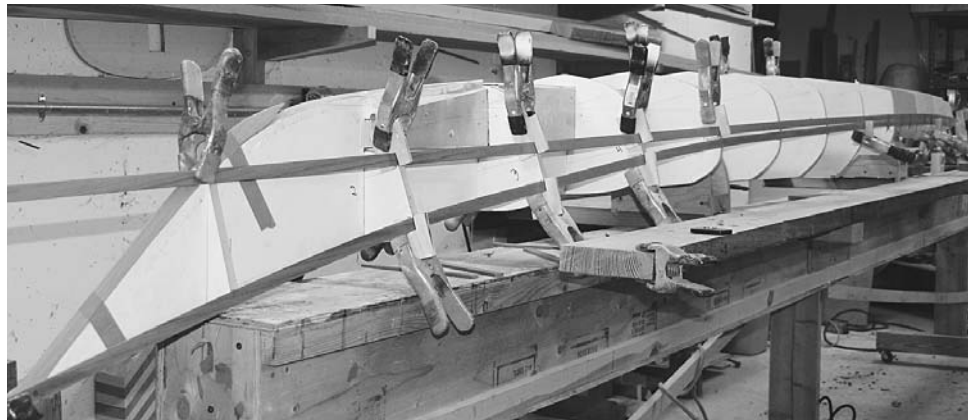
Figure 13-20. The first strip follows the sheerline (bottom strip), and the second follows a more straight line. This second strip actually follows a diagonal line that is parallel to the run of the chine. In this way, by the time you strip up as far as the chine, the strips will approximately follow the chine so the joint with the next strip will be easier than it would be if it went in some other obscure direction.
