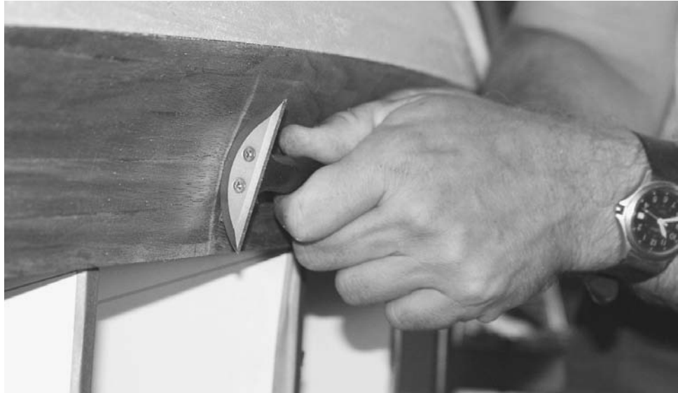
Figure 12-21. Hardwoods such as this walnut respond well to scraping. A quick scraping removes glue drips and starts smoothing the surface prior to sanding. A convex scraper does a good job in the tumblehome area.
