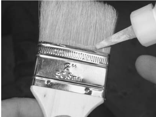
Figure 9-28. Chip brushes are good because they are cheap; that, of course, means they tend to shed bristles. This is usually not a big deal when wetting out the fiberglass because you remove any shed bristles when you squeegee excess resin off the glass, and the bristles become nearly invisible in the epoxy, so any remaining are not offensive. But when you do the fill coats the shed bristles cause drips, sags, and other surface irregularities that are better to avoid. A little CA glue along the top of the ferrule will glue in most of the loose bristles.
