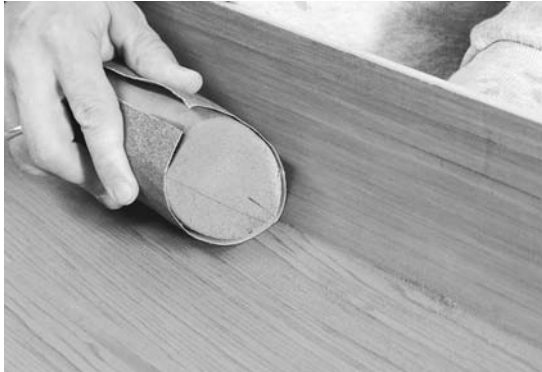
Figure 7-13. A fairing sander does not work well on interior surfaces, but after scraping and planing, you can get a quite fair surface by wrapping sandpaper around a chunk of soft foam or a shaped wooden sanding block with some foam cushion on it.
