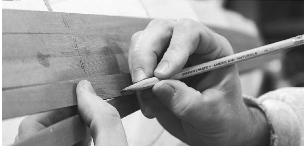
Figure 6-21. Long tapers such as for the cheater-strip area at the ends of a kayak are fitted in the same manner as other tapers. Hold the strip in place with the end aligned with the end of the tapered gap and mark where the new strip overlaps the gap, then whittle off the excess wood and plane the strip to fit. In these gaps the taper is often not a straight line but follows a curve, so the new strip must be slightly concave along its length. A couple of extra strokes with the plane near the middle of the taper is usually enough to create the curve.
