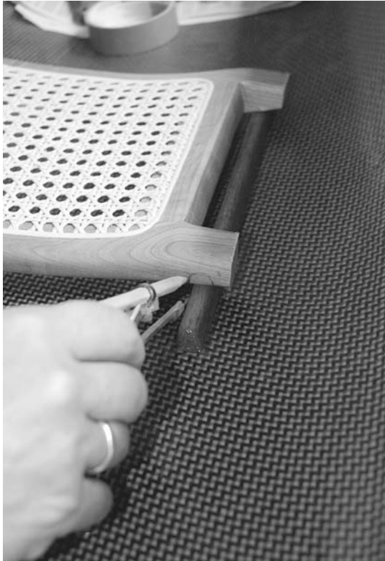
Figure 12-38. With the seat stringer on the bottom of the boat, I wanted to get the seat as low as possible. I notched the cross arms to fit over the stringer, which let it nestle down on the bottom. For a higher-mounted seat, this would not be necessary.
