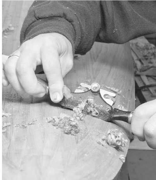
Figure 7-6. A spokeshave does a very nice job of shaping areas that are concave along their length. The goal is not to remove a lot of wood, but to shave off high spots.
