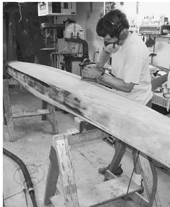
Figure 10-4. Systematically sand the whole surface with 60-grit sandpaper. If you start sanding into the fiberglass, stop and move on. If you are unable to eliminate all the shiny spots before sanding into the glass, apply another fill coat. When you can achieve a smooth and even surface with 60-grit sandpaper, step up to finer grades of sandpaper through 220-grit.
