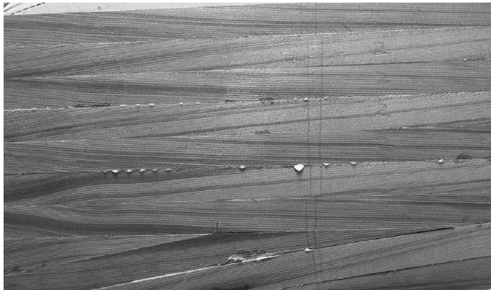
Figure 13-25. When book-matching strips you may want the grain to align across the whole face of the surface. The double line in this image was drawn across all the strips while they were aligned side by side on a workbench. Then they were fit together on the boat using these lines as alignment marks. This example uses an alternating book-matching scheme.
