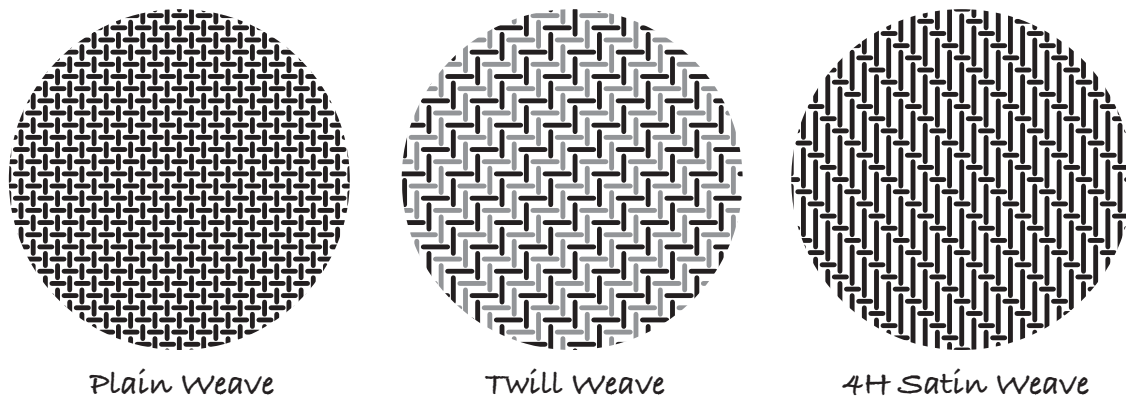
Figure 2-6. Fabrics are produced in many weave patterns. The “over-under-over-under” weave is called plain weave and is most typical. Keeping the yarns over a few extra times, or going under a few yarns before going over, produces fabrics with slightly different properties. The twill weave goes over two and under two. When made with two different yarns such as carbon and Kevlar, the pattern looks a little like houndstooth, with a distinctive repeating pattern. Because the yarns have few bends, there is less stress on the fibers, making them a little stronger. This is also true of satin weave where the yarns are under for several spots and hop over for one. This relatively loose weave is smooth and conforms easily to complicated shapes.
