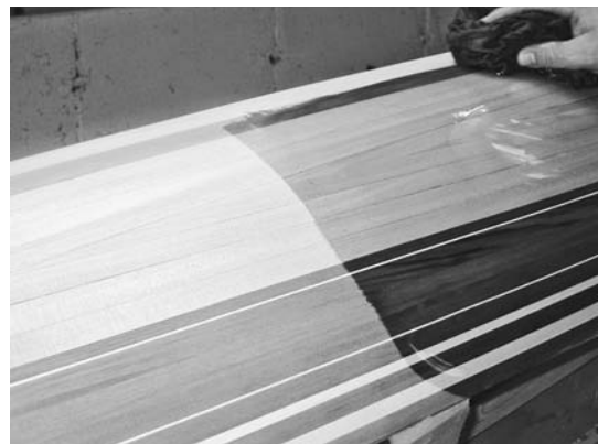
Figure 7-15. When you think you are about done sanding, wipe the whole surface down with a wet rag. This will help clean the surface of dust, highlight any scratches or raised and compressed grain, help point out any leftover glue, and give you your first indication of what the final finished look of the boat will be.
