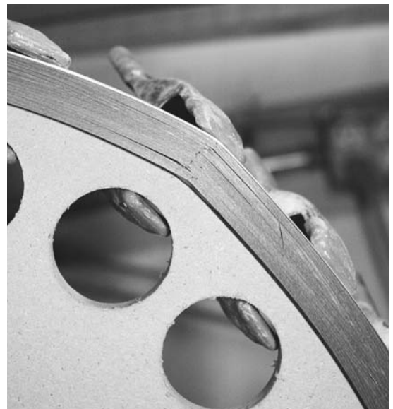
Figure 5-28. If the stem laminations are cut too thick they may break. Cut the next set thinner.
