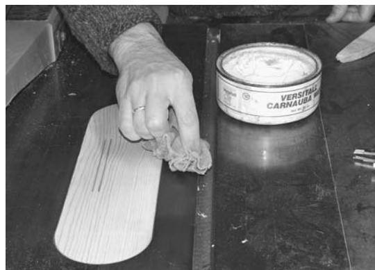
Figure 5-1. Applying some wax to the table of the saw will help material slide, making it easier to cut.
