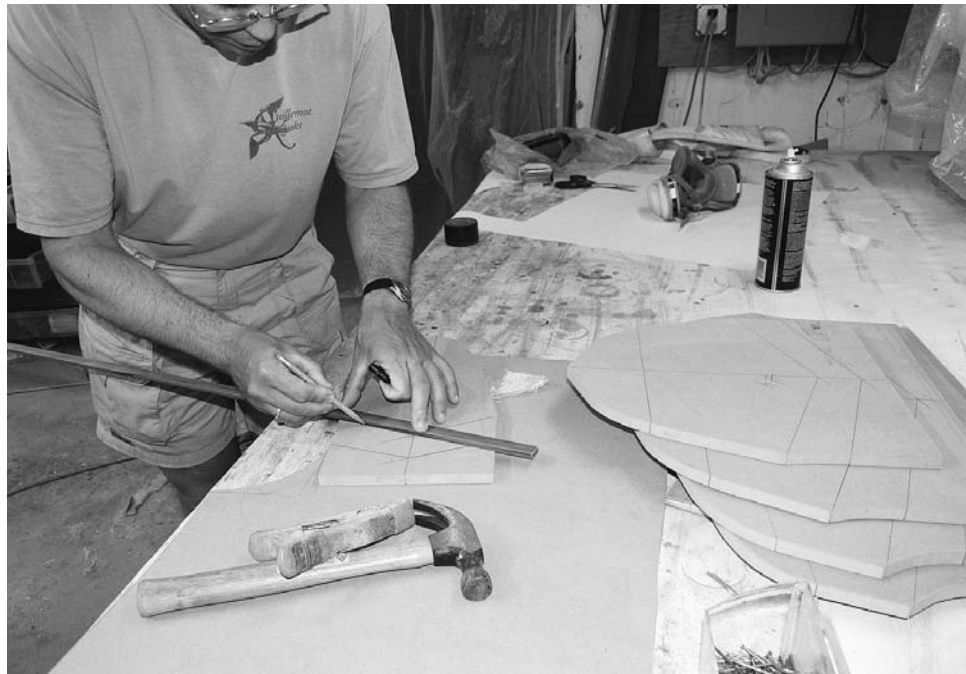
Figure 5-19. If you don't have reference lines on the forms, you should mark them as necessary. In this case I cut the front and back forms of the Nymph at the same time. One set had the original paper patterns with lines; the other set did not.
