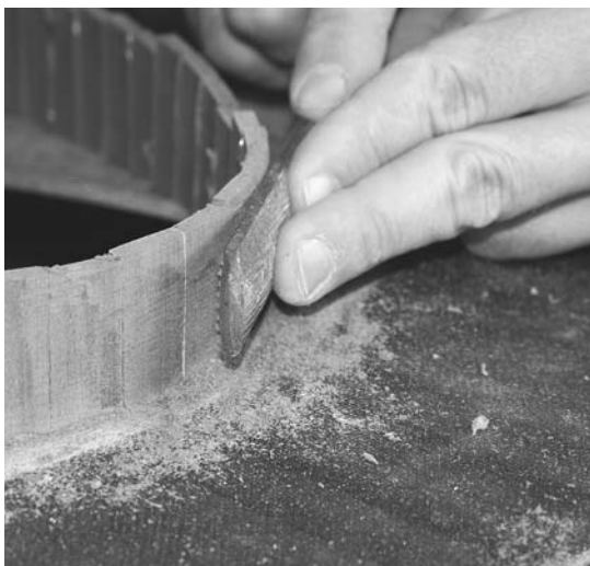
Figure 13-51. Clean up the hot-melt glue that squeezed out between the riser strips with a scraper. There will often be a small bead of glue at the bottom of each strip. This can be cut off with a utility knife. Smooth out the outside of the riser with a rasp and then sandpaper. Since the outside will be partially hidden by the lip, you don't need a perfect surface here. If you want to stain this area, do so after sanding, then paint the outside with epoxy, pipe in dookie schmutz to make a fillet, and apply a couple of layers of bias-cut fiberglass.
