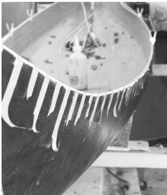
Figure 8-2. Staining some of the wood stains all of it. If you want an accent stripe, it may be easiest to add it after the wood has been stained. Here the outside of the hull has been stained and fiberglassed. I'm applying a thin strip of wood to the top edge, and then I'll glass the inside. I'll glass the outside when I attach the deck.
