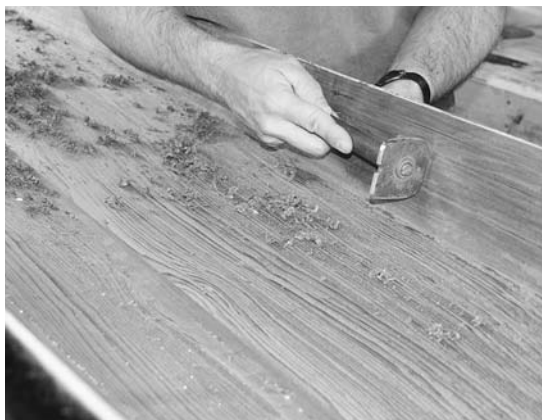
Figure 7-4. Working on the inside you may need to support the sides to minimize the chatter.
