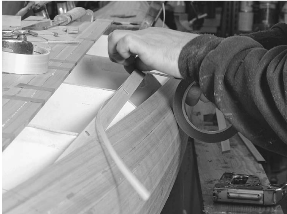
Figure 13-30. The deck has a feature line, or crease, near the cockpit. I wanted the strips to look like they go straight across this crease, but I also wanted to put a light-colored accent strip at the crease. I installed a temporary strip below the feature line to support the ends of the strips above the feature line. I also cut a very thin strip of maple. Here I am temporarily taping this thin strip of wood to the temporary support strip. This will create a light-colored strip in the finished boat. As I fill in the strips above the feature line, I will glue their ends to this maple piece, removing the tape as it gets in the way. After I have finished filling in above the feature line I will remove the temporary support strip and fill in below. The thin maple strip will remain in place.
