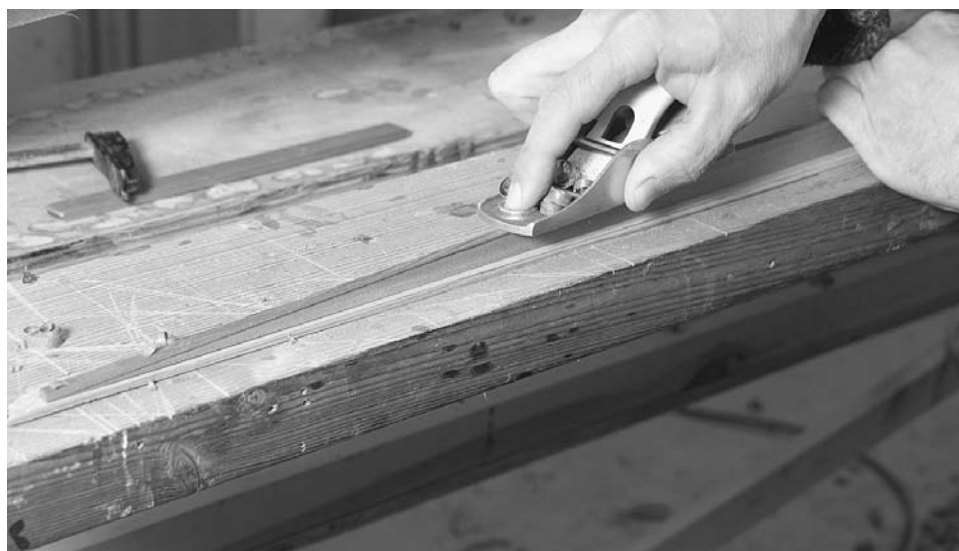
Figure 13-26. With long tapers you will likely need some support for the strip as you plane to assure an accurate joint. Here I am using the plank work surface mounted adjacent to the forms. A scrap strip supports the strip I am working on so I don't run into the table as I thin down the tip.
