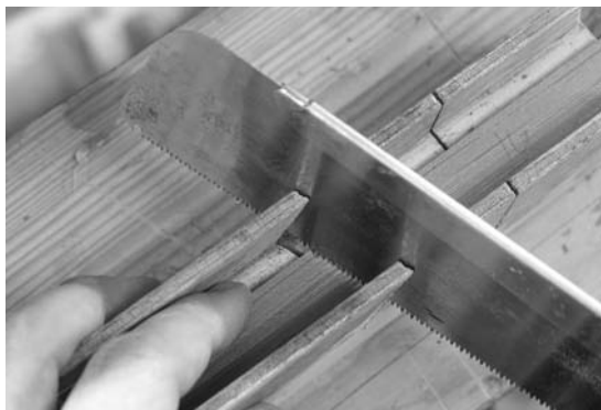
Figure 13-21. If you need to make a lot of butt joints, a little miter box will provide accuracy and consistency. I just took a block of pine a little wider than the strips, glued scrap plywood to the sides, and then cut a slot. Angle the cut across the box and also vertically. The specific angle is not very important as long as you use the same slot every time.
