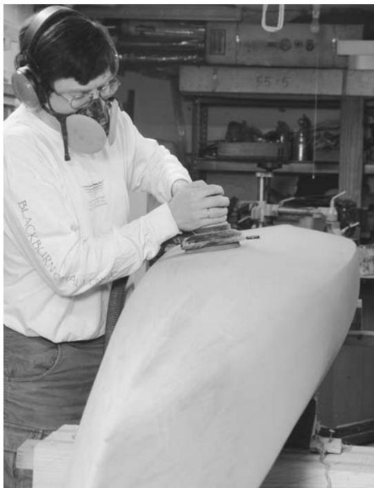
Figure 7-11. Hold your random orbital sander flat against the surface and keep it moving. Don't try to concentrate on one stubborn spot by angling the tool or stalling in one place.
