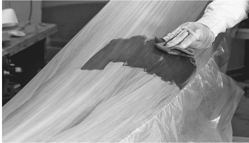
Figure 13-44. Non-oil-based stains are often very quick drying. To get a smooth, even color you need make your rag quite wet with stain. If your rag becomes dry it will not fill up the grain and the stain will become blotchy. Move quickly, continuously rewetting your rag. You may be able to even out the color by wiping it all down with a rag soaked in a suitable solvent. Two coats of stain will result in more even coverage, but will be darker. Let the stain dry thoroughly before flipping the boat over to stain the other side. Here I am staining right over the accent stripe. I will clean the stain off in the next figure.
