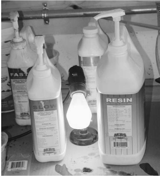
Figure 9-1. Epoxy suitable for fiberglassing usually comes in large containers with calibrated pumps to help measure out the proper ratio. Keeping the resin warm will reduce the viscosity, allowing it to wet out the cloth more easily.
