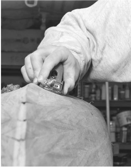
Figure 7-5. This modified block plane has a slightly radiused sole that works well for fairing out sections near the stem.
