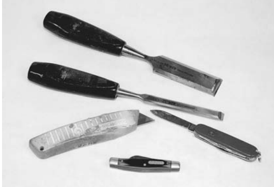
Figure 3-2. The tool I use the most fits in my pocket. The little Swiss Army knife shapes most of my strips. The pocketknife below it works almost as well. A replaceable-blade utility knife has a variety of trimming uses but is not as good at shaping strips. A couple of chisels are useful for shaving down high spots.
