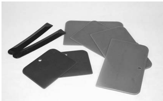
Figure 3-10. I use plastic applicators or squeegees to spread epoxy and remove excess resin from the cloth. Larger ones get the most use, but small ones are good for small areas. I use the little plastic mixing sticks on the left like a putty knife to smooth small spots or fillets.
