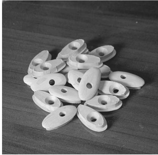
Figure 13-65. Sea kayaks typically have deck lines of shock cord to hold items such as water bottles on deck. For this boat, I ran the shock cord up through holes in the deck. To protect the end grain of the strips exposed by these holes, I created feed-through fittings. I made a pile of these feed-through fittings with a plunge router, a template, and router inlay bushing. I cut the outer shape with the sleeve off the inlay bushing, drilled a hole through the middle, and then cut the part of the board, leaving a ledge on the bottom. After cleaning these up on the sander, I taped the template securely to the deck, put the sleeve on the bushing, and cut a hole in the deck. The parts are pushed through from the inside, glued in place, sanded smooth, and then glassed over.
