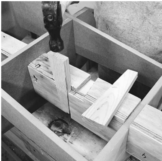
Figure 5-24. These wedges push all the forms tightly against the L spacers and the end forms. If you are gluing the strips to the forms to avoid staples, you can remove the wedges to break the shell free from the forms, then reinsert the wedges to return the forms to their proper location. (Note: Ignore the longitudinal forms shown in this picture; they were not used.)
