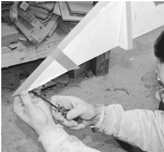
Figure 5-30. Secure the inner stem with tape and maybe a screw. Make sure the screw is accessible so it can be removed. Remove the tape before stripping over it.
