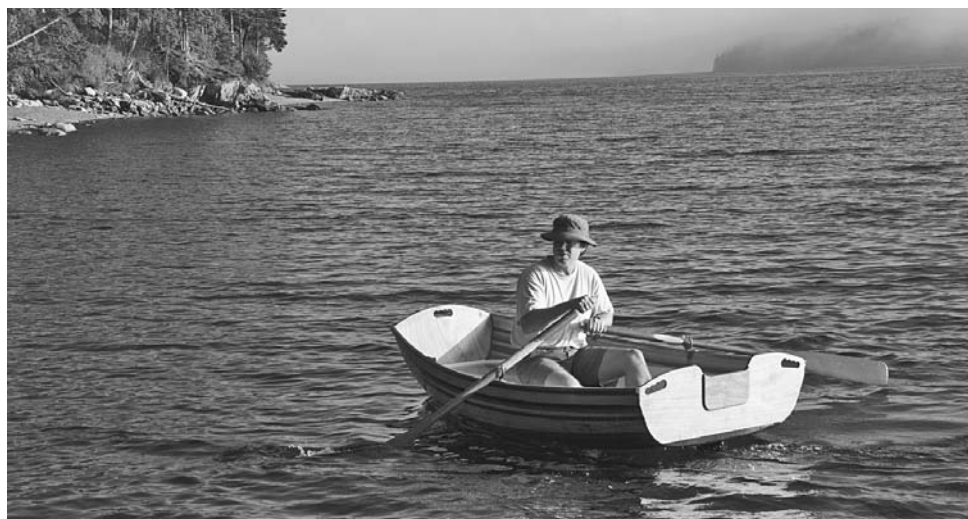
Figure 11-1. The Coot is a small dinghy or tender. The pram style with transoms at both ends makes it an easy boat to strip, and it is a suitable strip-building 101 project. A pram is a small rowing boat with squared-off ends, or transoms, at both ends. Having a transom at both ends gives you a short boat with a lot of capacity and stability, which makes it a very practical tender for a larger boat or yacht. Although I don't get into it here, it can also be easily adapted for sailing and would make a great first sailing boat for a child.
