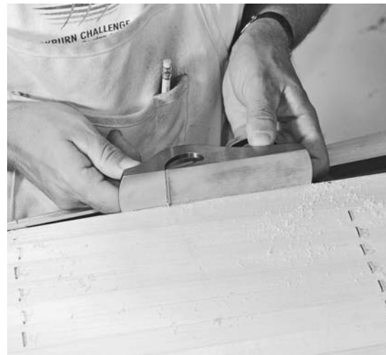
Figure 6-35. A rabbet plane can get in tight with the forms, allowing you to clean up the edge well.
