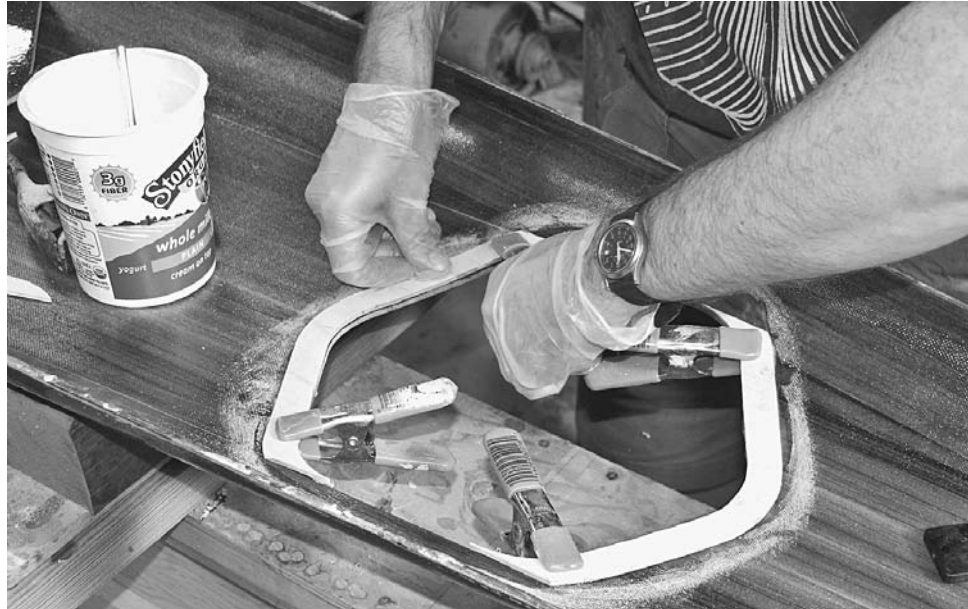
Figure 13-62. The hatches need a spacer between the lip and the deck to allow for a gasket. The spacer is set in epoxy thickened with colloidal silica to make a mayonnaise-like glue. Try to clean up any squeeze-out while the glue is still wet. After the glue has set, clean up the inside edge of the hole.
