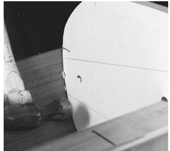
Figure 6-18. If you have not applied too much hot-melt glue during your staple-free construction, you should be able to break the glue free with a sharp rap of a hammer. The forms need to be released from the strongback enough that they can move without breaking.
