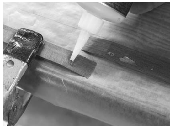
Figure 6-3. If you have the time, you can use carpenter's glue and a clamp to glue the scarf joint. Be sure the strips are aligned in a straight line; it is easy to have one end go off at a funky angle. For a quick joint, use CA glue. Spread glue on one surface, then spray the other with accelerant. Carefully align the ends and press the pieces together.
