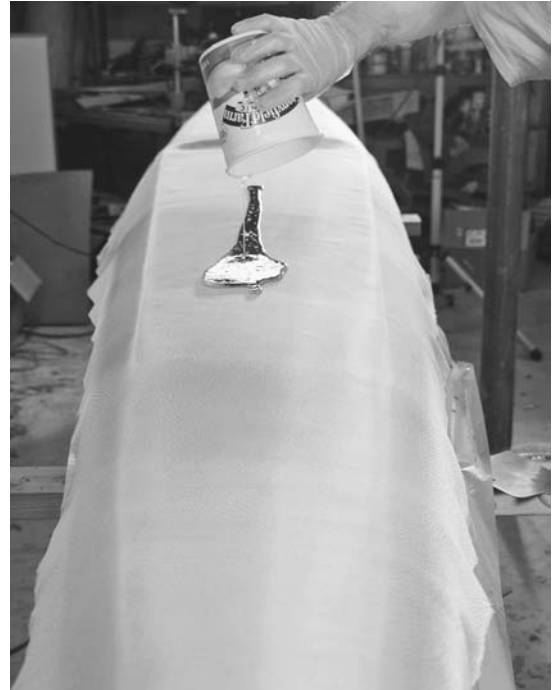
Figure 9-2. Once the epoxy is mixed, the chemicals start doing their thing. The longer they are in a concentrated mass the faster they will react. Dumping your mixing pot onto the boat quickly will slow down the reaction, giving you more time to work.
