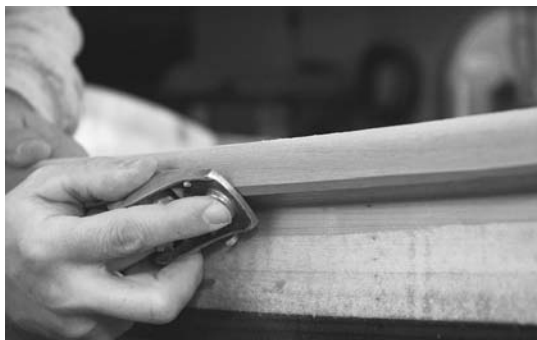
Figure 11-35. The edges of the outwale all start out with sharp corners. First plane down the exposed strip along the top edge so it is even with the outwale. Then use a round-over router bit to give the top edges a radius. The bottom is not at 90 degrees to the outer edge, so a standard round-over bit doesn't do the job. Instead, round it over by hand with a block plane. First create a wide chamfer, then knock the corners off the chamfer and sand it all smooth.
