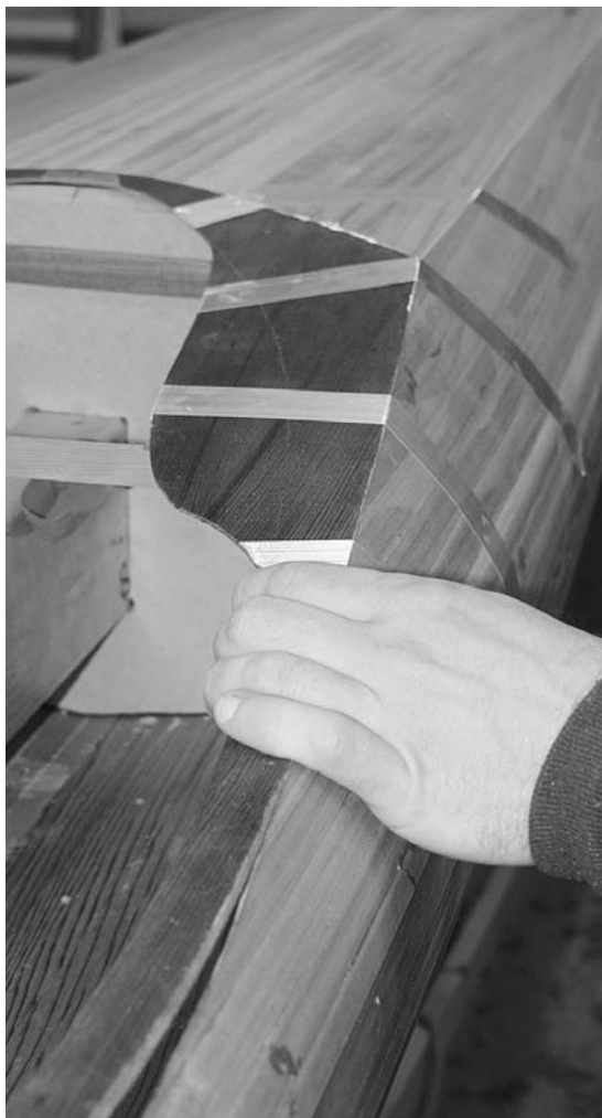
Figure 13-42. Apply glue to the edge of the recess assembly and secure it in place with strapping tape.
