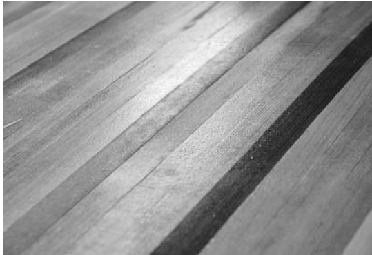
Figure 9-4. Wood will absorb the seal coat at different rates depending on grain orientation and other factors. Don't worry that some spots look dry (dull) and others wet (shiny). This is OK. Once the epoxy has cured it will seal the wood from absorbing more resin.
