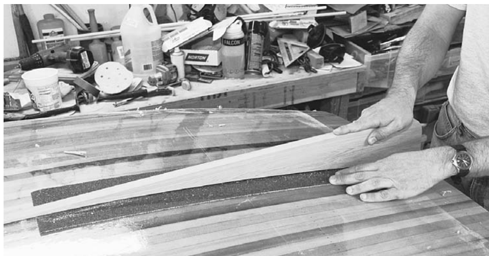
Figure 11-37. Such a short boat needs a little help going straight. A short keel at the stern of the boat, sometimes called a “skeg,” provides this directional stability. Cut a skeg out of some 1/2-inch plywood or 3/4-inch solid lumber to the approximate shape. Then lay a long piece of sandpaper on the spot where the skeg will be installed and rub it back and forth to create a tight seam. Round off the exposed edges of the skeg with a 1/4-inch-diameter router bit.
