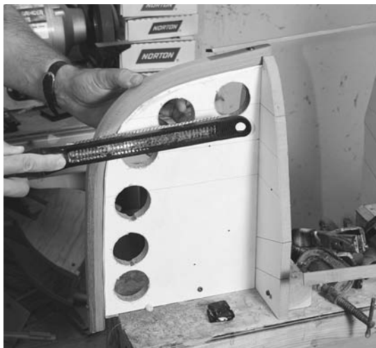
Figure 12-12. Use a rasp or plane to bevel the edge of the inner stem. Aim the rasp toward the edge of the next form as a guide to getting the angle right.
