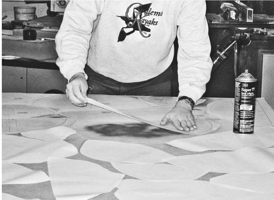
Figure 4-3. Instead of transferring lines from the drawing to your form material, cut out full-size drawings, glue them to the form material with spray adhesive, and cut out around the lines. This way all the reference lines are included on the forms.
