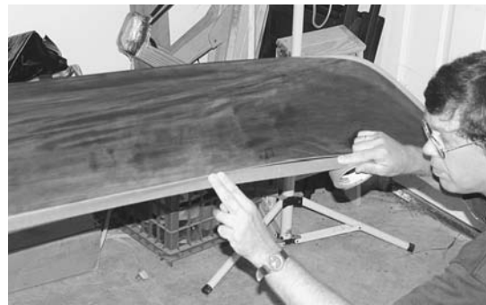
Figure 10-7. Mask off the lower edge of any area to be varnished to control any drips that may accumulate. Fold up the bottom edge of the tape to create a drip edge. Varnish the hull about 1 foot at a time, switching sides every 2 feet so you maintain a wet edge along the centerline. Remove the tape a minute or so after you have finished varnishing. Let the varnish dry, and then flip the boat over and repeat for the deck.
