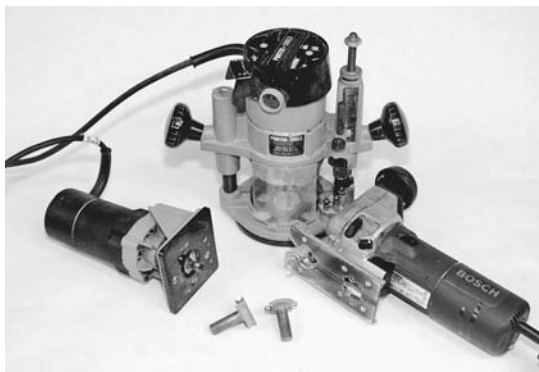
Figure 3-13. Some other useful power tools include routers and jigsaws. The large router in the middle is mounted in a plunge frame that can be used to make some specialty parts. Mounted to a table it can be used to mill cove-and-bead strips with the cutter bits shown below. The trim router on the left is useful for rounding over gunwales. The jigsaw on the right does a good job cutting hatches.
