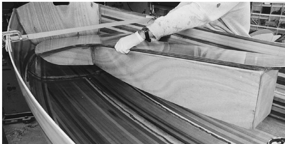
Figure 11-33. Install the seat assemblies on a bead of dookie schmutz. First prepare the boat surface by sanding the mounting area. Dry-fit the seats and draw the exact locations on the hull with a pencil. Place masking tape about 1/2 inch away from all the mounting points to contain any squeeze-out and a later fillet.
