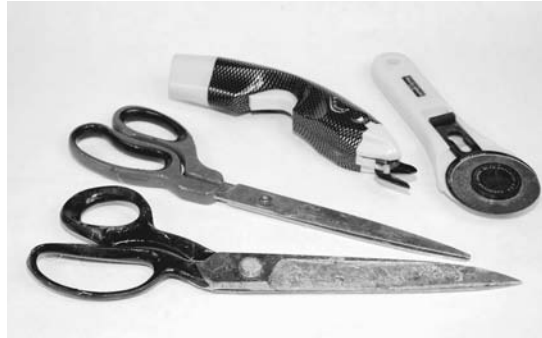
Figure 3-9. Fiberglass is usually cut with scissors. They will likely get coated with epoxy, and cutting glass dulls them, so don't go to the sewing kit thinking no one will notice. Second from the right is a battery-powered fabric cutter that may be worth the investment if you do a lot of fiberglass work. If you have a smooth surface to cut on, the rolling cutter on the right works well for cutting strips of cloth.
