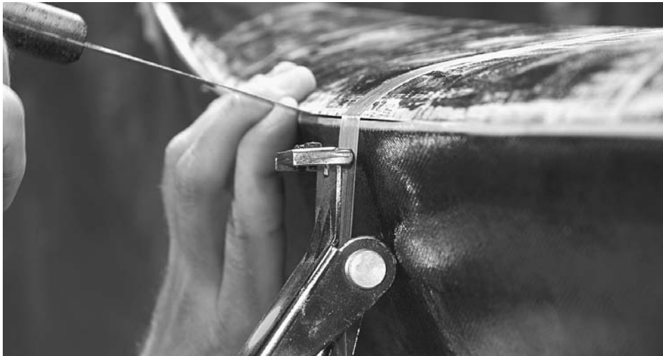
Figure 13-68. Align the rest of the deck-hull seam dry without any adhesive. Then hold it in place with strapping tape. (Fold over the free end of the tape on the roll so that when you peel off the tape you have something to grab.) If the deck does not align perfectly you can usually use hand pressure to push it into place; otherwise, slide a putty knife into the seam to lever it into alignment. Friction between the deck and hull keeps them in place; getting a lot of tension on the tape creates this friction. A tape dispenser with a cutter on the end will help you achieve this tension. Pull down hard on the packing tape as you align the seam, and press it down onto the hull securely before cutting it off the roll.
