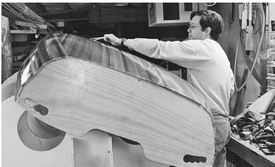
Figure 11-21. The width of this boat makes it difficult to get off the forms. Attach a loop of tape as a handle to get a grip on the boat if you are working alone. This is one of those times that having some extra help would make your work easier.
