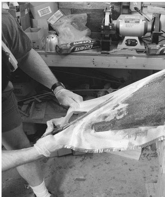
Figure 9-17. Most wrinkles need to be moved toward the ends of the boat. Depending on the shape of stem, you may need to trim the glass at the ends. While it is possible to wrap the trimmed glass around either side, I find it easier to let it come off straight and then trim it off later.
