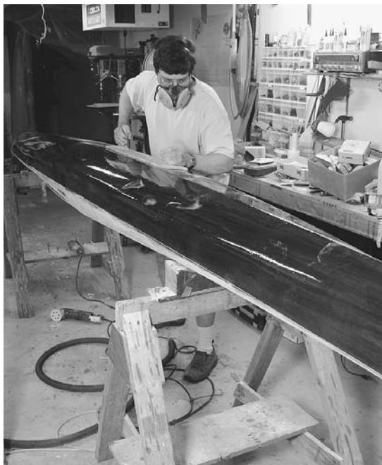
Figure 10-3. The fairing sander is an effective tool for leveling out any irregularities introduced in the fiberglassing and fill-coat stages of building.
