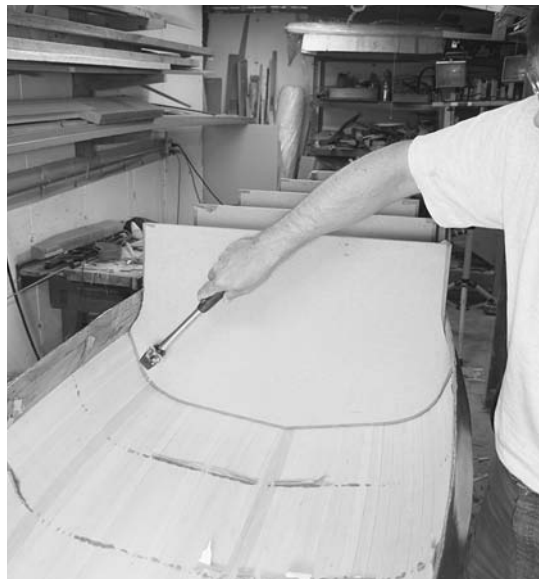
Figure 7-18. The staple holes will often wick a little epoxy onto the forms. This is why the forms have tape on the edges, but sometimes you may need a little persuasion to get the boat off. Some light raps with a hammer usually do the trick.
