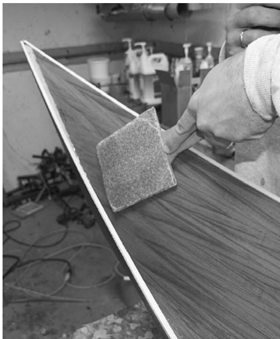
Figure 7-9. The sharp ends of the boat can be tough to reach to clean up. I glue some sandpaper to a paddle made of plywood to help me reach the tight spots.
