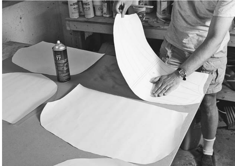
Figure 12-6. Each form is drawn out full size. These patterns are laid out on MDF, glued down with spray adhesive, and then roughly cut out with a jigsaw.
