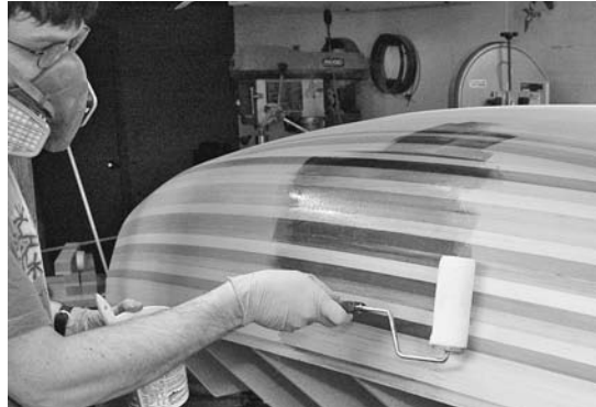
Figure 9-3. A seal coat limits how much epoxy is absorbed later when applying fiberglass. Brush on a little epoxy, then spread it around with a roller. There should be no need to thin the epoxy. The seal coat is not a requirement, but it does make the later coats that wet out the fiberglass a little bit easier to accomplish.
