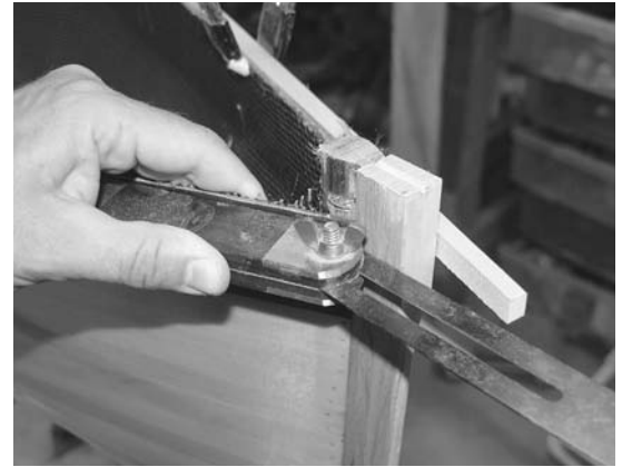
Figure 12-30. I extended the outwales onto the stem by tapering the ends. Use a bevel gauge to transfer the angle to the outwales.
