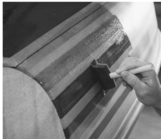
Figure 10-10. Varnish provides UV protection for the epoxy. You want at least three coats to be sure there is enough coverage. Mask off areas where you do not want varnish. In this case I did not want to varnish over the graphite powder-epoxy bottom. The varnish will flow slightly down the side. A line of tape on the gunwale keeps this flow from creating drips along the edge. Get the upper side when you turn the boat over to varnish the inside.
