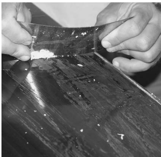
Figure 10-2. A cabinet scraper does a good job of leveling small irregularities. It can be used with a lot of precision to knock down a small drip. Larger drips can be attacked with a rasp or paint scraper.
