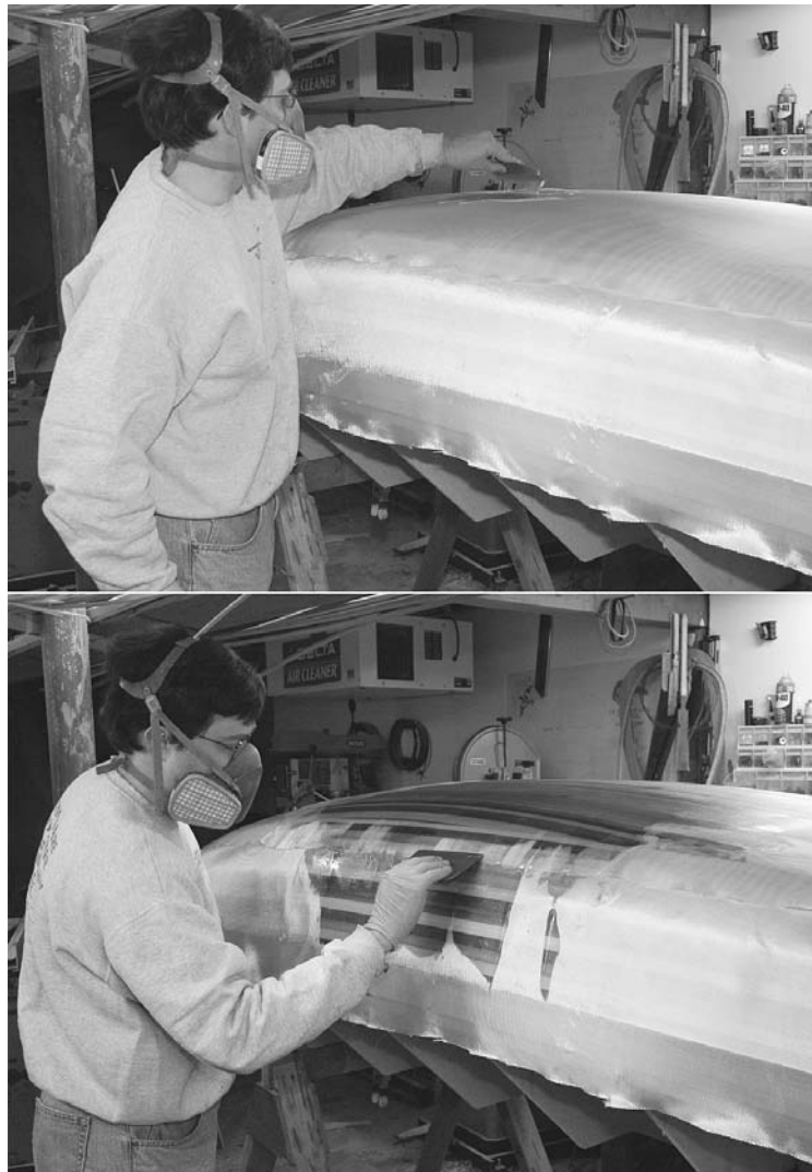
Figure 11-19. Cover the boat with 6-ounce fiberglass. The two layers on the bottom will soak up quite a bit of resin. Pour a puddle of epoxy on the bottom and spread it around with a squeegee. Work from the middle, down the sides, and then out toward the ends.
