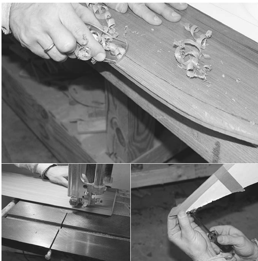
Figure 5-26. Boats with largely straight bow and stern shapes can use solid wood inner stems. If your plans include the pattern for the inner stem, use the pattern to mark the outer line. Cut to this line, then mark the bevel line. Bevel on both sides as far back as the bevel line. Cut the stem off the piece of wood and tape it onto the inner stem.
