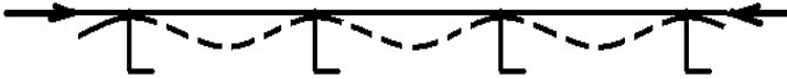
Fig. 12.7 Plate panel stiffened with high torsional rigidity stiffeners loaded with in-plane compressive stresses orthogonal to the longitudinal
