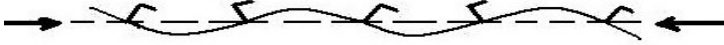
Fig. 11.4 Mode of deformation of a transversely stiffened panel under in-plane loading, the stiffeners has low torsional rigidity
