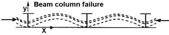
Fig. 11.8 Mode of deformation of a stiffener under in-plane compressive stresses, (beam column failure)
