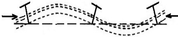
Fig. 11.9 Mode of deformation of a stiffener under in-plane compressive stresses, (low torsional rigidity of the supporting members)
