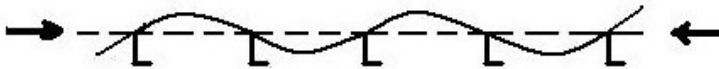
Fig. 12.18 Mode of buckling of transversely stiffened plate panel when the stiffeners have large torsional rigidity
