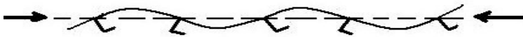
Fig. 12.8 Plate panel stiffened with low torsional rigidity stiffeners loaded with in-plane compressive stresses orthogonal to the longitudinals
