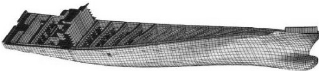
Fig. 5.22 Open deck container ship hull girder torsional deformation
