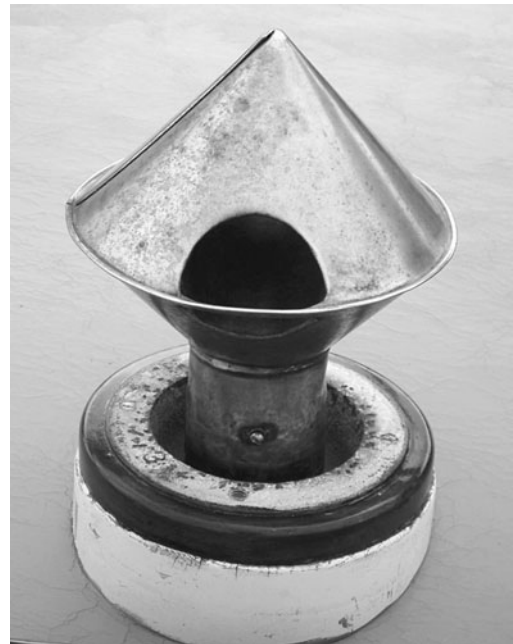
Figure 15-7. Smokehead with water-iron deck ring
