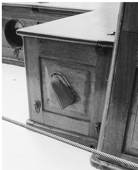
Figure 14-13. Clamshell vent on a locker
