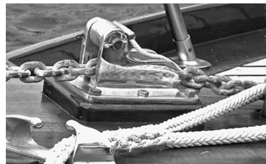
Figure 24-21. Close-up view of chain stopper
