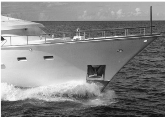
Figure 24-16. Anchors in hawsepipes (Courtesy Hargrave Custom Yachts)
