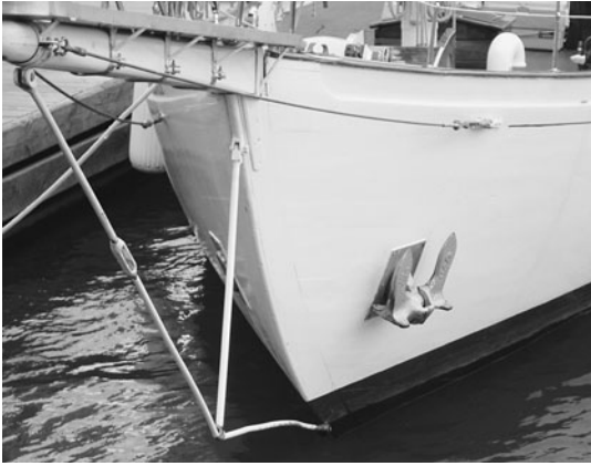
Figure 24-15. Bobstay damaged from anchor chain
