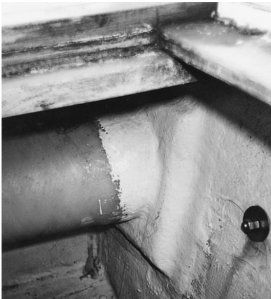
Figure 7-7. Exhaust tube glassed to transom—not a good idea
