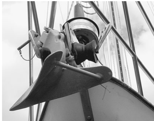
Figure 24-5. Bent and broken anchor roller (Courtesy Chris Wentz)
