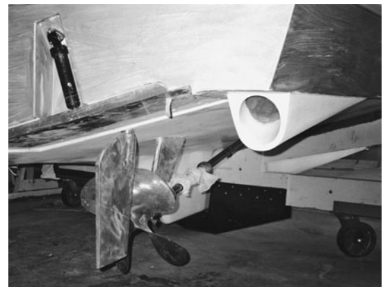
Figure 7-27. Exterior view of the Cape Dory's underwater exhaust system
