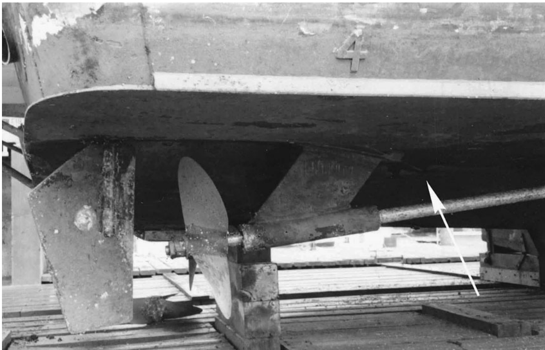
Figure 1-8B. Pocket viewed from starboard. The arrow indi- cates the forward end of the tunnel, which is too short on this boat
