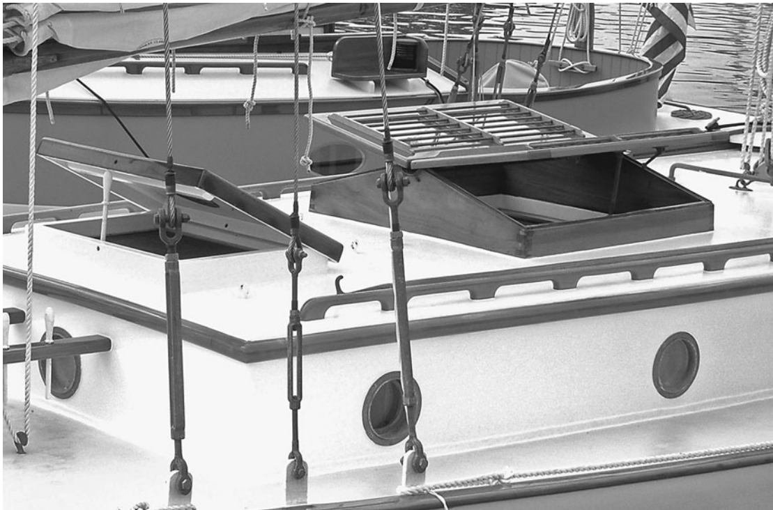
Figure 14-7. Open hatches and skylights provide plenty of vent area
