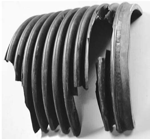
Figure 9-12. Flexible bellows failure from stress corrosion (Courtesy Applegate Industrial Materials, Inc.)
