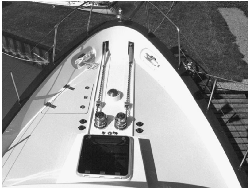
Figure 24-11. Twin vertical windlasses and anchor rollers
