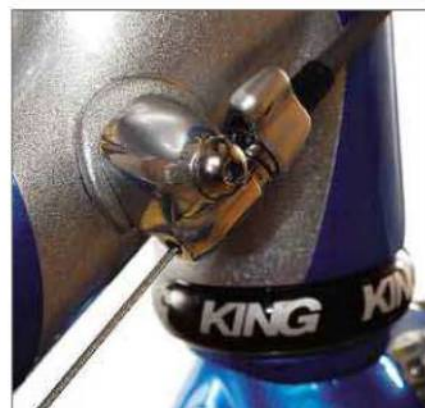
Shimano adjusters have a lever that can be turned to micro-adjust the gears as you ride. Seeing as most frames come without the standard-type bosses, these adjusters are becoming rare.
