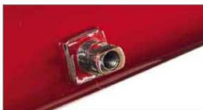
Gear-adjusters are attached to most older frames via a brazed on boss.
