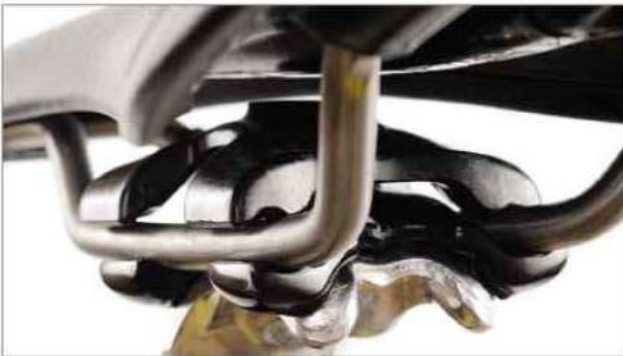
The saddle clamp is in two halves – one holds the saddle to the post and the other adjusts the angle of the saddle.
