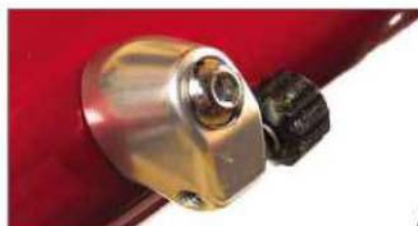
Campagnolo gear-adjusters rely on knurled-threaded adjusters with a spring under them to hold them in place – these do require cleaning and lubricating with a light oil to keep them easy to adjust.
