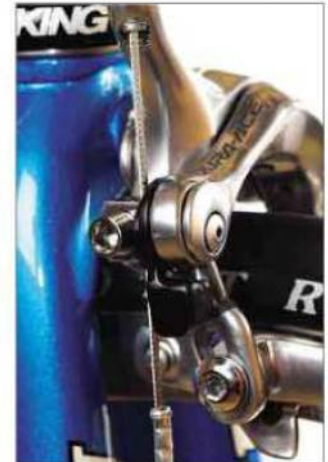
Shimano brakes use a small lever on the brake itself, next to the fixing bolts.
