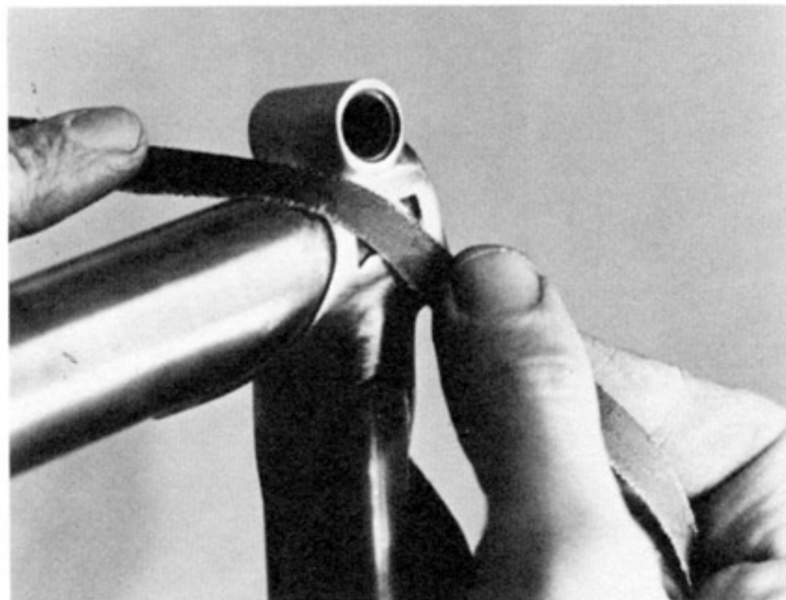
P8.36 Contours are finished with narrow strips of production cloth.
