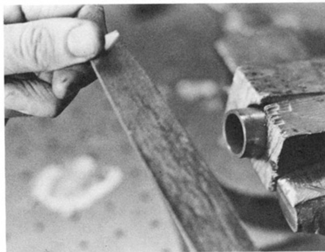
P7.3 Filing the steering tube OD to fit the crown hole. Note tube blocks.
