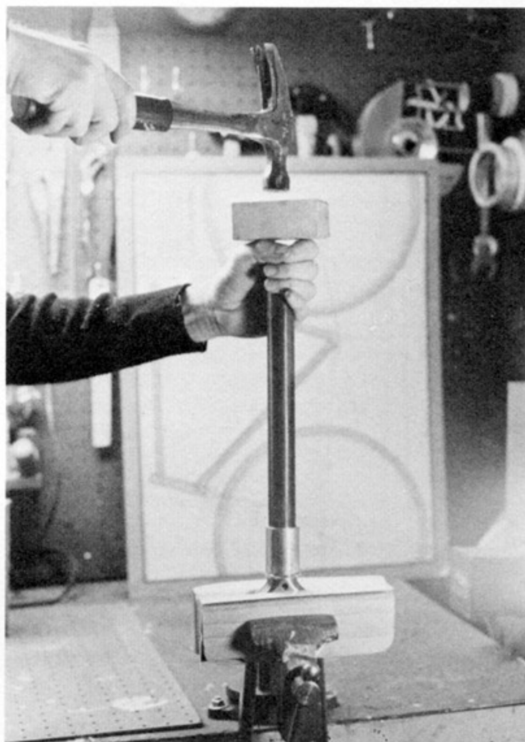
P10.25 Setting the crown race. Lower tube is a short piece of soft aluminum conduit which is used to prevent damage to the race surfaces.
