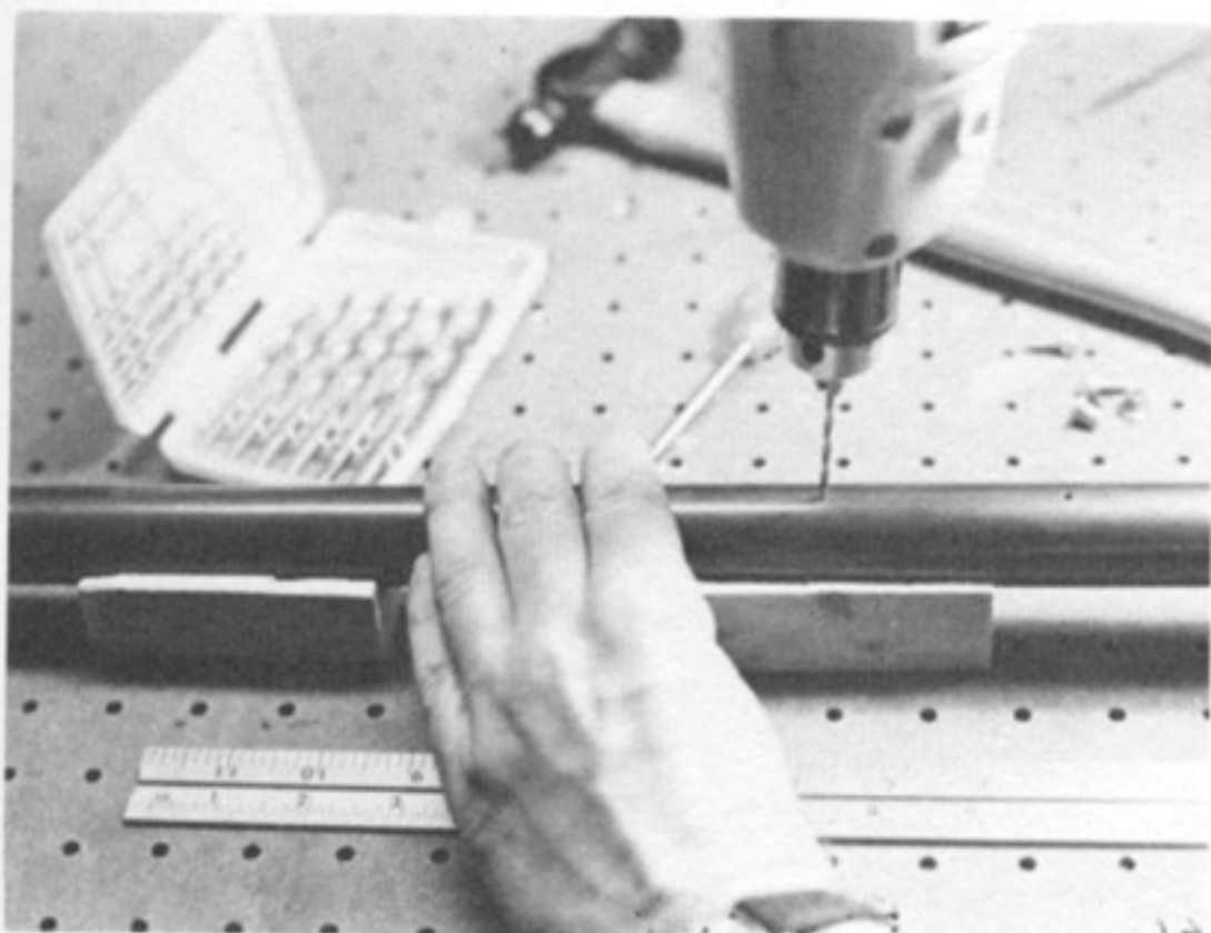
P9.32 Drilling cage nut holes. Note use of tube blocks for support.
