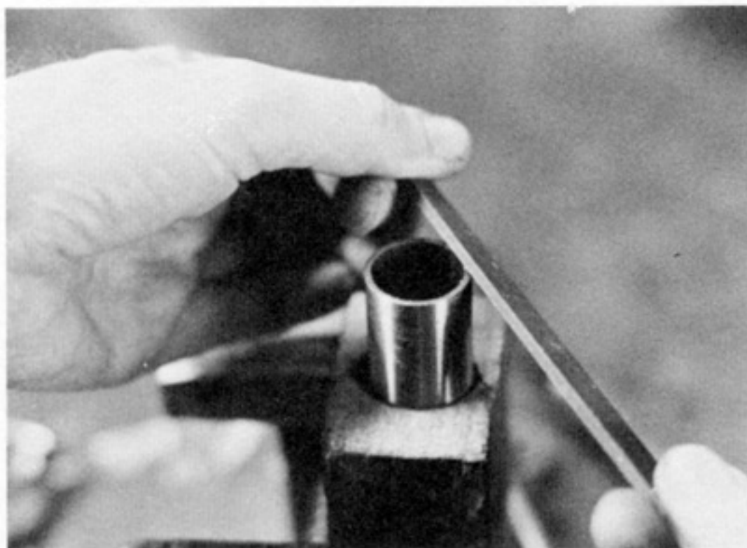
P10.34 Chamfering the end threads.
