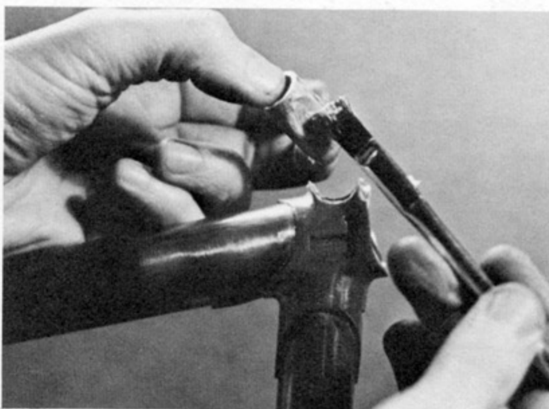
P8.33 Fluxing the bolt tube.
