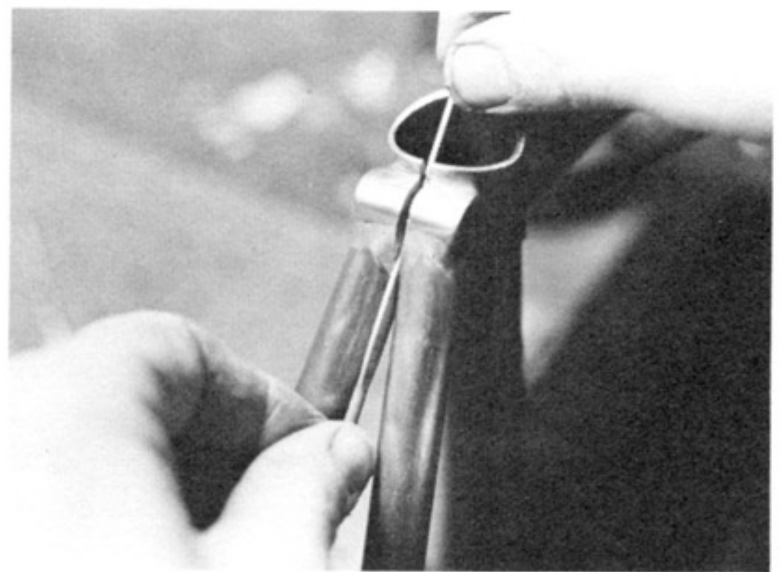
P10.2 Widening the slit with a warding file.
