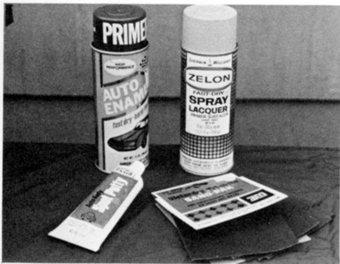
P11.1 Surface preparation and priming supplies. Spray cans of primer (left) and primer/surfacer (right), body putty, and assorted "TRI-M-ITE" papers.
