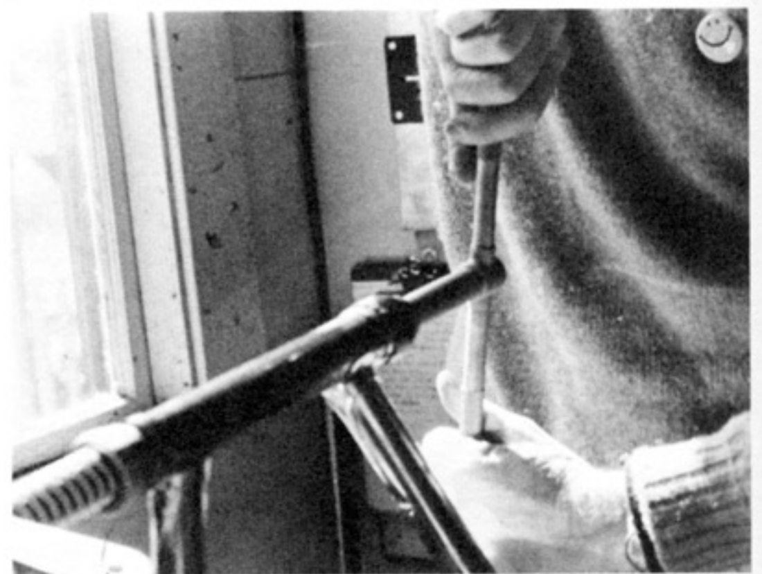
P10.14 Maintain even pressure to keep the tool cutting.
