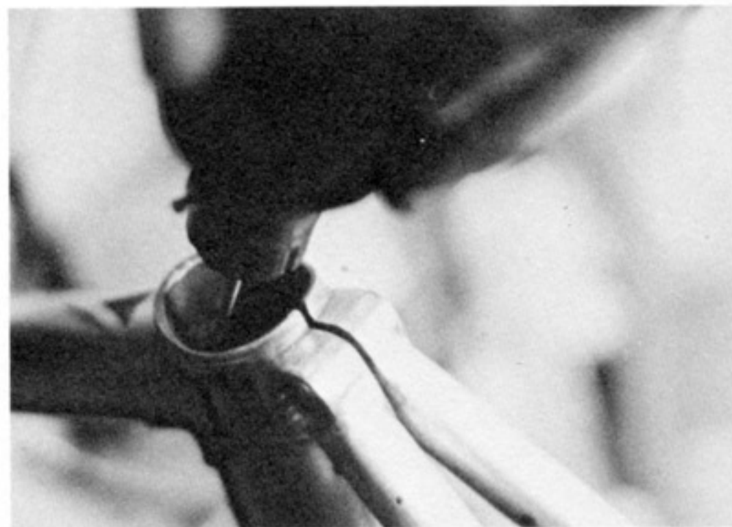
P10.5 Special operation for "concealed" brake conduit design. A slot is cut in the seat tube wall to provide passage of the conduit. Seat post must be similarly slotted in this type design.
