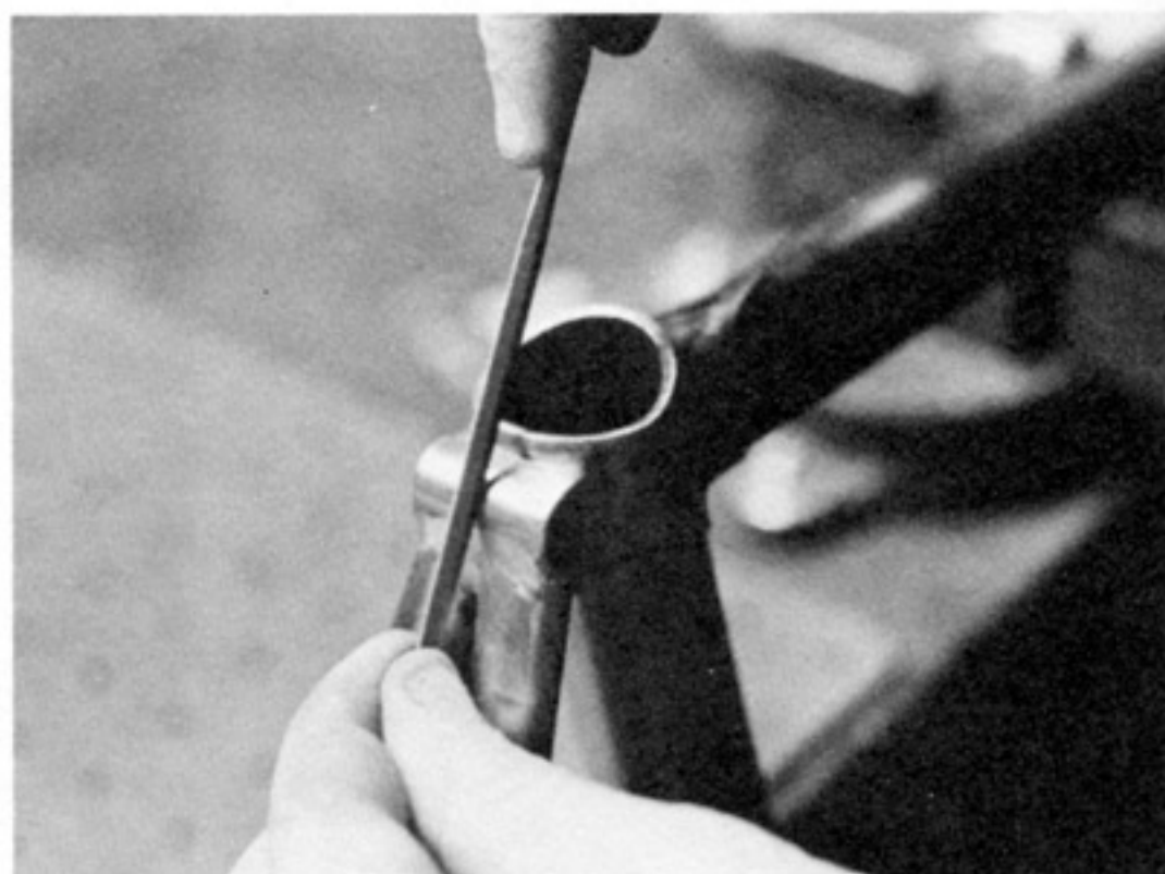
P10.4 Finish-contouring the seat attachment.
