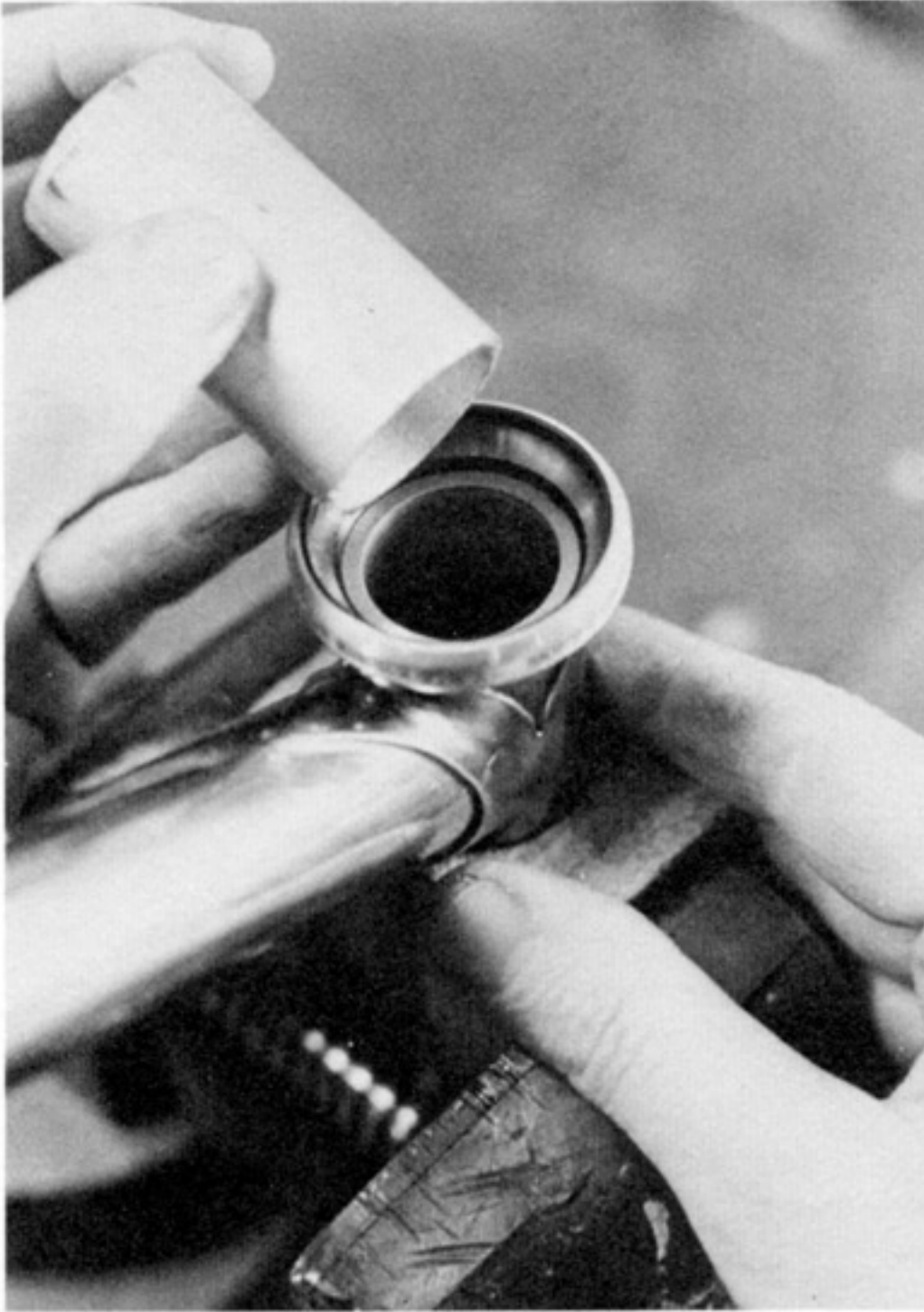
P10.19 Preparing to install the bottom head race.
