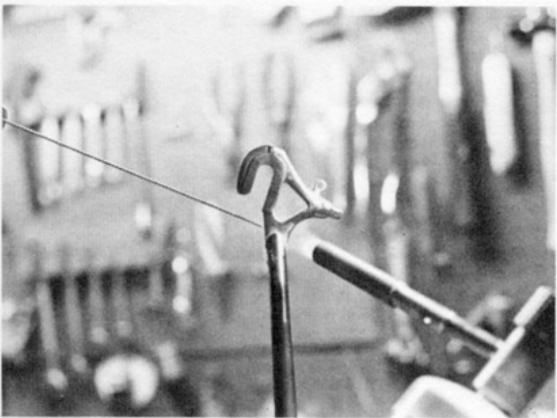
P9.6 Brazing a drop-out to a chain stay.
