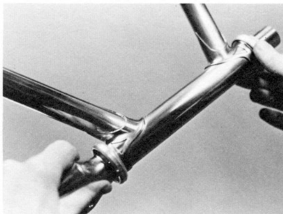
P10.26 Assembling the fork to the frame.
