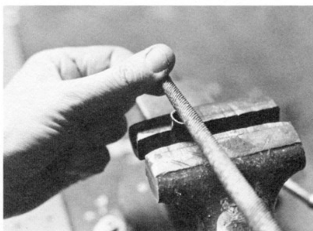
P9.10 Stay ends are contoured to fit the bottom bracket shell's ID.
