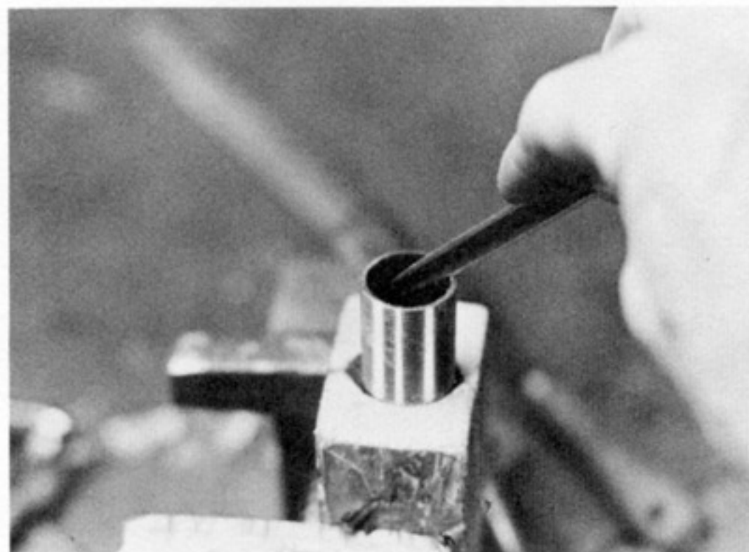
P10.35 Using a machinist's scraper to de-burr the tube ID and clean up the end threads.
