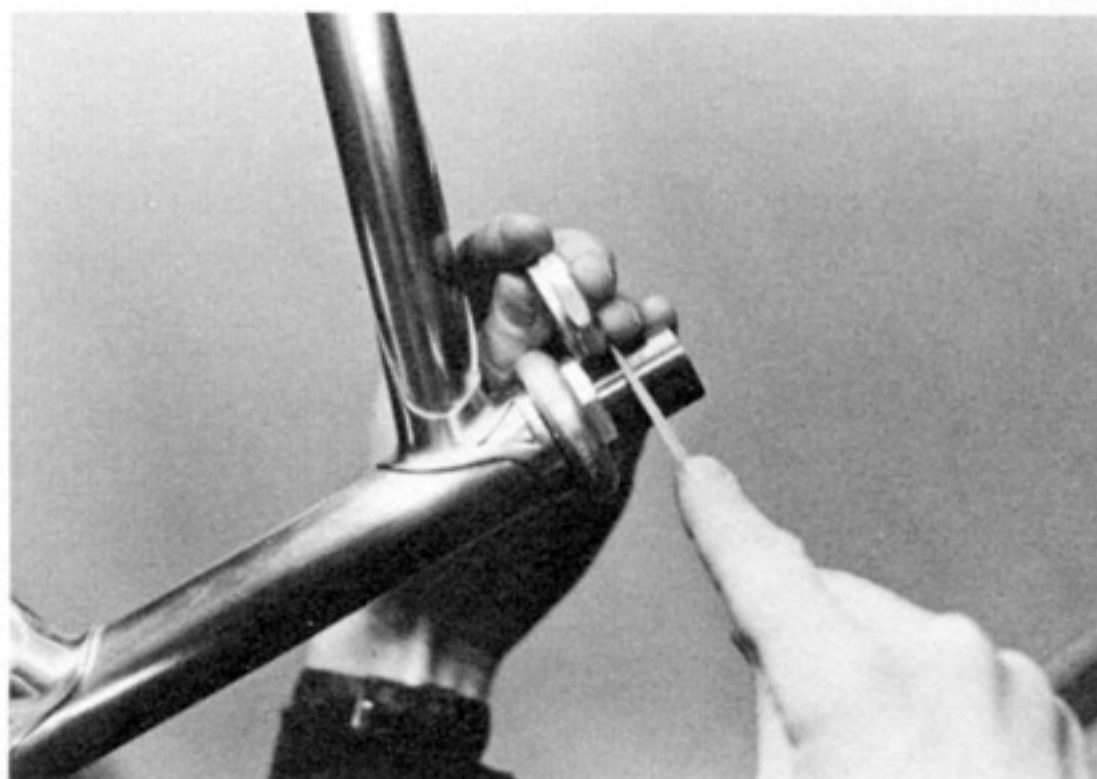
P10.31 The steering tube is marked for cutting. Nut and washer are used to determine proper length.
