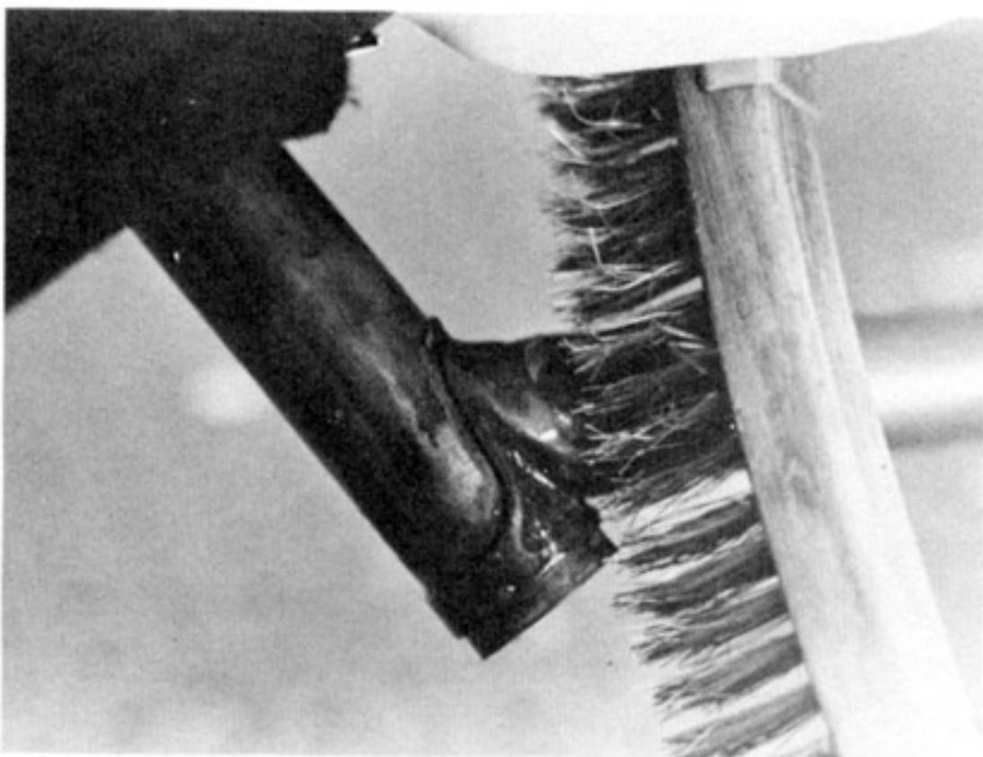
P8.25 After brazing, carbon deposits and residual flux are removed by wire brushing.
