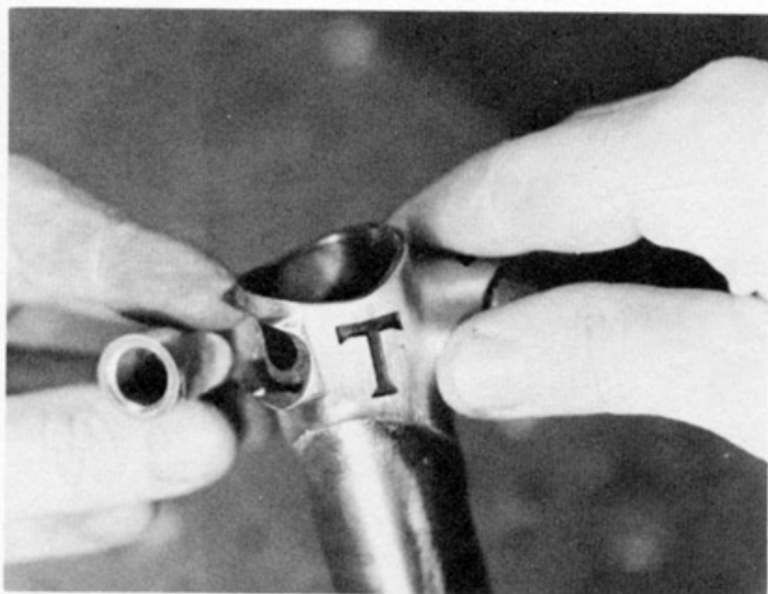
P8.31 Lug with ears partially removed. Concave slots have also been filed into the bolt tube and seat tube to provide proper fit.
