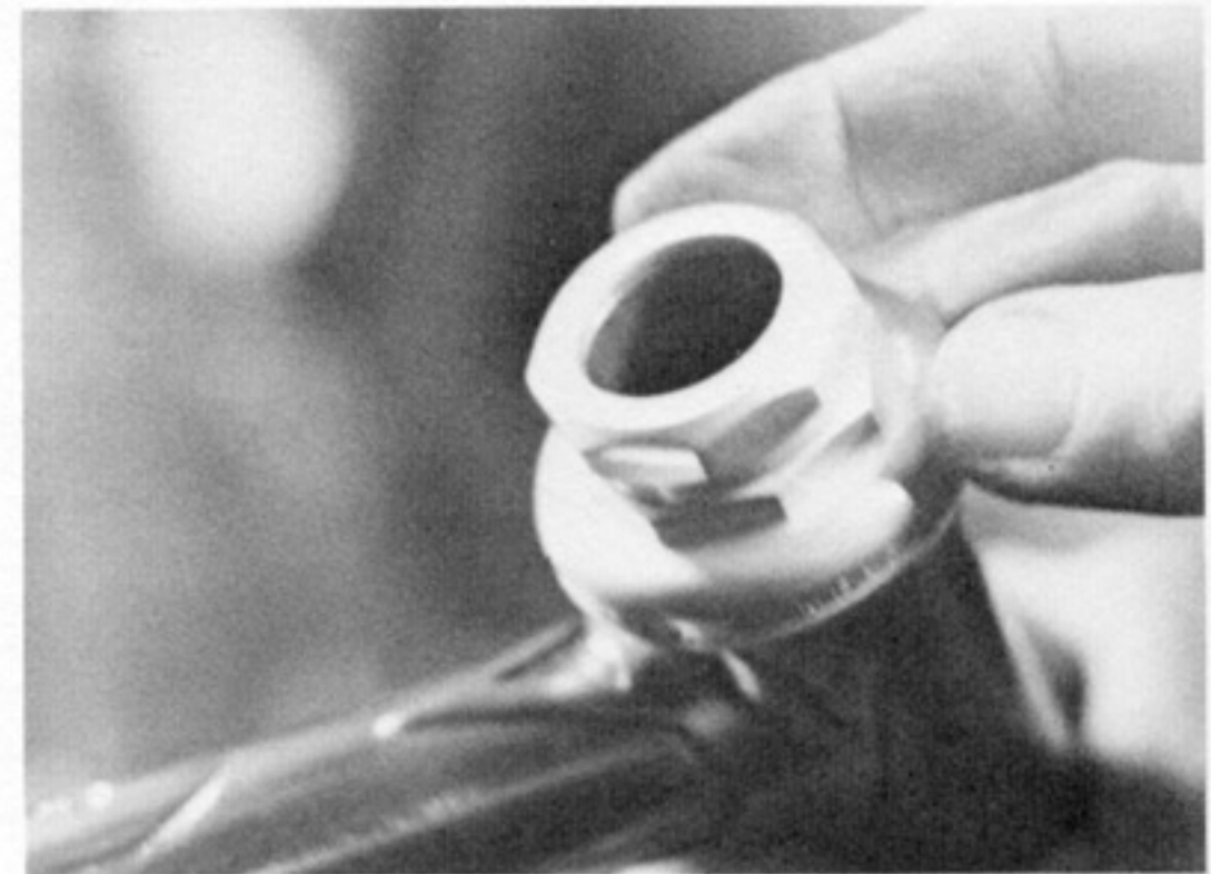
P10.38 The mounted headset assembly. Note slight clearance between end of steering tube and underside of lock nut.
