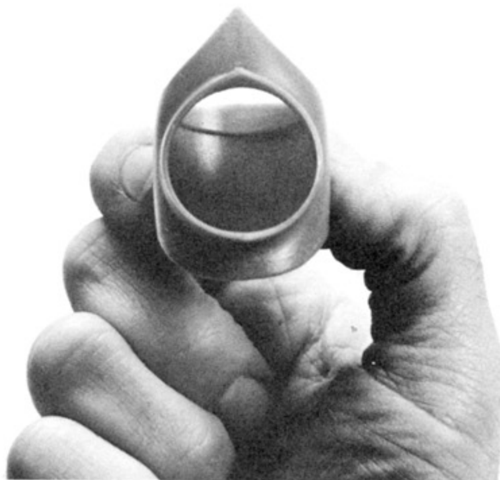
P6.3 Front view of a Henry James "wax" seat lug. Note integrally cast shoulder against which the seat tube will rest. Top of the lug is already contoured to final shape.
