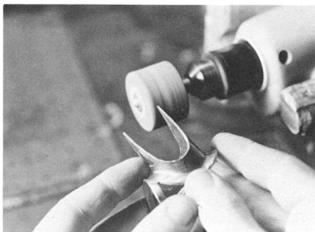
P8.14 "Pointing" lugs using a small grinding wheel.
