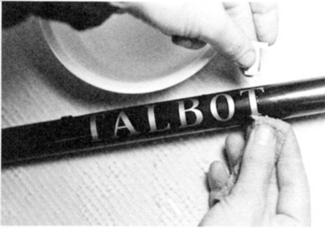
P11.16 Applying decals to the down tube. Tube surface is first wetted with decal setting solution.
