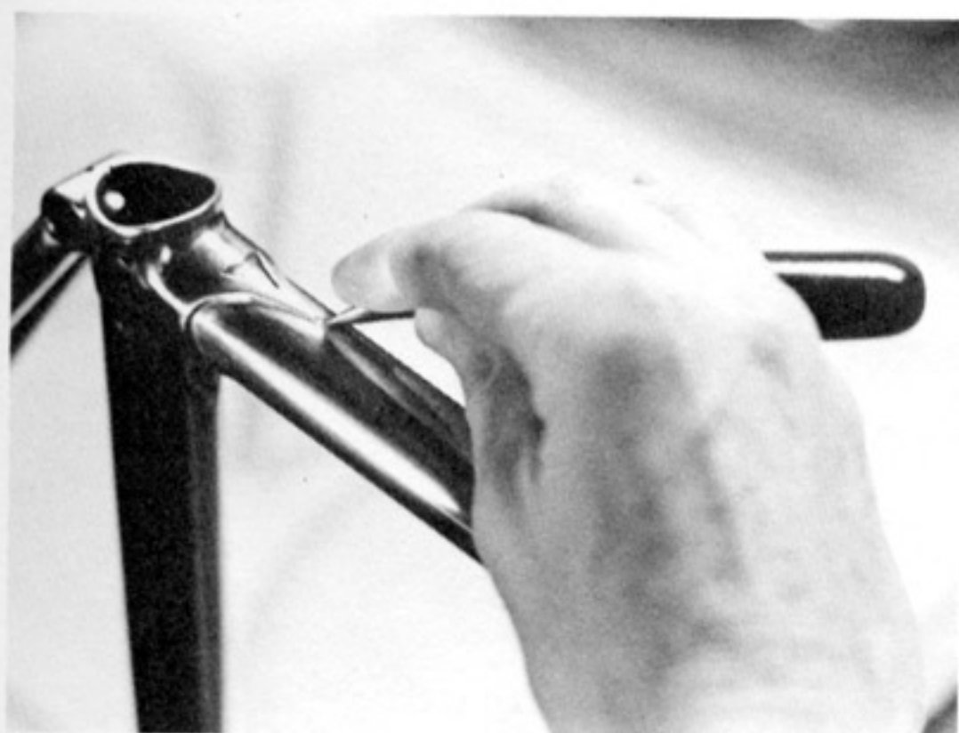
P10.7 Cleaning up lug seams with a curved burisher.
