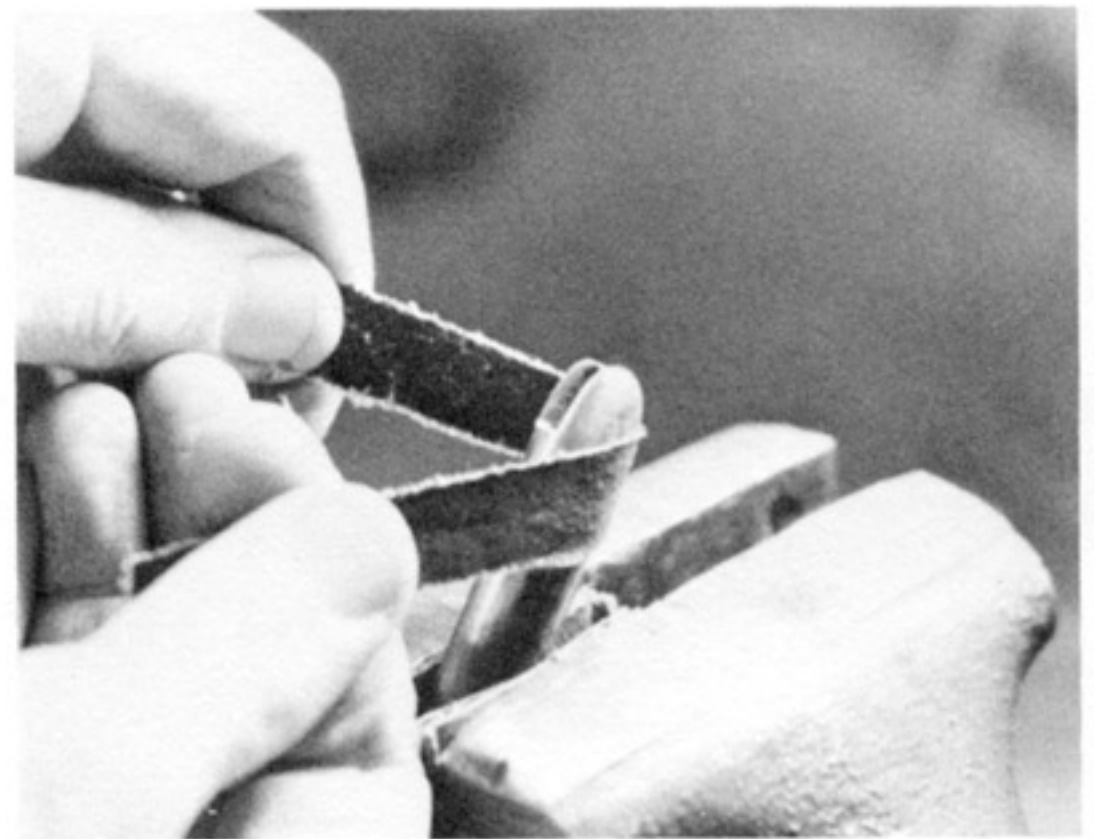
P9.4 Finishing up a stay end with production cloth.
