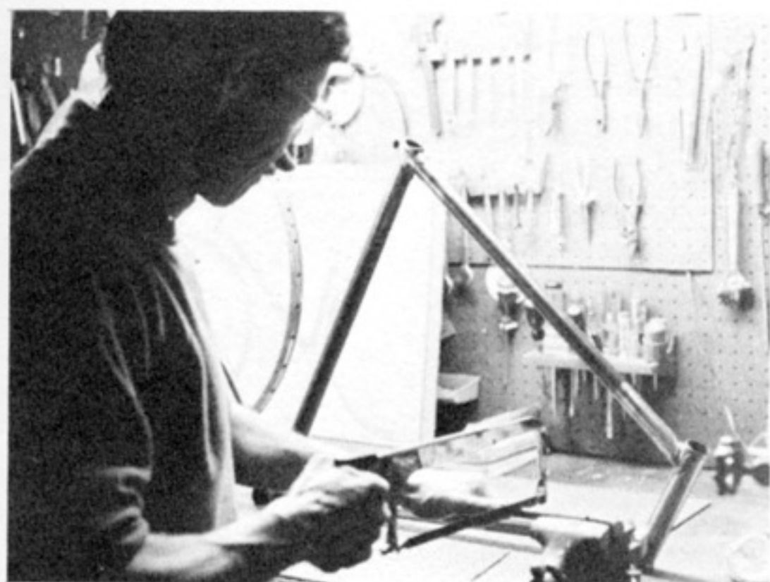
P9.12 Shortening a seat stay. Leave extra length for final mitering.
