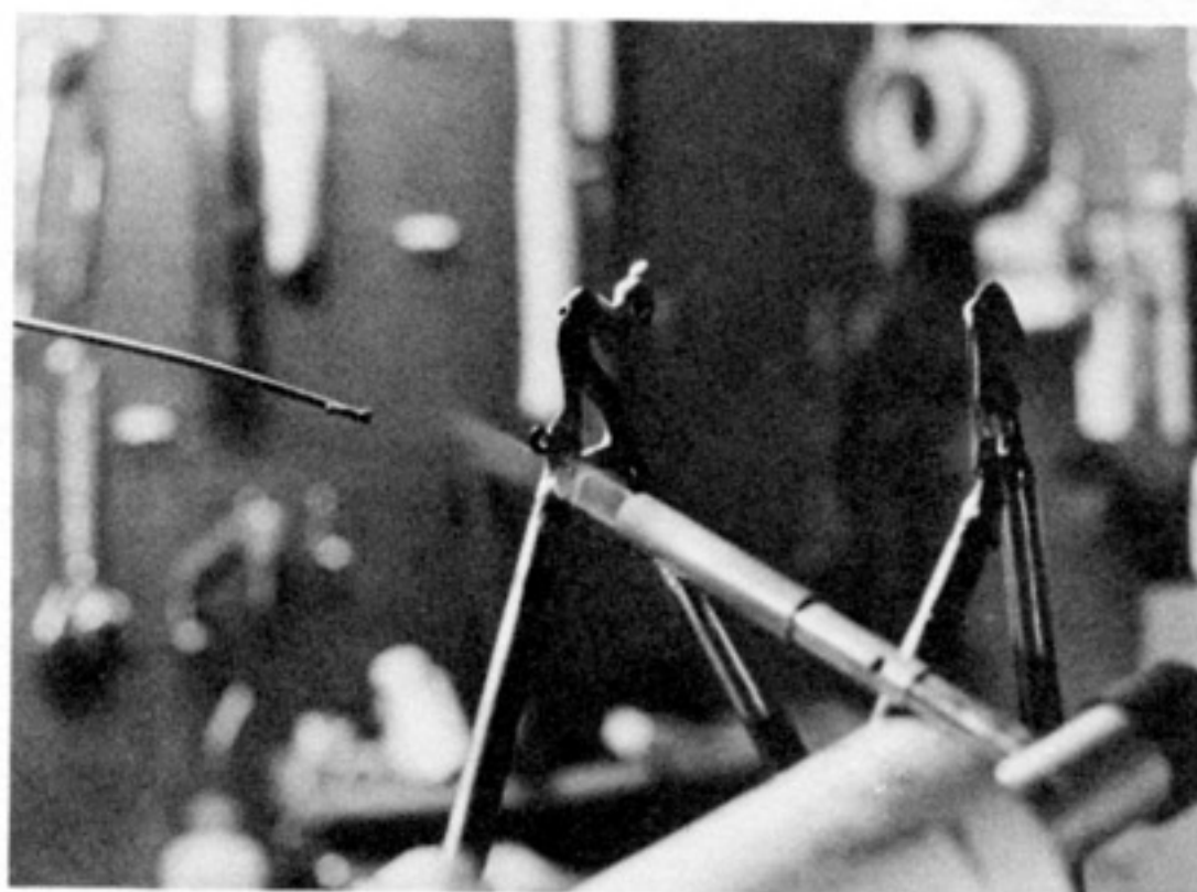
P9.20 Seat stays are brazed to dropouts to make the "V" assemblies.
