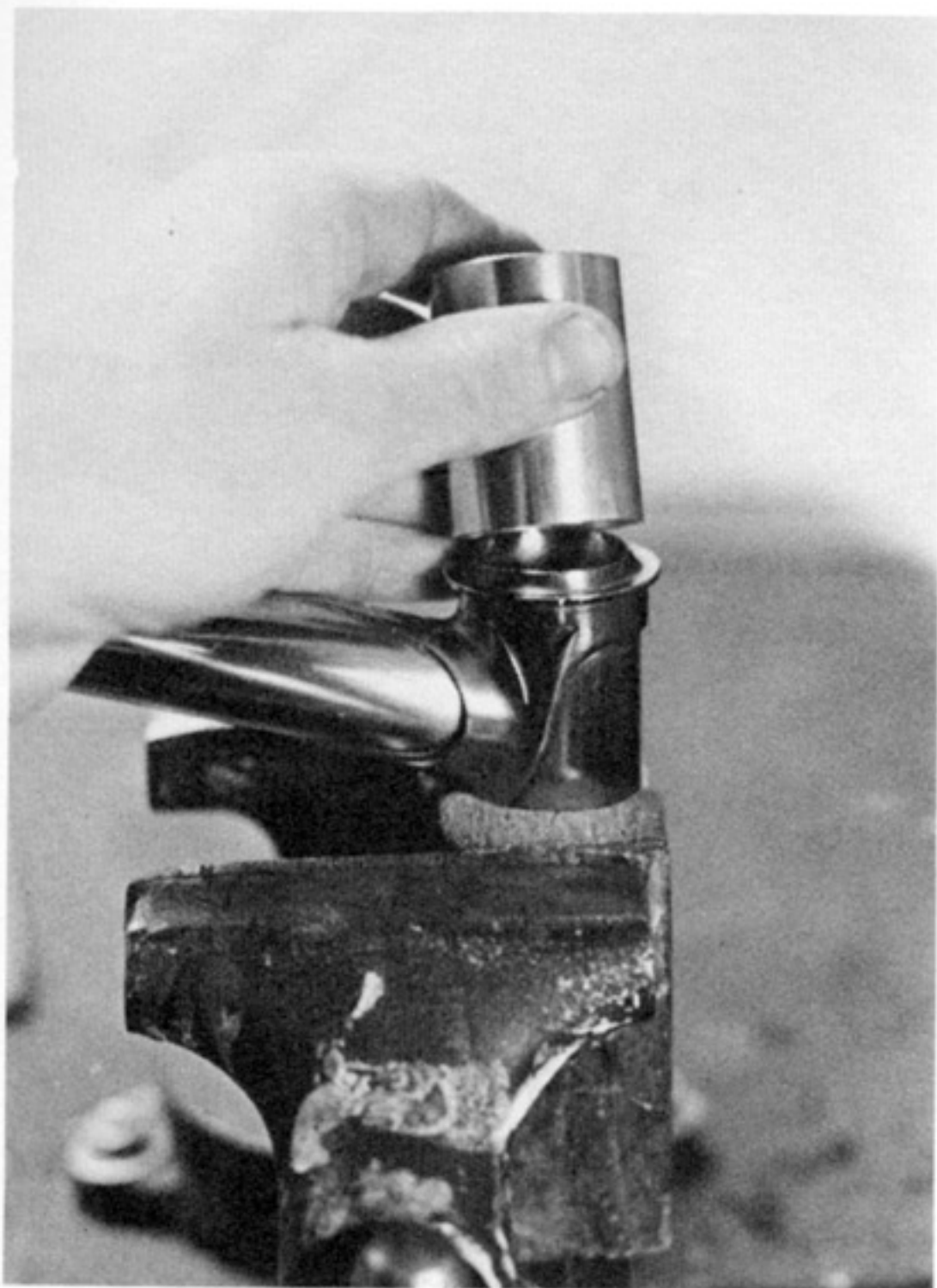
P10.16 Set-up for installing the top head race; short aluminum tube is used to prevent damage to race surfaces.
