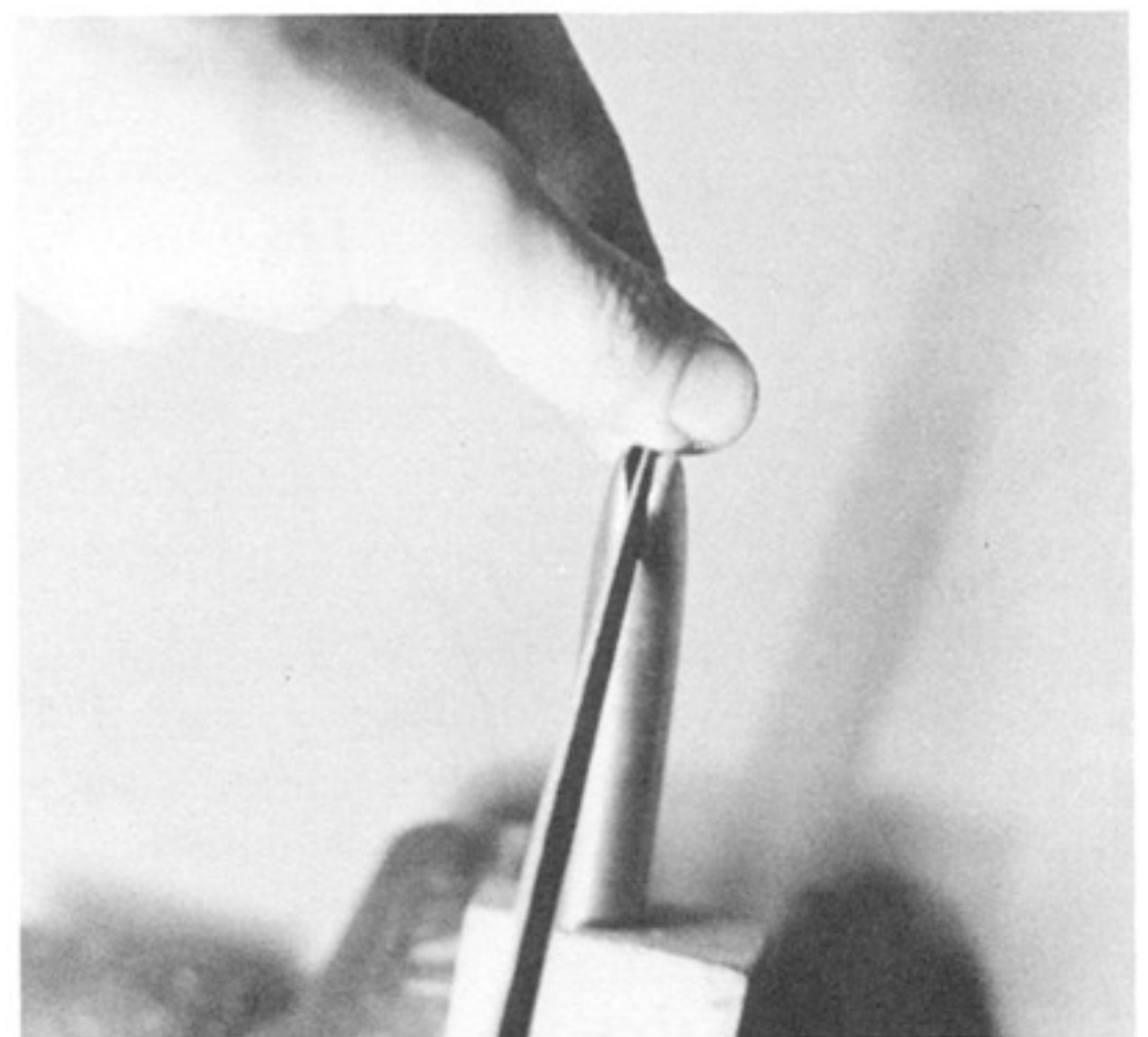
P7.7 Reopening the slot with a warding file.
