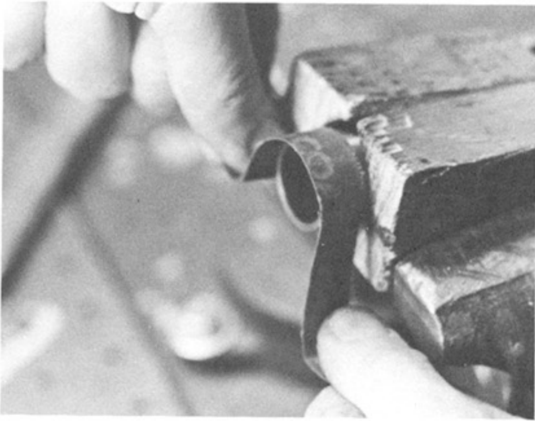
P7.4 Sanding helps maintain concentricity.
