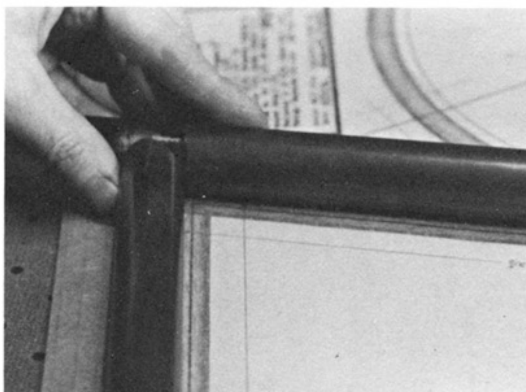
P8.8 Checking seat tube angle and fit.
