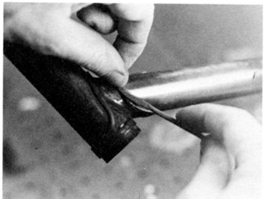
P8.27 Lug seams are best finished using rifflers.
