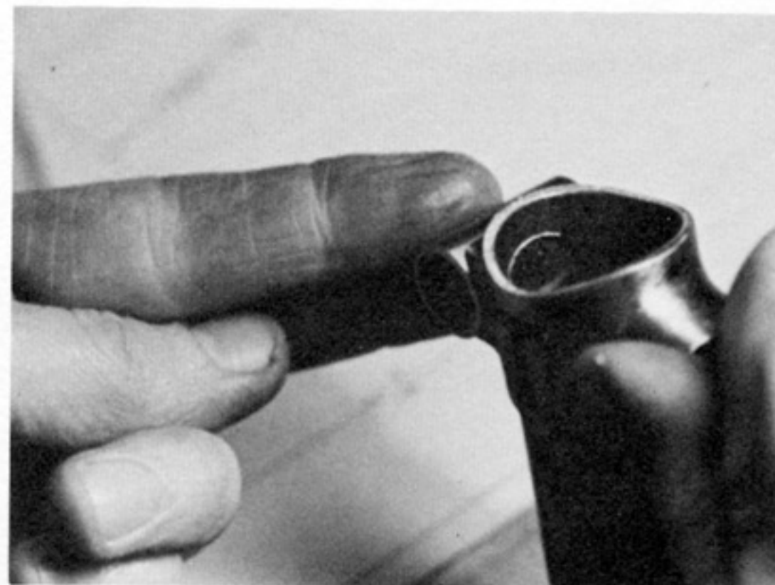
P8.32 Checking bolt tube fit.
