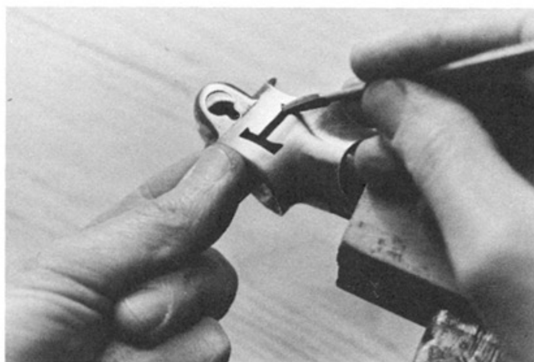
P8.15 Using a riffler to file a custom cut-out in the seat lug. Lug is clamped between wood blocks for added support.
