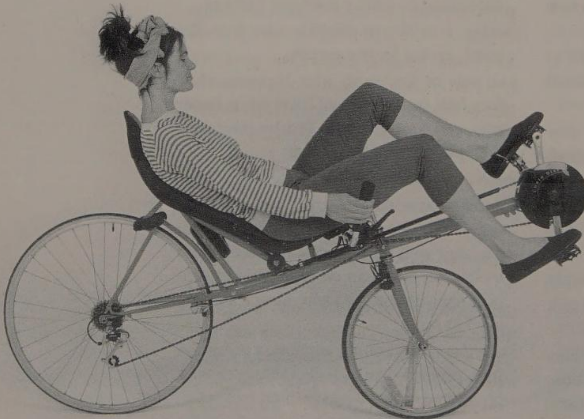
This M5 is one of their first designs and is still produced. It's a steel-framed classic with standard rear elastomer suspension. (photo: M5)
