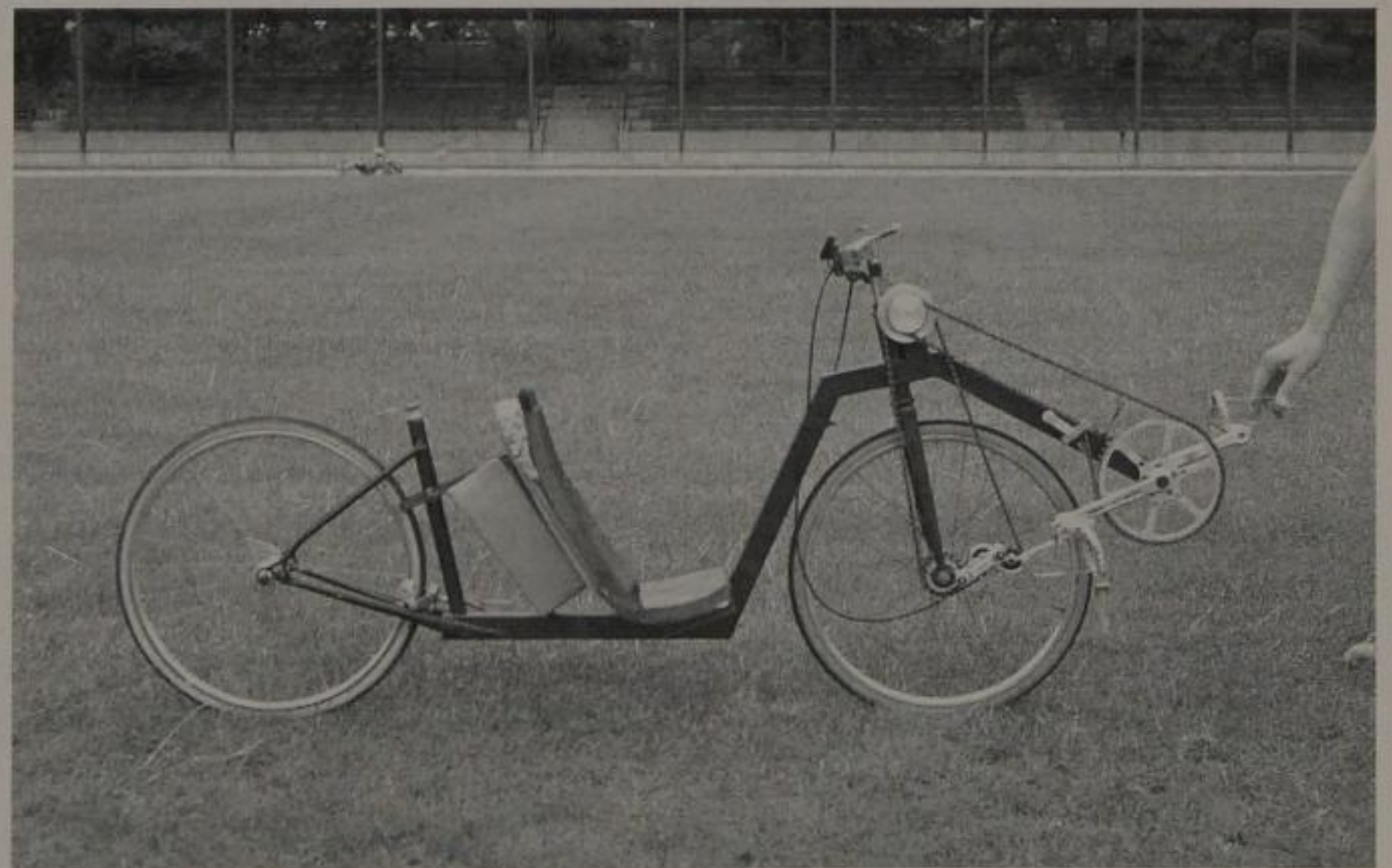
This homebuilt lowracer is shown without its fairing. It has flex-chain front-wheel drive with an intermediate gear located at the head tube. This is strictly a racing bike because as you turn the handlebars the chain twists, making low-speed, sharp turns difficult. Foot-strike is also an issue.
