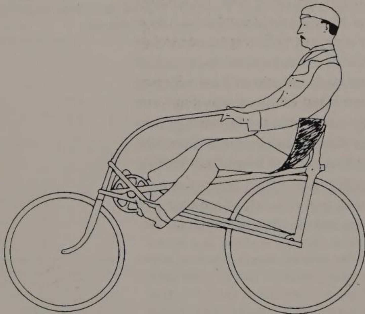
Challand's 1897 model appears to be more practical. It foregoes the full body drive in favor of a pedal crank. This machine fascinated the press. (Drawings based on article in Olms Press.)
