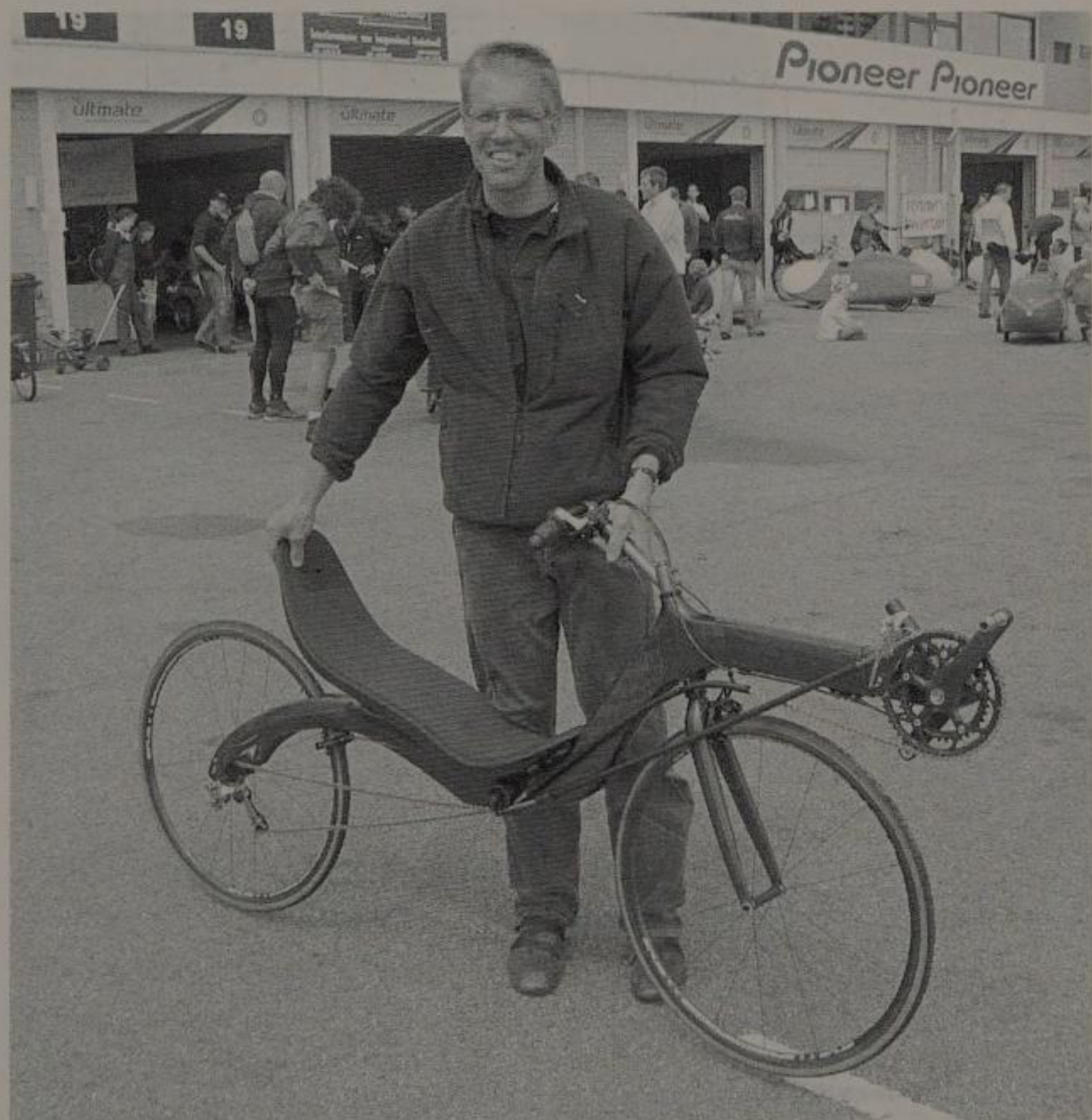
Bram Moens of M5 is proud of this bike, unveiled at the 2006 Cycle Vision expo: the lightest production recumbent, a 16.5-lb highracer. (photo: M5-ligfietsen.com )
