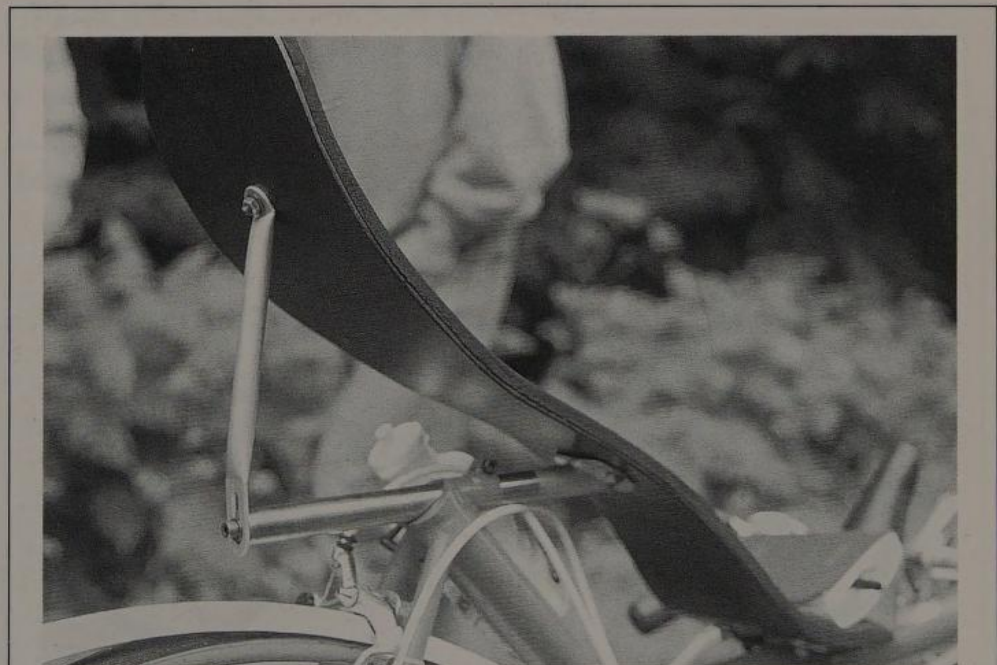
Seat adjustment on this bike is made via a modified seatpost and road-bike style seat tube lug, creating an unusual but effective support.
