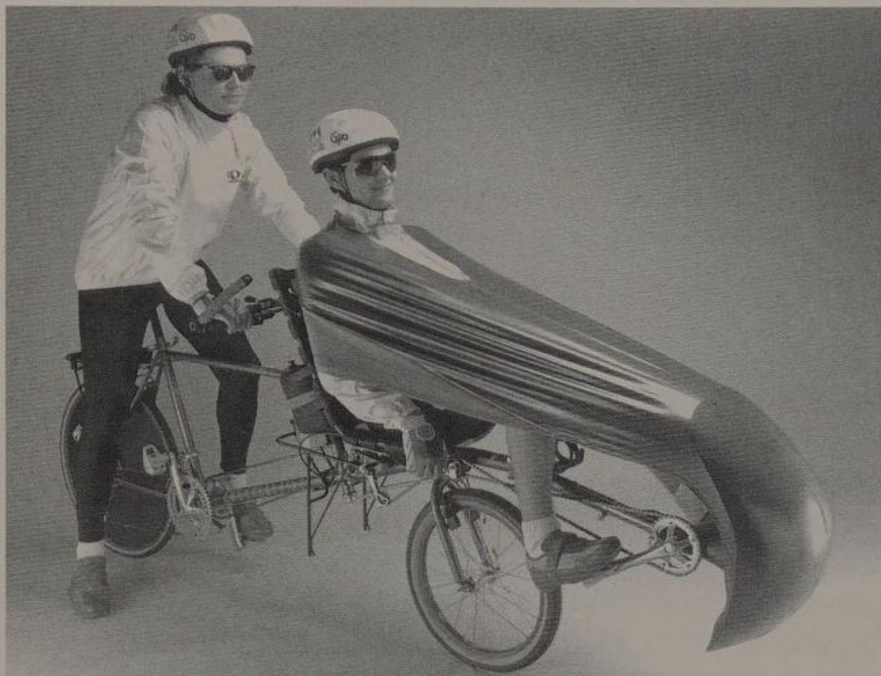
The Bilenky "Viewpoint," a mixed-position tandem, puts the stoker in the front in a reclining position, while the captain sits upright in the rear and steers. A fairing can be fitted to boost speed. Bilenky also offers handcycling and child stoker-seat options. (photo: Counterpoint)
