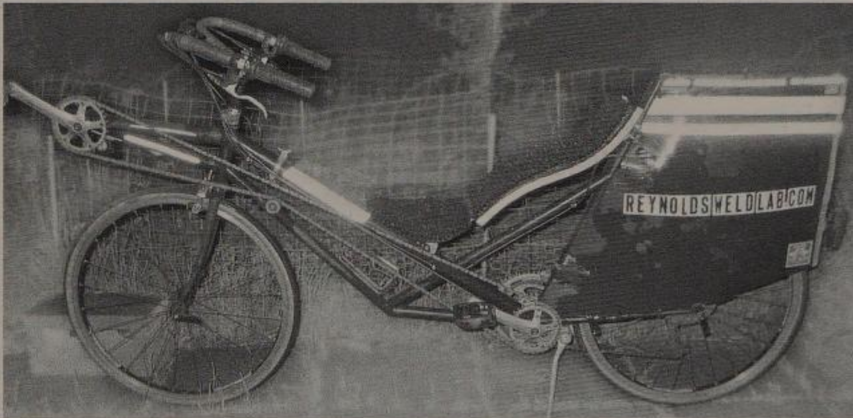
George Reynold's “Redundant” prototype converts in seconds between upright and recumbent modes. (photo: G. Reynolds)
