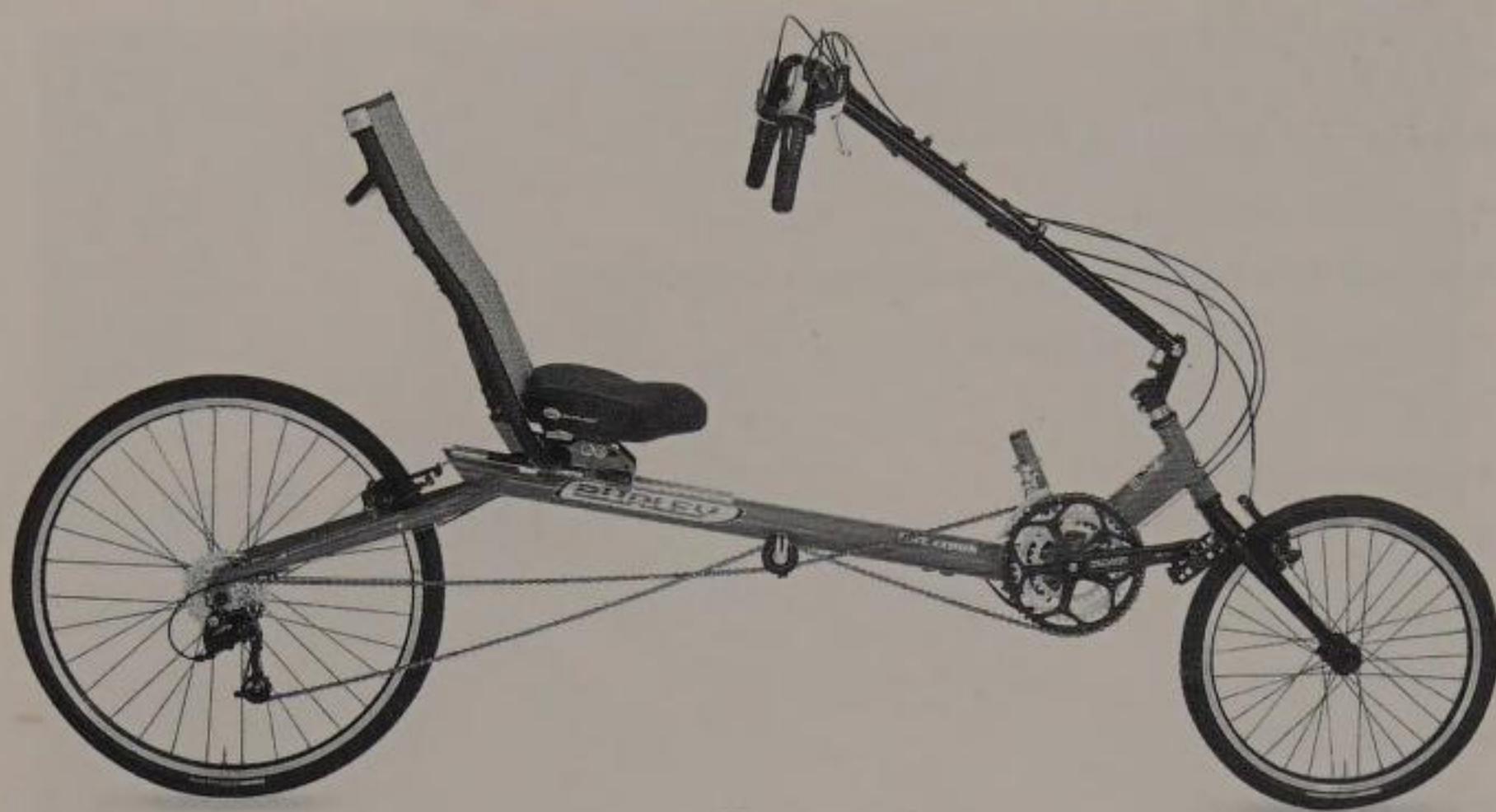
Burley's affordable "Jett Creek" features a pivoting handlebar for easy step-over and a long wheelbase for comfort.
