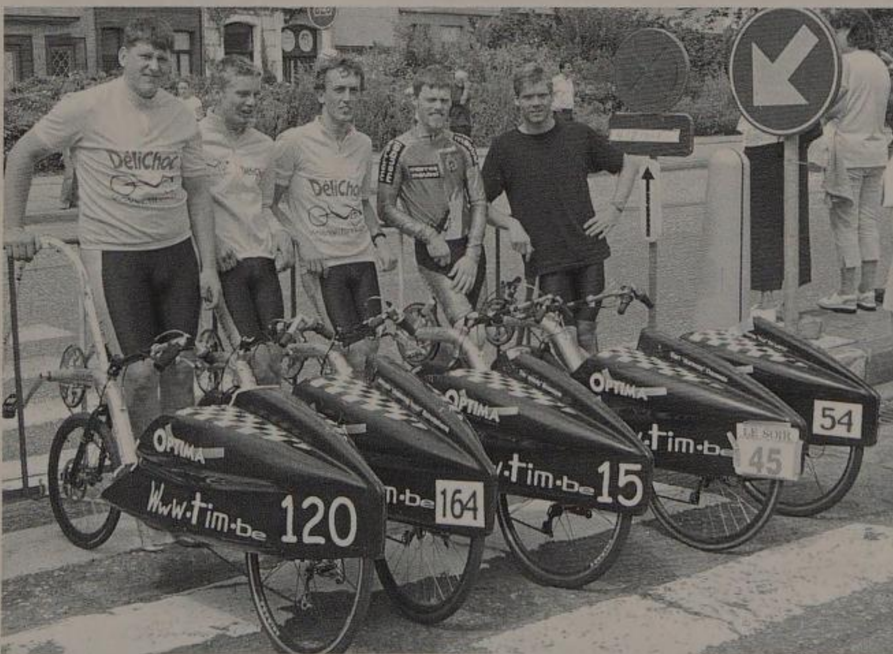
This team of Optima lowracers uses carbon rear fairings all pulled from one mold, greatly economizing on time, labor, and costs—and giving the team a stylish, unified look. (photo: www.tim.be)
