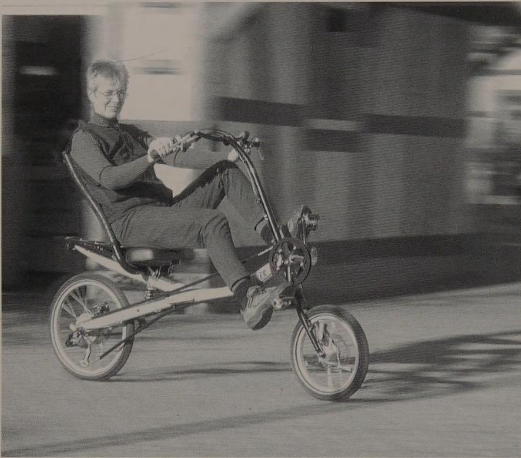
The "Spirit" compact from HP Velotechnik is a well-conceived urban recumbent with rear suspension and sporty crank height. (photo: HP Velotechnik)
