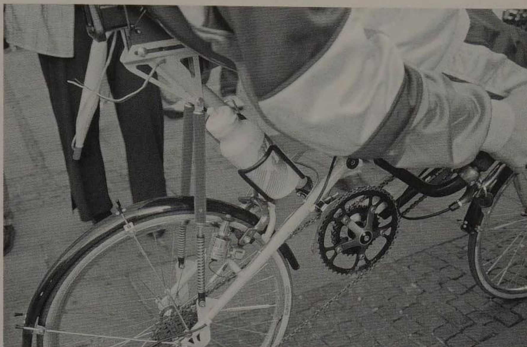
Various items can be used to create suspension. Here, somebody used the pistons from a car trunk lid.
