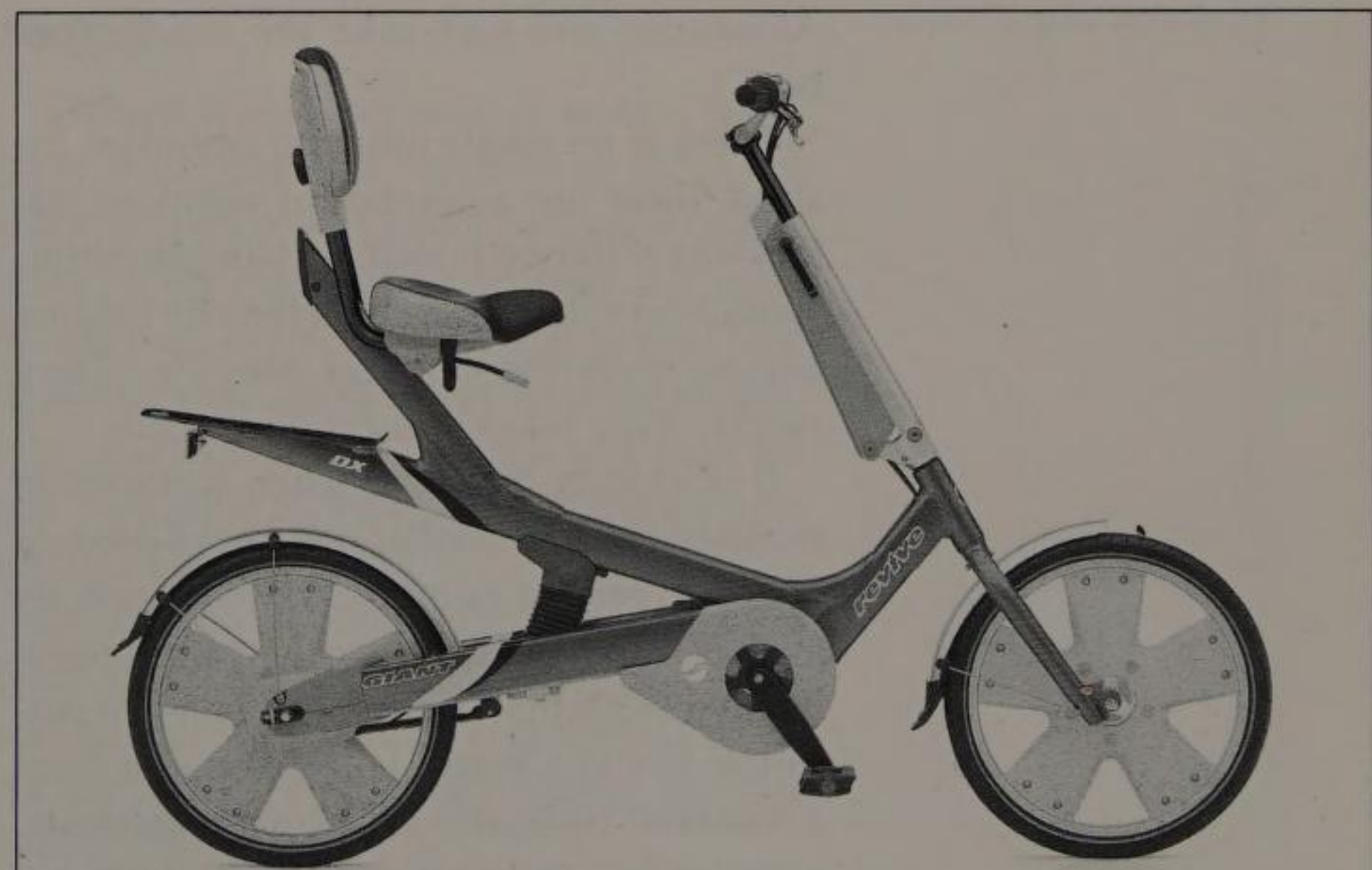
The Giant “Revive” semi-recumbent is designed for comfort and ease of use. (Giant studiously avoided the term “recumbent.”) The DX model pictured here includes a Shimano Nexus 7-speed internal hub. The enclosed drive system, rear shock, and cargo platform—along with budget pricing—make it a good city bike.
