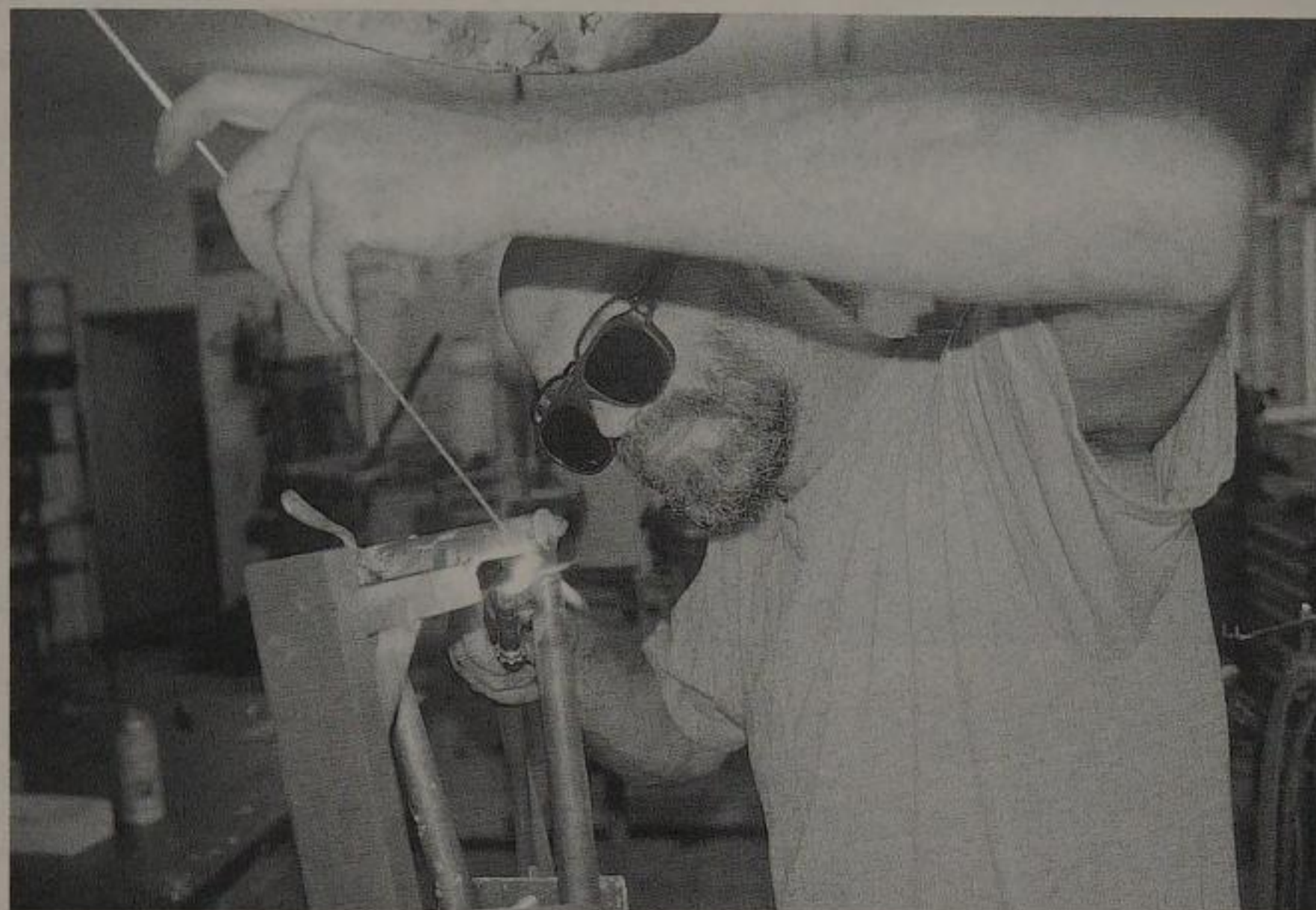
Kurt Pichler brazing a fork dropout. He's an expert builder and also produces the Pichlerrad line of bikes in Germany.
