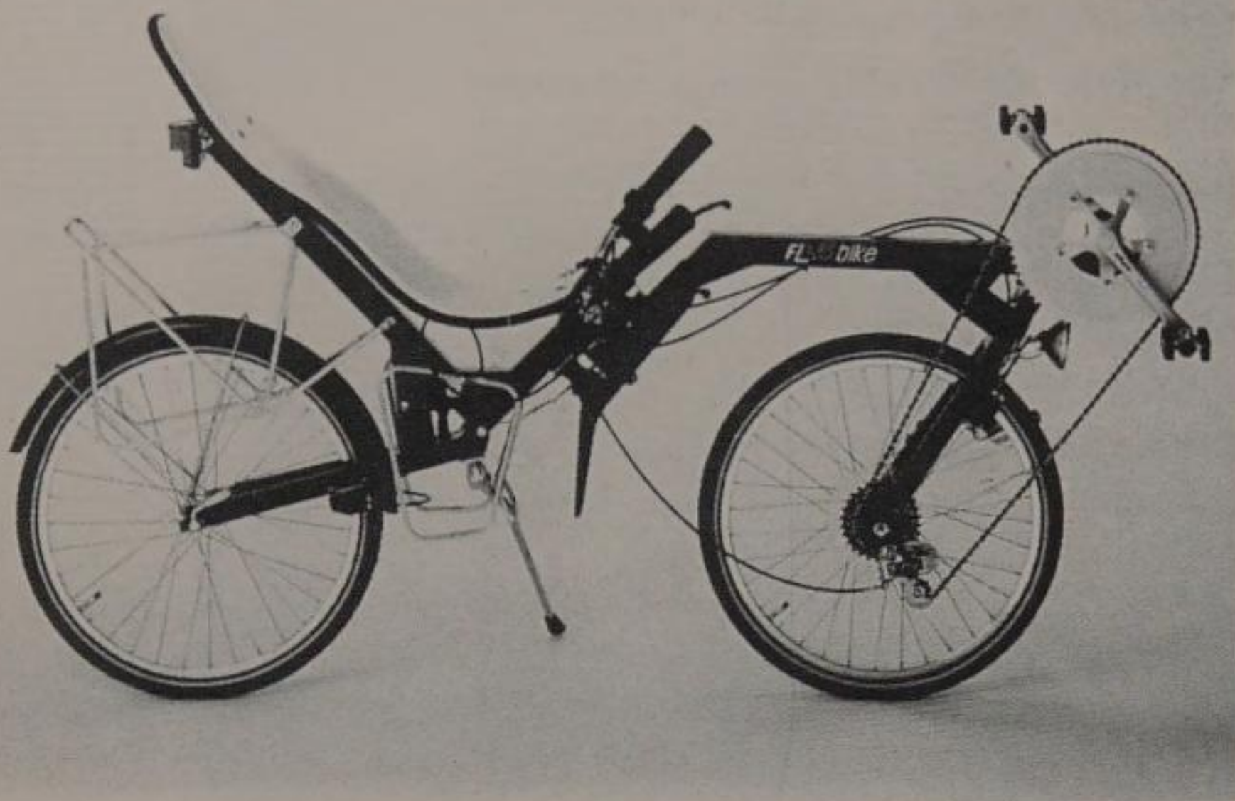
The pivoting front drive of a Flevo Bike connects the entire drive unit with the front fork. The frame and mechanism swing together to steer—a feeling that takes a lot of getting used to. (photo: Pichler)
