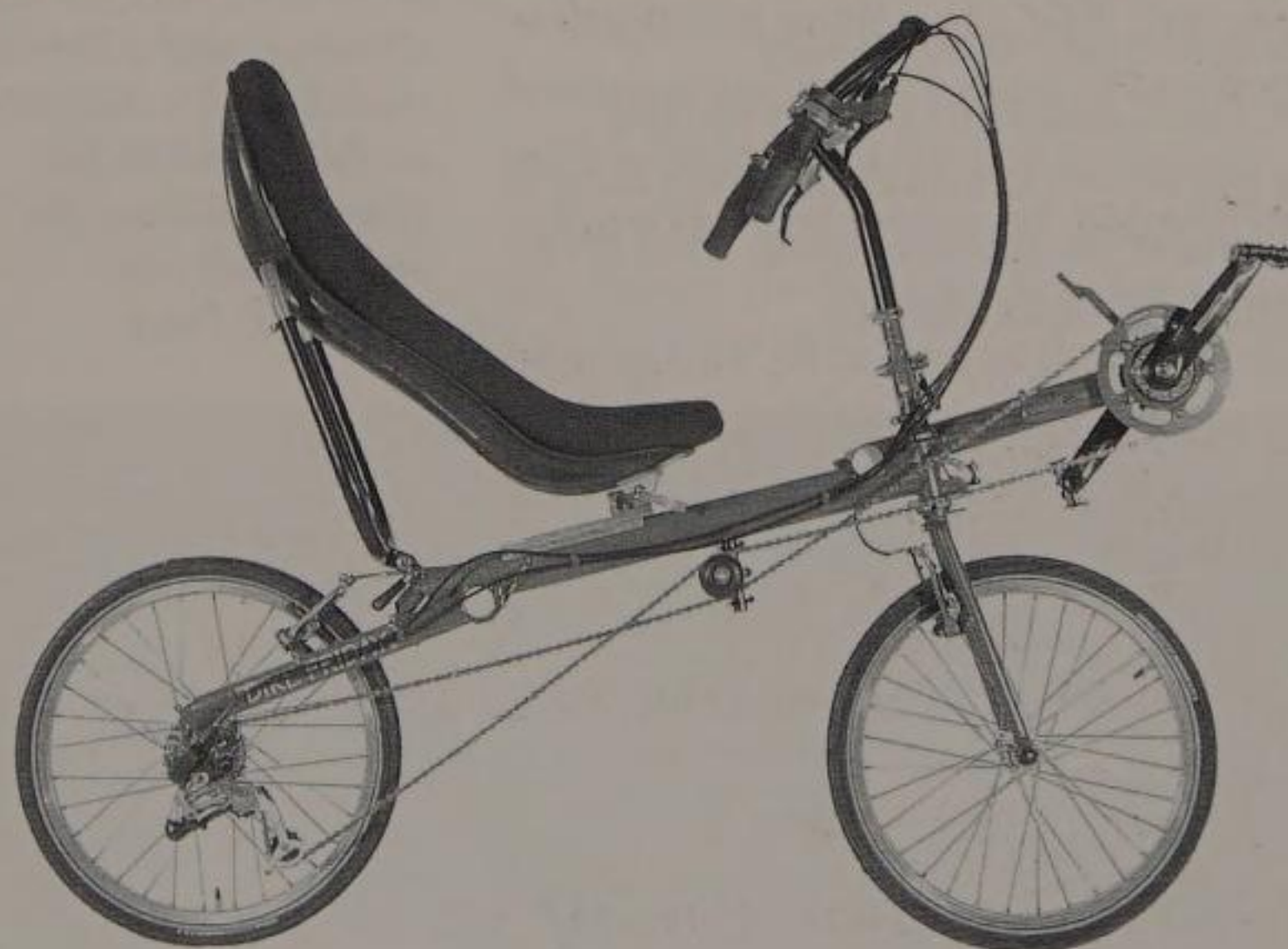
Bike Friday's "Sat R Day" folding recumbent with 20-inch (451mm) wheels fits in a suitcase. Bike Friday is a highly regarded maker of high-end folders. (photo: Bike Friday)
