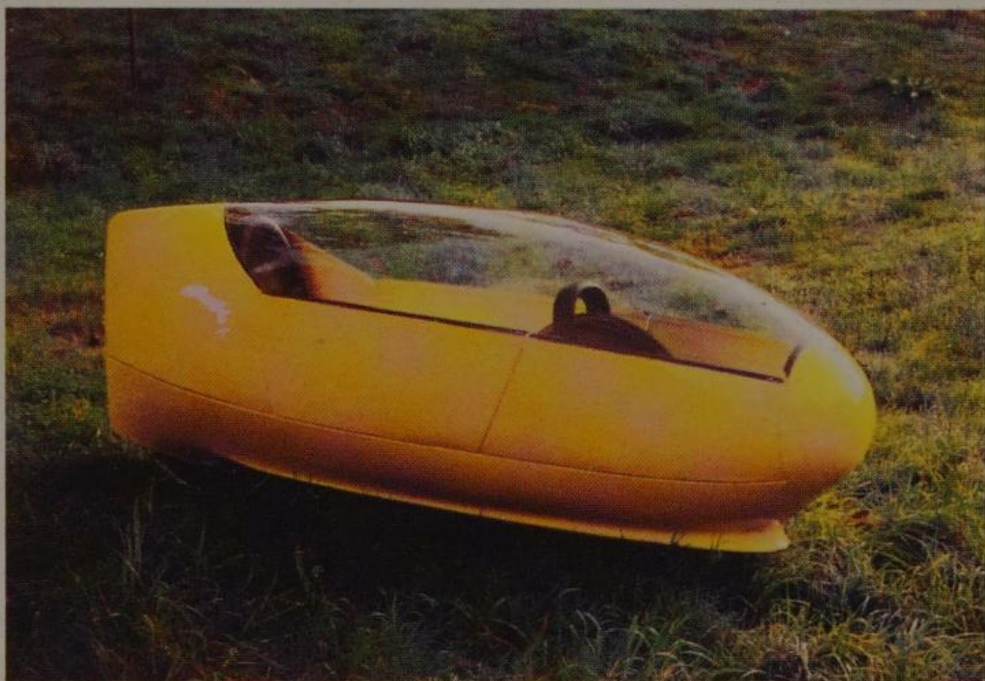
Fairing made by Zillner Design: – establishing the measurements with a “wooden man’s” help – skeleton – original form – female mold – mounted fairing (photos: Zillner Design)
