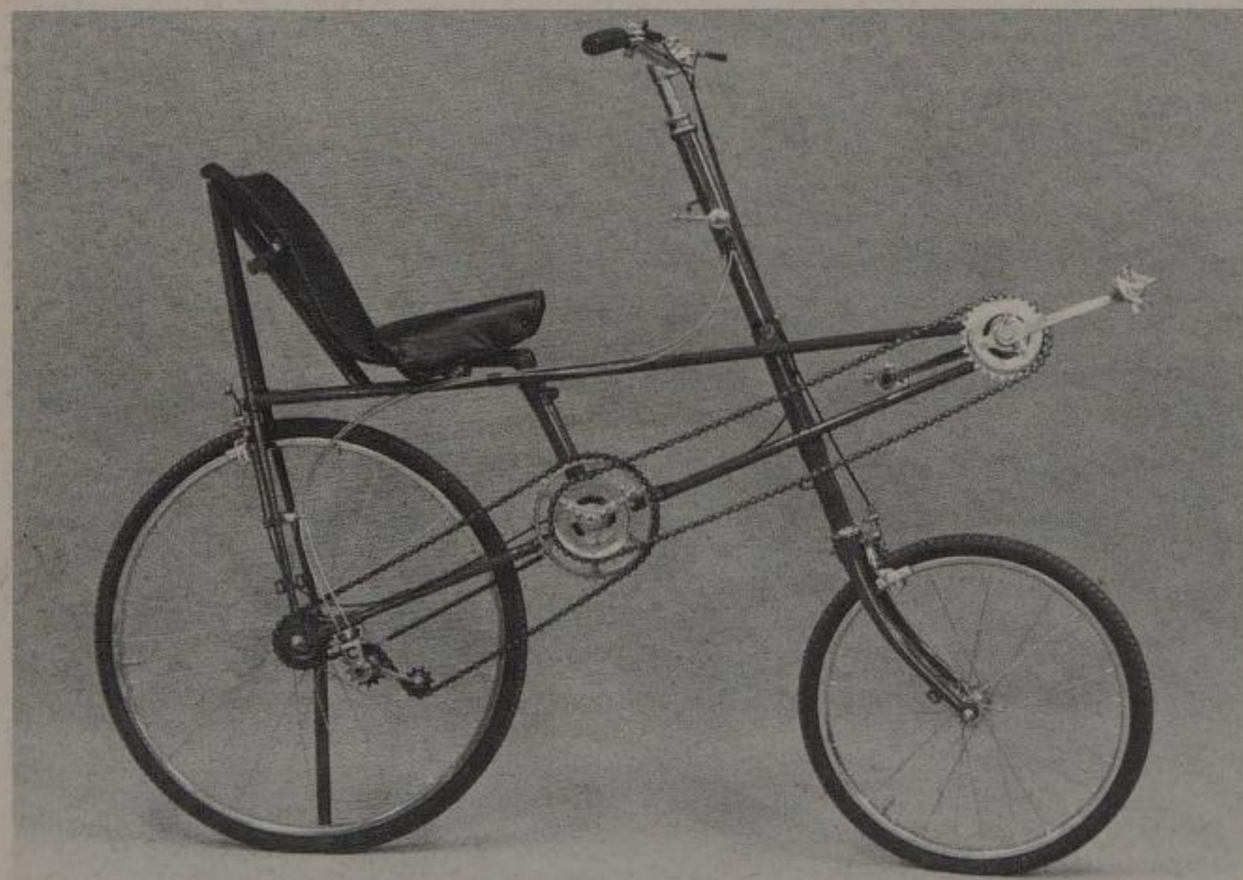
To handle the play in the chain, an intermediate cogwheel was added in 1936. (photos: Mark Hall Cycle Museum)
