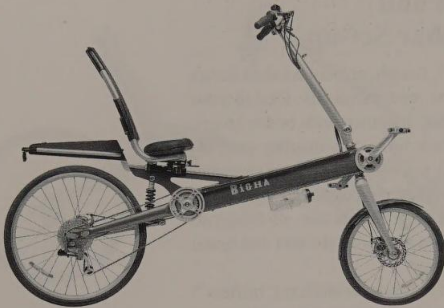
The BigHA (Apache for “because”), is a feature-packed, luxury CLWB-type recumbent whose seat, back support, and handlebars are easily adjustable. An optional handlebar console includes lights, turn signals, speedo, heart rate monitor, wind direction sensor, and horn. They emphasize high-tech direct ordering via their website.
