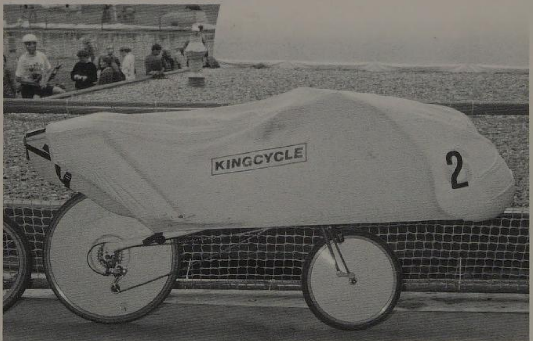
The compact "Kingcycle" SWB was sold with optional rear fin, front nosecone, and a cloth fairing, making for a fast club racer.
