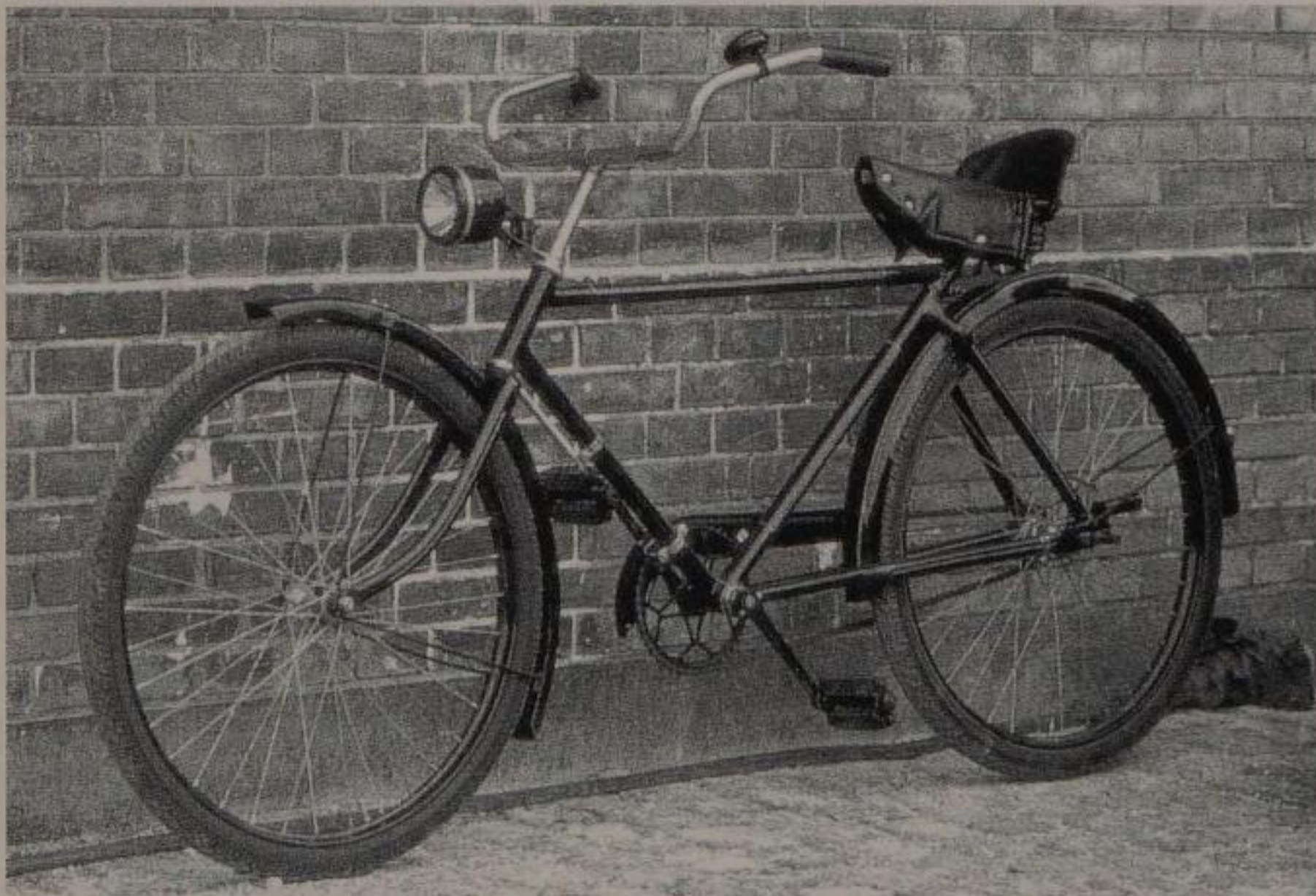
The Danish "Sofacykel" from 1935 has a "crank forward" design. Back to the future! Not a real recumbent, it nonetheless had a special position in the bike market and can, historically speaking, be categorized as a semi-recumbent. The handling is extremely slow due to the shallow head-tube angle. A spring dampens fork-flop when turning.
