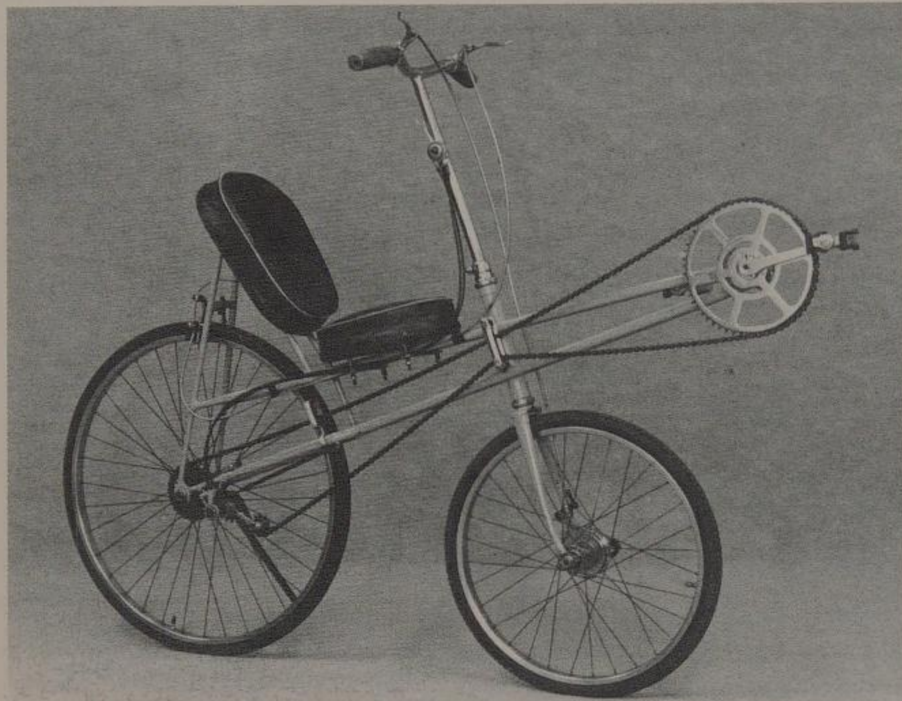
The Cyclo Gear Co. introduced the "Cyclo Ratio" in 1935, a short wheelbase recumbent with an improved four-gear shifter.
