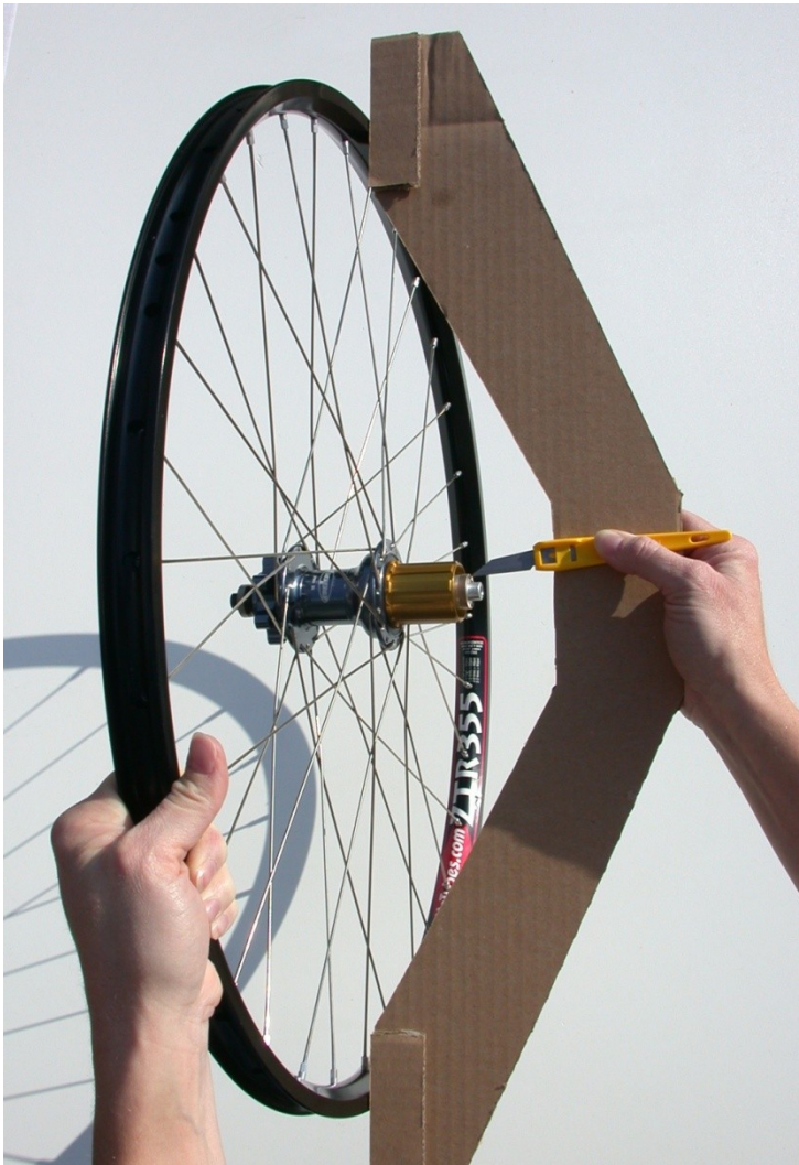
Figure 23 Cardboard dishing tool
