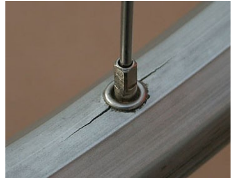
Figure 56 Fatigue crack in rim
