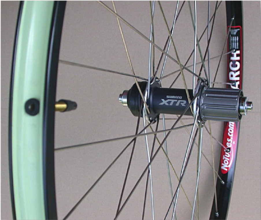
Figure 46 The aligned valve and hub label.
