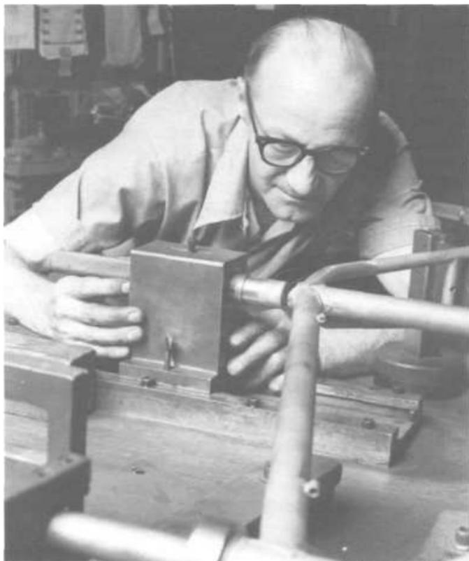
**Figure 17-1:** Ferenc Makos, at an aligning table, makes sure the Paramount frame is perfectly aligned and straight.
