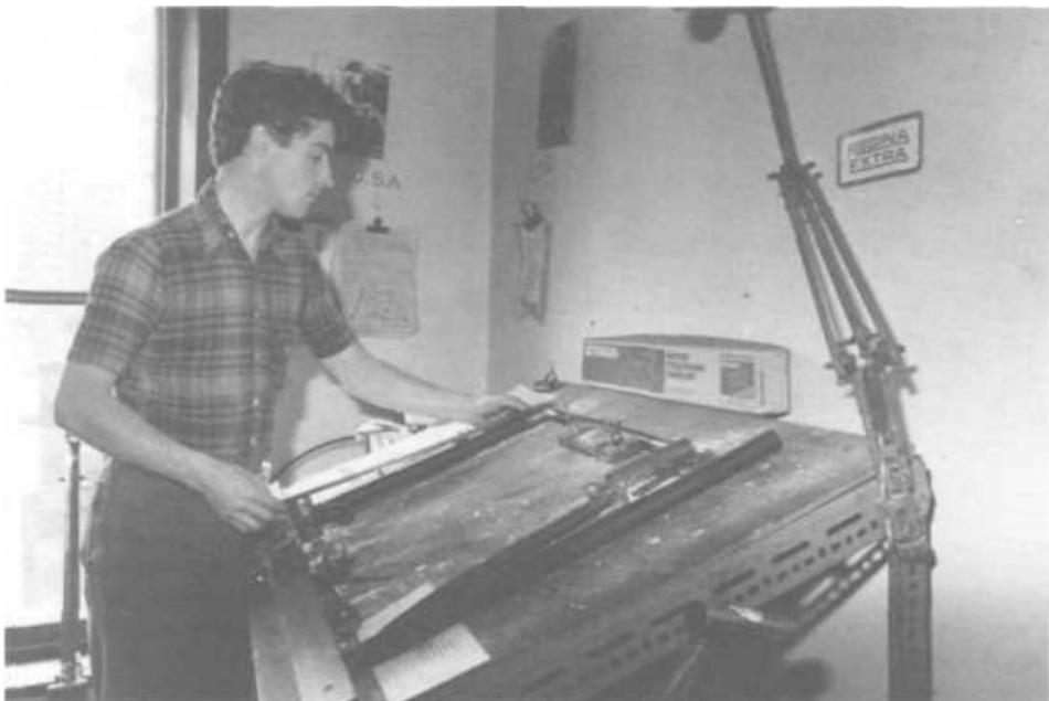
Figure 7-2: Harry's "Ouija board" for frame setup. The clipboards on the left contain specific frame geometry requested by the customer.
