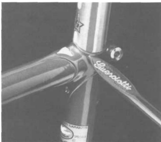
**Figure 1-14:** The semi-wrap stay can be made in two ways. It can be chamfered with a plate brazed over the opening, or it can be a plug such as ones sold by the lug manufacturers. Guerciotti uses the flat surface to personalize his frames.
