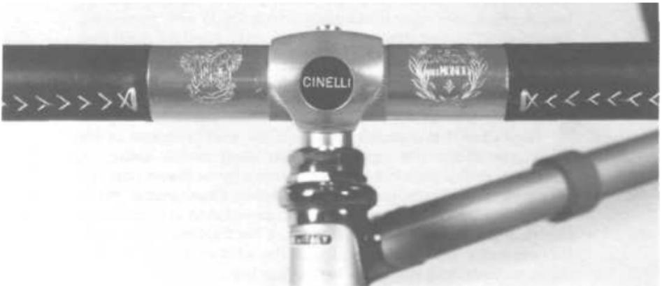
Figure 14-3: The new, redesigned (and very expensive) Cinelli handlebar stem. The new design eliminates the traditional front bolt for tightening the handlebar. The removal of the bolt results in improved aerodynamics.
