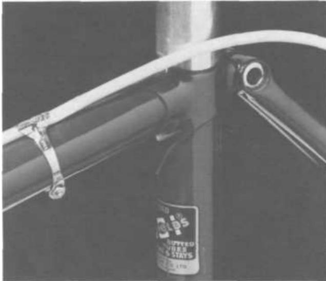
**Figure 1-19:** Fastback seatstay. This style is preferred by many time trialists because it gives the appearance of being light. In reality, it can be heavier than the semi-wrap stay because large amounts of metal are needed for the seat lug to attach the seatstays near the seat binder bolt.
