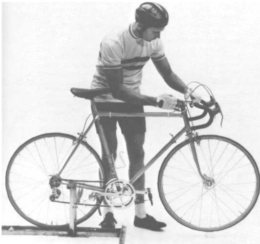
**Figure 20-6:** Determining stem length. Some people believe that the length of a handlebar stem can be determined by placing the elbow on the tip of the saddle with the fingers extended. . . . This is not true. This measurement does not consider the overall length of the arm and body combined.
