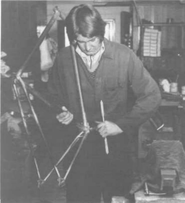
Figure 5-1: "Cleaning" the bottom bracket. Note tool used for this procedure (see figures 3-5 and 3-6 in chapter 3).
