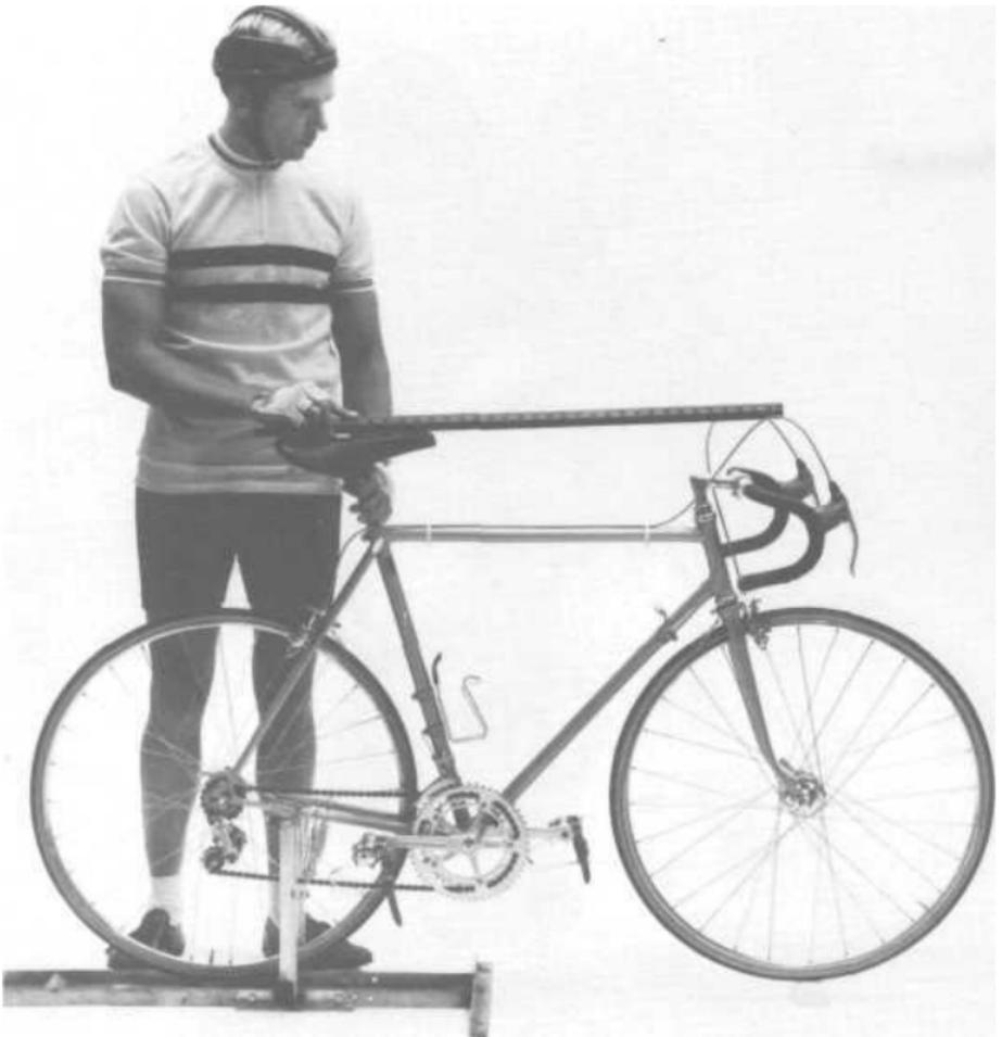
**Figure 20-1:** Setting saddle angle. The front of the saddle should be slightly higher than the back of the saddle. Placing a yardstick on the saddle makes this critical adjustment easier to set. Never allow the tip of the saddle to be lower than the back of the saddle.
