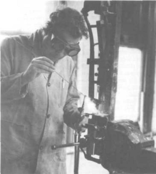
**Figure 5-2:** Builder brazing the fork crown at JRJ Cycles.
