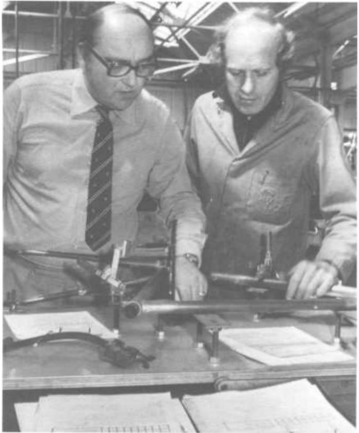
**Figure 9-1:** Gerald O'Donovan (left) and one of the technicians discuss the setup of a frame prior to brazing.
