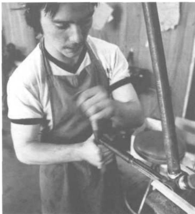
**Figure 18-8:** One of the four or five frame builders at Proteus Design. Here shown reaming out the bottom bracket chainstay opening.
