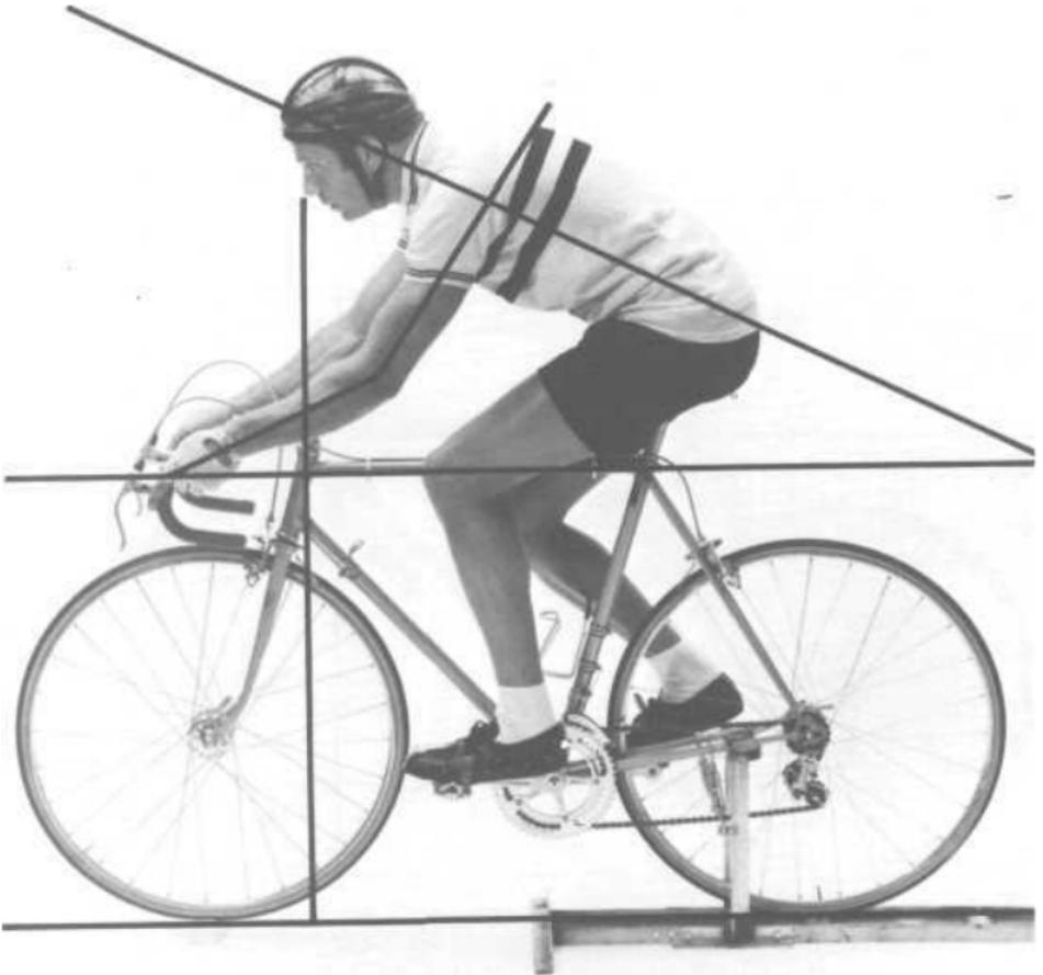
**Figure 20-12:** Incorrect handlebar position (long stem, Position 2). The rider's weight is too spread out. Too much weight is placed on the front wheel. The rider supports himself without the help of his shoulders.
