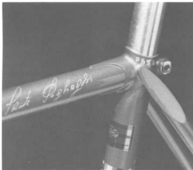
**Figure 1-16:** Note the beefy-looking, 16-mm. semi-wrap stay used on this 58-cm. track bicycle. Pogliaghi (see chapter 16) adds a personal touch to his bicycles with a transfer of his signature on the top tube.
