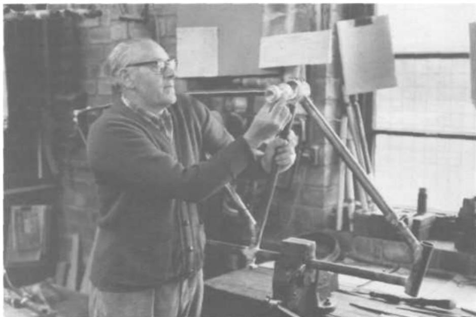
Figure 8-2: Jack Taylor fits the bottom bracket on a custom tandem.
