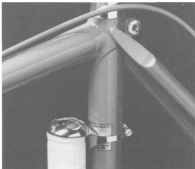
**Figure 1-17:** A completely different variation of the semi-wrap stay. This is a chamfered stay which has a curved top plate brazed over the opening.
