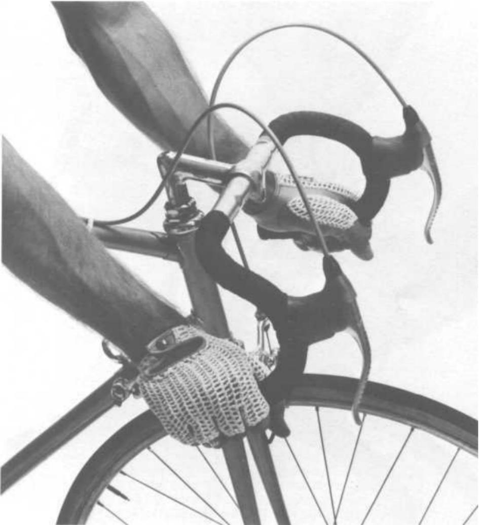
**Figure 22-5:** Incorrect Position 3. The wrist is not straight and the hand is too close to the end of the handlebar. This position drastically reduces your control of the bicycle. Check for yourself. Try weaving back and forth with your hands in this position. Now try the same test with your hands correctly placed. The increase in stability should be immediately obvious.
