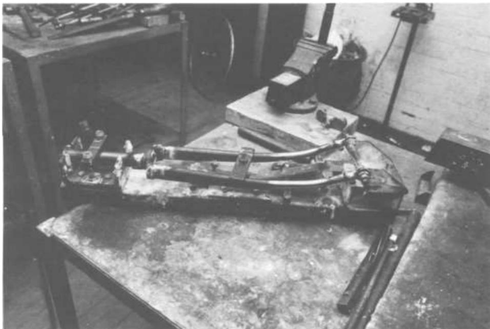
**Figure 1-5:** Fork jigs are usually fairly simple and variations between builders are slight. This is a jig used by Bob Jackson (chapter 5). The fork has just been brazed and therefore has a very rough appearance.
