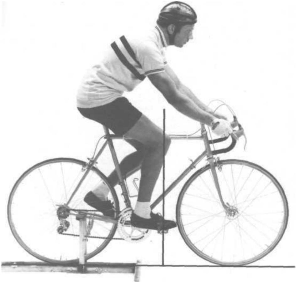
Figure 20-3: Horizontal adjustment of the saddle. The saddle position from front to back is adjustable to compensate for individual variances in upper leg length and riding style. To correctly adjust the saddle, sit on the bicycle with both feet in the toe clips. The saddle is correctly adjusted when a plumb line from the center of the knee falls through the pedal axle of the foot when it is in the forward position with the crank parallel to the ground.
