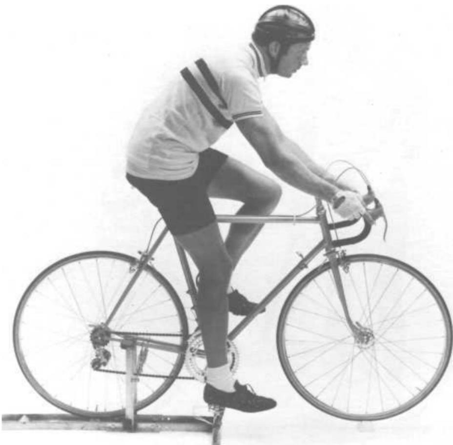
Figure 20-2: Setting saddle height. The saddle height should be adjusted with the rider on the bicycle with both heels on the pedals. Adjust the height of the saddle to allow for a slight bend in the knee at the bottom of the stroke. Quick Check: Pedal backwards with both heels on the pedals. If the hips sway, the saddle is too high.
