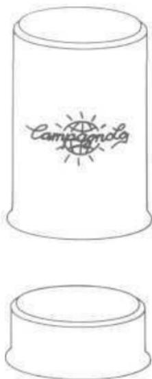
**Figure 21-3:** The plastic protective sleeve is designed to fit inside the bottom bracket on bicycles which have a cutout bottom bracket shell. The sleeve will protect the precision bearings from dirt and water during normal use.
