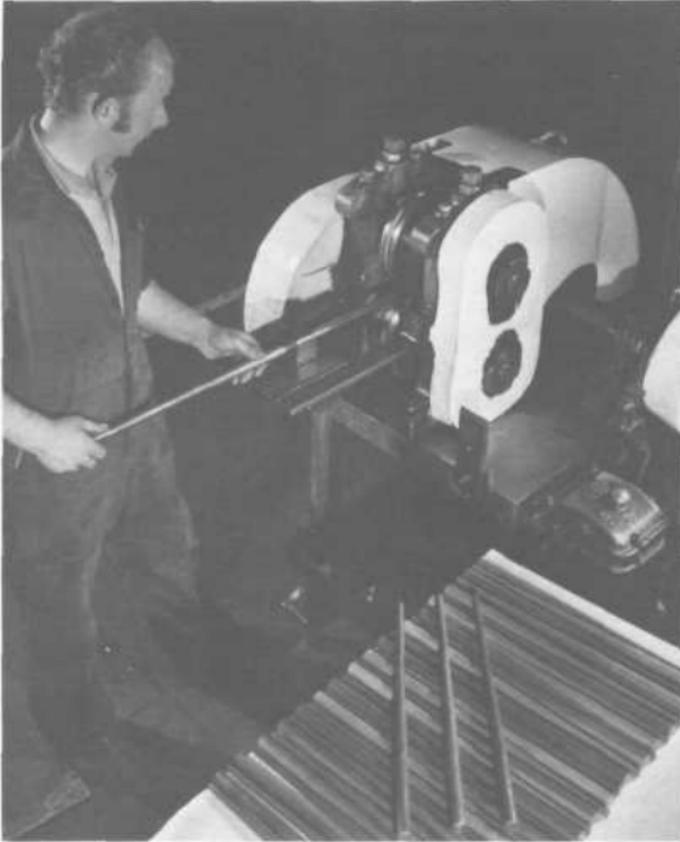
**Figure 2-3:** This method of tapering stays and fork blades is seldom used now. TI Reynolds found it difficult to locate and train persons with the necessary "touch" to feed the tubing to the machine by hand. Consequently, the process is now handled entirely by machine.
