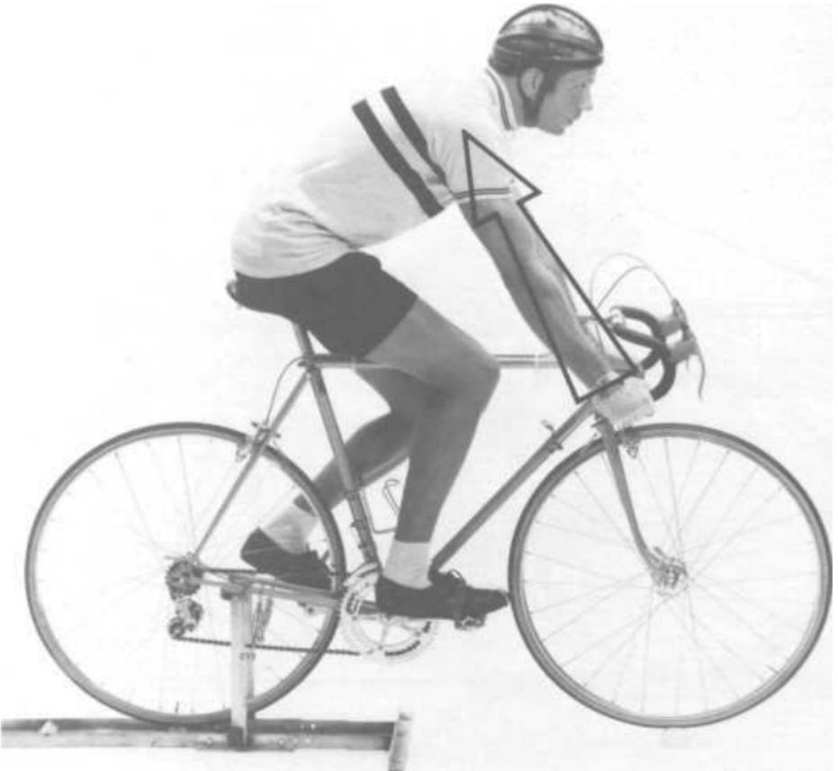
**Figure 20-10:** Incorrect handlebar position. The hands are located too far toward the ends of the handlebars and the arms are stiff. All road shock is transmitted directly into the rider's body from the wrist to the shoulder. The arm is not acting as a shock absorber.
