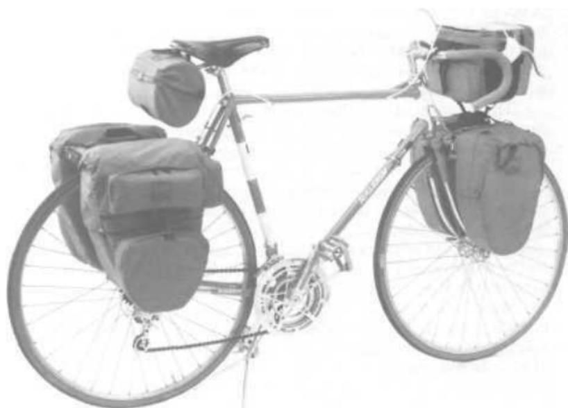
**Figure 20-17:** Proper frame loading for touring requires proportionate weight distribution and a system that minimizes the tendency of the packed materials to move.
