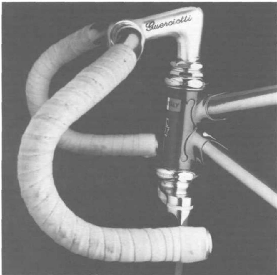
**Figure 20-14:** Correct handlebar stem adjustment. The handlebar stem should be placed far into the steering tube. If the stem is too high, the expander bolt will be located near the threaded section of the steering column. The normal stress on the stem will adversely affect the top of the steering column and it can break! The repair cost is substantial since a whole new fork would be required.
