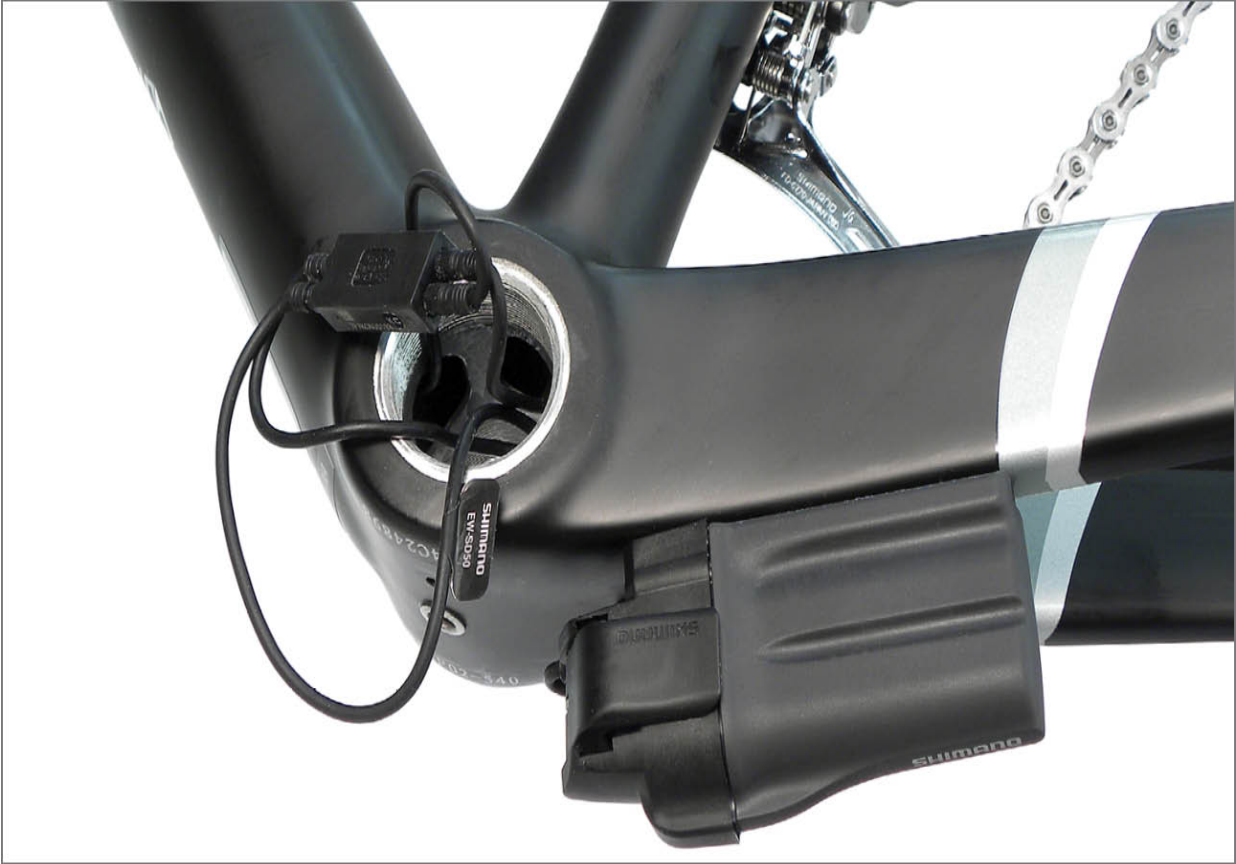
FIGURE 11.5: Internally installed junction box
