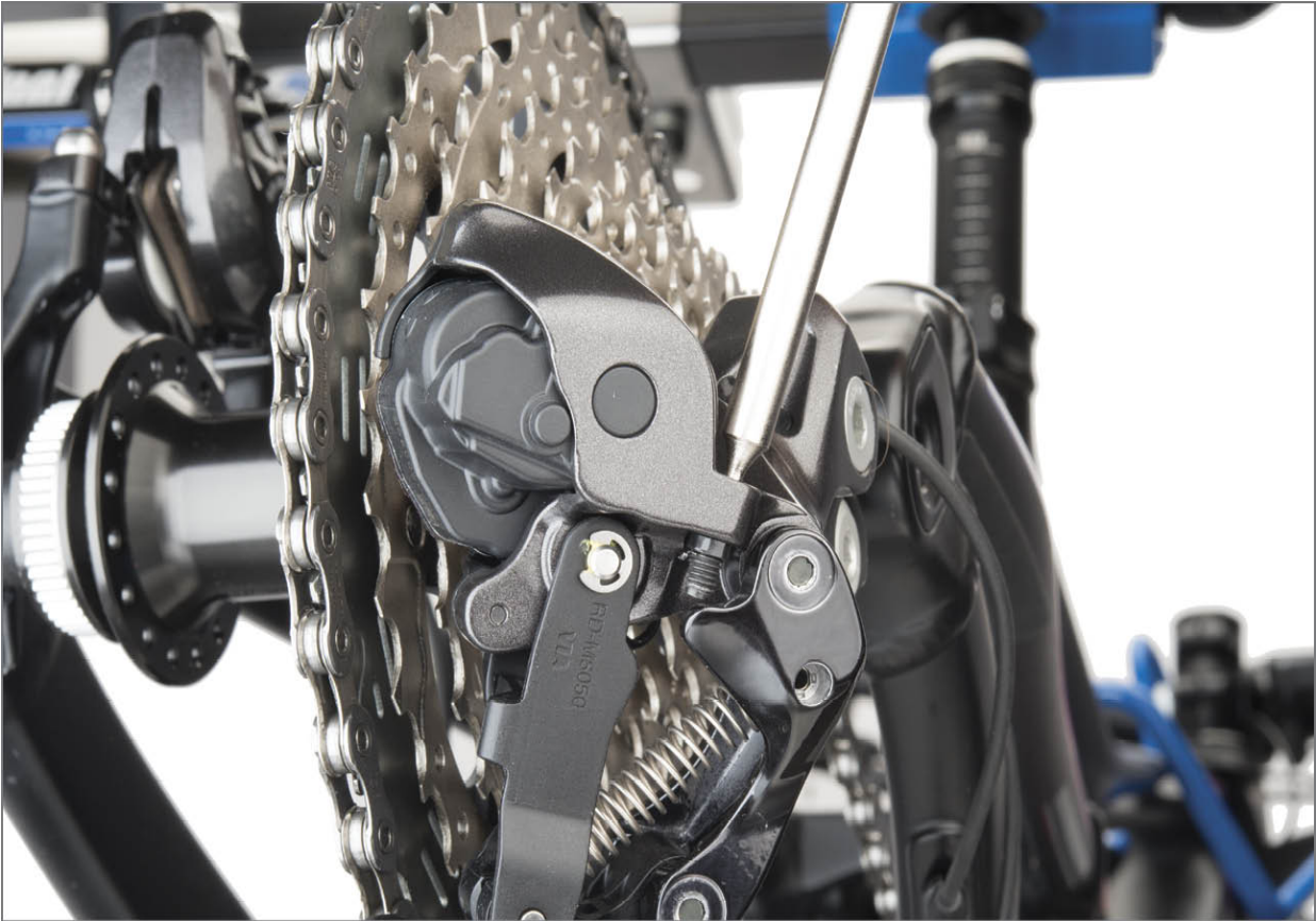
FIGURE 11.17: Tighten L-limit screw until lightly contacting linkage
