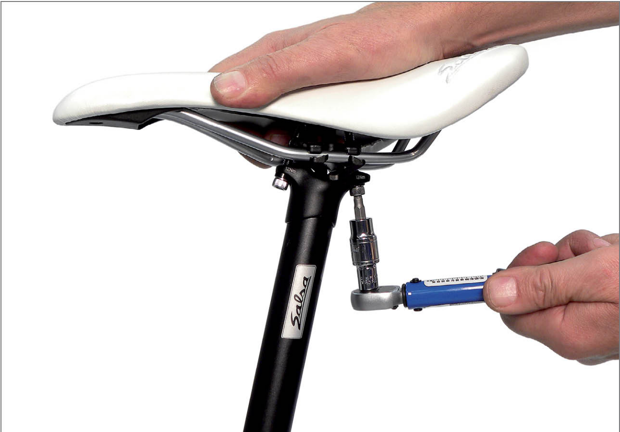
FIGURE 15.21: Secure saddle rail binder bolts by alternating tightening when two bolts are used
