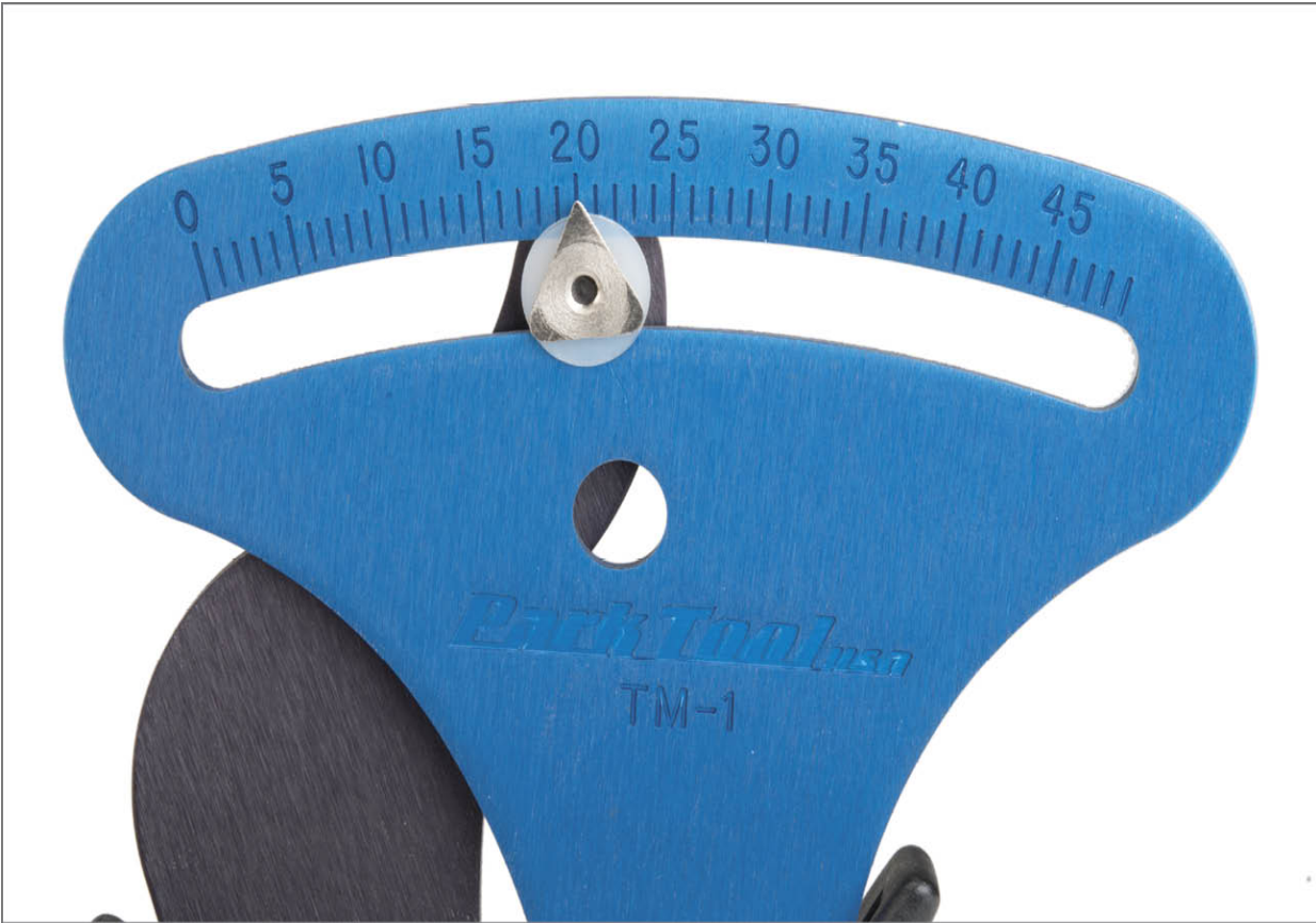
FIGURE 5.25: Deflection reading of 20 on the TM-1. Use Conversion table to determine correlated pulling force.
