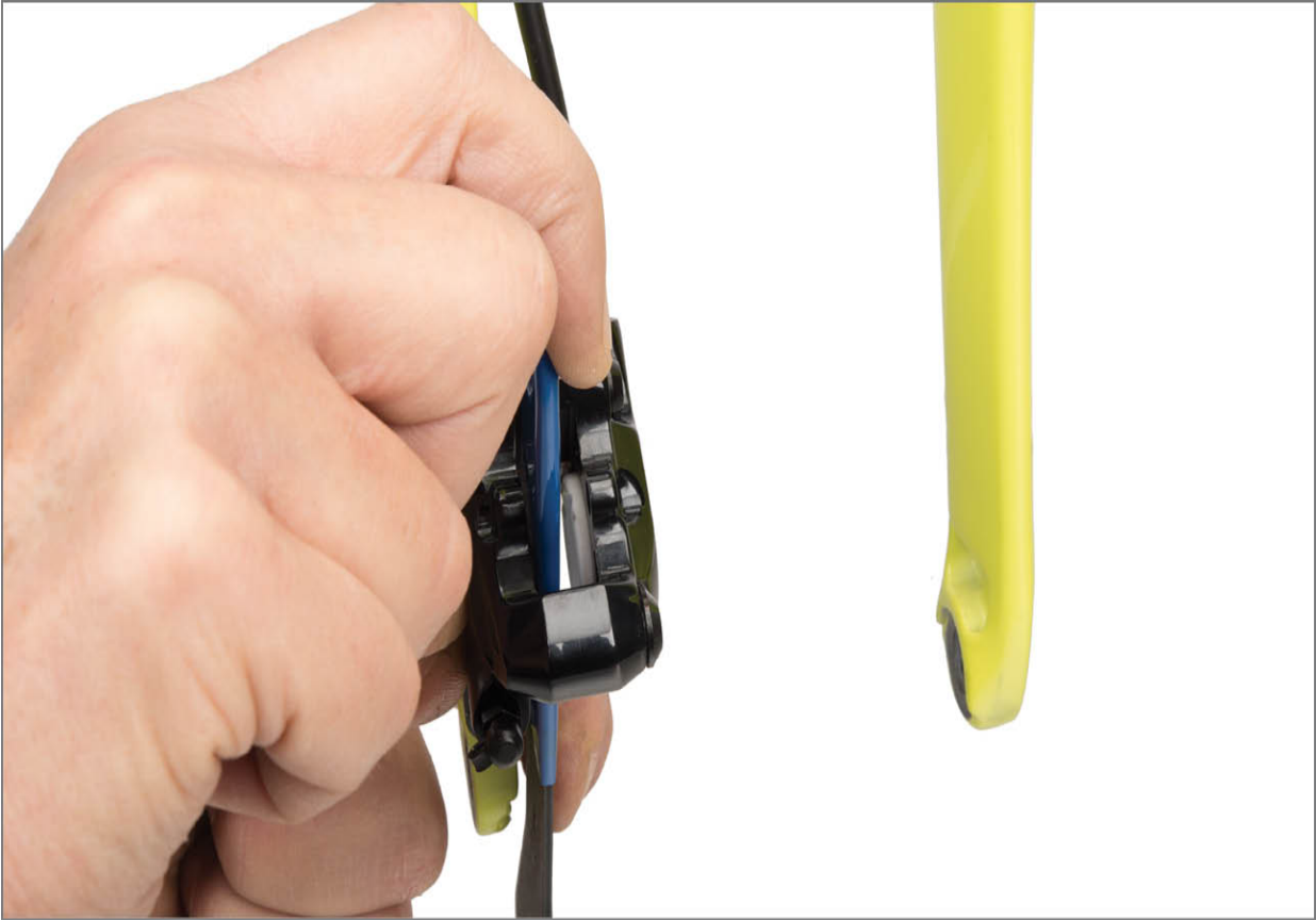
FIGURE 13.26: Push pistons back into relative sides of brake body
