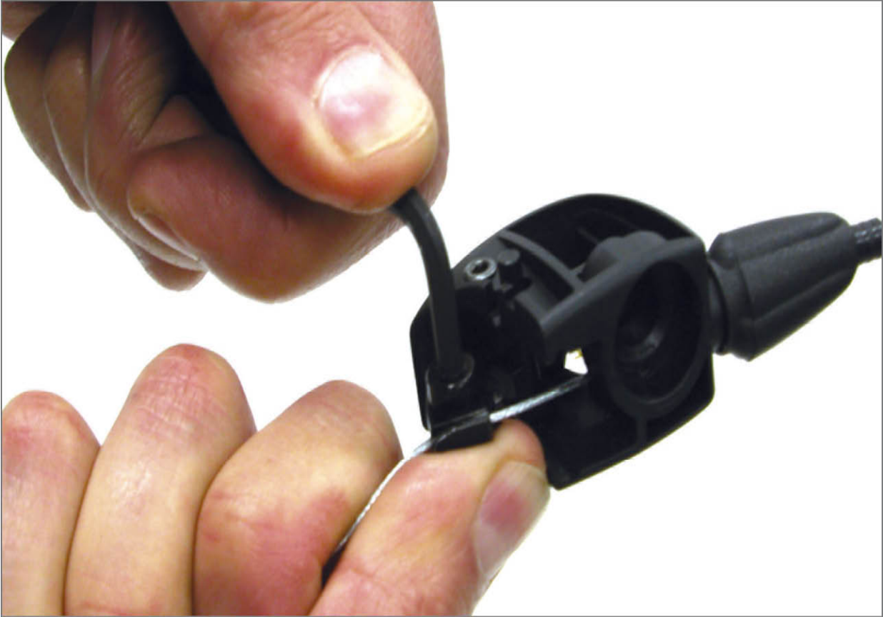
FIGURE 12.6: Pull cable snug and secure pinch bolt
