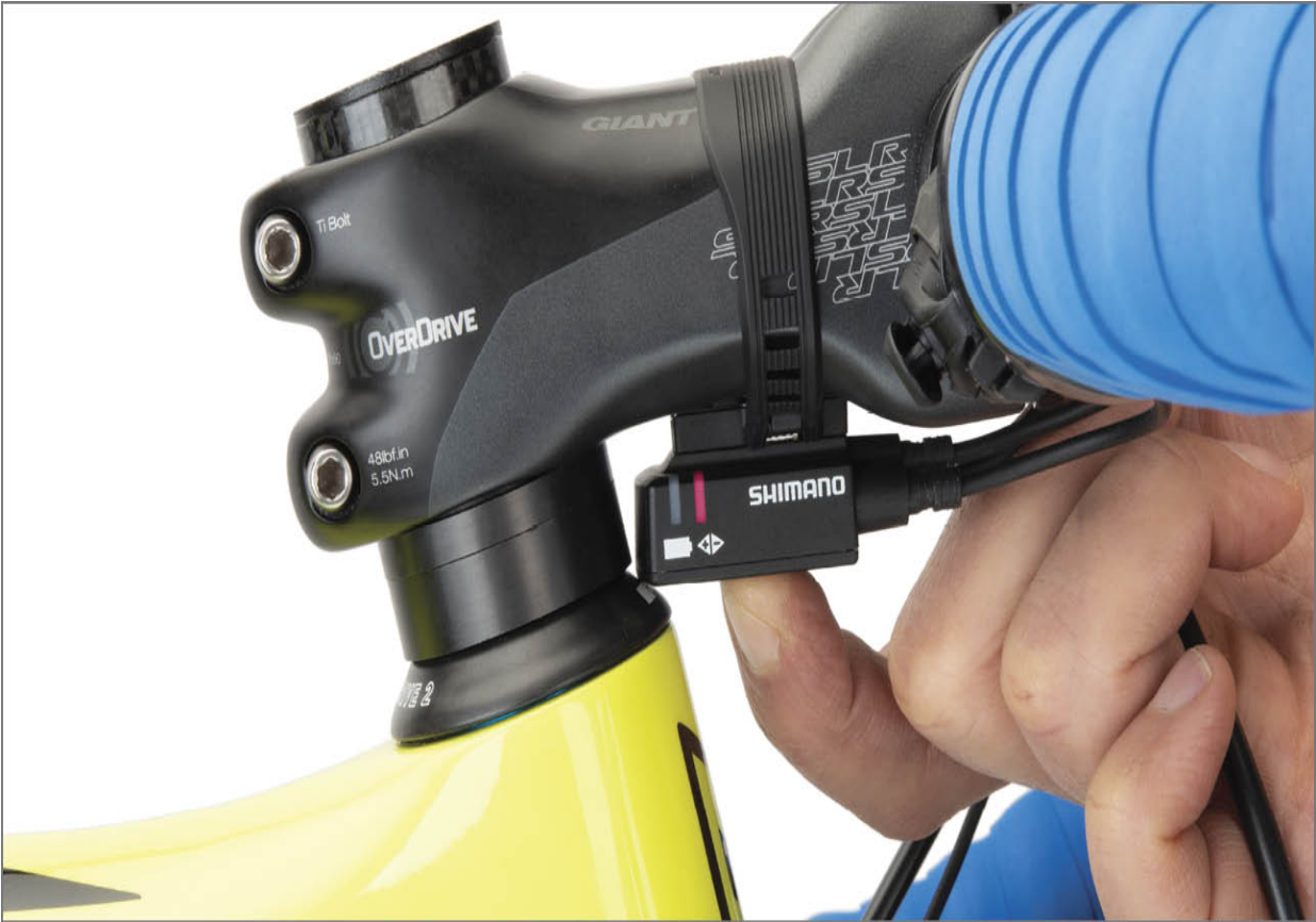
FIGURE 11.14: Press and release button at junction box to enter Adjustment Mode
