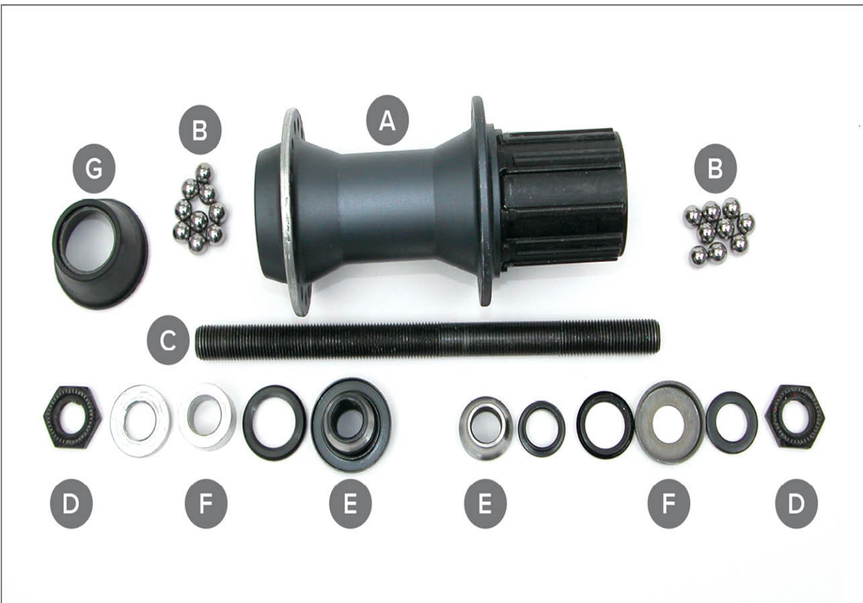
FIGURE 4.6: Parts of a common Shimano® rear hub: (A) hub shell, (B) ball bearings, (C) axle, (D) locknuts (E) cones, (F) washers, (G) rubber seal
