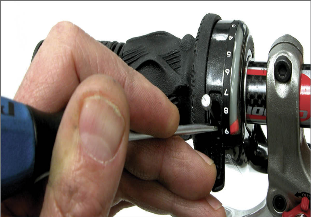
FIGURE 10.18: Use small screwdriver to access and remove cable end
