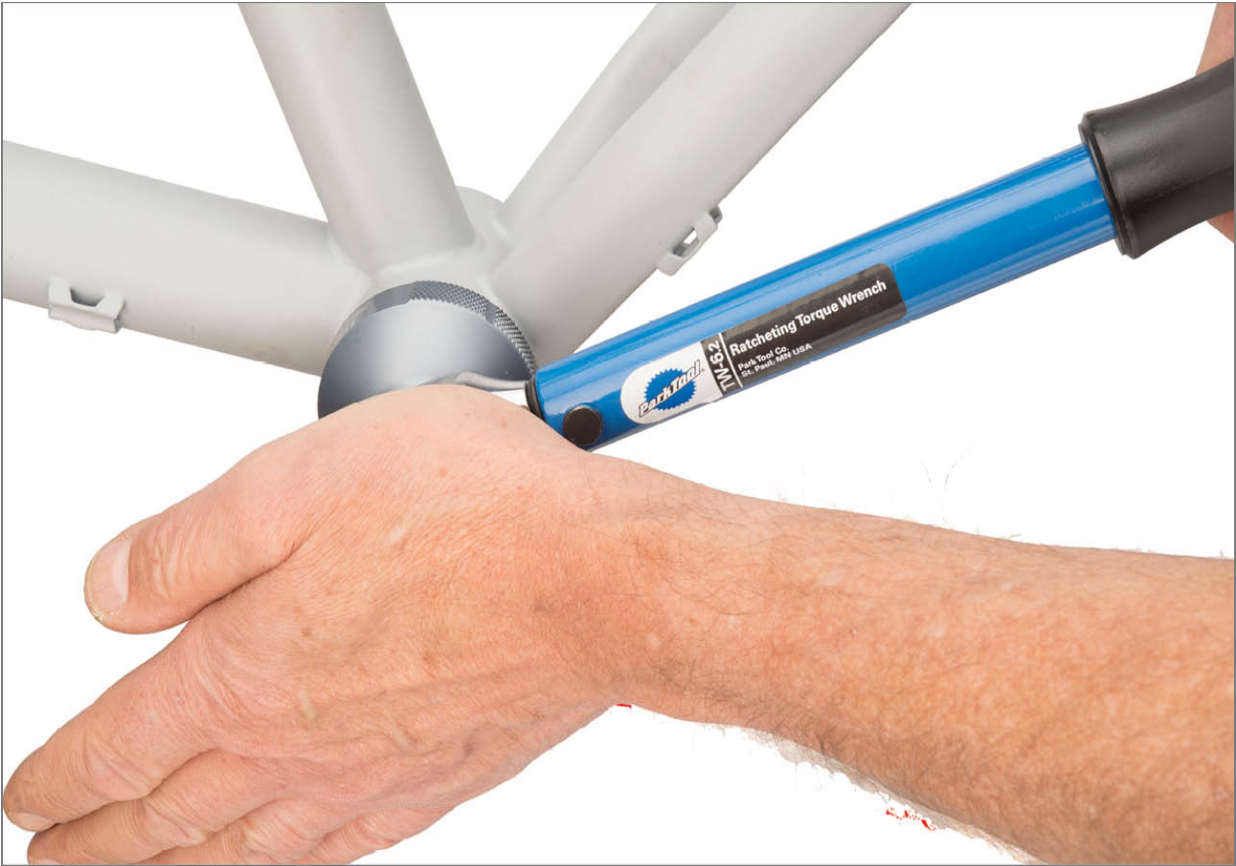
FIGURE 7.47: Hold tool firmly to bottom bracket tool fittings as it is tightened
