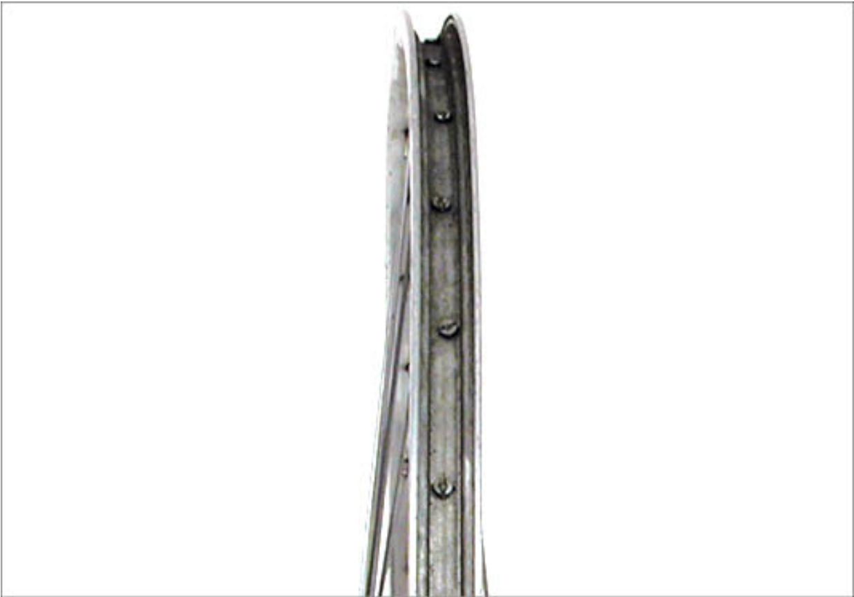
FIGURE 5.28: Wheel rim deformed beyond repair
