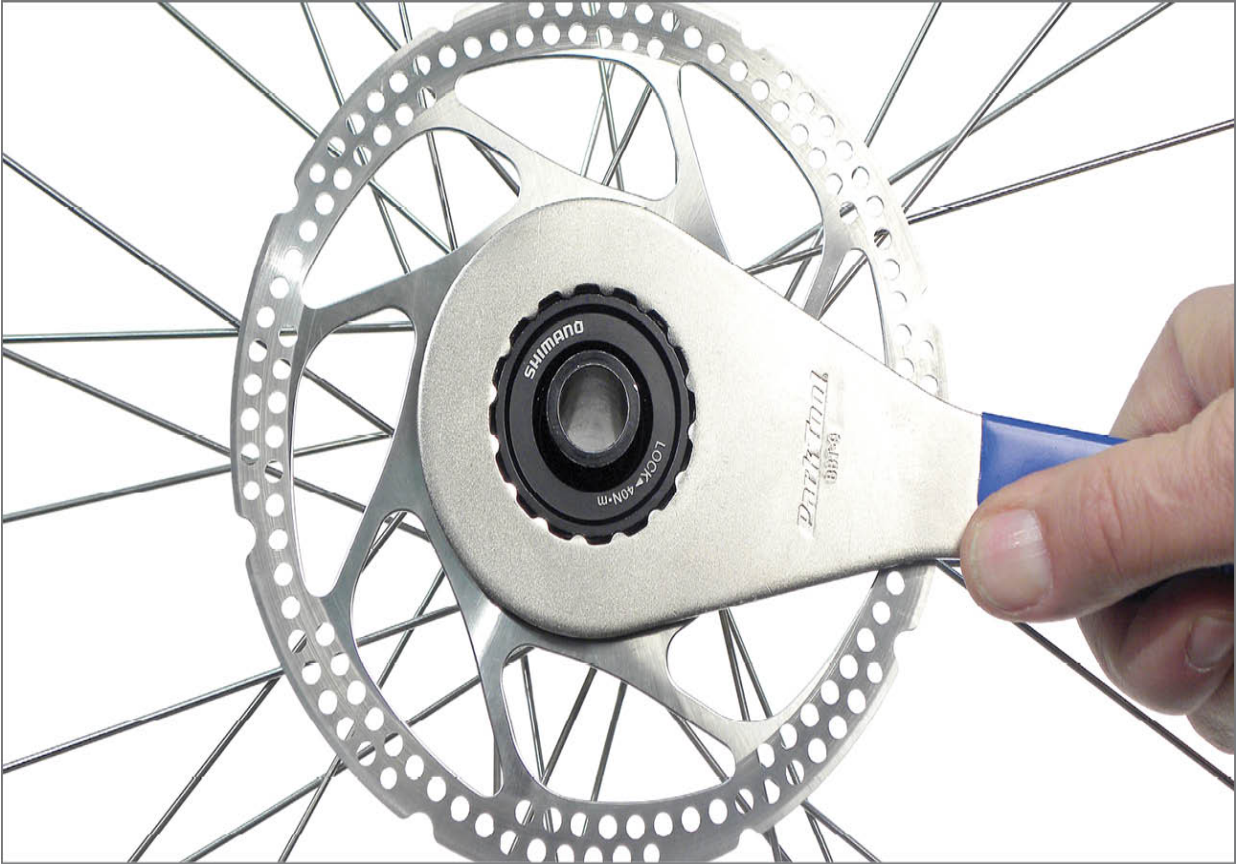
FIGURE 13.15: Center-lock rotor on thru axle hub using BBT-9
