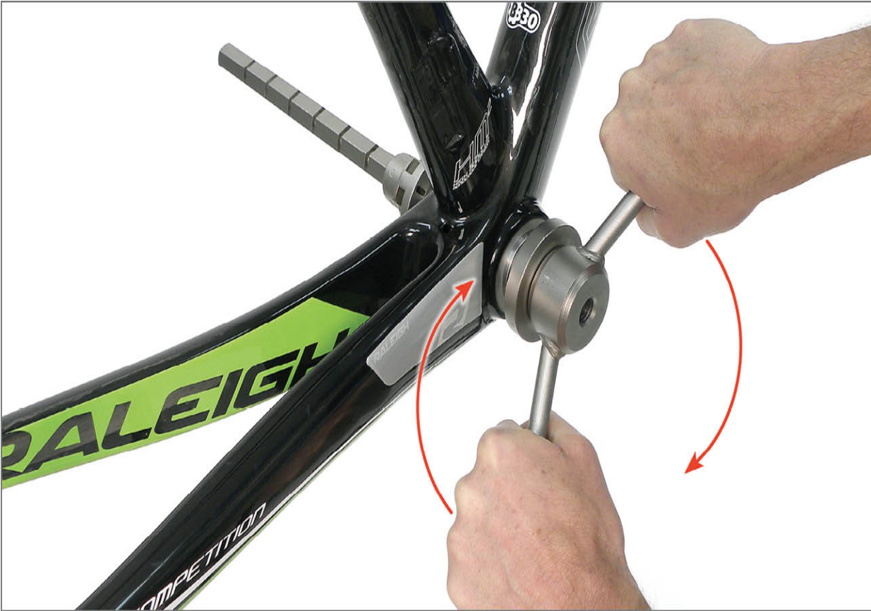
FIGURE 7.42: Press bearings with steady pressure from press until dead stop is felt
