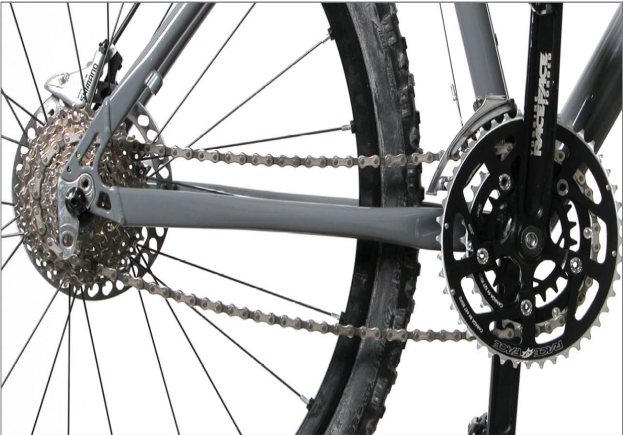
FIGURE 19.2: Bypass derailleur to create a makeshift single-speed
