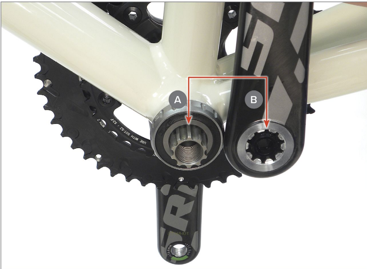
FIGURE 7.9: “Teeth” (A) of spindle must align with “grooves” (B) at crank interface
