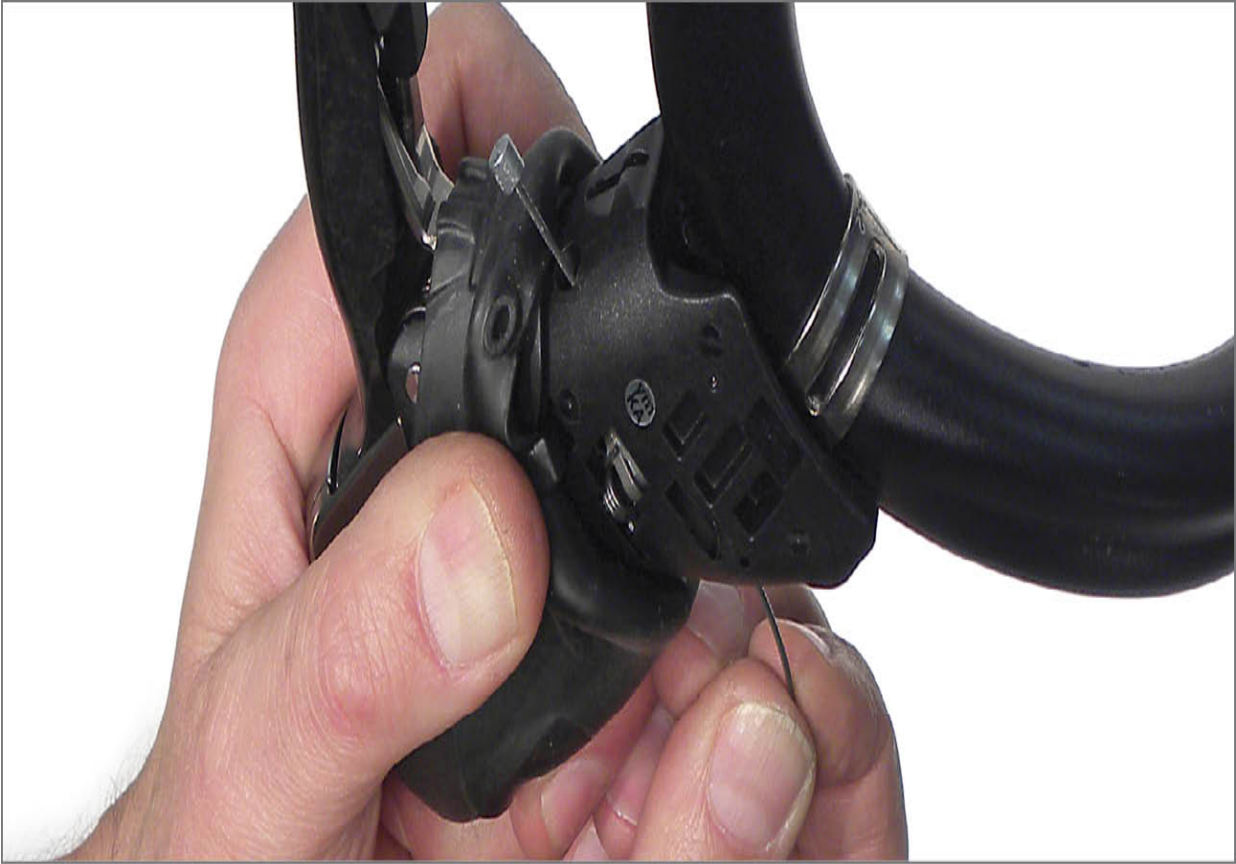
FIGURE 10.23: Cable access hole located under the lever body
