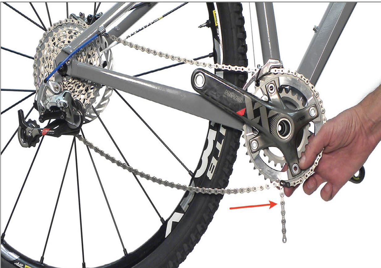
FIGURE 8.7: Wrap chain on largest front and rear sprockets without engaging rear derailleur
