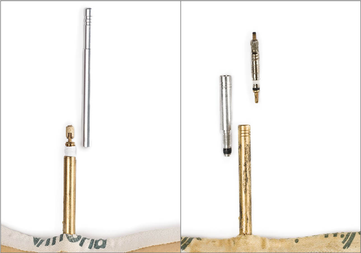
FIGURE 2.44: Left: simple valve extender with locknut loose Right: removable valve core with double-threaded extender
