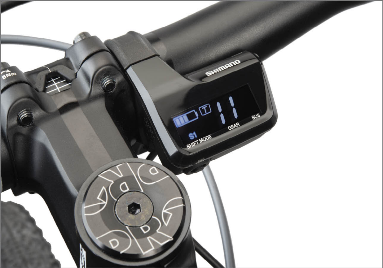
FIGURE 11.4: MTB Di2 junction box with display of gear, mode and battery life
