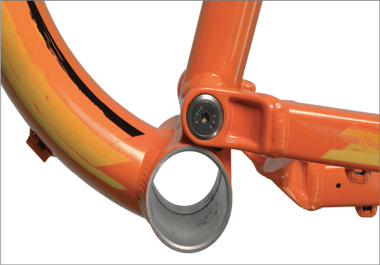
FIGURE 7.35: Left side (non-drive) of PF30 bottom bracket shell seen on full suspension frame
