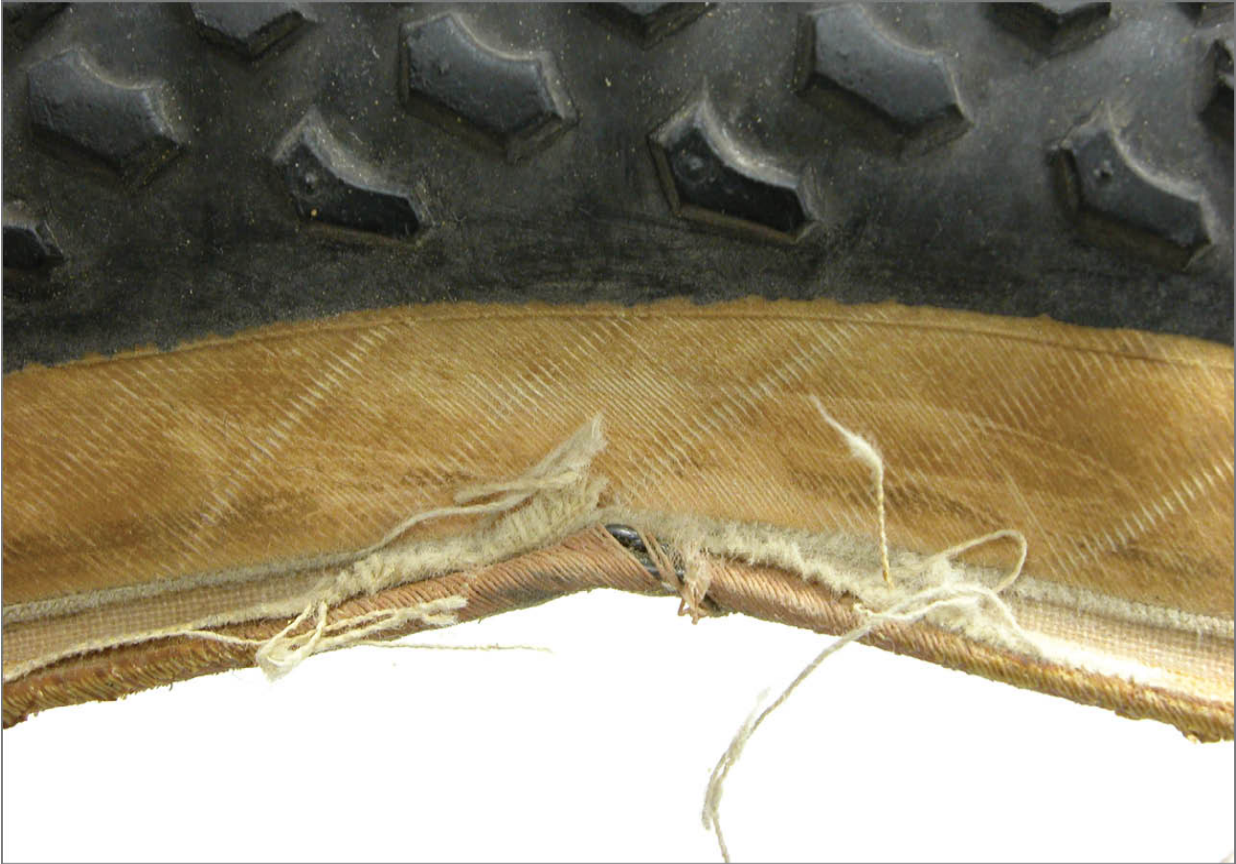
FIGURE 2.26: Failure of tire bead cannot be repaired
