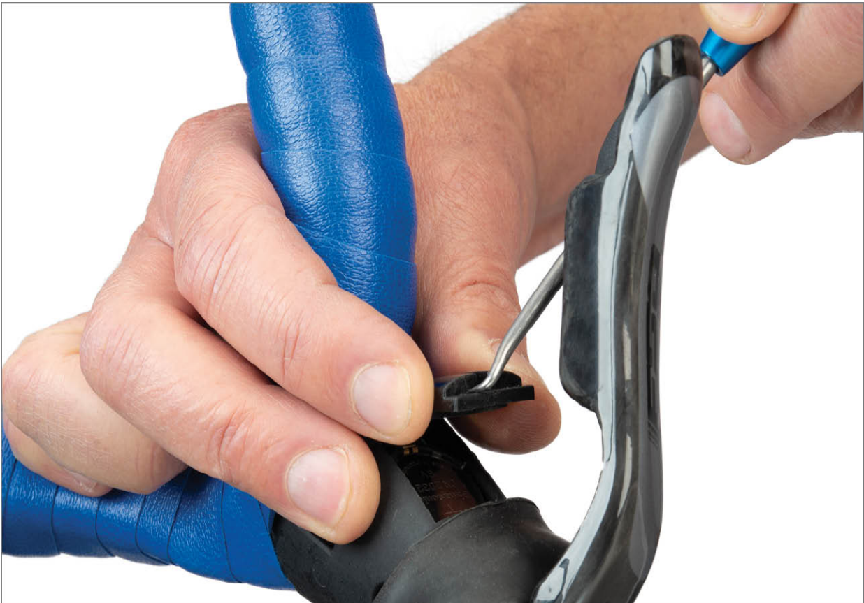
FIGURE 11.25: Battery cover below shift lever body
