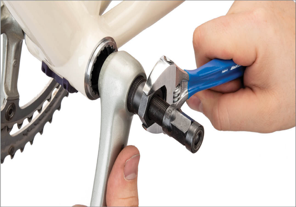
FIGURE 7.10: Thread and tighten hex fitting of puller securely into crank threads before extracting crank
