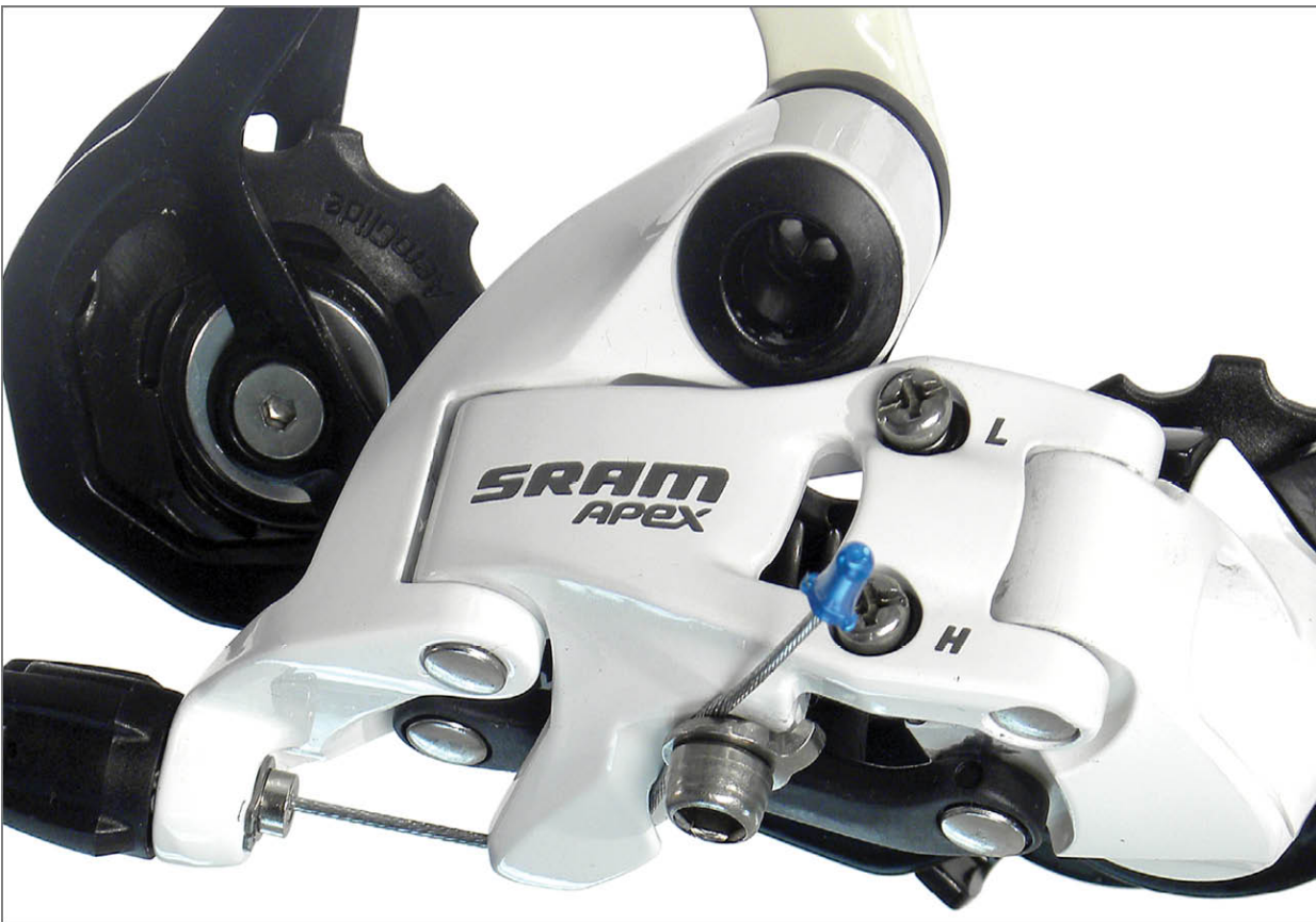
FIGURE 10.57: Derailleur cable routing through pinch mechanism
