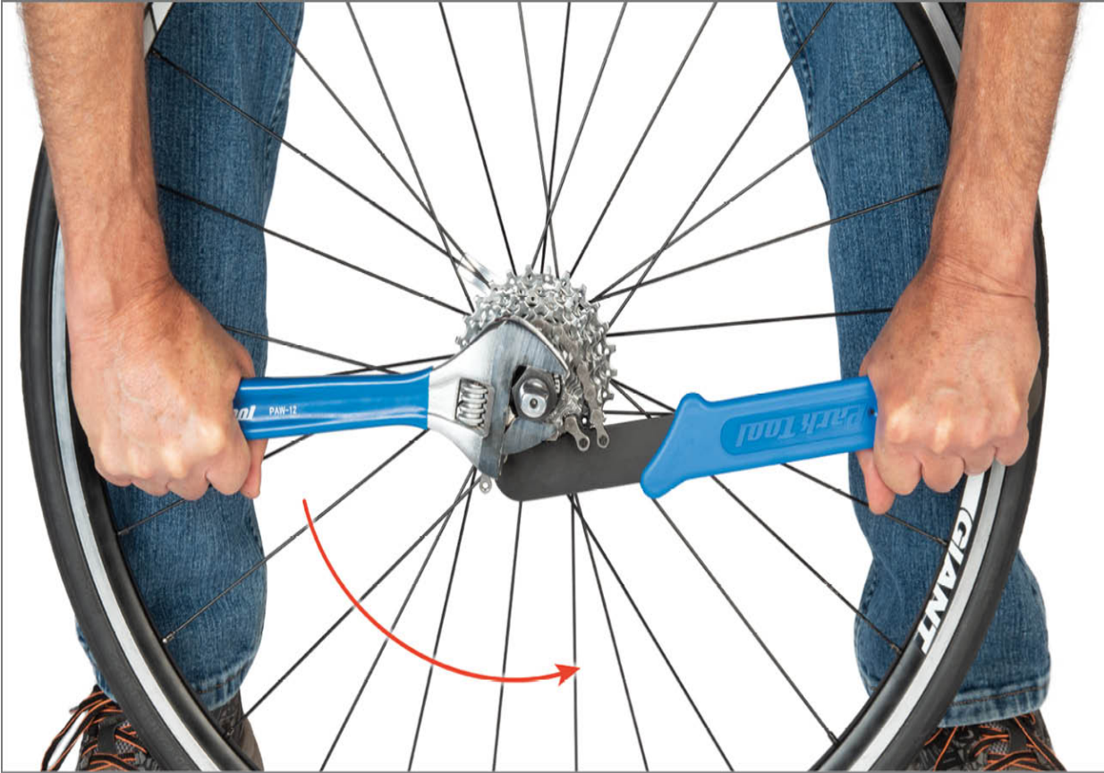
FIGURE 3.5: Use body weight to help loosen lockring, with wrenches
