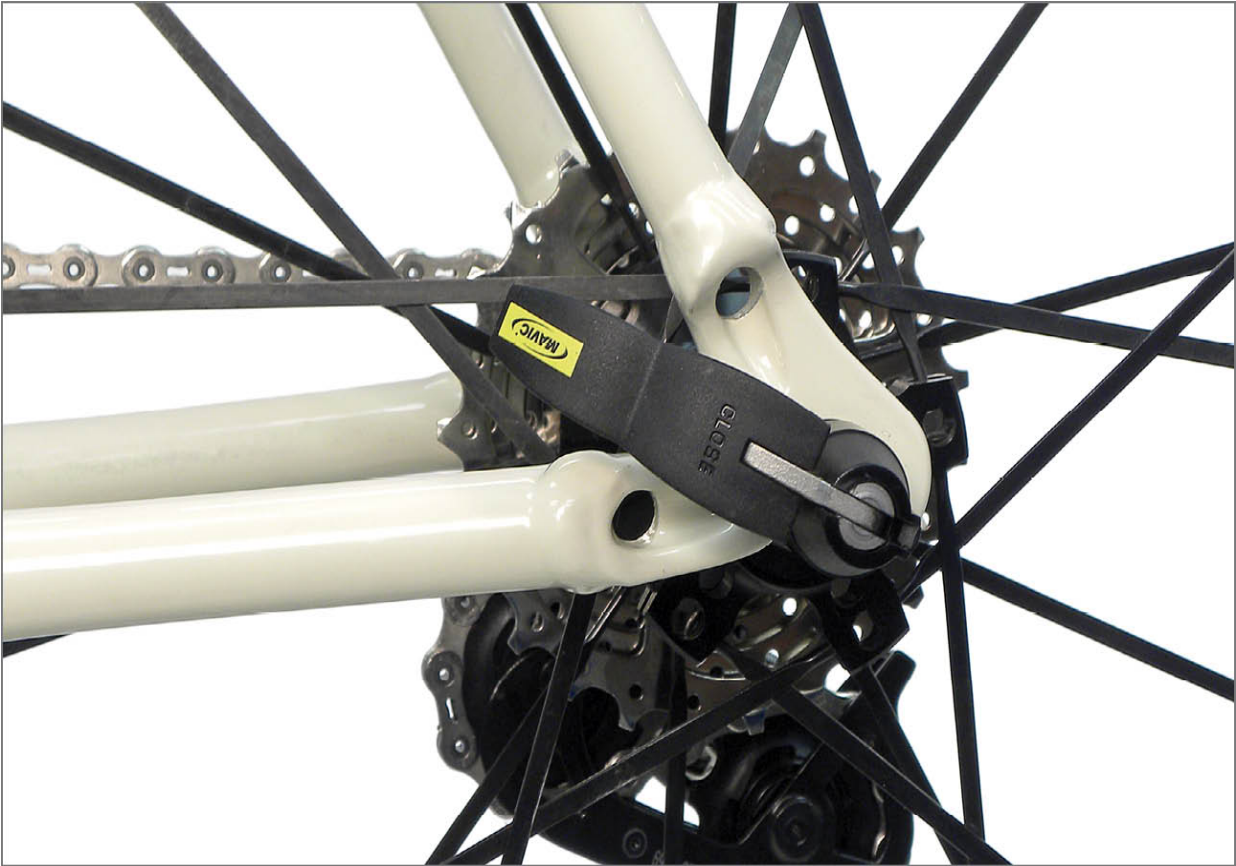
FIGURE 2.70: Align lever between chain and seat stays
