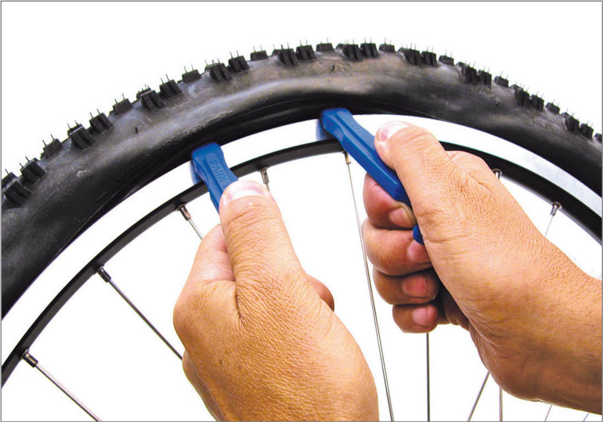
FIGURE 2.18: Engage tire levers under tire bead and lift
