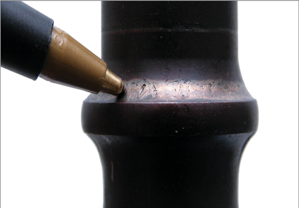
FIGURE 7.64: Trace bearing surfaces to feel for roughness and pits
