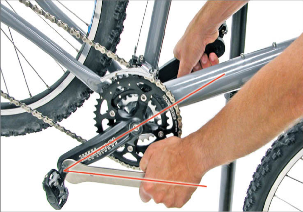
FIGURE 9.4: Good mechanical advantage for securing pedals
