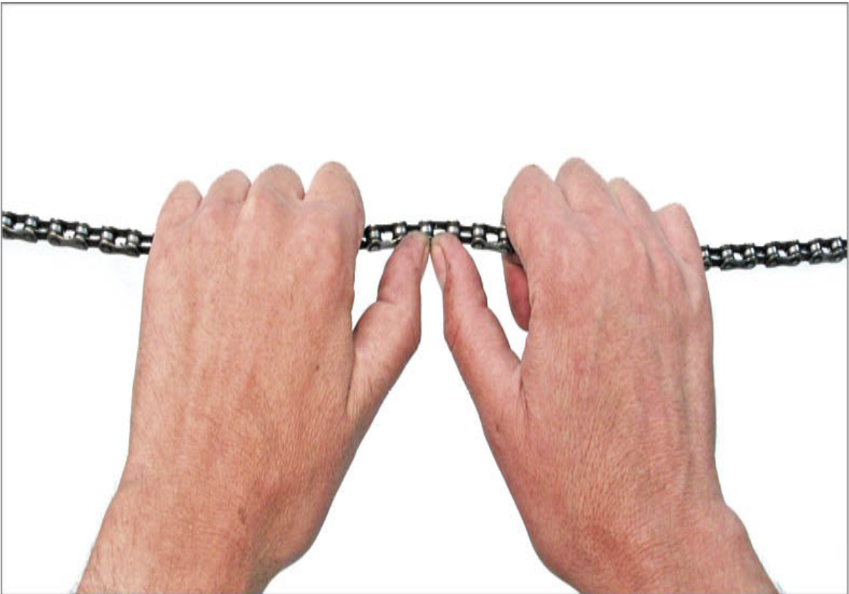
FIGURE 8.27: Grab chain and flex laterally at tight link
