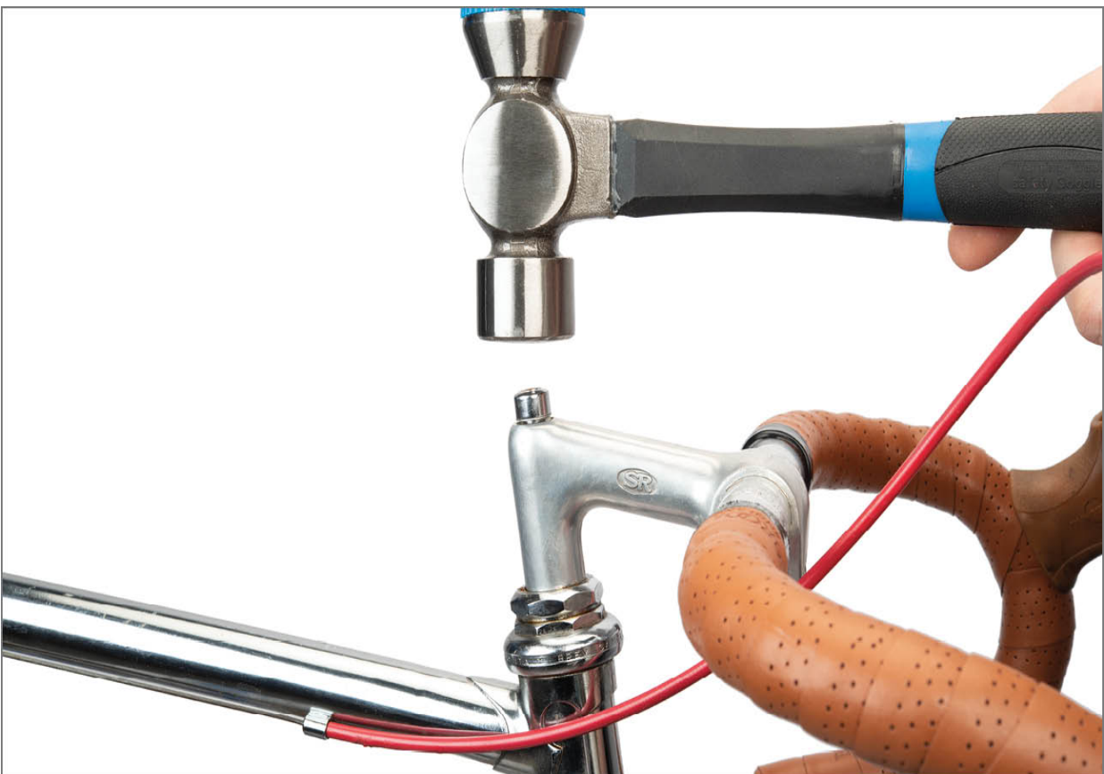
FIGURE 16.18: Drive stem binder downward to free stem from column
