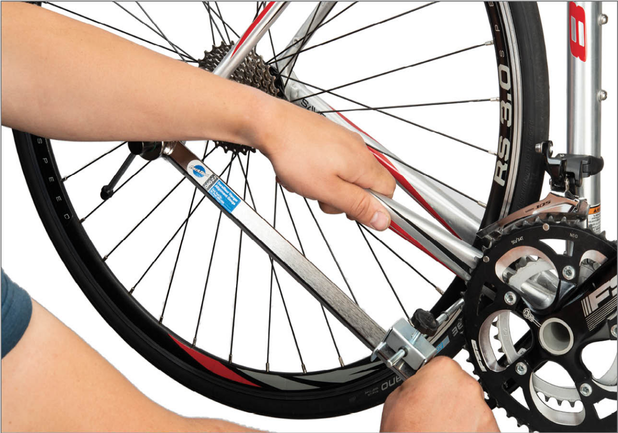
FIGURE 10.73: Use frame to leverage and control bending of hanger
