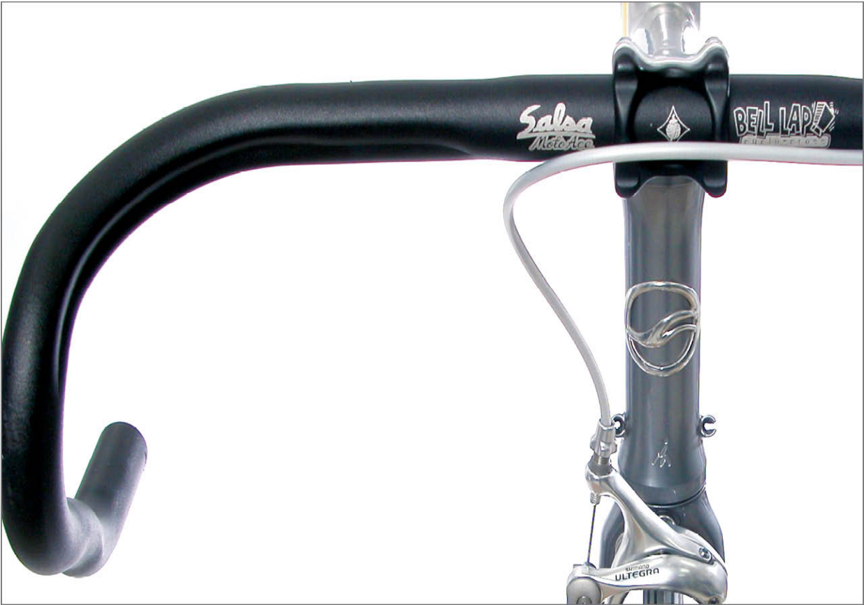
FIGURE 14.10: Housing passes housing stop, indication housing is too long
