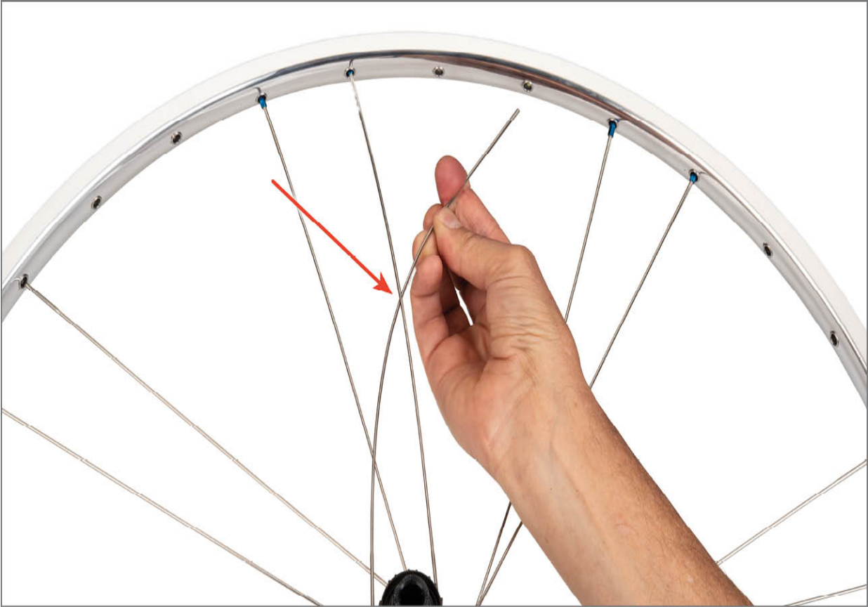
FIGURE 6.21: Third set spokes are flexed to go under the first set spokes at cross
