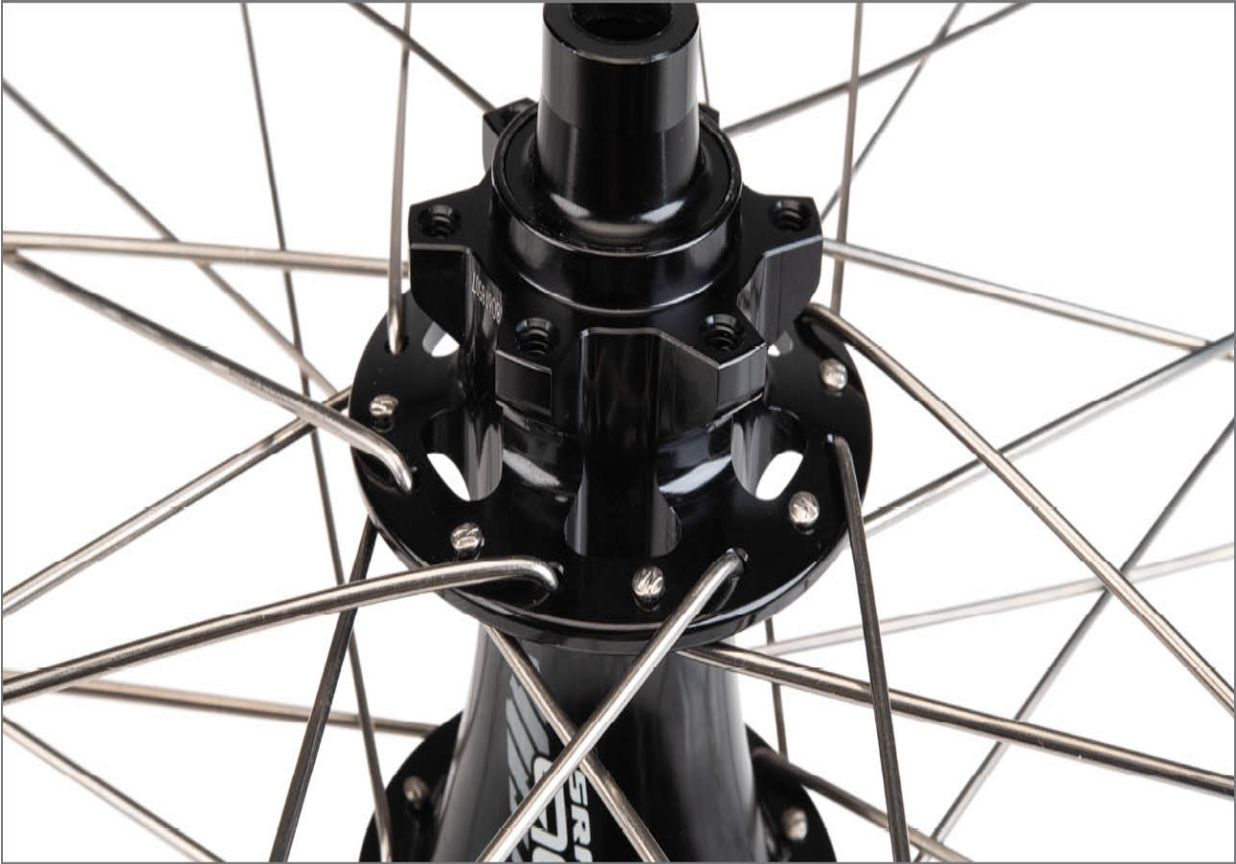
FIGURE 6.3: J-bend spokes in compatible hub
