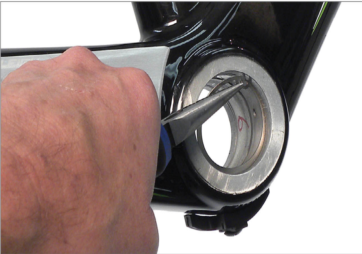
FIGURE 7.44: Remove C-clips bearing stops in shell before installing conversion adaptor
