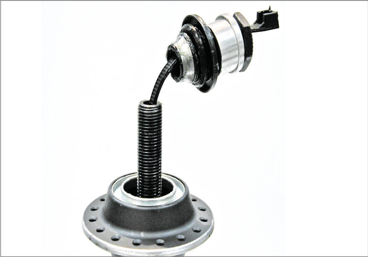
FIGURE 4.9: Hold parts together in disassembly order with zip tie or string
