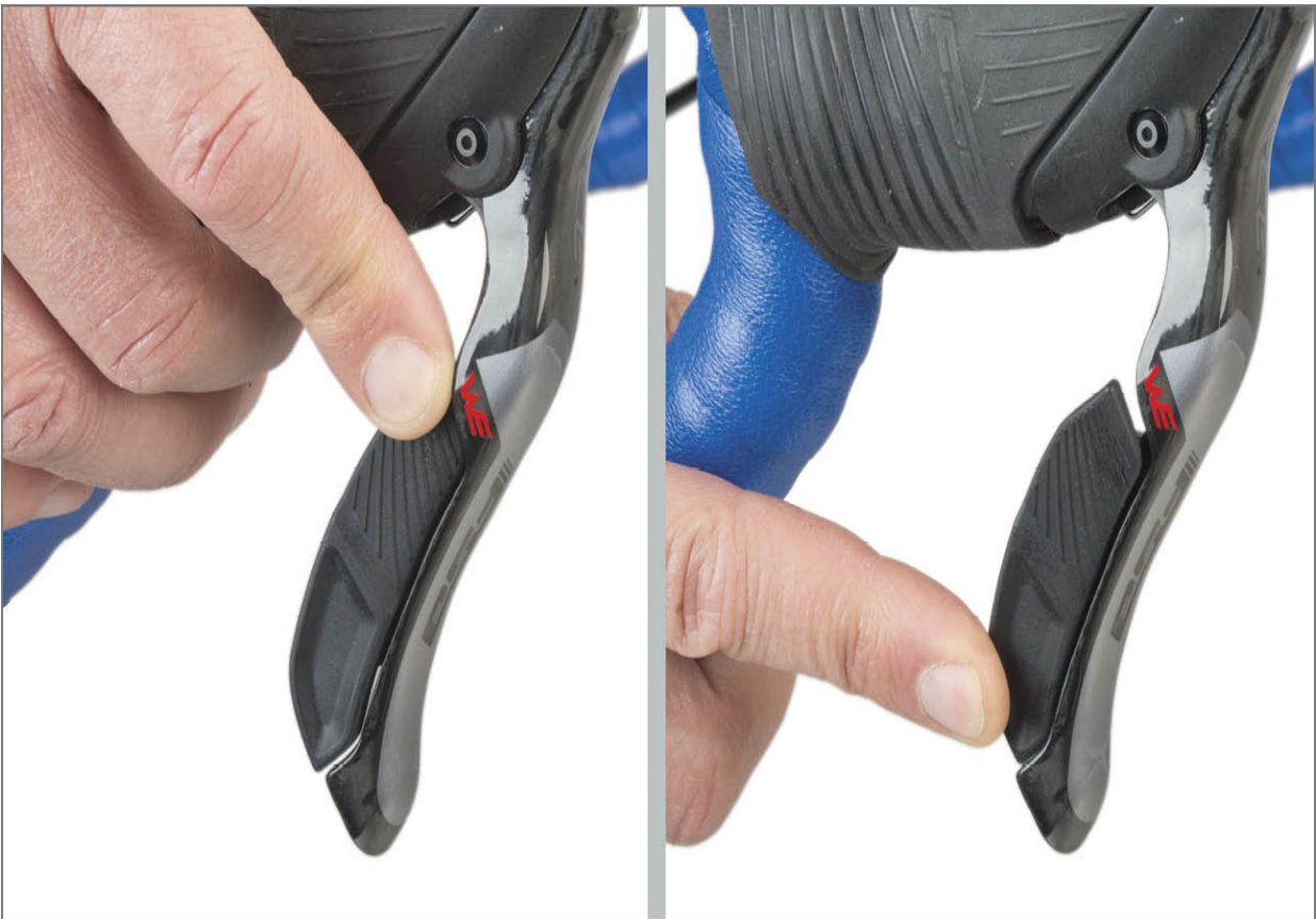
FIGURE 11.24: Rear derailleur inward and outward portion of shift paddles
