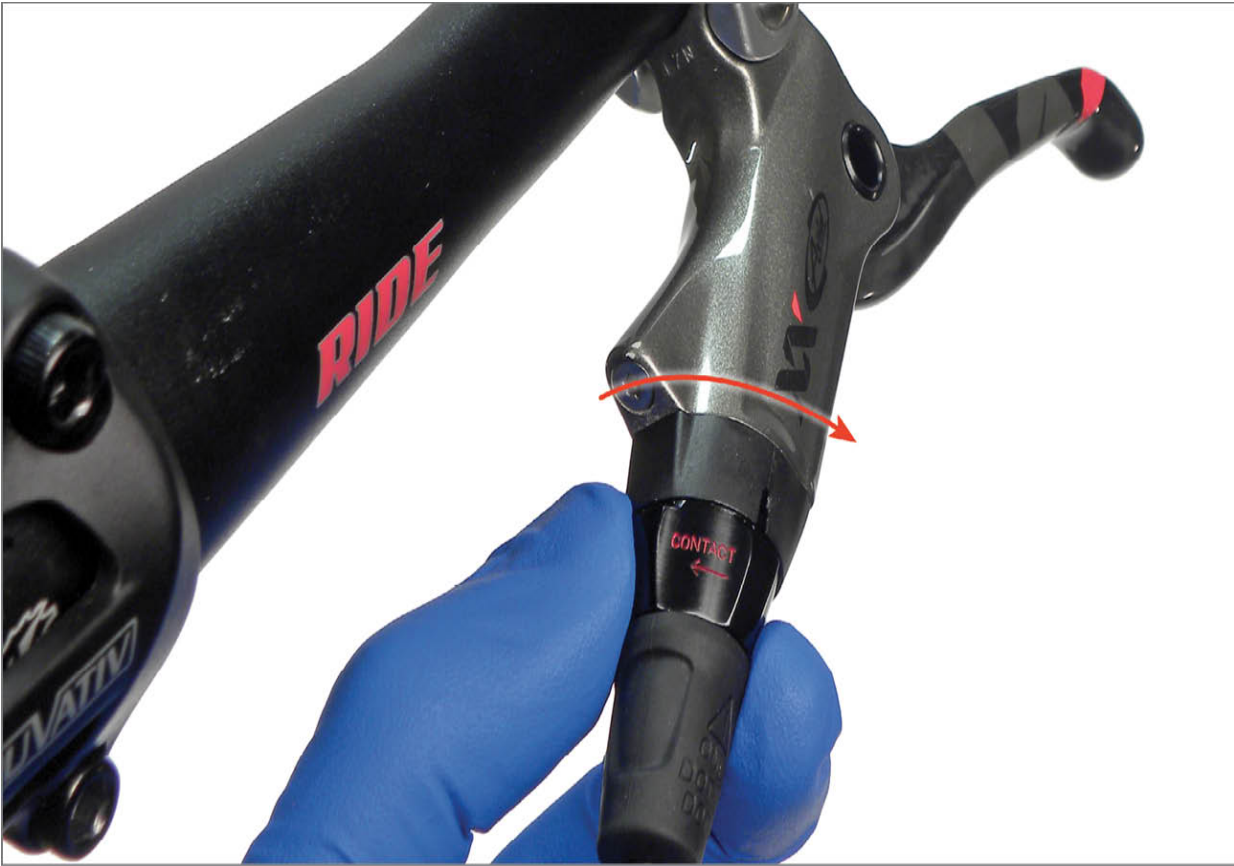
FIGURE 13.45: Adjust contact adjusting knobs
