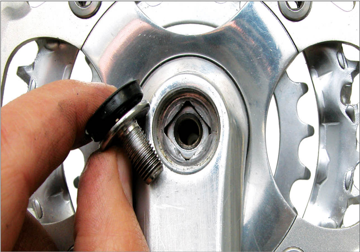
FIGURE 7.3: Square crank hole with square spindle inside
