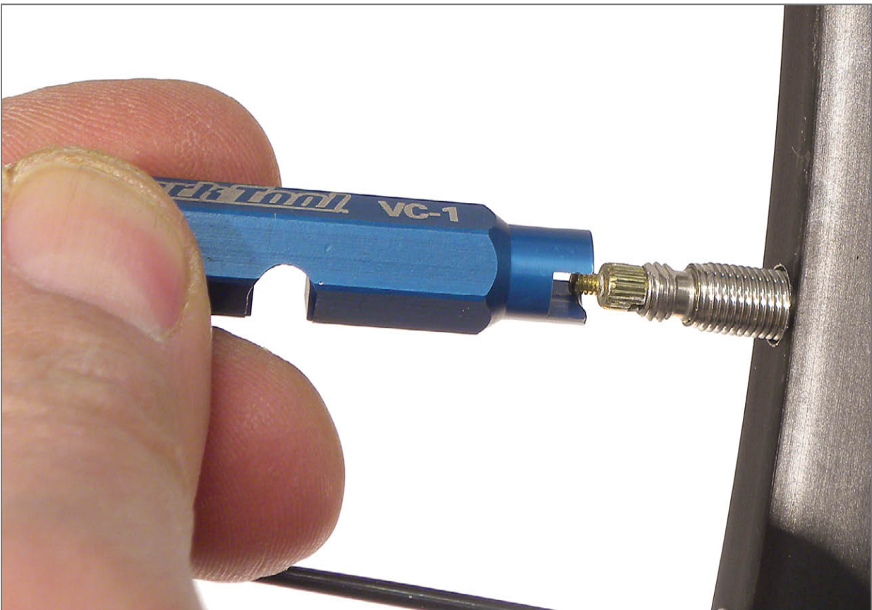
FIGURE 2.35: Inspect end of Presta valve for wrench flats
