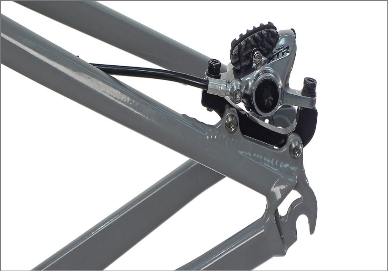
FIGURE 13.3: International Standard (IS) mounting system holding a caliper mounted to a Post Mount (PM) adaptor
