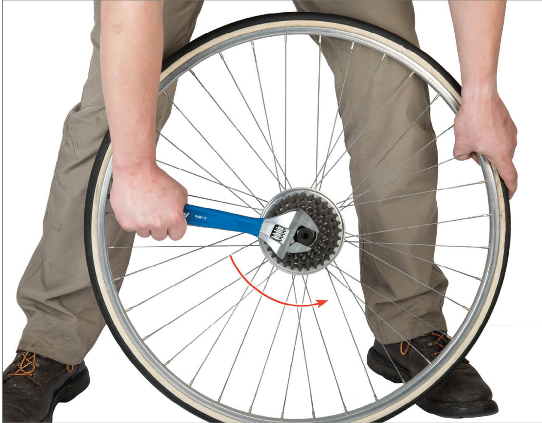
FIGURE 3.10: Turn tool counterclockwise to loosen freewheel
