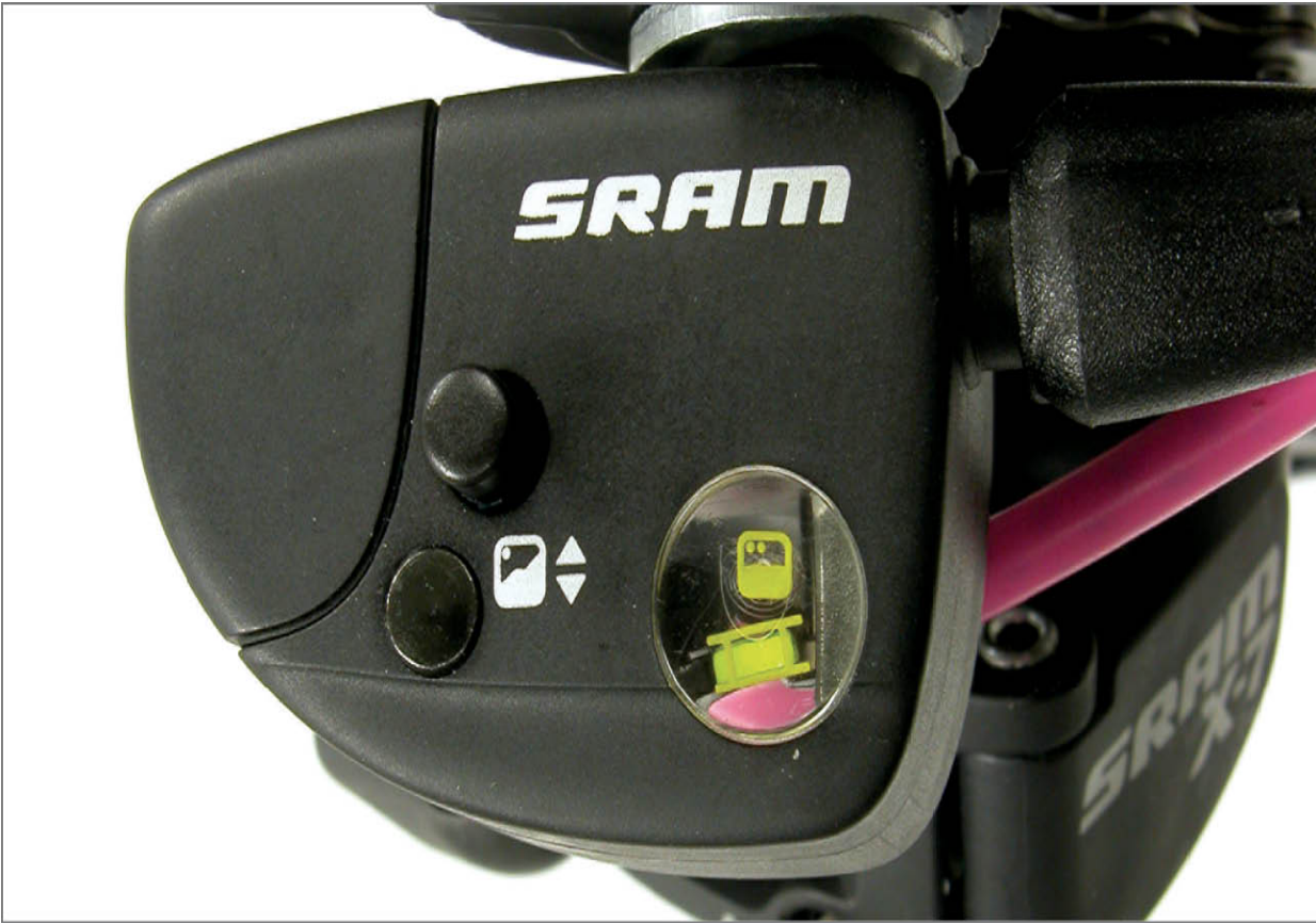
FIGURE 12.3: Adjust cable tension until yellow mark is aligned between lines
