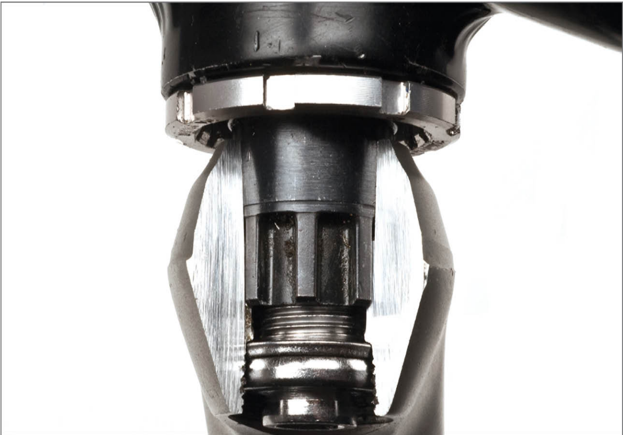
FIGURE 1.3: Bolt under tension creates pressure to keep the crank pressed securely to spindle
