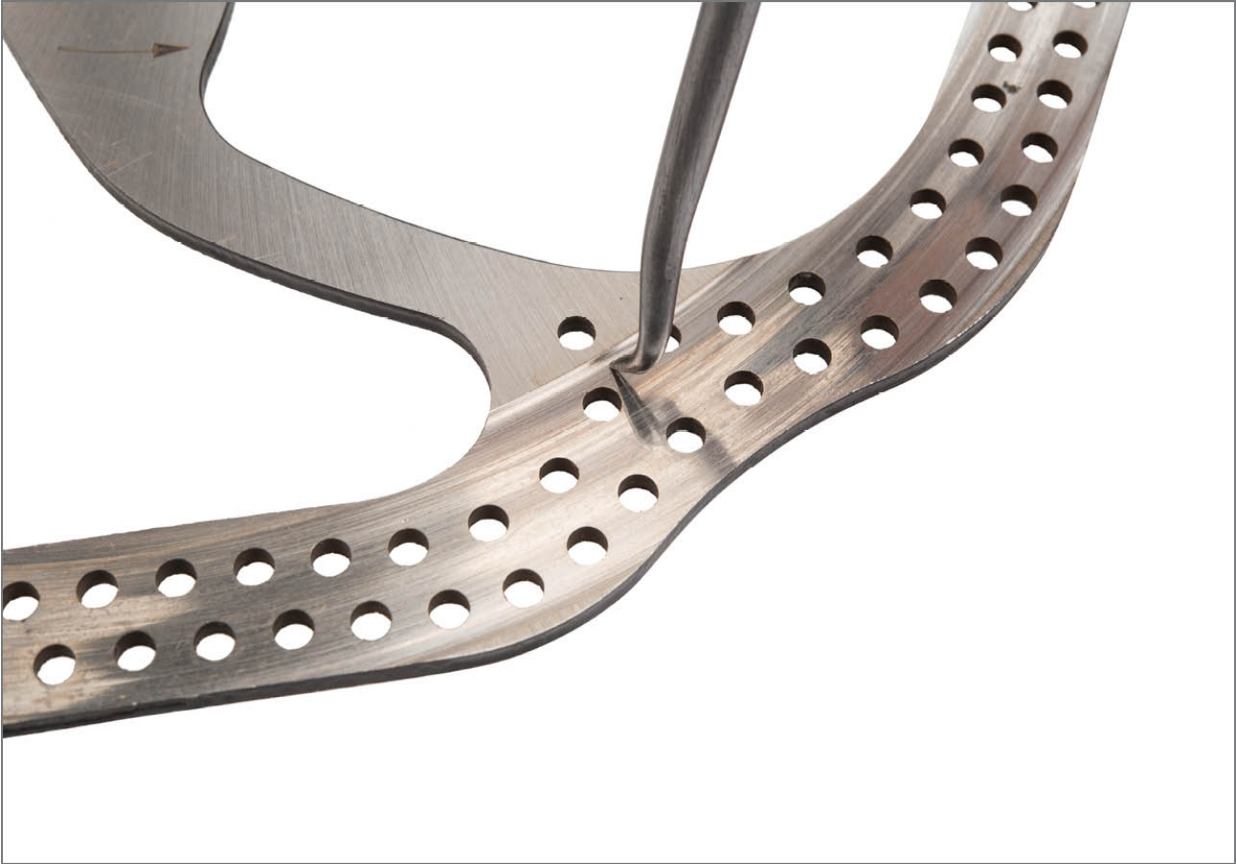
FIGURE 13.16: An obvious step in braking surface from pad wear requires rotor replacement
