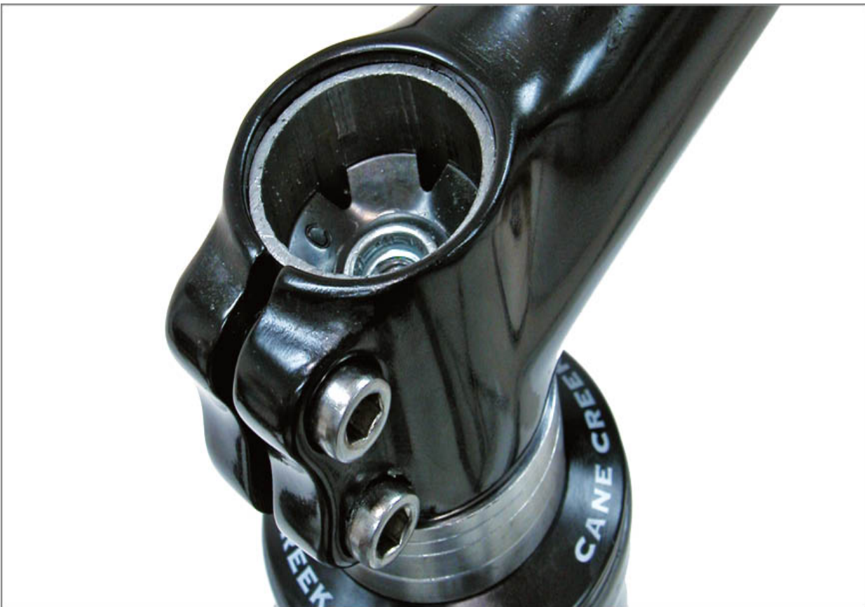
FIGURE 16.12: Steel and aluminum steering columns can be recessed below top of stem
