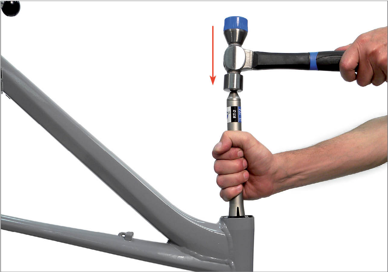
FIGURE 16.23: Drive race from head tube with race tool and hammer
