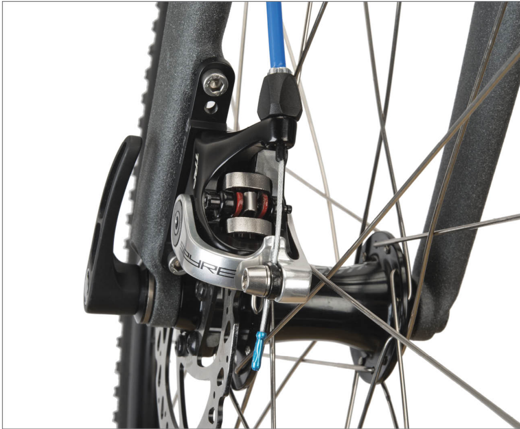
FIGURE 13.63: The double lever arm design moving both pads to the rotor
