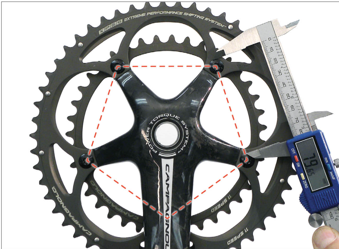
FIGURE 7.67: Measure one cord of pentagon by measuring from bolt-to-bolt
