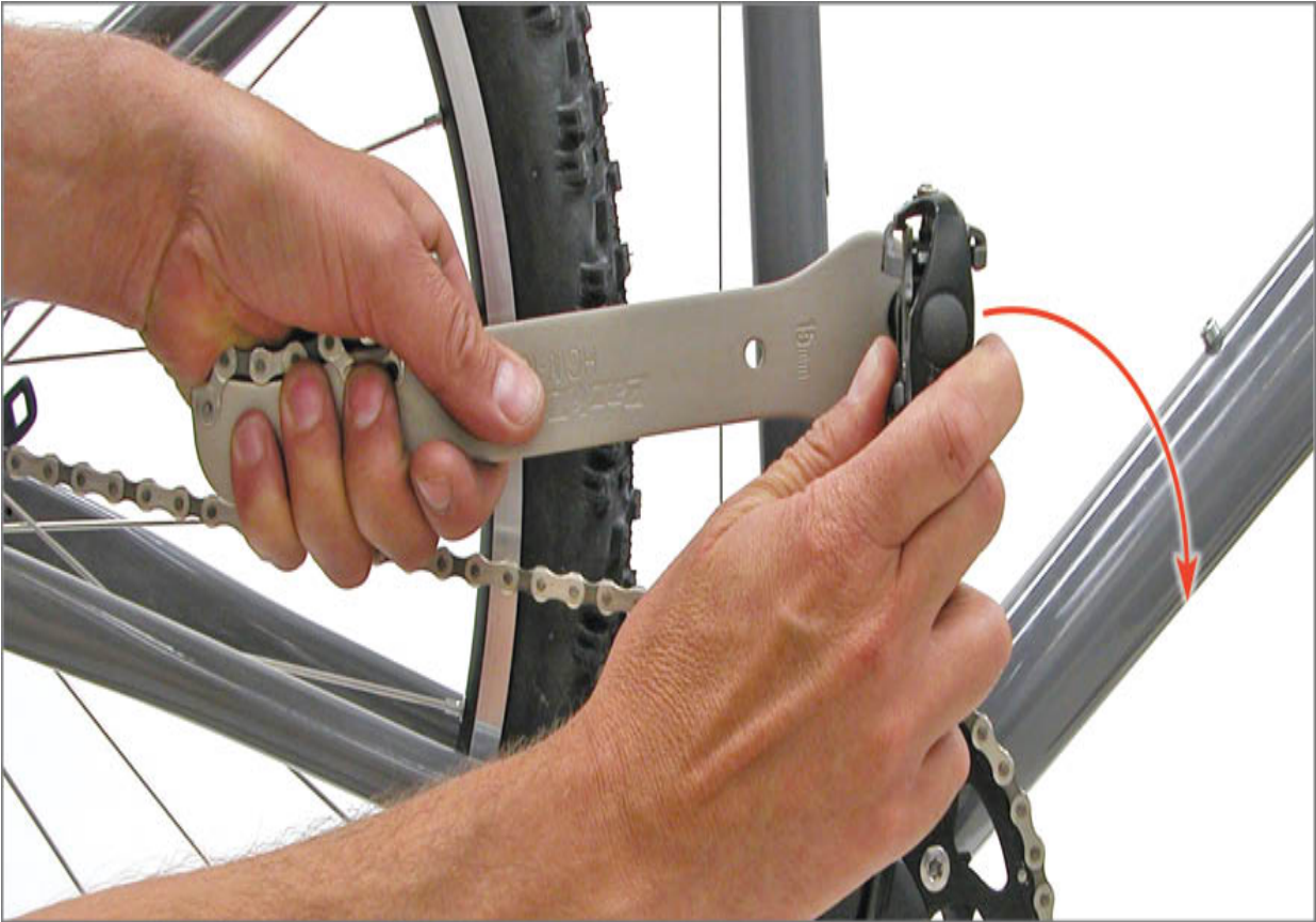
FIGURE 9.2: Pedal in a forward direction to remove pedal from cranks
