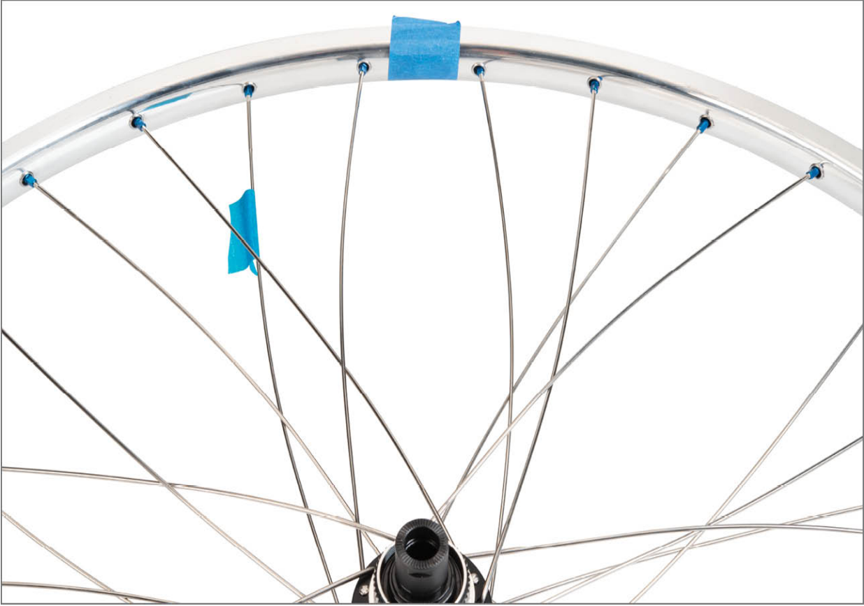
FIGURE 6.24: Check the set of spokes is interlaced at crossing
