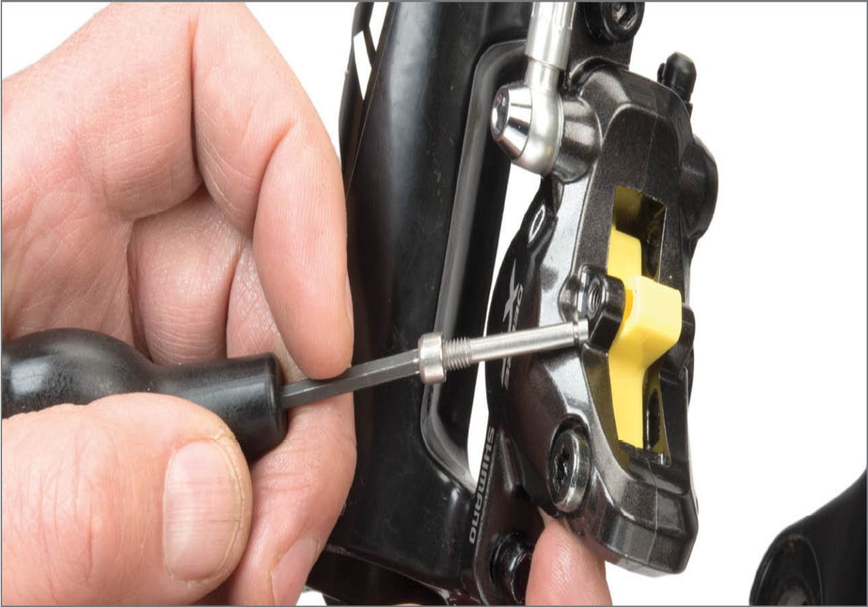
FIGURE 13.27: Install brake bleed blocks
