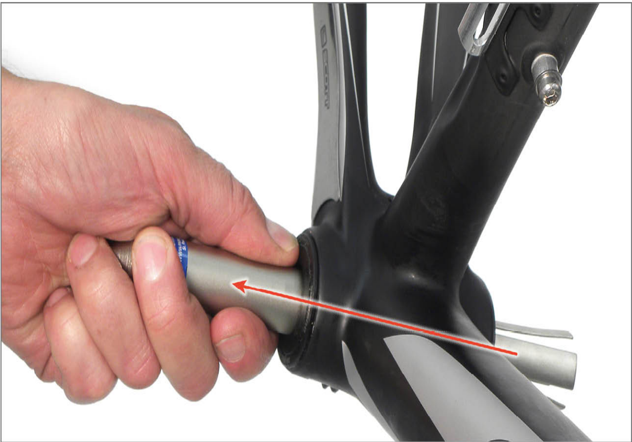
FIGURE 7.39: Pull BBT-90.3 through shell until it engages back of adaptor
