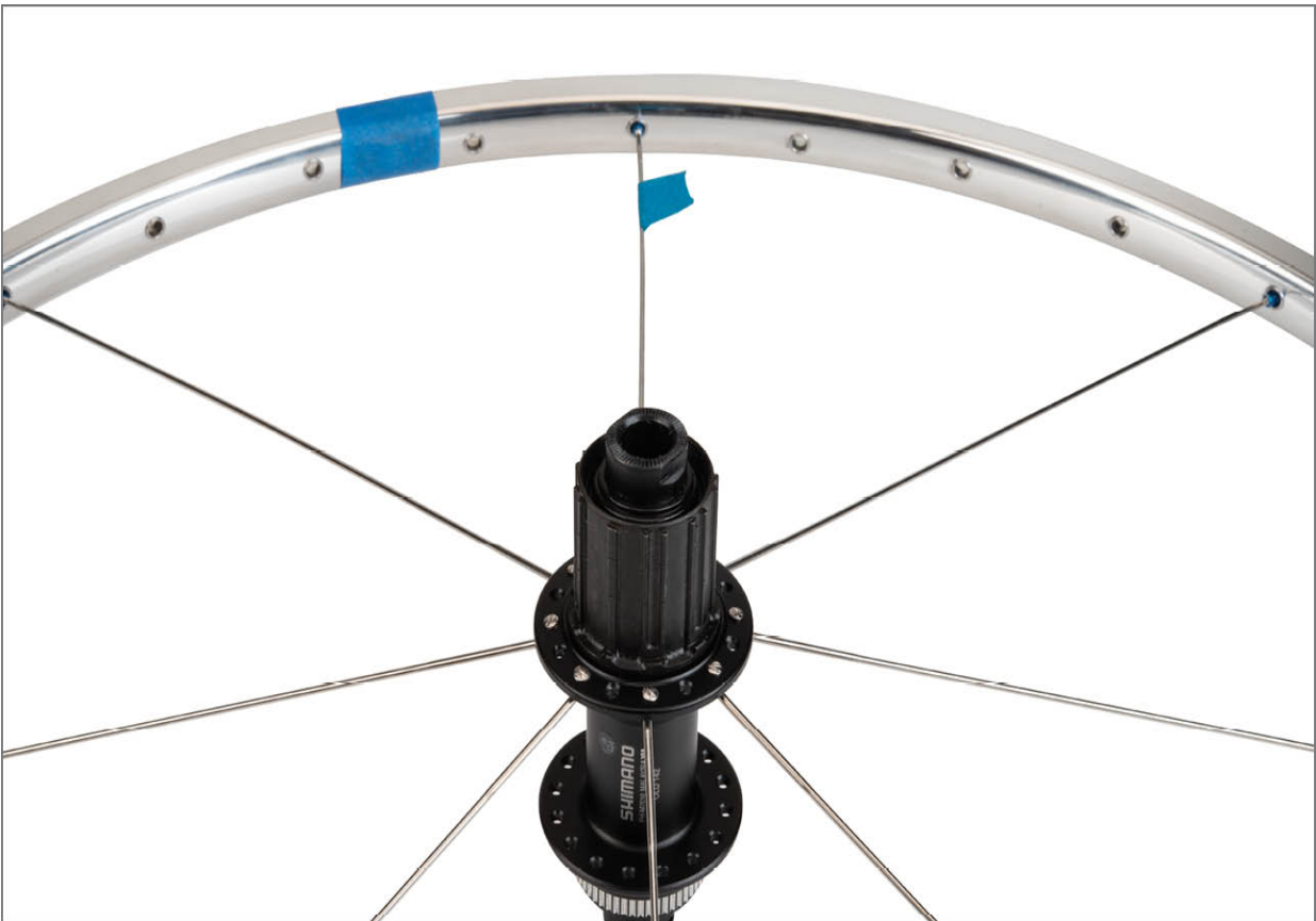
FIGURE 6.15: First set of spokes laced into rim
