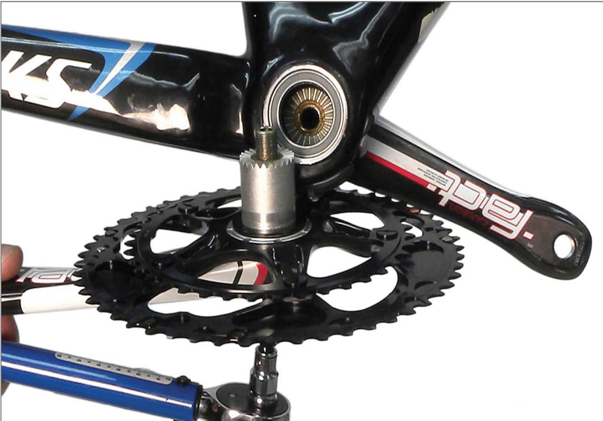
FIGURE 7.29: Specialized® crankset and BB30 bracket shell
