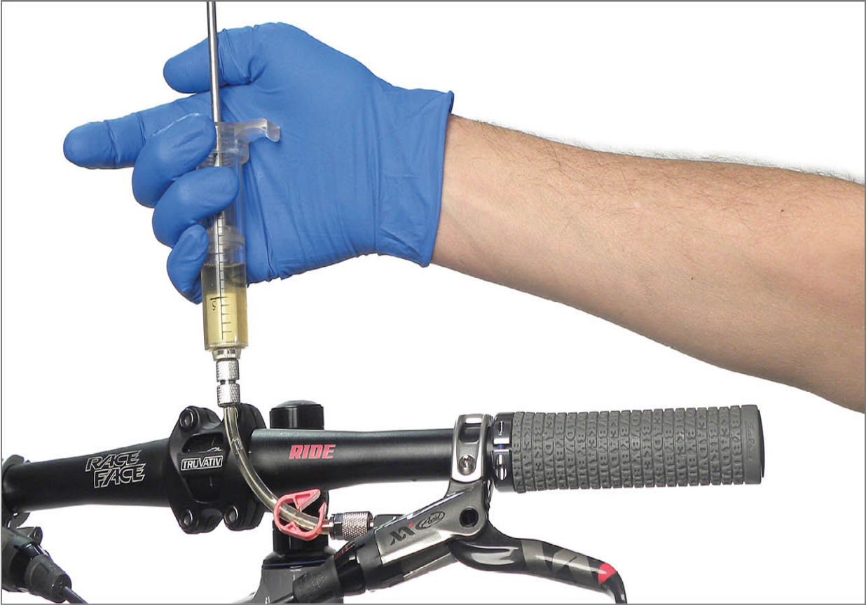
FIGURE 13.51: Fluid from lower syringe accepted by syringe at lever
