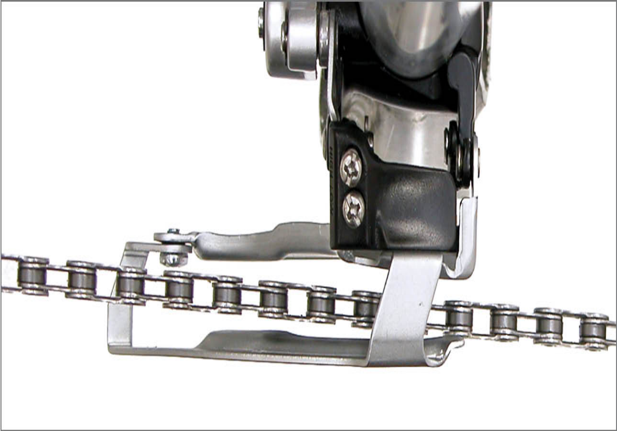
FIGURE 10.44: Cage rotated too far counterclockwise. Notice rear end of cage is outward compared to chain.
