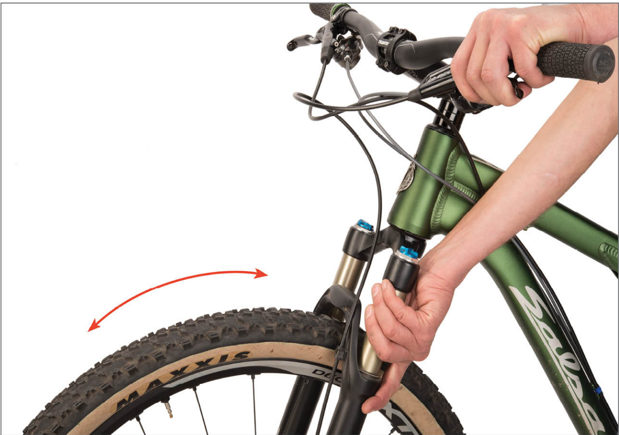
FIGURE 18.2: Feel for knock or movement between stanchions and sliders while holding front brake and pushing bike fore and aft
