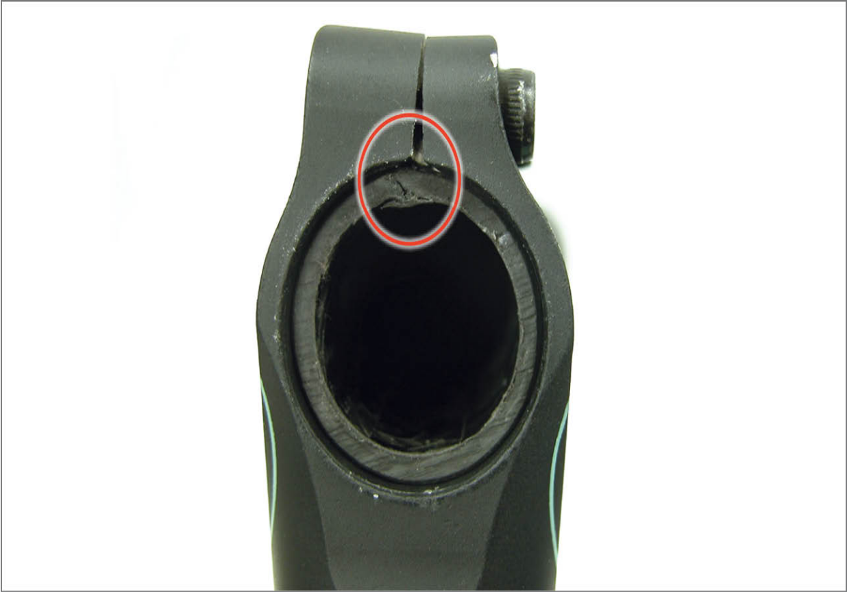
FIGURE 16.14: Recessed carbon fiber columns are susceptible to cracking from stem binder bolt pressure
