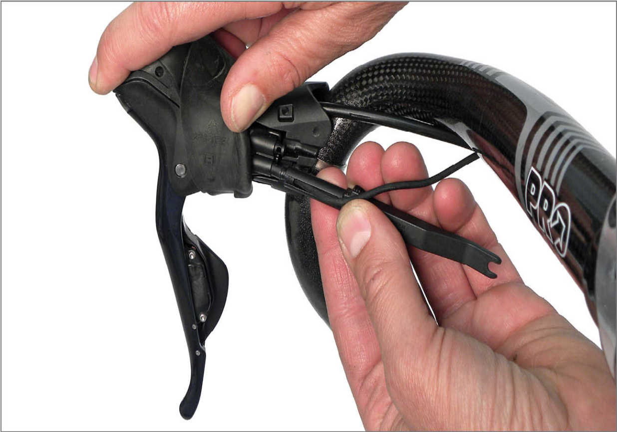
FIGURE 11.6: Use Shimano's special wire tool for plugging and unplugging wire in shift levers
