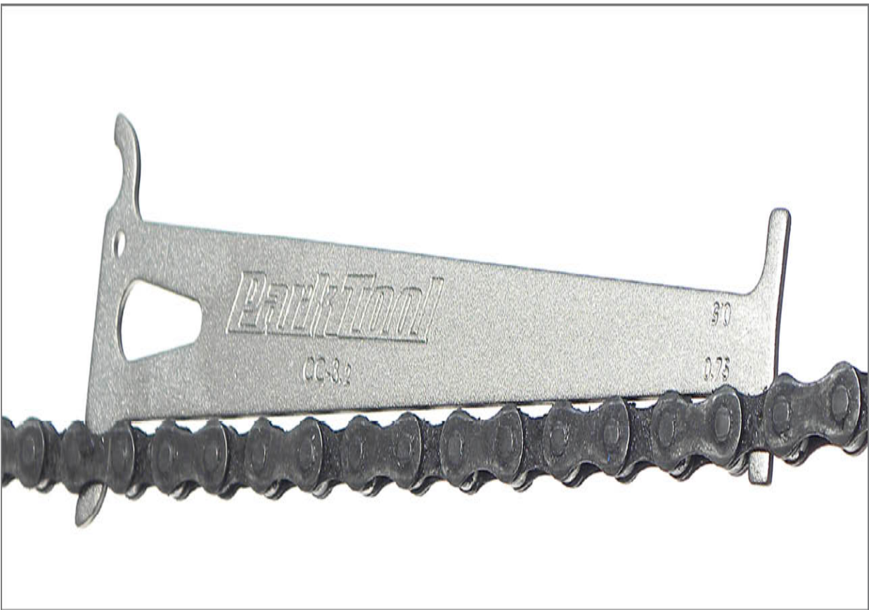
FIGURE 8.37: Park Tool CC-3.2 Chain Checker indicating a worn chain
