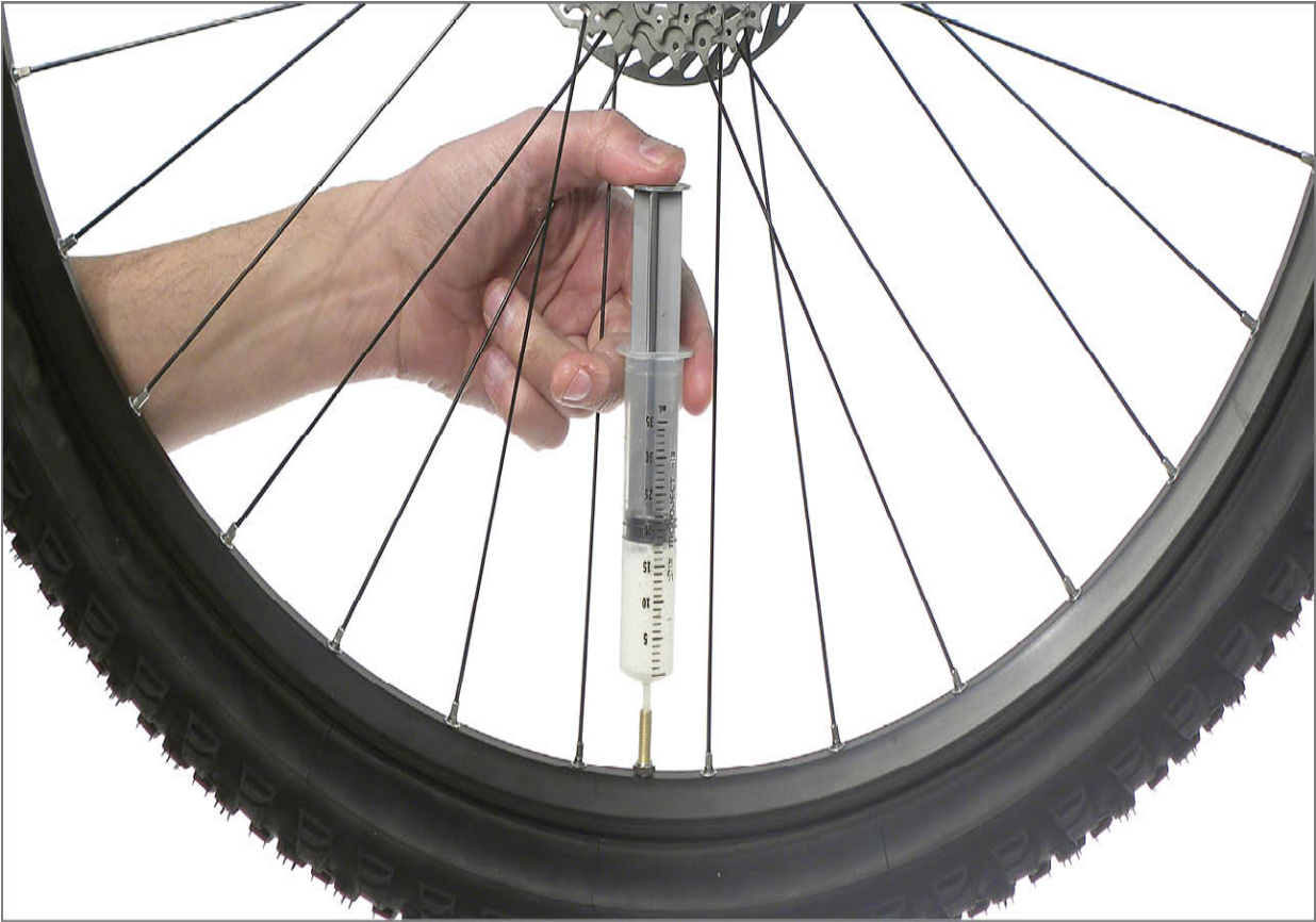
FIGURE 2.57: Inject sealant after tire bead is seated
