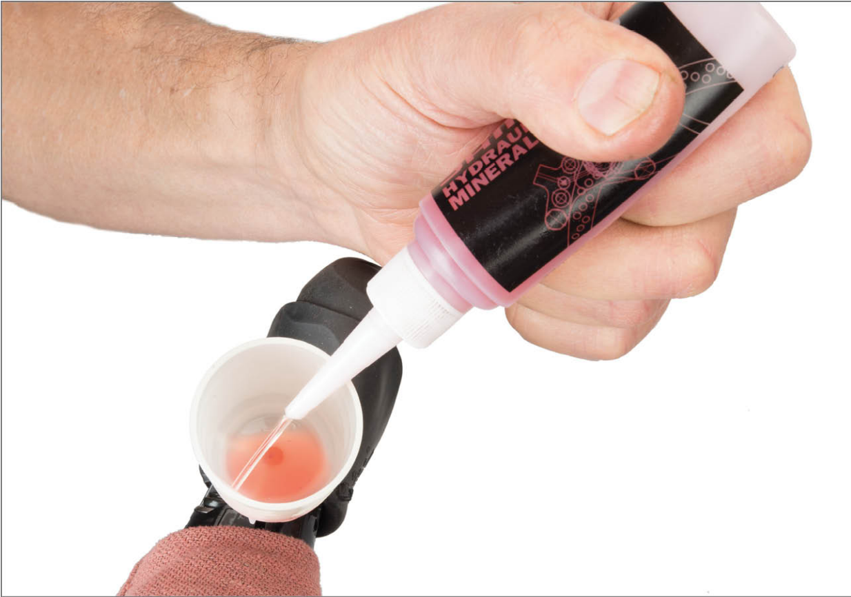
FIGURE 13.35: Inspect at lever and fill cup before it fully drains
