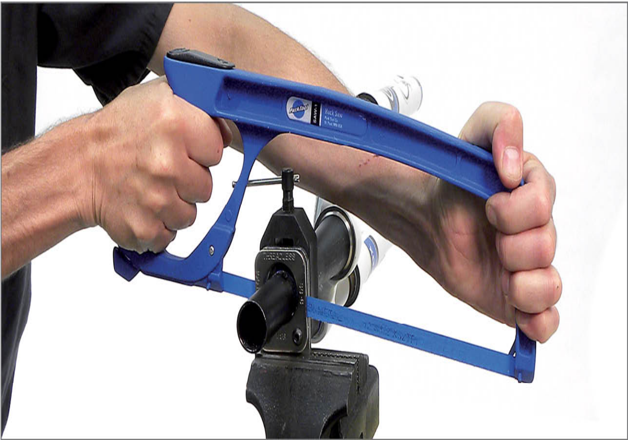
FIGURE 16.30: Cut with pressure in the forward cut and do not force blade into column
