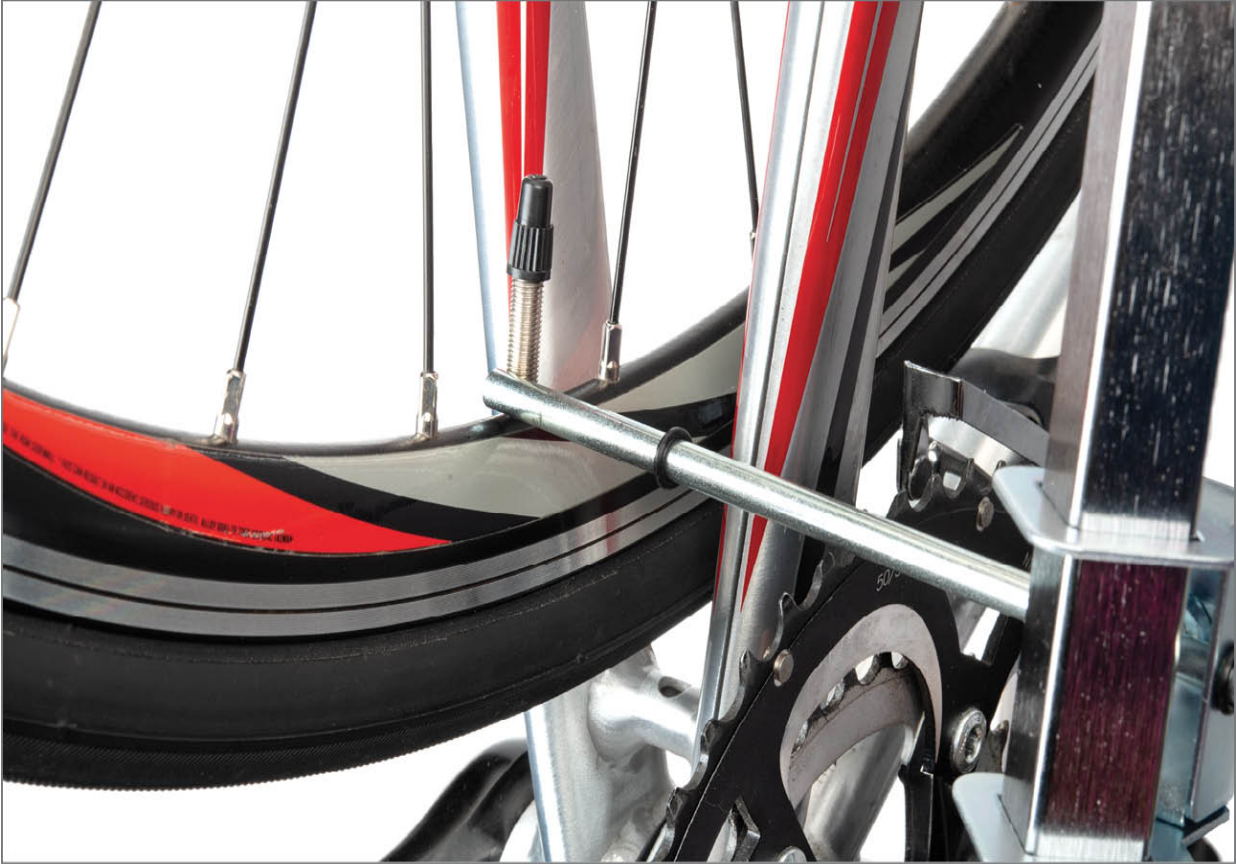
FIGURE 10.72: Reset gauge if it falls inside rim
