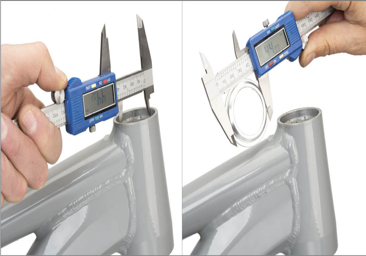
FIGURE 16.25: Measure and compare inside diameter of head tube to outside diameter of pressed cup
