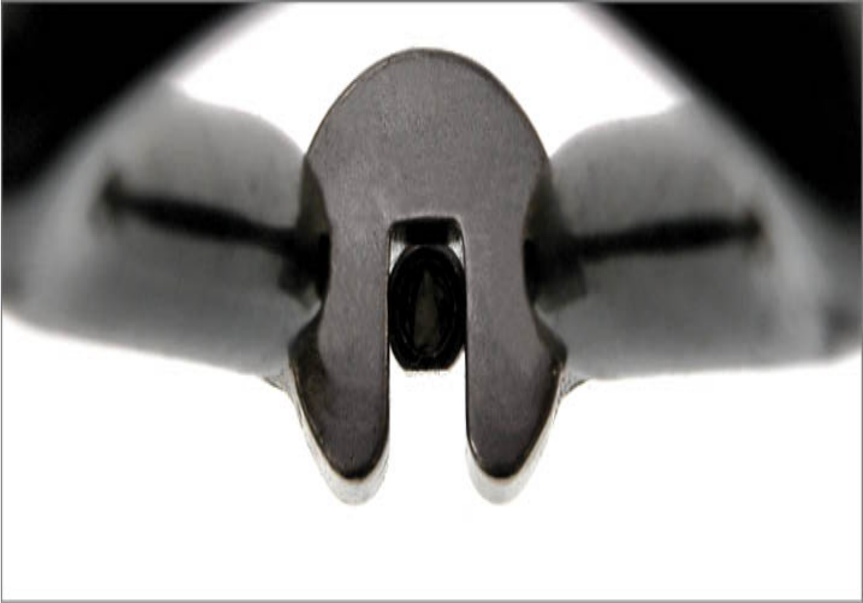
FIGURE 5.4: Properly sized wrench for nipple wrench flats
