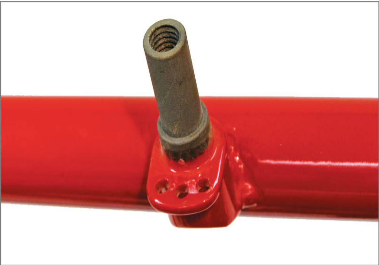
FIGURE 14.27: Brake caliper mounting stud with spring mounting holes for linear pull or cantilever-style brake arms
