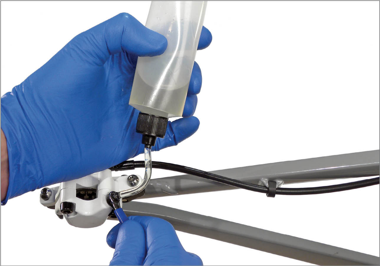
FIGURE 13.41: Alternately squeeze and release bottle to draw out bubbles from caliper
