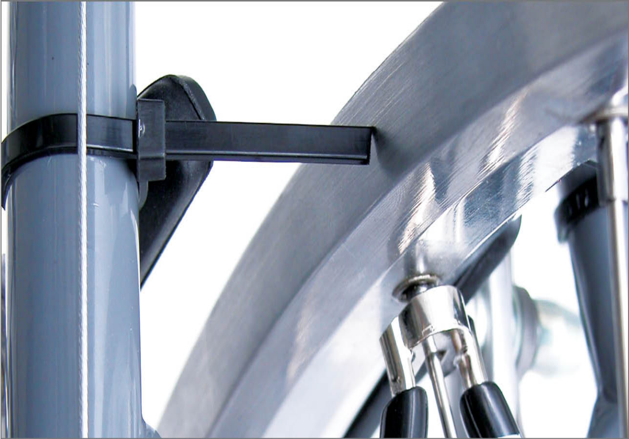
FIGURE 5.15: Isolate rim lateral deviation
