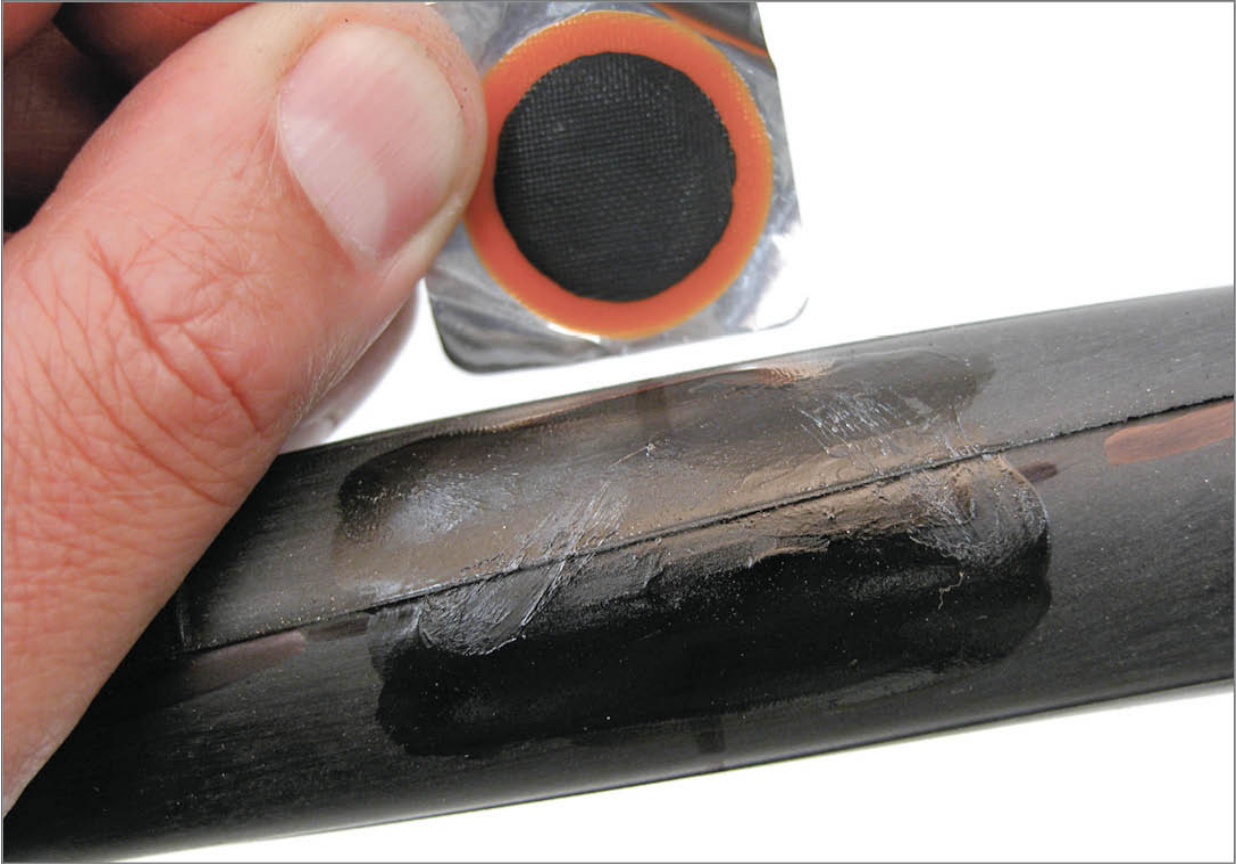
FIGURE 2.32: Spread a thin, wide layer of self-vulcanizing fluid
