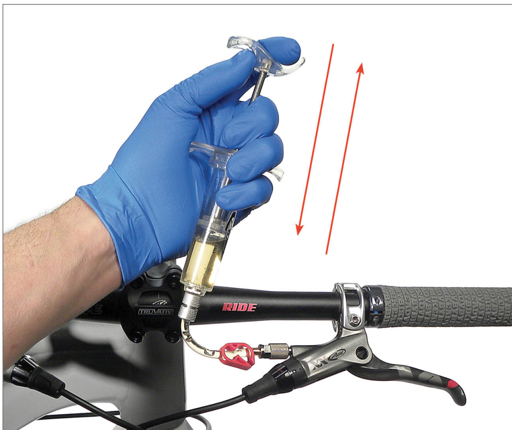
FIGURE 13.55: Push and pull repeatedly at lever to clear lever of air
