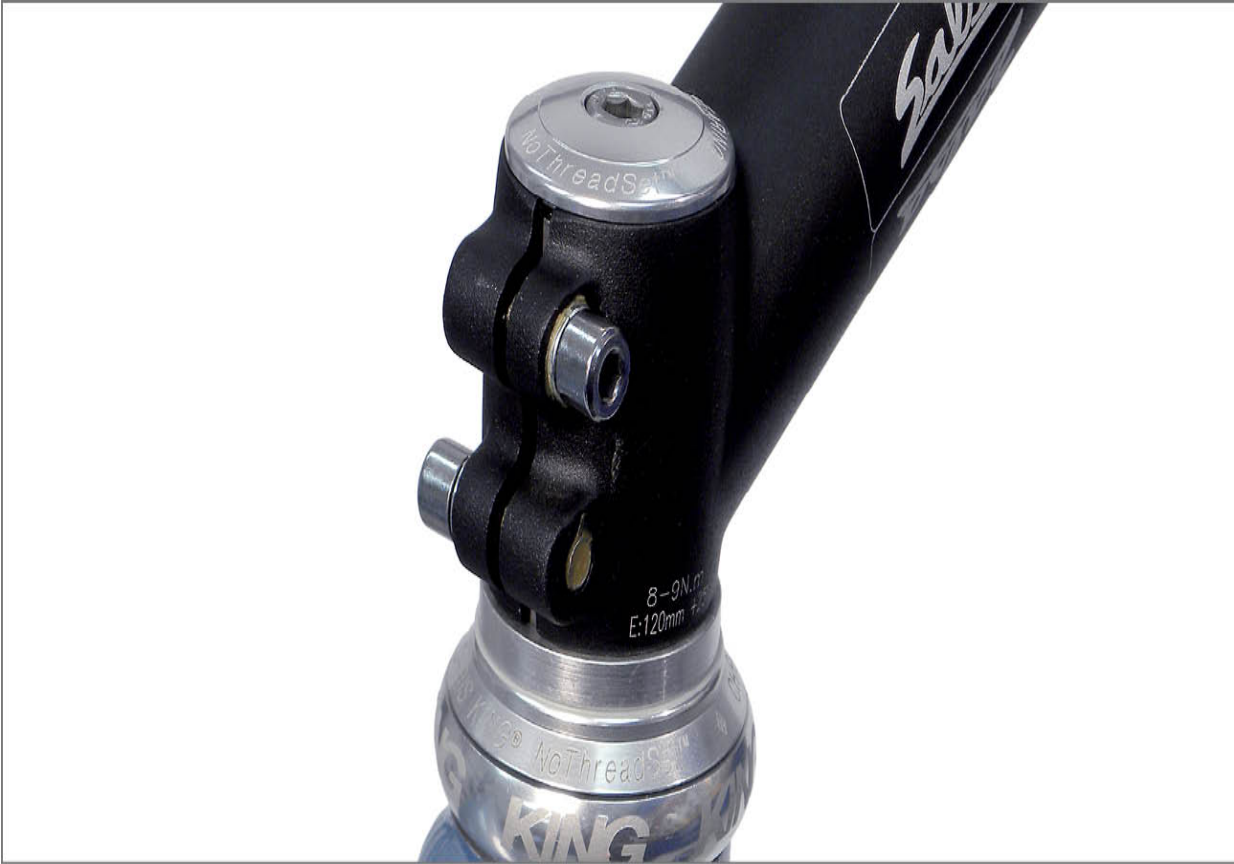
FIGURE 16.3: Threadless headset with external pressed cups (EC) with threadless stem and top cap
