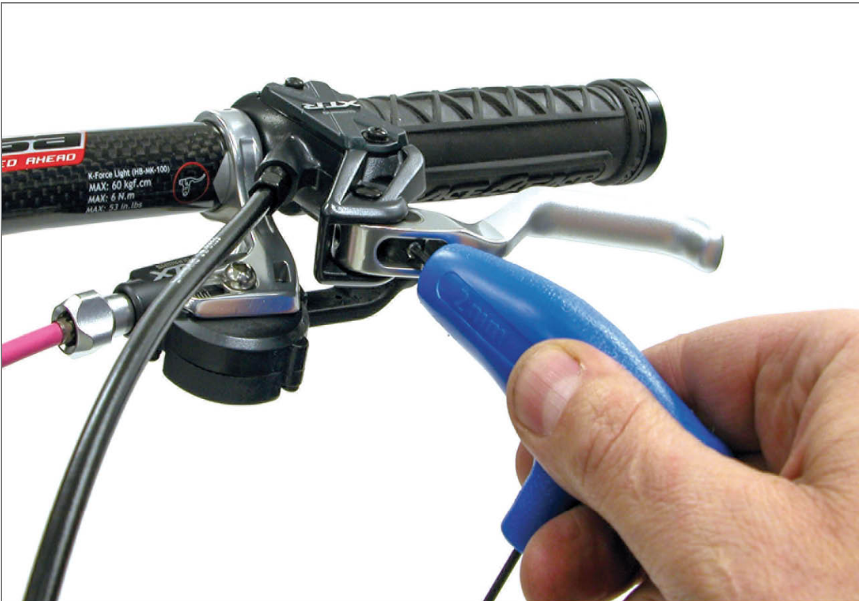
FIGURE 13.20: Brake lever reach adjustment screw on a Shimano® lever
