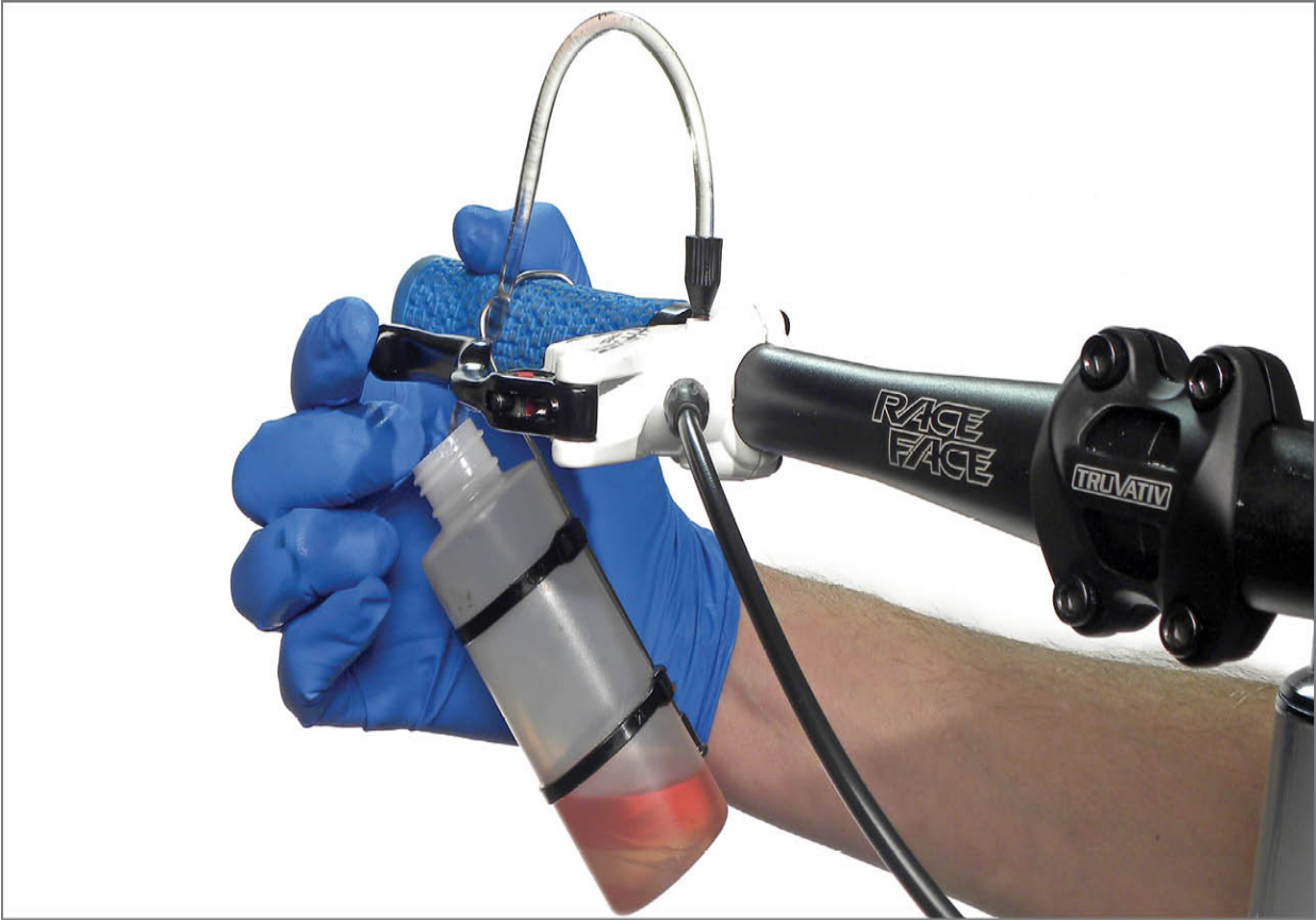
FIGURE 13.42: Pull slightly on lever and allow it to snap forward to release bubbles
