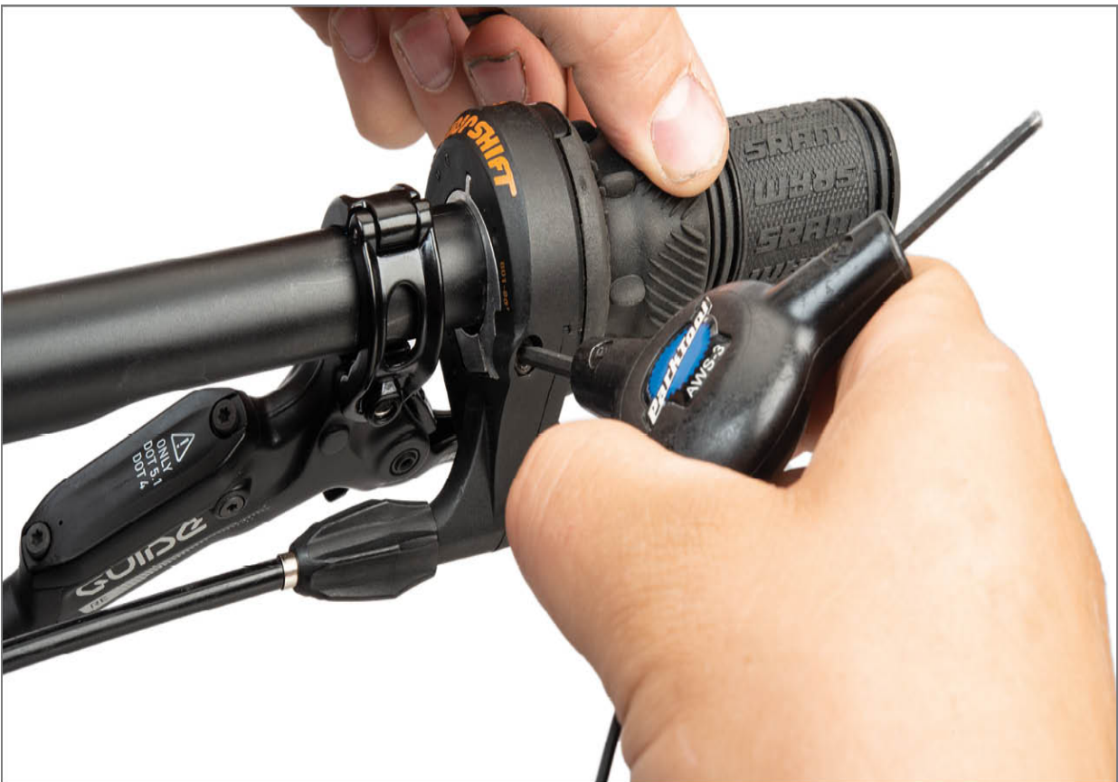
FIGURE 10.17: Location of setscrew in SRAM® twist grip shifter
