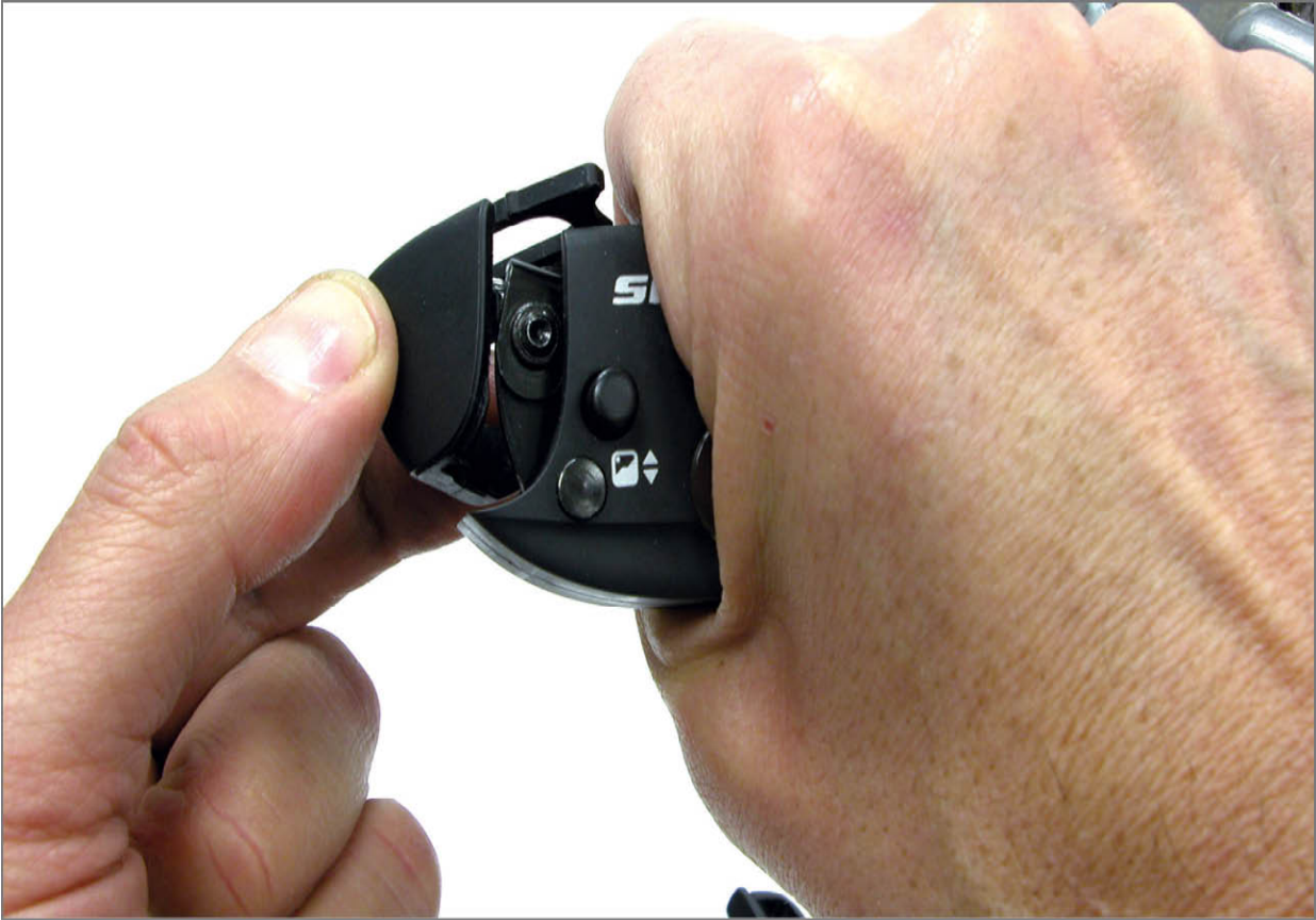
FIGURE 12.4: Hold Clickbox and pry corner down and away
