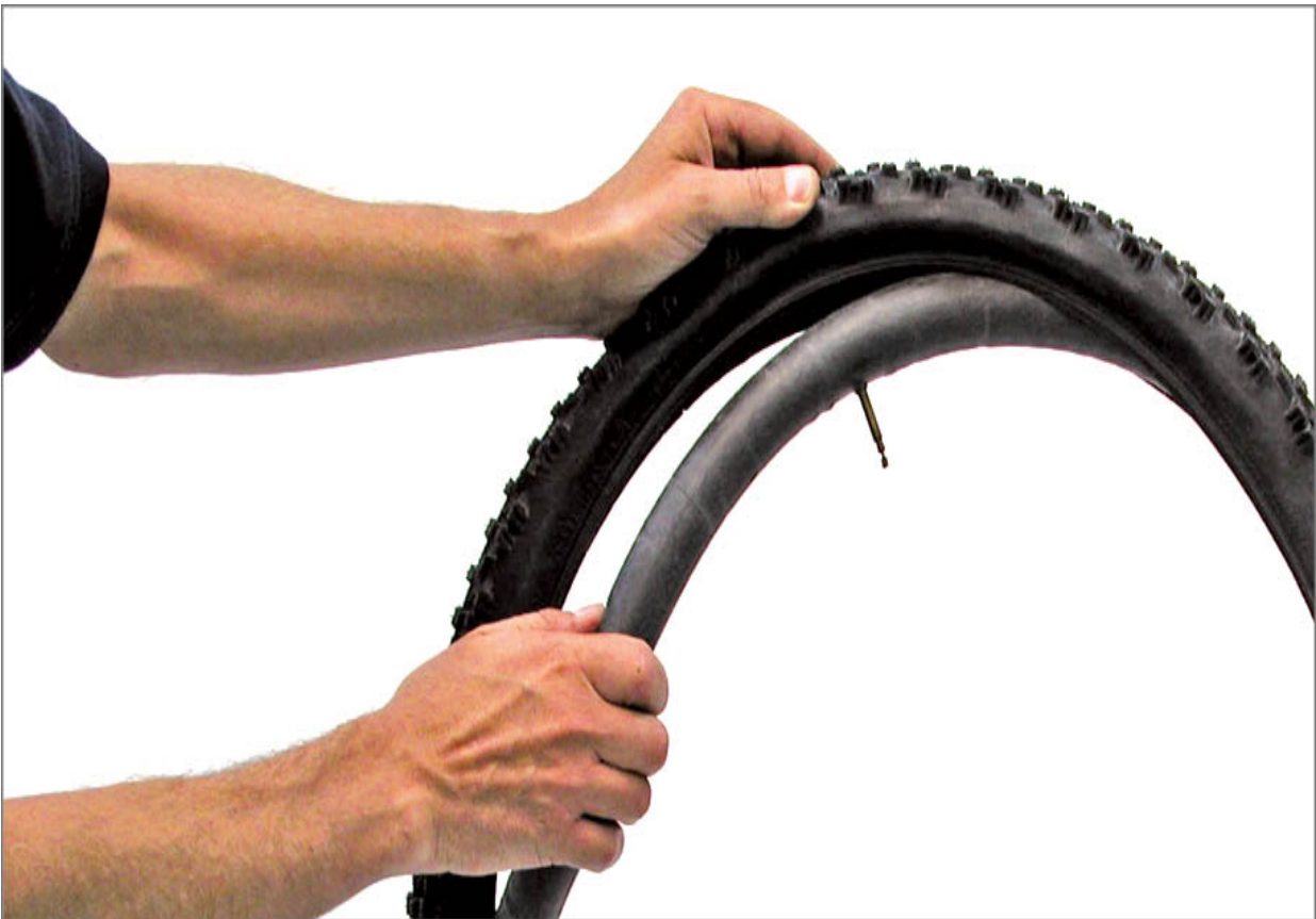
FIGURE 2.47: Place tube into tire before mounting tire to rim
