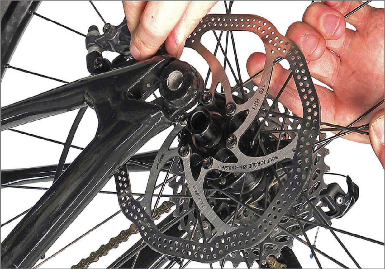
FIGURE 4.4: Closed dropout and a 12mm rear thru axle hub
