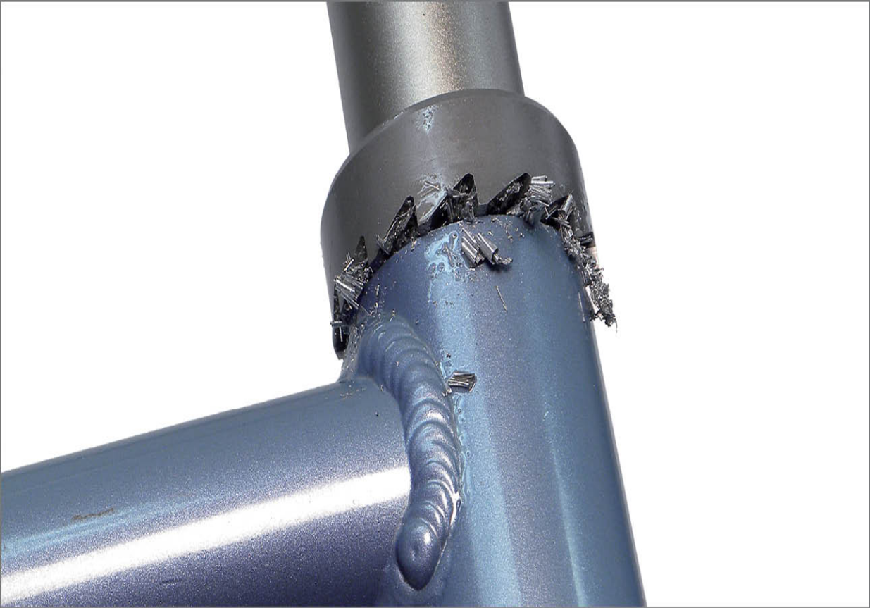
FIGURE 16.1: Facing head tube surface to improve bearing adjustment
