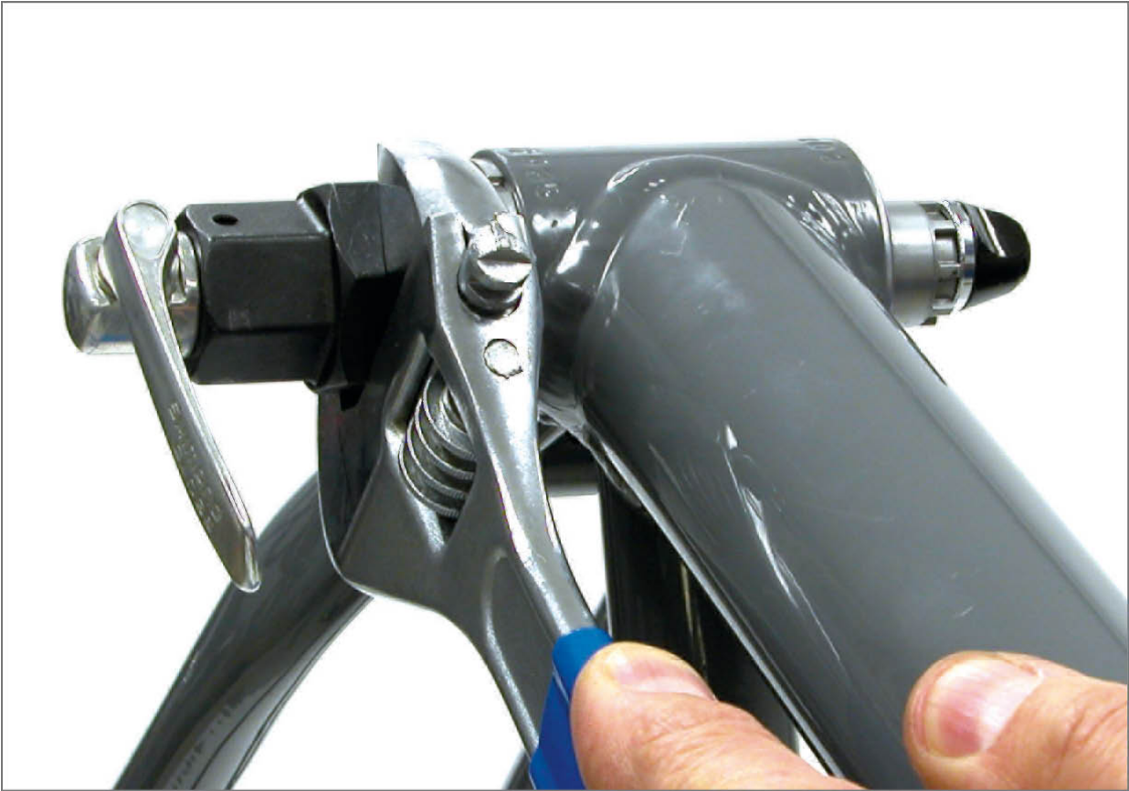
FIGURE 7.57: Use hub skewer to secure tool snug to fittings of cartridge main body and adaptor
