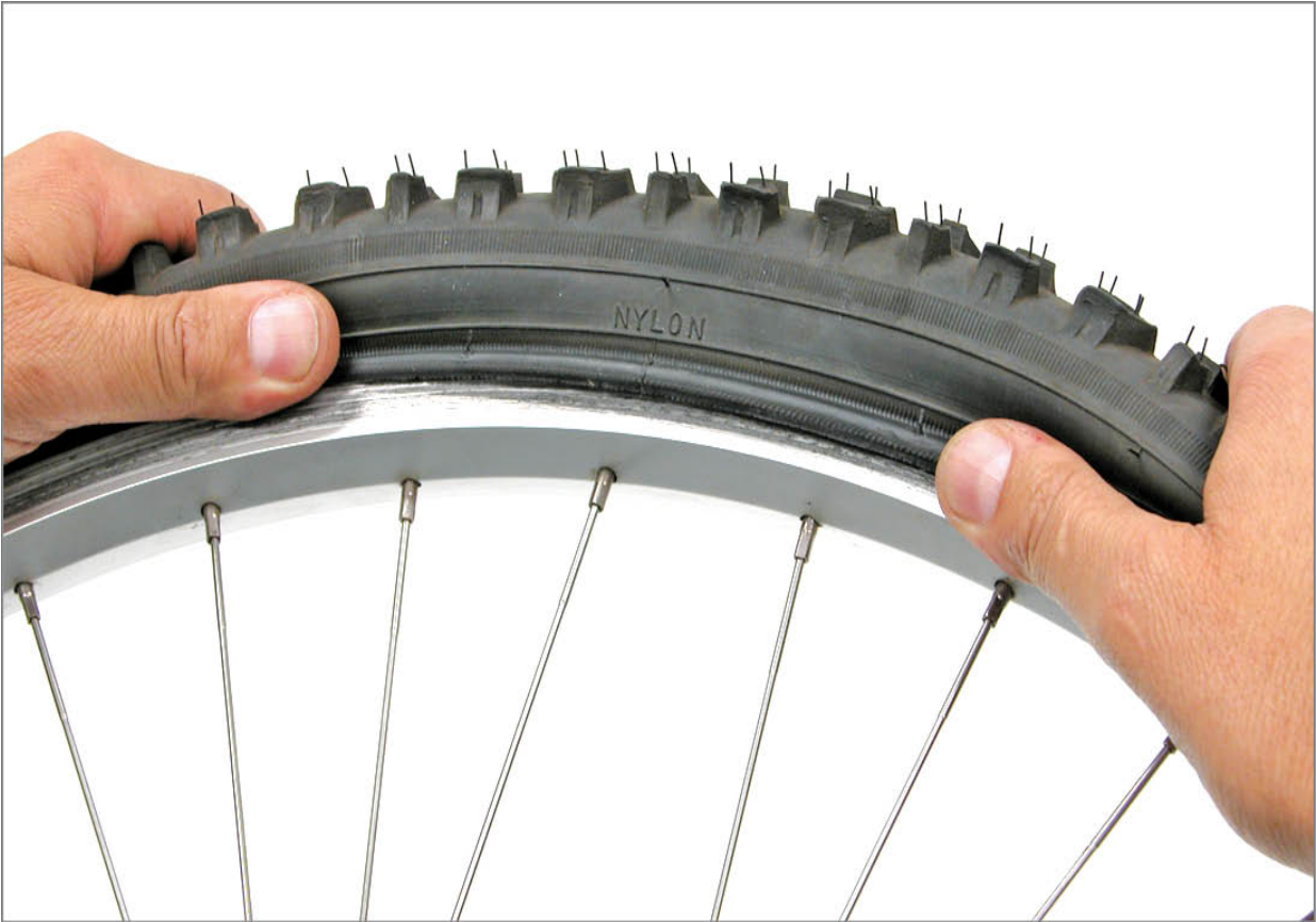
FIGURE 2.49: Push tire bead up and over rim sidewalls
