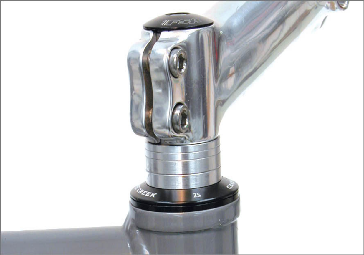
FIGURE 16.5: ZS or “zero stack” headset design
