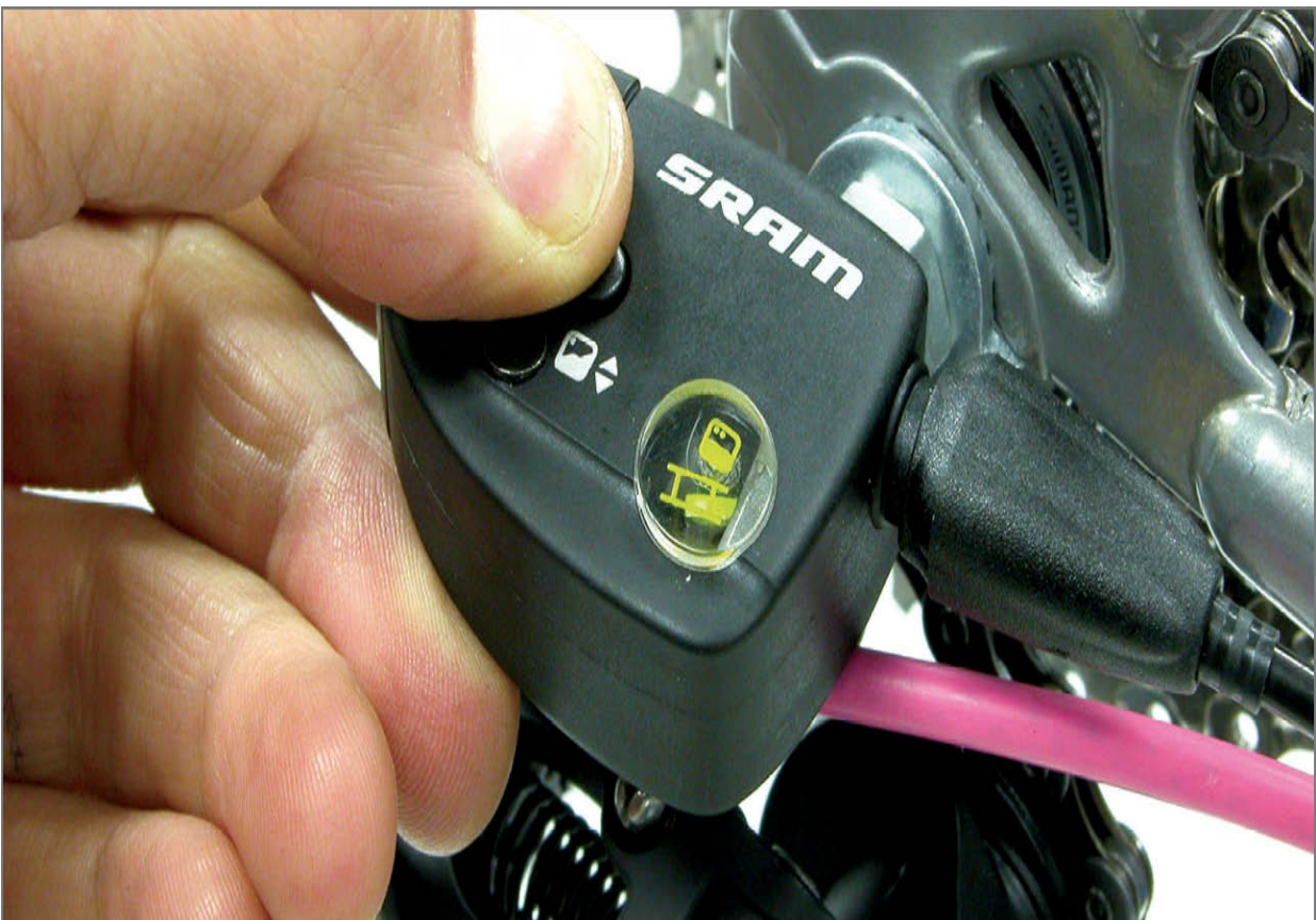
FIGURE 12.2: Remove Clickbox to access axle nuts
