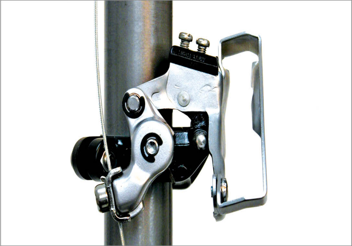
FIGURE 10.37: Top swing cage with top pull cable
