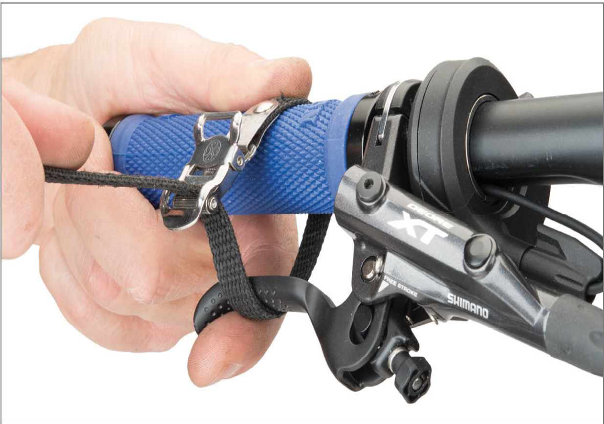
FIGURE 13.23: Hold lever to maintain pad pressure
