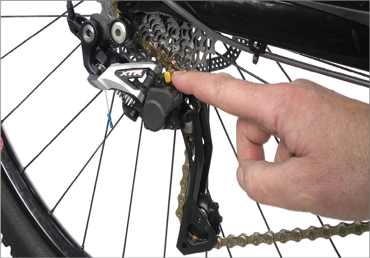
FIGURE 2.8: Push on-off lever upward to return derailleur to clutch operation mode
