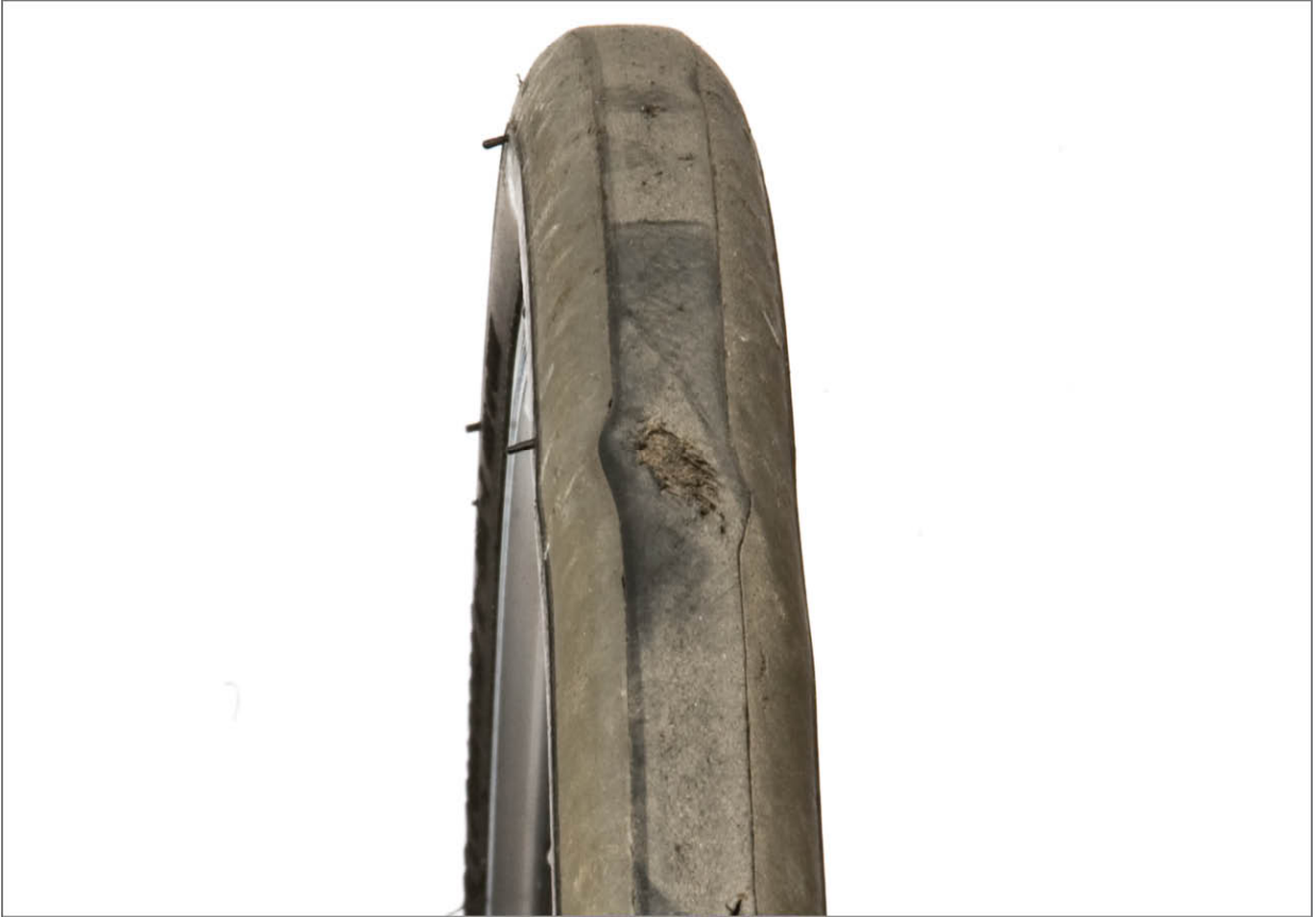
FIGURE 2.29: Damaged tread and casing
