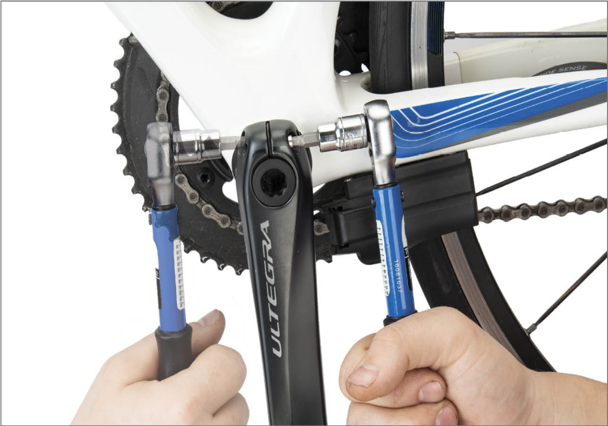
FIGURE 7.16: Alternate tightening sides until both sides are pulled fully tight
