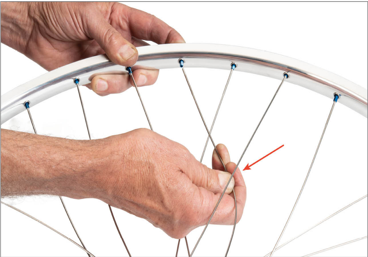
FIGURE 6.23: Spoke is flexed under crossing on way to rim
