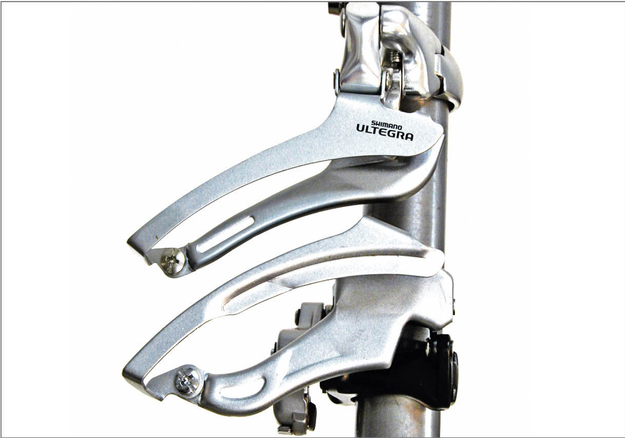
FIGURE 10.33: Top: shallow cage design Bottom: deep cage design
