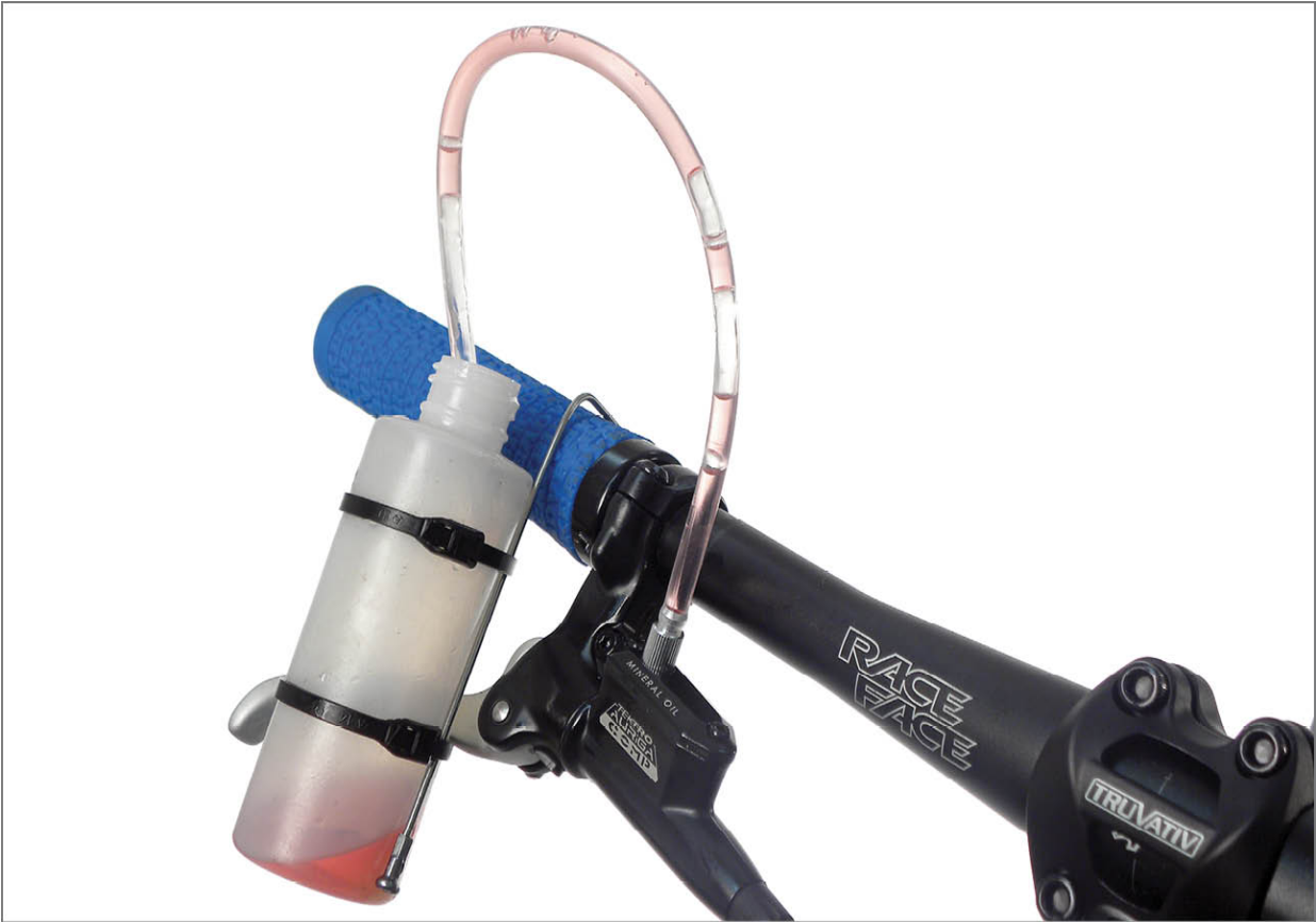
FIGURE 13.62: Push fluid upward into bottle after opening up bleed nipple
