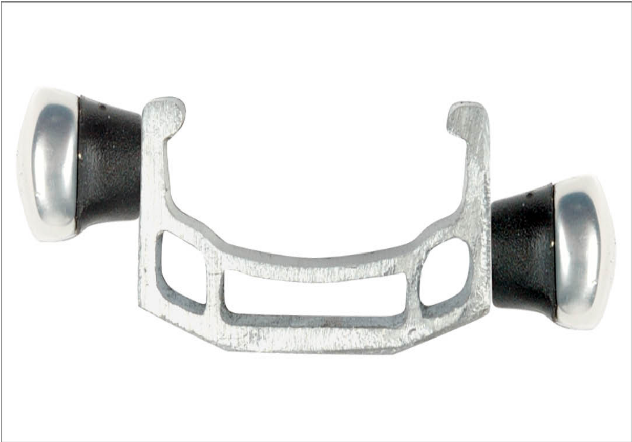
FIGURE 14.23: Pad of left set to top of rim braking surface, while pad on right set to bottom of rim braking surface
