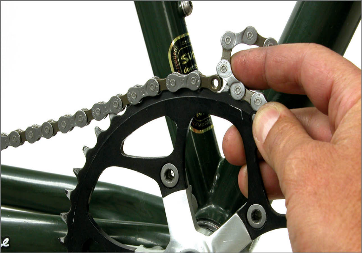
FIGURE 8.29: Use front ring to help hold chain end for sizing
