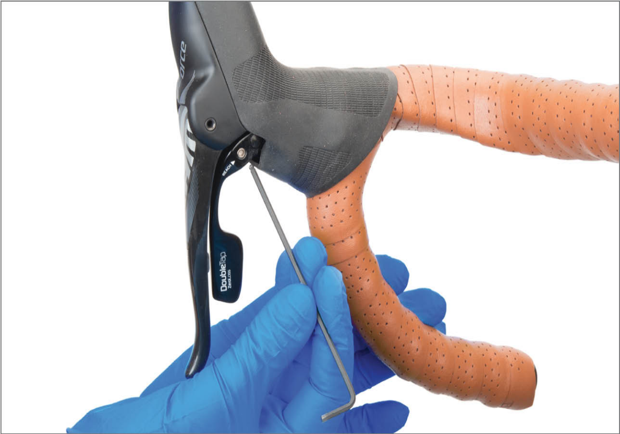
FIGURE 13.44: Turn road lever reach adjustment knob counterclockwise
