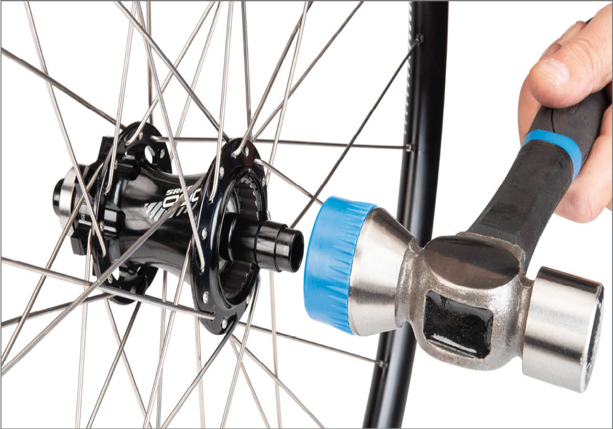
FIGURE 4.25: Drive axle from drive side with a mallet
