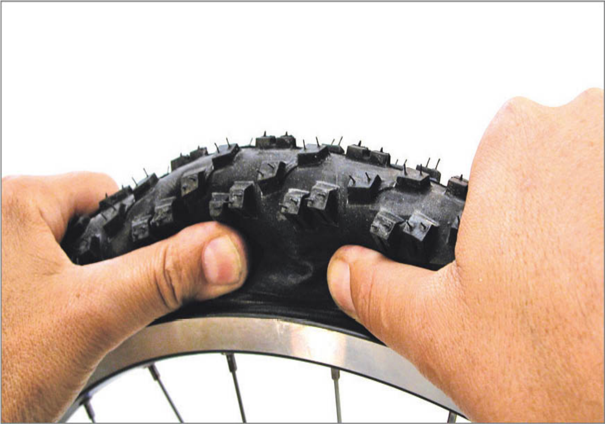
FIGURE 2.17: Push tire bead from sidewall the entire perimeter of wheel
