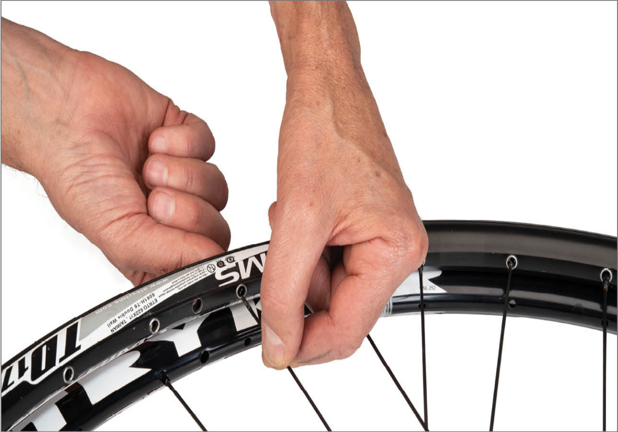
FIGURE 6.25: Transferring spokes after taping rims together
