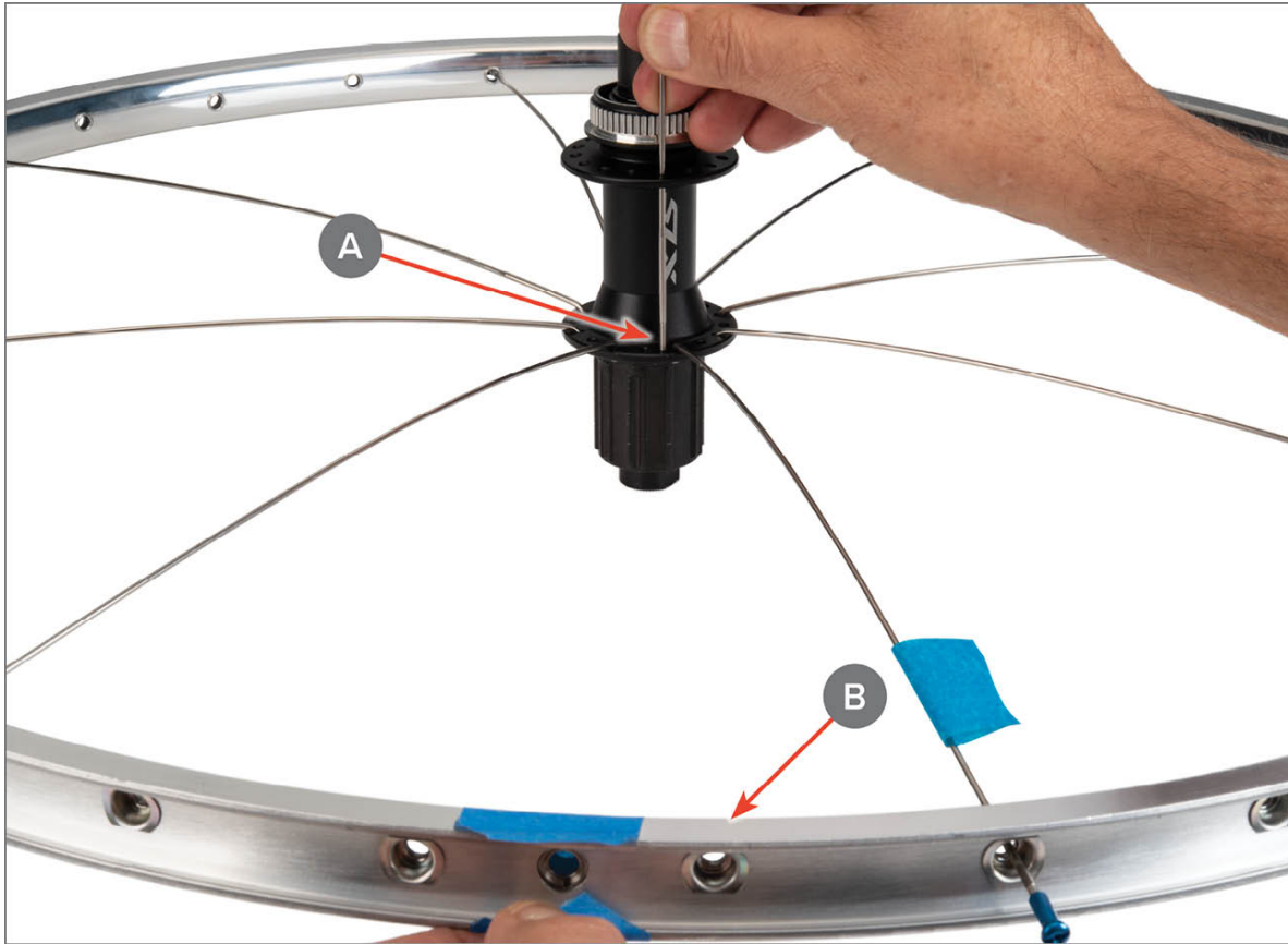
FIGURE 6.18: Select hole in left flange relative to Valve Reference Spoke
