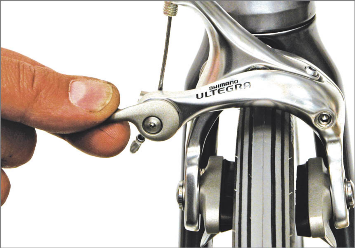
FIGURE 2.2: Side-pull or dual-pivot rim caliper may have quick-release at caliper arm
