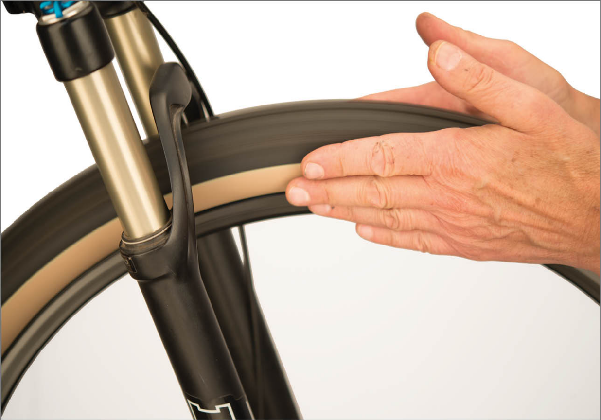
FIGURE 2.28: Bulges or deformities in casing indicate thread failures
