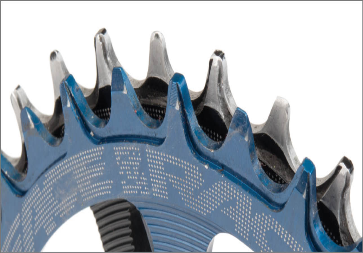
FIGURE 7.69: New teeth on blue ring compared to worn teeth on black ring
