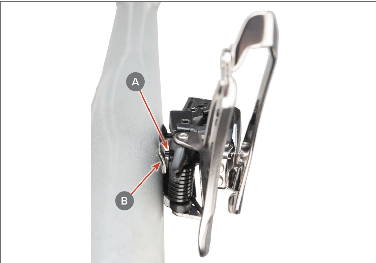
FIGURE 10.51: Support bolt (A) pushing against backing plate (B) to brace the front derailleur
