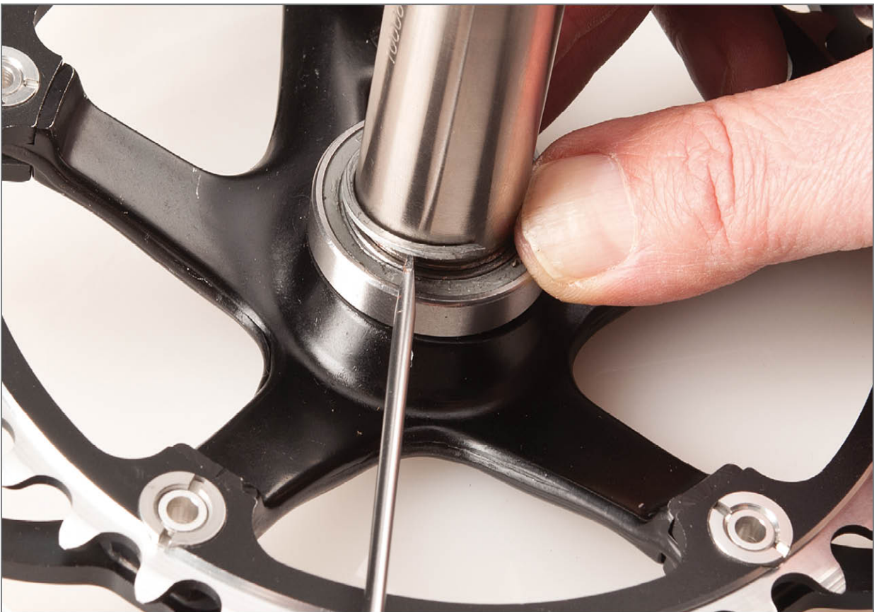
FIGURE 7.51: Remove right-side C-clip from spindle before pulling bearing
