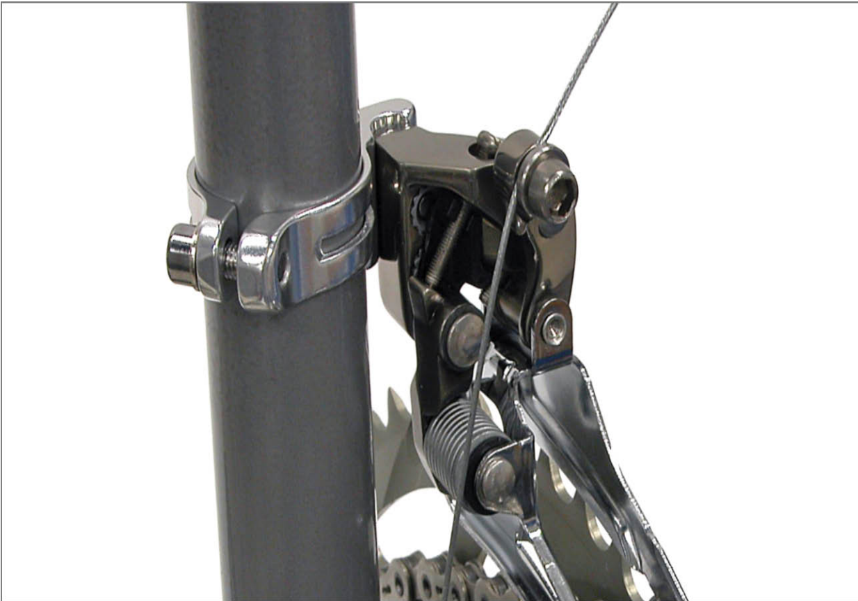
FIGURE 10.31: Clamp-on adaptor for a “braze-on” type front derailleur
