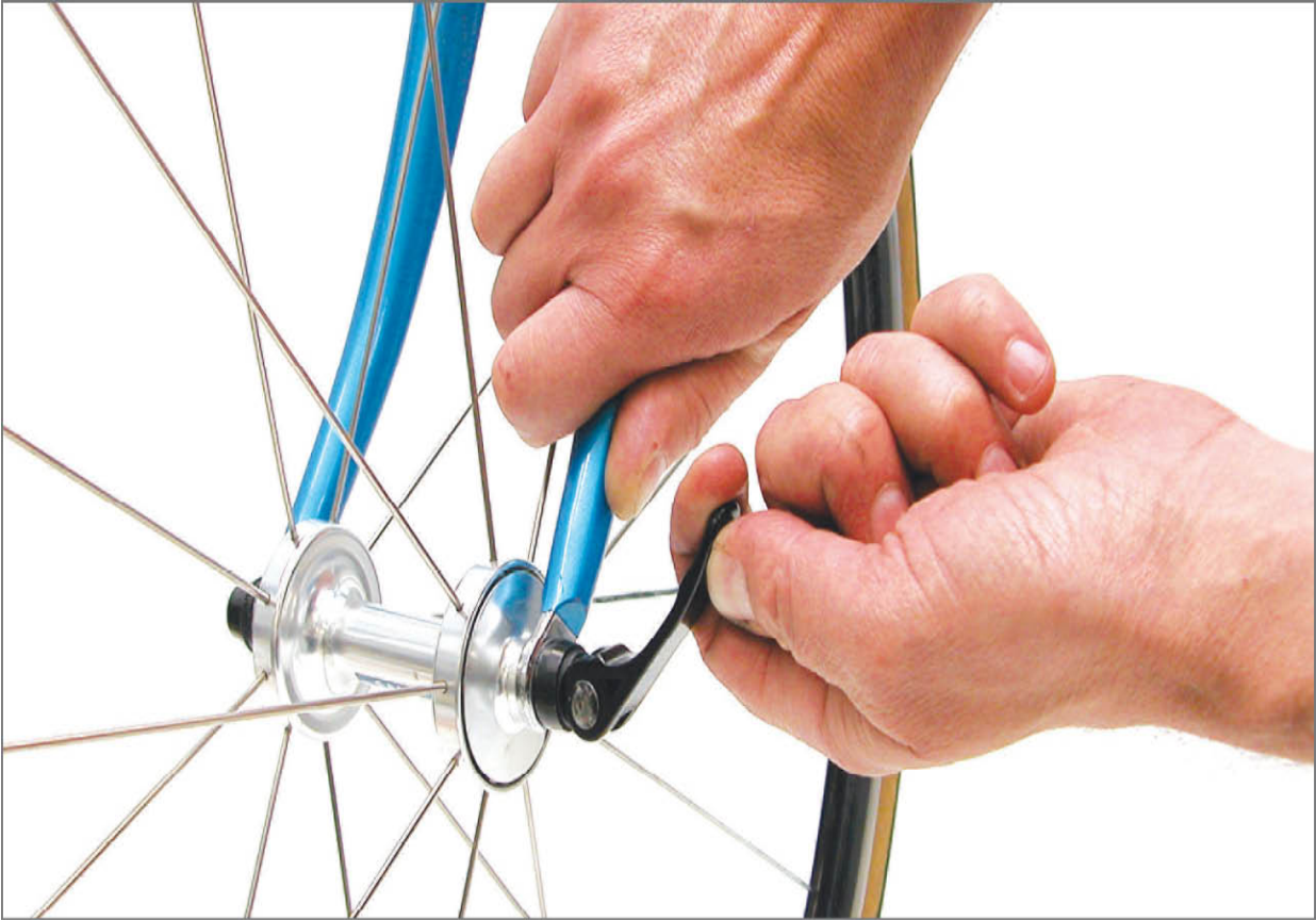
FIGURE 2.6: Puller lever from closed to open position
