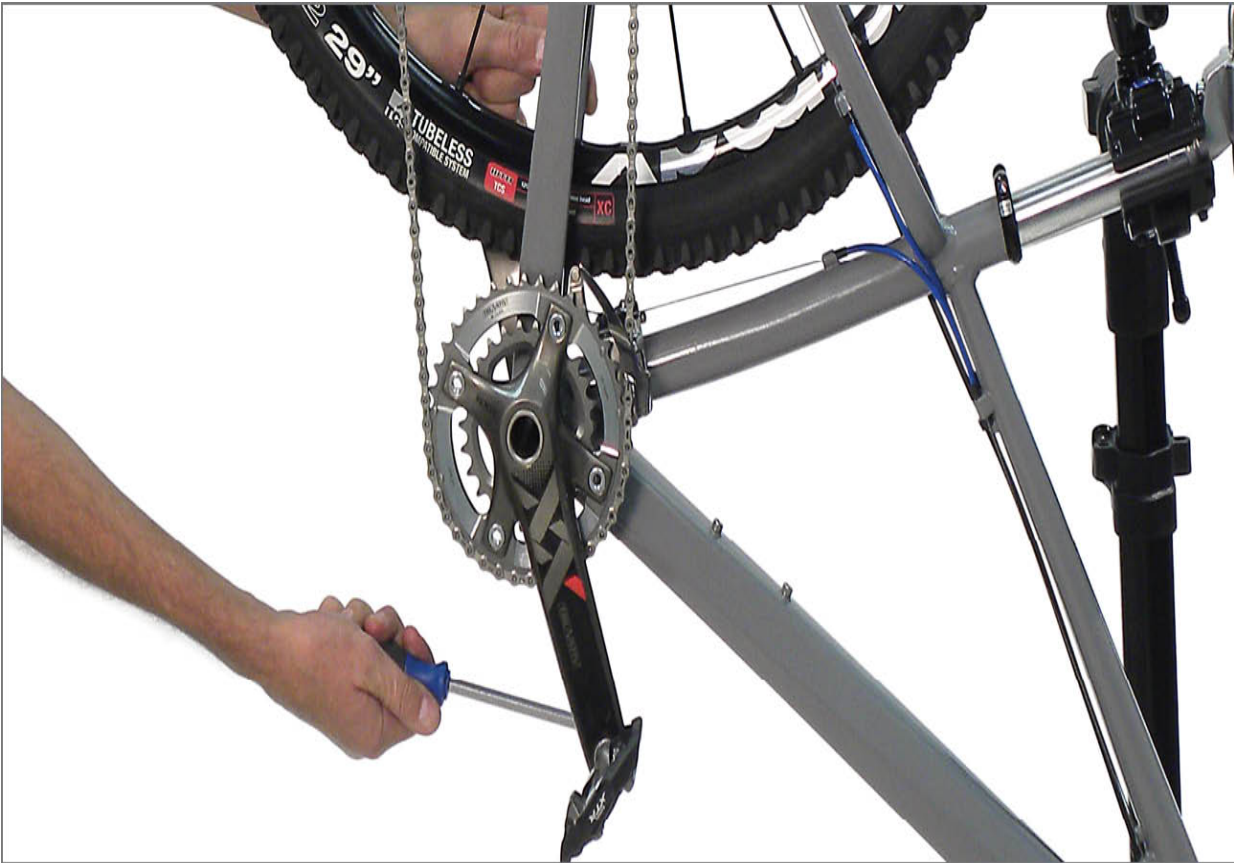
FIGURE 9.1: Pedal wrench fitting behind crank at end of pedal axle
