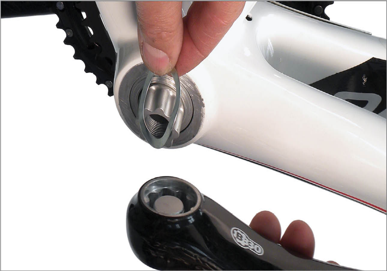
FIGURE 7.17: Wave washer between crank and bearing
