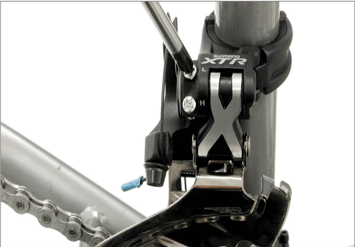
FIGURE 10.47: Location of limit screws
