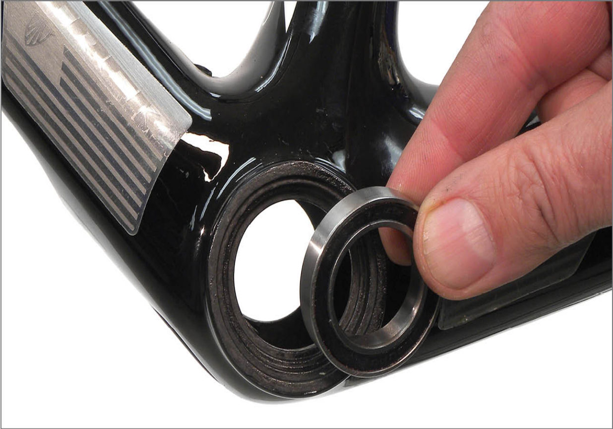
FIGURE 7.33: BB90 frame shell in a Trek® bottom bracket shell, shown with cartridge bearing
