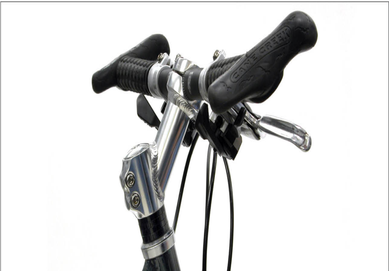
FIGURE 15.3: Secure bar ends so they do not move under load
