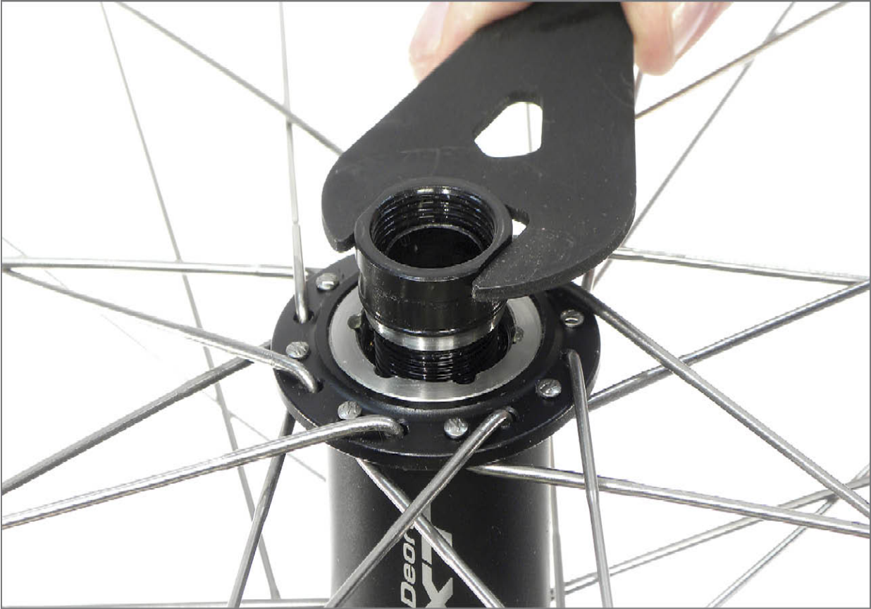
FIGURE 4.10: Adjustable cup-and-cone thru axle front hub
