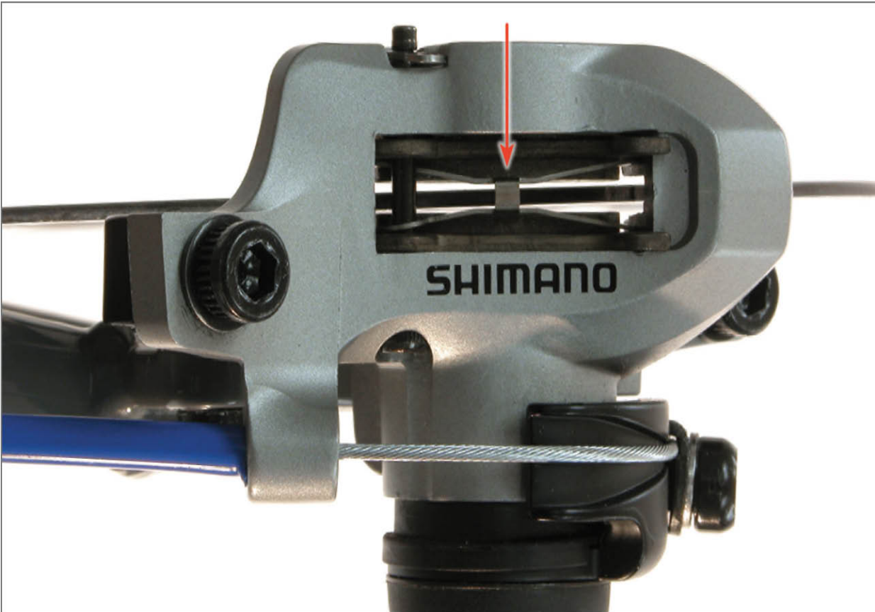
FIGURE 13.8: Return spring positioned between pads
