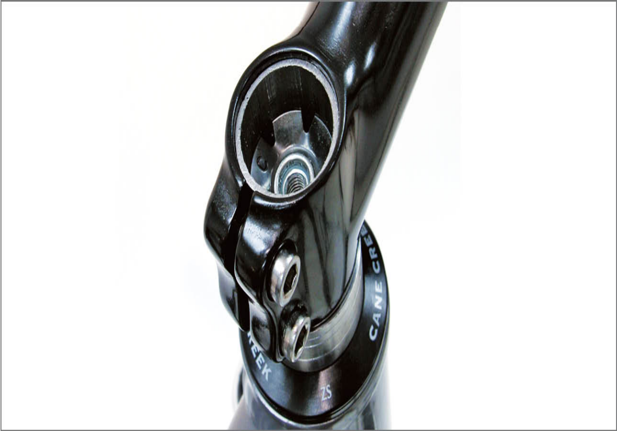
FIGURE 15.17: Thread column recessed below stem top
