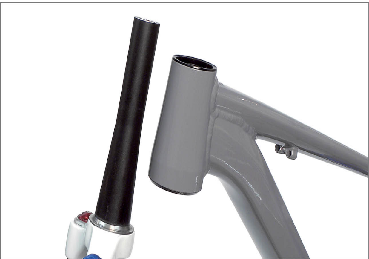
FIGURE 16.7: Mixed headset standards. Lower head tube is ZS56/40, and upper headset is ZS44/28.6
