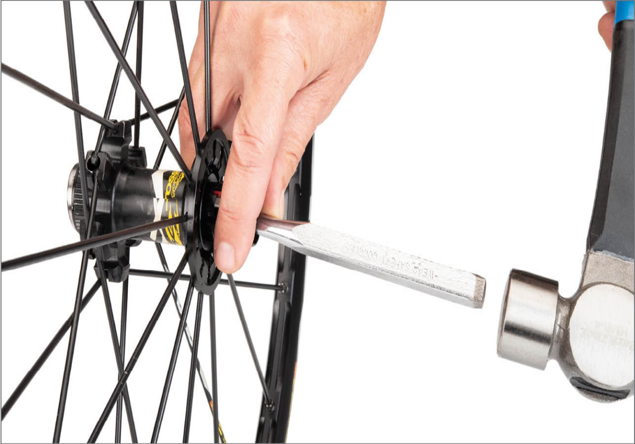
FIGURE 4.27: Use punch and hammer to walk bearing out of hub shell by alternating impacts
