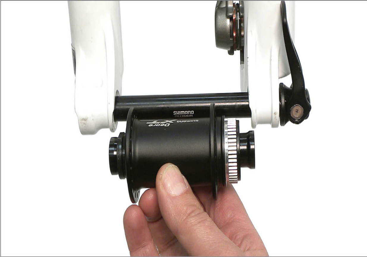
FIGURE 4.3: 15mm axle thru axle hub in 100mm hub width
