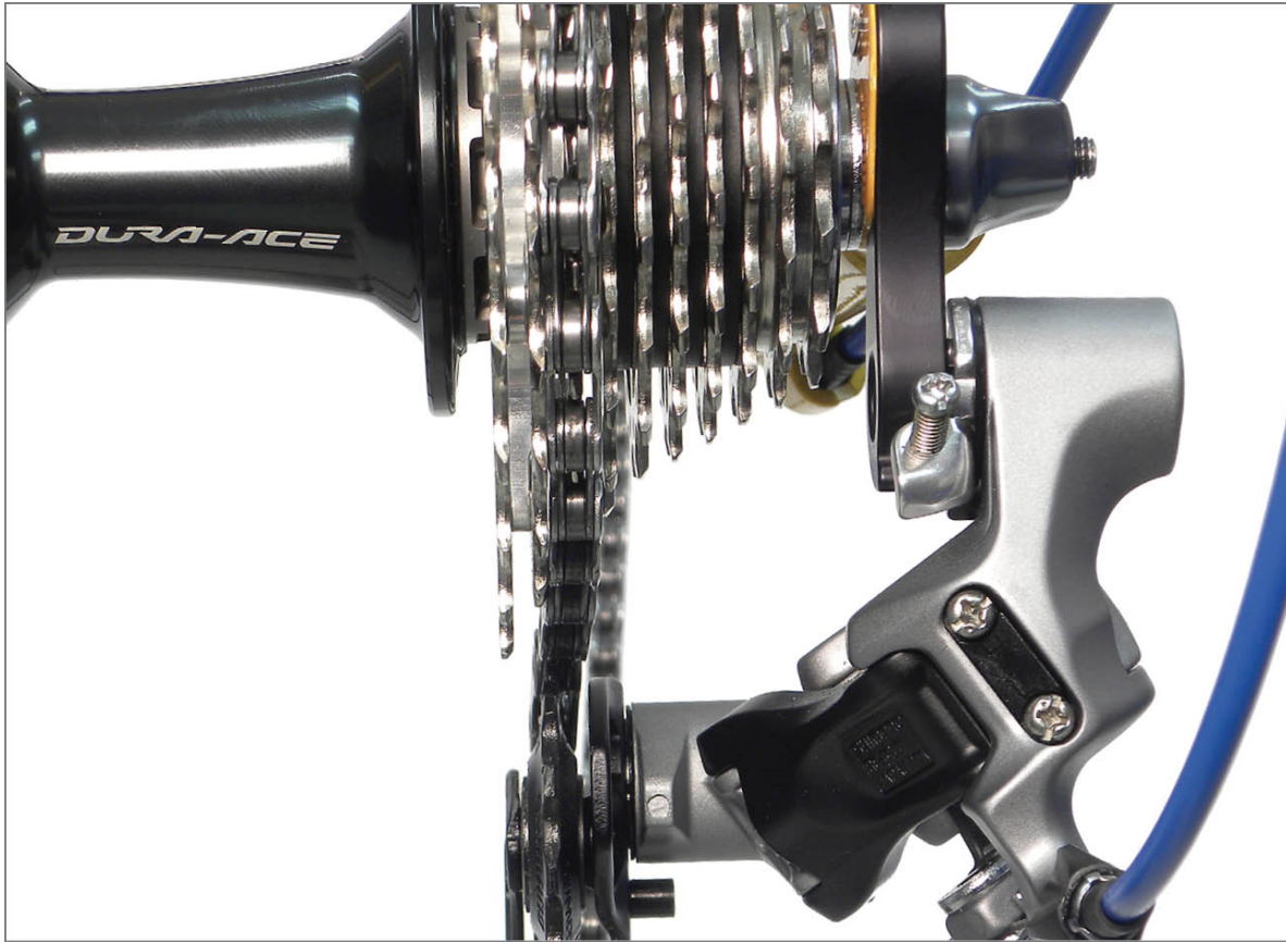
FIGURE 10.61: Chain positioned too far inward resulting in a rattle against sprocket
