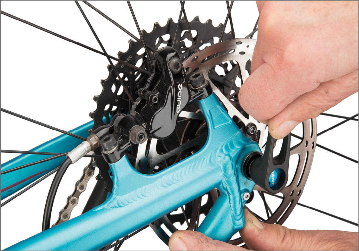
FIGURE 2.14: Tighten lever and then position lever as desired
