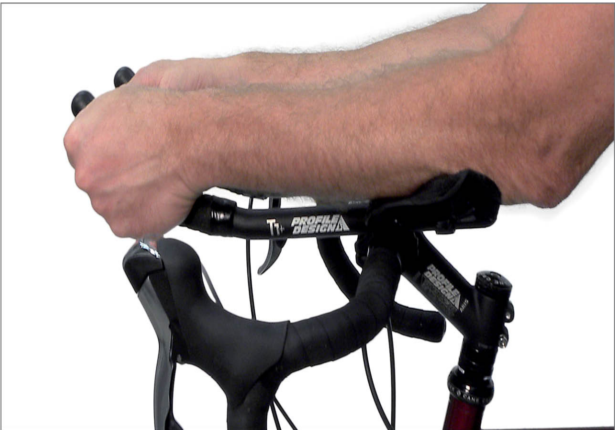
FIGURE 15.8: “Clip-on” aero bars mounted to drop handlebars
