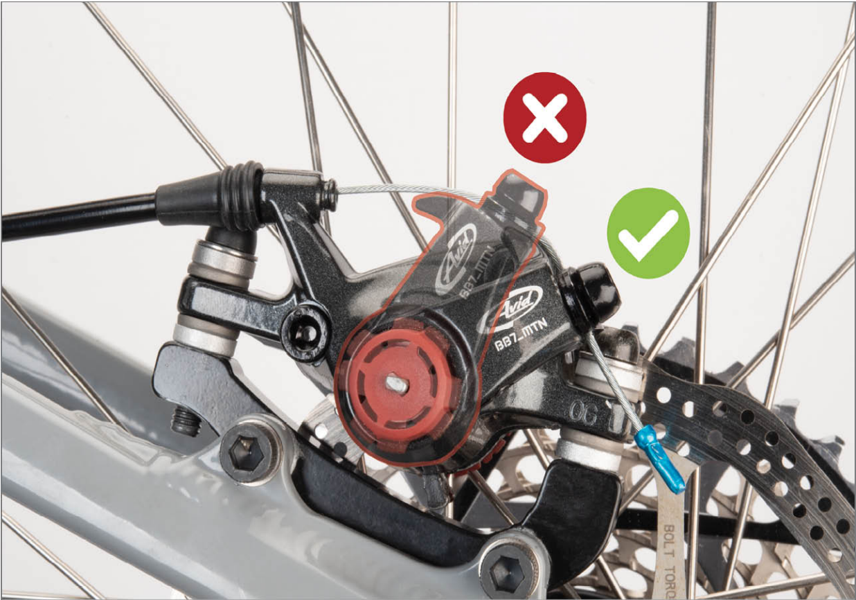
FIGURE 13.64: With brake lever open, caliper arm must start in back position
