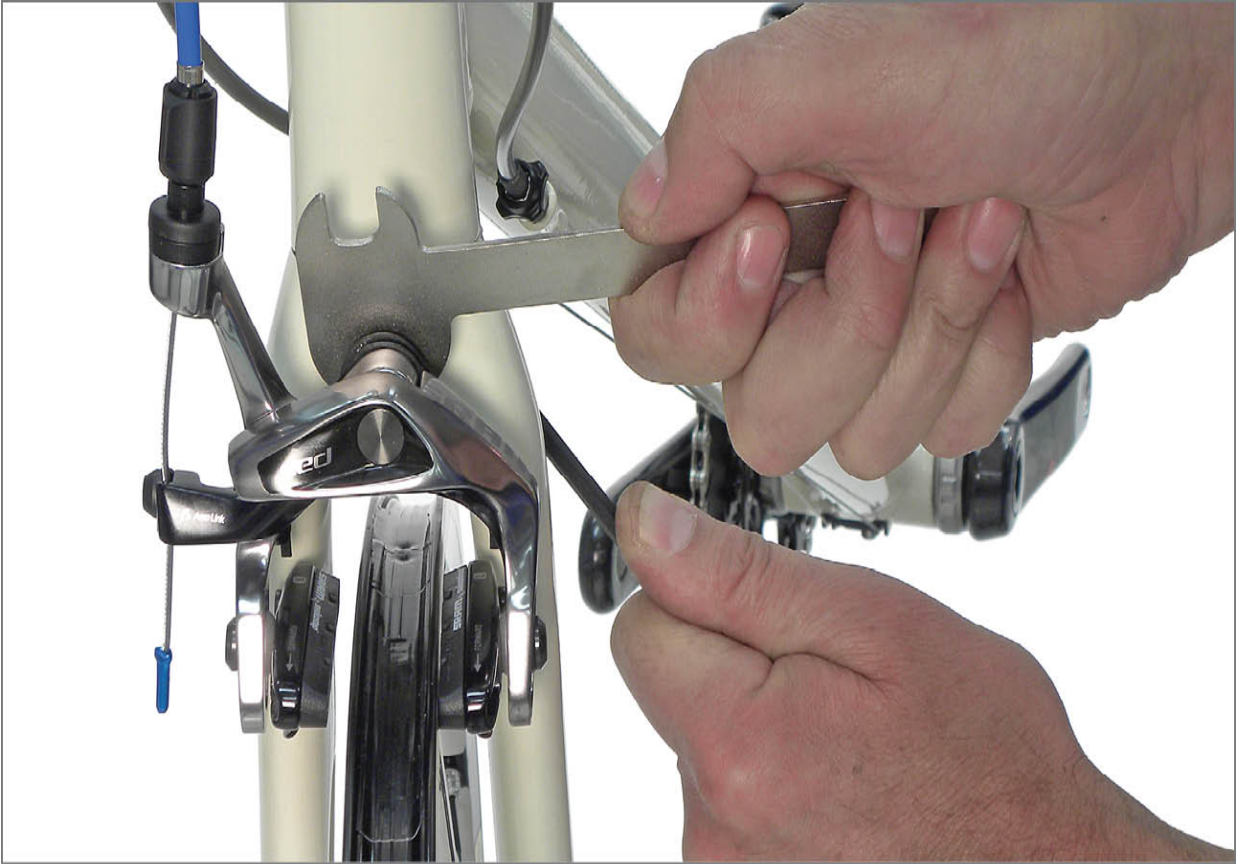
FIGURE 14.45: Move caliper using wrench on flats of brake stud with second wrench on mounting nut
