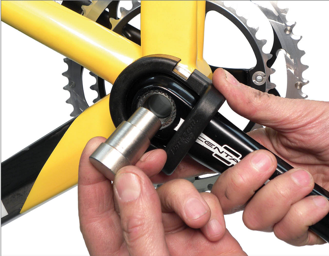
FIGURE 7.25: For aluminum crank install molded pad and extension plug
