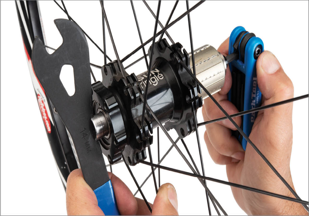
FIGURE 4.21: Hold slotted axle on left while turning right end cap to remove
