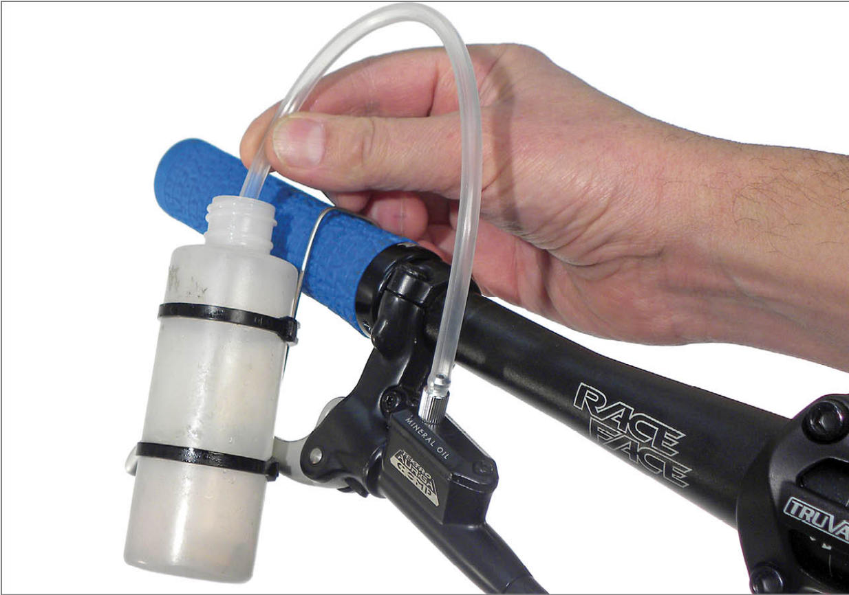
FIGURE 13.60: Brake fluid will bleed into waste bottle
