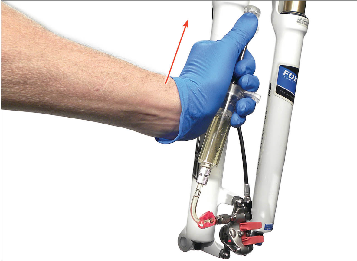
FIGURE 13.53: Pull back on plunger to create vacuum at caliper
