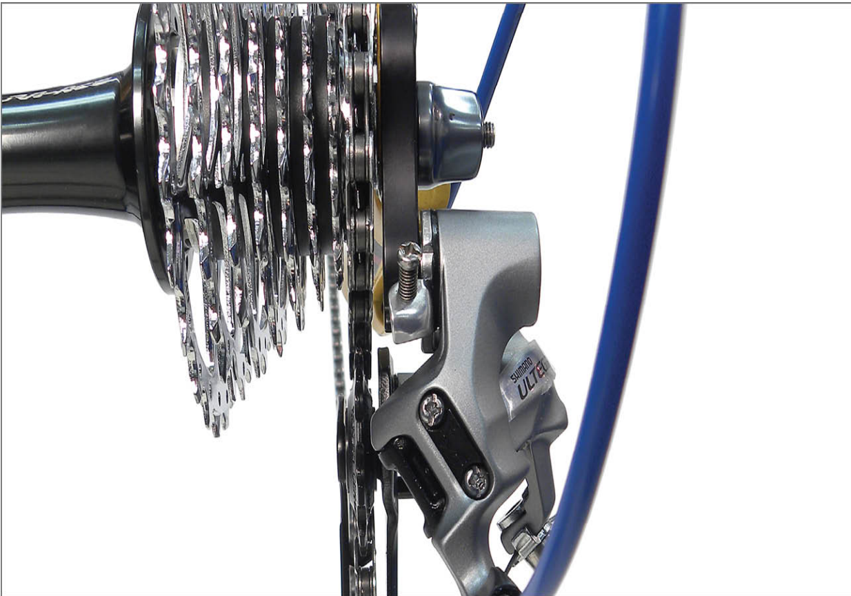
FIGURE 10.59: Inspect the H-limit by view behind and under the rear cogs
