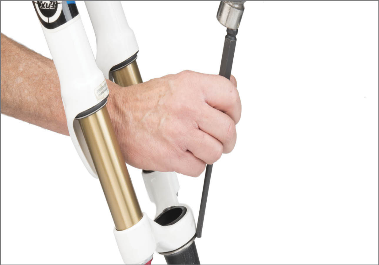
FIGURE 16.24: Carefully tap alternate side repeatedly to remove race
