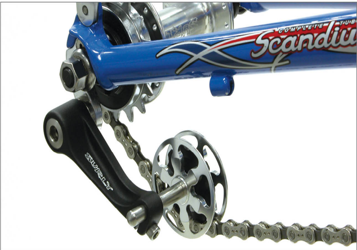
FIGURE 8.31: Vertical dropout with chain tension device
