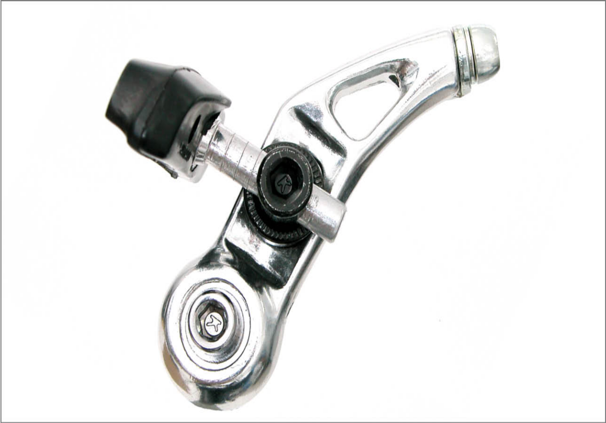
FIGURE 14.34: Smooth stud pad with curved washer system
