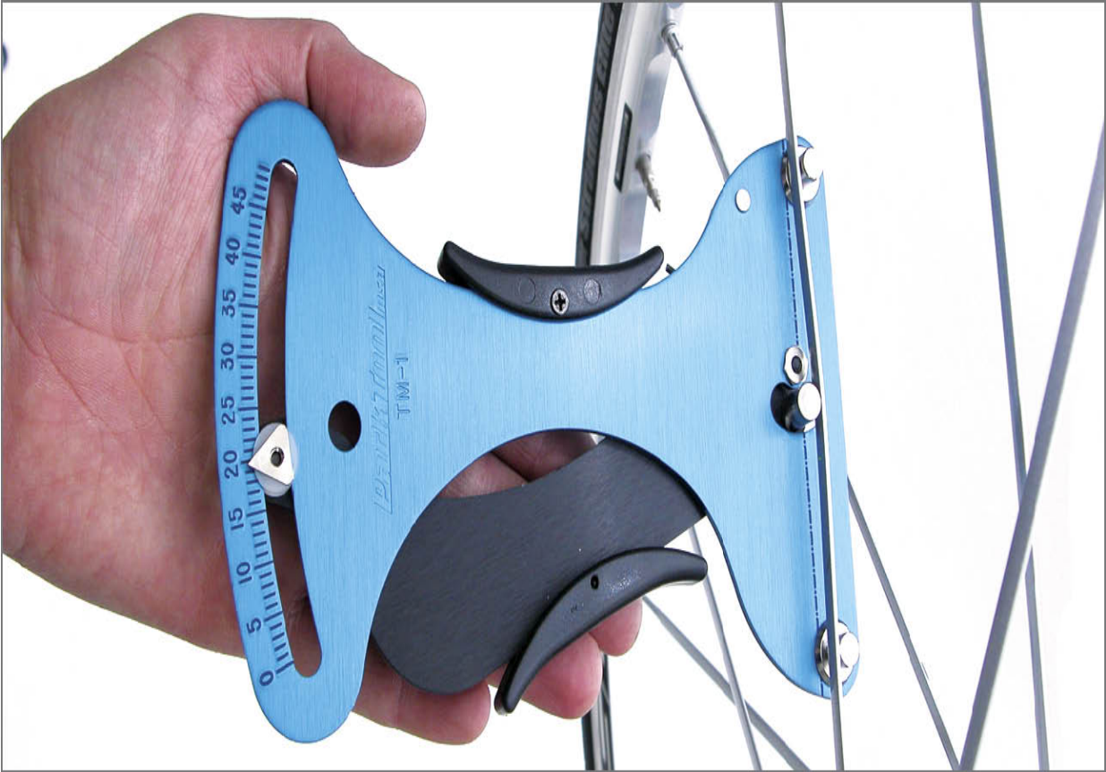
FIGURE 5.9: Spoke tension measurement with a tensiometer
