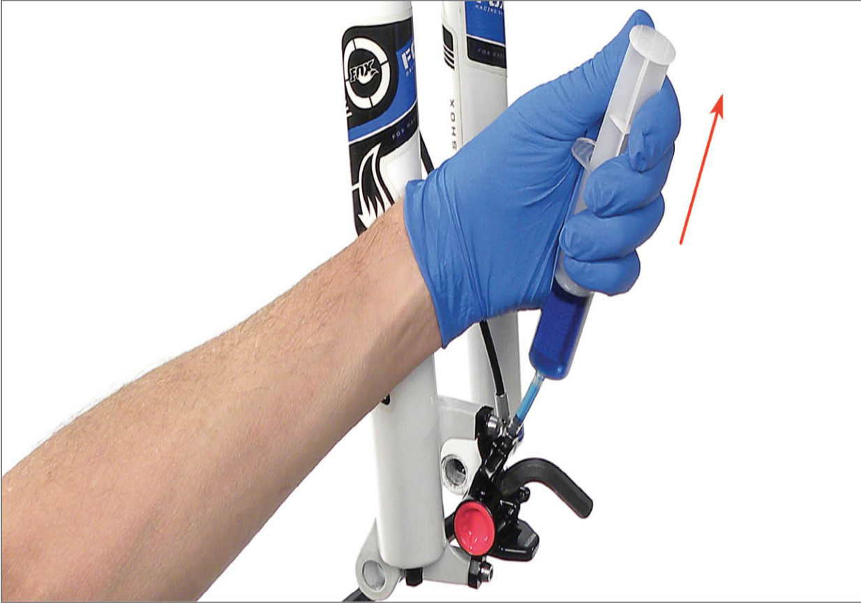
FIGURE 13.39: Alternatively push and pull at syringe to remove air from caliper
