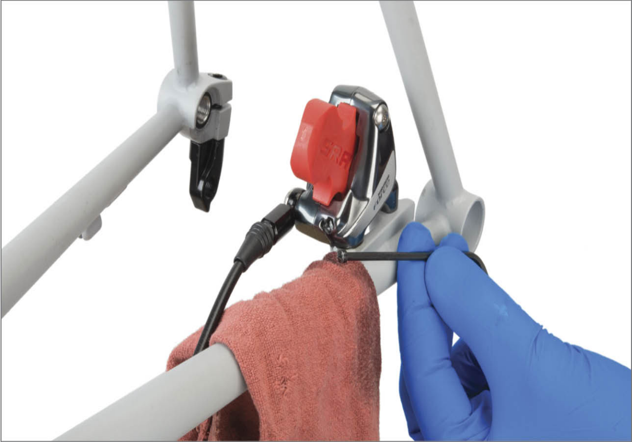
FIGURE 13.47: Remove bleed port screw at caliper
