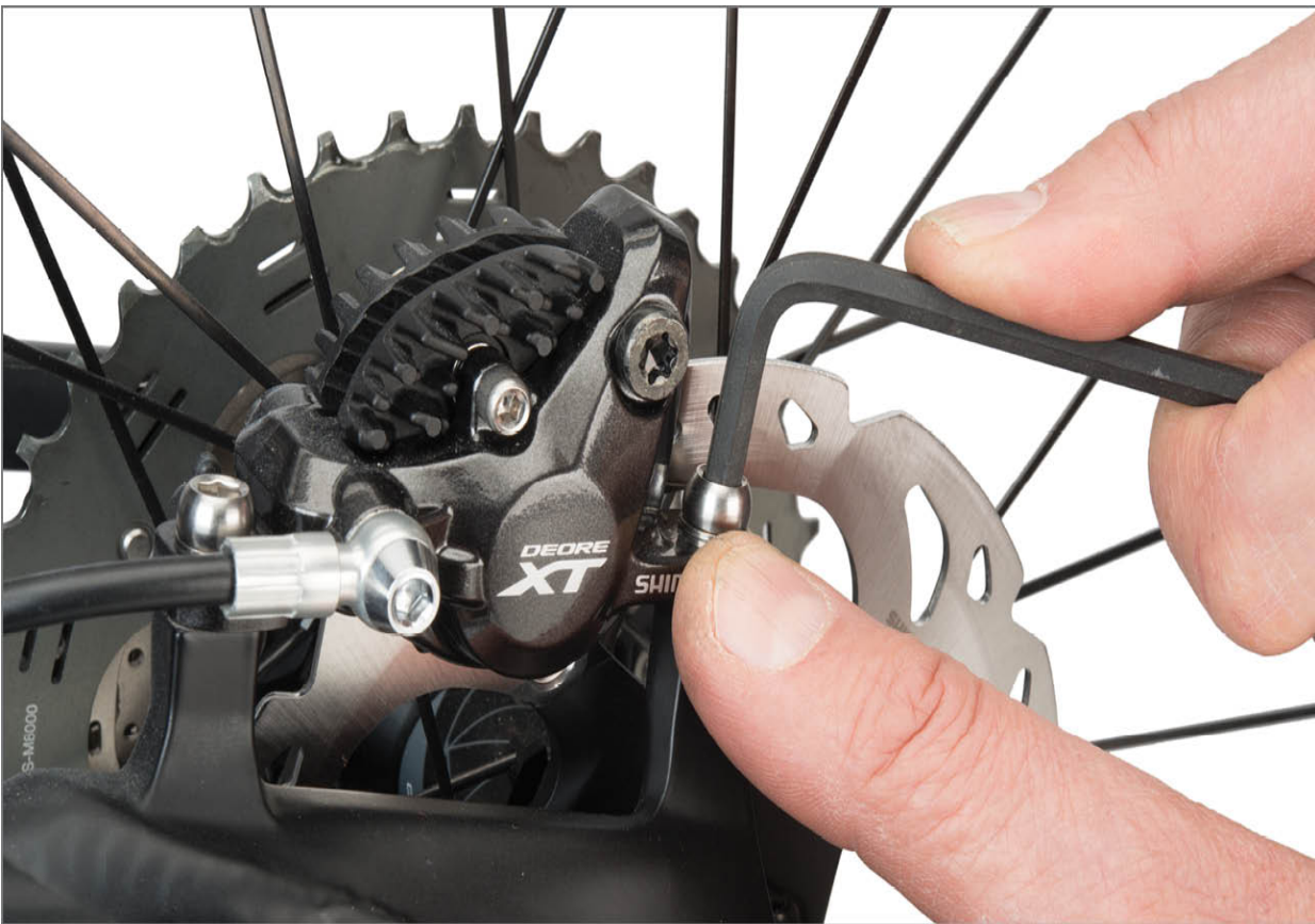
FIGURE 13.24: Align caliper pad to rotor and then tighten caliper-mounting bolts
