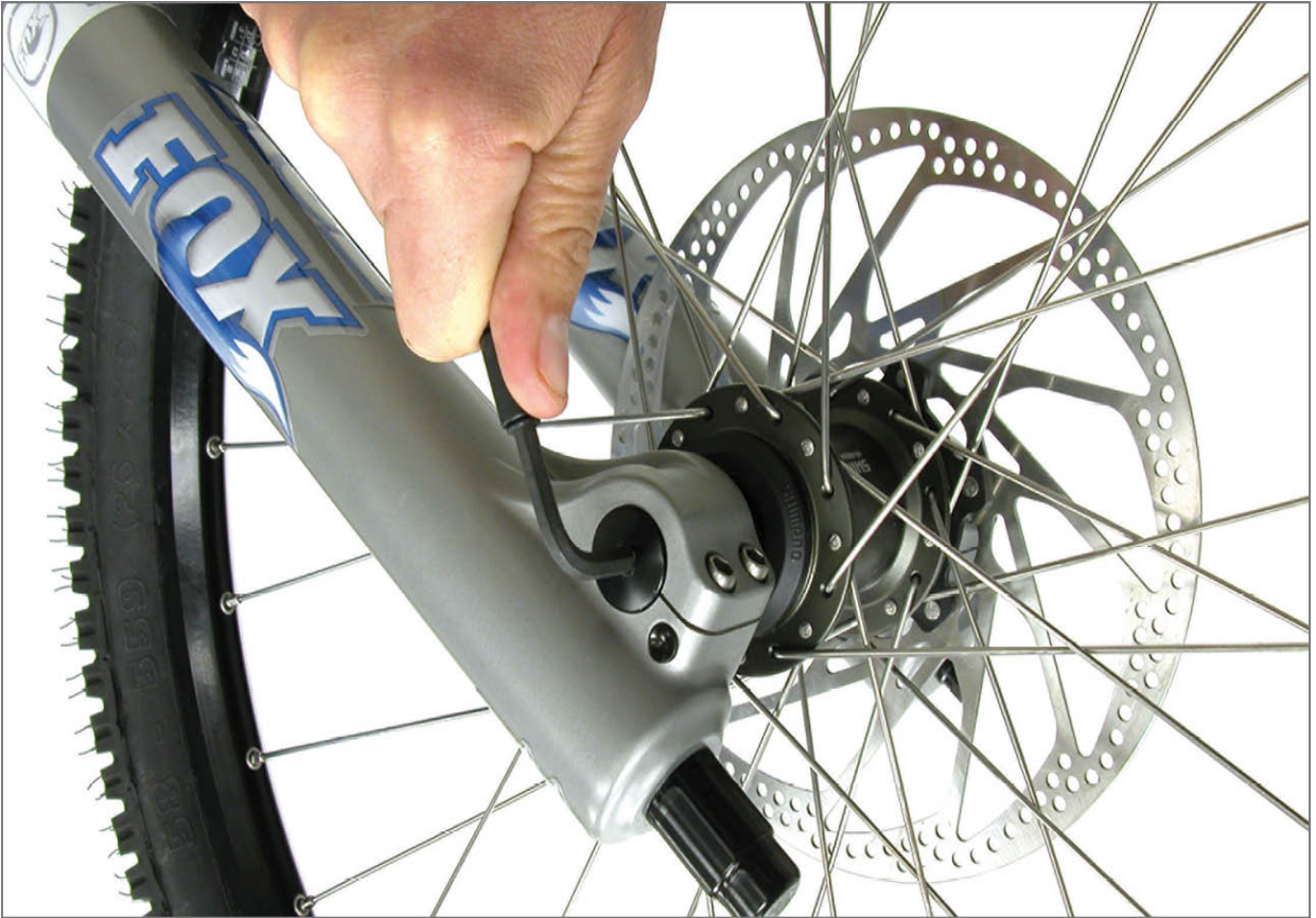
FIGURE 2.16: 20mm thru-axle fork and hub
