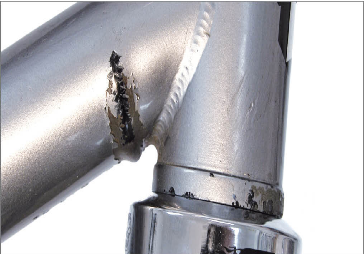
FIGURE 19.3: Bent frame at head tube
