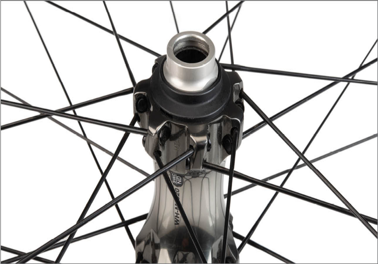
FIGURE 6.2: Straight pull spoke in compatible hub
