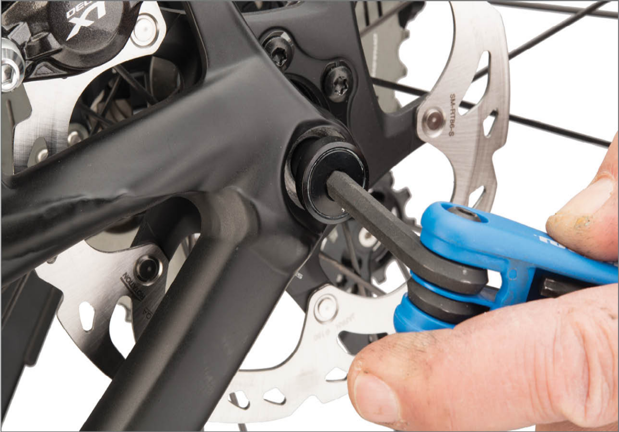
FIGURE 2.15: 6mm hex wrench removing axle
