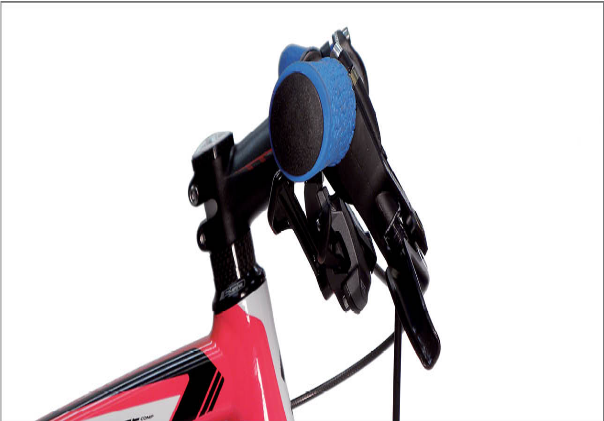
FIGURE 15.1: Upright handlebar rotated to a level or flat position
