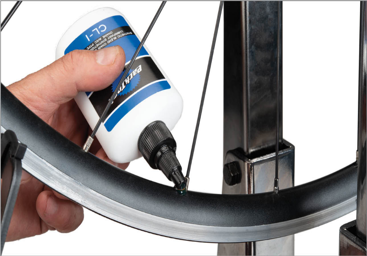
FIGURE 5.11: Use gravity to draw down a small drop on thread of spoke and allow it to drip to rim-nipple interface
