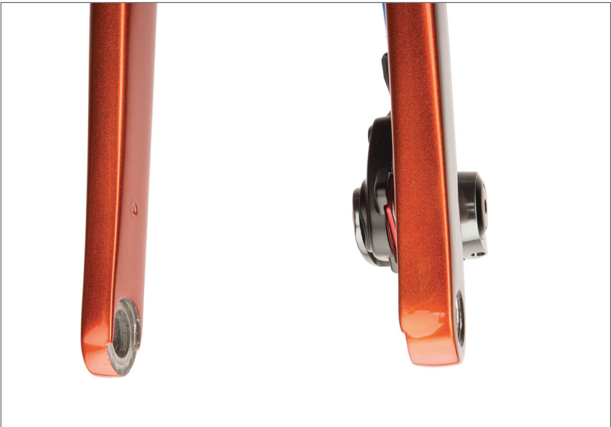
FIGURE 2.72: Recess in thru axle fork to accept end cap of hub
