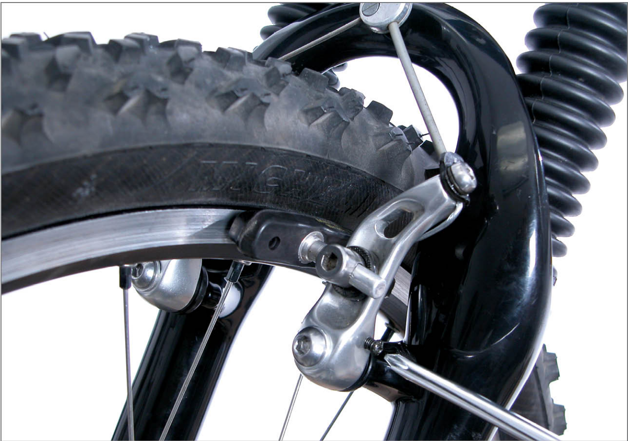
FIGURE 14.39: Use spring tension adjusting screw to center pads to rim
