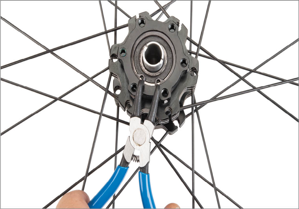
FIGURE 4.23: Inspect for and remove any C-clip using snap ring pliers
