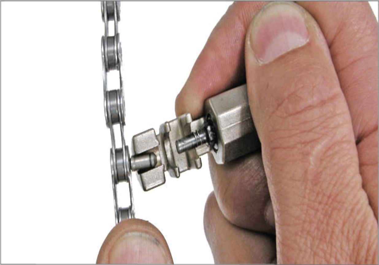
FIGURE 8.17: Break off pilot by twisting to the side
