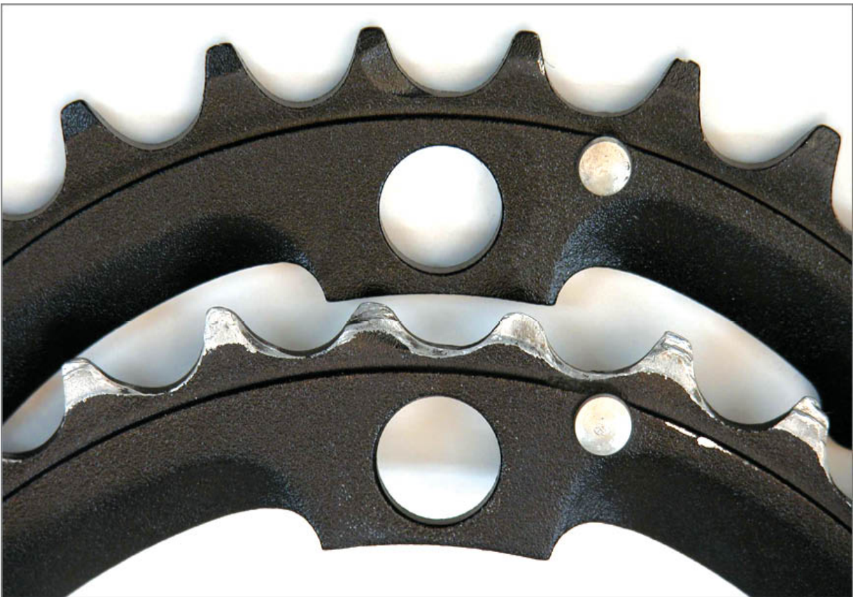
FIGURE 7.73: An obvious difference between an old ring and new ring
