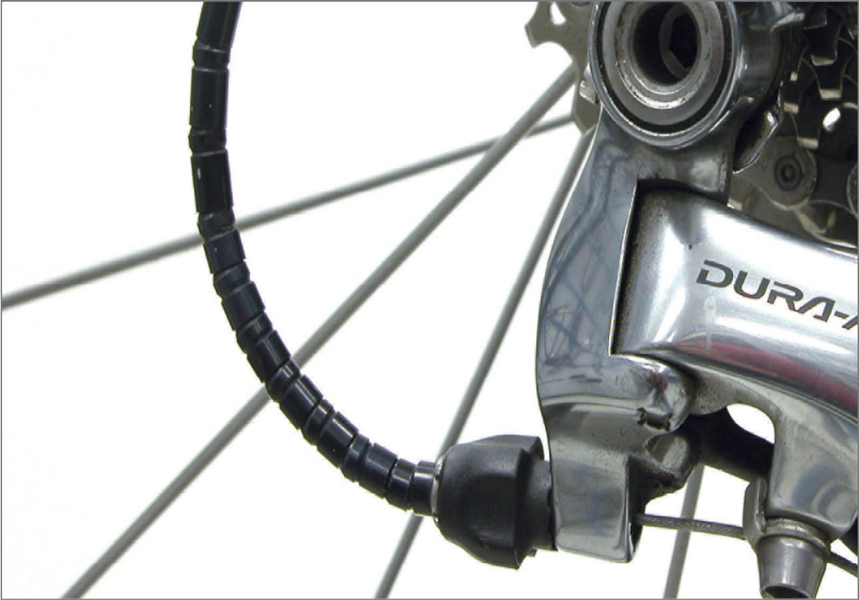
FIGURE 10.3: Articulated housing on a rear derailleur
