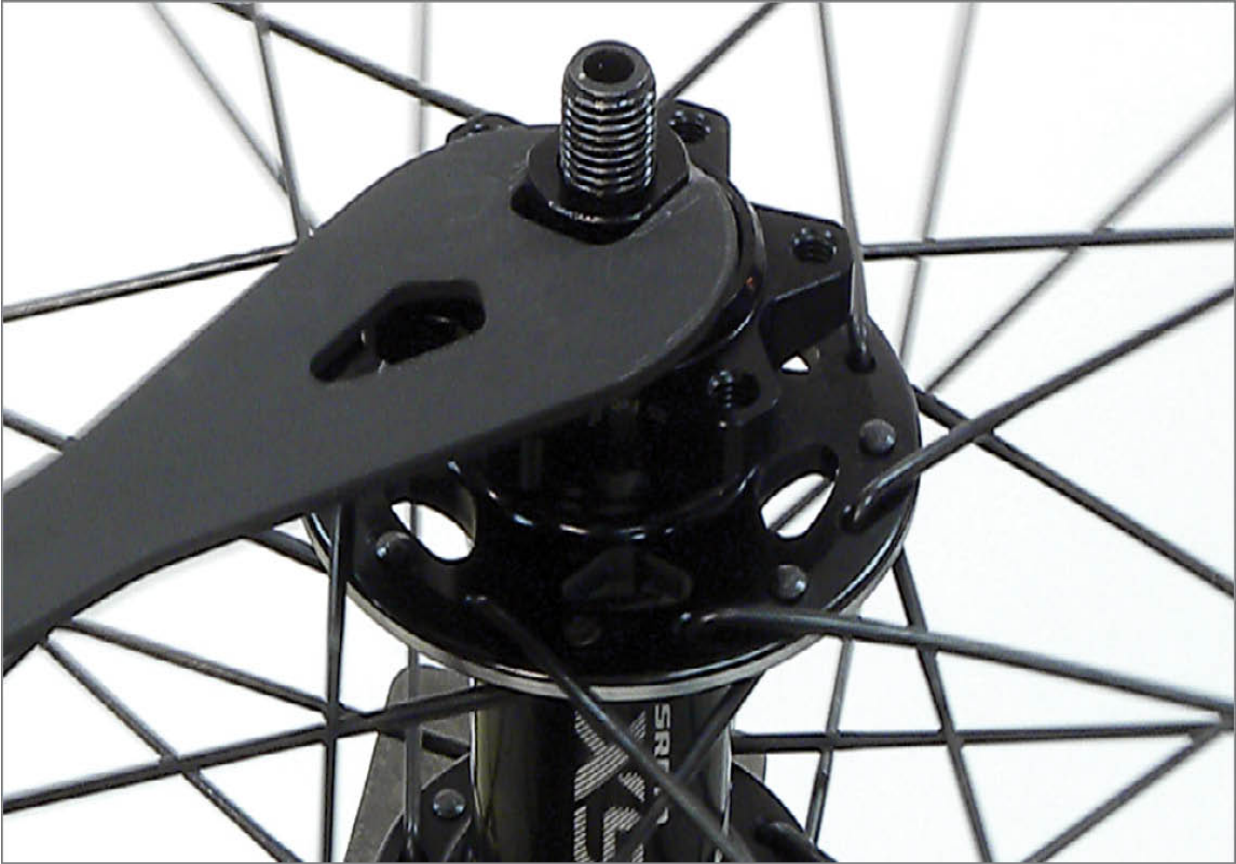
FIGURE 4.5: Cone wrenches are required to service the narrow flats of hub cones
