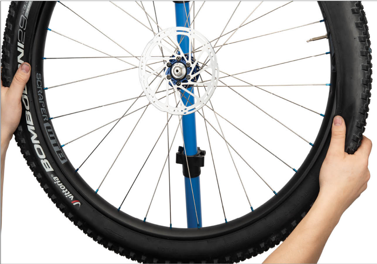
FIGURE 2.56: Engage beads from bottom working upward
