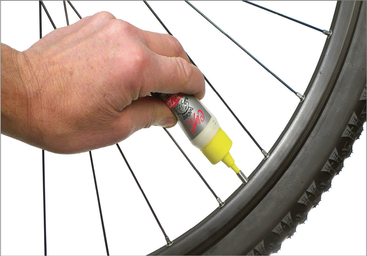
FIGURE 2.36: Rotate valve to allow sealant to easily enter the tube
