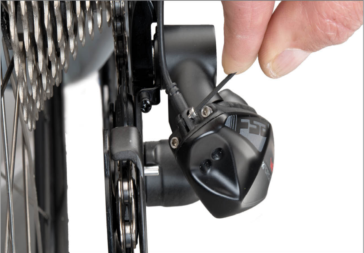
FIGURE 11.27: Rear wire plug pinch screw
