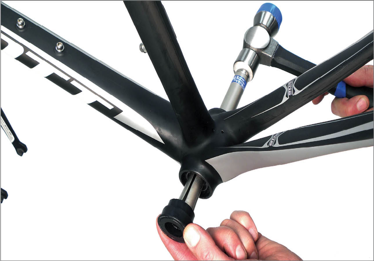
FIGURE 7.40: Use hammer and BBT-90.3 to drive bearing from bike
