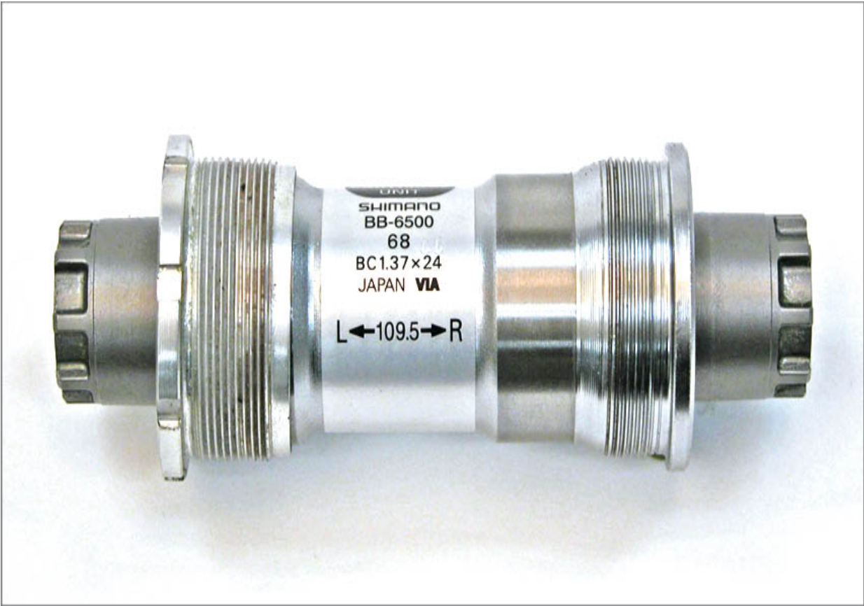
FIGURE 7.58: Bottom bracket marking indicating appropriate side of bike
