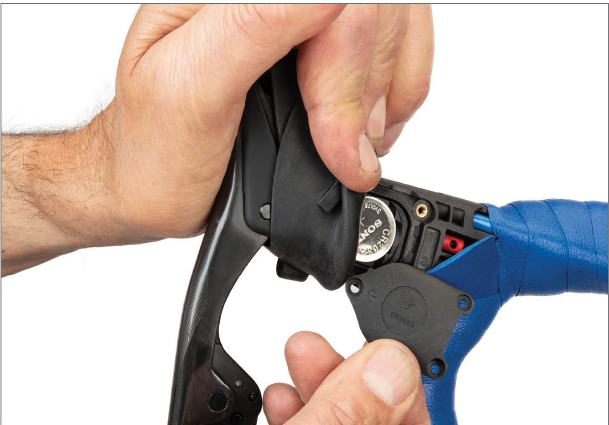
FIGURE 11.18: Battery is under the cover on inside of lever body
