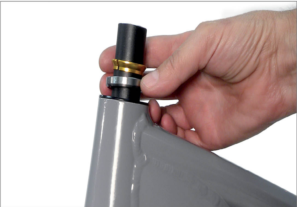
FIGURE 16.9: Cartridge bearing orientation
