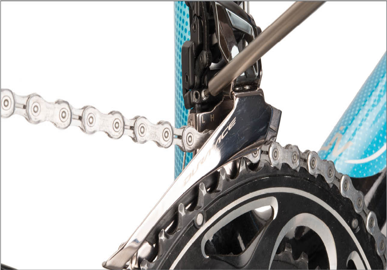
FIGURE 10.52: The Shimano® toggle design front derailleur and H-limit screw
