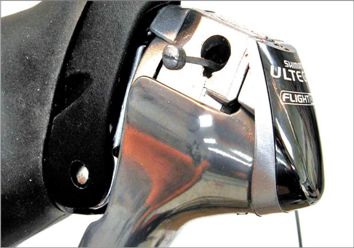
FIGURE 10.22: Feed cable through socket at top of lever
