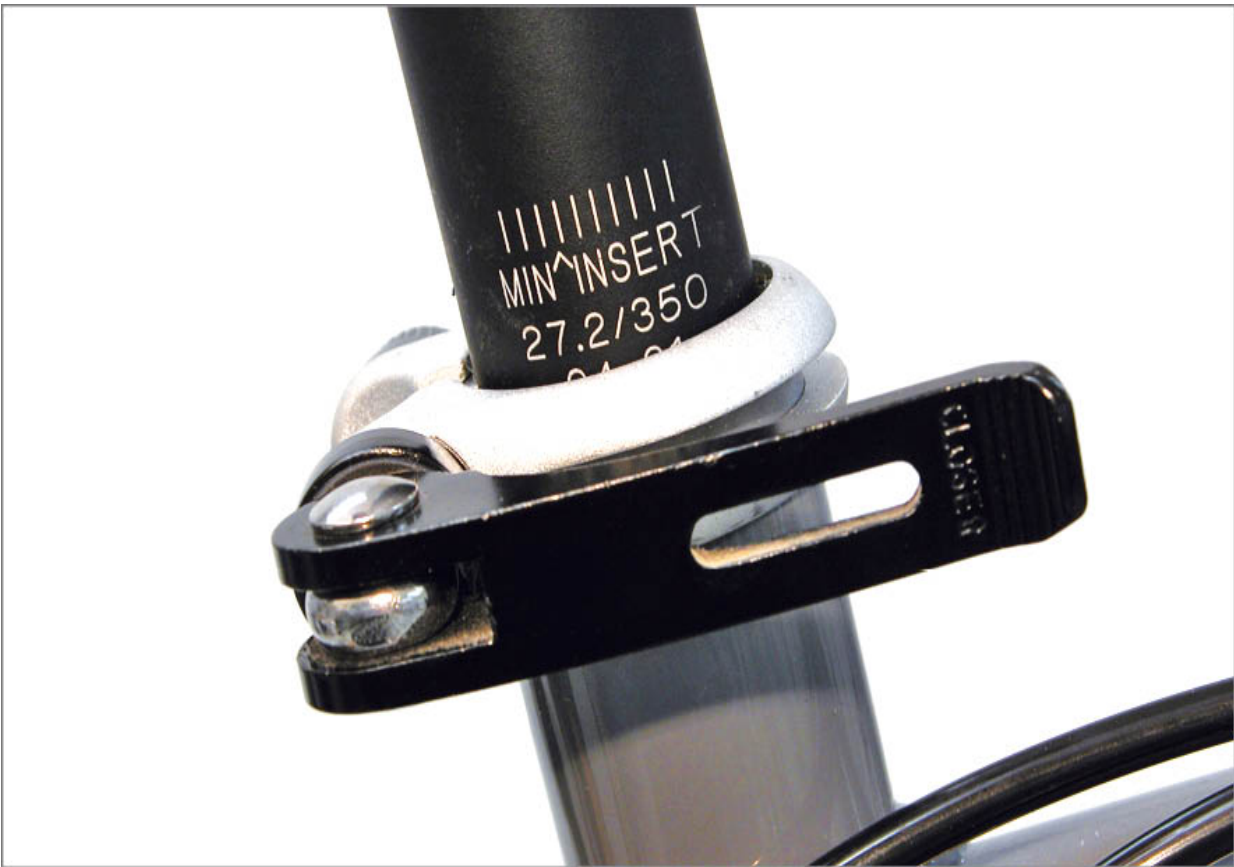
FIGURE 15.25: Post is too high if minimum insertion line is seen
