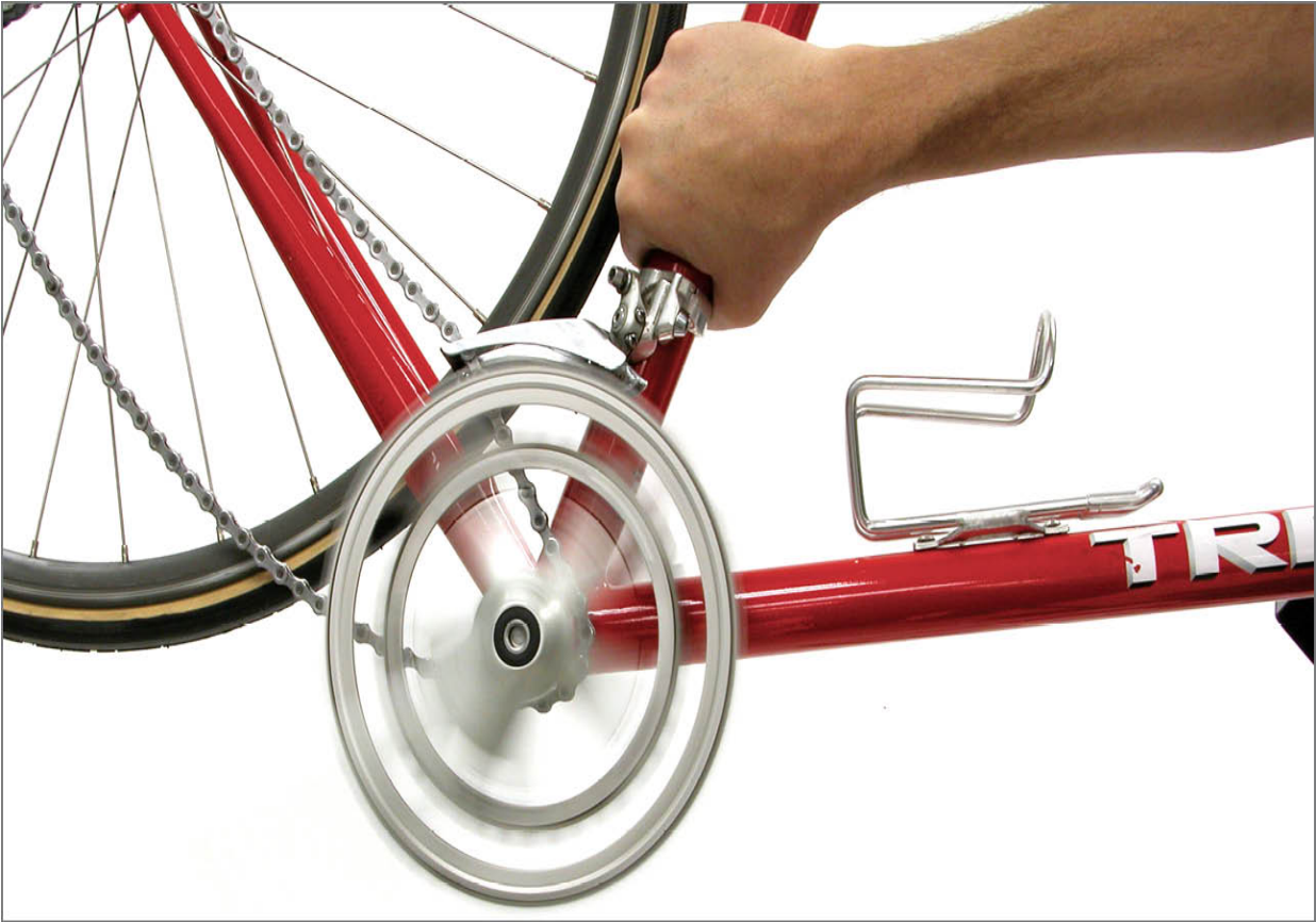
FIGURE 7.30: Spin cranks to feel for grinding on a worn bottom bracket bearing
