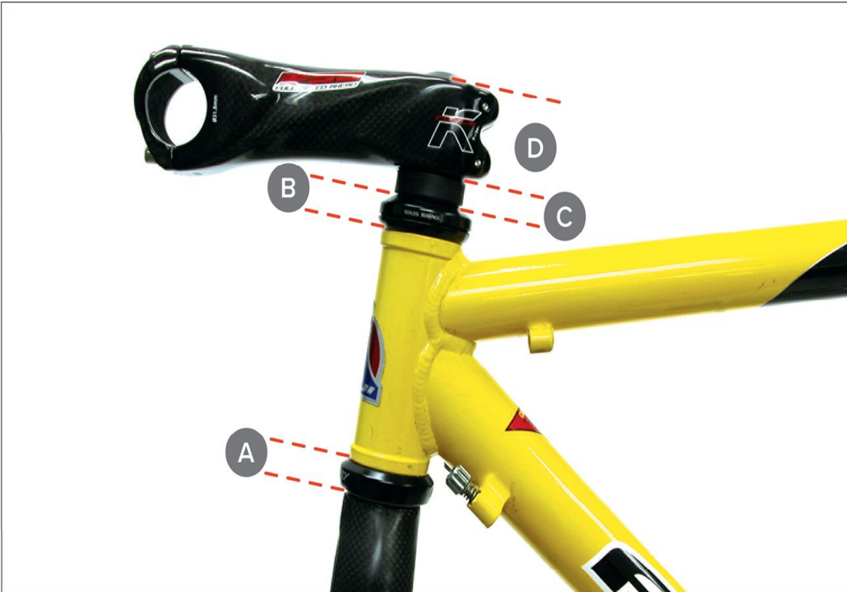
FIGURE 16.20: Stack height is composed of: (A) lower stack height, (B) upper stack height, (C) any spacers; stem height (D) not included
