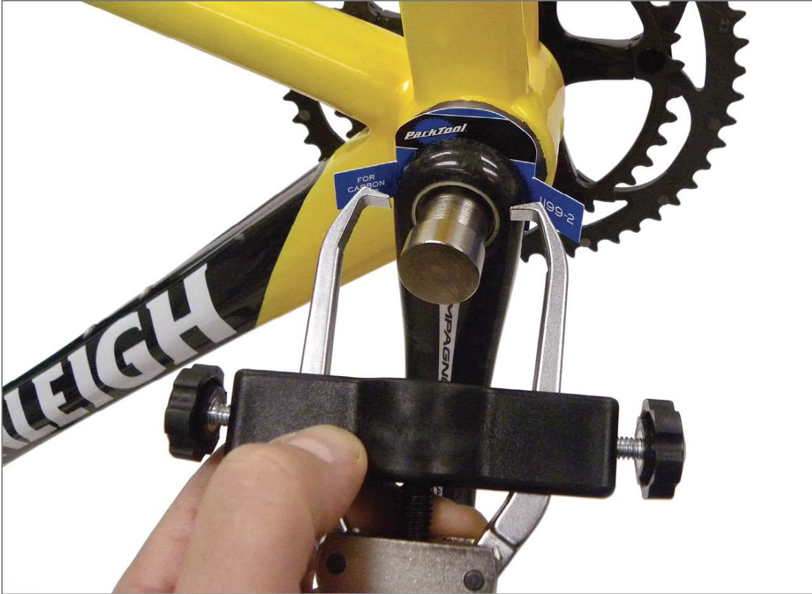
FIGURE 7.26: Fiberboard protection in place on carbon fiber crank
