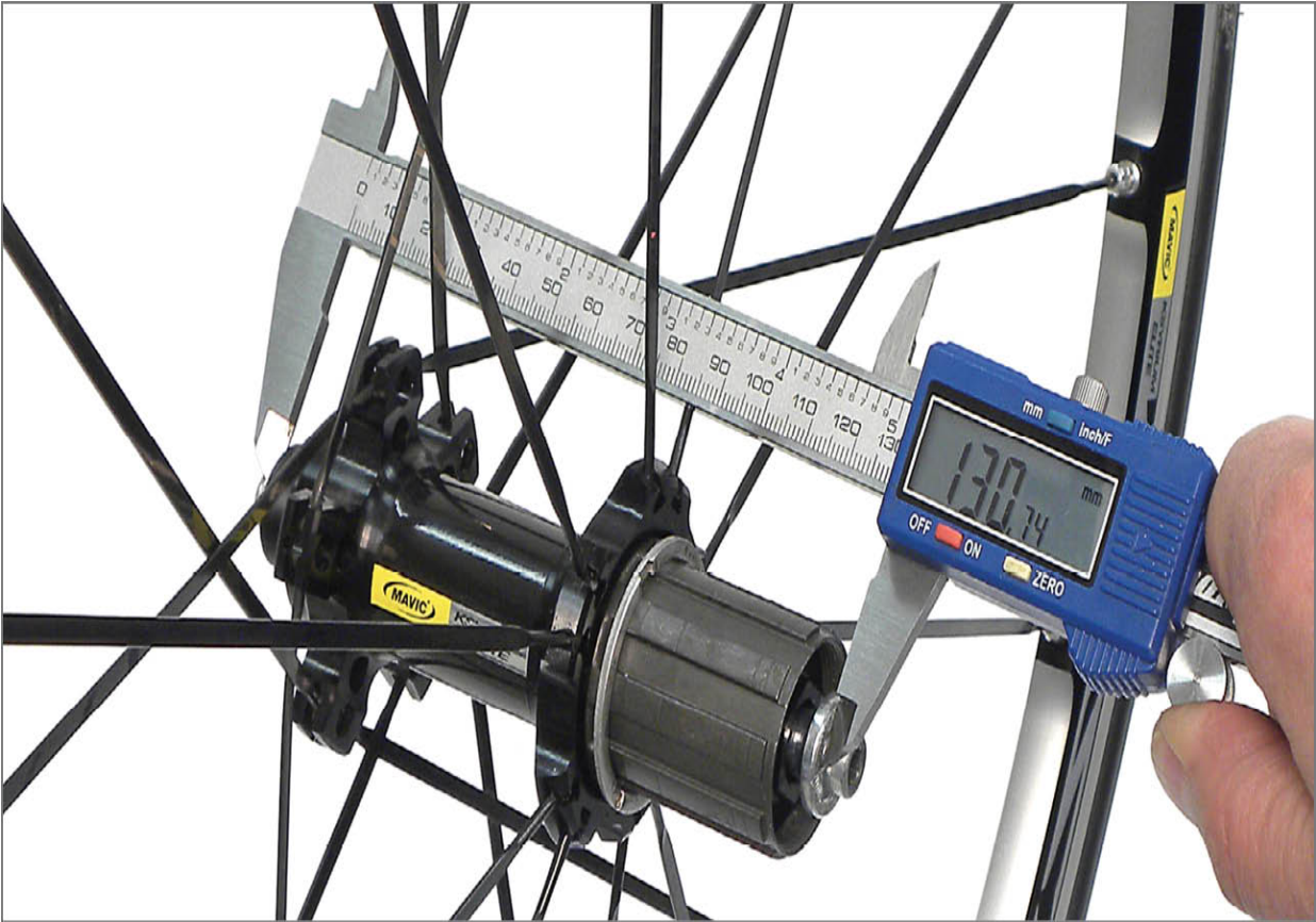
FIGURE 4.2: Measuring rear hub width
