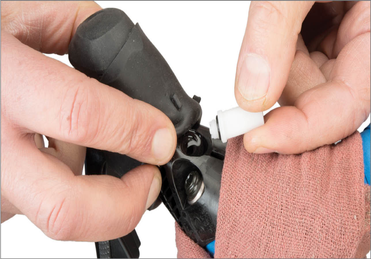
FIGURE 13.29: Bleed port and extension on drop bar lever
