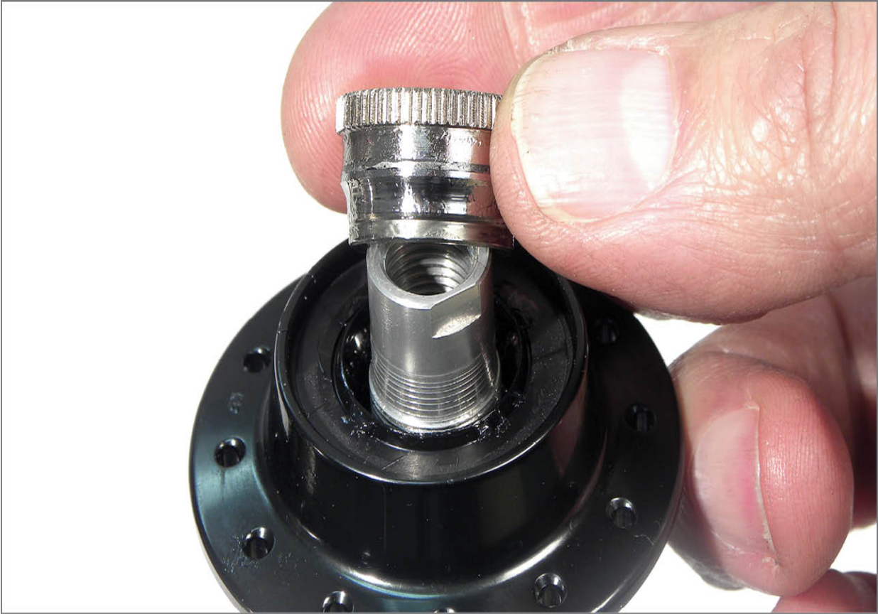
FIGURE: 4.16: Shimano® Dura-Ace® 9000 rear hub threaded cone and axle
