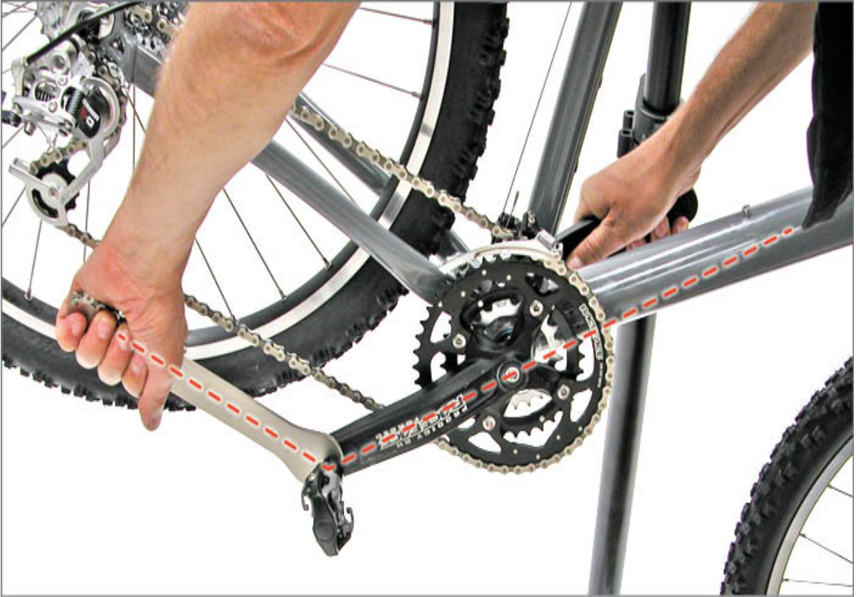
FIGURE 1.6: Poor mechanical advantage
