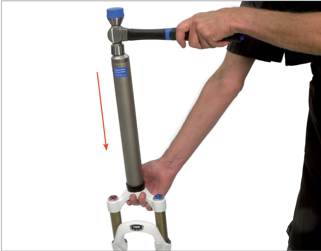
FIGURE 16.28: Installing the fork crown race with a crown race setter
