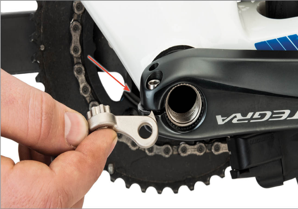
FIGURE 7.14: Lift stop plate to pull off Shimano® Hollowtech® II crank
