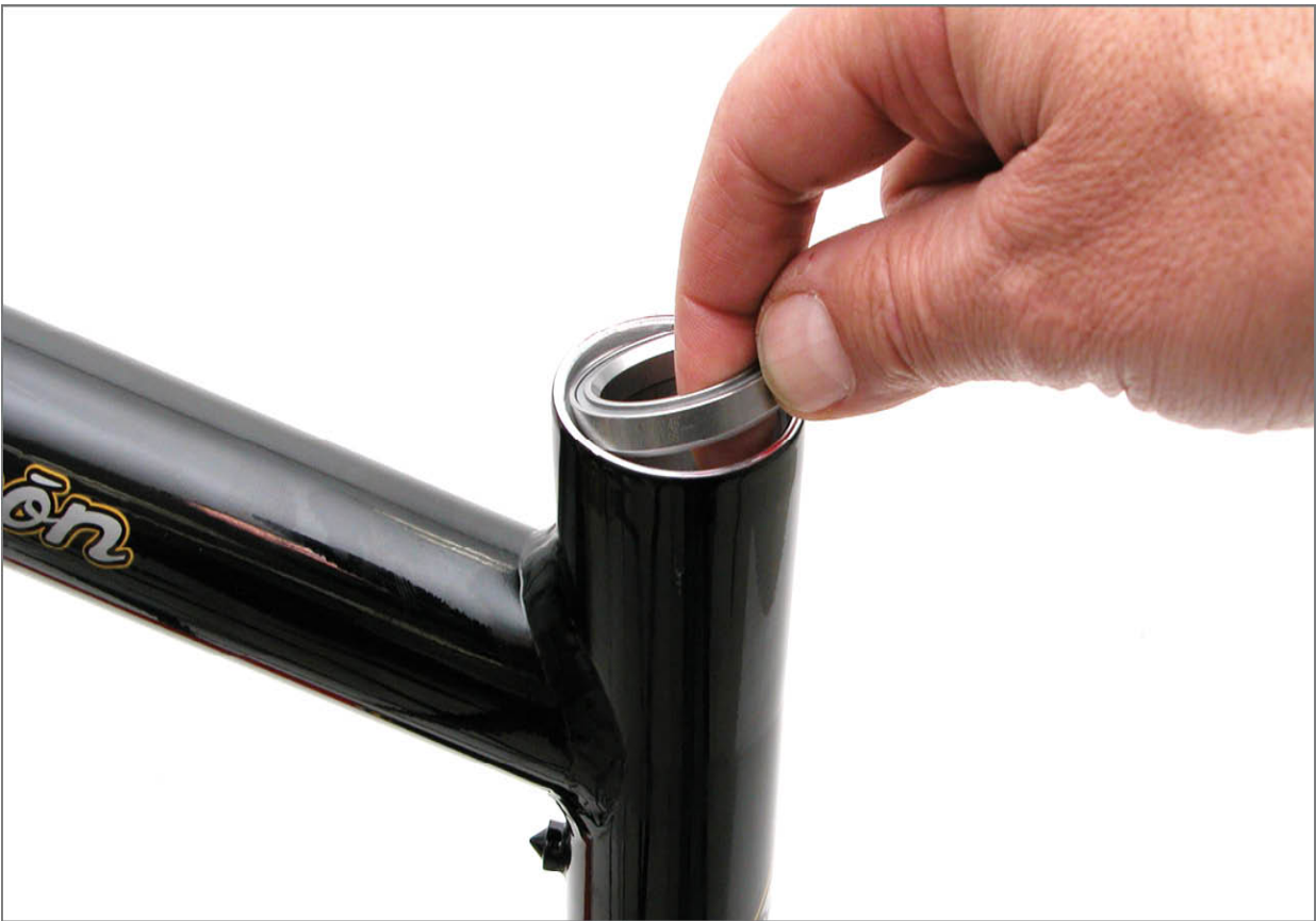
FIGURE 16.21: Removing the slip fit integrated bearing from an IS headset
