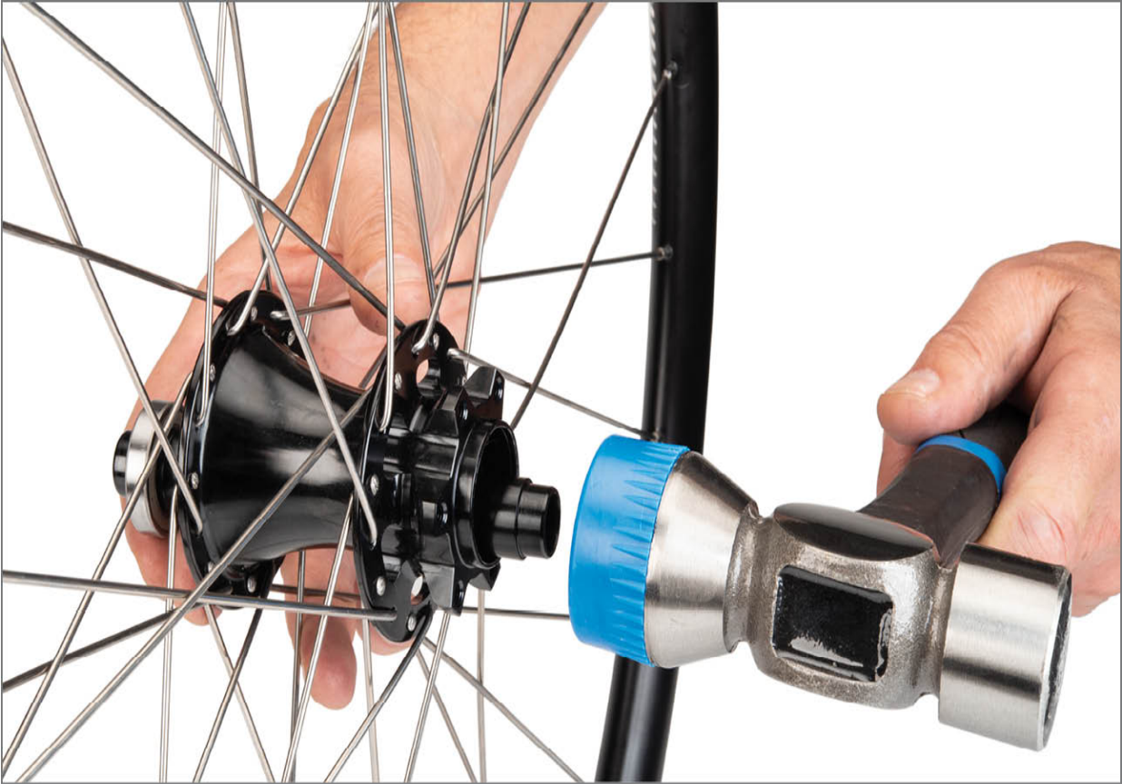
FIGURE 4.26: Use sleeved axle as a punch to remove second bearing
