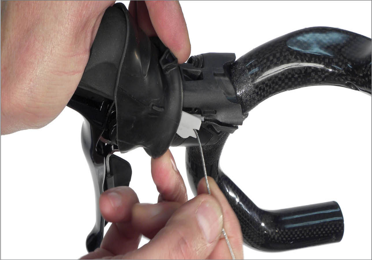
FIGURE 10.24: Use cable to pull open cable access cover
