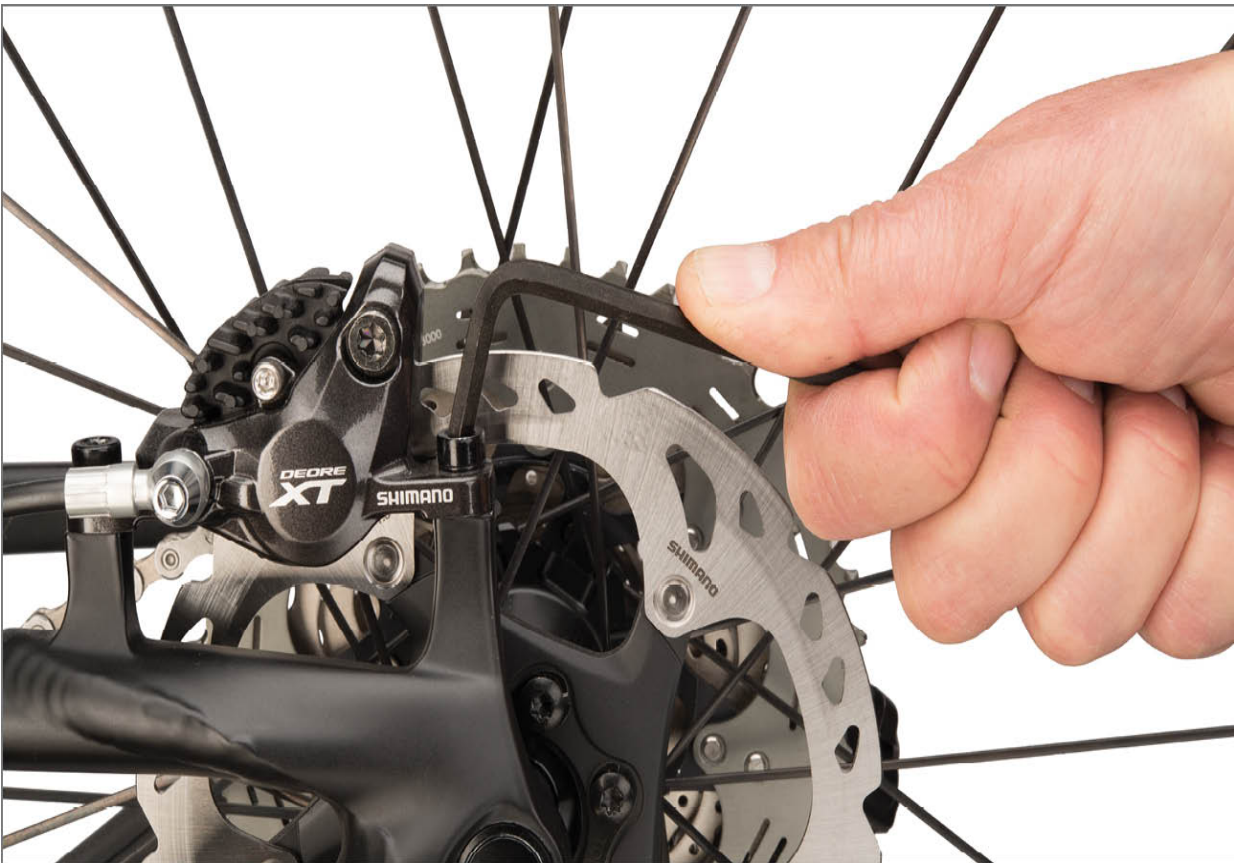
FIGURE 1.9: Poor tool alignment will damage bolt and wrench
