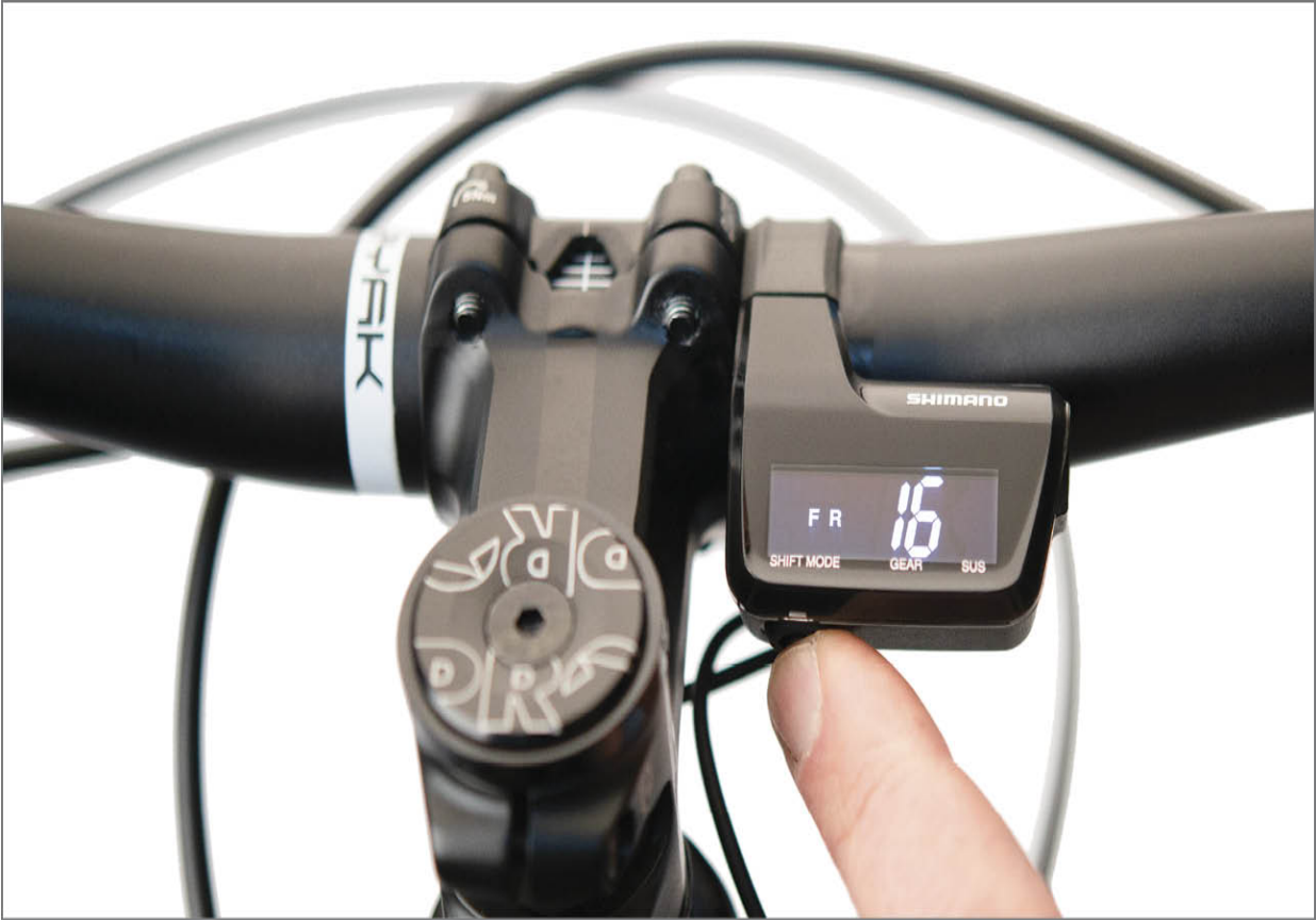
FIGURE 11.15: Press and release shift mode button on MTB Di2® to enter
