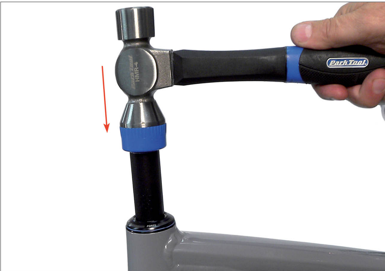
FIGURE 16.10: If necessary drive fork column down using a mallet
