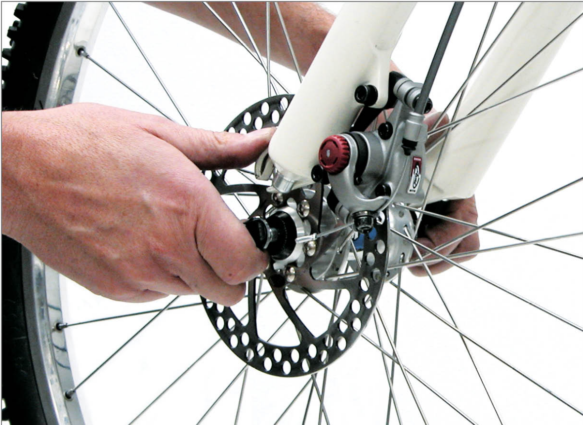
FIGURE 2.71: Guide rotor between caliper disc brake pads
