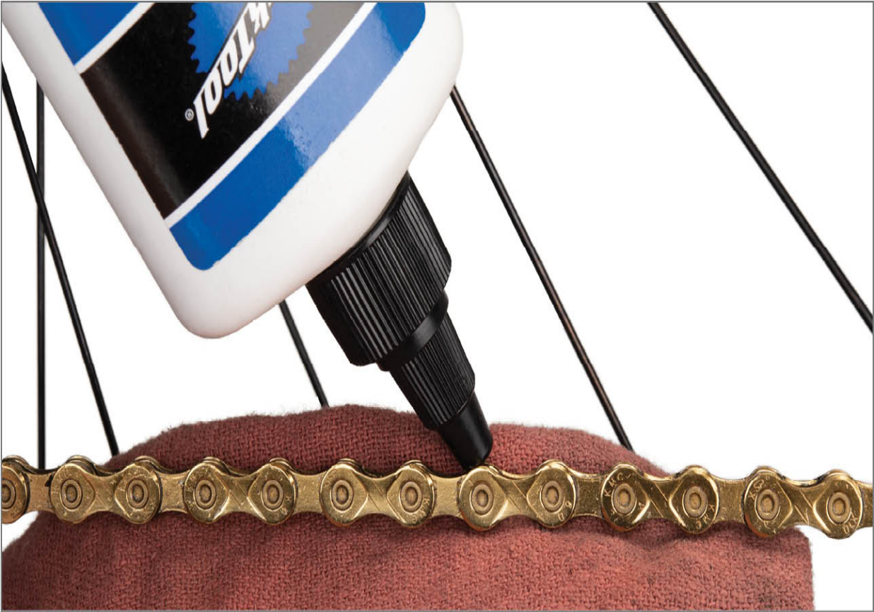
FIGURE 8.39: Lubricate and inspect chain in the same procedure
