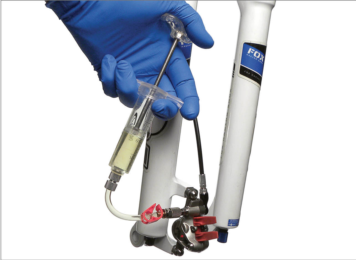
FIGURE 13.50: Push fluid through caliper toward brake lever
