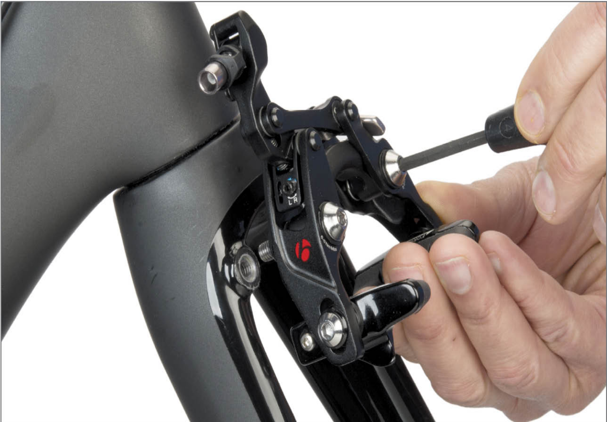
FIGURE 14.46: Direct mount fittings on fork that accept mount bolts of direct mount brake
