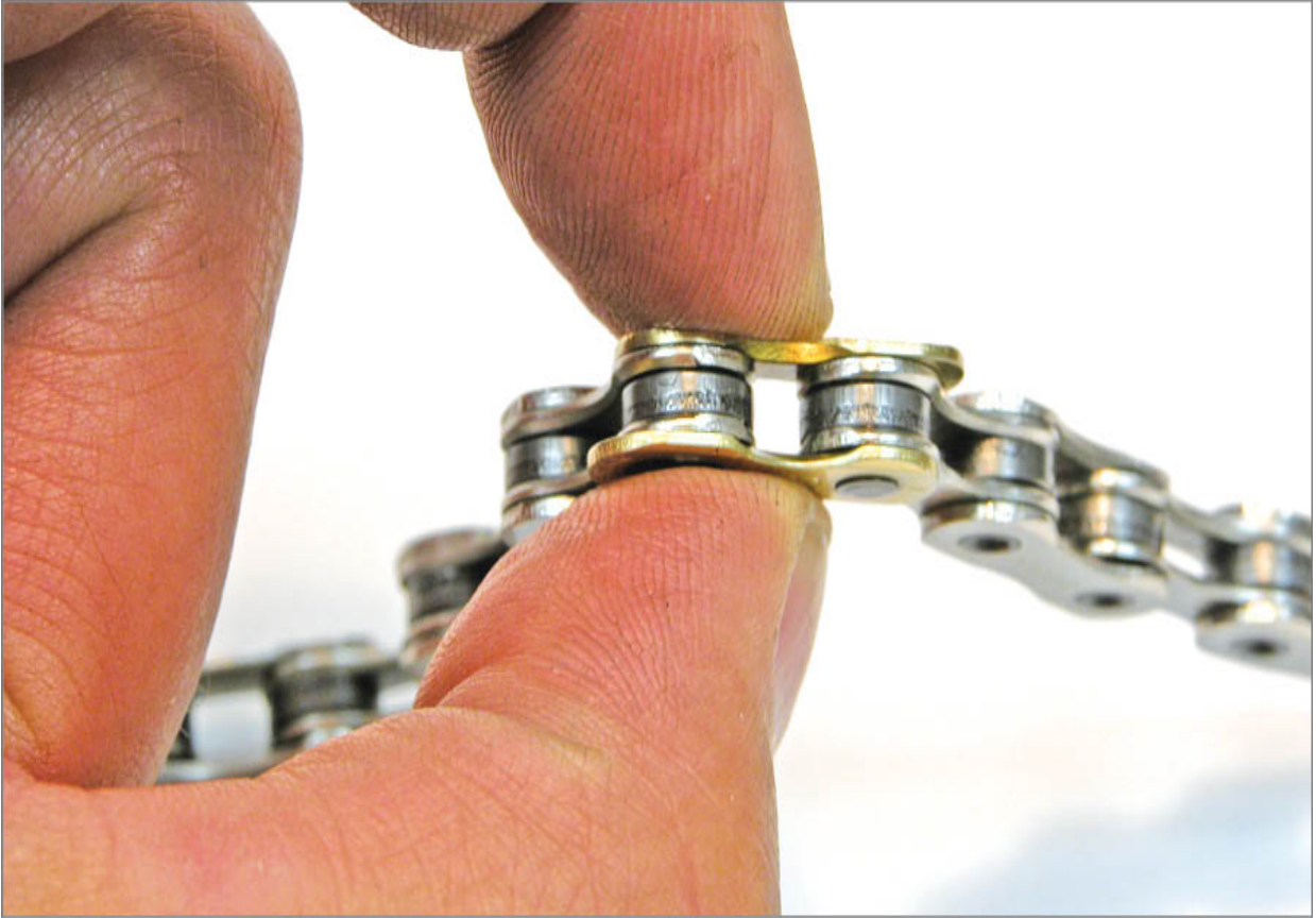
FIGURE 8.24: Push plates in opposite directions to remove
