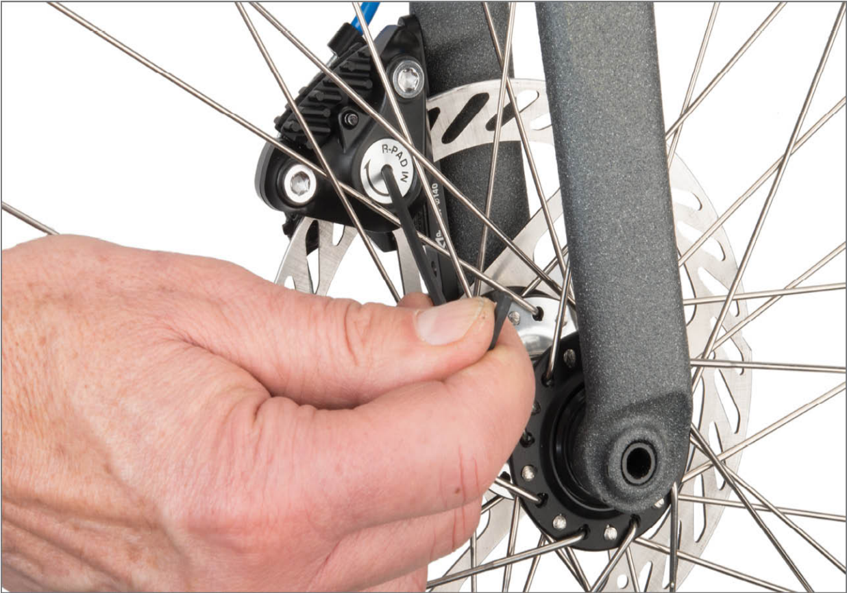
FIGURE 13.65: Use adjusting pad screw to move pad to rotor
