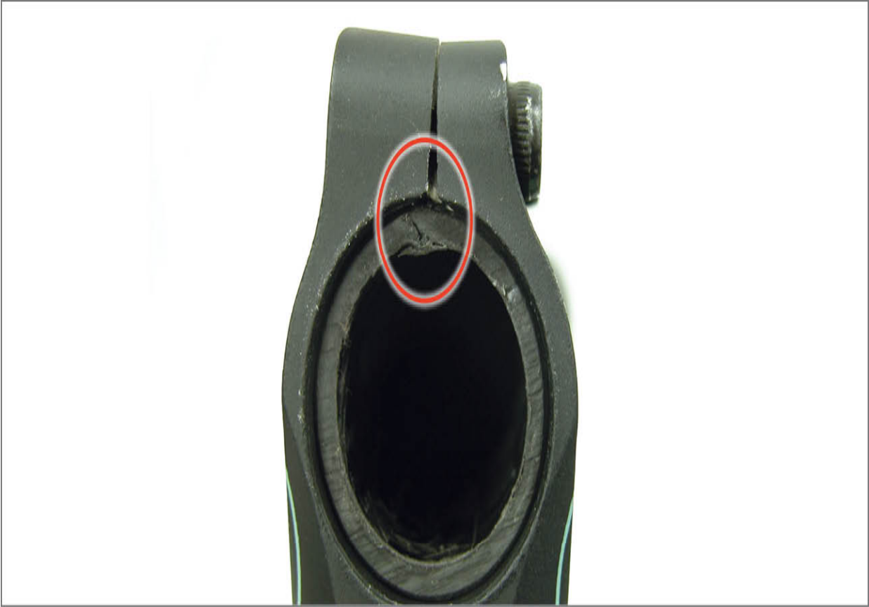
FIGURE 15.20: Cracked steering column from stem binder bolt
