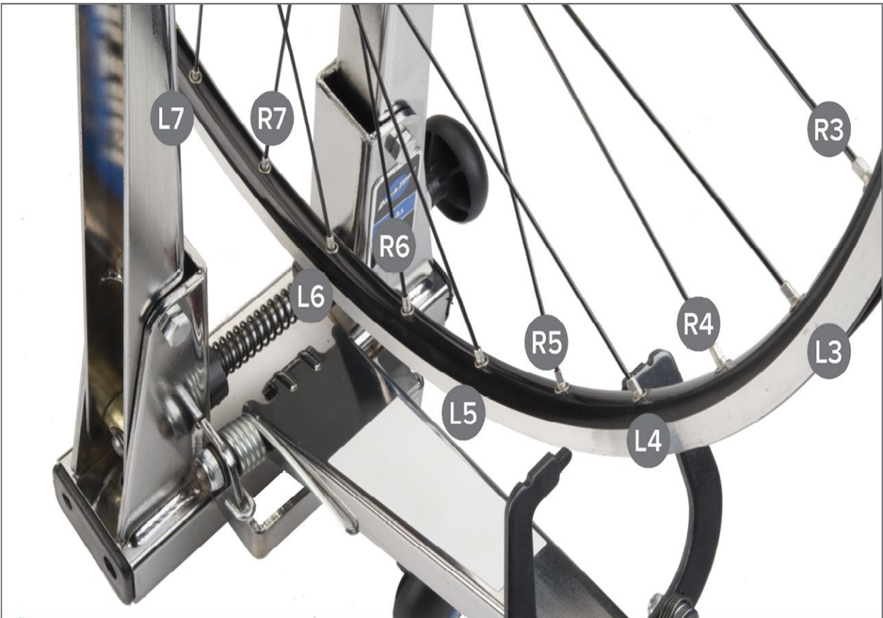
FIGURE 5.14: Use changes in spoke tension to move sections of rim
