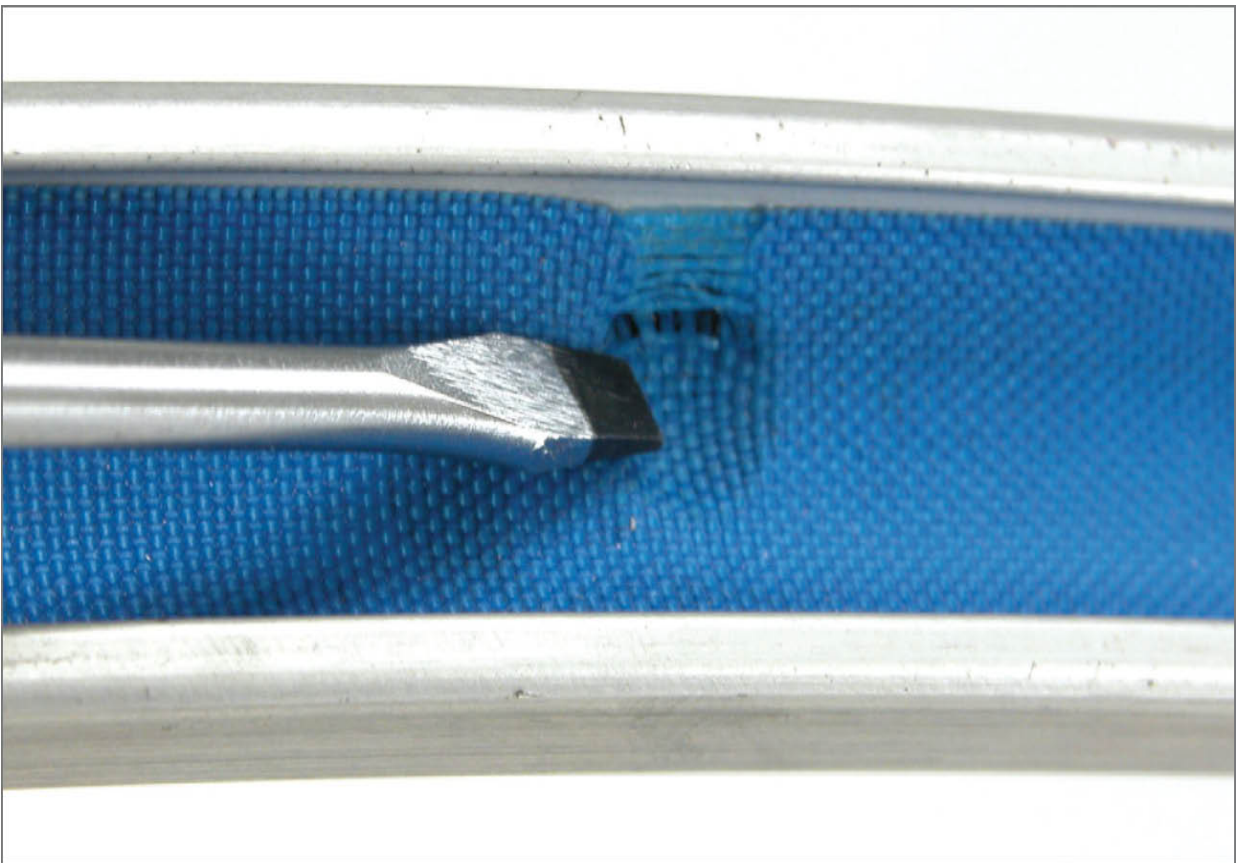
FIGURE 2.30: Holes in rim strip will cause flats
