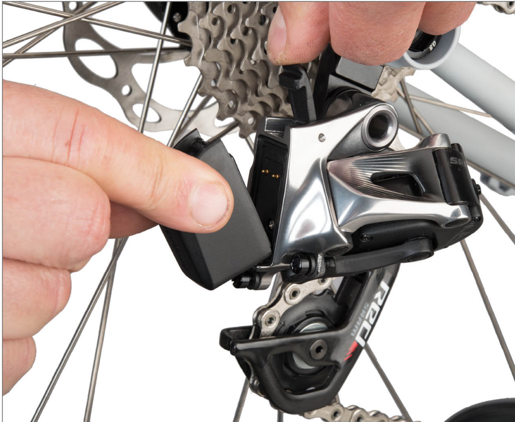
FIGURE 11.20: Battery attachment to rear derailleur
