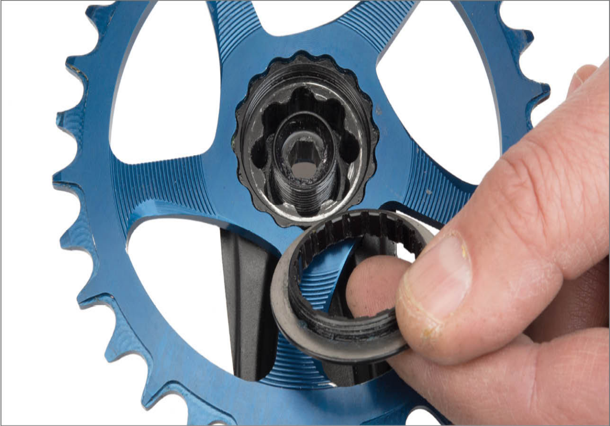
FIGURE 7.68: Direct mount chainring of a Race Face® crank
