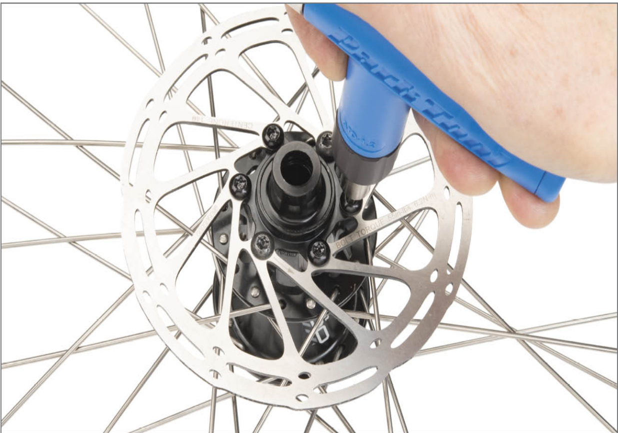
FIGURE 13.14: Secure rotor bolts using T25 driver
