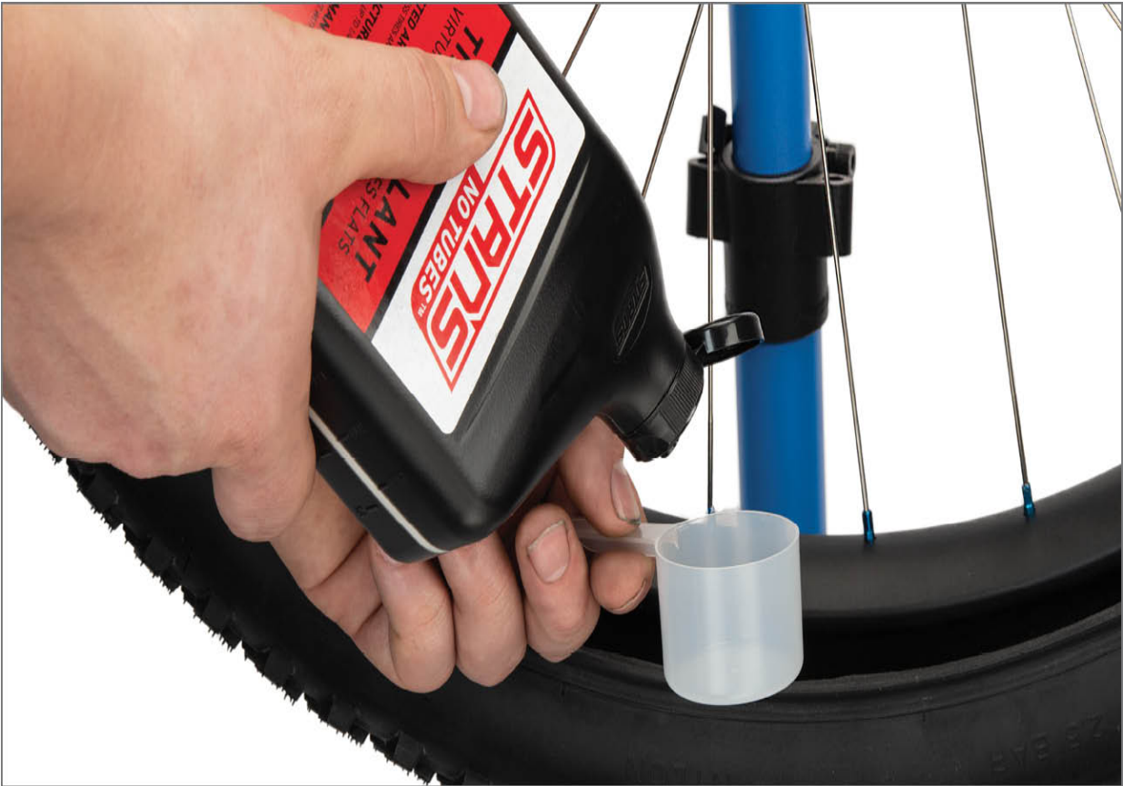
FIGURE 2.55: Pour in fluid at bead opening at bottom
