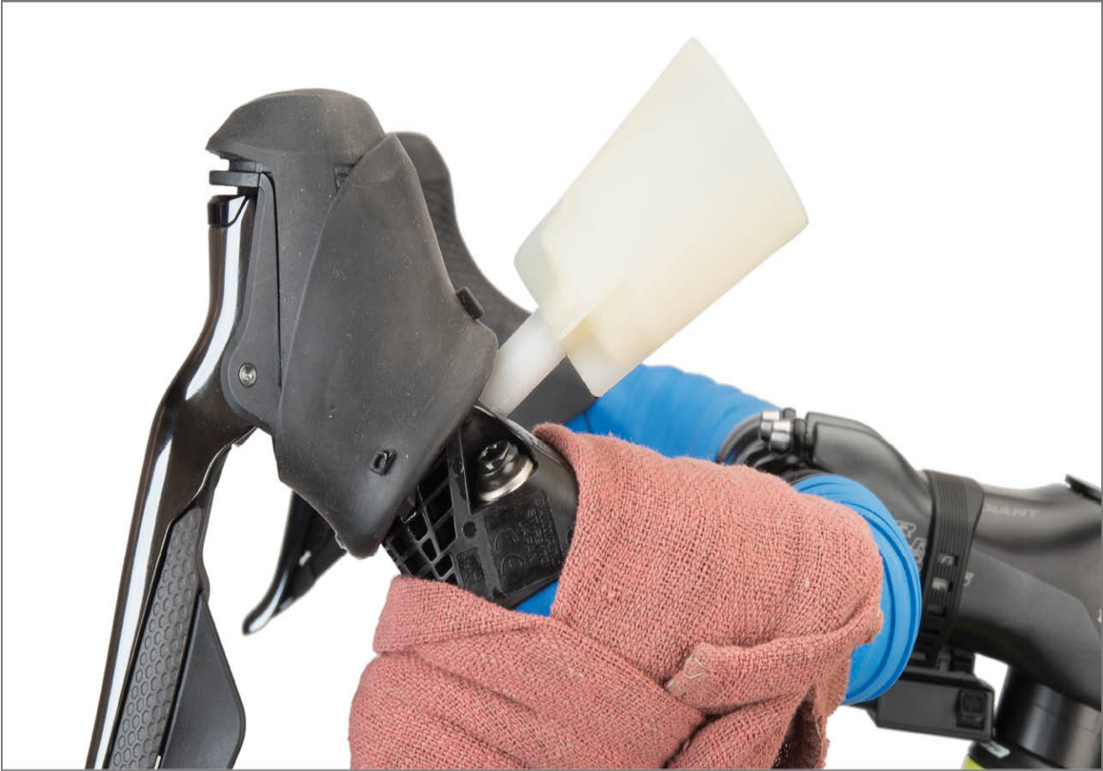
FIGURE 13.31: Rotate so funnel is 45 degrees from vertical
