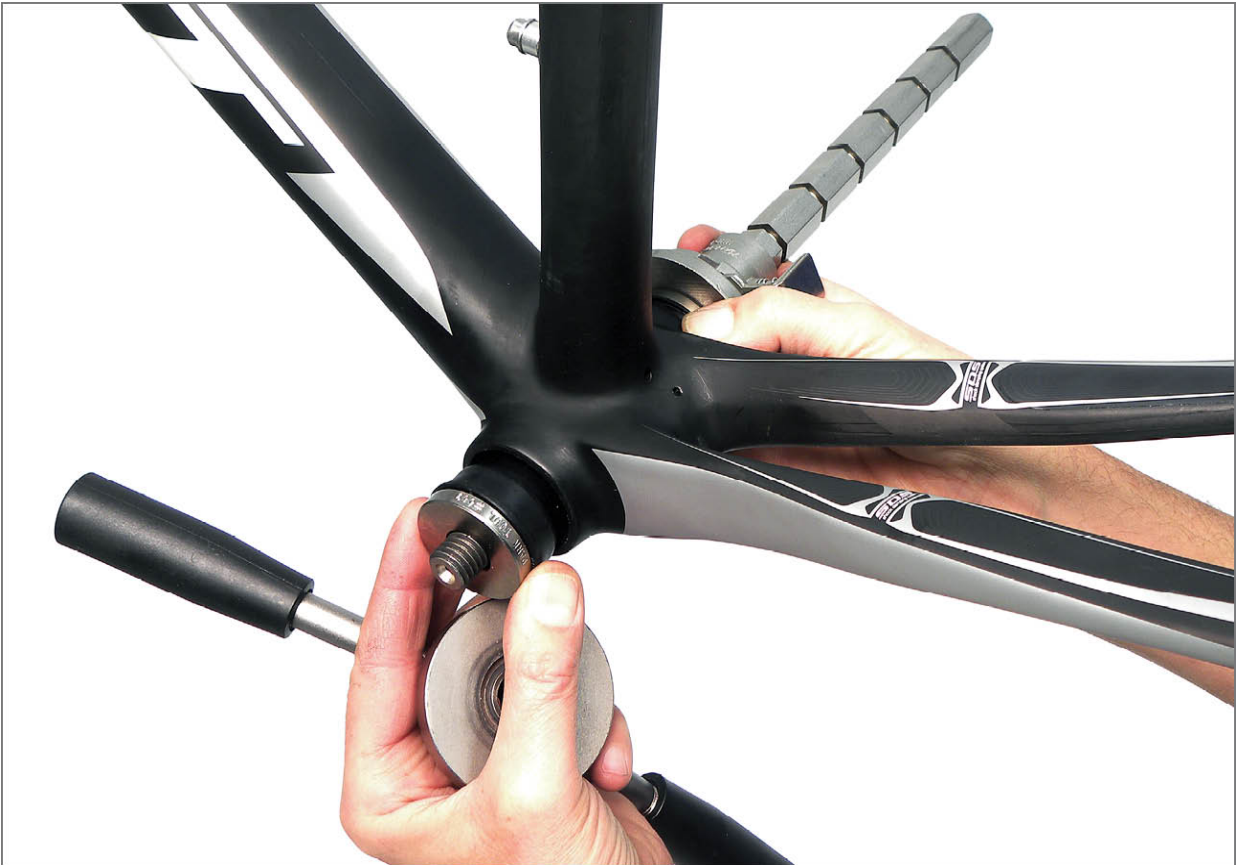
FIGURE 7.43: Install headset press through shell and engage bushings and bearings
