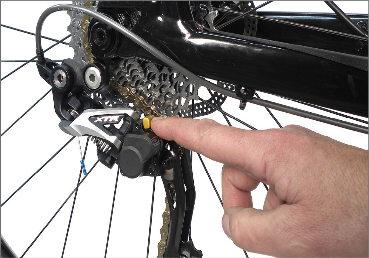
FIGURE 10.66: Push “on-off” lever upward to return derailleur to clutch operation mode
