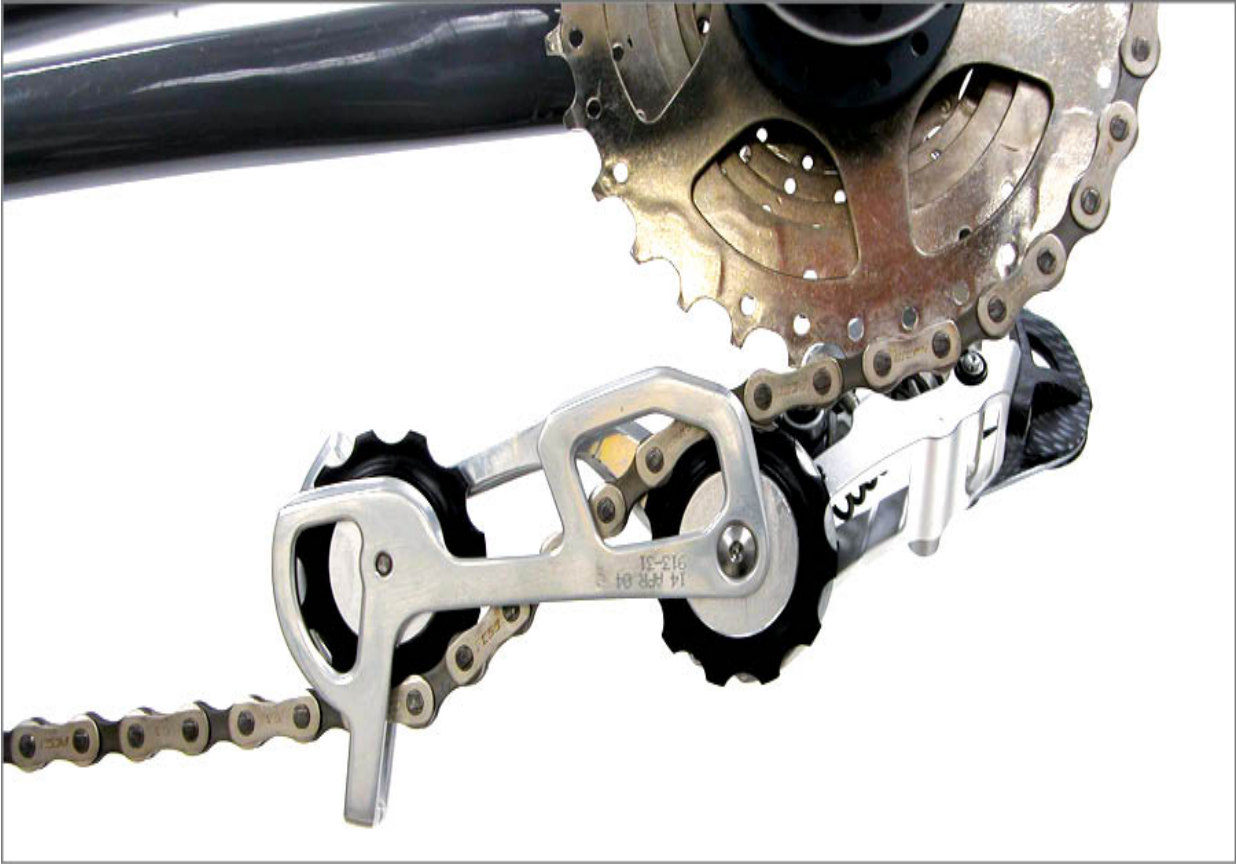
FIGURE 8.4: Double bends at each pulley indicate adequate chain length
