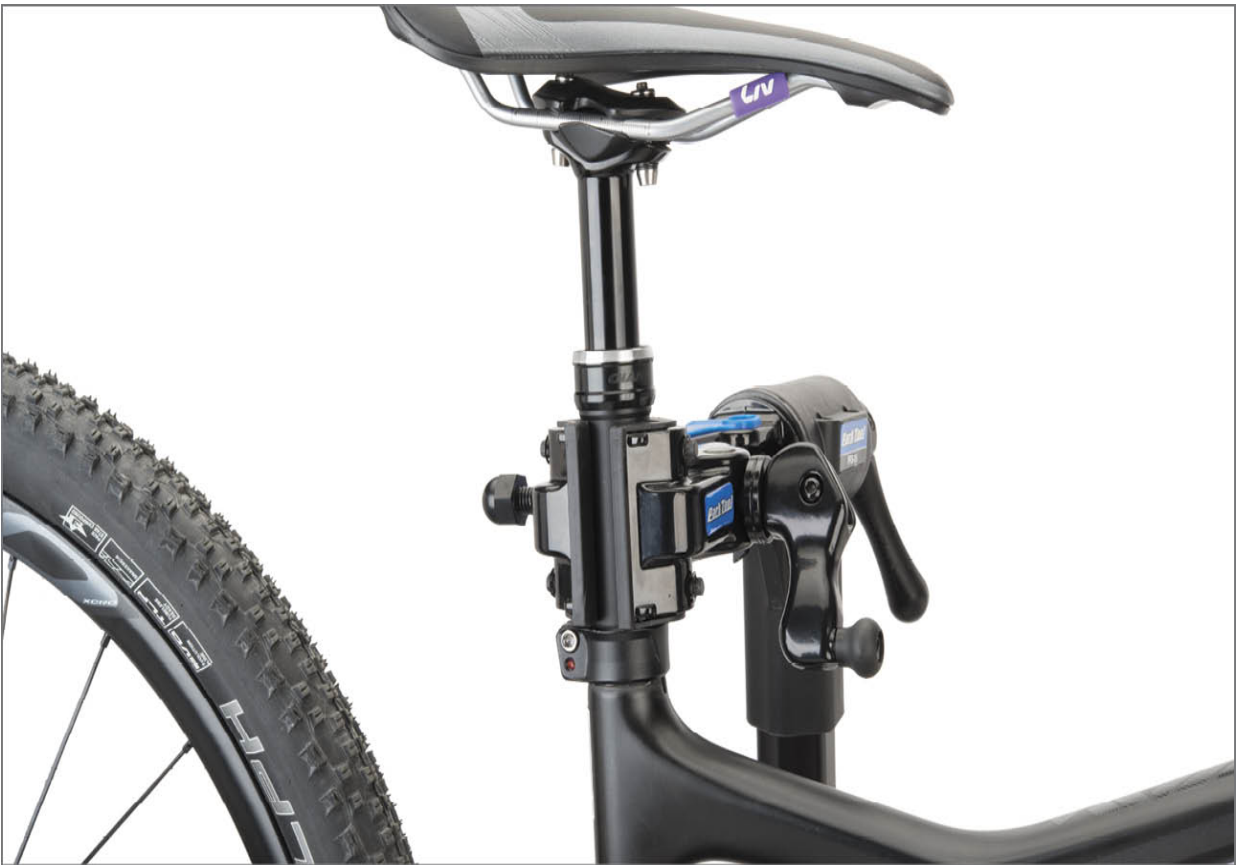
FIGURE 1.11: Clamping the bike by seat post
