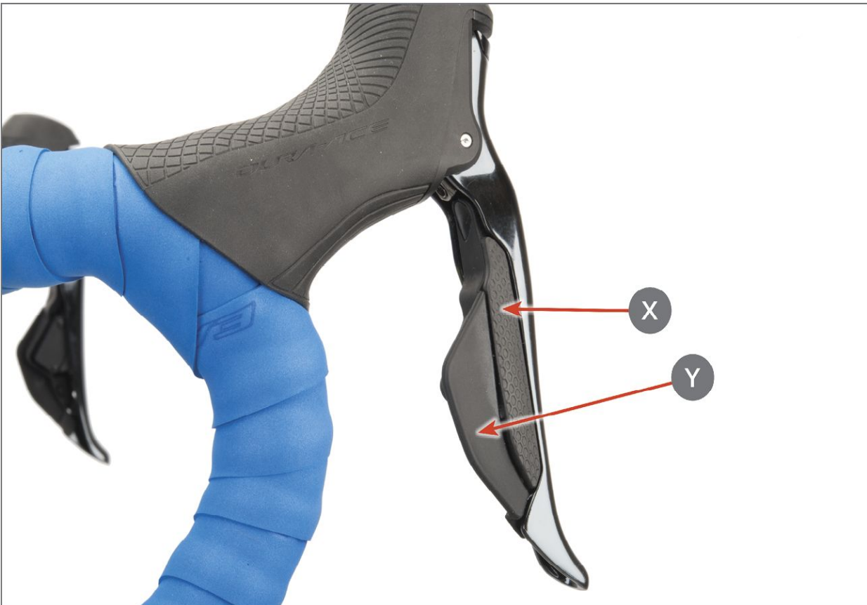
FIGURE 11.1: X and Y switches located on a drop brake lever
