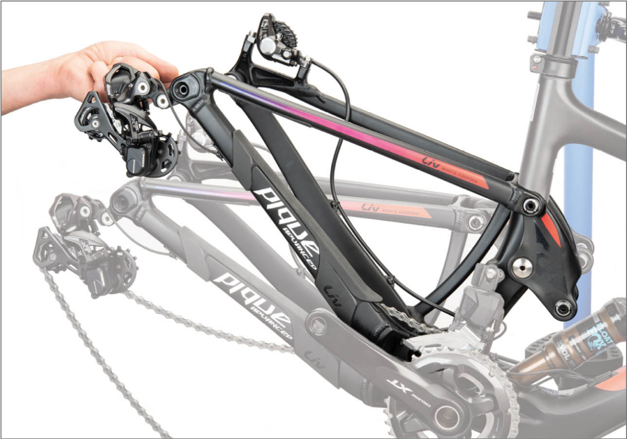
FIGURE 18.4: Unbolt rear shock and feel for easy movement up and down
