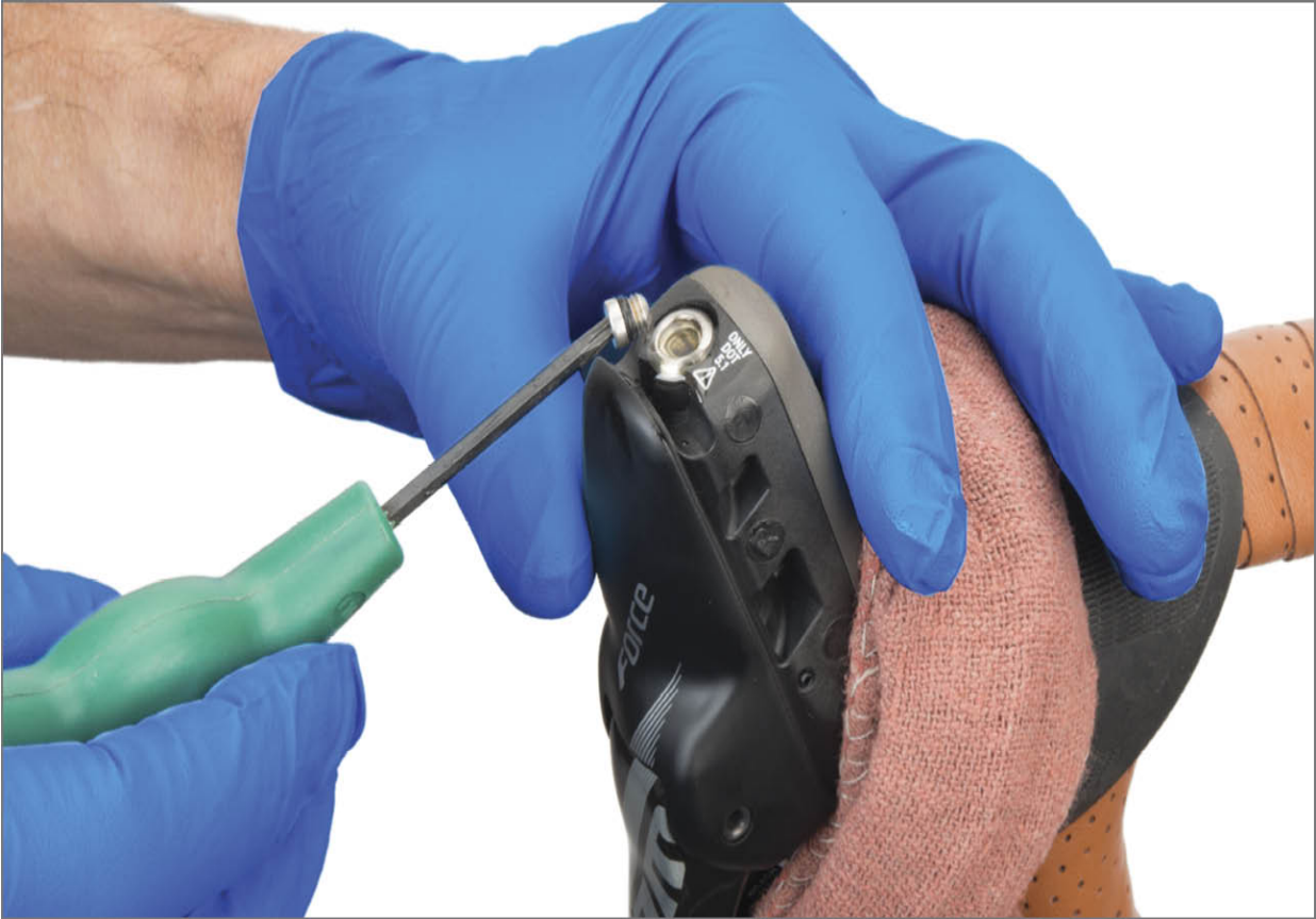
FIGURE 13.48: Open bleed port at brake lever after protecting area with rag
