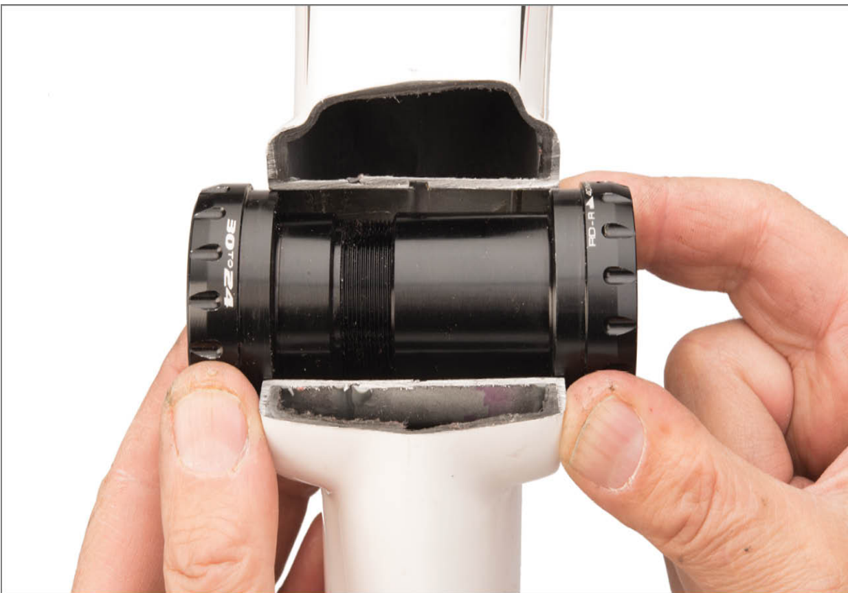
FIGURE 7.46: Cutaway of shell during installation of thread-thru bottom bracket
