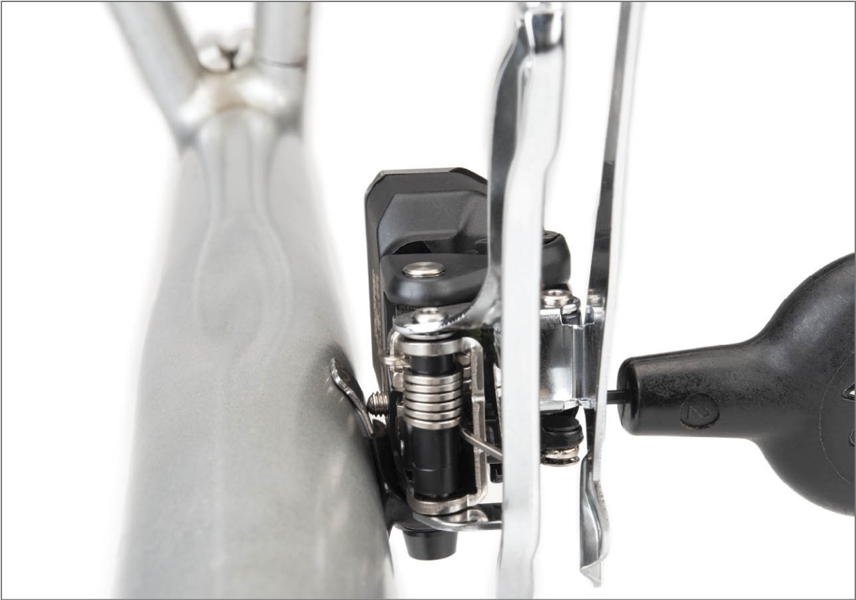
FIGURE 11.10: Support screw location for setting cage angle with braze-on derailleur mount
