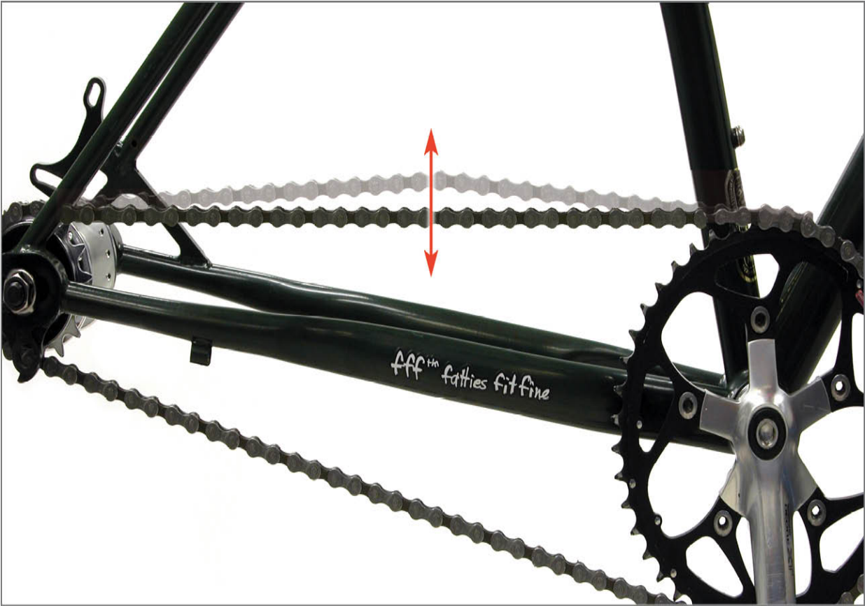
FIGURE 8.30: Pull up and down at middle of chain to test chain tension
