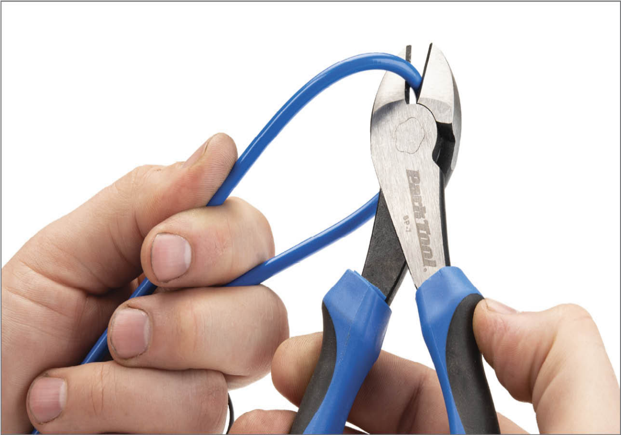
FIGURE 14.11: Flex the wound housing to open coils for side cutters
