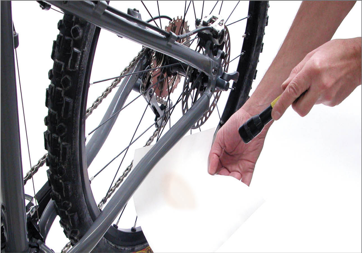
FIGURE 13.21: Use white background to help view caliper alignment to rotor
