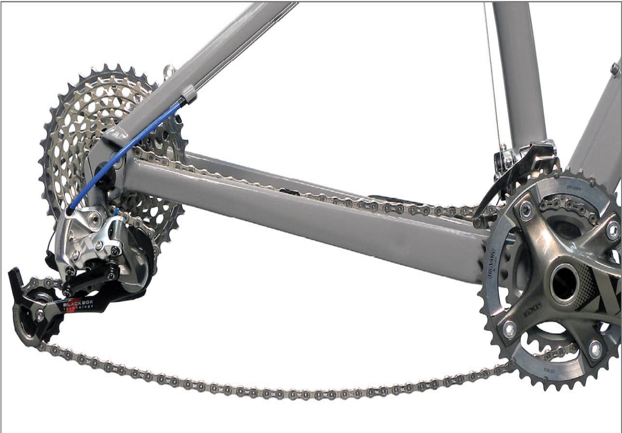
FIGURE 8.2: Chain sag in smallest front to smallest rear sprocket position
