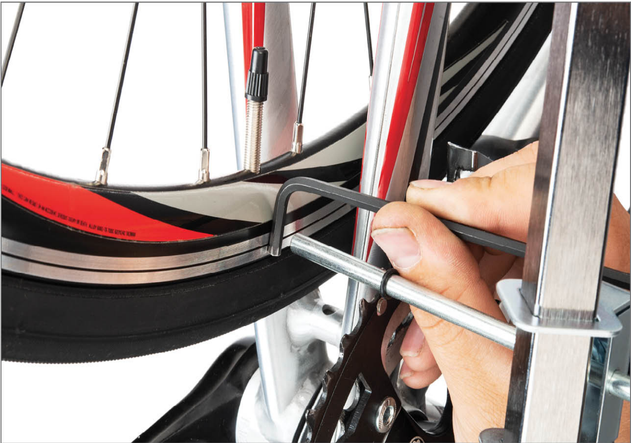
FIGURE 10.71: Gauge indicating misaligned hanger
