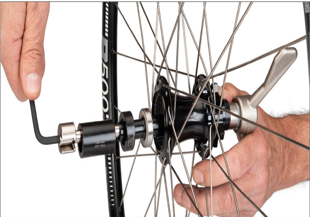
FIGURE 4.29: Installing bearings with bearing press HBP-1
