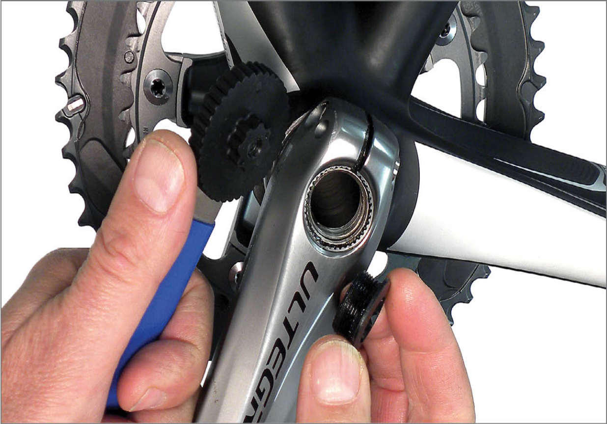
FIGURE 7.13: Remove crank cap after pinch bolts are loose
