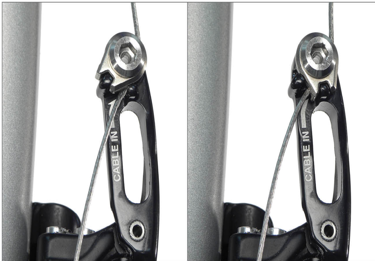
FIGURE 10.54: The two routing options at the notched washer
