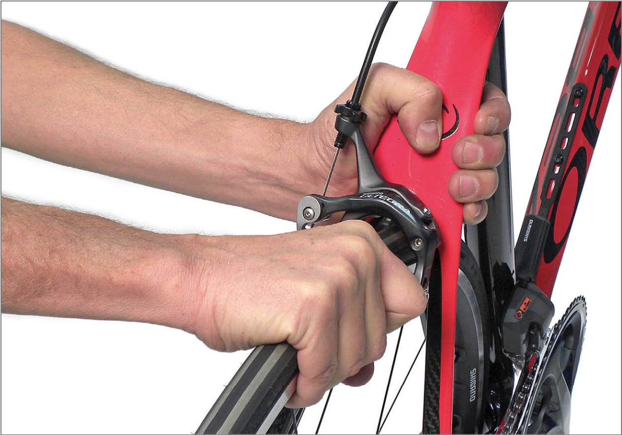
FIGURE 4.14: Grab wheel and pull side-to-side laterally to check for knocking of bearing play
