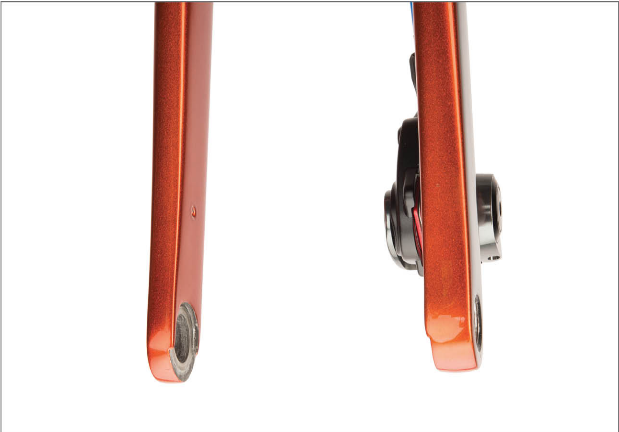
FIGURE 2.11: Enclosed fork ends of a thru axle bike
