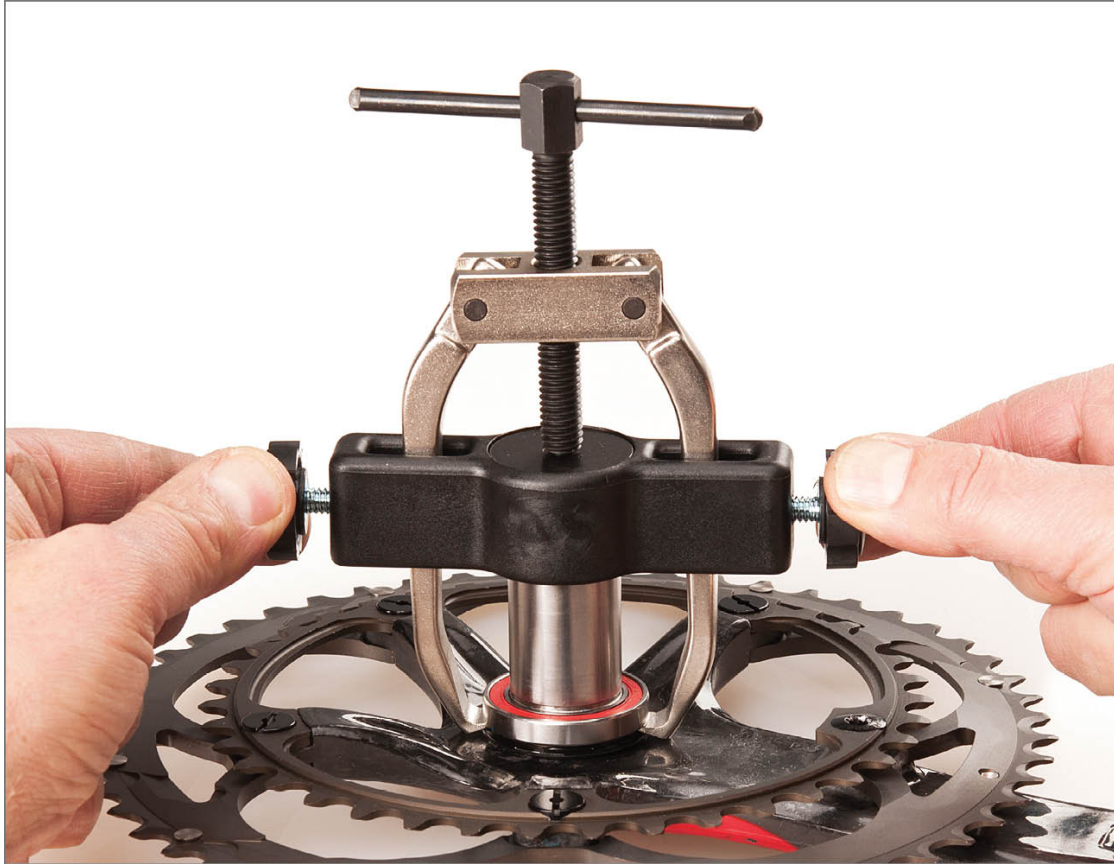
FIGURE 7.49: Engage puller fingers over bearing and secure knobs
