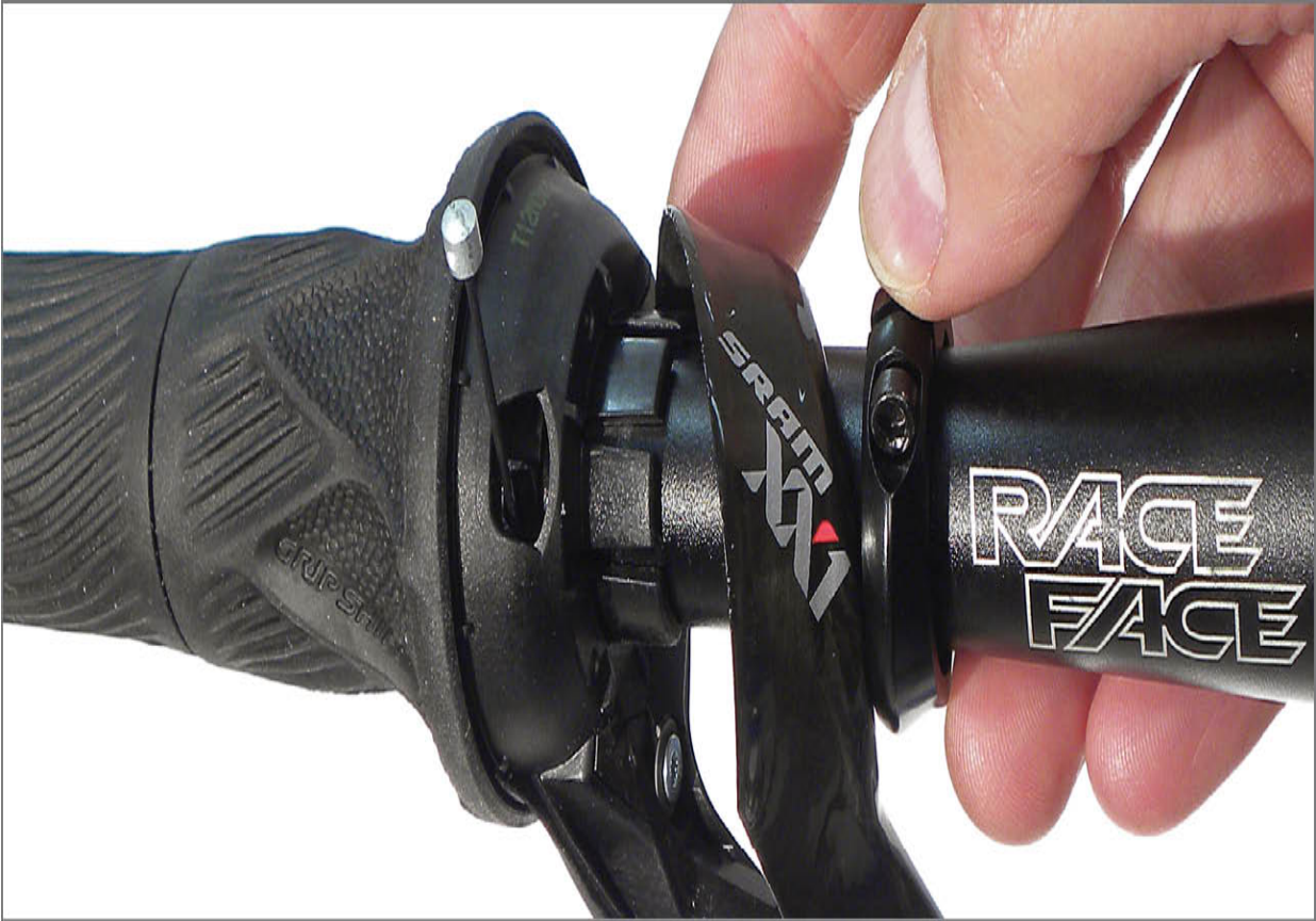
FIGURE 10.19: Remove SRAM® XX1® twist grip retaining ring and shrouding to expose cable end
