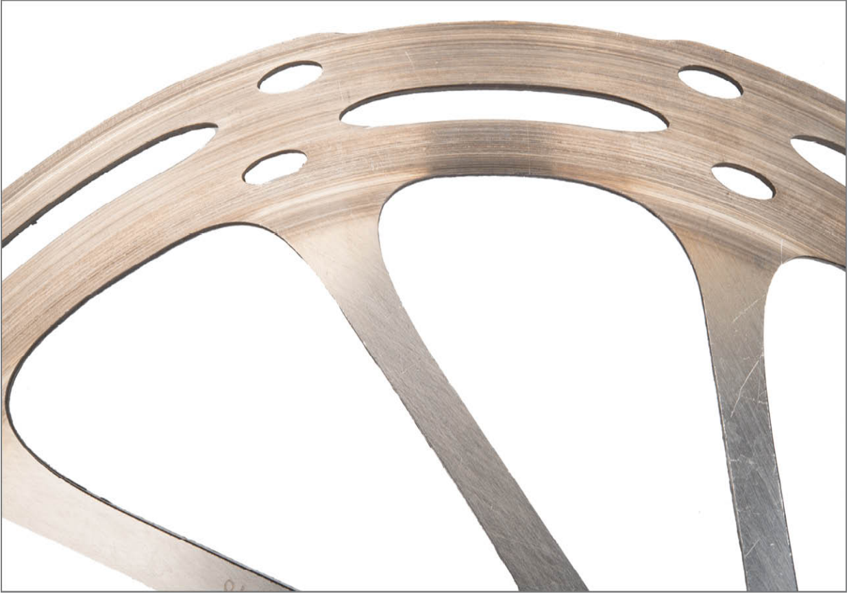
FIGURE 13.18: Typical rotor showing burned in effects
