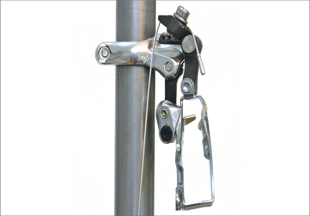
FIGURE 10.34: Bottom swing design with bottom pull cable
