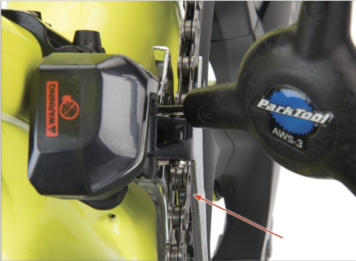
FIGURE 11.11: Slight gap from chain to cage while setting H-limit screw
