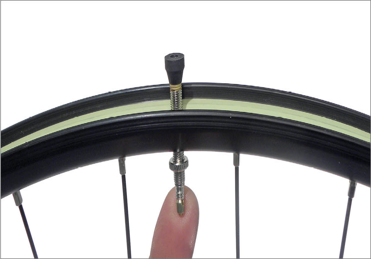
FIGURE 2.59: Secure tubeless valve through rim sealing tape
