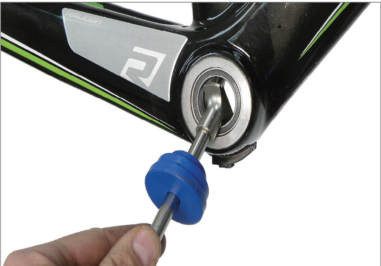
FIGURE 7.36: Engage foot of BBT-30.4 through bearing and push foot to opposite bearing
