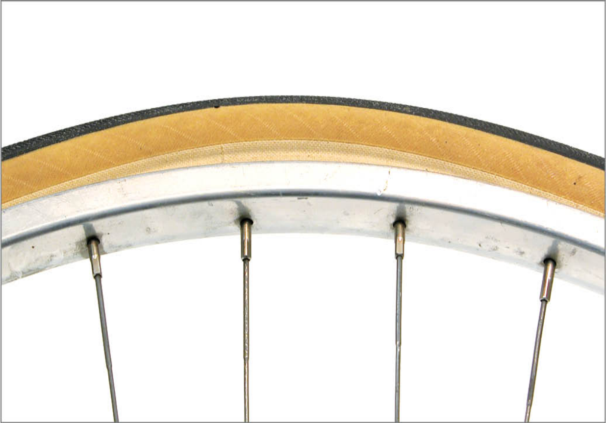
FIGURE 2.51: This bead seat line is bulging upward from improper tire seating. Deflate immediately and reseal tire.
