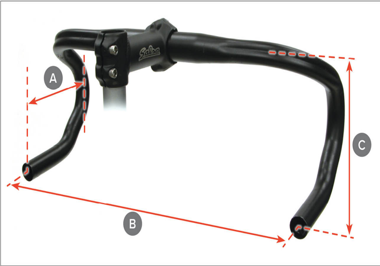
FIGURE 15.6: (A) Drop bar reach, (B) Width, (C) Drop
