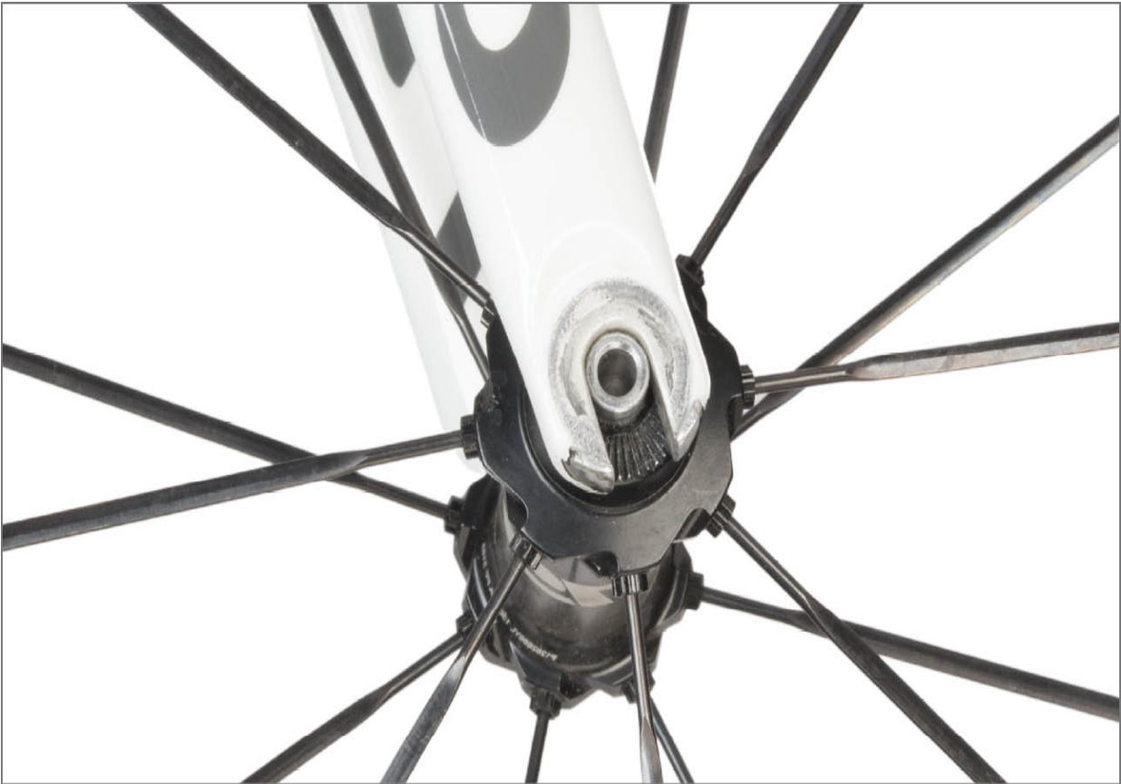
FIGURE 4.1: Open dropout on fork seen without quick-release skewer
