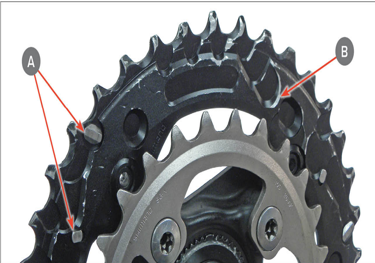
FIGURE 7.71: Note wear marks as the black anodizing wears off during shift (A) Upshift “pick up pegs” to lift chain to large ring, (B) Down shift ramps
