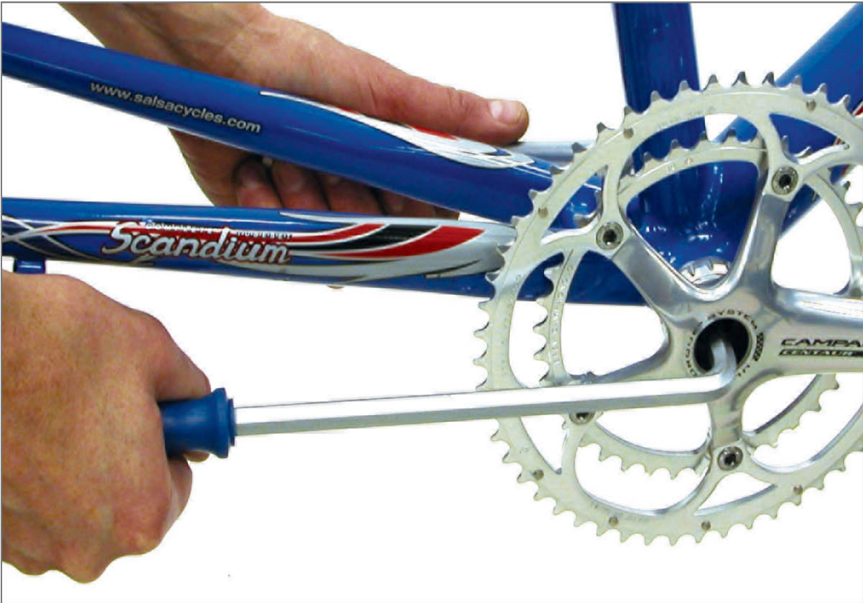
FIGURE 7.22: Remove crank bolt with 10mm hex key
