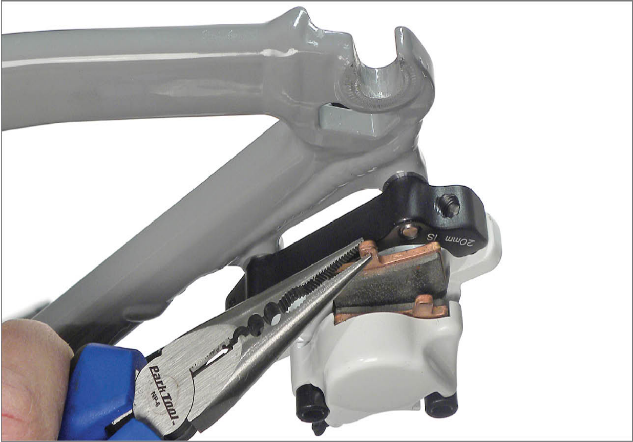
FIGURE 13.11: Use pliers to remove Hayes® pads with spring clip
