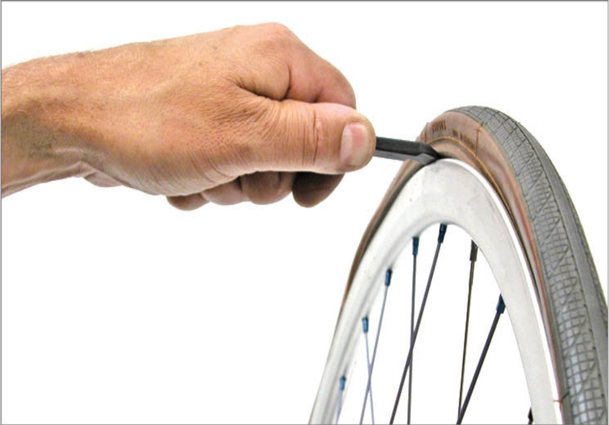
FIGURE 2.50: Use levers if necessary to lift bead over edge of rim
