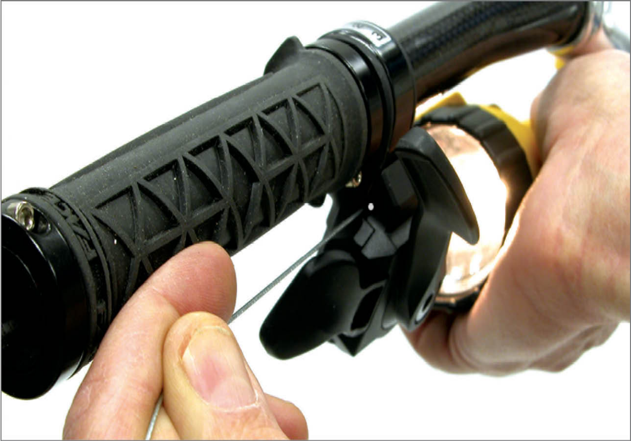
FIGURE 10.14: Use flashlight to help find route for cable end
