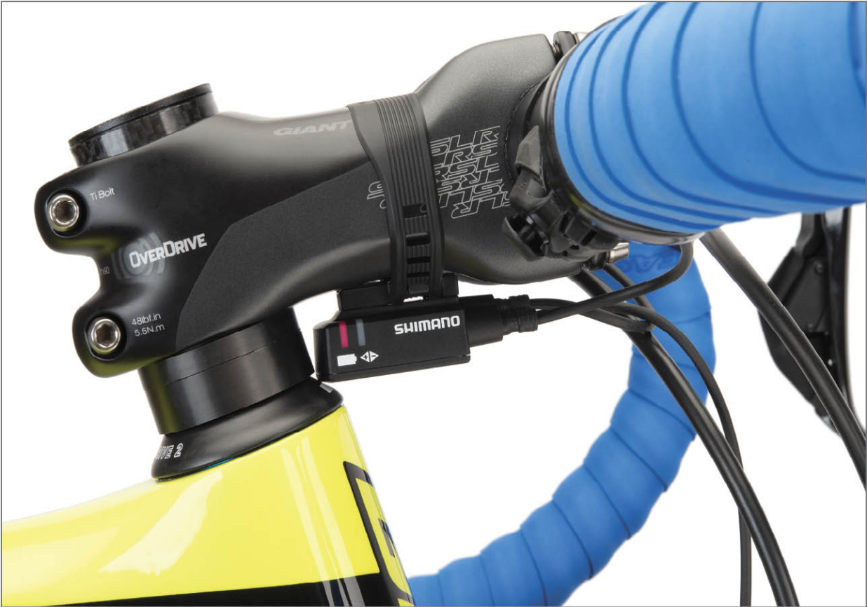
FIGURE 11.3: Front junction box secured below stem
