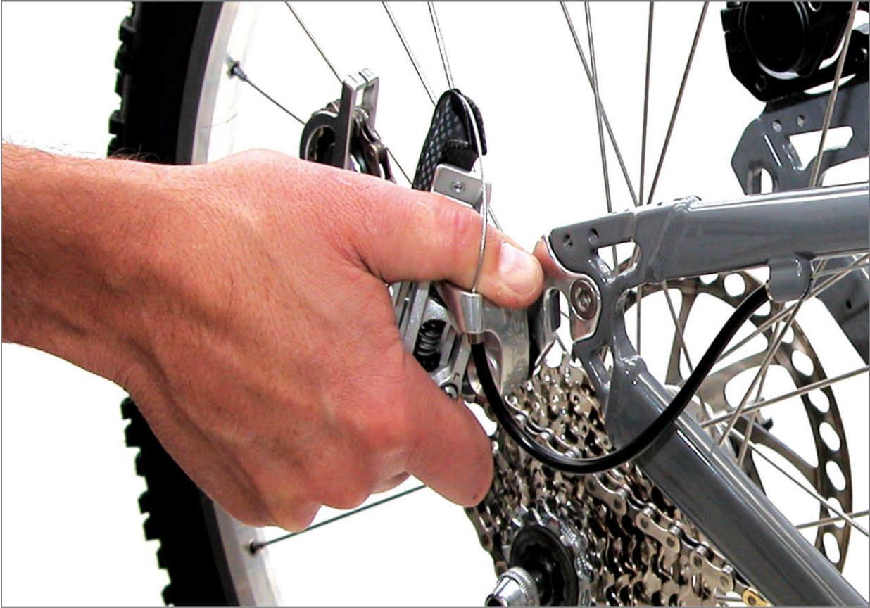
FIGURE 2.7: Pivot rear derailleur back to clear wheel and cogs of frame
