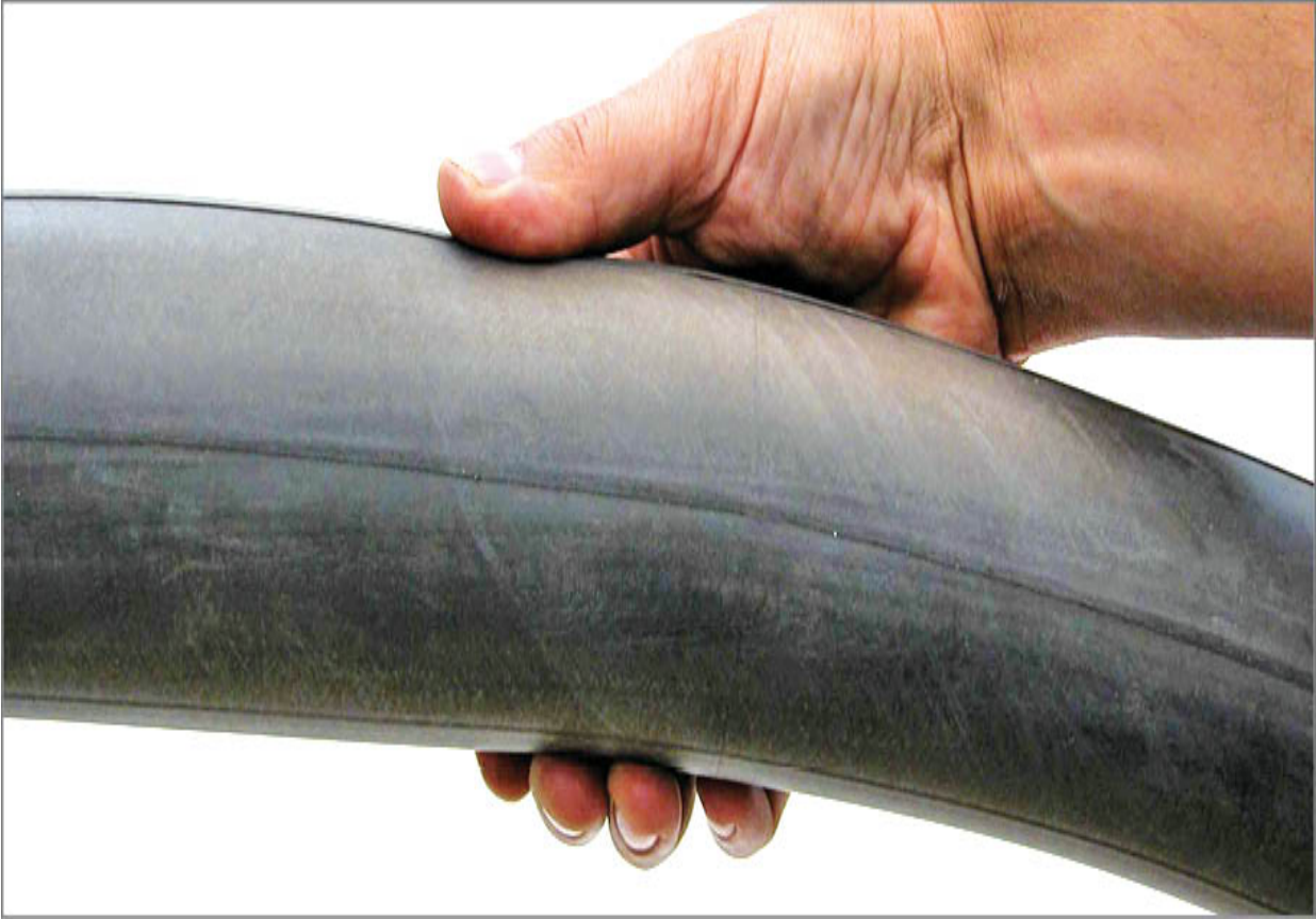
FIGURE 2.20: Inner tube inflated for inspection of small holes
