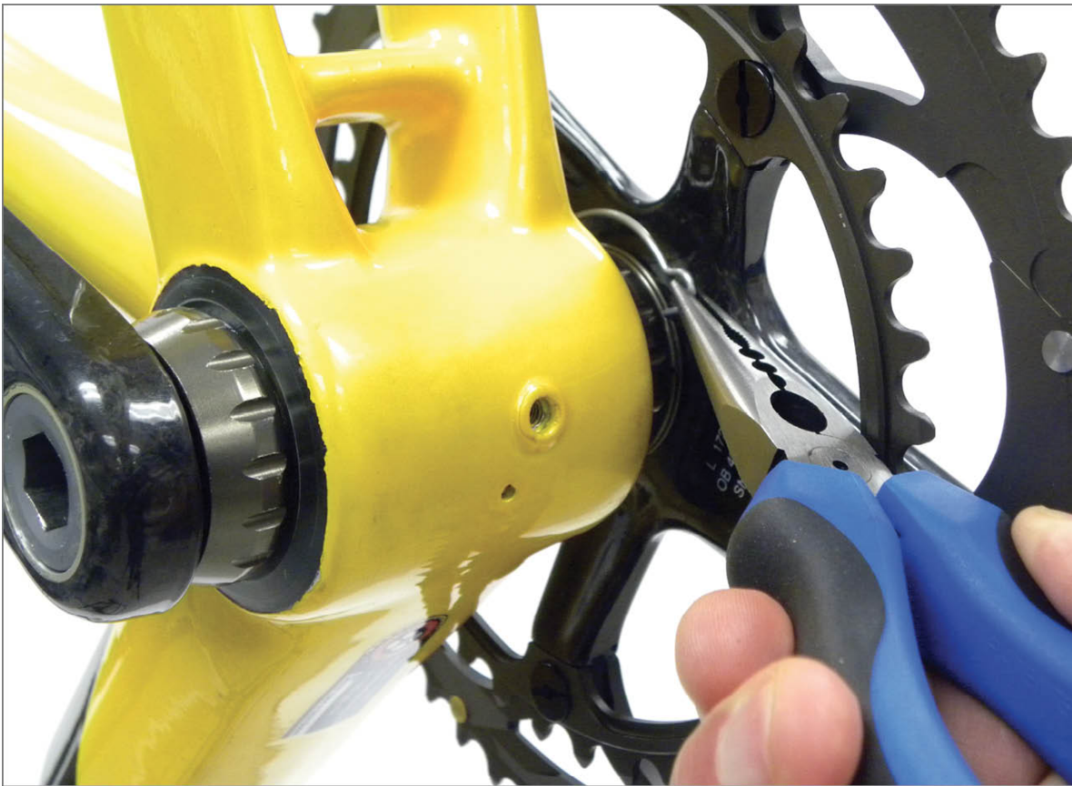
FIGURE 7.24: Remove clip from drive-side adaptor
