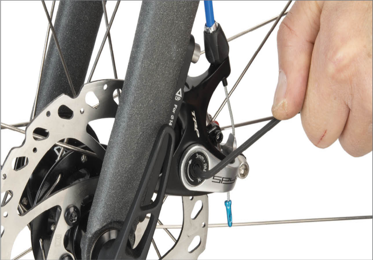
FIGURE 13.68: Adjust both pads evenly until pressing against rotor
