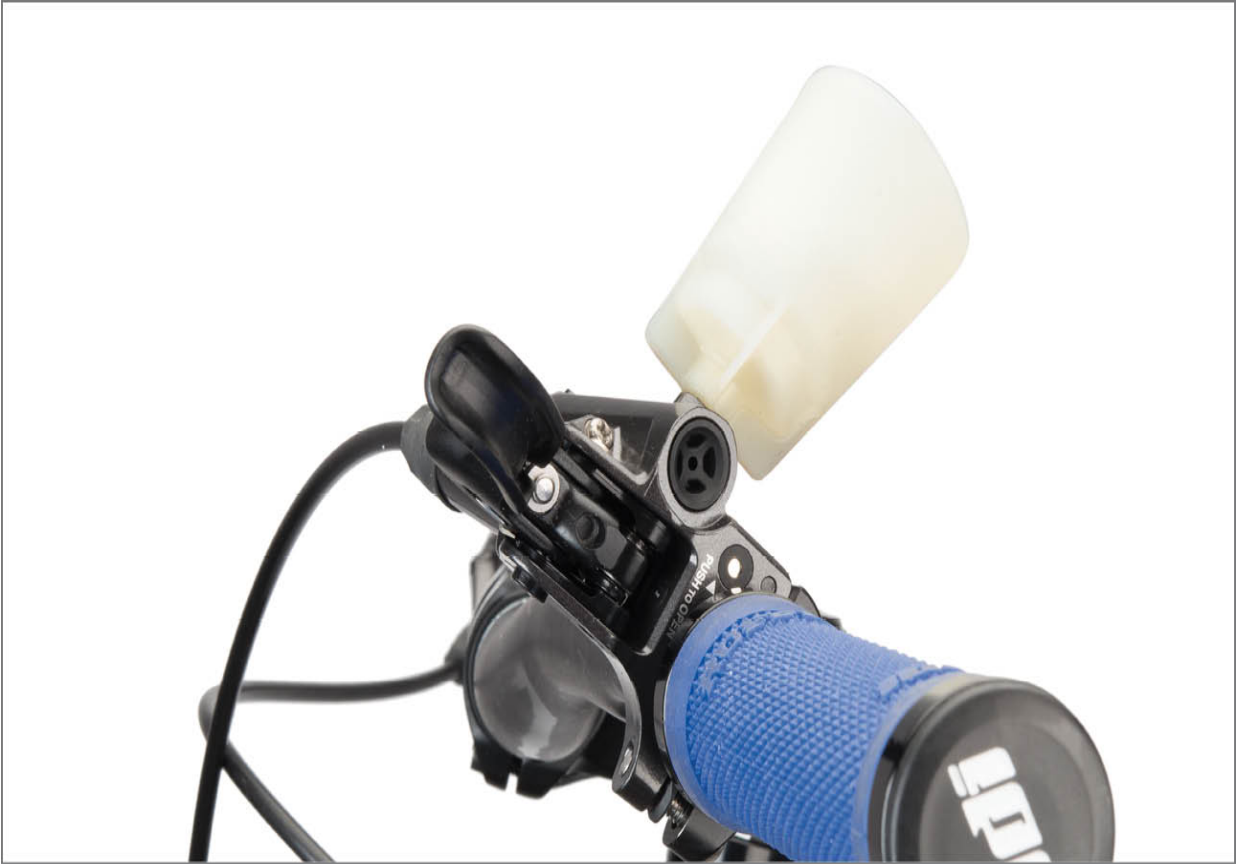
FIGURE 13.30: Rotate brake lever so funnel is 45 degrees from vertical
