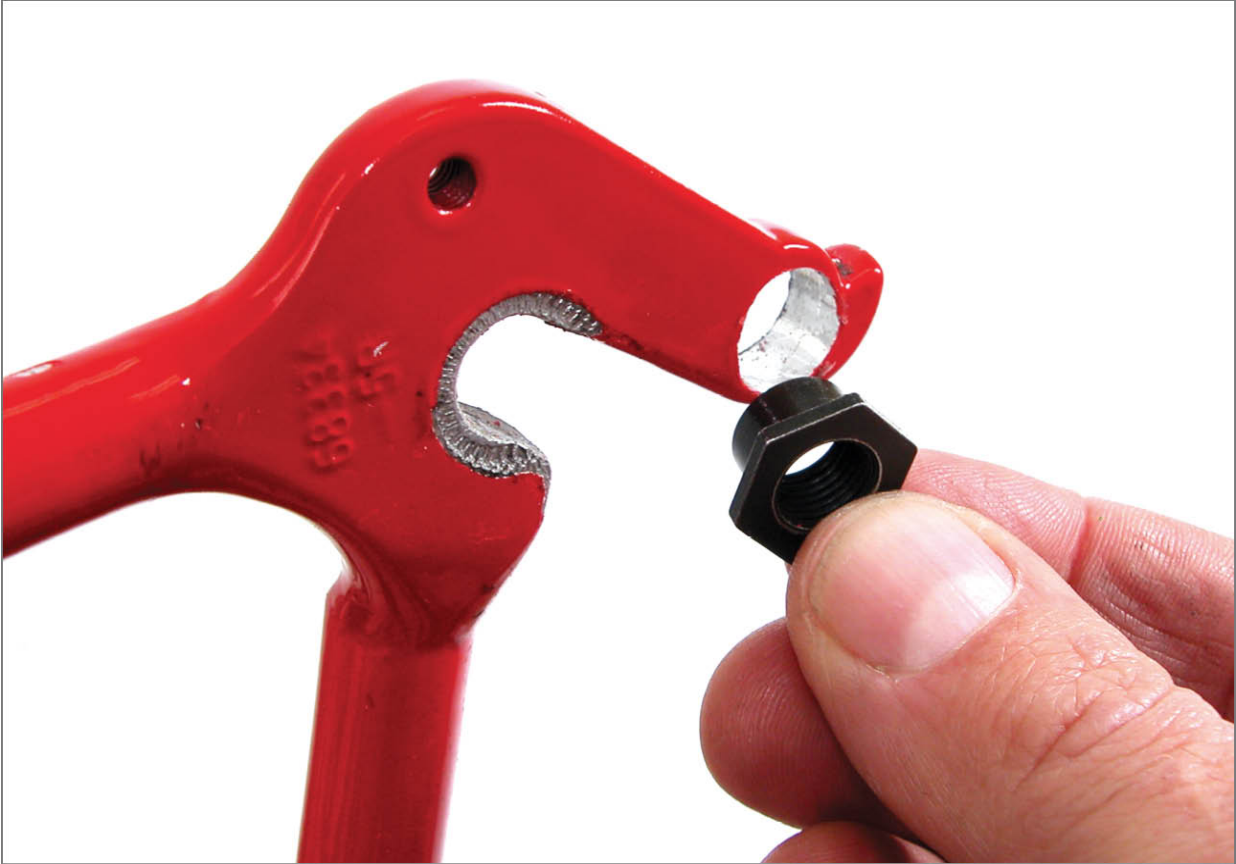
FIGURE 10.76: T-nut thread repair of a stripped hanger
