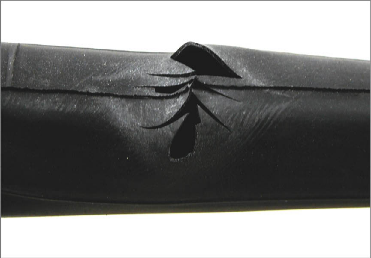
FIGURE 2.23: Shredded holes indicate blow out
