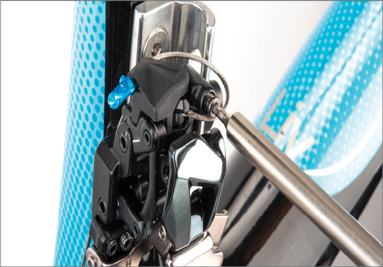
FIGURE 10.53: Turn adjustment screw to rotate the cable pinch bolt system and control cable slack
