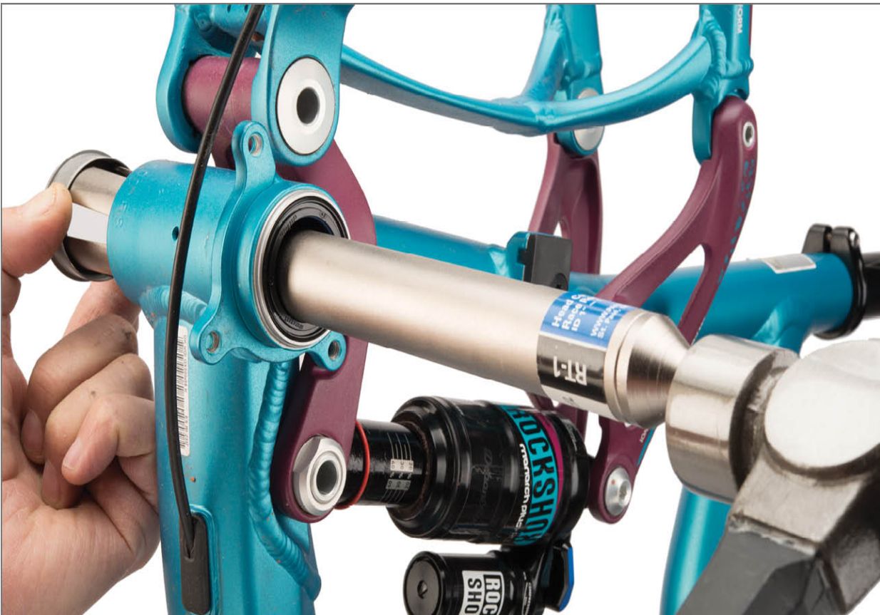
FIGURE 7.38: Strike RT-1 to drive press fit SRAM® DUB™ adaptor from shell
