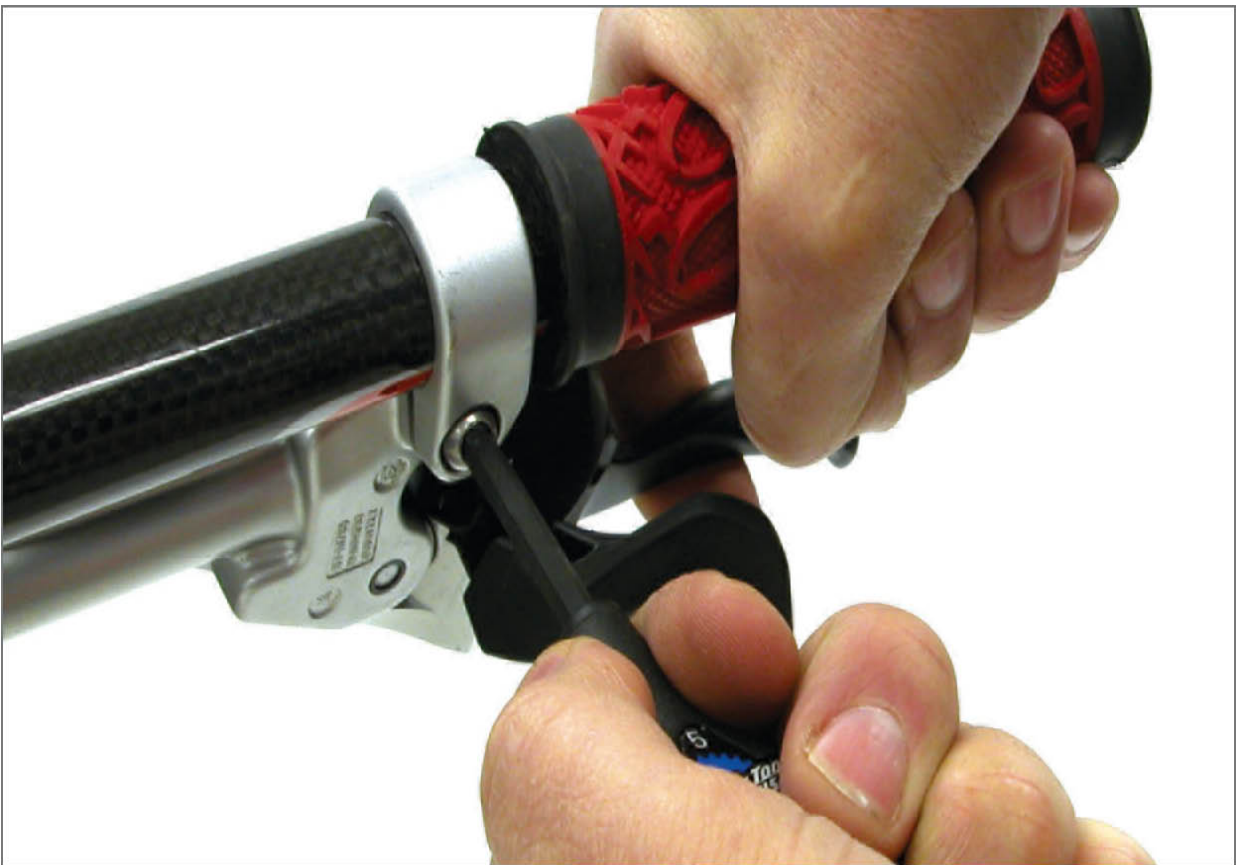
FIGURE 14.1: Rotate levers for comfortable reach
