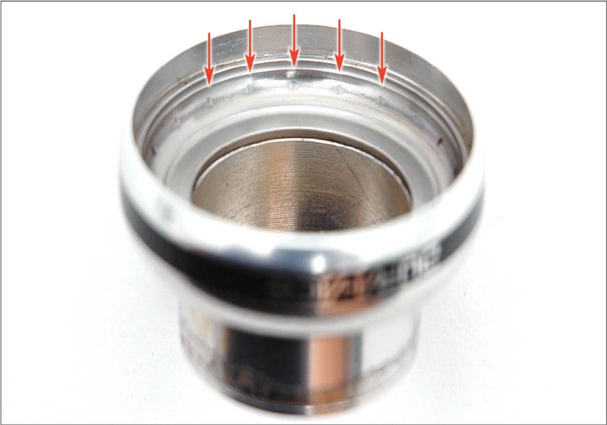
FIGURE 16.8: Pits and dents indicating a worn headset cup
