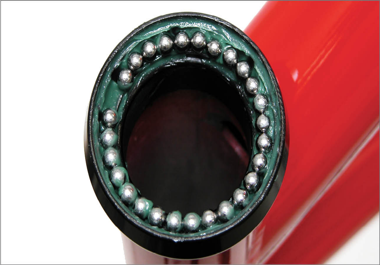
FIGURE 16.15: Loose ball bearings in the headset cup with gap so bearings can move freely
