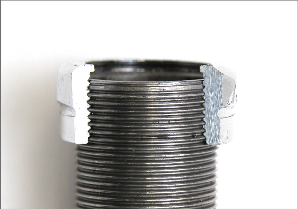
FIGURE 16.36: Cutaway of locknut on threaded column. Locknut lip should not contact top of column.
