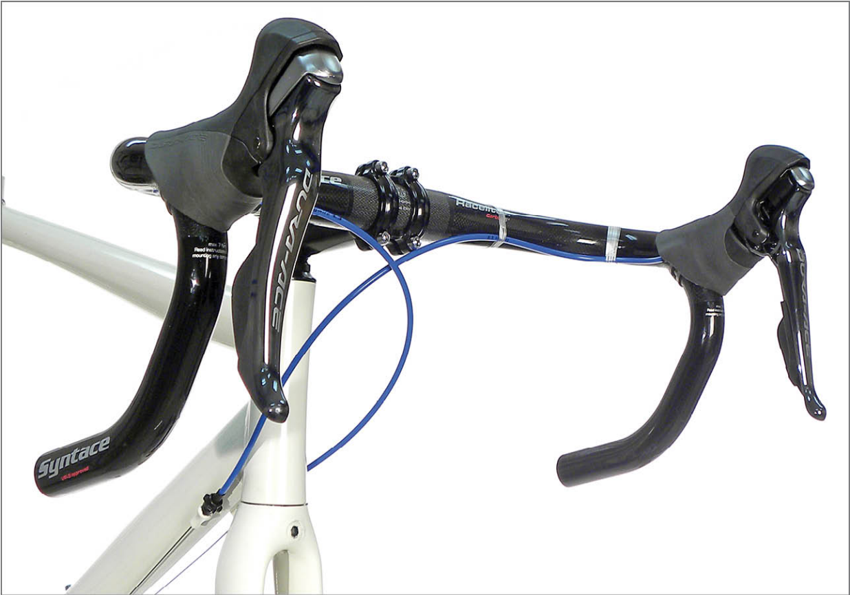
FIGURE 10.10: Shift housing routed to cross over from levers to housing stops. Notice cable must again cross back under down tube.
