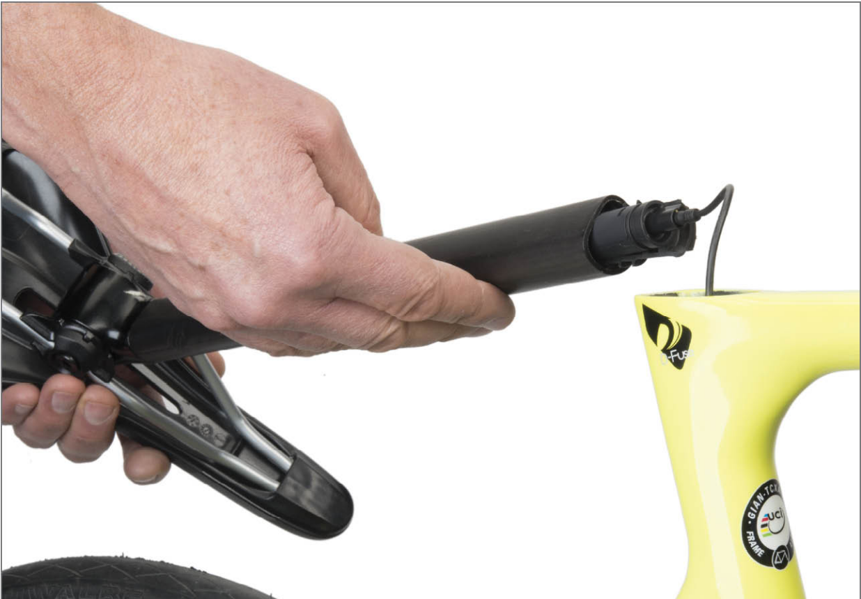
FIGURE 11.7: Internal battery installed inside seat post
