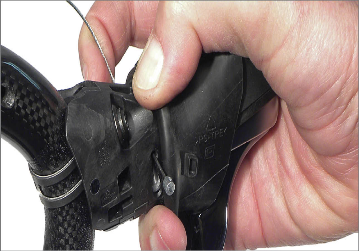
FIGURE 10.25: Install cable from inside face of lever and up through the top of lever body
