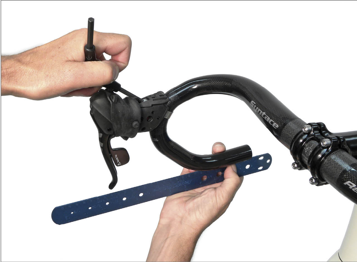
FIGURE 14.3: Adjust lever height along hook of drop bar
