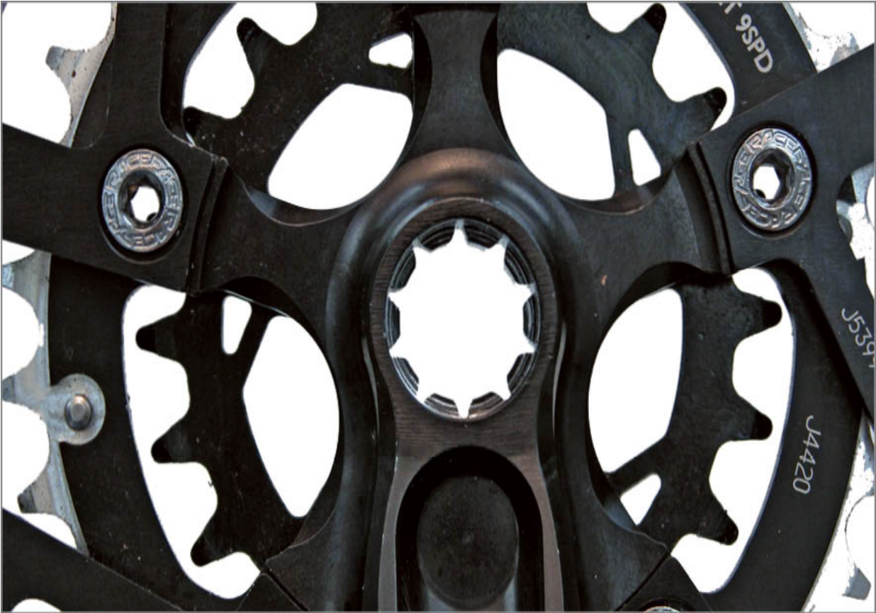
FIGURE 7.4: ISIS Drive crank with 10 splines
