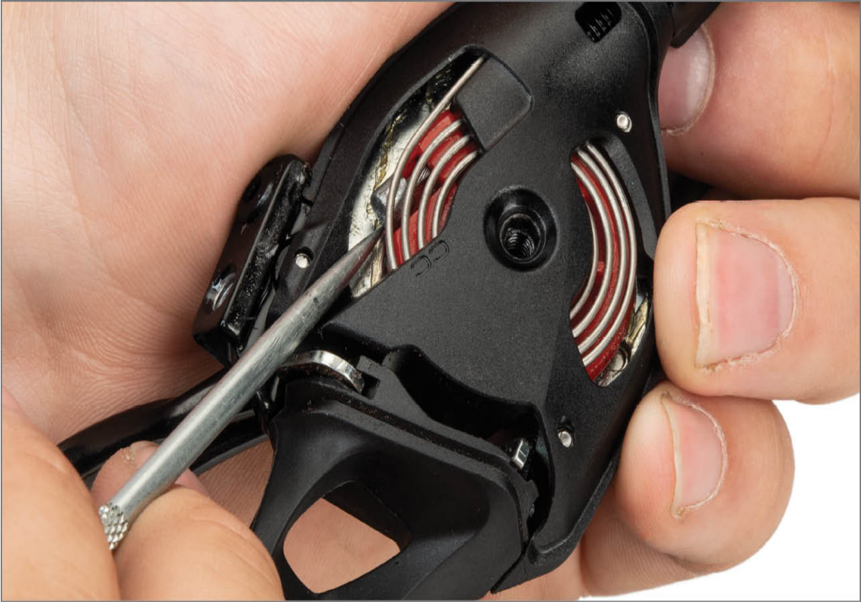
FIGURE 10.16: Carefully lift cable head from socket
