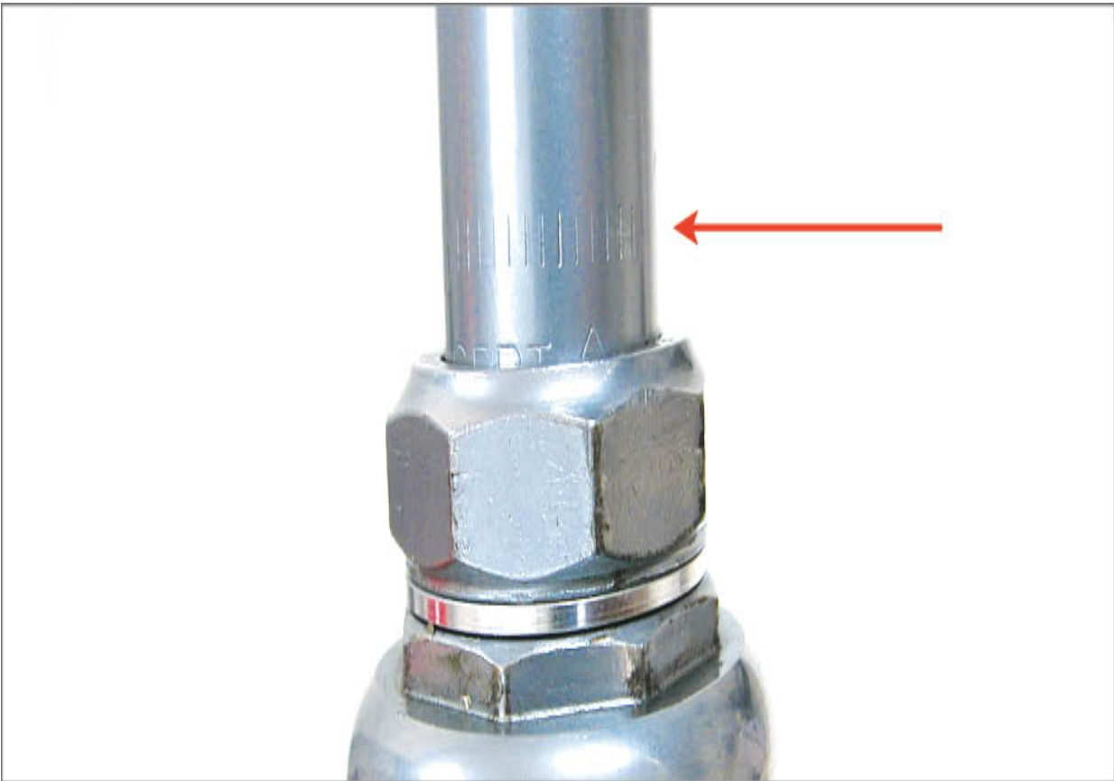
FIGURE 15.13: Example of stem set too high. "Max height" line must not be visible
