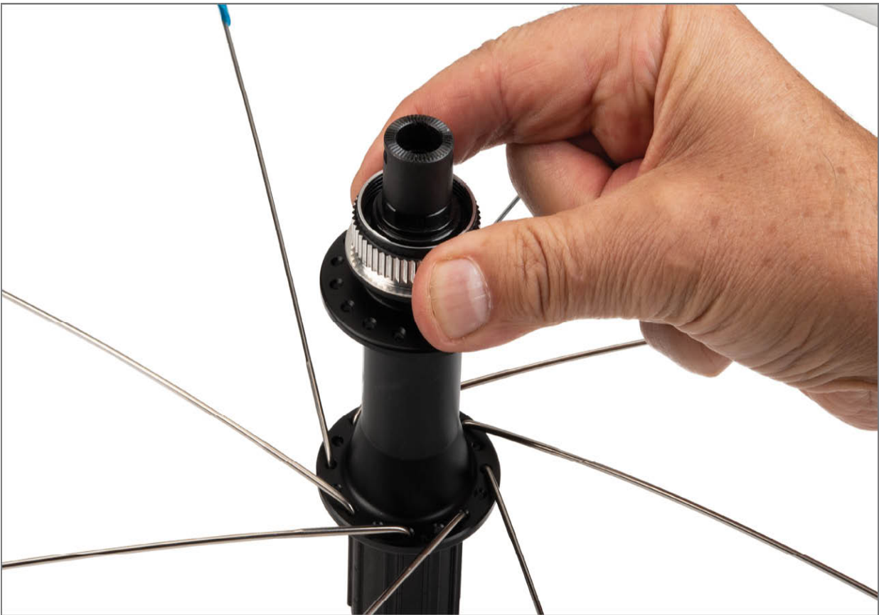
FIGURE 6.16: Rotate hub to determine direction of first spoke set while viewing valve hole
