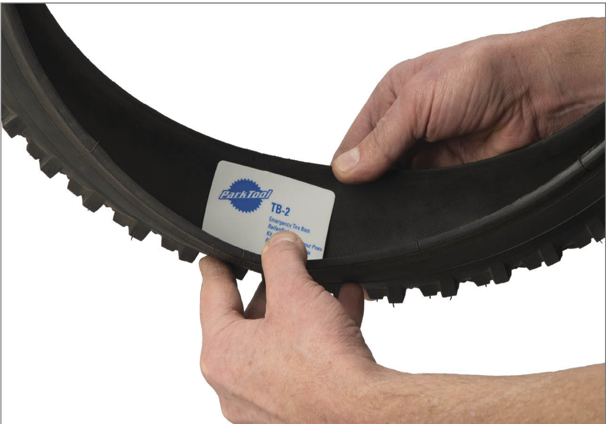
FIGURE 2.38: Place TB-2 Emergency Tire Boot over the cut in tire and replace tire as soon as possible
