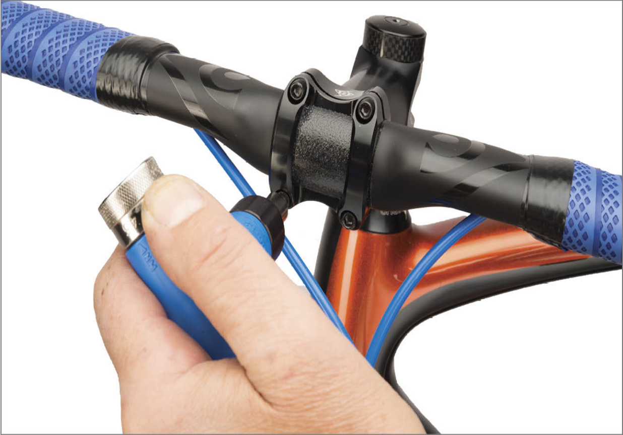
FIGURE 1.4: Using a torque limiter tool to secure handlebar binder
