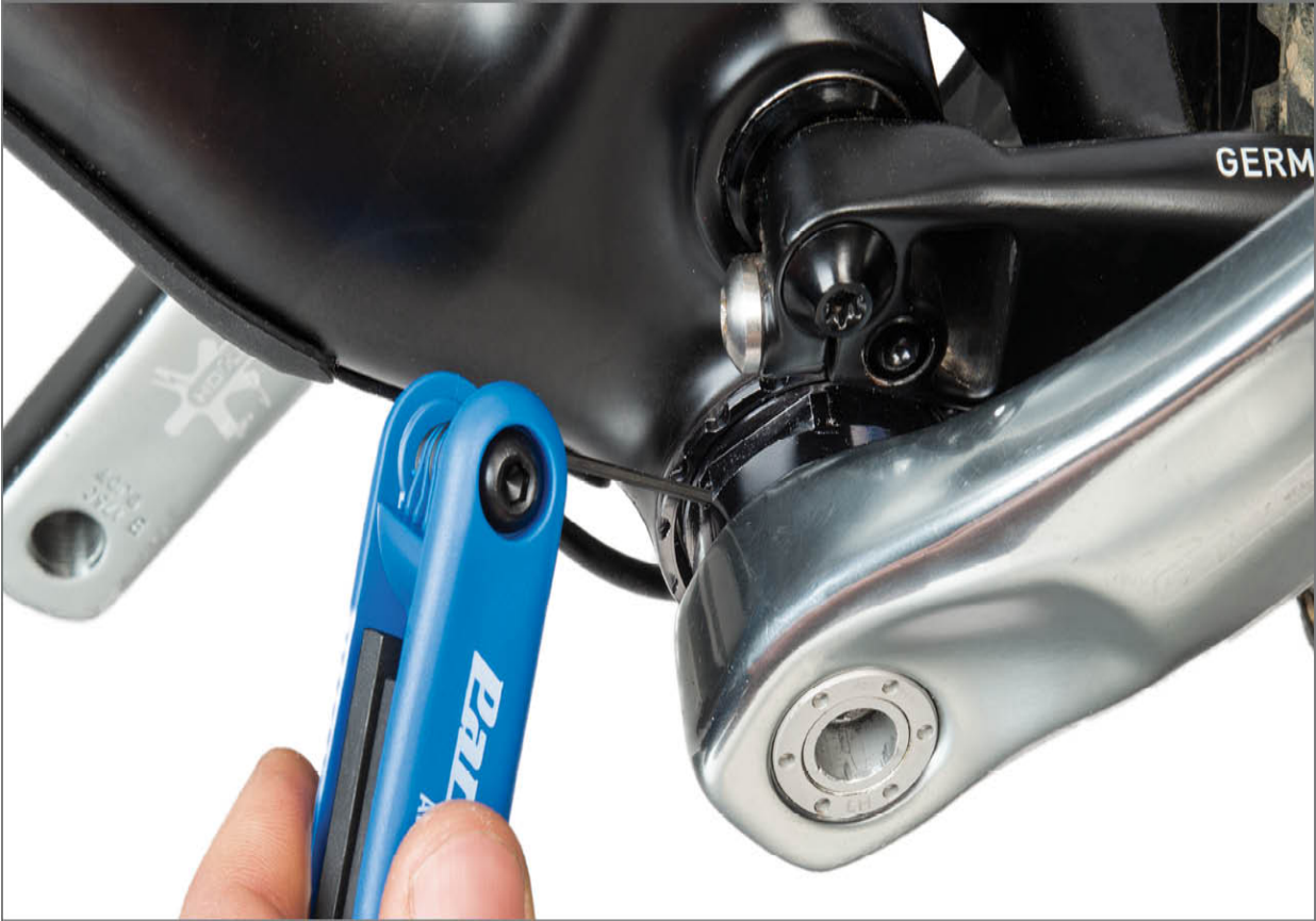
FIGURE 7.20: Tighten set screw to prevent adjusting ring movement
