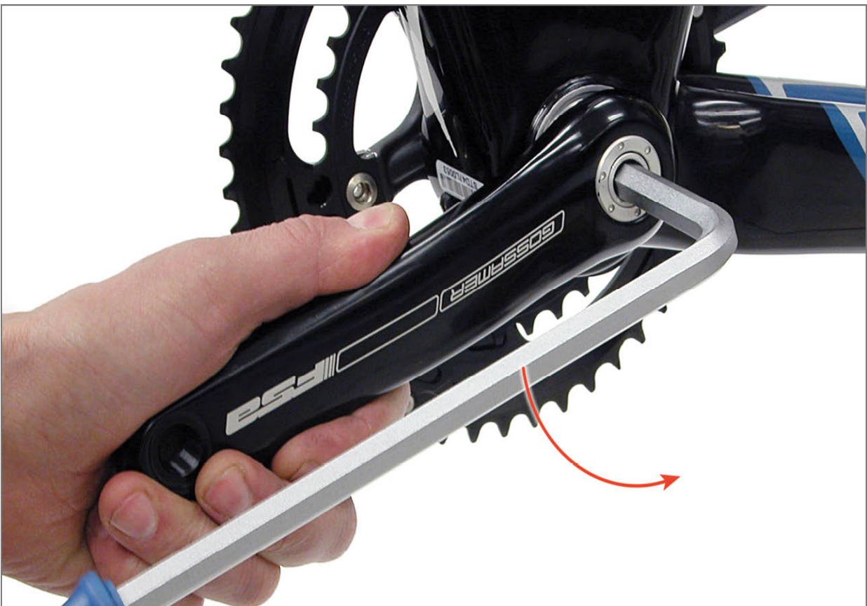
FIGURE 7.7: Self-extracting crank with hex wrench in place for crank removal
