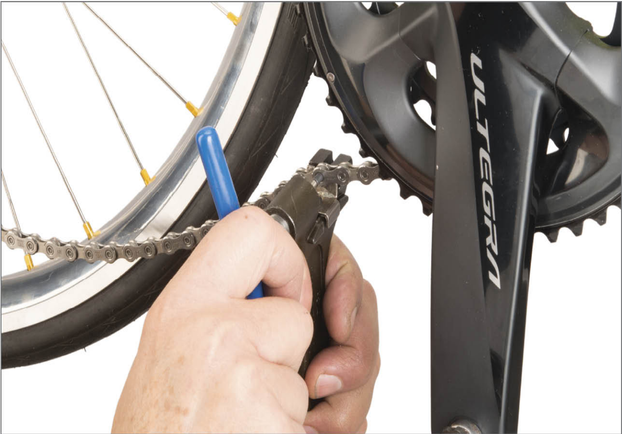
FIGURE 8.12: Push connection rivet toward the inside
