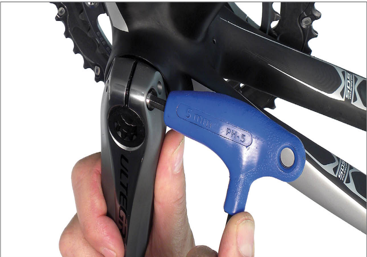
FIGURE 7.12: Loosen both pinch bolts of compression slotted cranks
