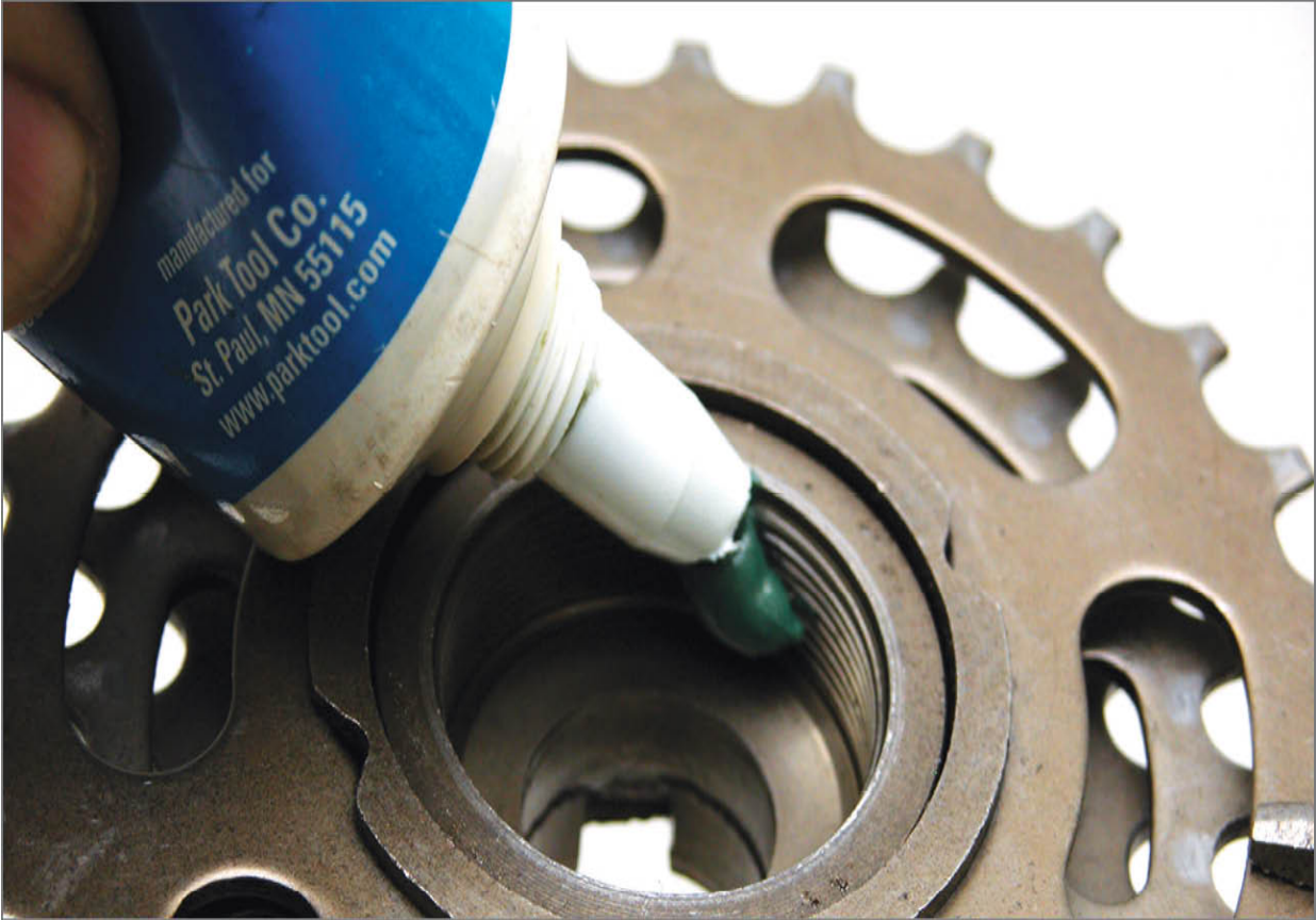
FIGURE 3.11: Heavily grease threads of freewheel
