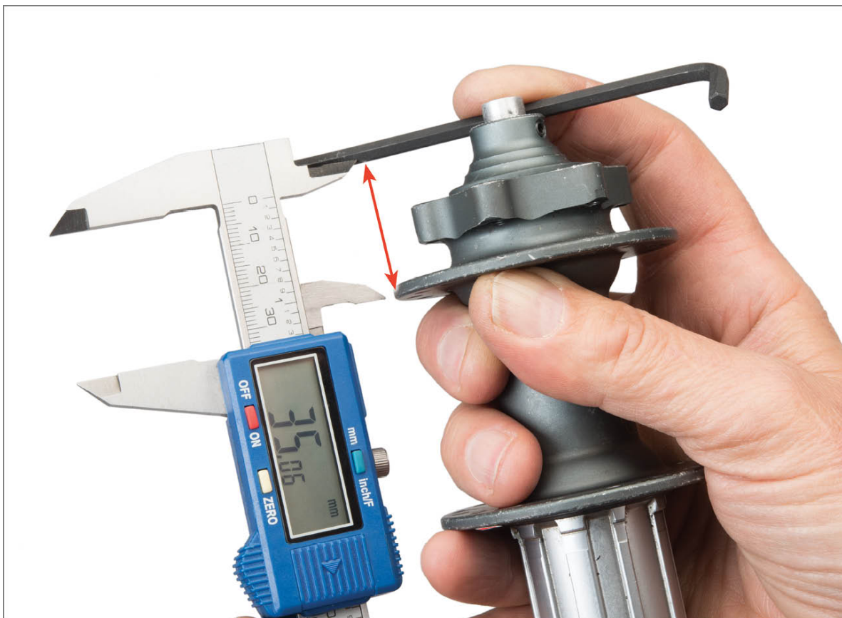
FIGURE 6.6: Extending hub contact face to measure distance to flange
