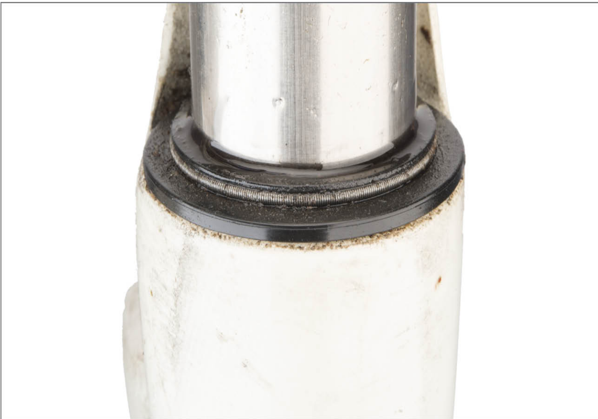
FIGURE 18.3: Suspicious fluid weepage indicating possible seal failure
