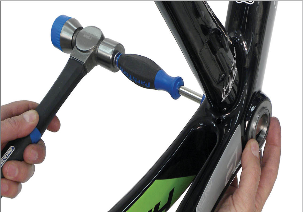
FIGURE 7.37: Strike tool end to drive out bearing from shell
