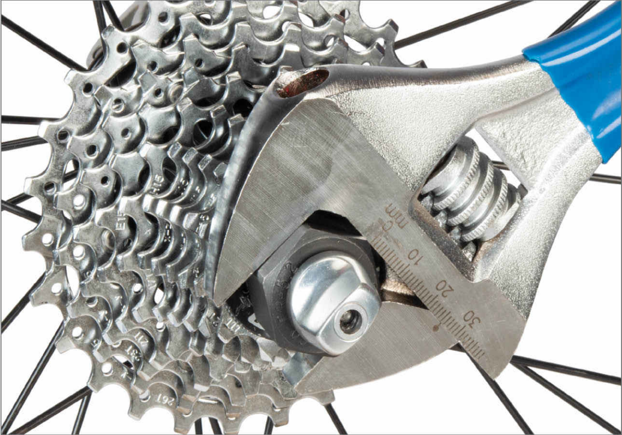
FIGURE 3.4: Use skewer and nut to hold tool firmly in place
