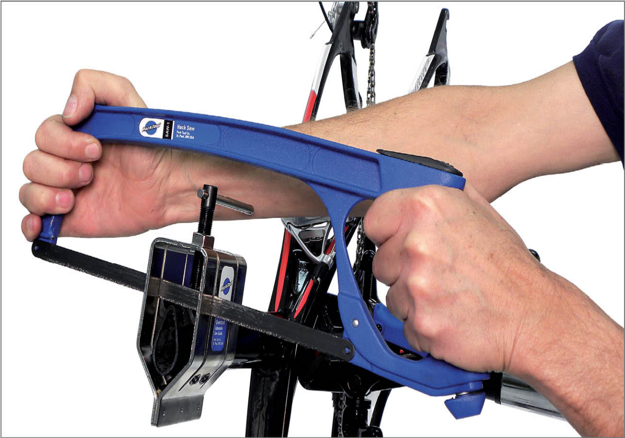
FIGURE 15.27: Trim integrated seat tubes using SG-7.2 saw guide
