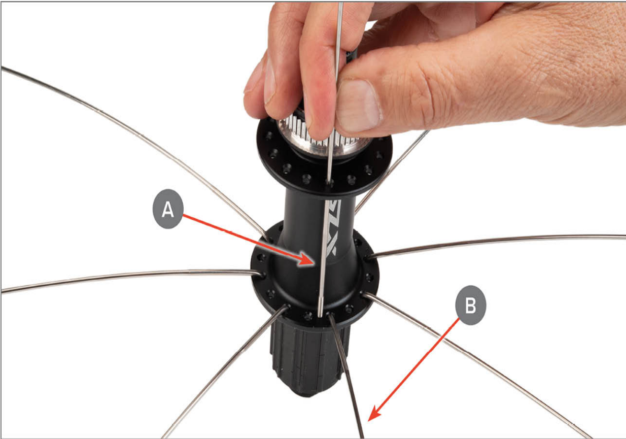
FIGURE 6.17: First spoke of left flange used as straight pointer to select correct left flange hole
