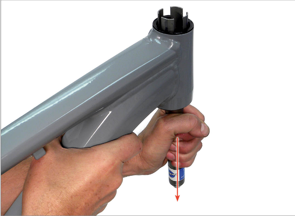
FIGURE 16.22: Draw the Race Tool RT-1 or RT-2 through head tube small end first
