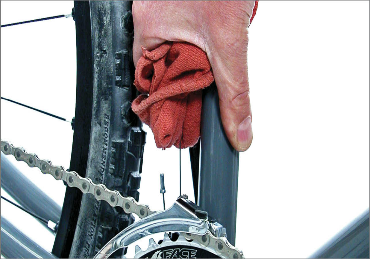
FIGURE 10.49: Pull cable by hand or lever to force derailleur to limit screw
