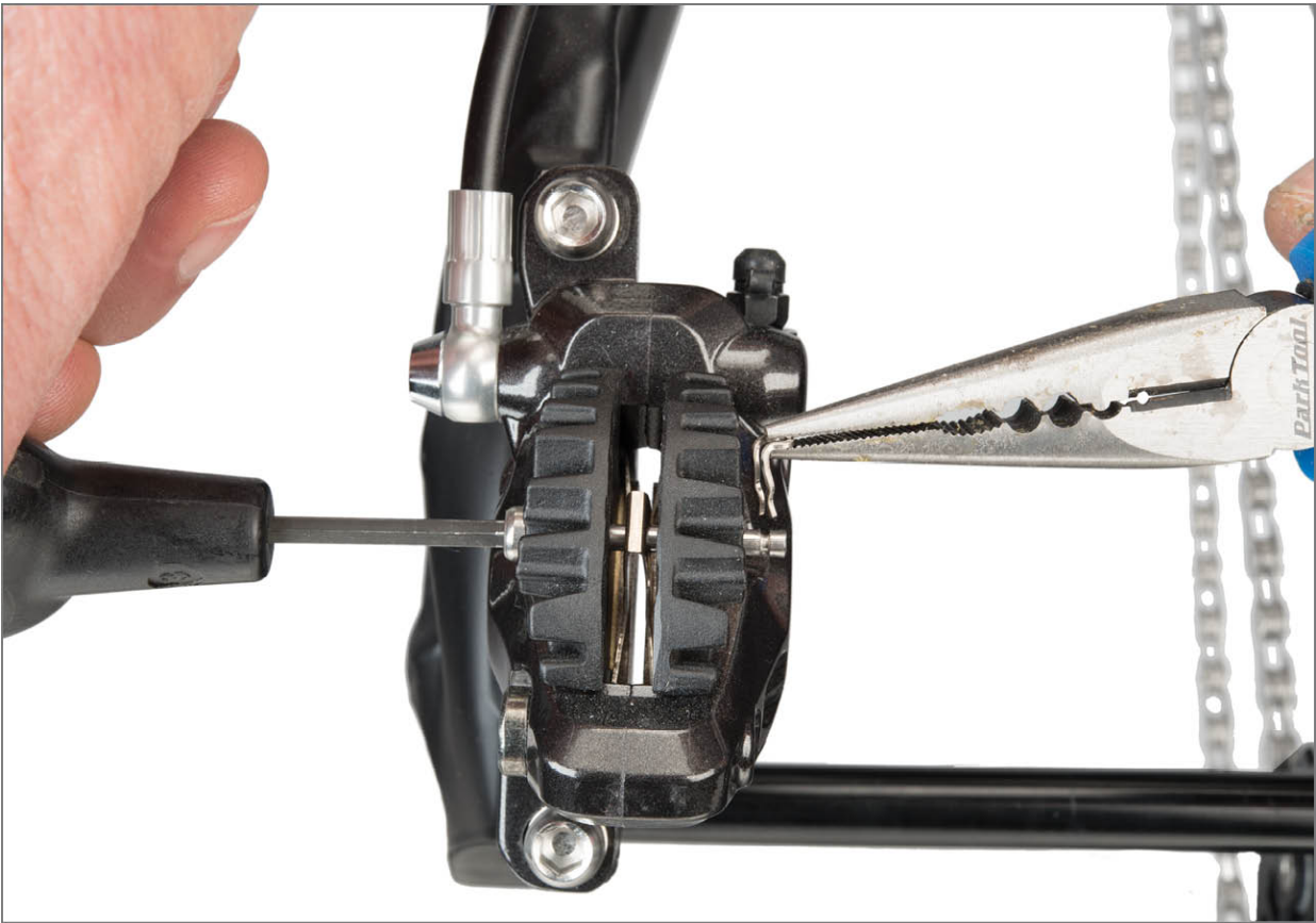
FIGURE 13.9: Remove bolt clip and unthread pad-fixing bolt
