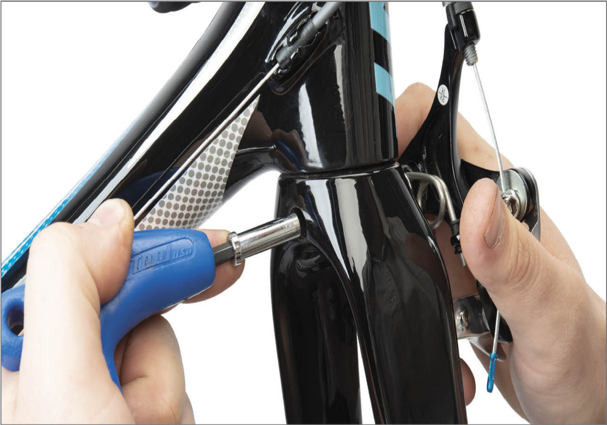
FIGURE 14.42: Hold caliper centered while securing mounting nut
