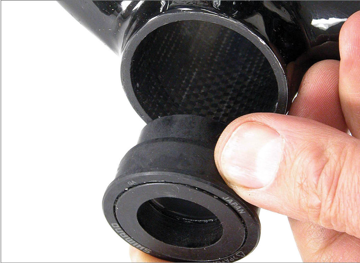
FIGURE 7.32: PF41 (BB86) shell with pressed bearing adaptors
