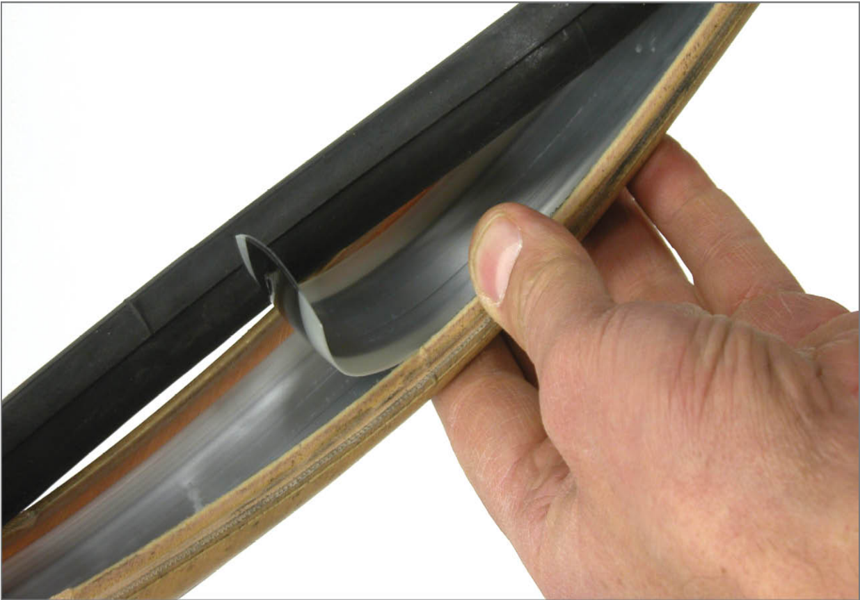
FIGURE 2.37: Tire liner placed inside tire body
