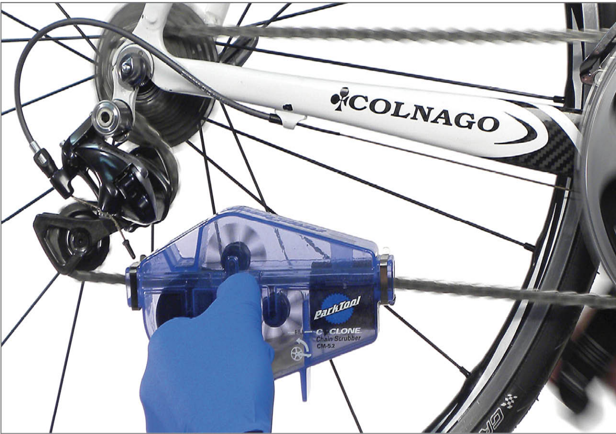
FIGURE 8.38: Chain cleaning with chain still on bike
