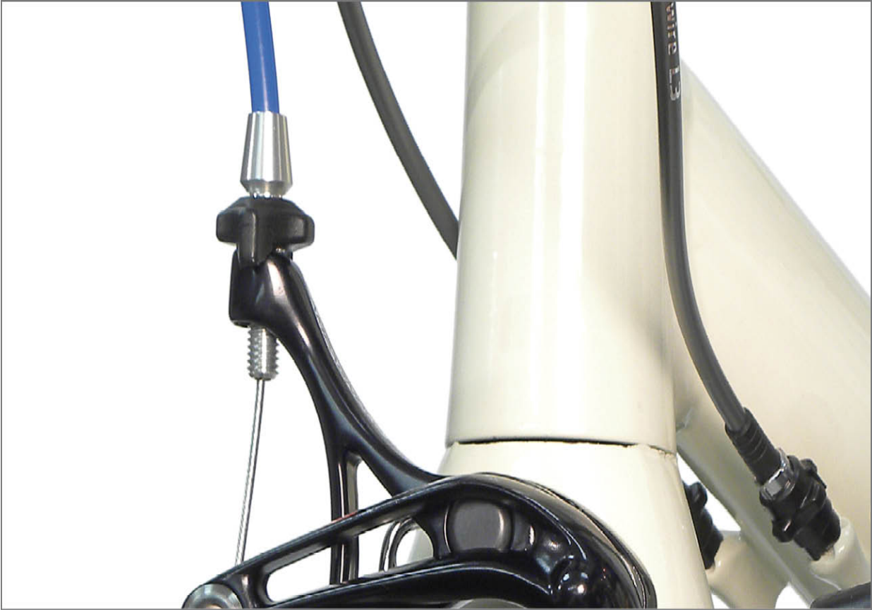
FIGURE 14.16: Adjusting barrel to control cable slack
