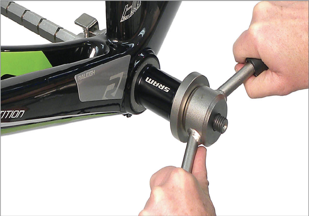
FIGURE 7.45: Pressing the aluminum conversion sleeve into a BB30 shell
