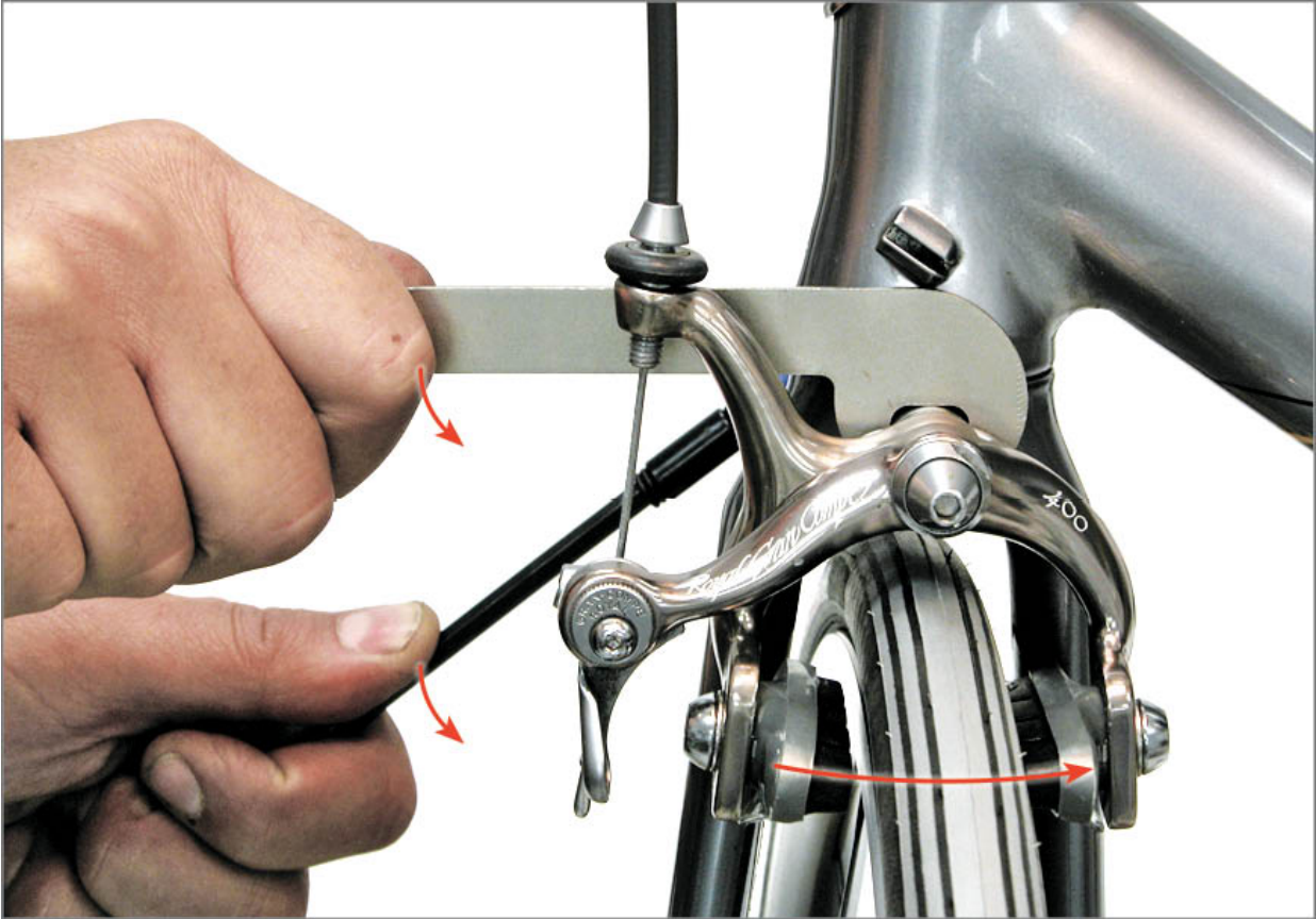
FIGURE 14.48: Centering side pull with centering flats on brake stud
