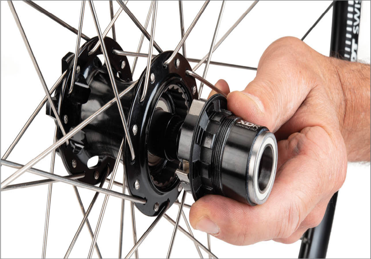
FIGURE 4.22: Remove freehub by pulling outward
