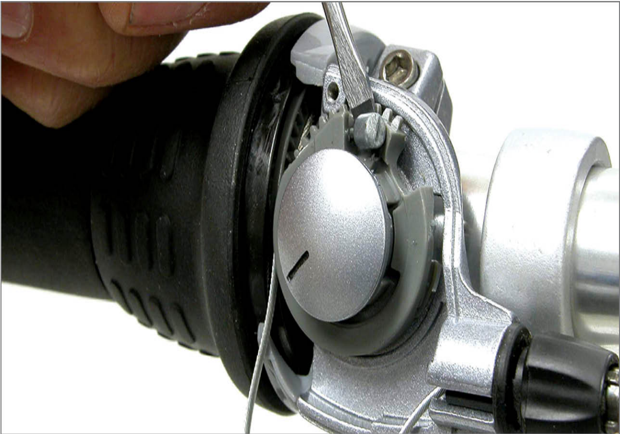
FIGURE 12.13: Shift cable attachment in Revoshift® lever
