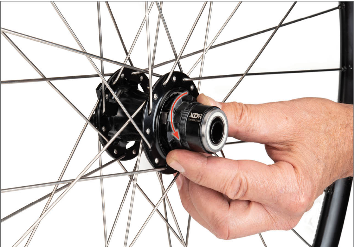
FIGURE 4.30: Slide freehub on axle and rotate counterclockwise while engaging into hub shell
