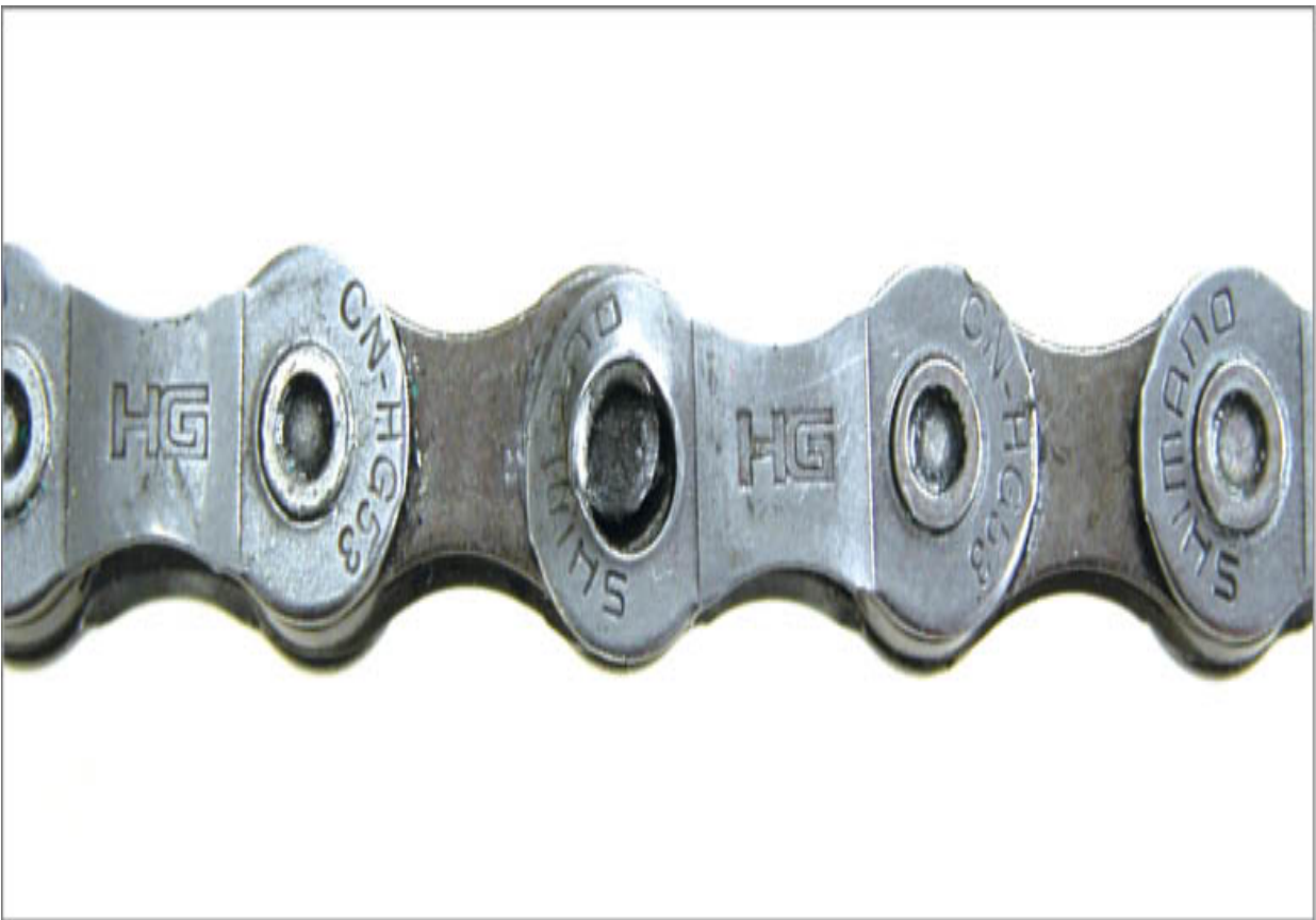
FIGURE 8.33: Damaged side plate. Repair on plate is not possible
