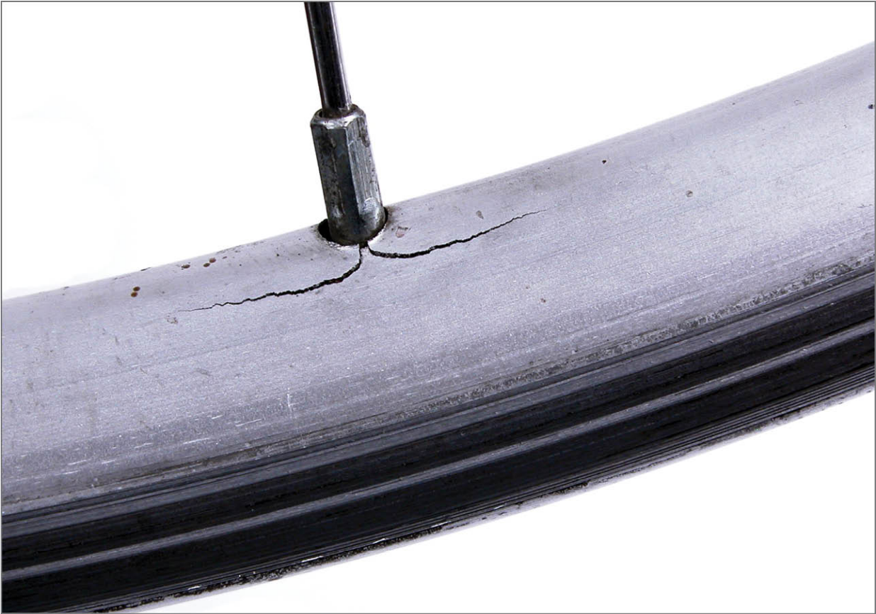
FIGURE 5.23: Crack in rim from excessive spoke tension
