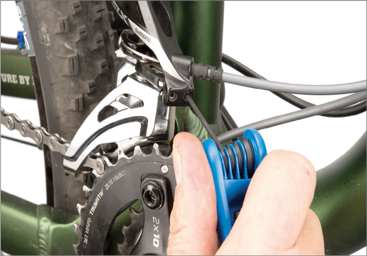
FIGURE 10.39: Side swing design front derailleur
