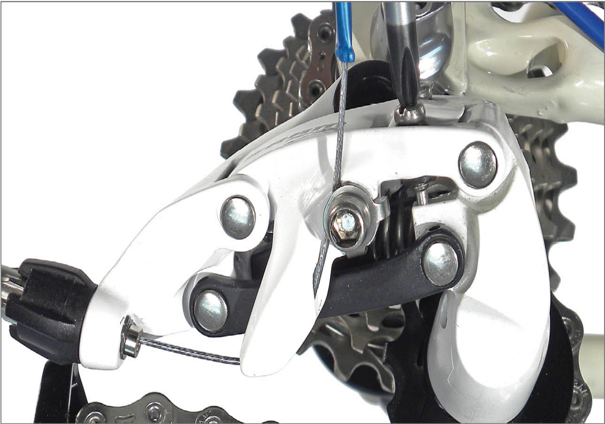
FIGURE 10.58: Inspect end of limit screw to determine which limit it control
