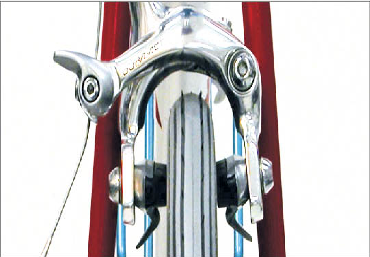
FIGURE 5.8: Center error with wheel sitting too far to right side
