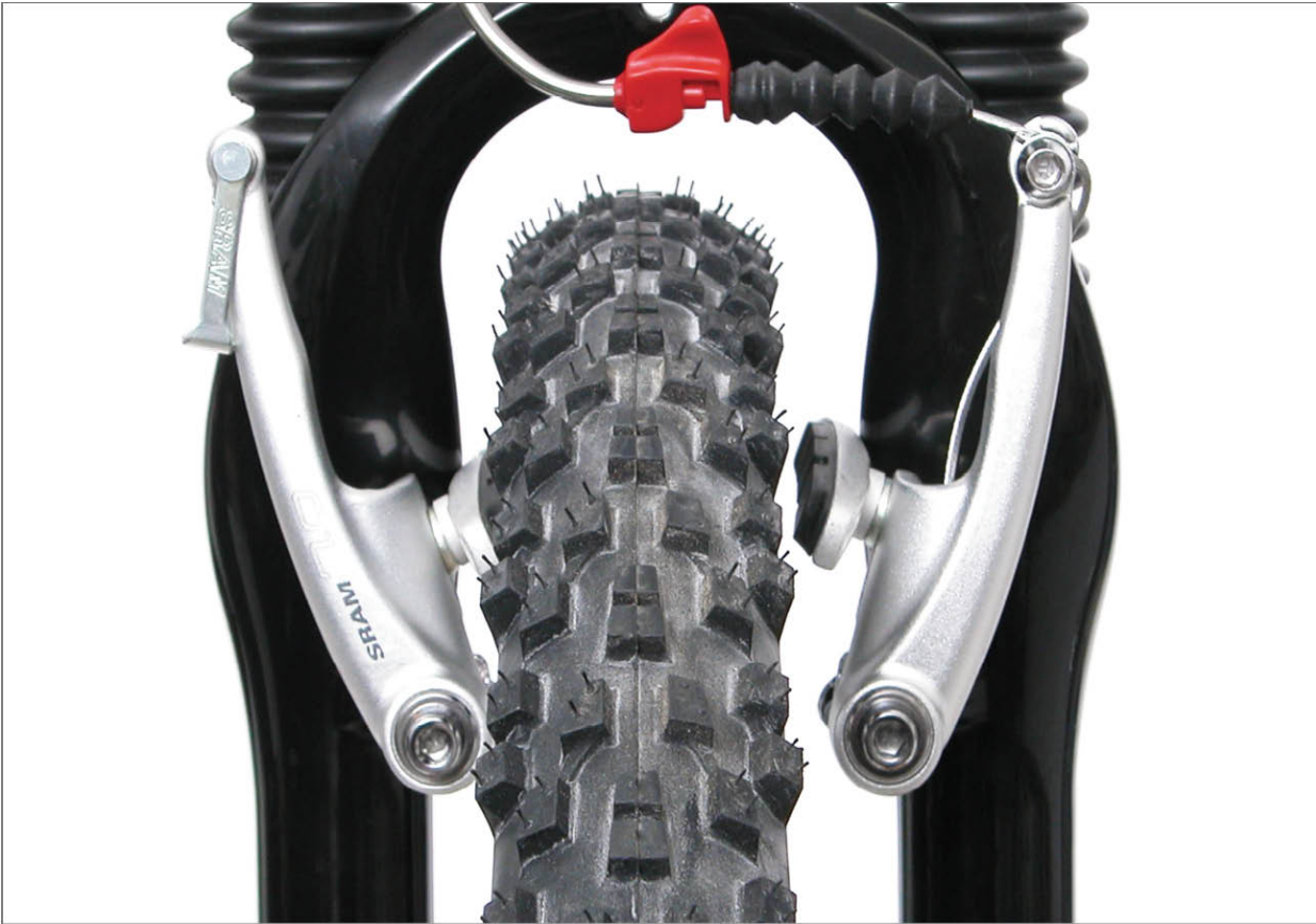
FIGURE 14.22: Misaligned wheel off-set to mechanic's left side
