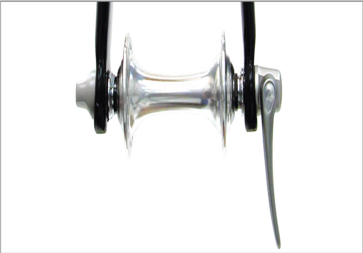
FIGURE 2.62: Quick-release lever in fully open position
