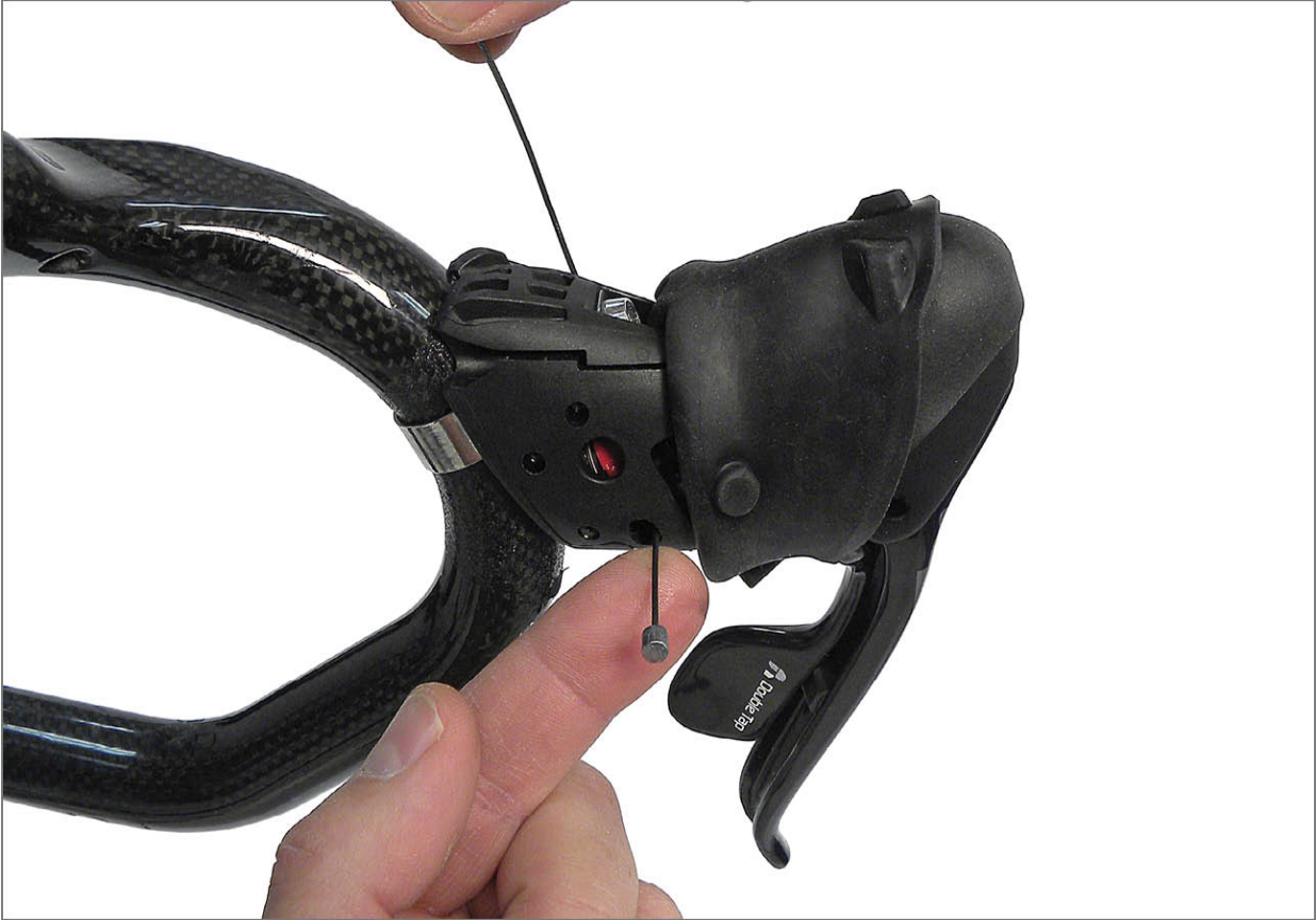
FIGURE 10.27: Cable access is from the inside of lever body and cable exit hole is on upper side of body
