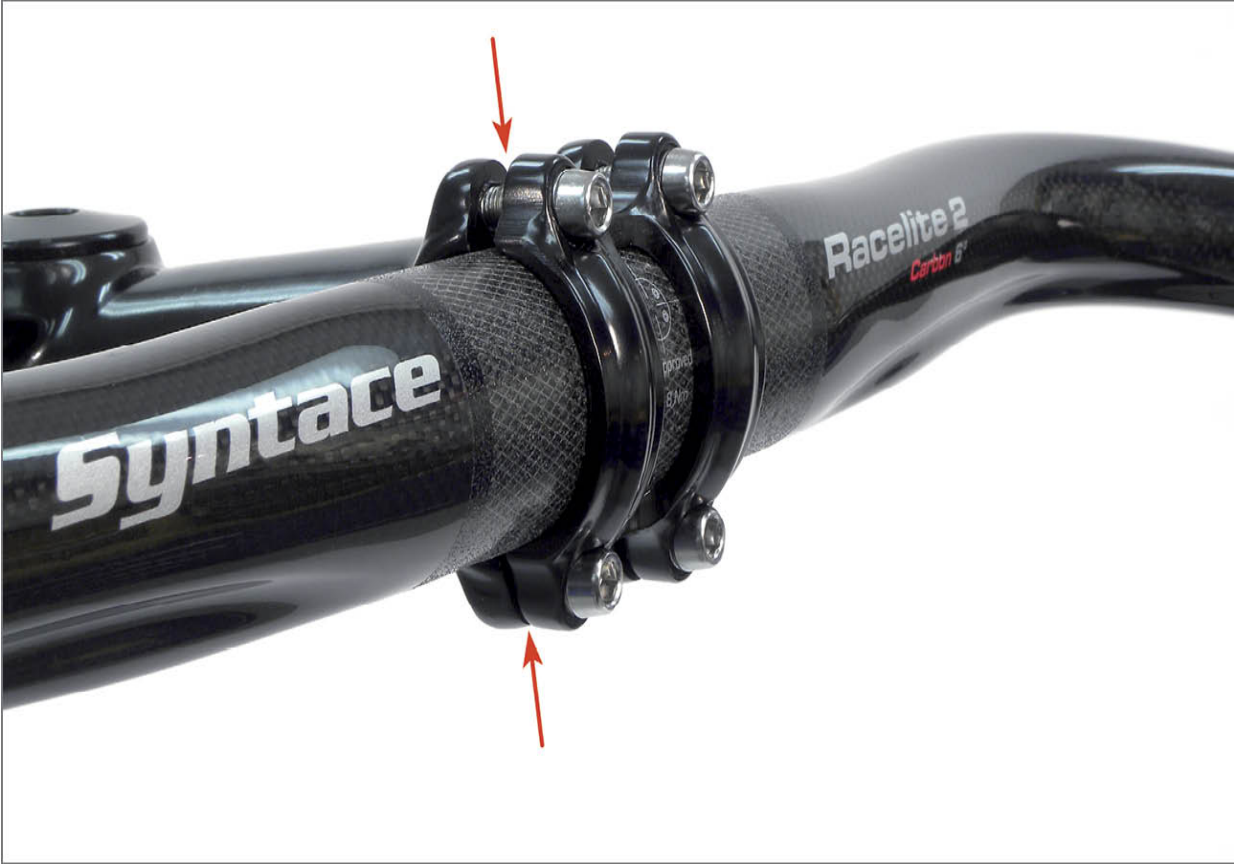
FIGURE 15.10: Gap between faceplate and stem body must be even between top and bottom plates
