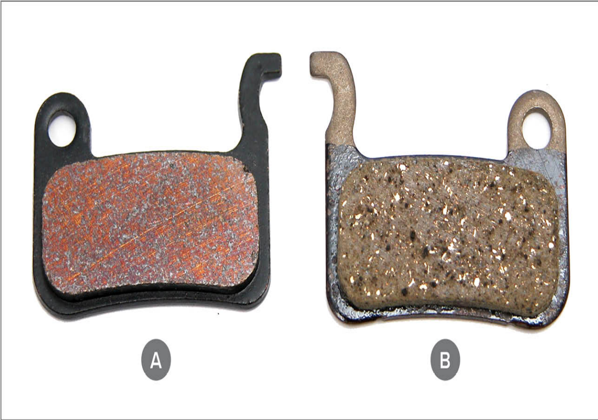
FIGURE 13.7: (A) Semimetallic disc brake pad, (B) Resin disc brake pad
