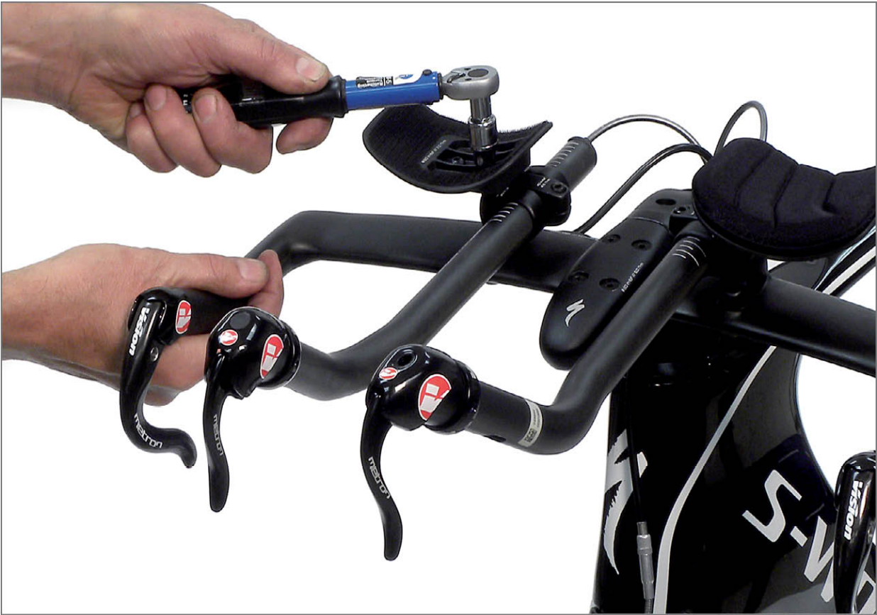
FIGURE 15.9: Secure all fittings on integrated aero bar systems
