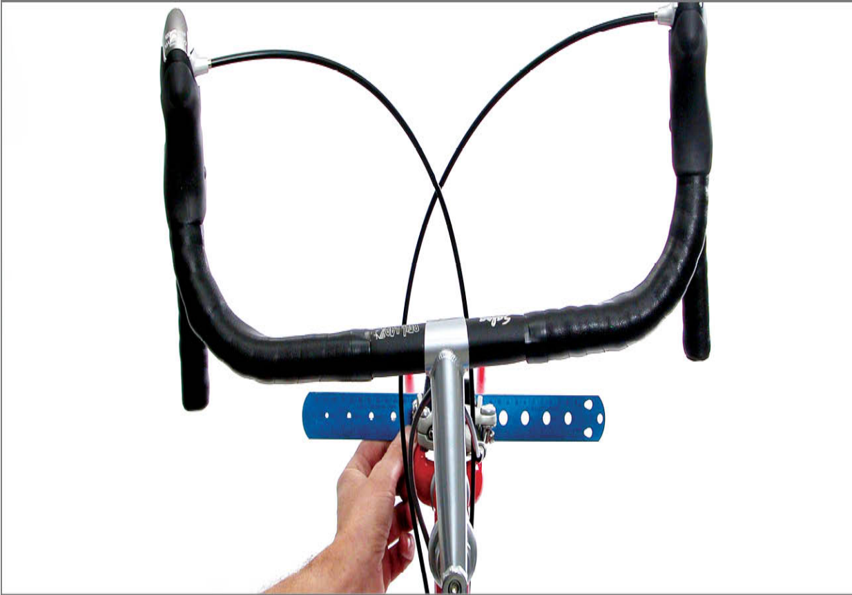
FIGURE 15.14: Straightedge shows bars and stem are not aligned
