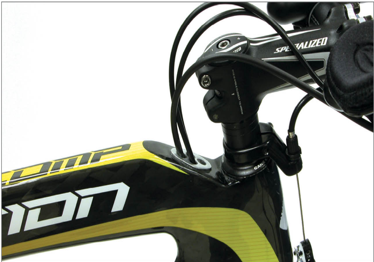
FIGURE 10.12: Internal routing for shift and brake housing
