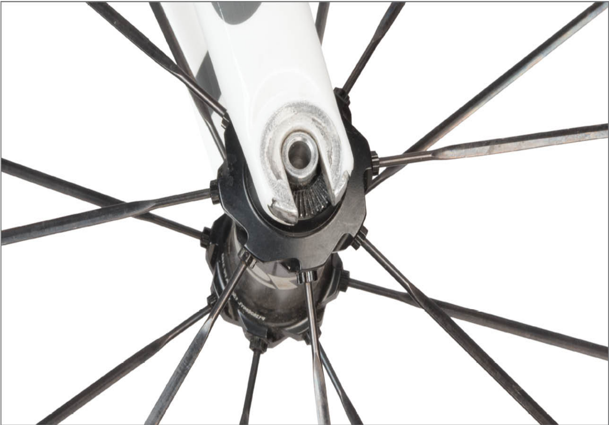
FIGURE 2.1: Open slot design of fork seen without skewer
