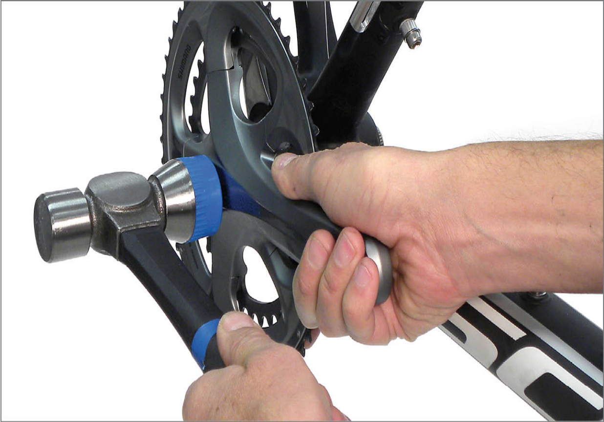
FIGURE 7.15: If necessary choke up on mallet handle and tap crank fully into bottom bracket bearing adaptors
