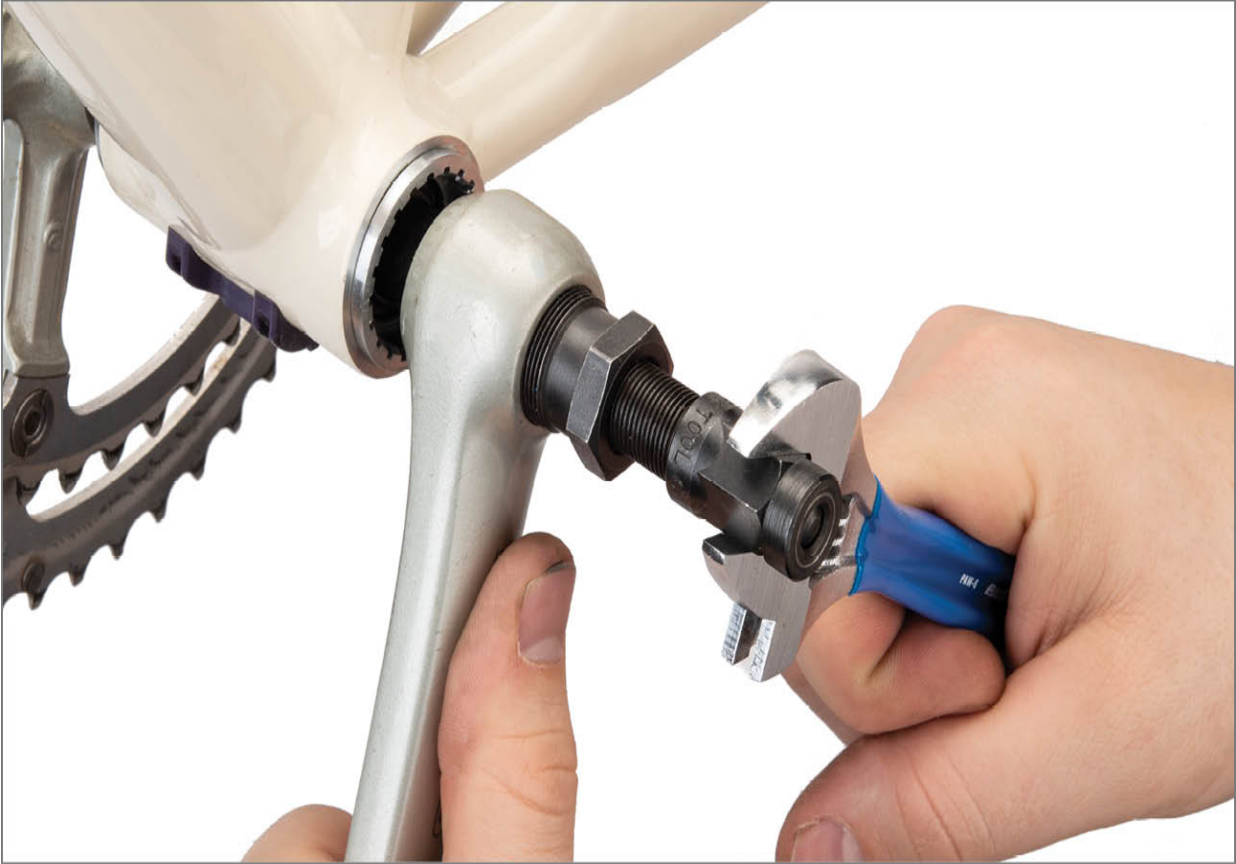
FIGURE 7.11: Remove crank from spindle by turning driver of crank remover
