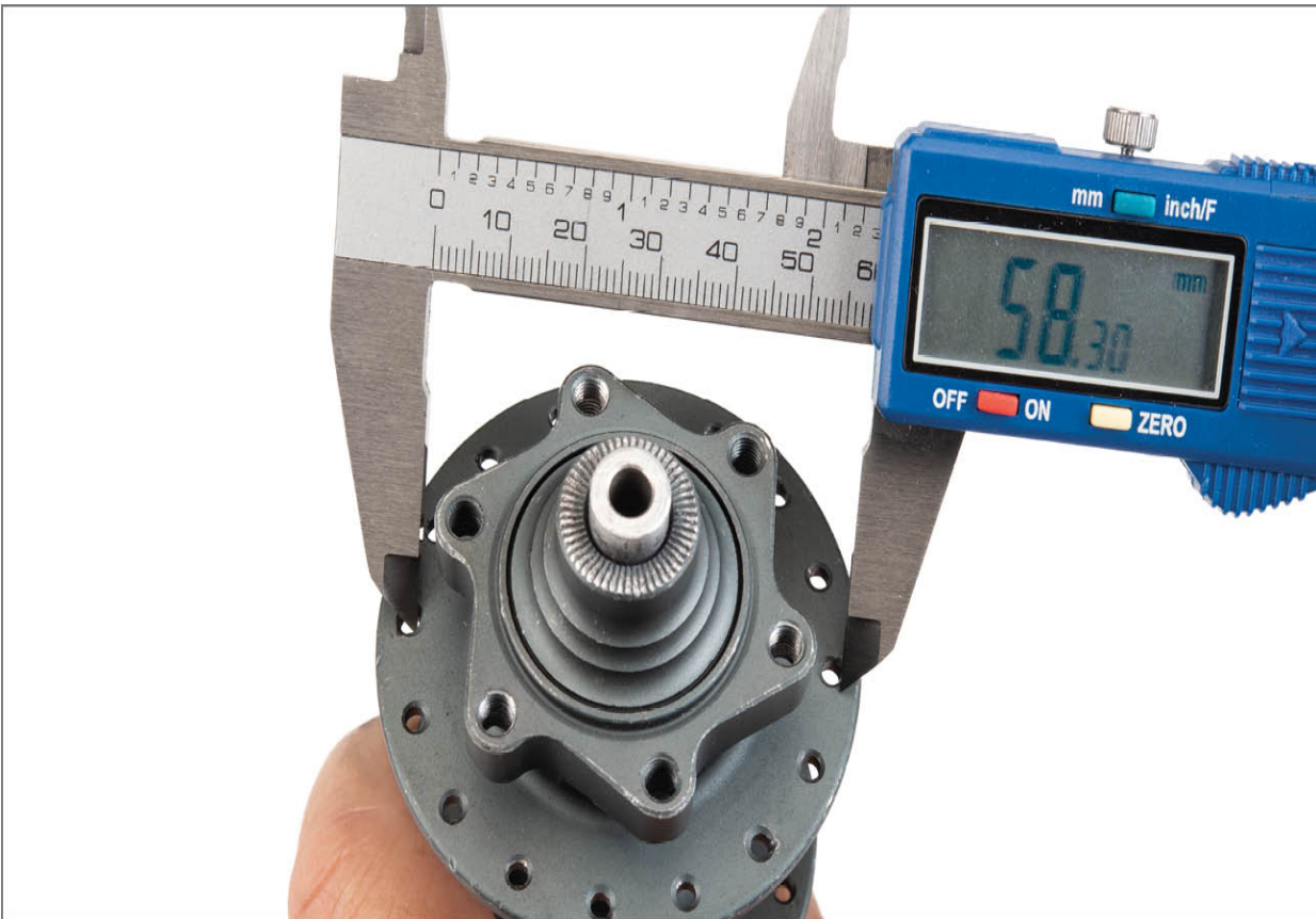
FIGURE 6.4: Measure directly opposite spoke holes from inner edge to outer edge
