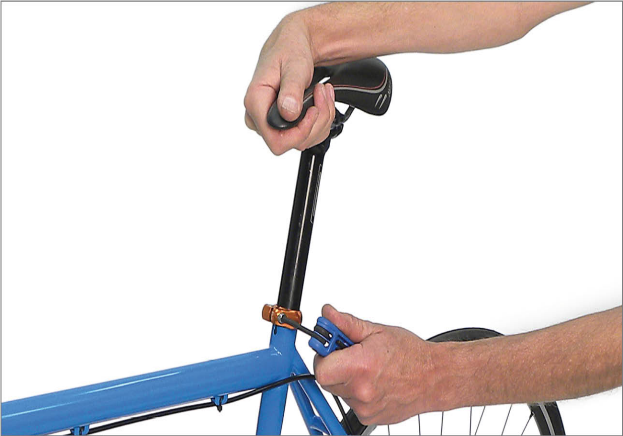
FIGURE 15.24: Test saddle rotation by twisting with one—not two—hands
