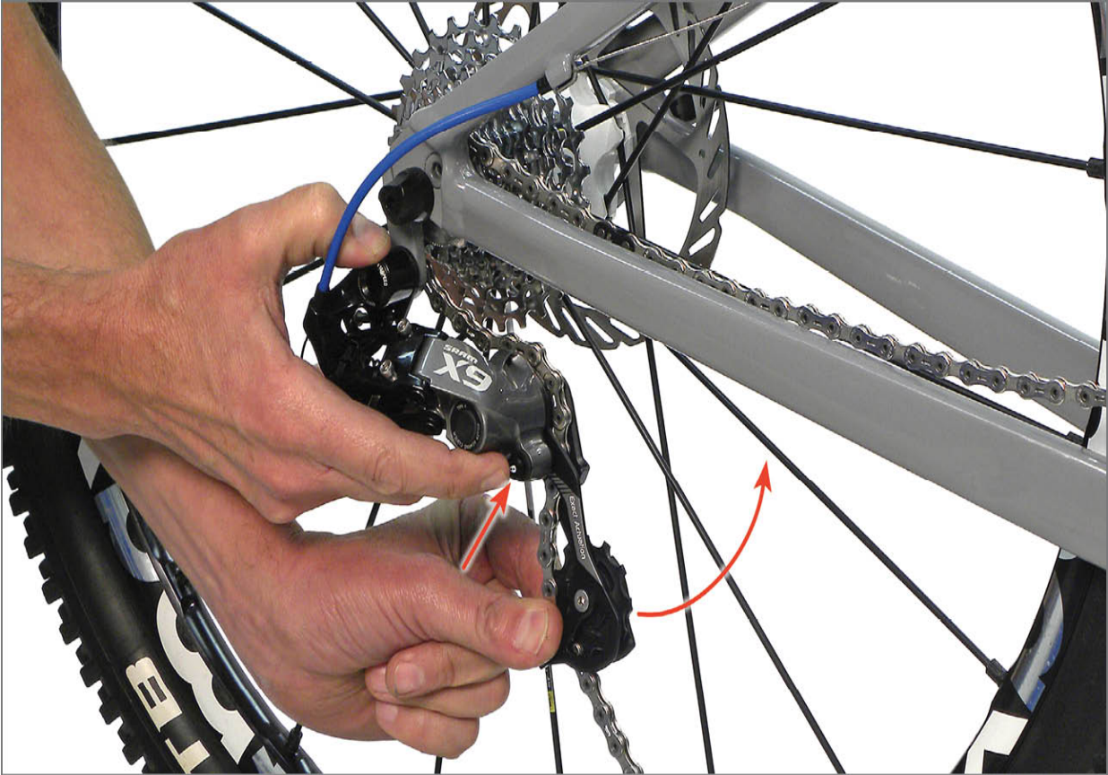
FIGURE 2.9: Push forward on lower pulley and depress cage lock button to hold
