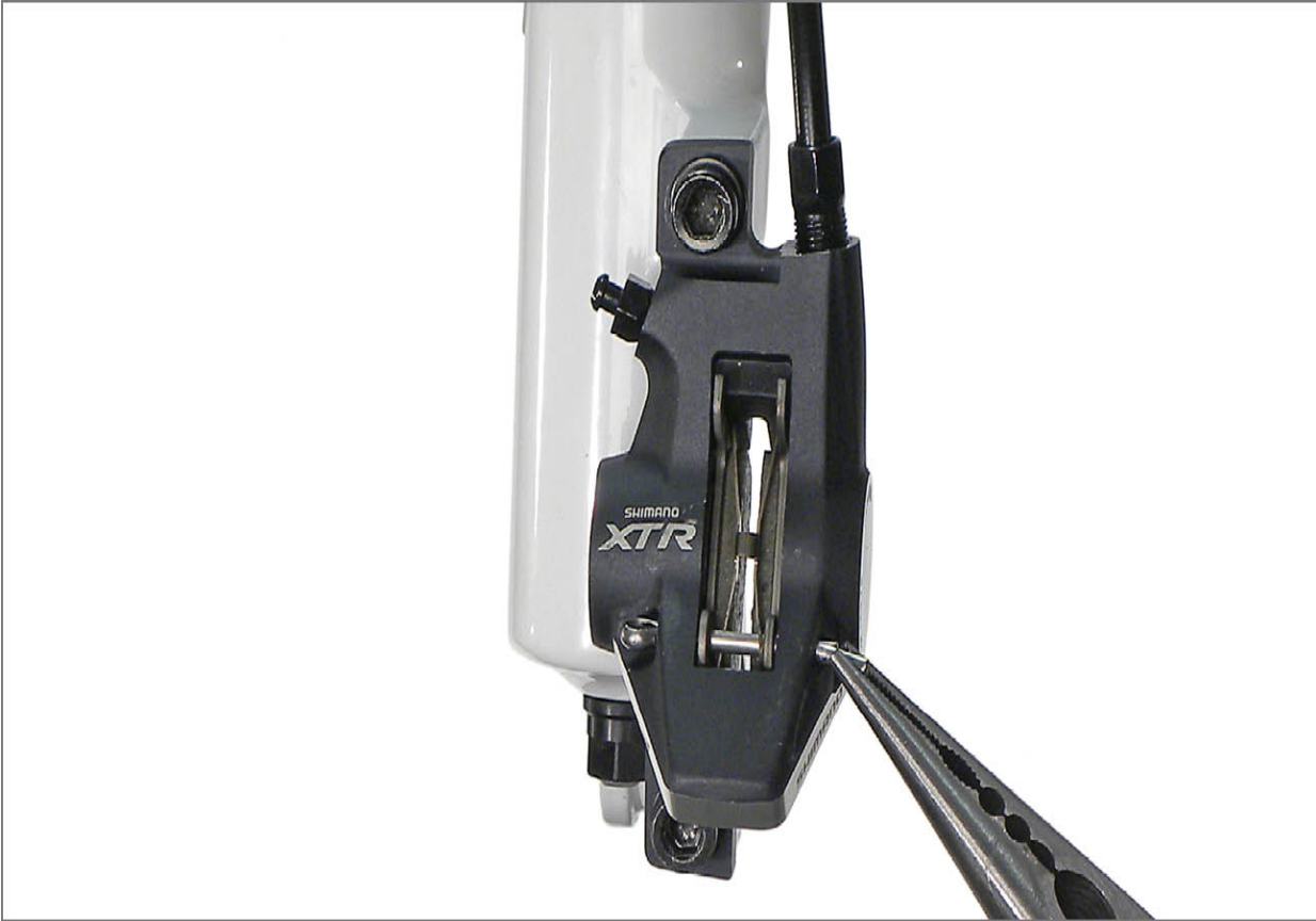
FIGURE 13.10: Straighten cotter pin before pulling from body
