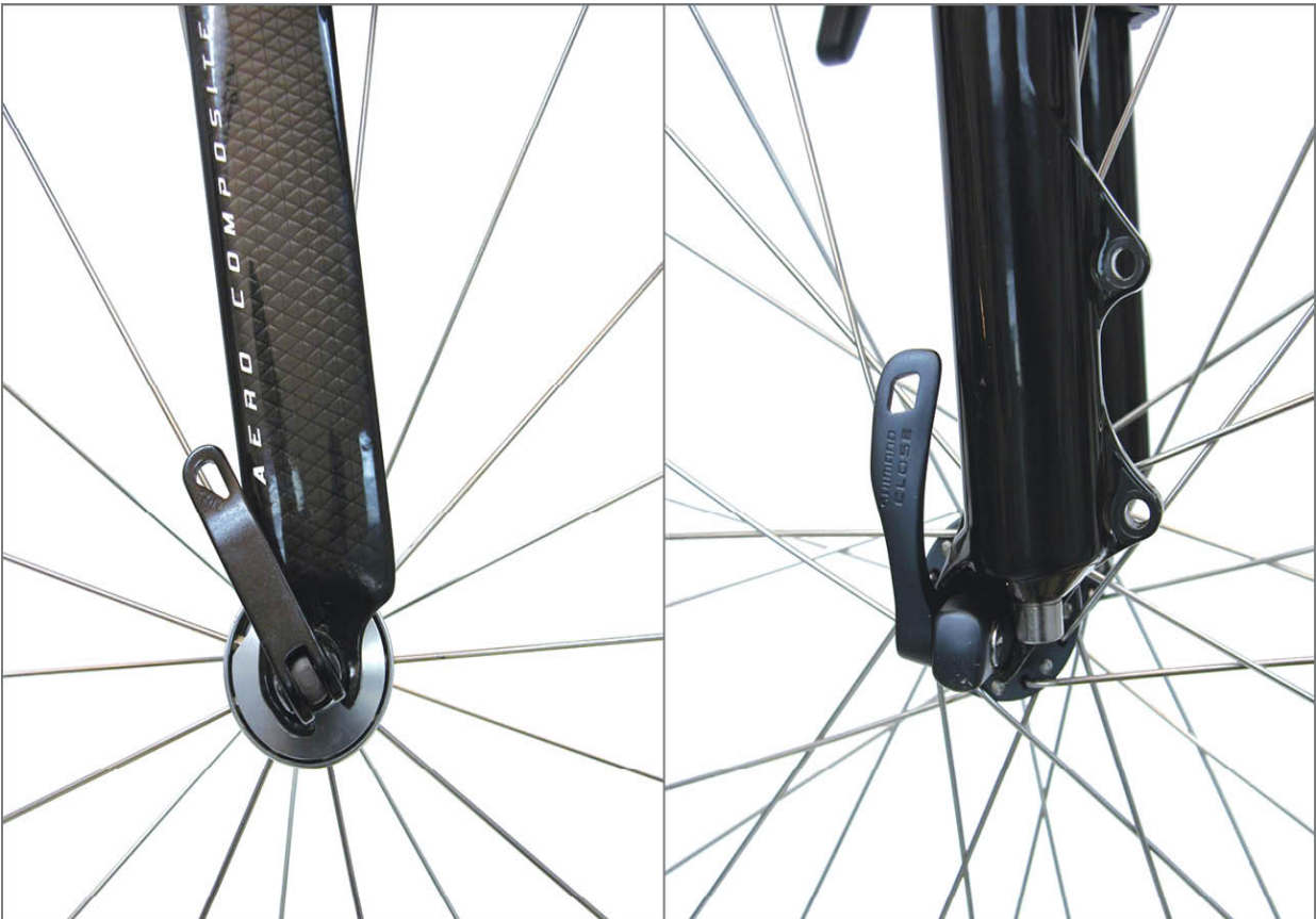
FIGURE 2.68: Place lever just in front of fork blade when possible
