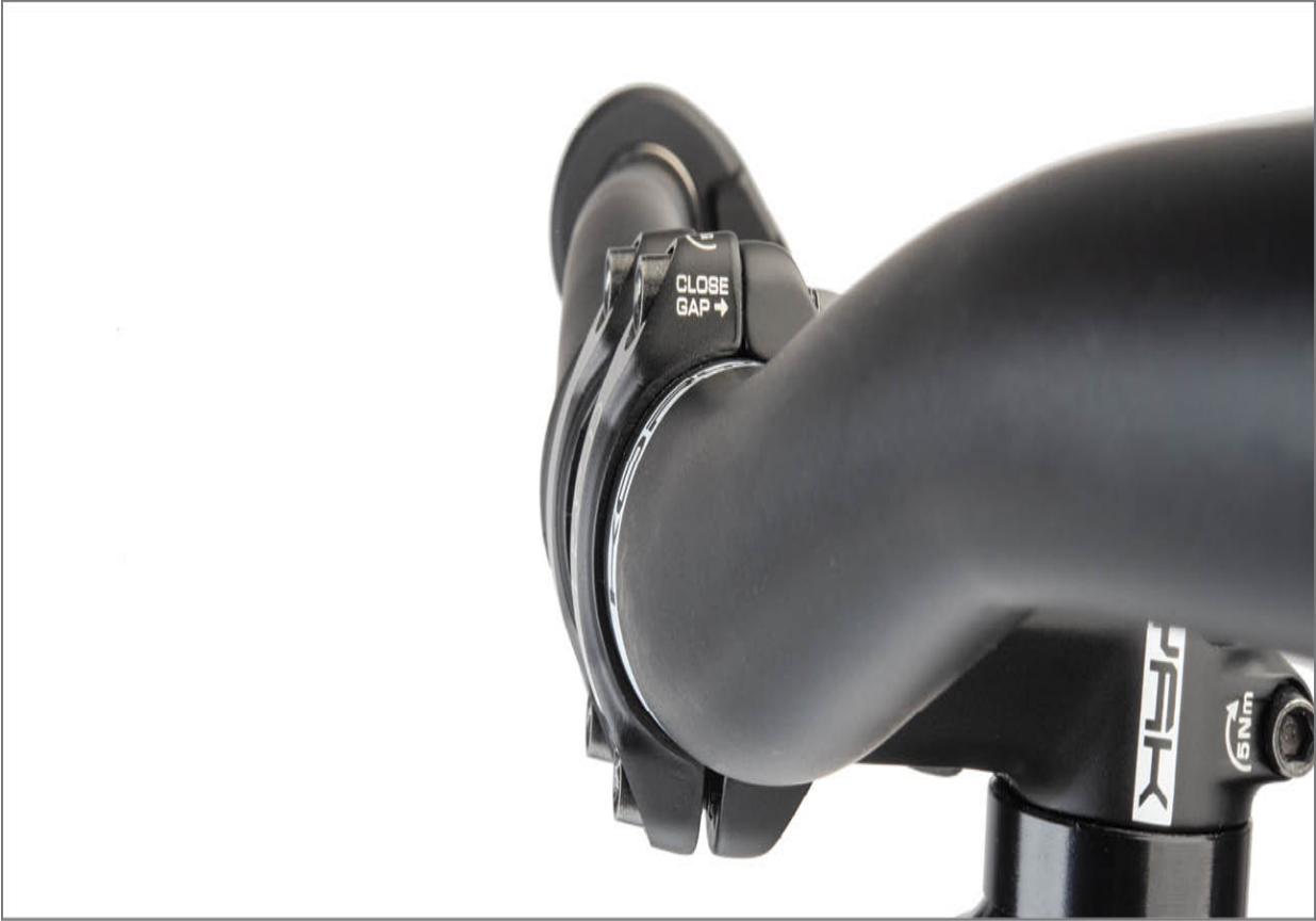
FIGURE 15.11: With “zero gap” stem design, snug top bolts before fully tightening lower bolts
