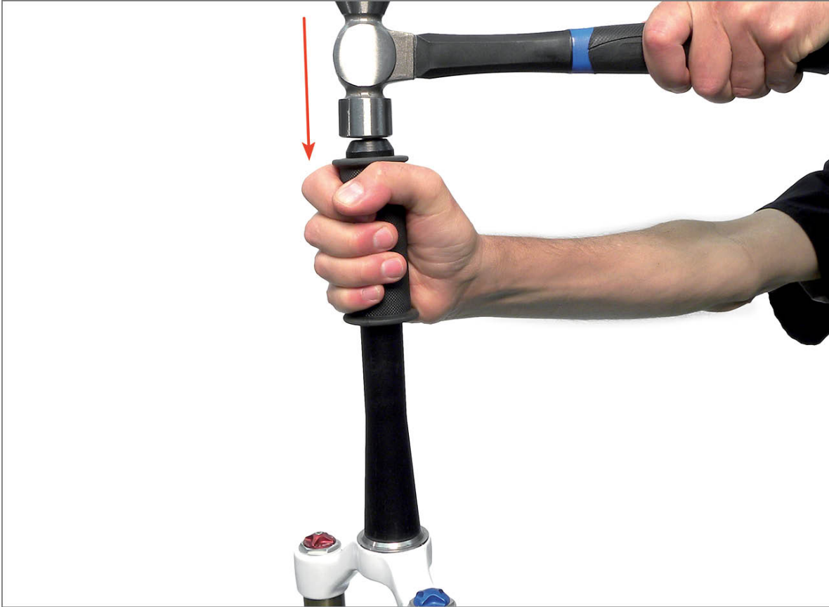
FIGURE 16.35: Using TNS-4 to drive star nut down while keeping it aligned
