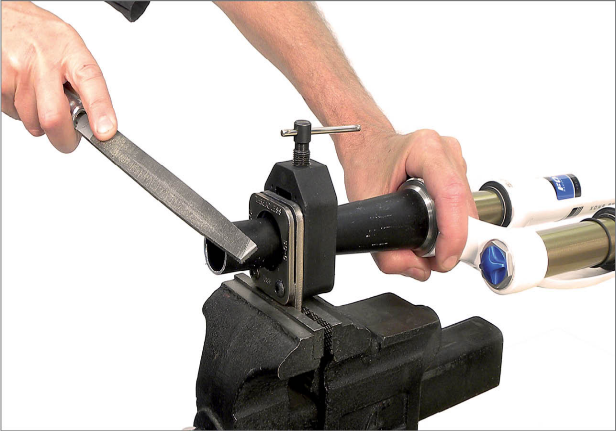
FIGURE 16.31: Deburr and finish end of column before installation
