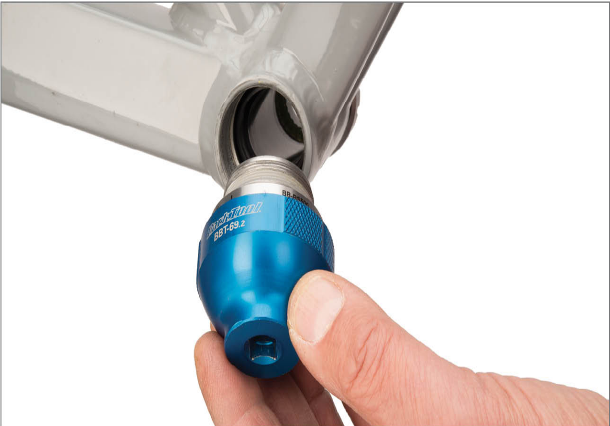
FIGURE 7.56: Install dust sleeve into adaptor and thread adaptor into frame
