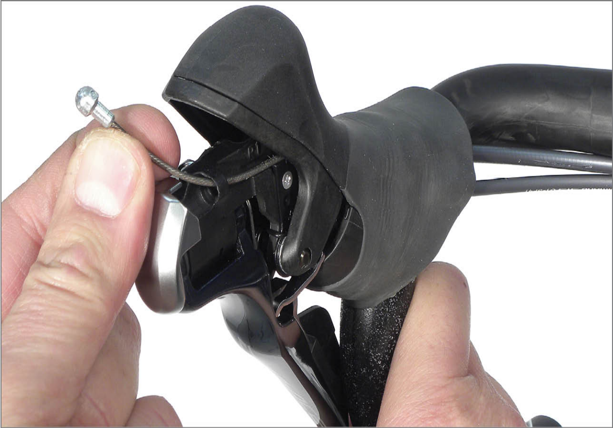
FIGURE 14.4: Insert brake cable from front of lever
