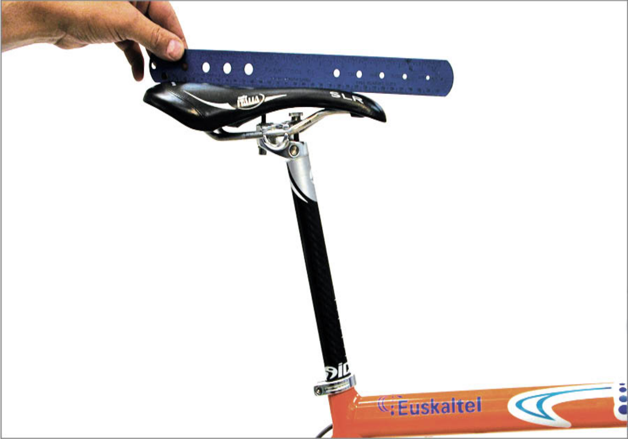
FIGURE 15.22: Use straightedge to extend saddle line when adjusting tilt
