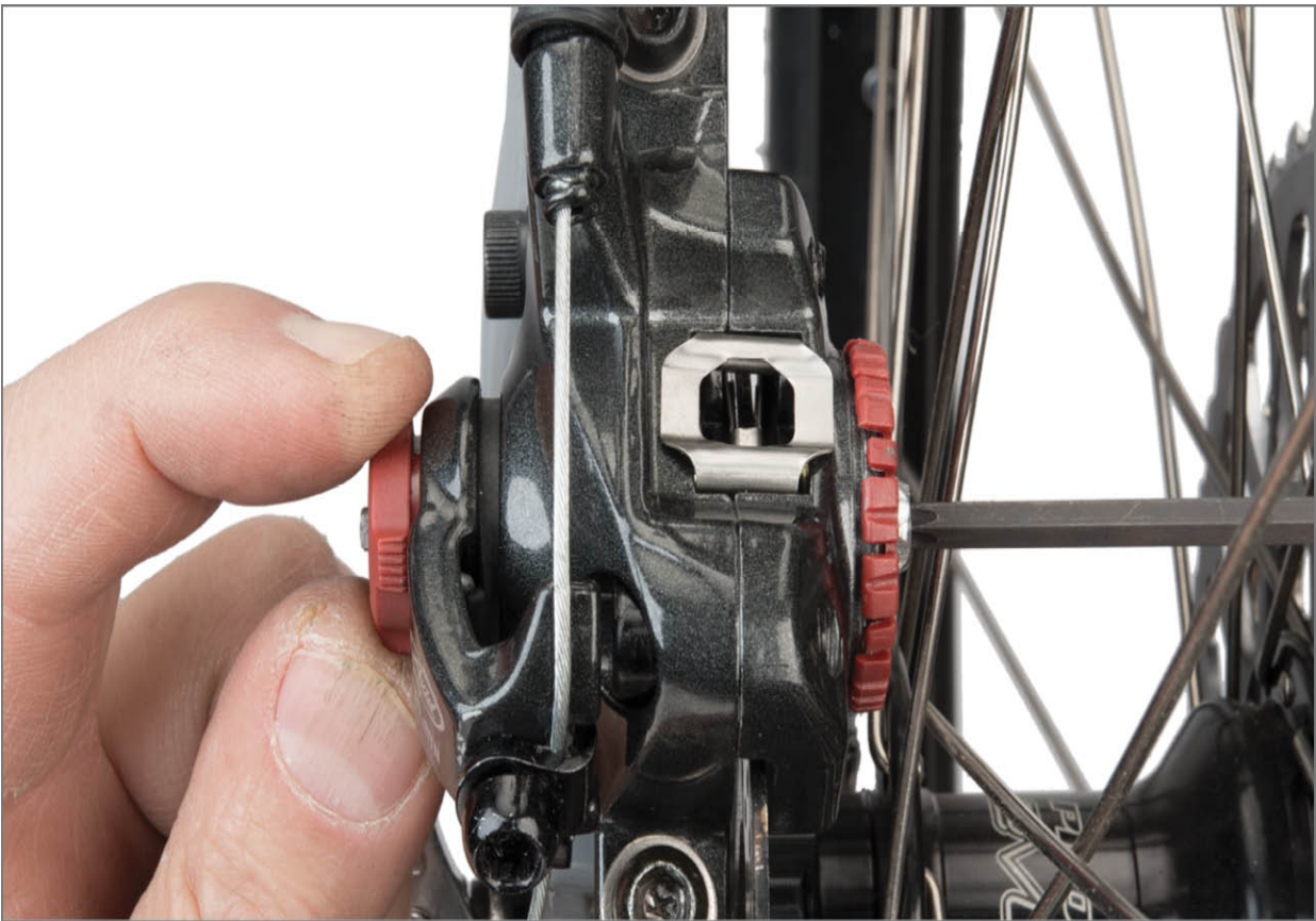
FIGURE 13.13: Dial mechanical caliper pad adjustment screws
