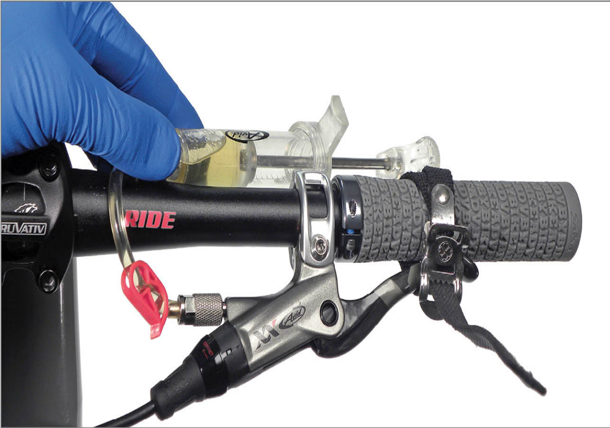
FIGURE 13.52: Pull and hold lever to handlebars after closing lever syringe clip
