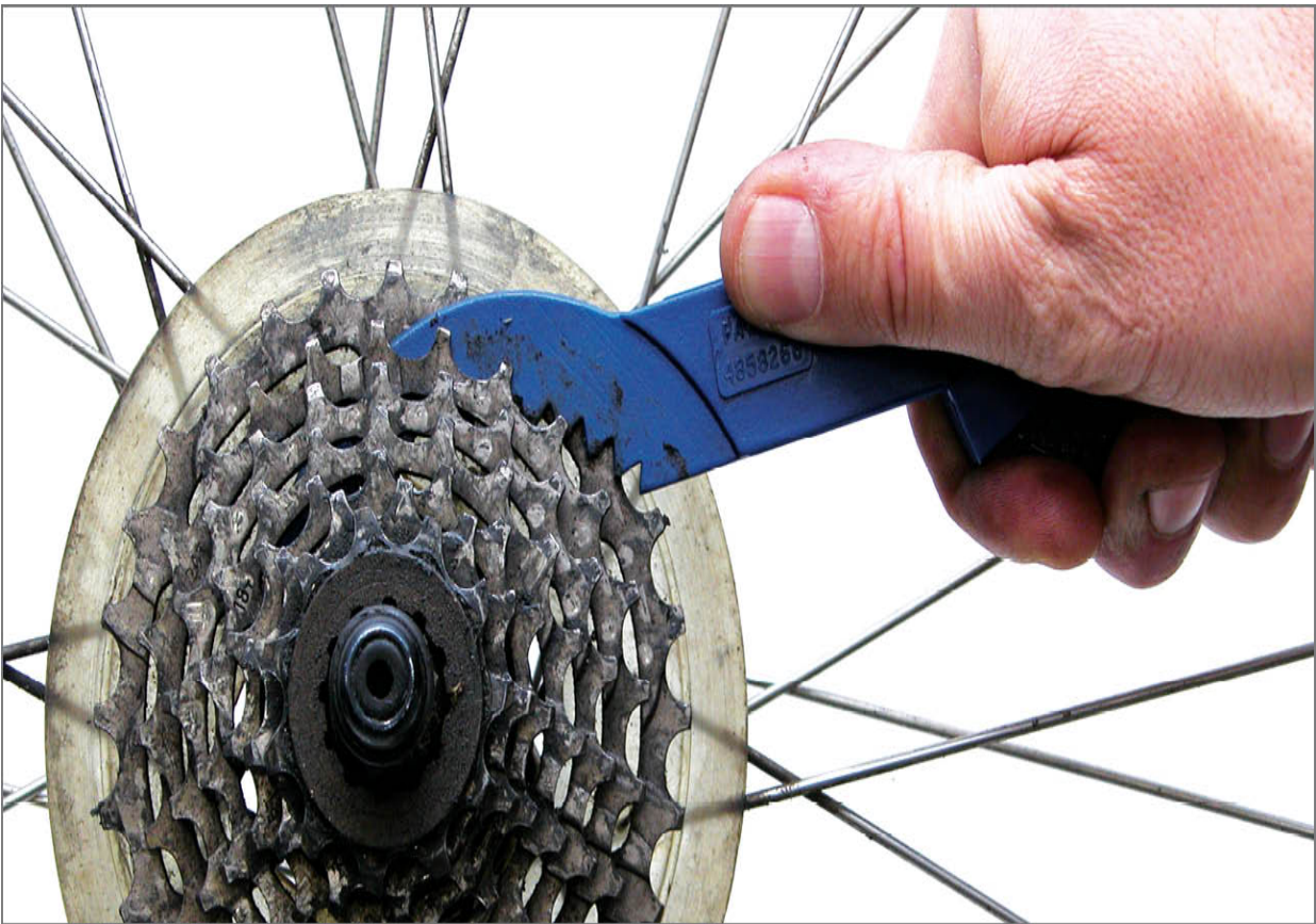
FIGURE 3.17: Cleaning debris between sprockets with the “comb” of GSC-1
