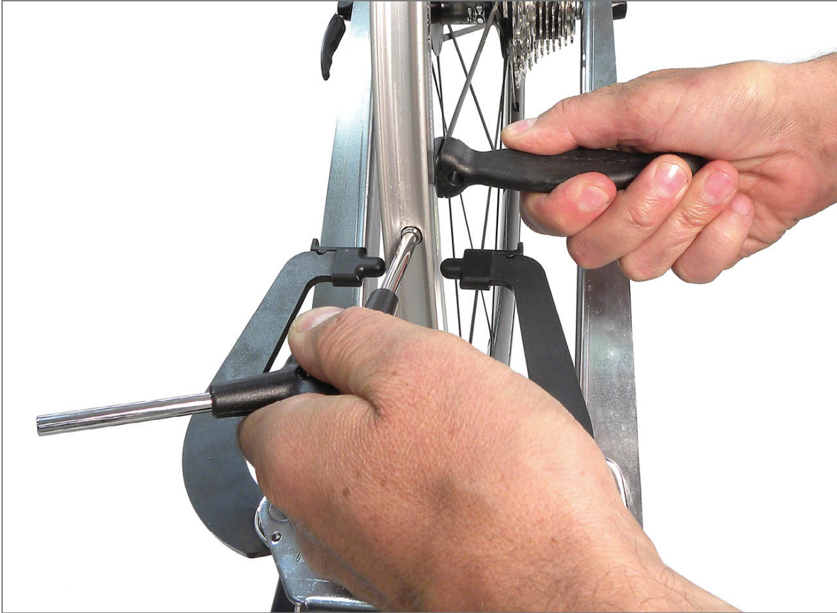
FIGURE 5.5: Truing a rim with internal nipples
