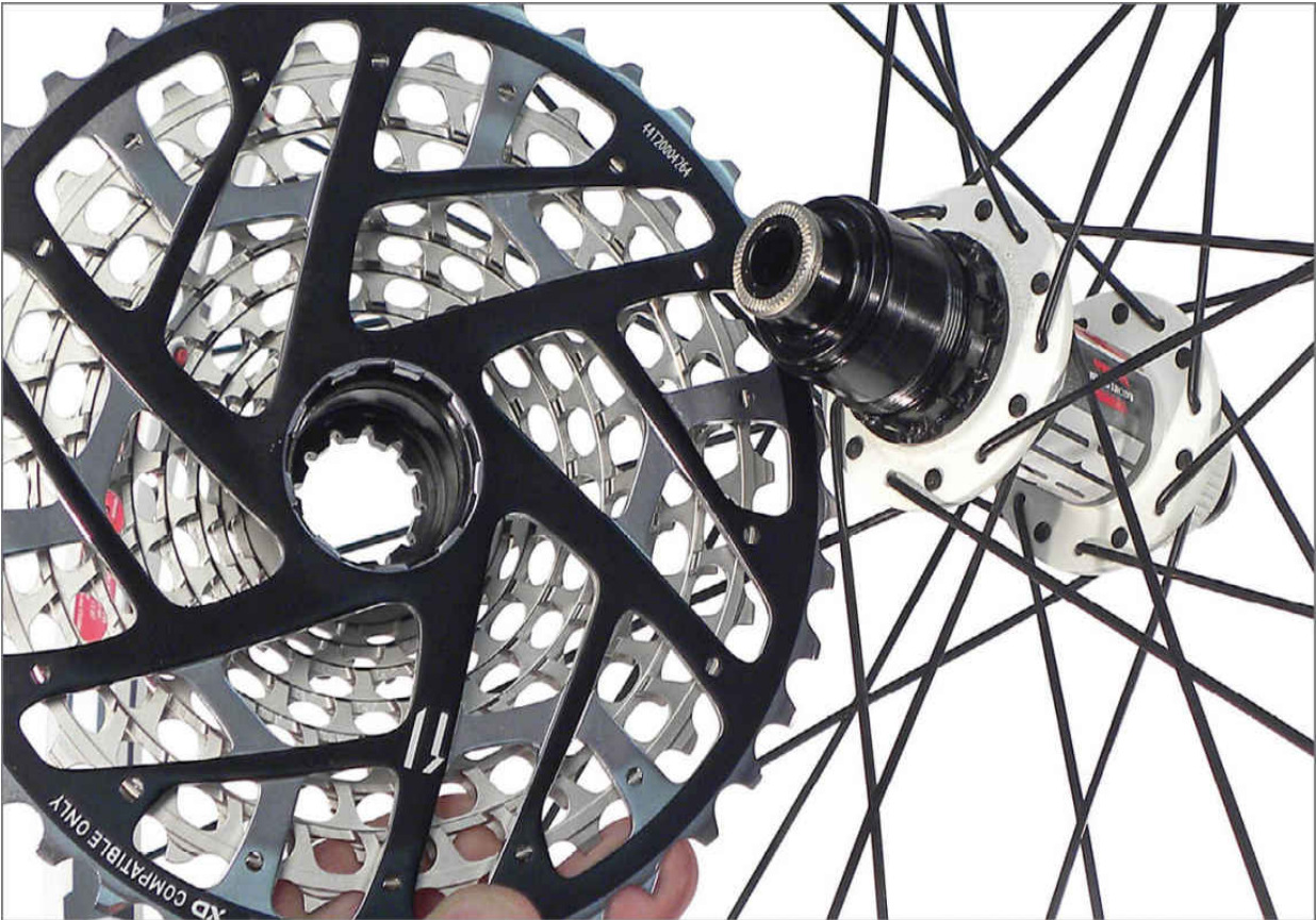
FIGURE 3.8: SRAM® XX1® cassette with special freehub body
