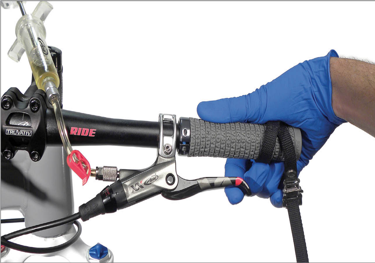
FIGURE 13.54: Release brake lever slowly while pushing caliper syringe
