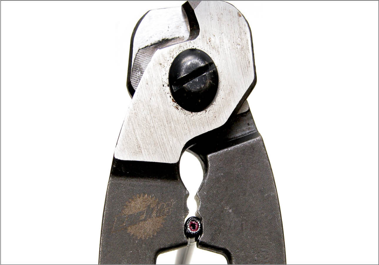
FIGURE 10.5: Reshape compressionless housing after cutting
