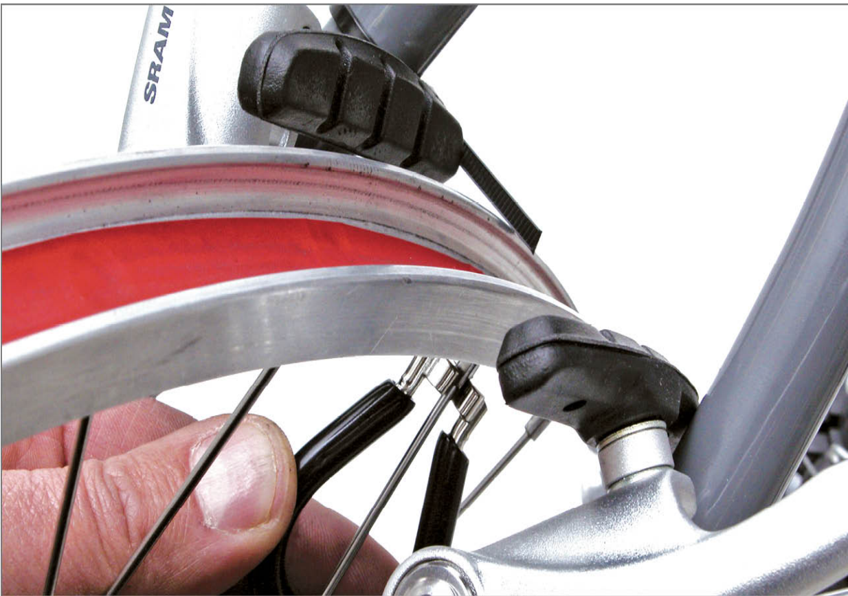
FIGURE 5.18: Isolate radial runout and select left-right pair of spokes to correct
