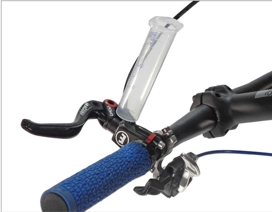
FIGURE 13.37: Install syringe into bleed port at lever
