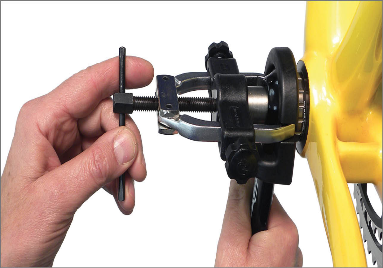
FIGURE 7.28: Turn driver of puller clockwise to pull arm from spindle
