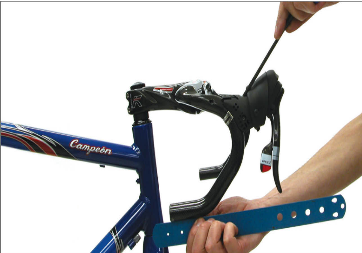
FIGURE 10.21: Align brake/shift levers relative to lower section of drop handlebars
