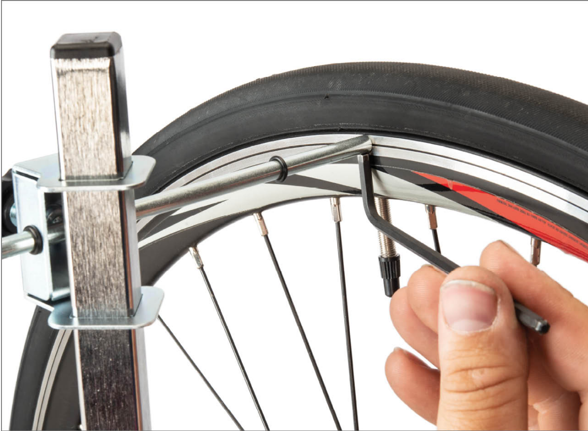
FIGURE 10.74: Use a 4mm hex wrench as a go/no-go gauge when checking tolerance
