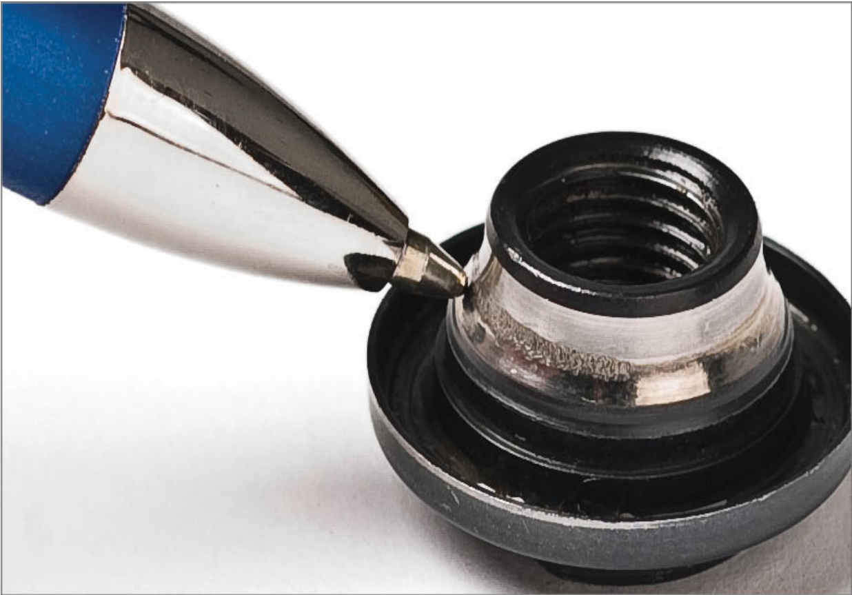
FIGURE 4.11: Look and feel for pits along ball path of cone
