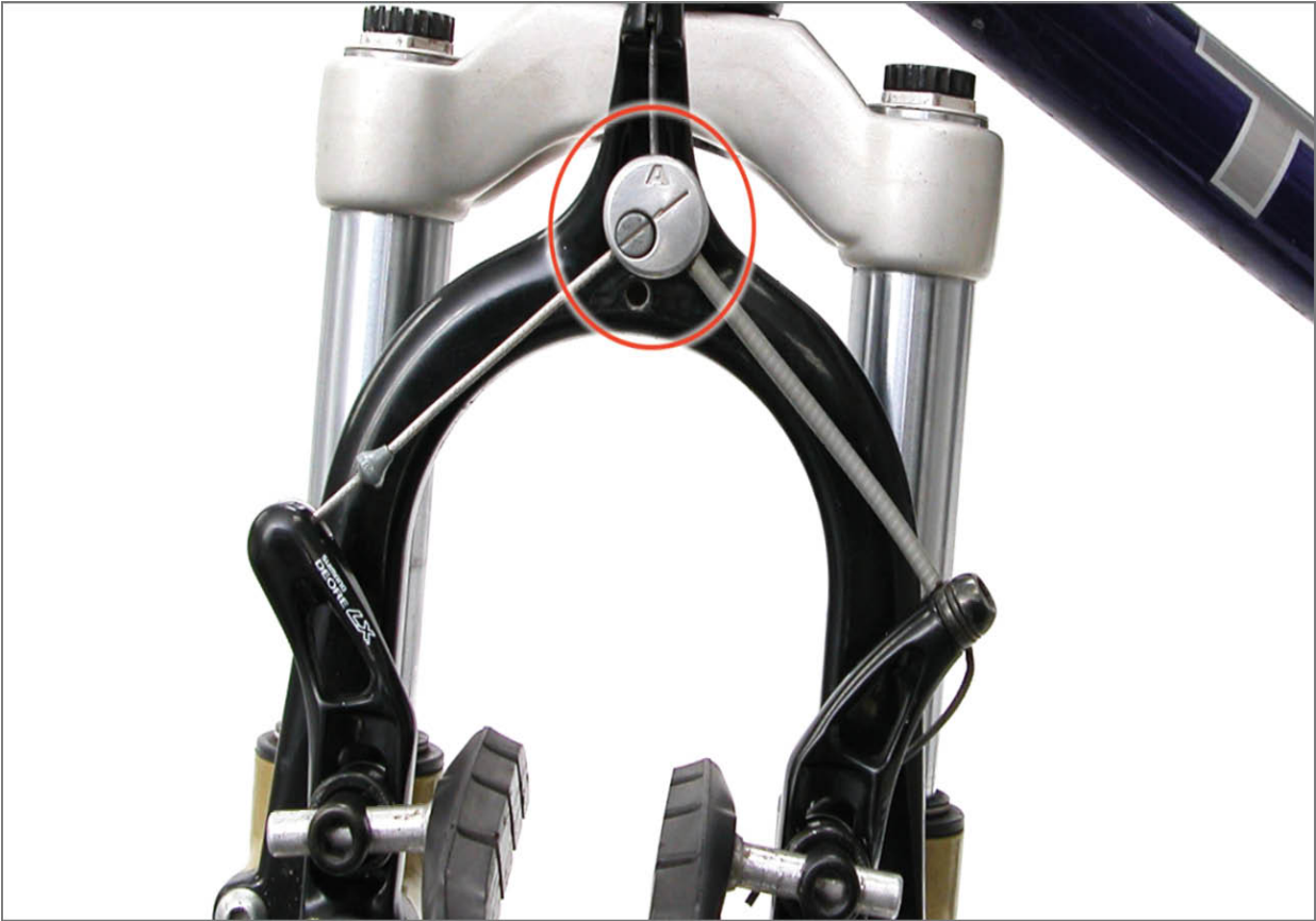
FIGURE 14.36: Straddle wire link unit
