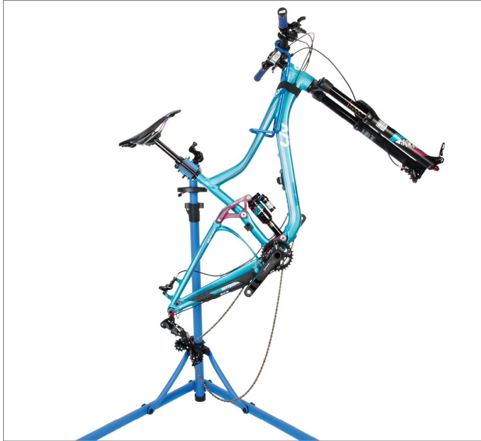
FIGURE 13.46: Rotate complete bike as necessary to achieve upward flow from caliper to lever bleed port
