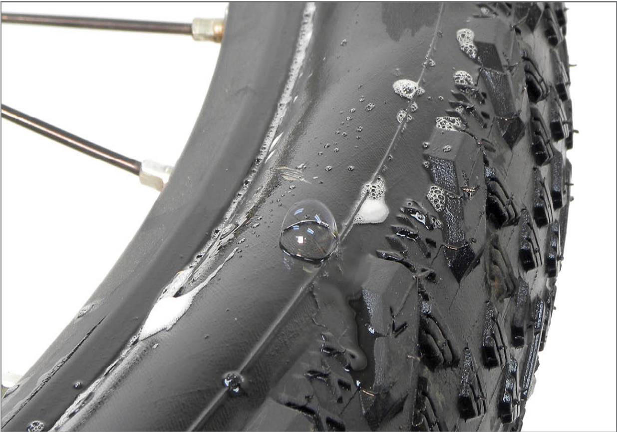
FIGURE 2.60: Bubbles showing air seepage through tire sidewalls of a conversion system
