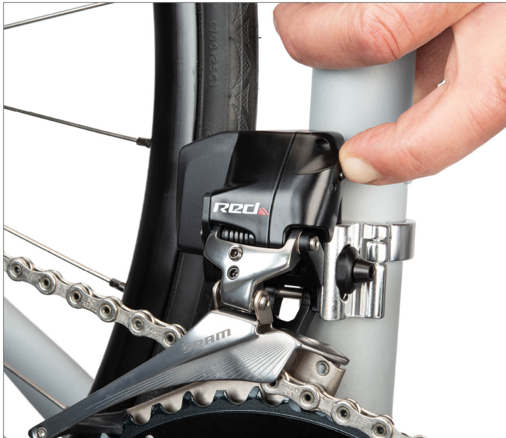
FIGURE 11.21: Use function button on front derailleur body while working on bike in repair stand
