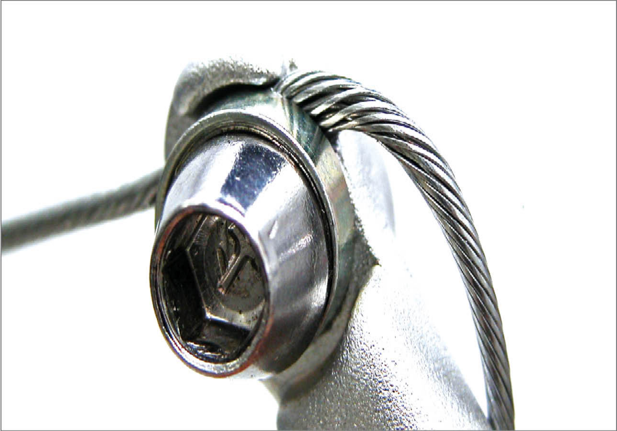
FIGURE 14.15: Pinch bolt will flatten the cable
