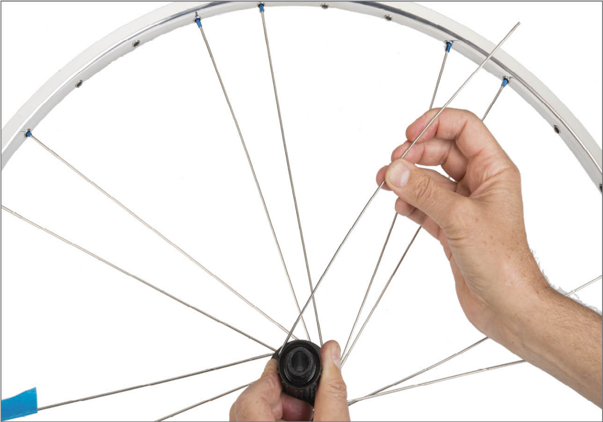
FIGURE 6.20: Third set spokes will radiate opposite direction of previous spokes
