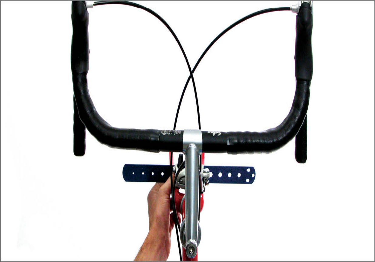
FIGURE 15.15: Straightedge on fork legs is parallel to bar, which indicates aligned stem
