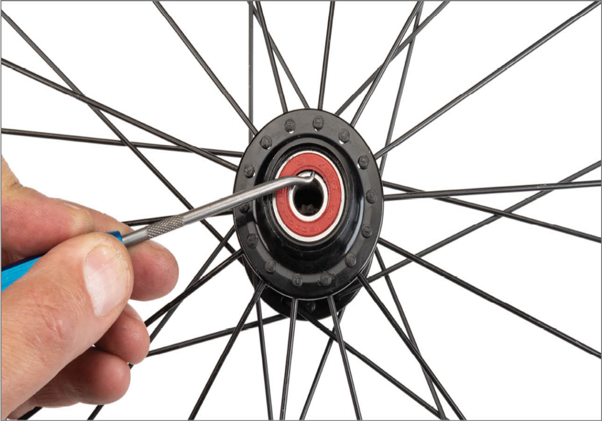
FIGURE 4.19: Remove seal carefully from inner edge
