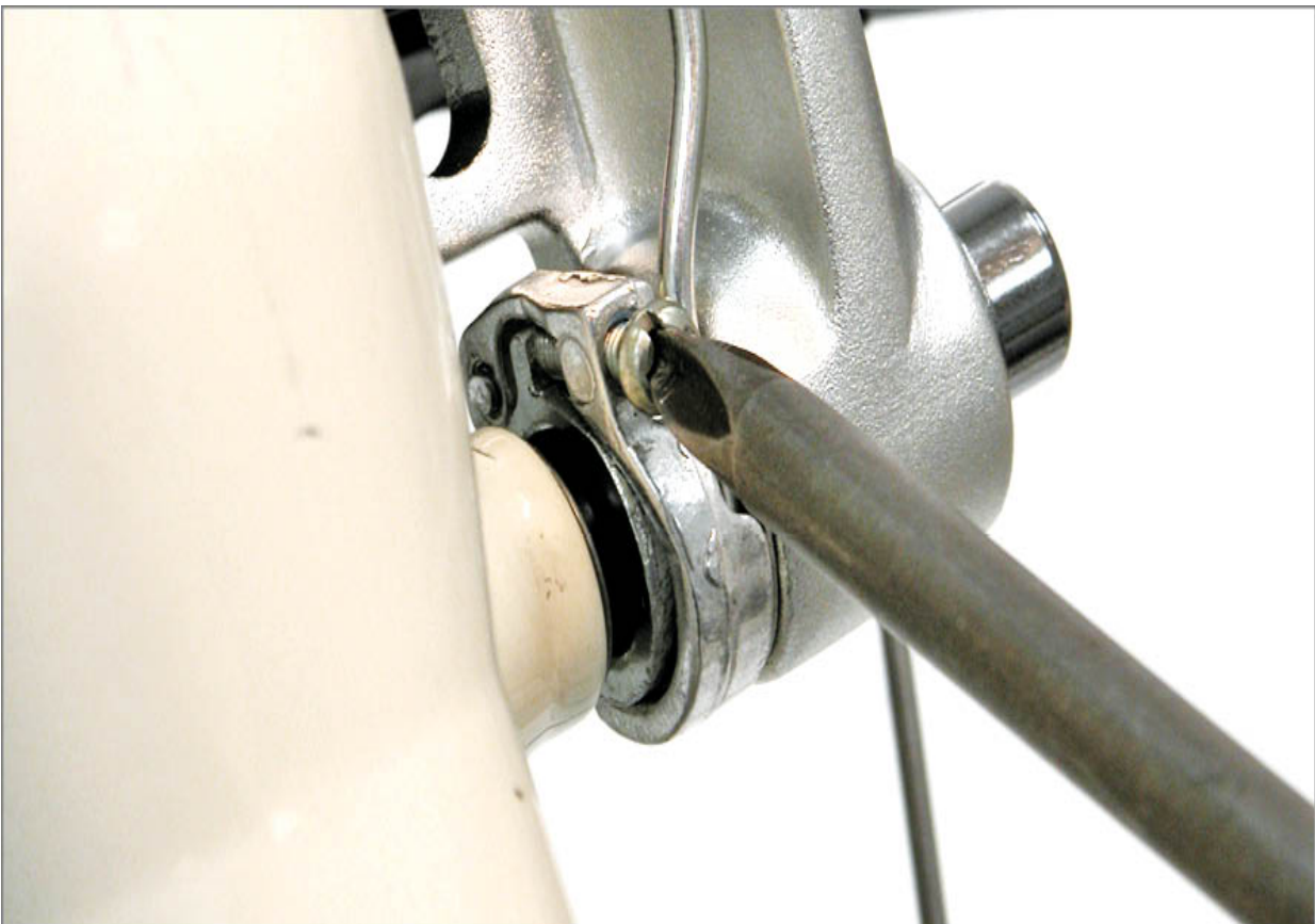
FIGURE 14.32: Use screw to change spring tension when centering pads to rim
