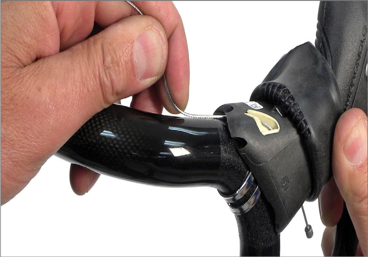
FIGURE 10.26: Cable access is under lever body
