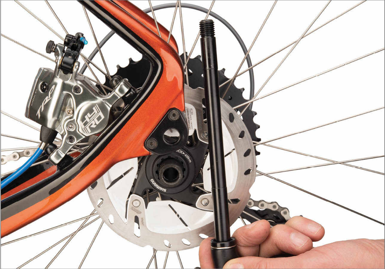
FIGURE 2.12: Rear thru axle wheel being installed
