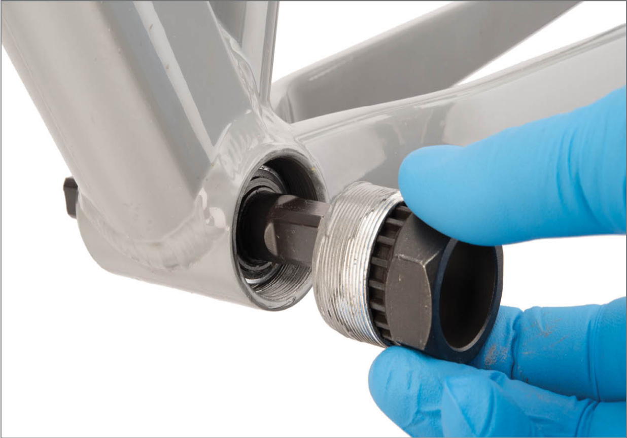
FIGURE 7.61: Secure cartridge bottom bracket main body and adaptor with proper torque
