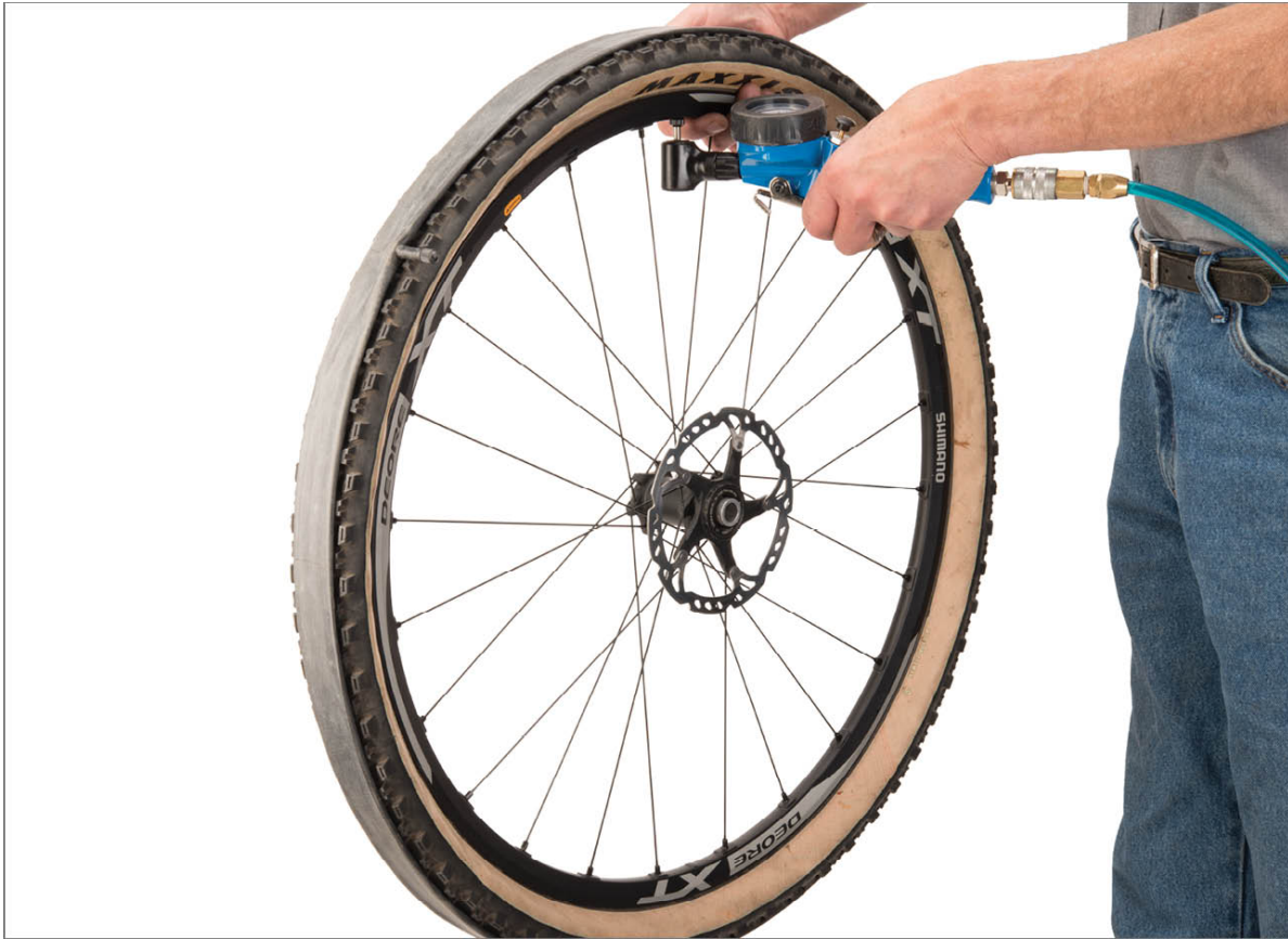
FIGURE 2.54: Use an inner tube as a strap to hold bead to rim
