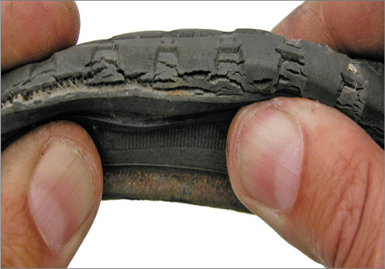
FIGURE 2.27: Cracks in casing or tread indicate tire rot
