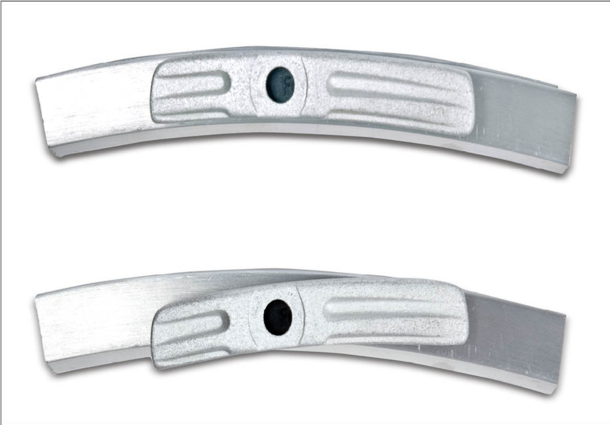
FIGURE 14.24: Top pad showing proper tangent alignment to rim with front and back of pad square to rim. Lower pad showing improperly set pad with front and back of pad not square.
