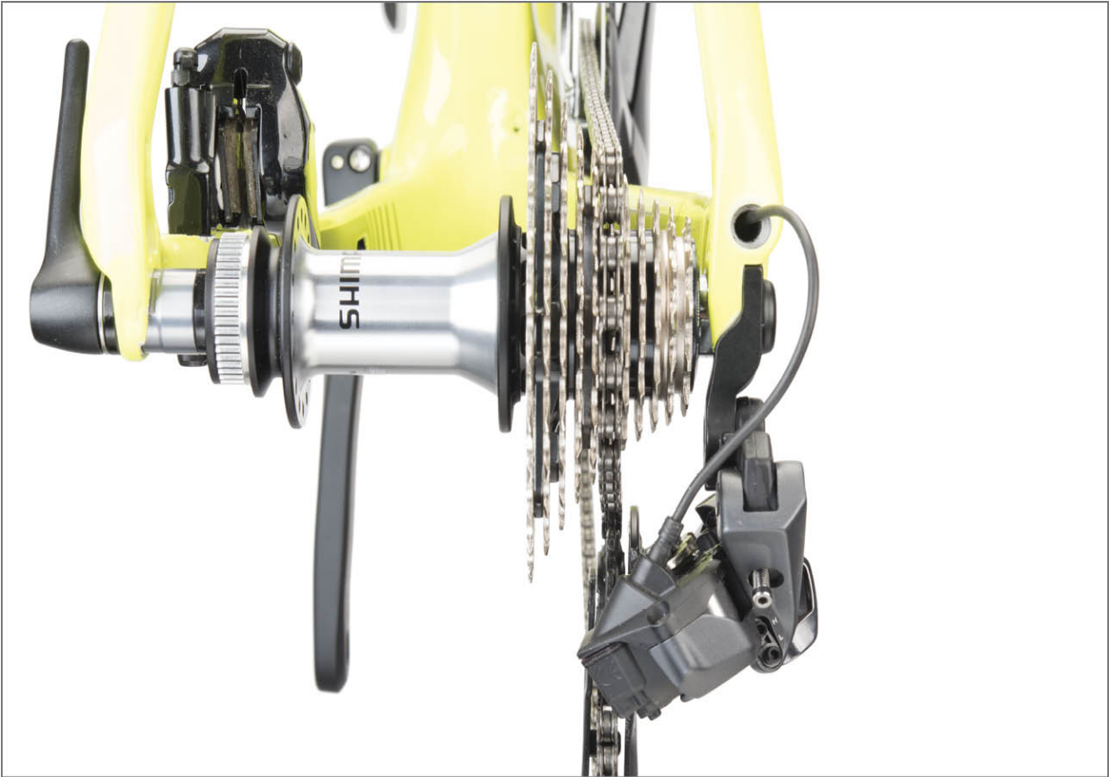
FIGURE 11.13: Shift to middle cogs to adjust rear derailleur
