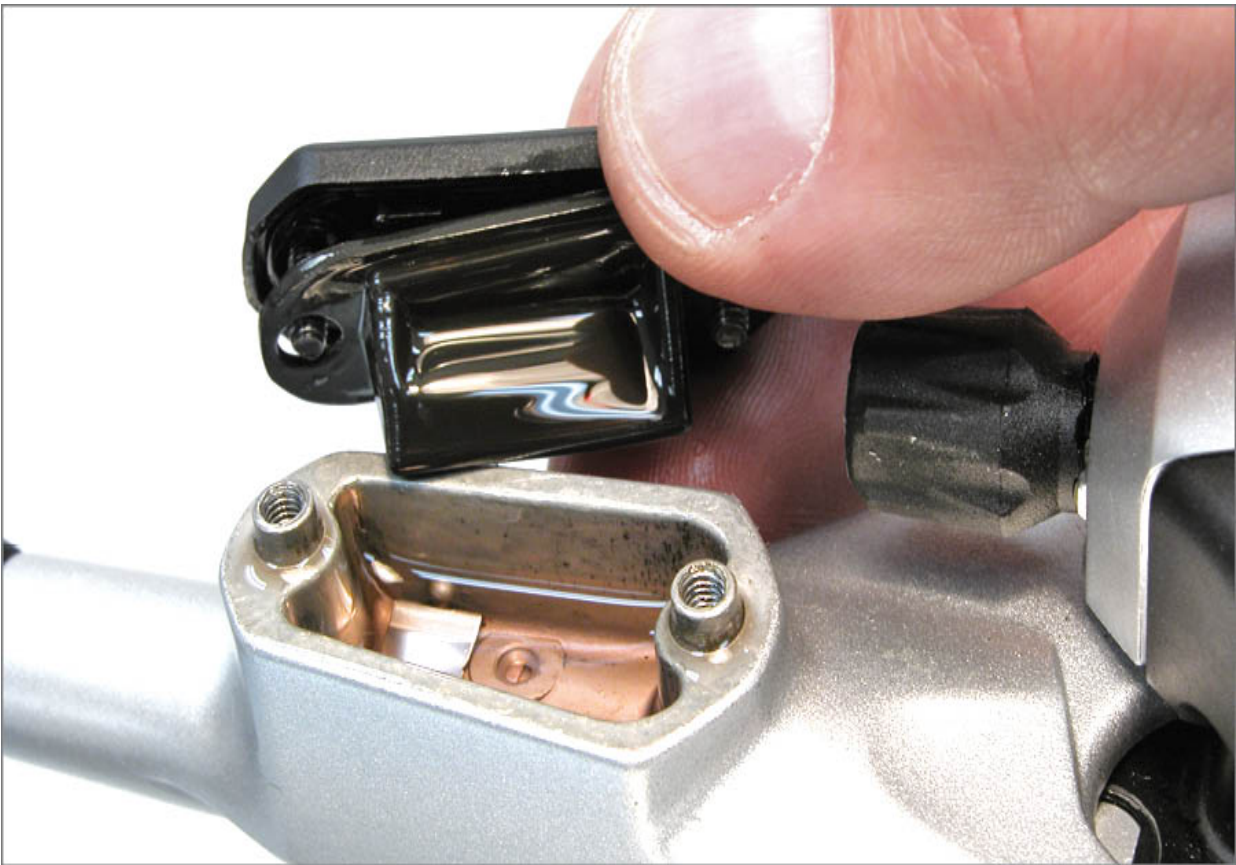
FIGURE 13.19: Reservoir and bladder at brake lever
