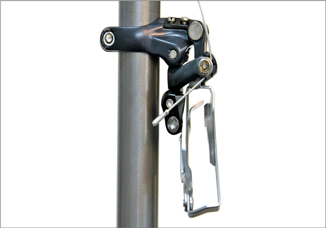
FIGURE 10.35: Bottom swing design with top pull cable
