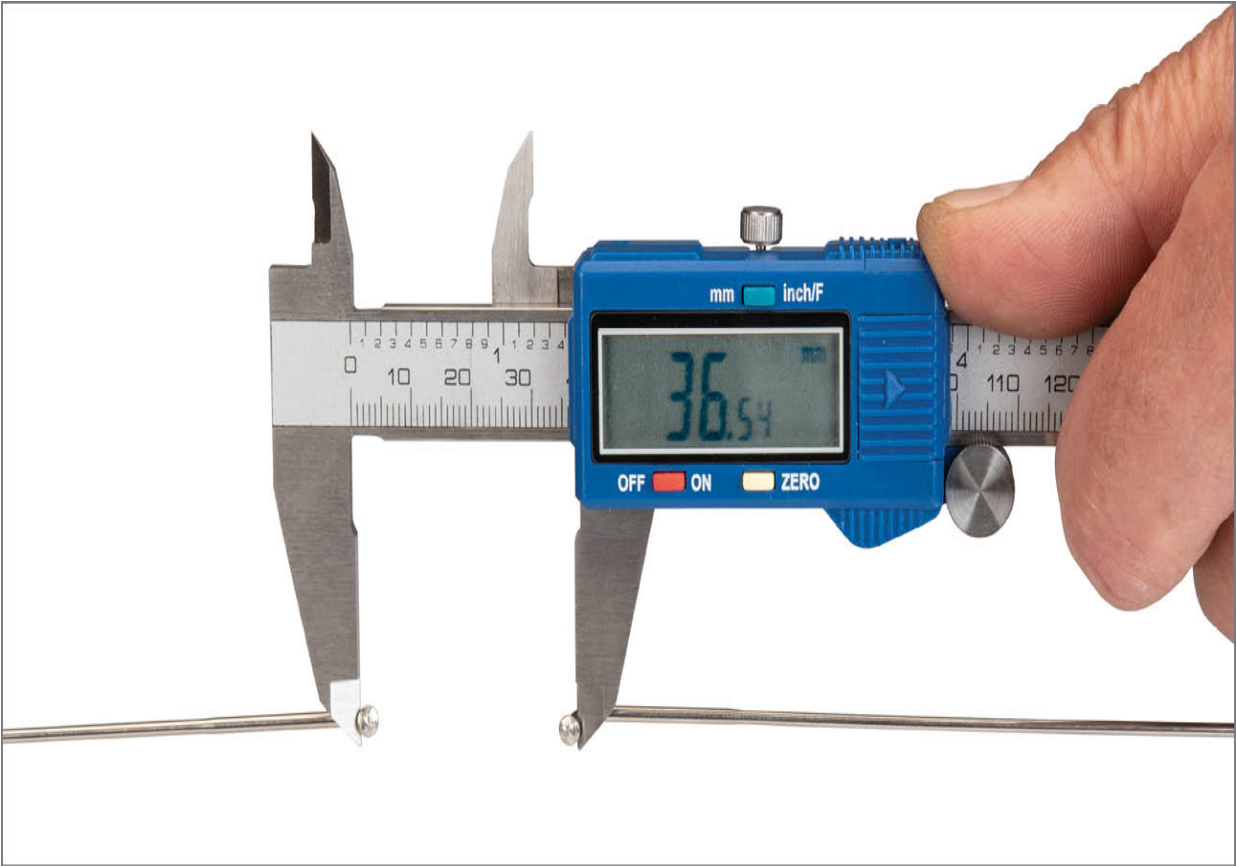
FIGURE 6.12: Measure inside J-bend and add to total length of spokes
