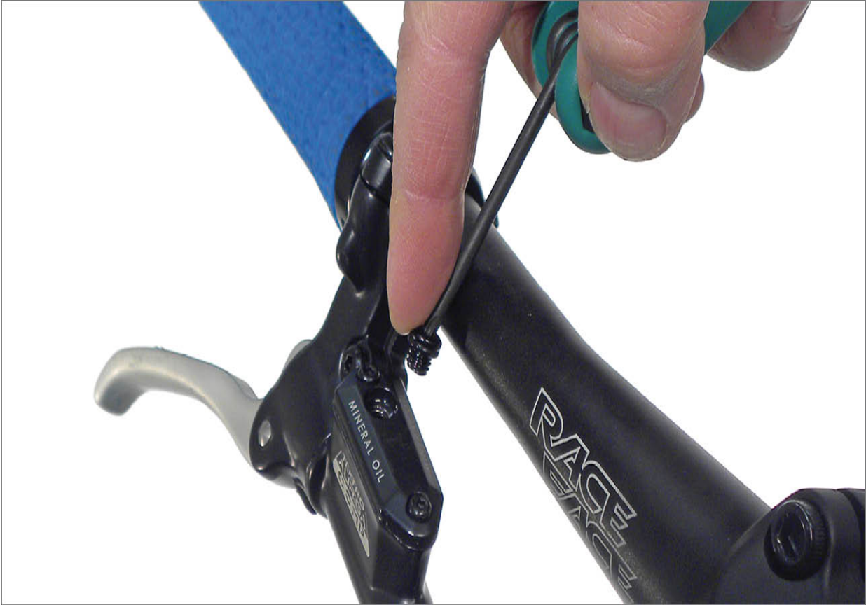
FIGURE 13.59: Remove bleed port screw
