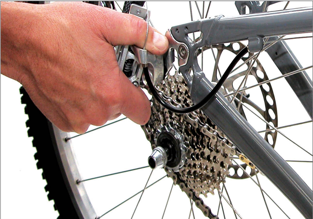
FIGURE 2.67: Pivot derailleur back to clear wheel and cogs
