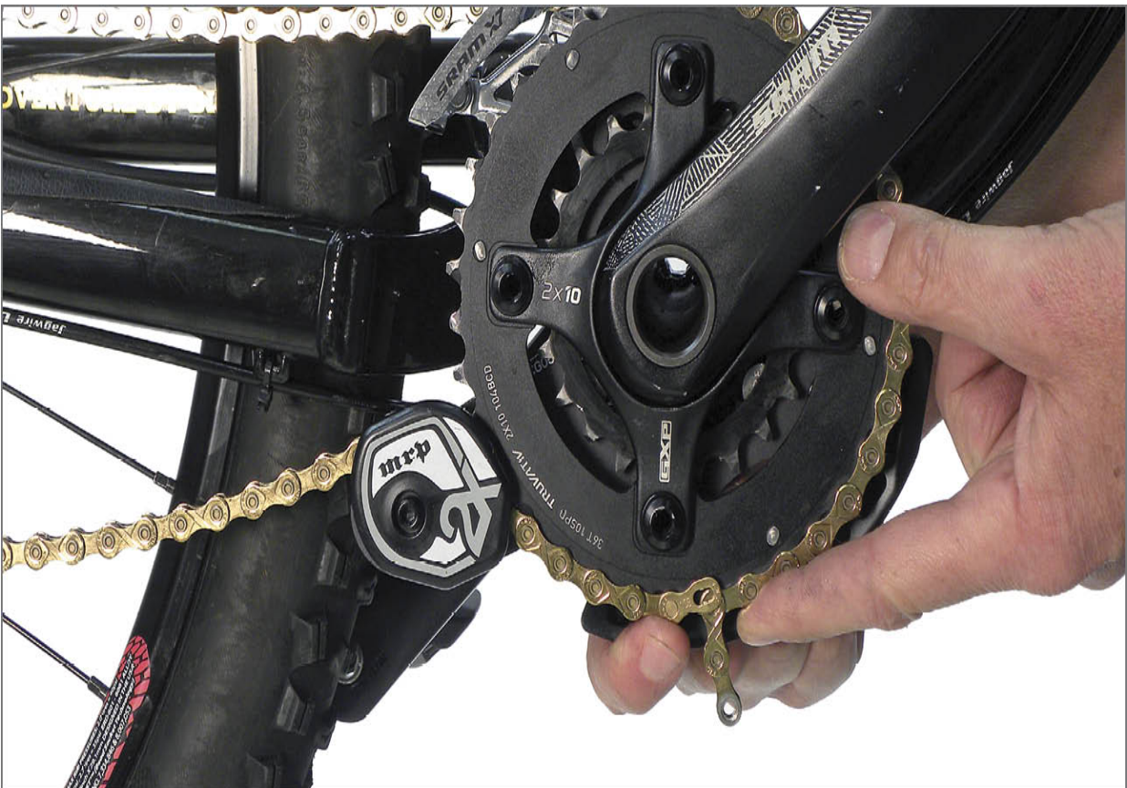
FIGURE 8.9: Engage chain pulley of guide when sizing chain
