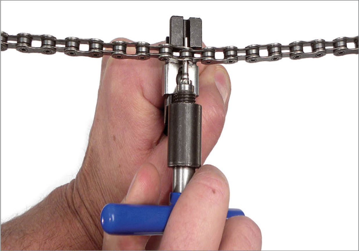
FIGURE 8.11: Driving chain rivet from chain plates
