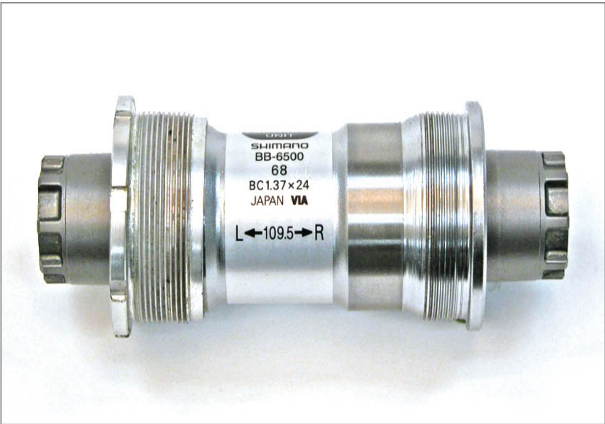
FIGURE 7.31: Bottom bracket marking indicating side of bike
