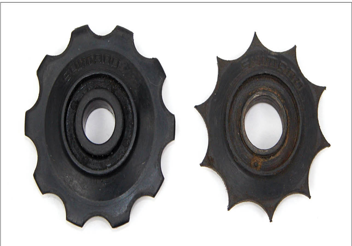
FIGURE 10.77: Unworn pulley wheel on left and extremely worn pulley wheel on right
