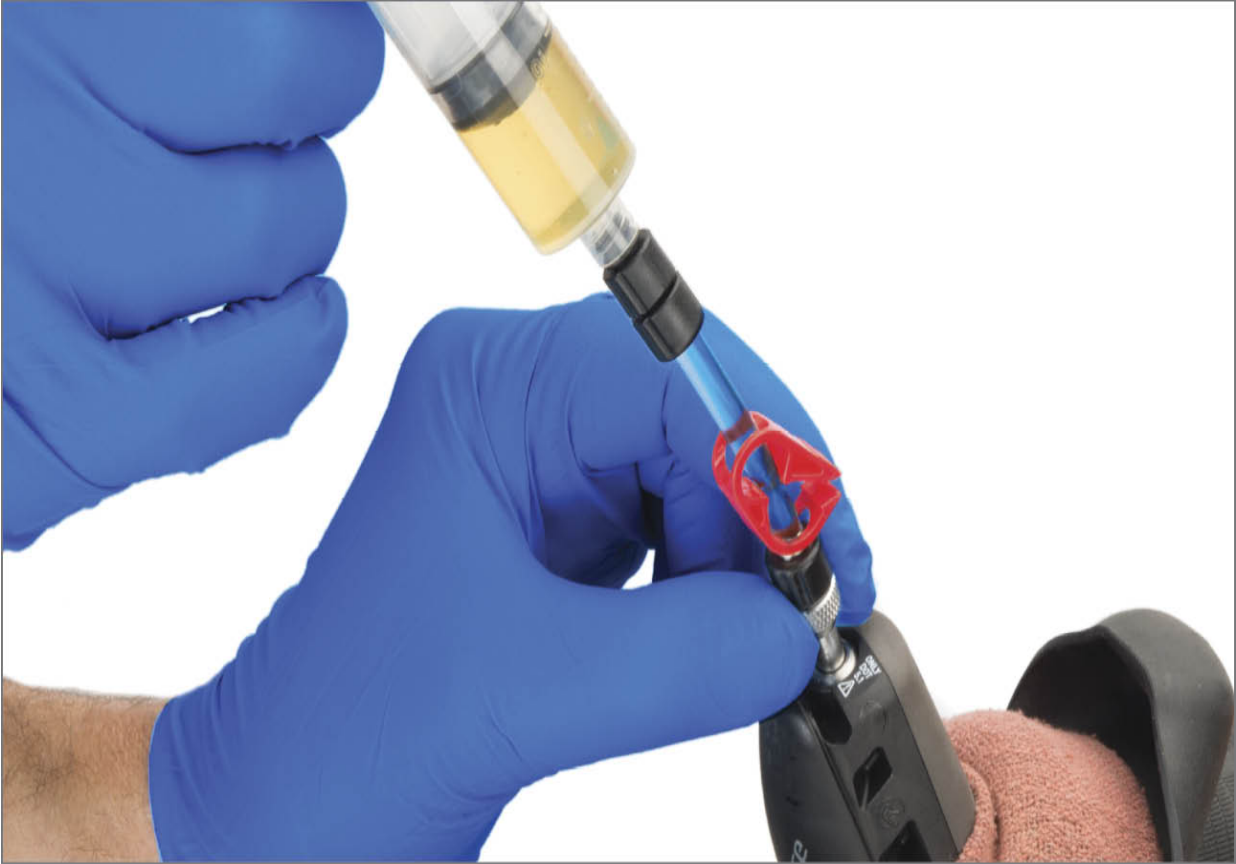
FIGURE 13.49: Thread in syringe at caliper
