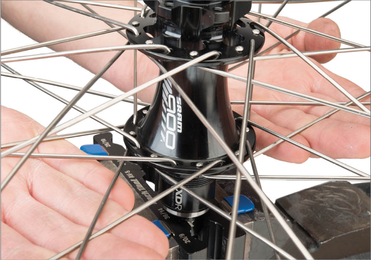
FIGURE 4.20: Use soft jaws in vise to hold end caps while pull up on wheel
