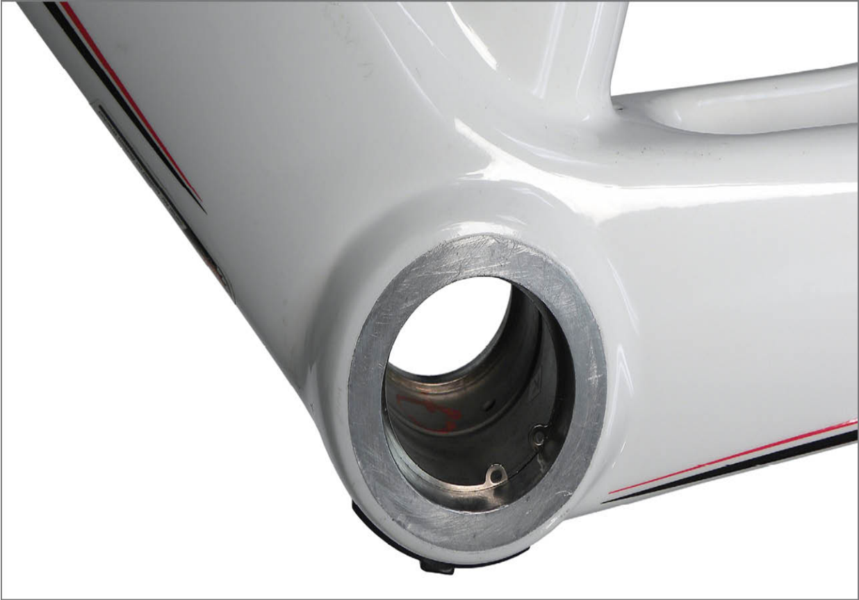
FIGURE 7.34: BB30 shell with C-clip bearing stops in place
