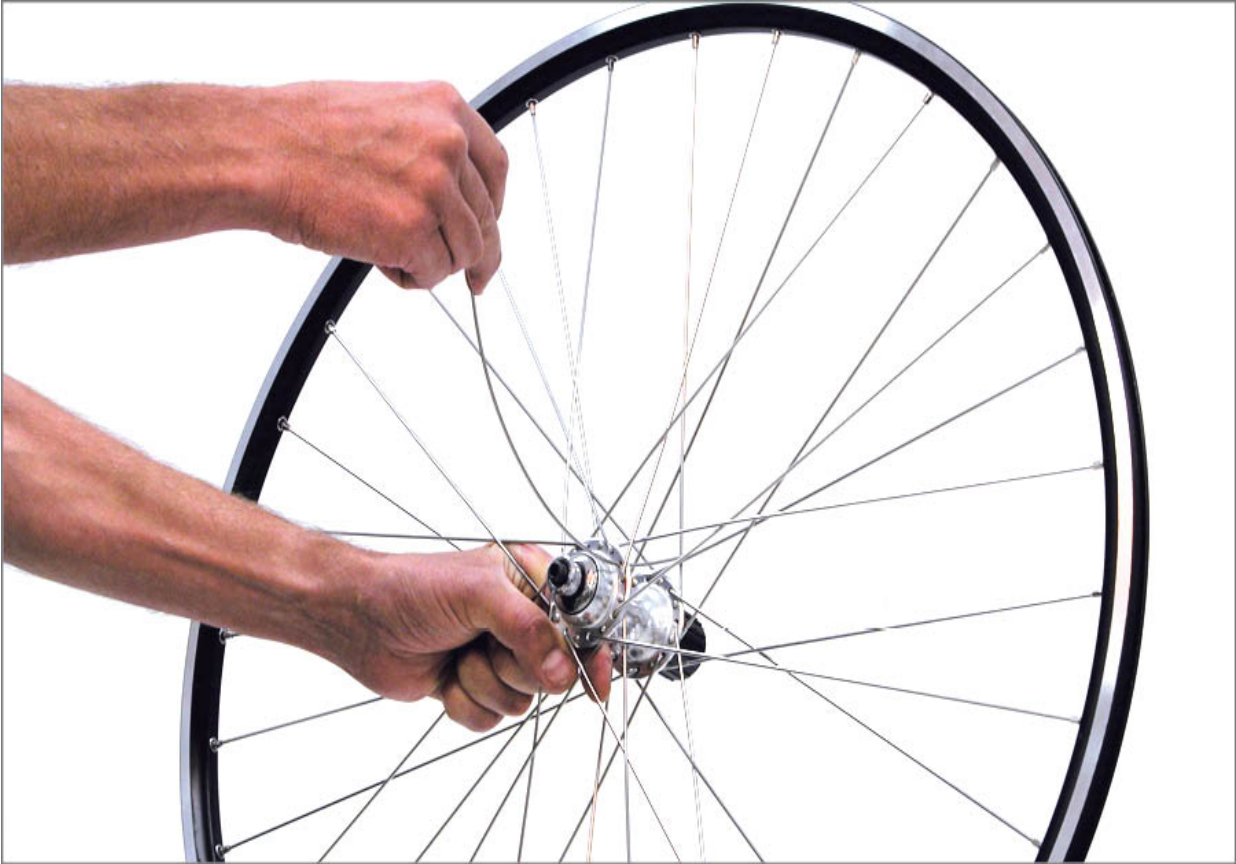
FIGURE 5.27: Flex spoke as needed to lace into wheel
