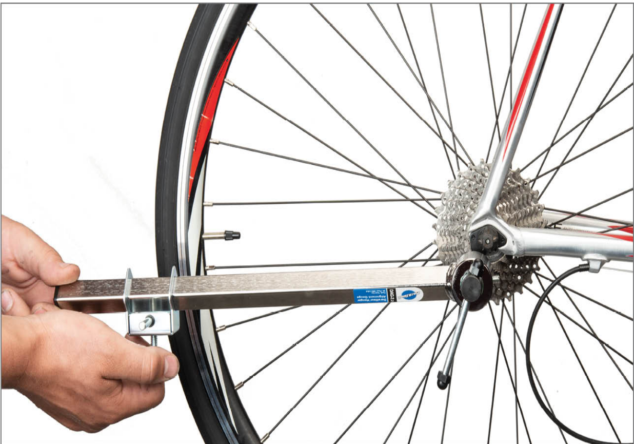
FIGURE 10.70: Set DAG-2.2 gauge to reference rim at the nine o’clock position
