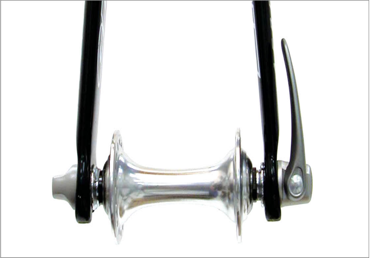
FIGURE 2.64: Closed skewer lever should be parallel to center plane of bike
