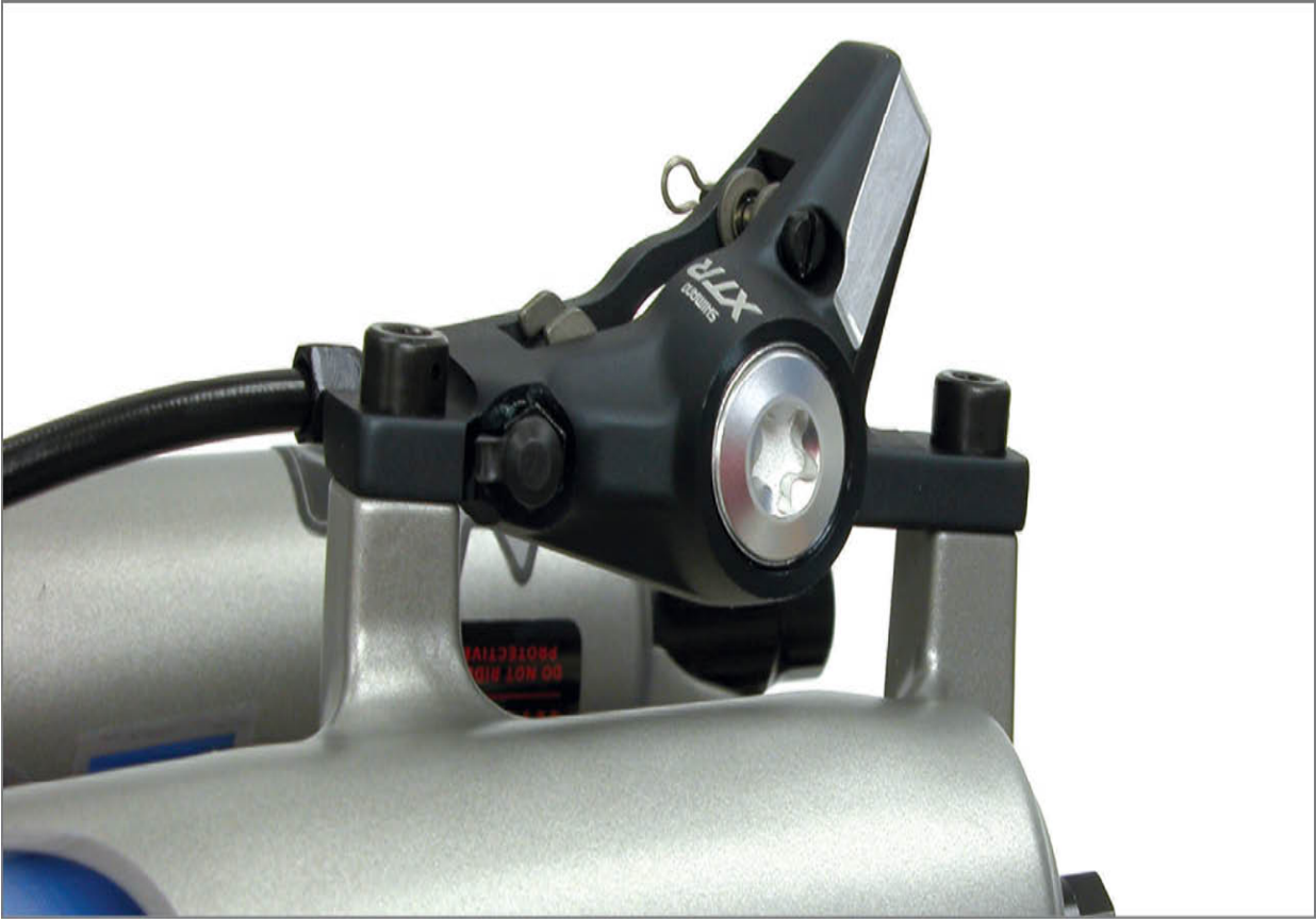
FIGURE 13.4: Post Mount (PM) system on compatible fork
