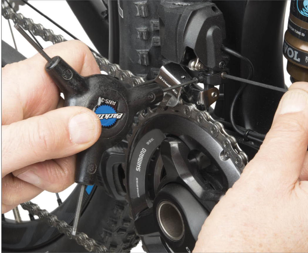
FIGURE 11.12: Position front derailleur to 0.5mm gap after unlocking cage fixing bolt in front
