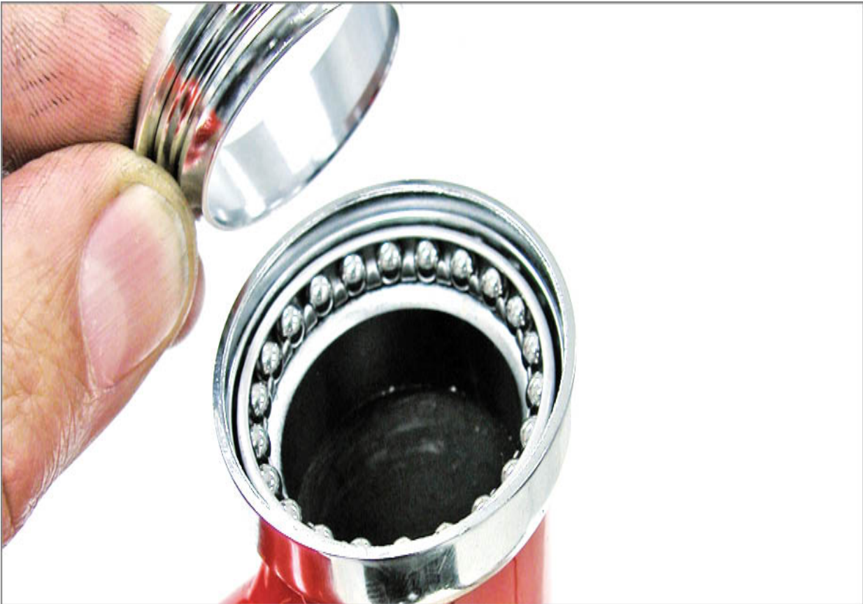
FIGURE 16.11: Open side of cage should face cone-shape of race
