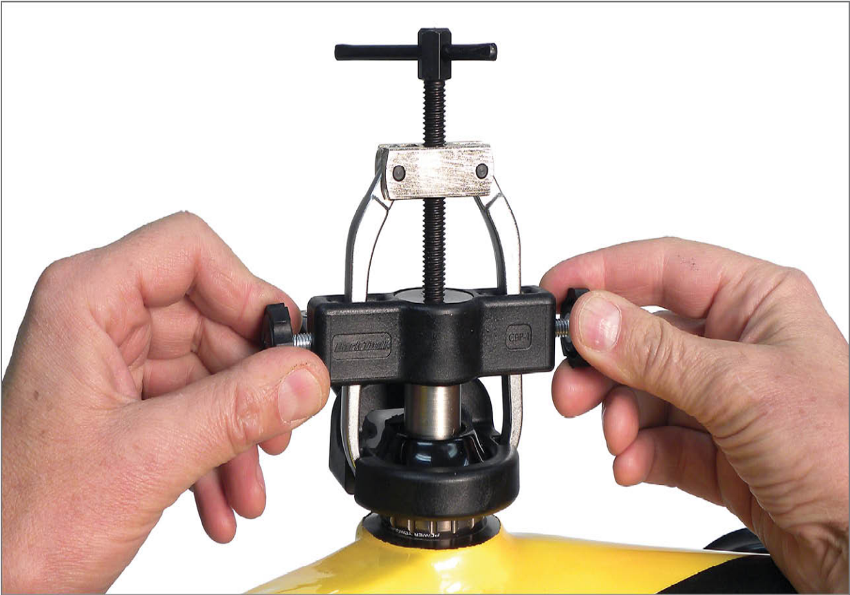
FIGURE 7.27: Engage caliper fingers and secure knobs to remove play
