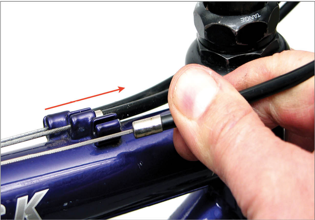
FIGURE 10.11: Remove housing from frame stops to clean and lubricate
