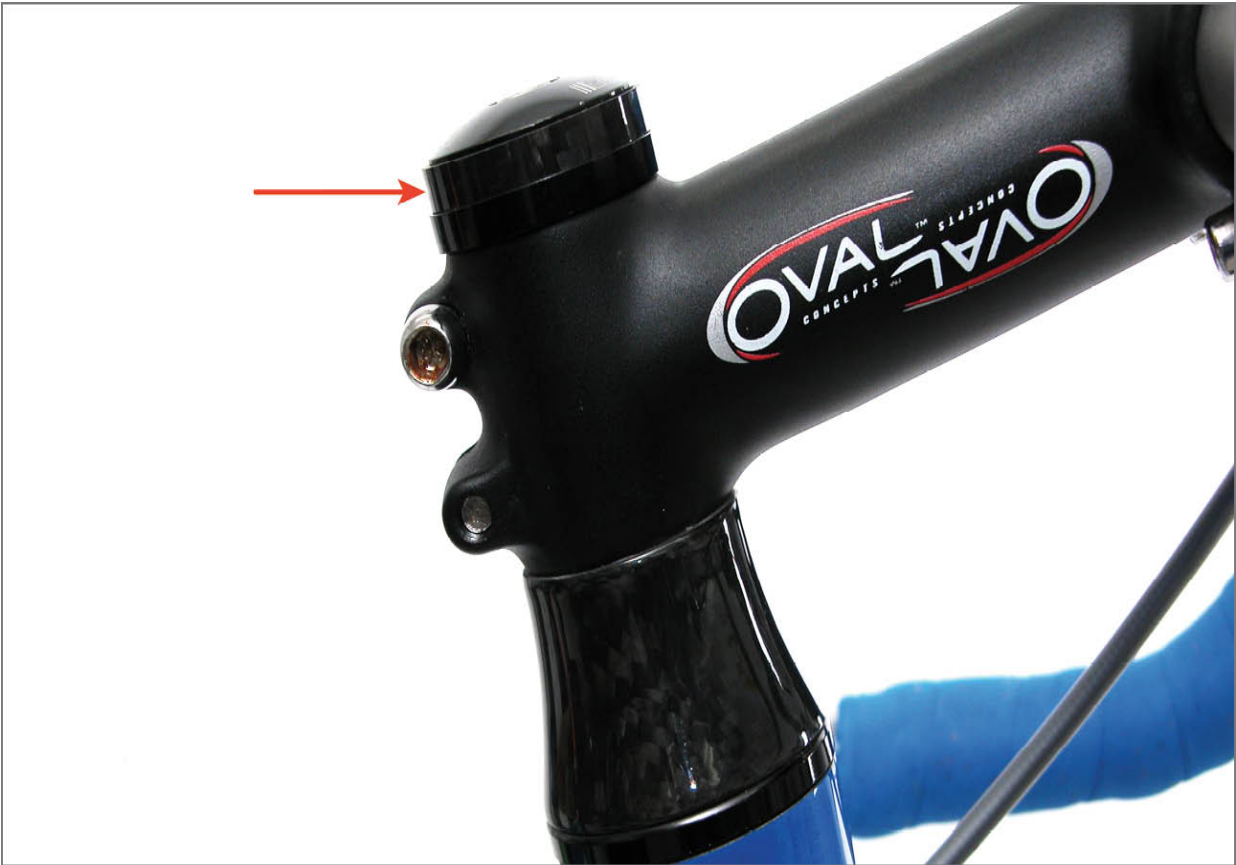
FIGURE 16.13: Spacer added to increase clearance between top cap and column top
