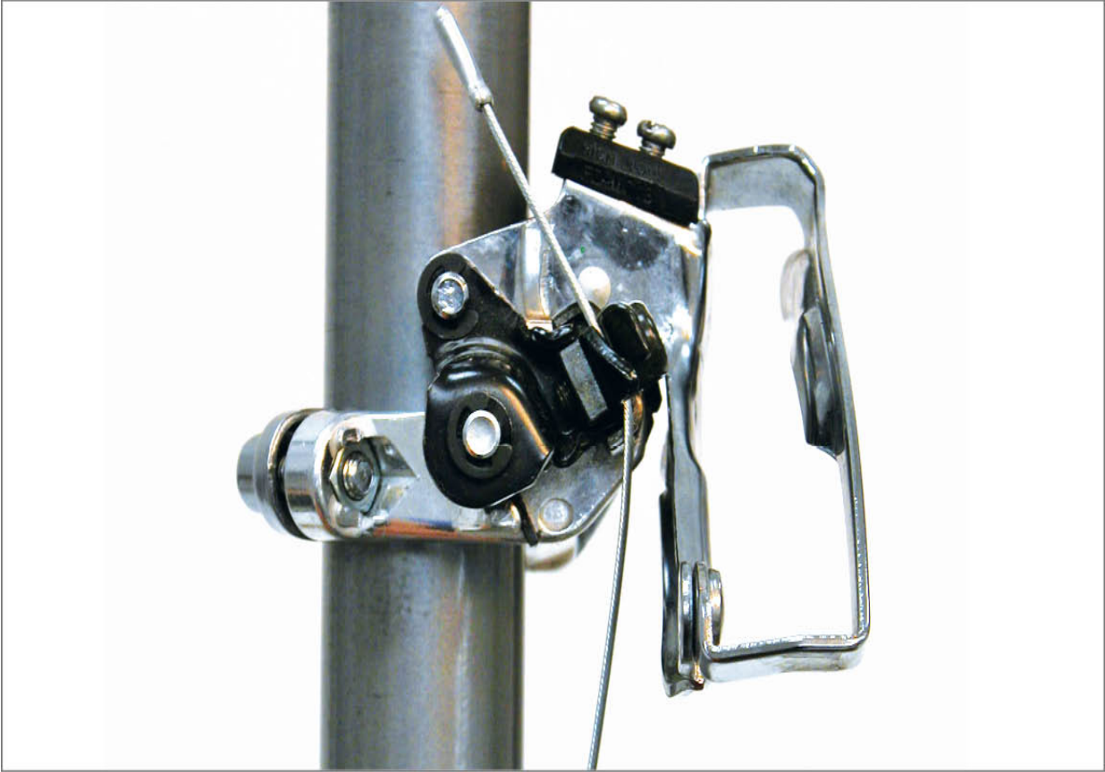
FIGURE 10.36: Top swing cage design with bottom cable pull
