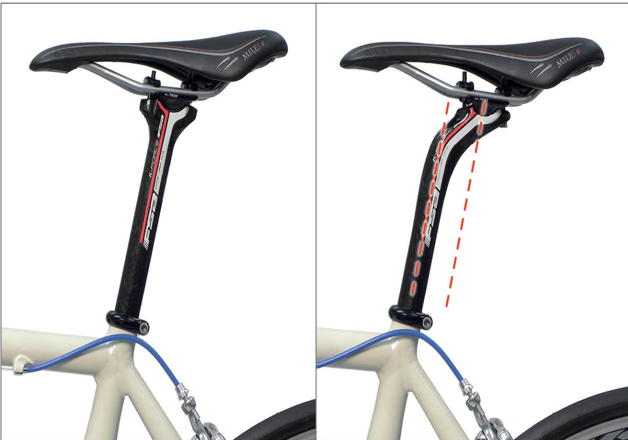
FIGURE 15.23: Post on the left has no offset; post on the right has 32mm offset
