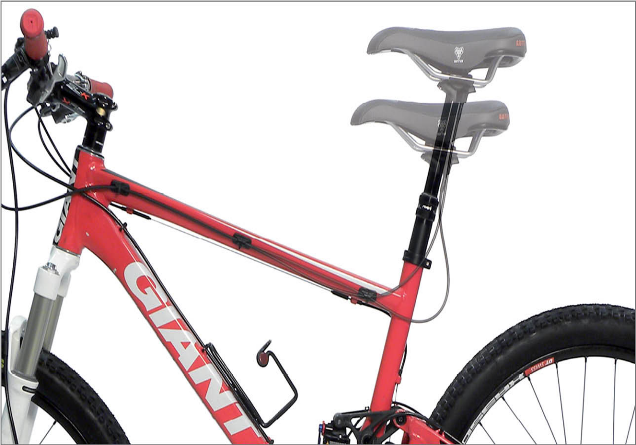
FIGURE 15.29: Range of height options for an adjustable height seat post
