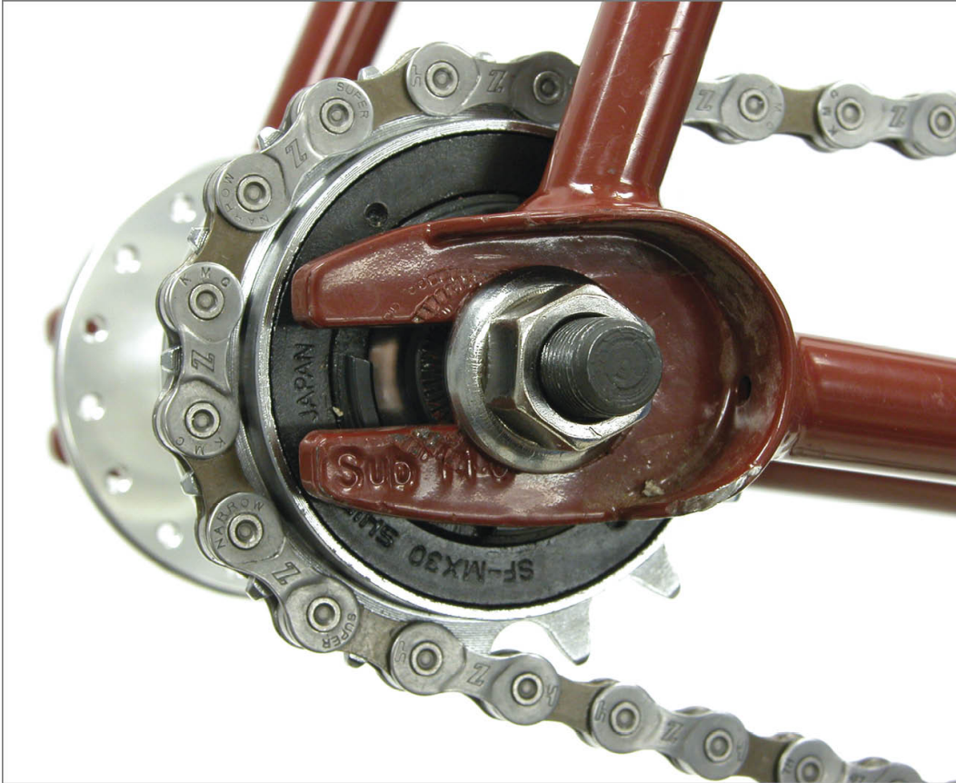
FIGURE 2.73: Solid axle in a horizontal dropout
