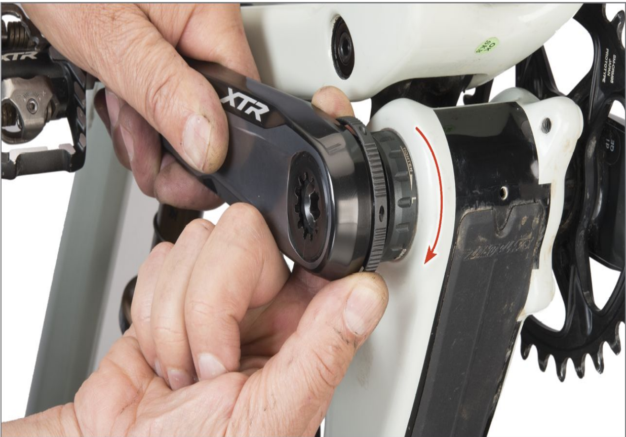
FIGURE 7.19: Use adjuster ring to remove any crank movement relative to bearings
