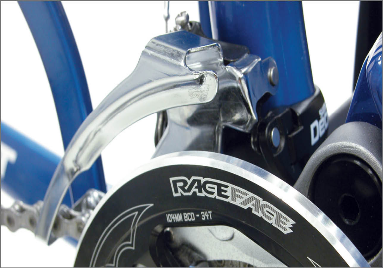
FIGURE 10.42: Chain guards can sometimes prevent good derailleur height
