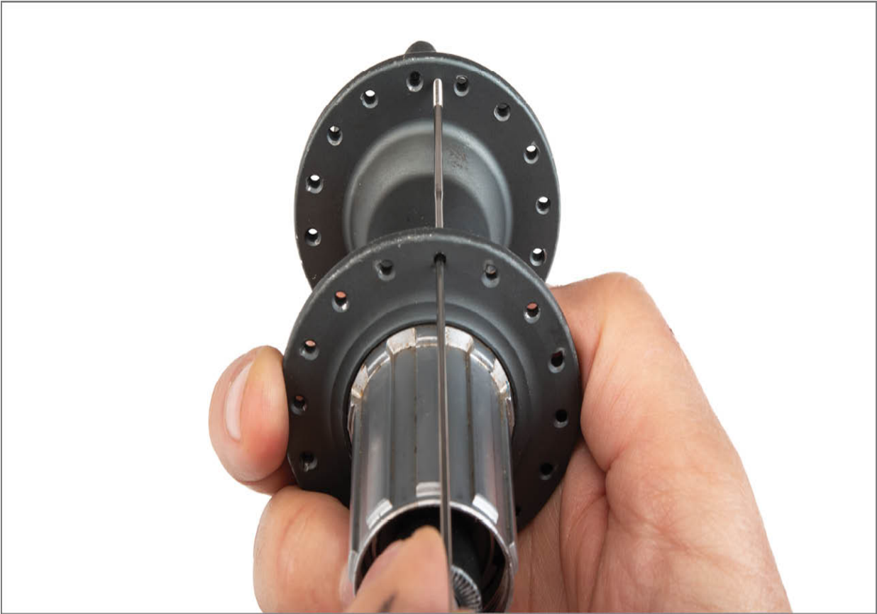
FIGURE 6.8: Hub flange spoke hole alignment is offset left-to-right
