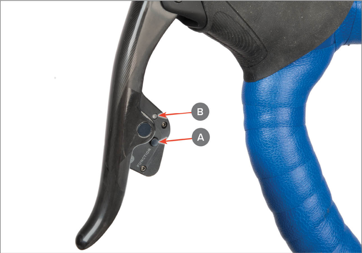
FIGURE 11.19: Function button (A) and indicator button (B)
