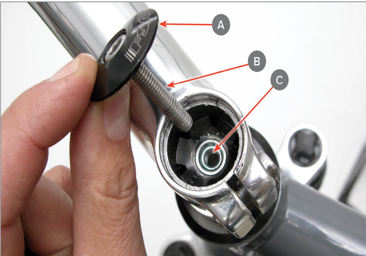
FIGURE 16.16: Threadless stem with (A) top cap, (B) adjusting bolt, (C) star nut in column
