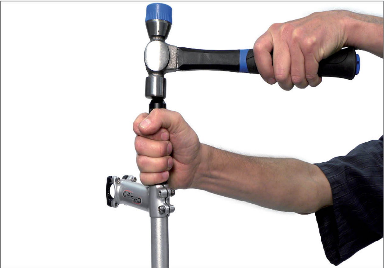
FIGURE 16.34: Using a stem to help align TNS-1 and star nut
