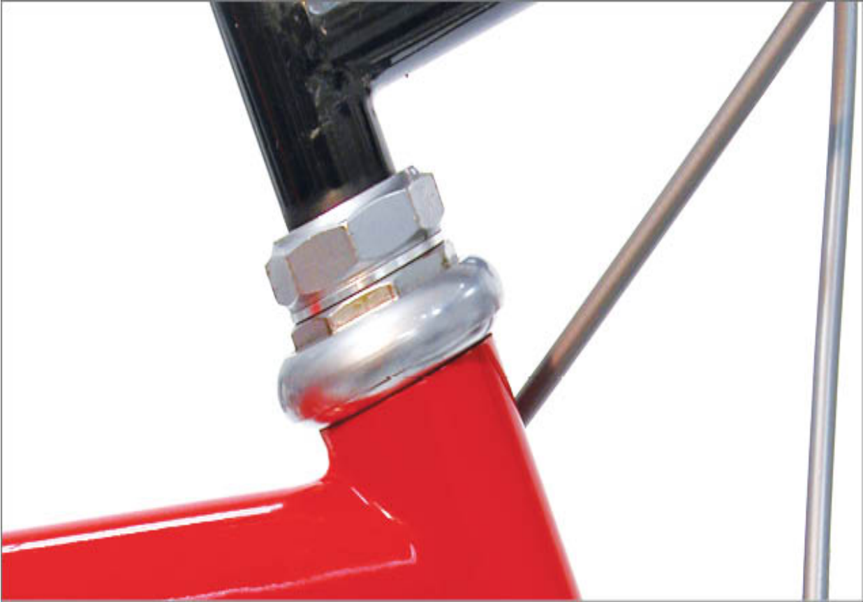
FIGURE 16.2: External cups (EC) of a threaded headset with quill stem installed
