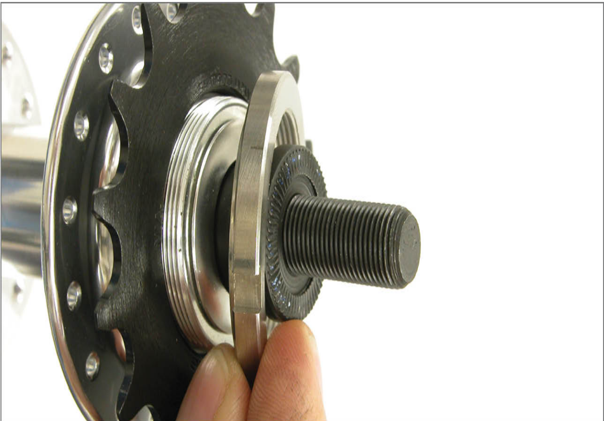
FIGURE 3.18: Lockring and single speed fixed gear cog
