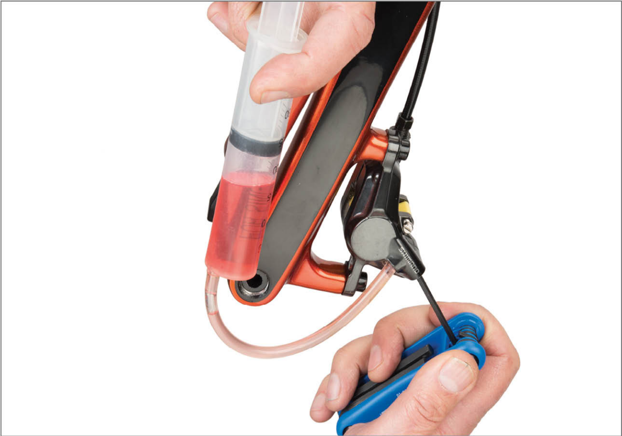
FIGURE 13.33: Internal caliper bleed nipple open with hex key
