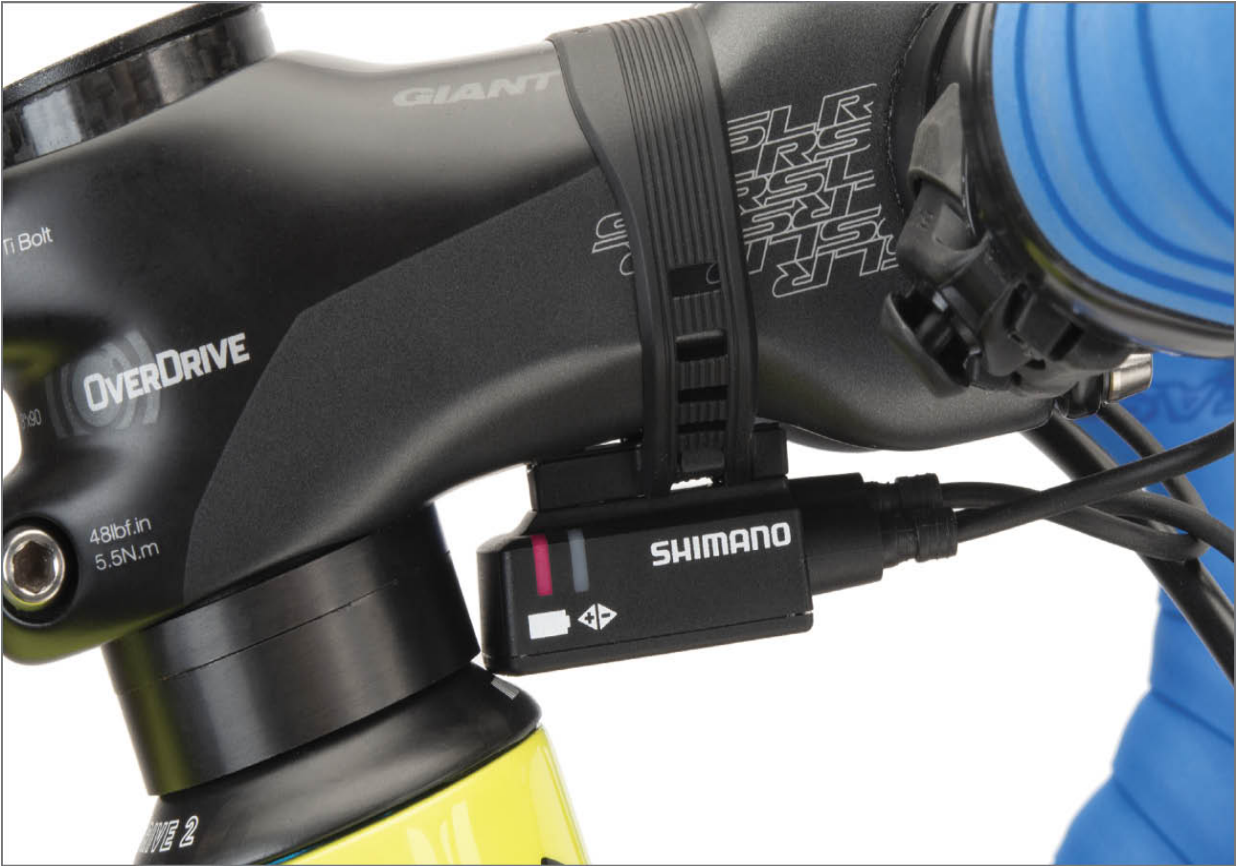
FIGURE 11.8: Press Y-switch and watch for lights at junction box
