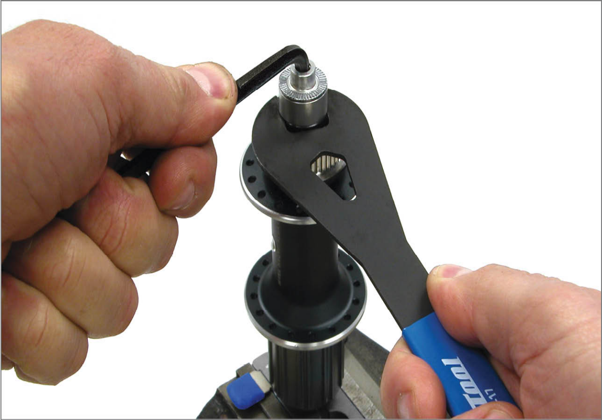
FIGURE 4.8: Loosen any left-side locknut
