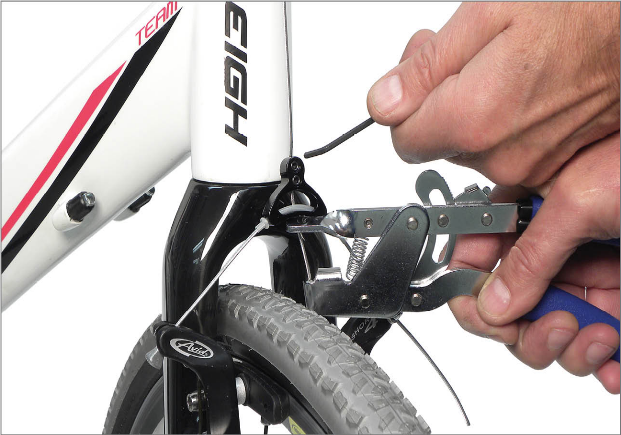
FIGURE 14.40: Use primary cable carrier to bring pads to rim
