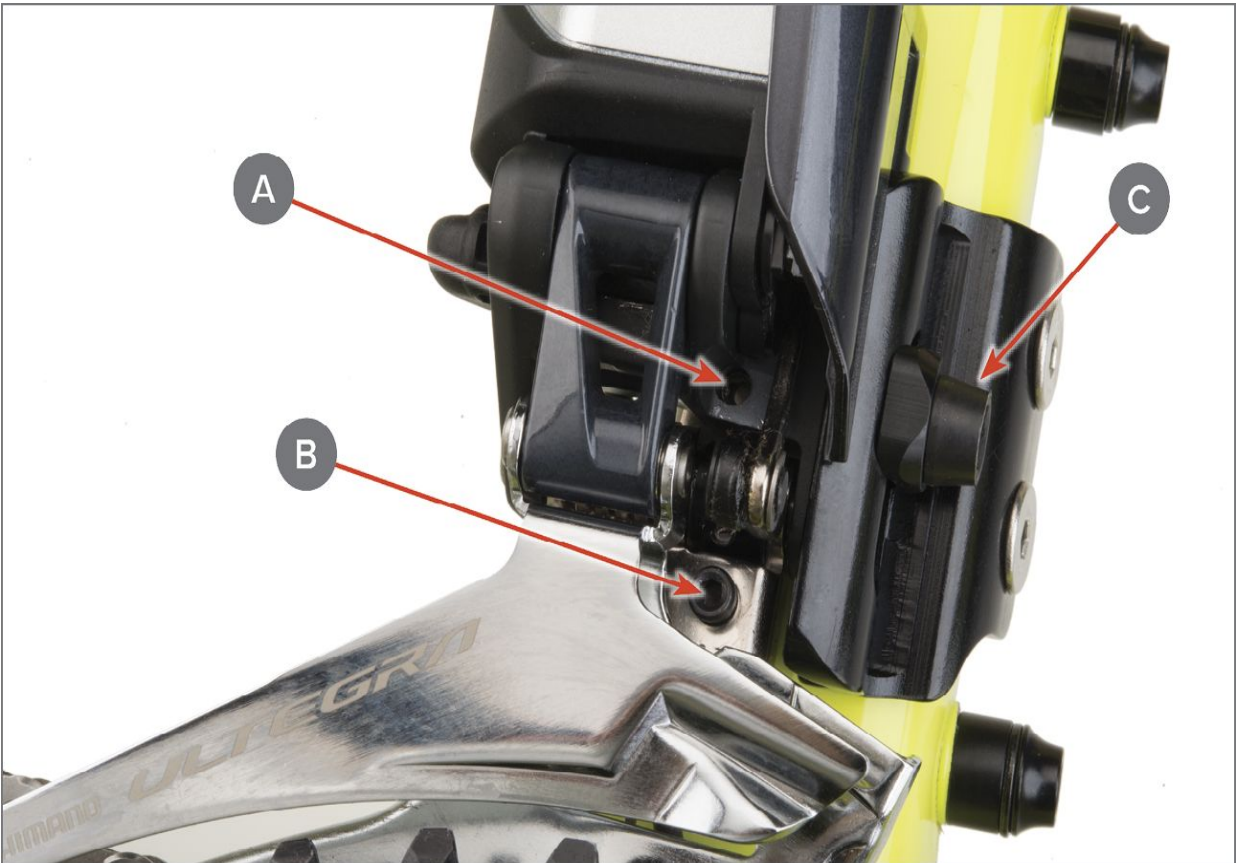
FIGURE 11.9: Front derailleur and adjustment screws: (A) rotation adjustment screw, (B) H-adjustment screw, (C) height adjustment screw
