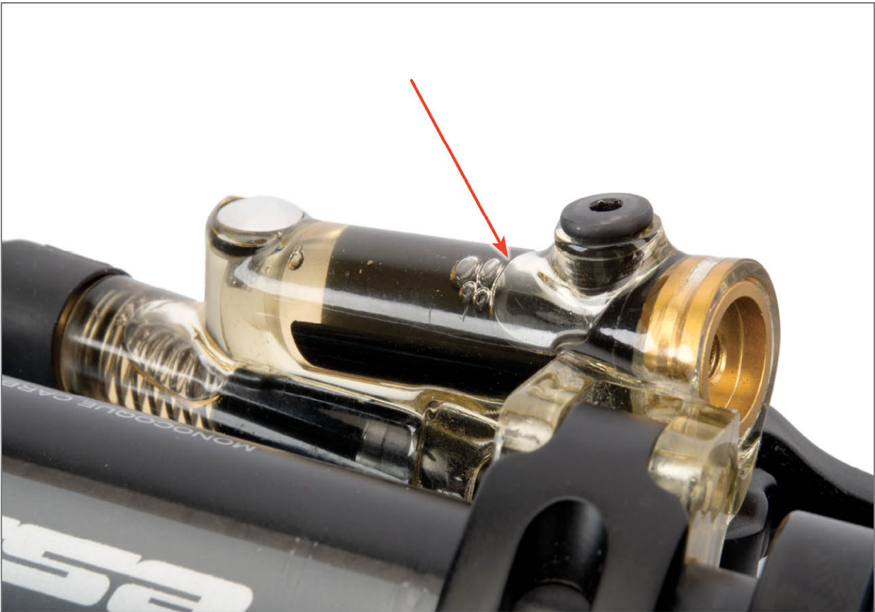
FIGURE 13.25: Air bubble seen inside clear model of brake lever
