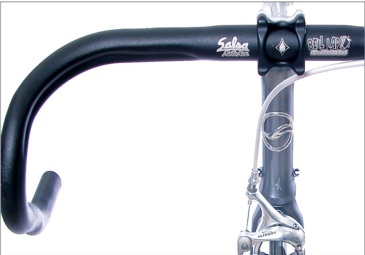
FIGURE 14.9: Housing enters stop in a straight line, indicating a good length
