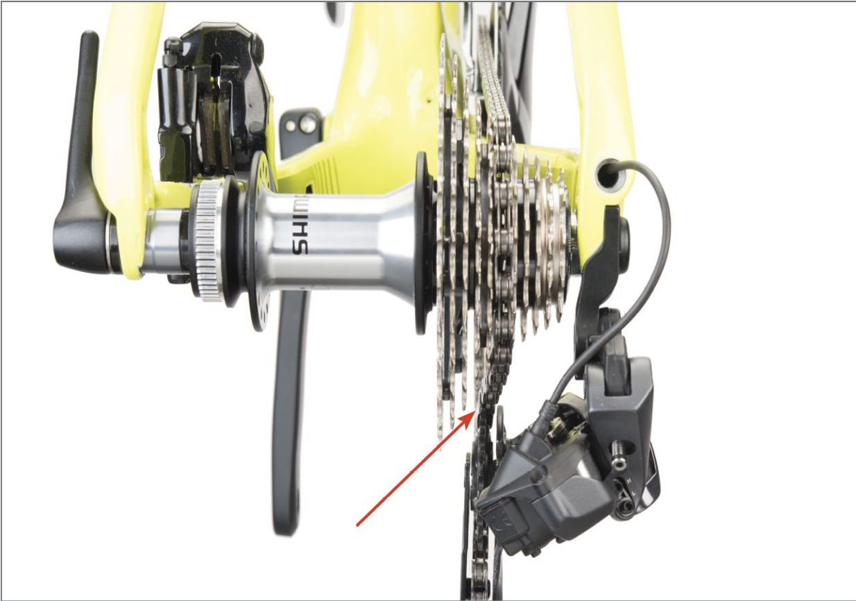
FIGURE 11.16: Use adjustment mode to intentionally move cage too far inward, then move back outward until quiet
