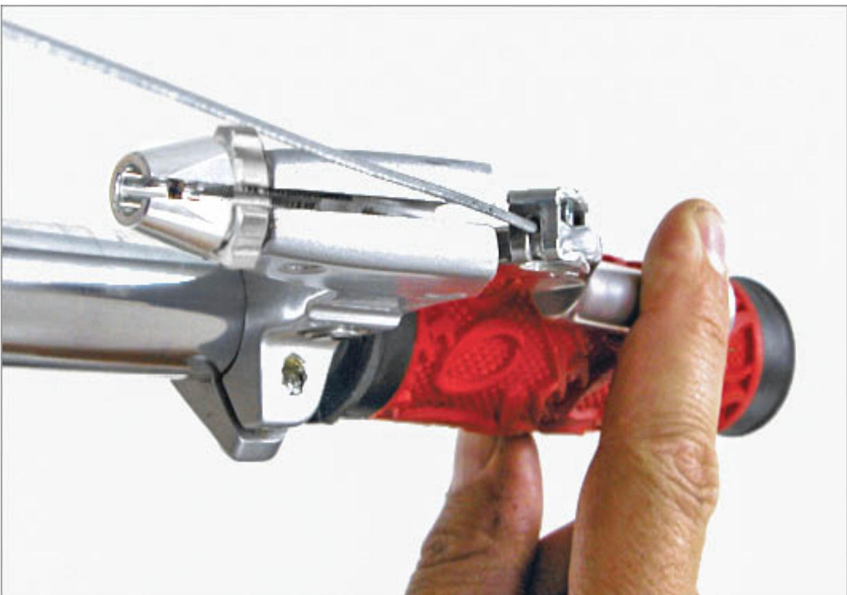
FIGURE 14.2: Use slots in lever body to engage and disengage cable end
