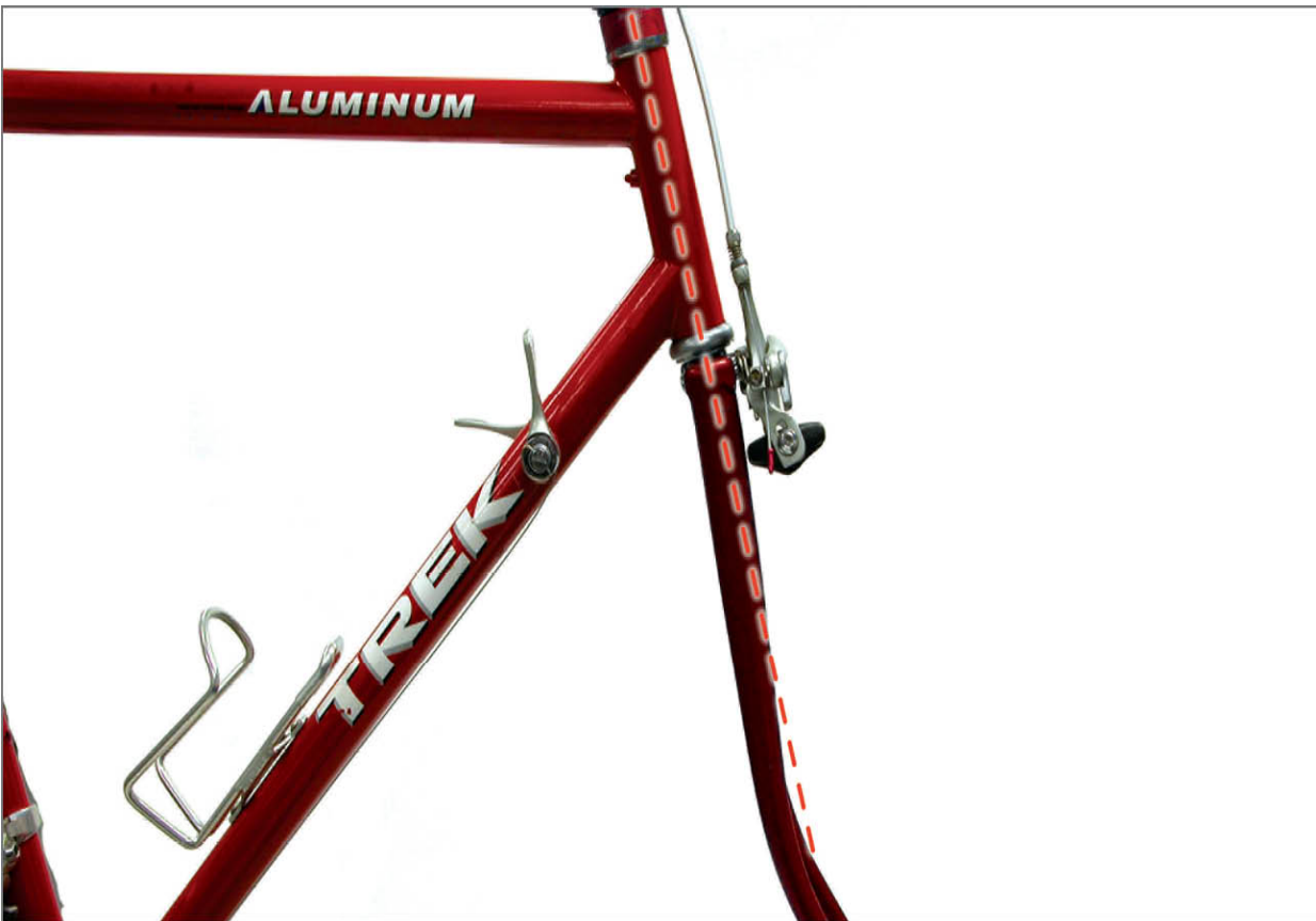
FIGURE 17.2: Bent front fork blades
