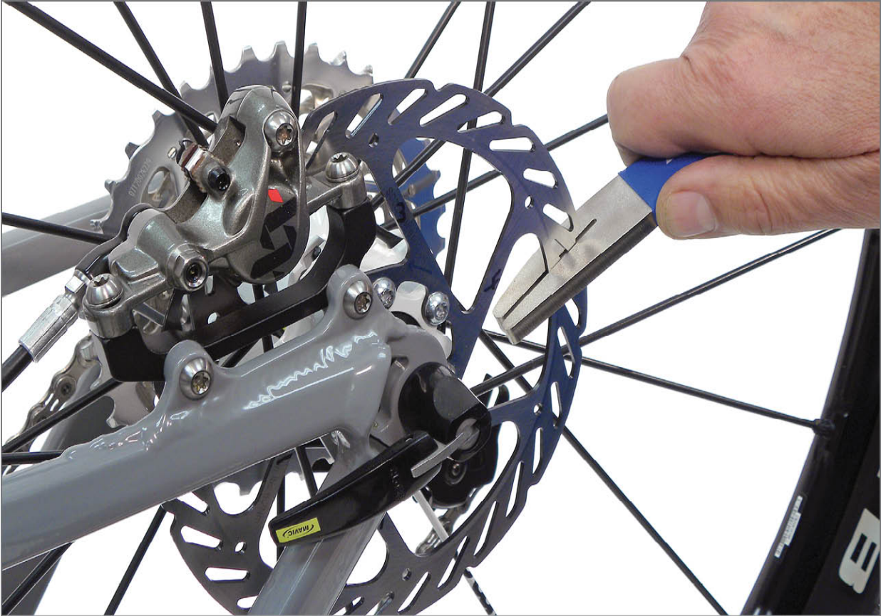
FIGURE 13.17: Move area to be rebent away from caliper body before bending rotor left or right
