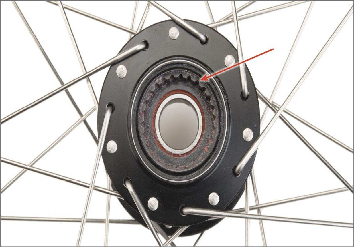
FIGURE 4.24: Swiss® ratchet rings require a proprietary tool from the manufacturer for disassembly
