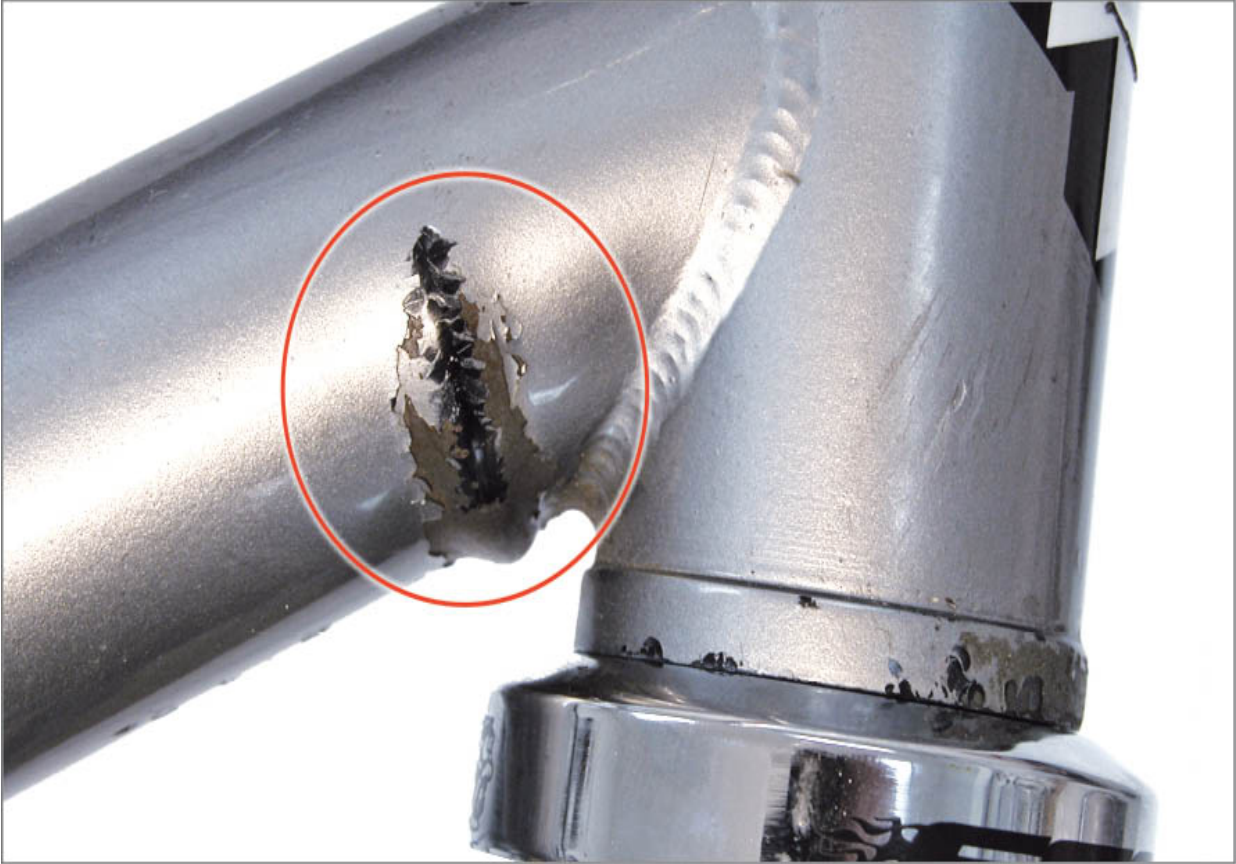
FIGURE 17.6: Bent tubing on down tube from impact
