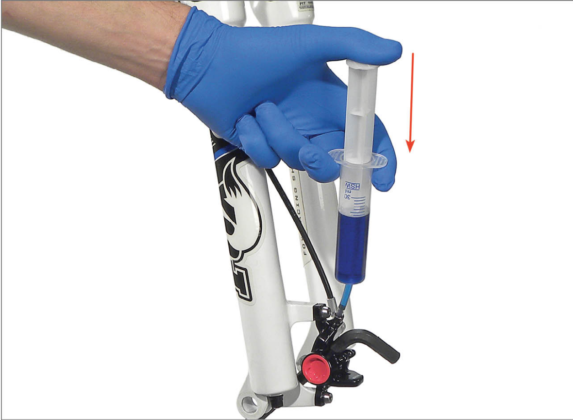
FIGURE 13.38: Push fluid from caliper upward to lever
