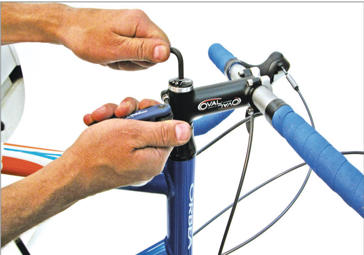
FIGURE 16.17: Make bearing adjustment at top cap only when stem binder are loose
