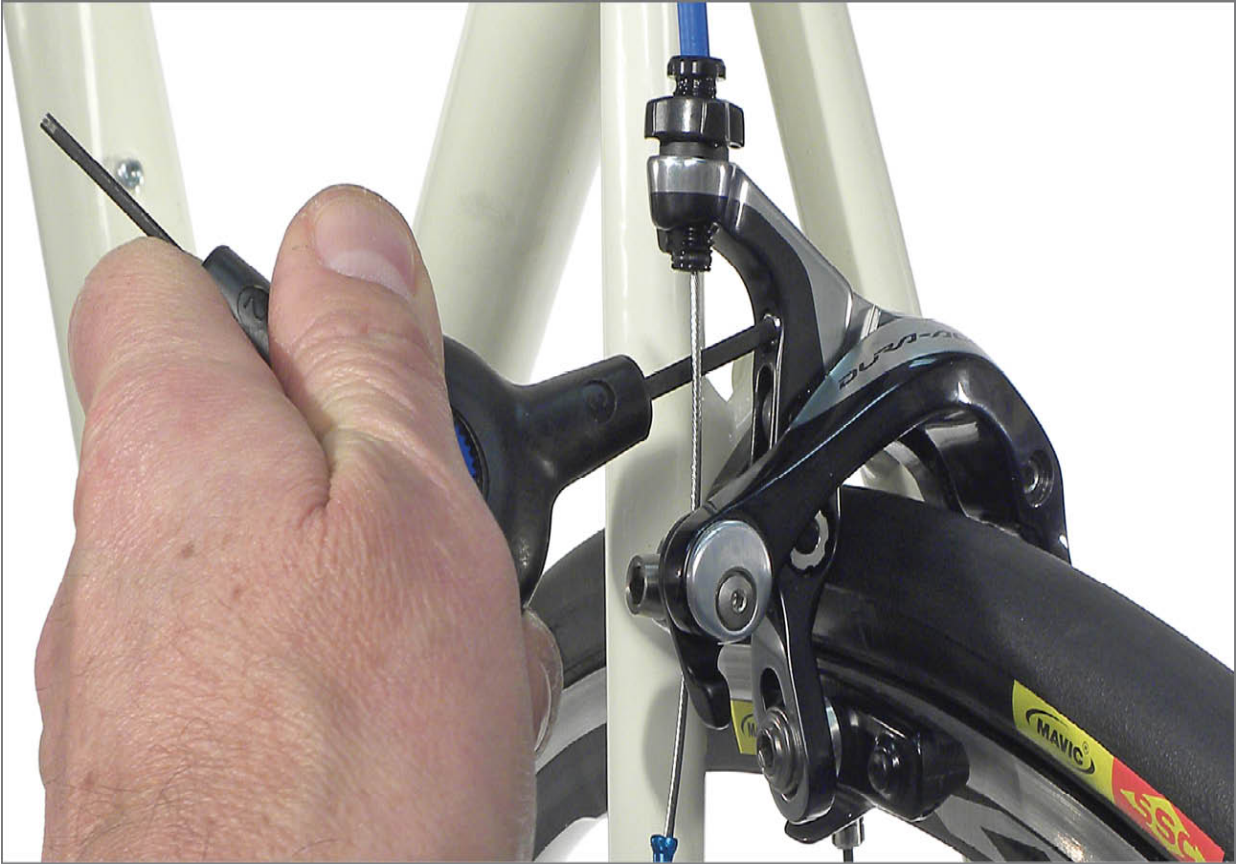
FIGURE 14.44: Centering screw location of Shimano® PR-9000
