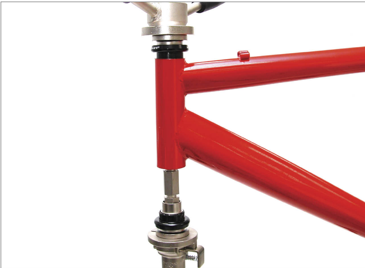
FIGURE 16.26: Arrangement of cups and pressing guides for the HHP-2 Headset Press
