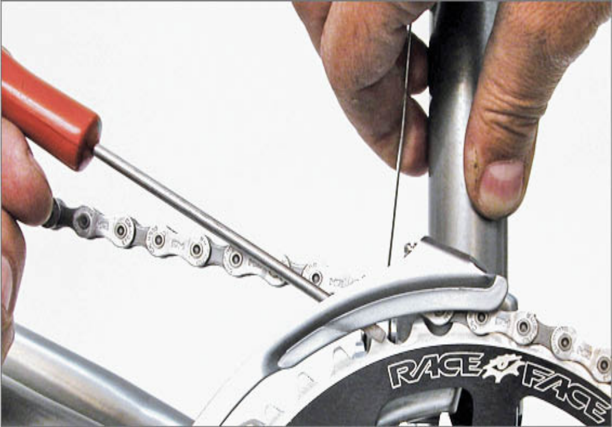
FIGURE 10.50: View gap at closest point between chain and derailleur cage
