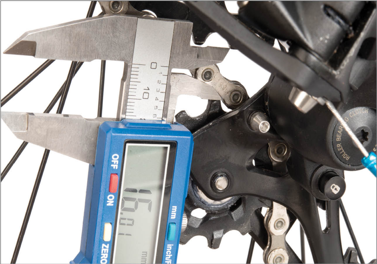
FIGURE 10.65: Set gap between G-pulley and largest sprocket
