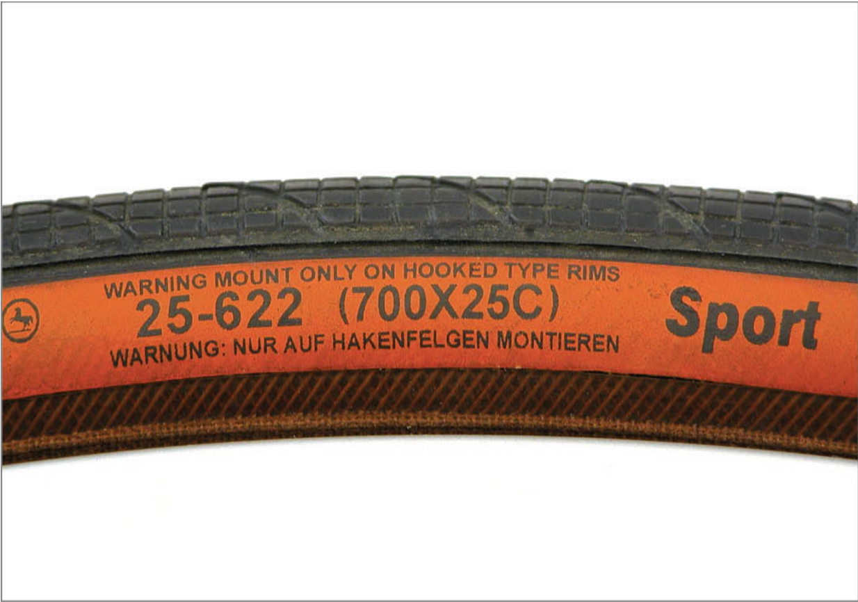
FIGURE 2.46: ISO (ETRTO) sizing numbers on tire label along with French sizing
