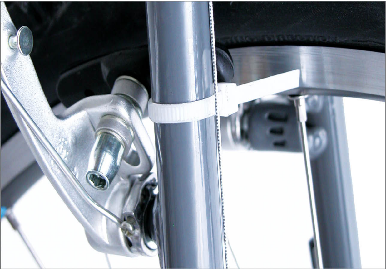
FIGURE 5.10: Use zip ties for reference indicator if truing stand is unavailable
