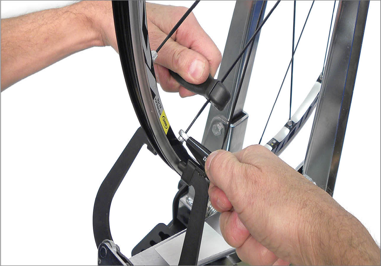
FIGURE 5.13: Use Park Tool BSH-1 to prevent bladed spoke twisting
