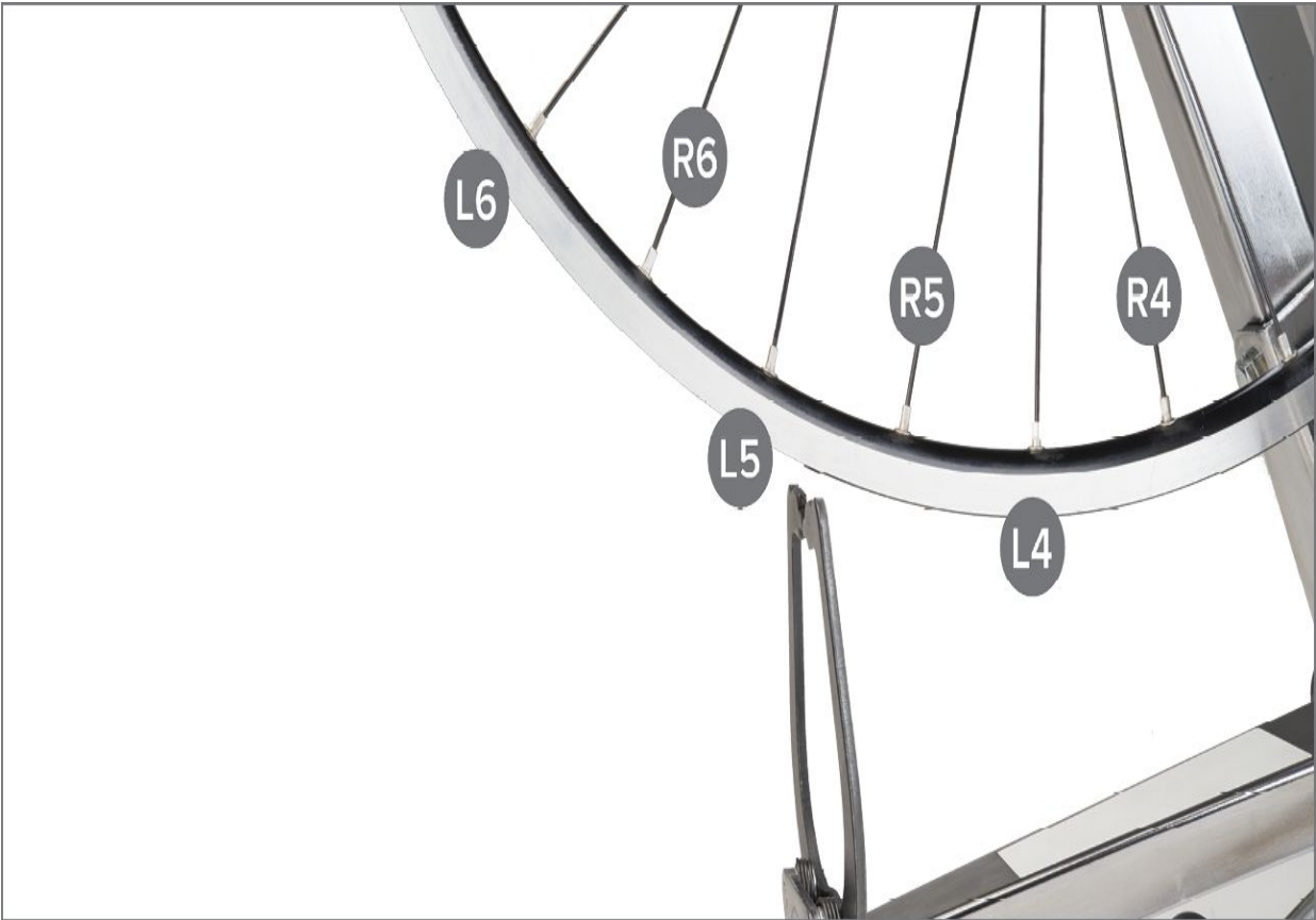
FIGURE 5.17: Correct radial error using both left and right-side spokes
