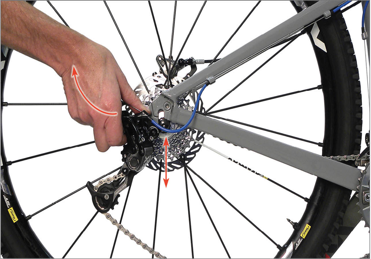
FIGURE 2.10: Remove and install wheel with cage in locked position
