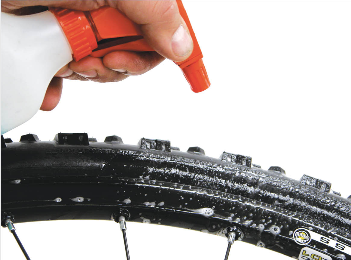
FIGURE 2.53: Soapy water can help bead seat into rim
