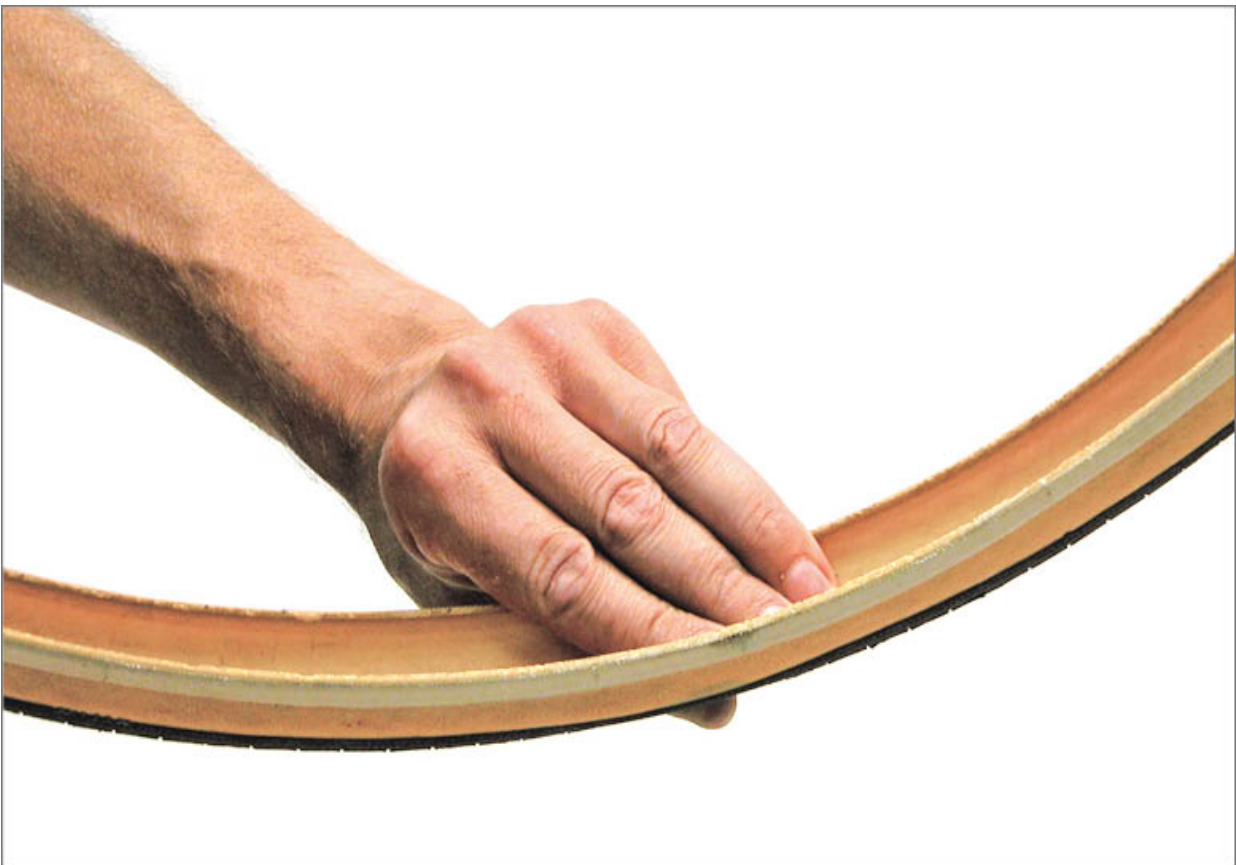
FIGURE 2.25: Carefully feel inside the case with fingertips
