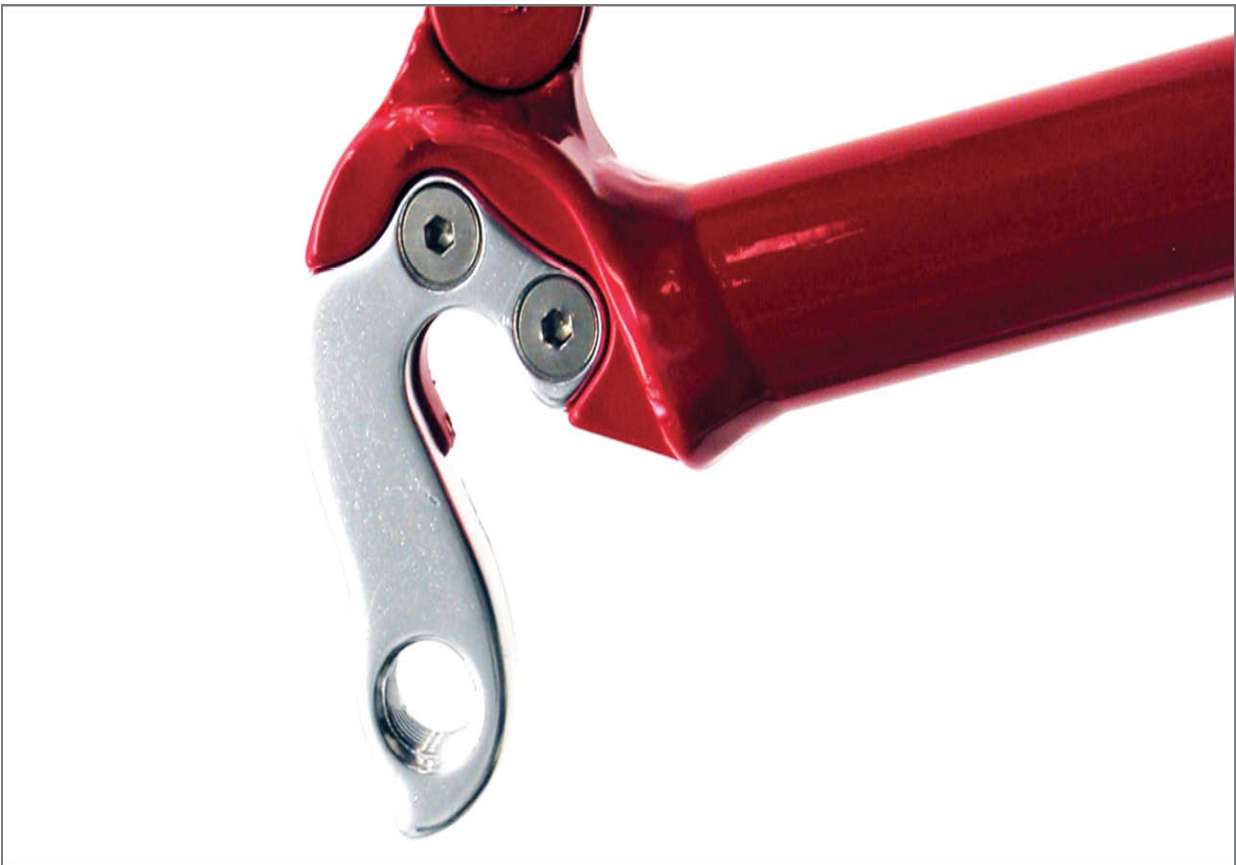
FIGURE 10.69: Replaceable type derailleur hangers should be checked for proper alignment
