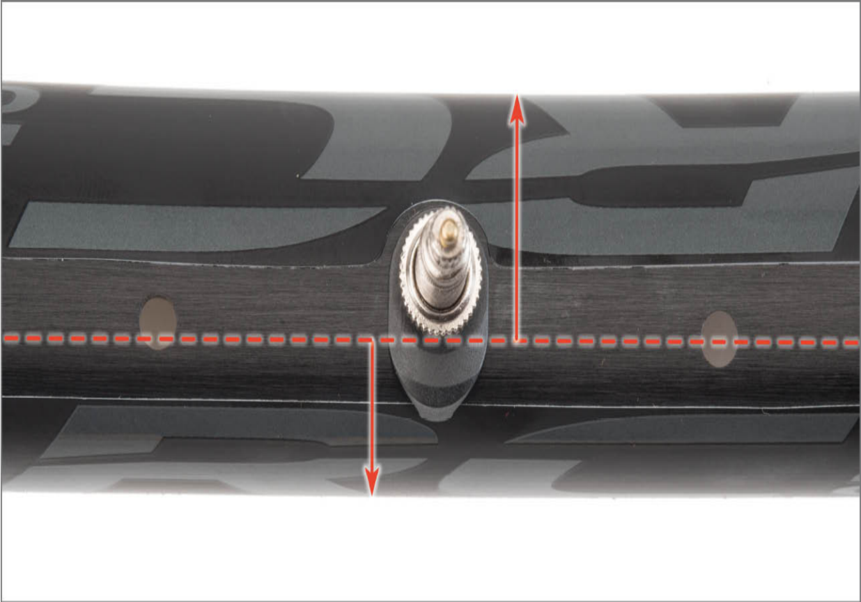
FIGURE 6.10: Asymmetrical rim design to reduce left-to-right spoke tension differences
