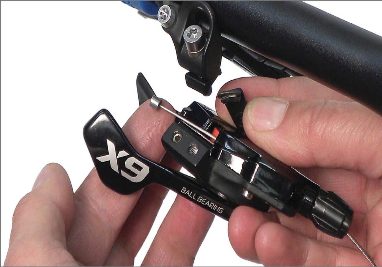
FIGURE 10.15: Pull up on rubber cover to expose cable access hole
