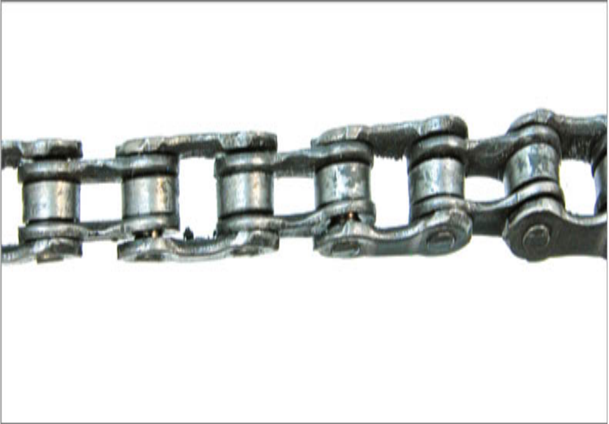
FIGURE 8.34: Any twist in the chain requires complete chain replacement
