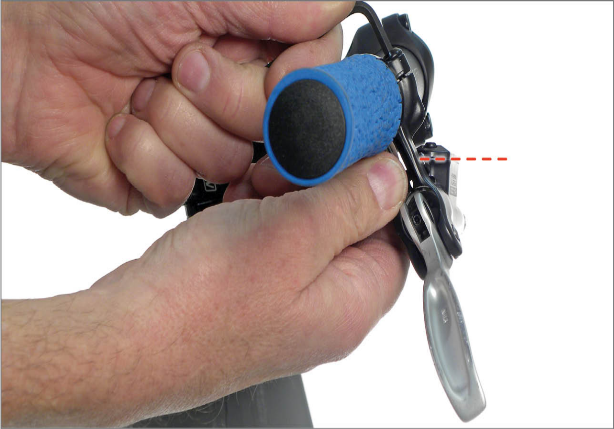
FIGURE 13.58: Adjust lever so reservoir cap is flat to ground
