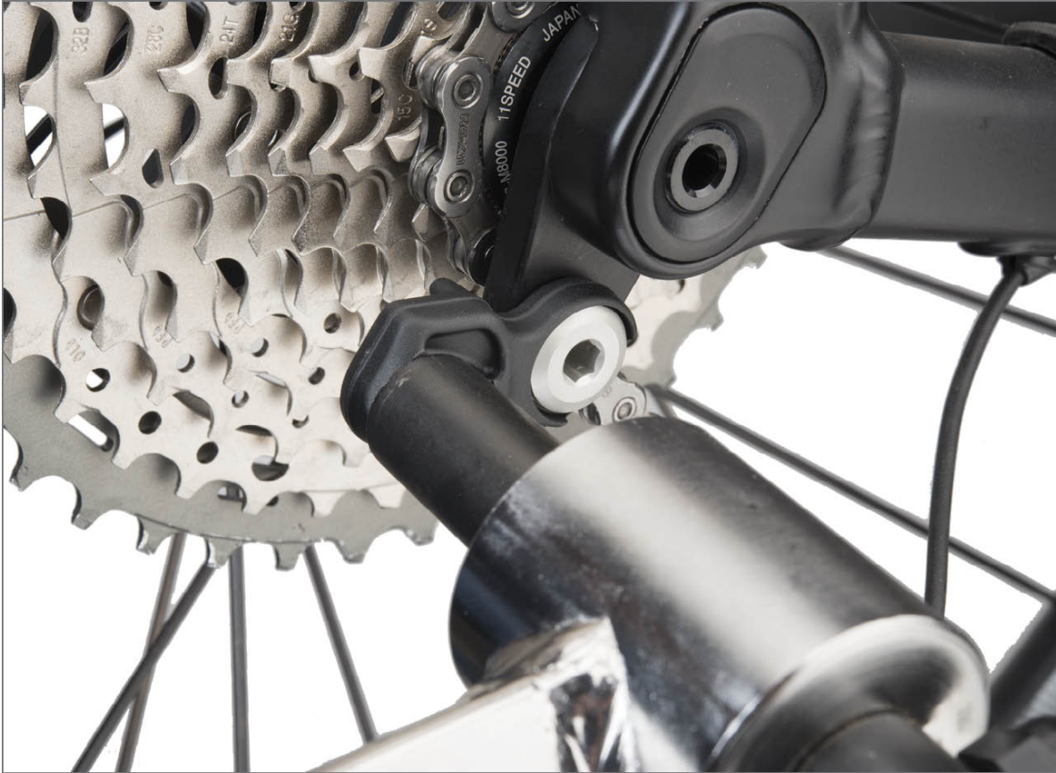
FIGURE 10.75: Check alignment of the B-link for best derailleur alignment
