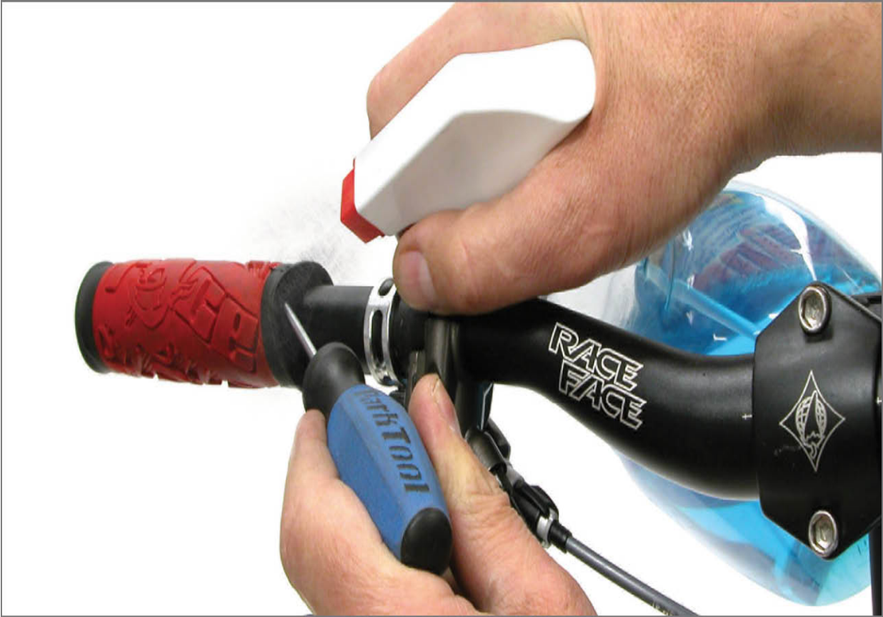
FIGURE 15.4: Move levers inward, then lift grip to inject liquid spray
