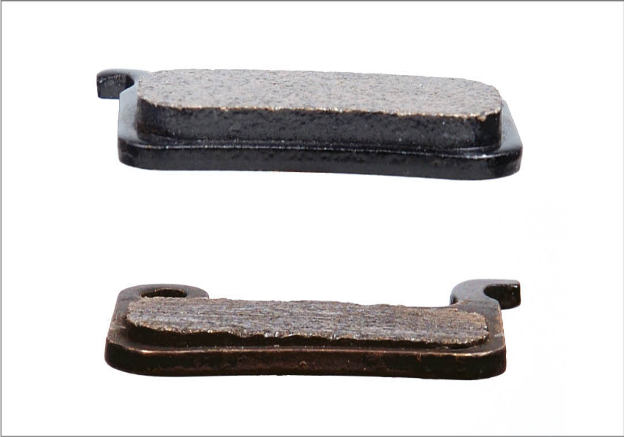
FIGURE 13.22: Pad above is new, while used pad below shows signs of misalignment of caliper to rotor
