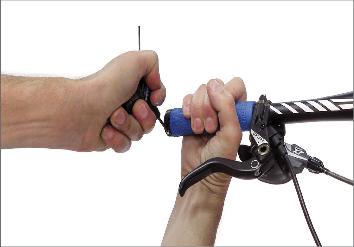
FIGURE 15.5: Secure set screws on locking grips
