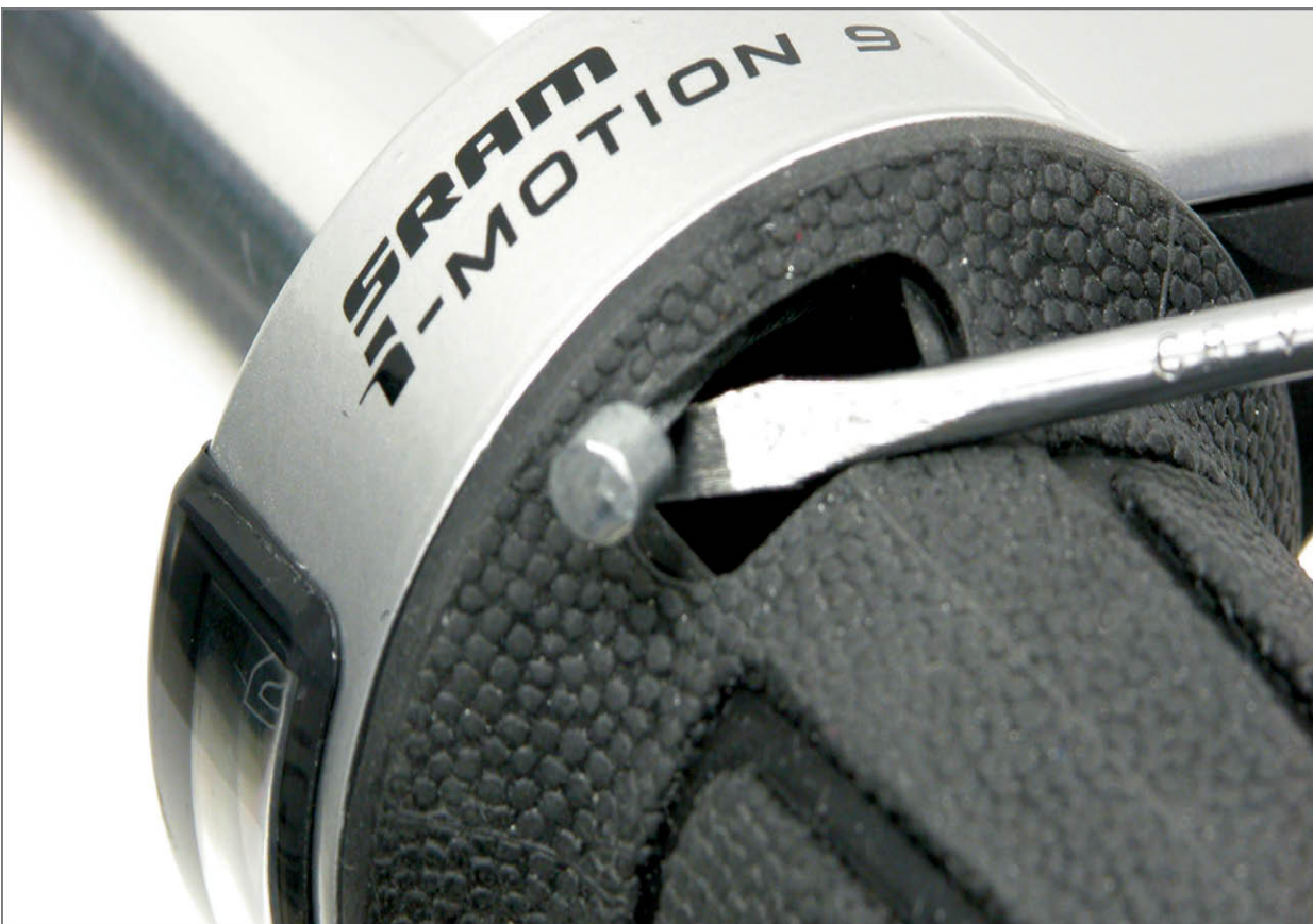
FIGURE 12.9: Remove cable from shifter
