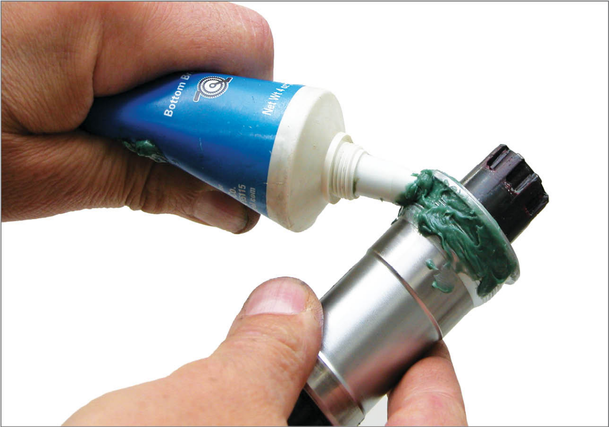
FIGURE 7.59: Lubricate threads of the bottom bracket
