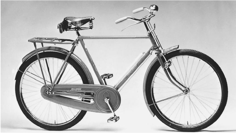
Figure 9.6 Raleigh Roadster bicycle with a gear case.
