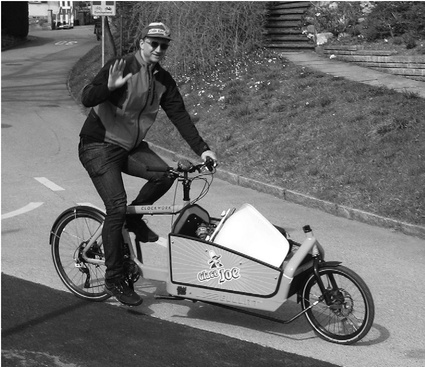
Figure 10.21 Modern Long John-type delivery bicycle.
