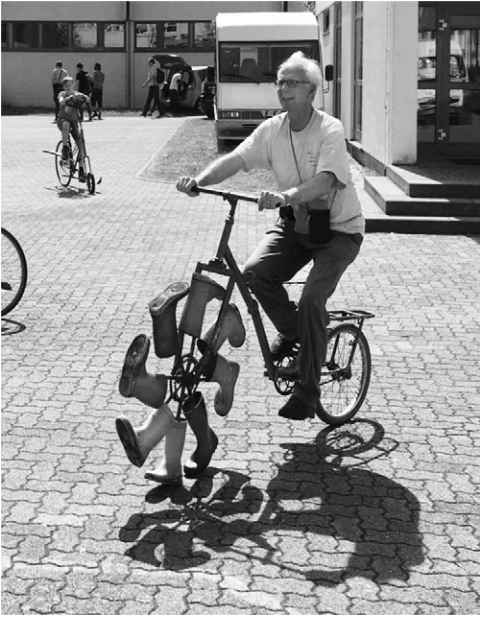
Figure 8.5 Bicycle with booted spokes. Bicycles can be perfectly adequately balanced and steered not just with the use of large wheels, but also using very small wheels, skis, or as shown here, spokes with boots on them! (Photo by Jean Gerber.)
