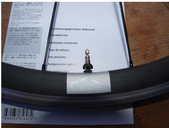
Figure 3.5 New valve inserted with rubber seal.
