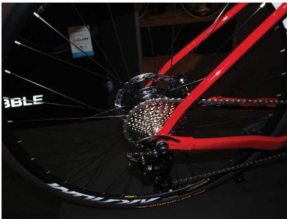
Figure 2.10 Specially shaped rear stays for large gear block.
