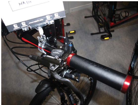
Figure 6.7 Combined gear and brake lever.
