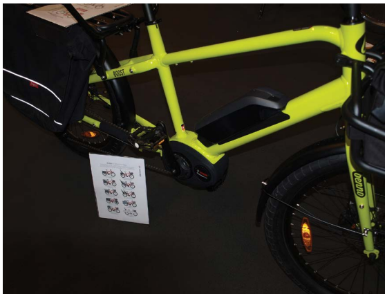
Figure 7.6 Electric motor in bottom bracket – I.
