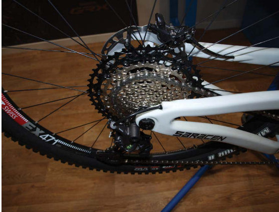
Figure 4.9 Extreme wide range gear set-up.
