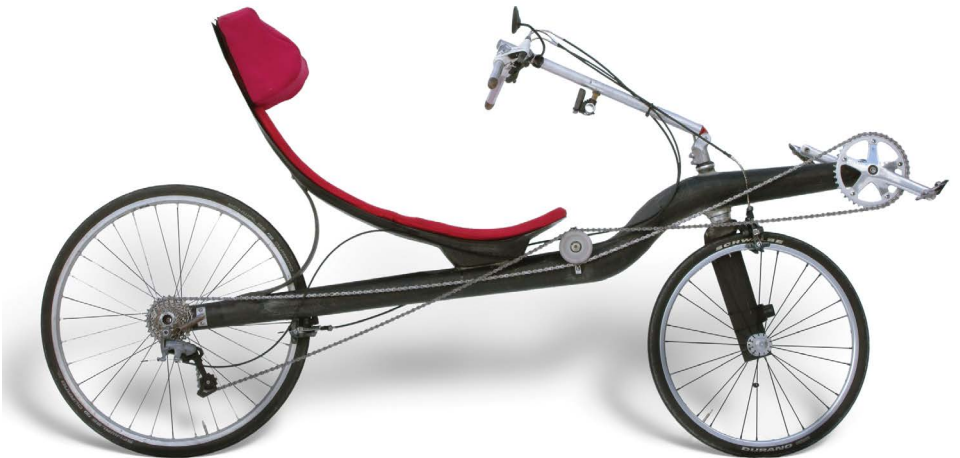
Figure 1.18 Rat racer GT—a minimalist, back to basics design approach in 2015 for a recumbent bicycle used for please rides around the English country lanes.
