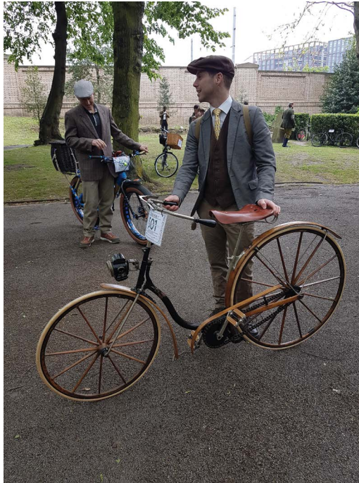
Figure 1.23 Safety bicycle with wooden rims.
