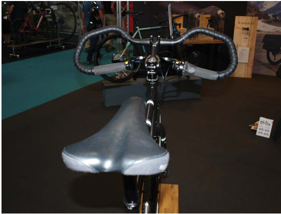
Figure 6.6 Multi-position loop bars - 2.
