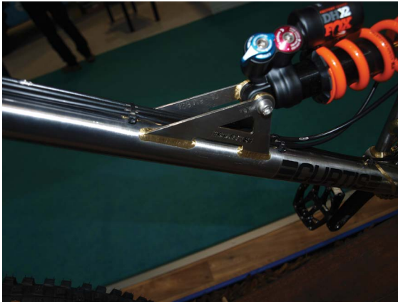
Figure 2.12 Custom mountain bike with fillet brazed steel tubing—rear suspension.
