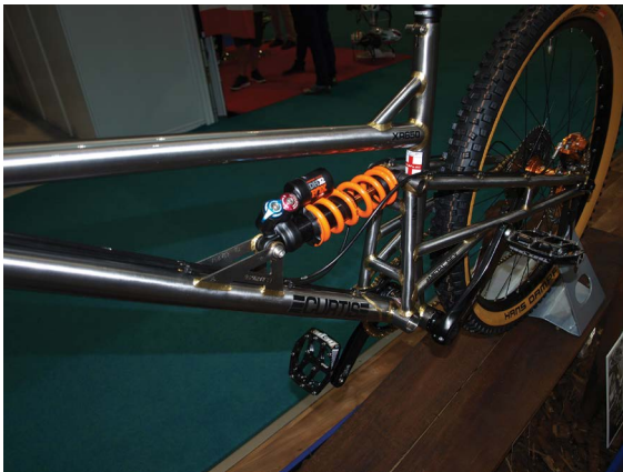
Figure 2.15 Stiffened seat tube.
