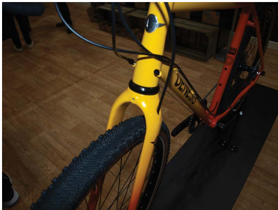
Figure 5.3 Hydraulic hose for front brake in fork.
