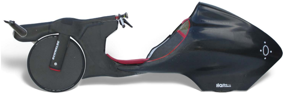
Figure 1.16 Rat racer extension—a part-faired HPV built for racing in 2014; it won a number of races. Its style is similar to that of formula racing cars, very purposeful shape.
