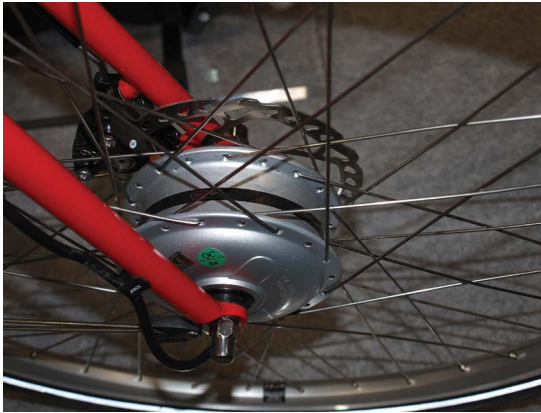
Figure 7.8 Close up of front wheel electric motor.
