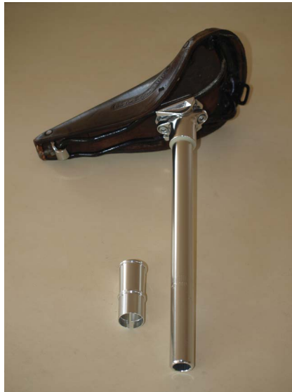
Figure 6.3 Seat post and size adaptor sleeve.
