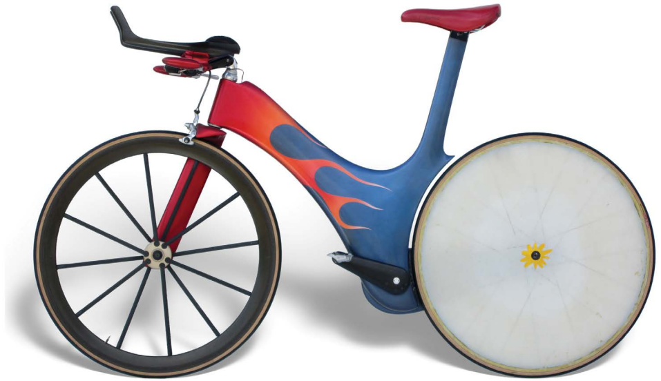
Figure 1.15 Last monocoque—designed for, but never ridden by, Abraham Olano in 1999. Abraham Olano is the only racing cyclist to have won both the World Road Race Championship and the World Time Trial Championship. The monocoque is made from pre-preg carbon fibre in two halves bonded together. The aerodynamic chain case houses a chain which is especially made with links almost half the size as those on other bicycles.
