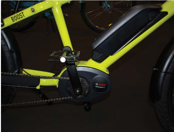
Figure 7.7 Electric motor in bottom bracket – 2.
