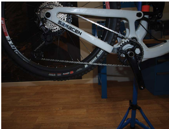
Figure 4.10 Wide chain angle 2nd view.
