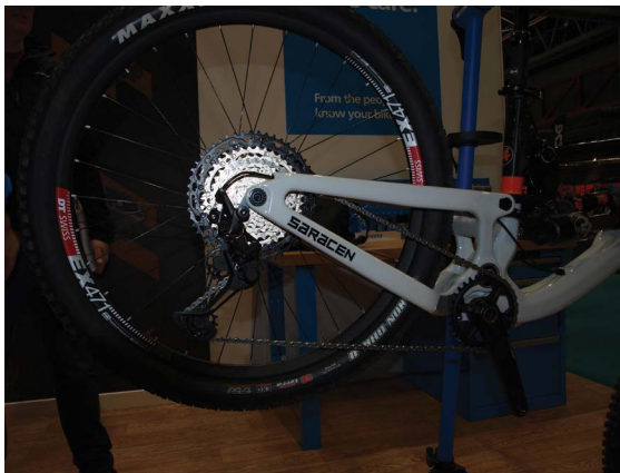
Figure 4.8 Very long arm with wide range cassette.
