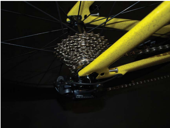
Figure 4.4 Mechanical wide range rear changer.
