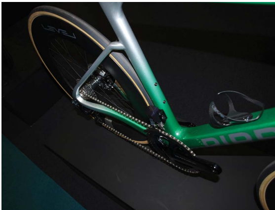
Figure 4.14 Very clean-cut electronic gear set-up.
