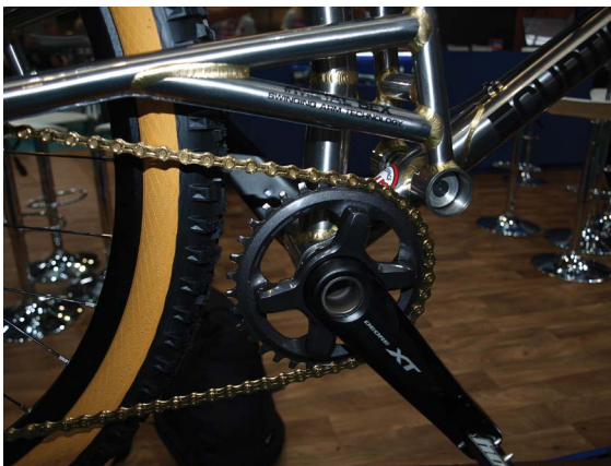
Figure 2.18 Complex bottom bracket and swinging arm set-up.
