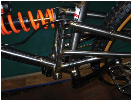
Figure 2.14 Spring and shock absorber mounting.
