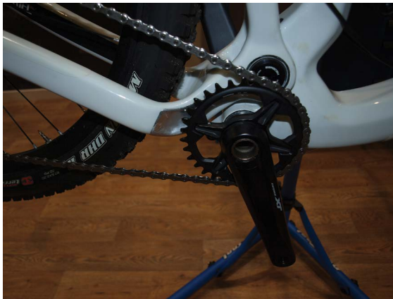
Figure 4.6 Super small single chain ring.
