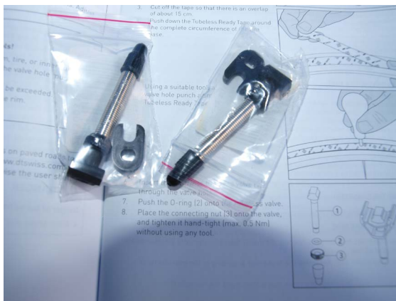
Figure 3.2 Valves for converting to tubeless.
