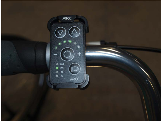
Figure 7.5 Electric motor control panel.
