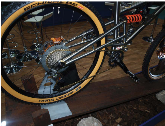
Figure 2.17 Small chainring and large rear block cassette.
