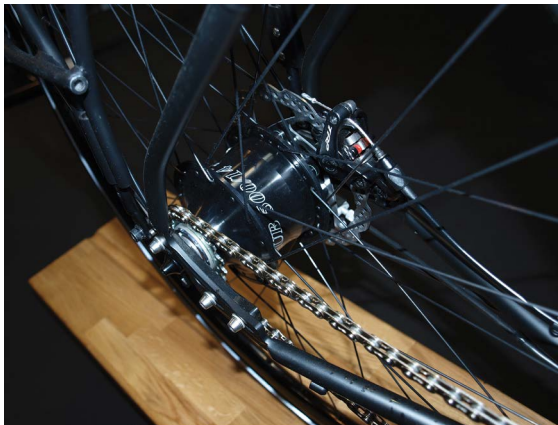
Figure 4.15 Hub gear set-up on steel framed bicycle.
