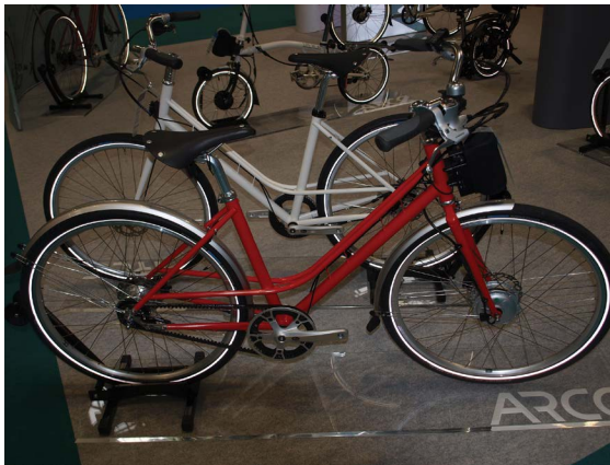
Figure 7.4 Step through bicycle with electric motor in front wheel.
