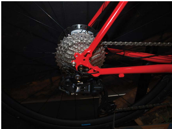
Figure 4.12 Electronic rear changer with wire in stay.
