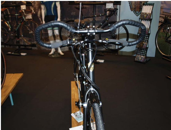
Figure 6.5 Multi-position loop bars - 1.
