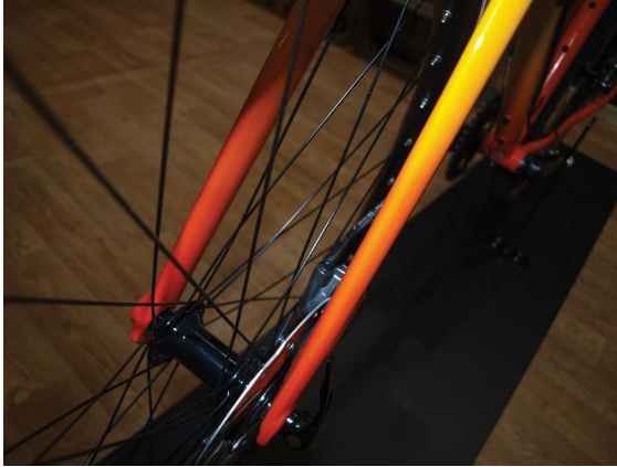
Figure 5.4 Detail of hydraulic hose at lower end of fork.
