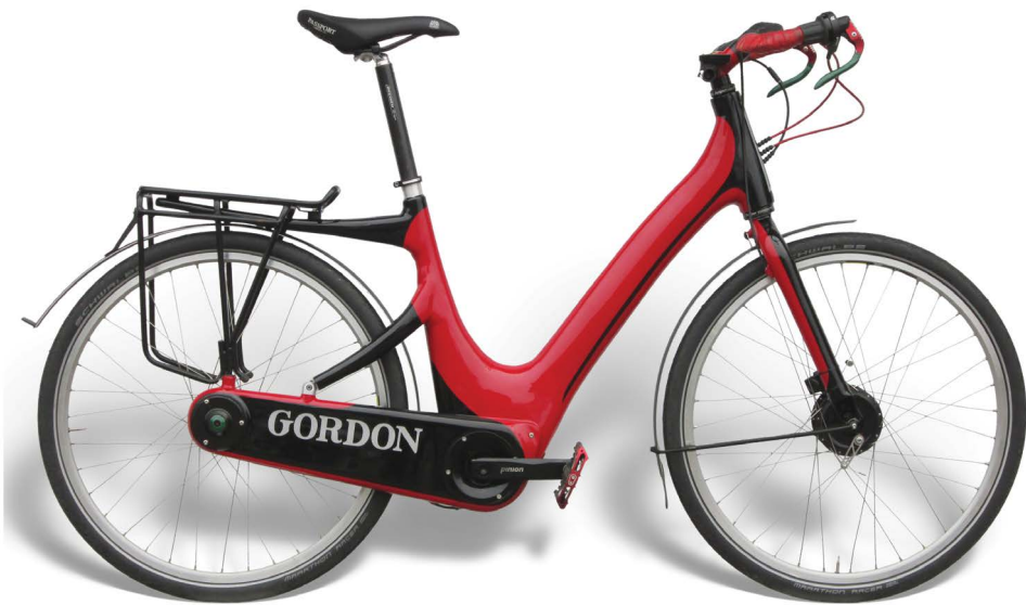
Figure 1.19 Gordon—designed in 2015, and now becoming the basis for many commuter bicycles and electric bicycles. It is reminiscent of 1960s mopeds and old Dutch step throughs. A style seen on London streets as Santander bicycles. This one is amazingly light weight carbon fibre with a pinion gear drive.
