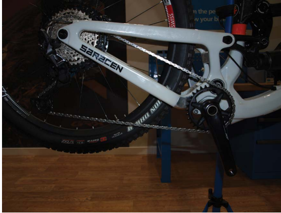
Figure 4.7 Exceptionally wide chain angle.
