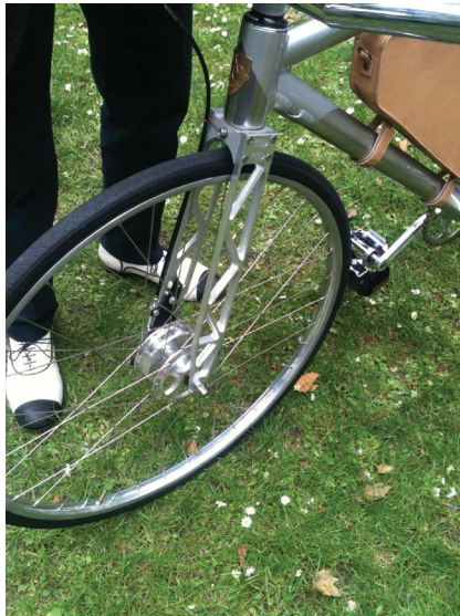
Figure 2.11 Computer numerical control machined forks.
