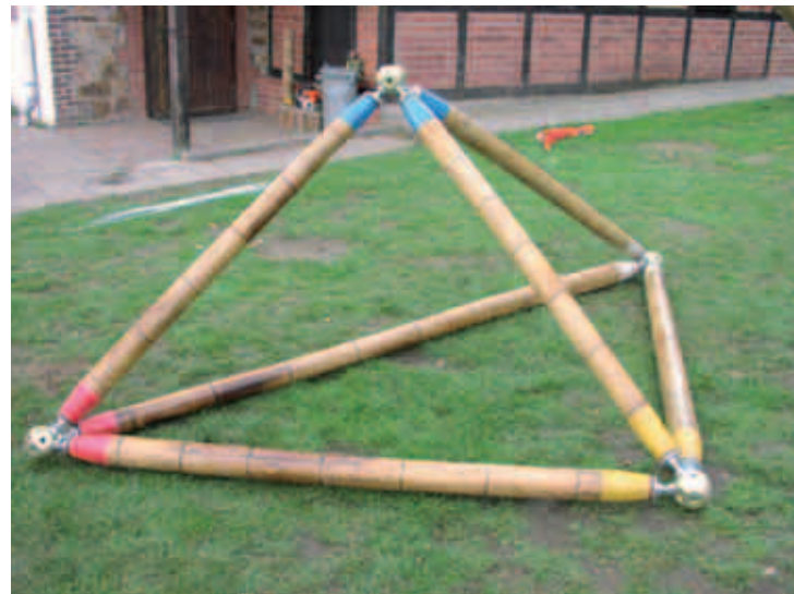
Figure 3-13: The development of bamboo connection to avoid eccentricity of load transfer with a space frame connector (courtesy of Chair of Structures and Structural Design, RWTH Aachen)
