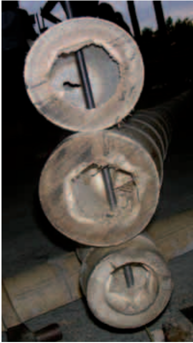
Figure 3-8: The capability of bolted joint to connect three big bamboos at once
