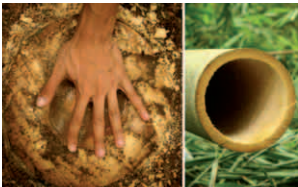
Figure 2-5: The extreme difference of the diameter and wall thickness between lower and upper part (courtesy of Arif Rabik)
