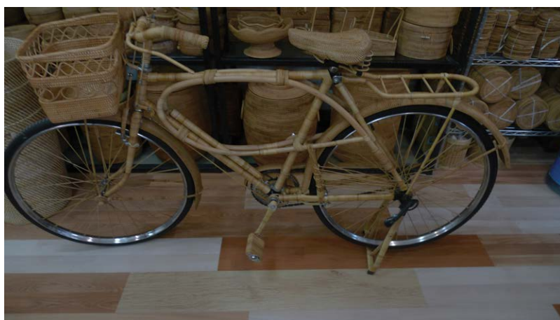
Fig. 2.75. A bike made of bamboo ( Fargesia sp.) in Yunnan Province, China (Zhu Zhaohua).
