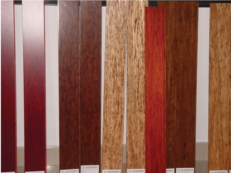
Fig. 3.85. Different types of floorings made from pressed bamboo material (Zhu Zhaohua).
