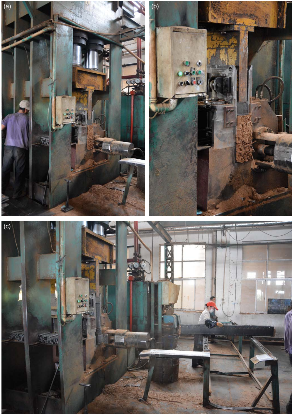
Fig. 3.83a,b,c. Photos of a pressing machine for processing pressed bamboo material in Anji, Zhejiang Province, China (Zhu Zhaohua).
