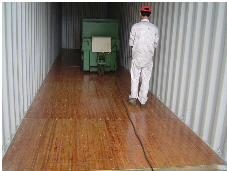
Fig. 2.82. The floor of a container built with bamboo (Zhou Guomo and Shi Yongjun, 2012).
