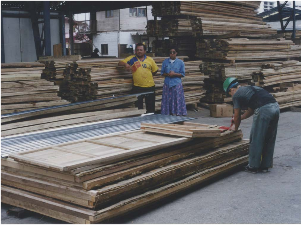
Fig. 3.28. The bamboo processing factory Viviendas Hogar Cristo in Ecuador produces 70 sets a day of houses for the poor (Zhu Zhaohua)
