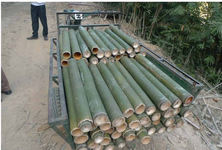
Fig. 4.5. Culm sections from Schizostachyum funghomii , which has long internodes (80–120 cm). It is very suitable for weaving products. (Zhu Zhaohua).
