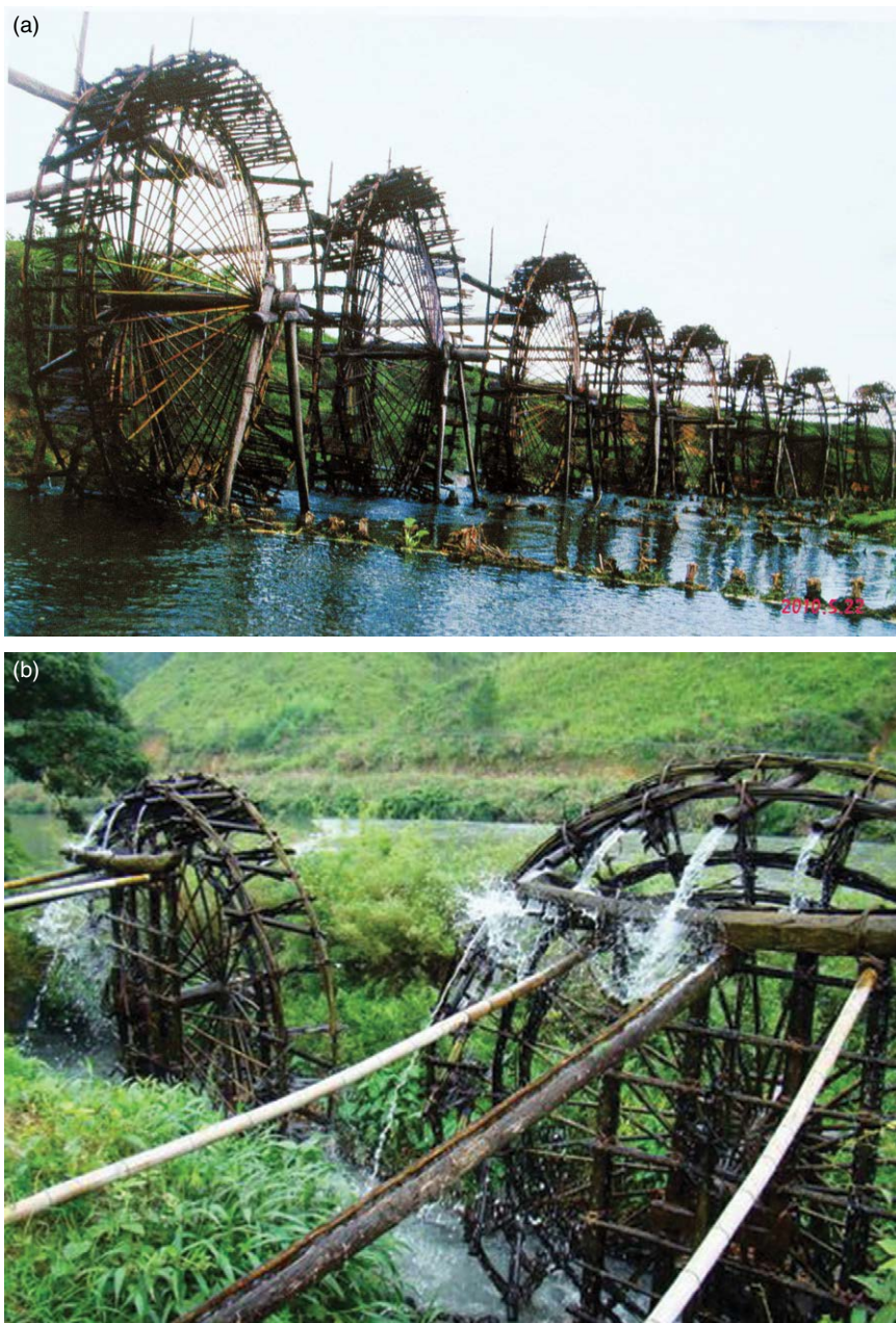
Fig. 2.58a,b. High-speed winders (irrigation water wheels) made of bamboo (Museum of Bamboo Weaving Articles in Qingshen, Sichuan Province, China).
