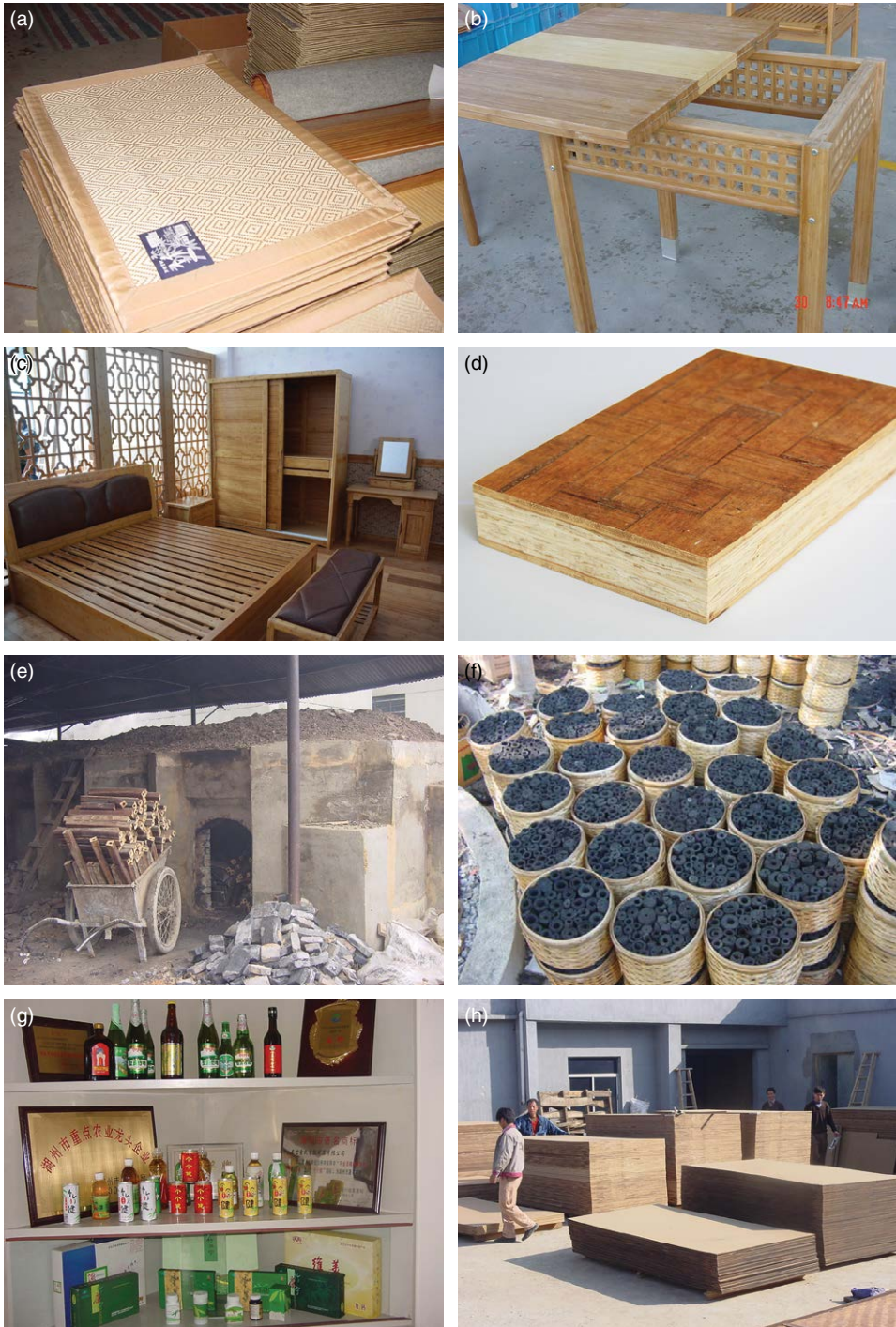
Fig. 3.42. Bamboo products: (a) mats; (b–c) laminated furniture; (d) wood composite block; (e) making charcoal bricks from bamboo sawdust; (f) charcoal; (g) bamboo leaf extracts; and (h) particle boards (Zhu Zhaohua).
