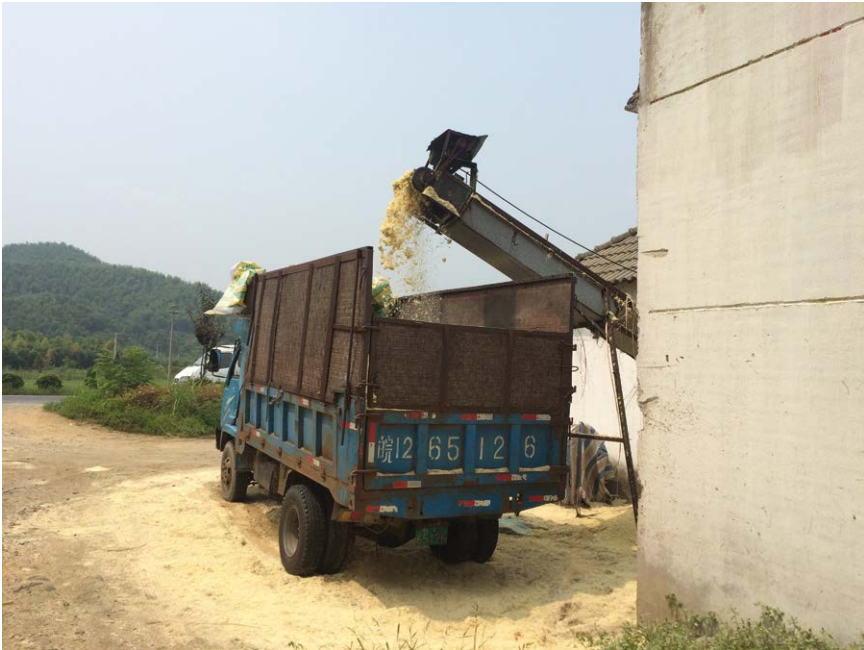
Fig. 3.39. Large amounts of sawdust from the primary processing factory are automatically collected and loaded on to a truck, which transports the sawdust to other factories producing particle boards, biomass fuel pellets and charcoal (Zhu Zhaohua).
