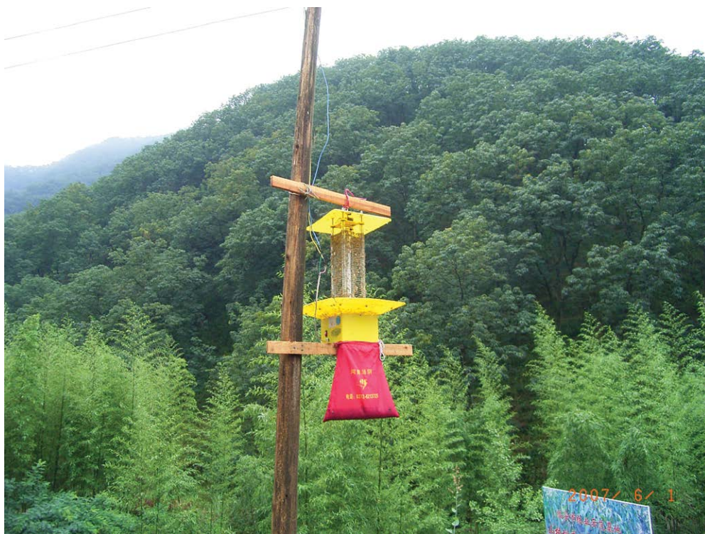
Fig. 3.75. A solar-powered black light lamp emitting UVA light placed in a bamboo forest in Anji, Zhejiang Province, China, for insect control/trapping; one lamp can control about 6 ha (Anji Forestry Bureau).
