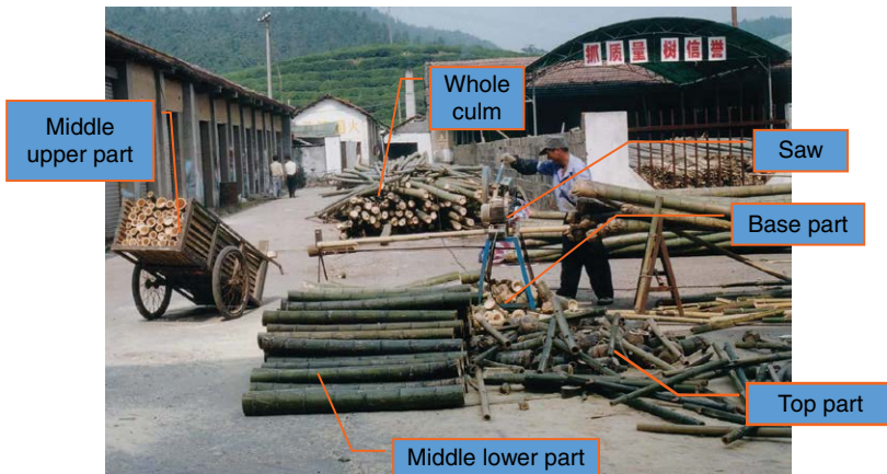
Fig. 3.34. Raw cutting at a bamboo primary processing factory, Anji, Zhejiang Province, China, 2005 (Zhu Zhaohua).
