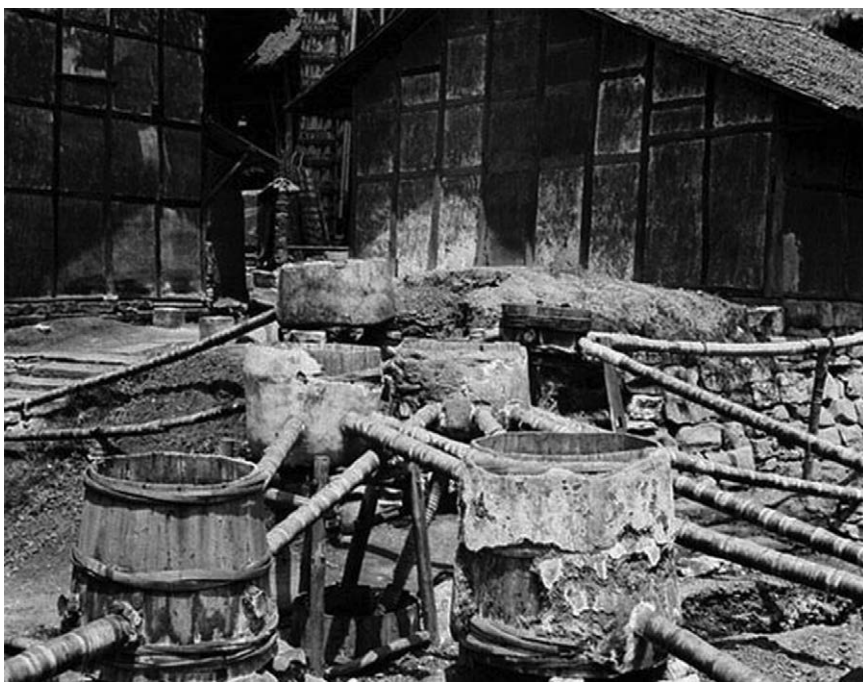
Fig. 2.60. Salt mining using bamboo tools (from the Museum of Salt Exploration in Zigong, Sichuan Province, China).
