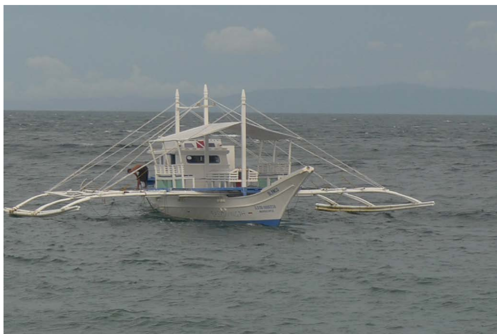
Fig. 2.81. A bamboo sightseeing ship in the Philippines made with 70% of materials from bamboo (Zhu Zhaohua).
