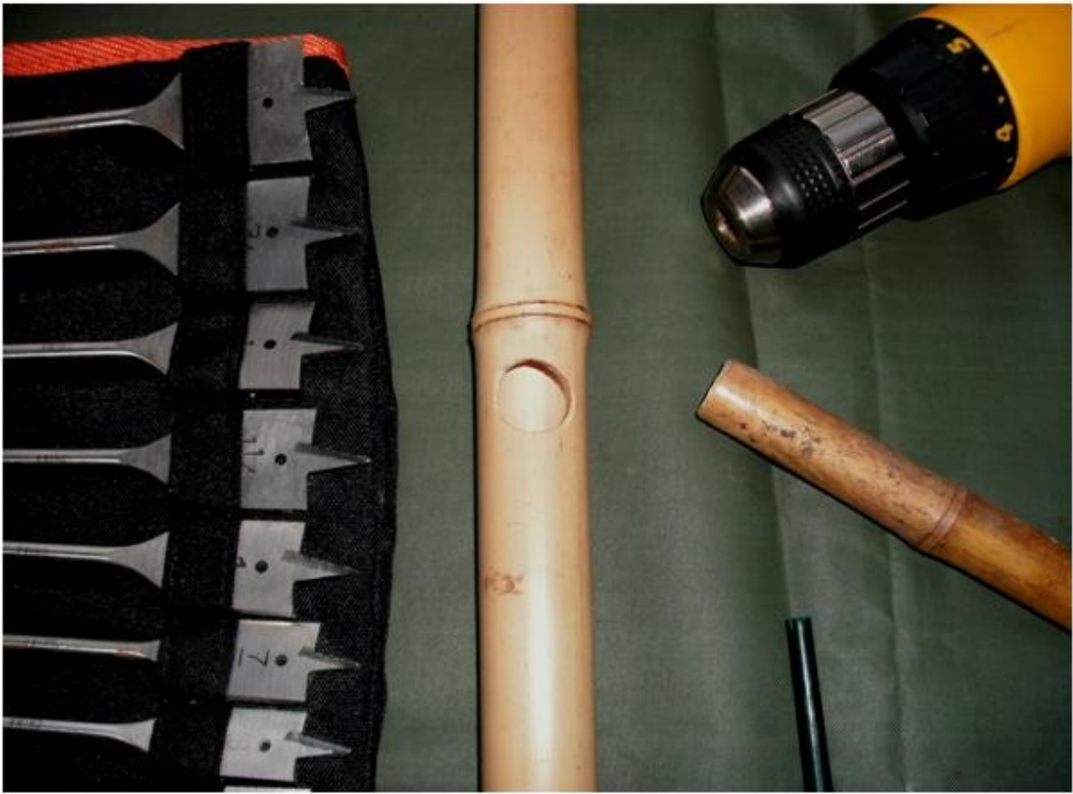
This joint is a pegged socket joint. A hole is drilled into an upright, the right size to fit a smaller cross-pole.
