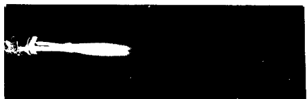
j. Neutral Flame – Cutting Oxygen flowing
