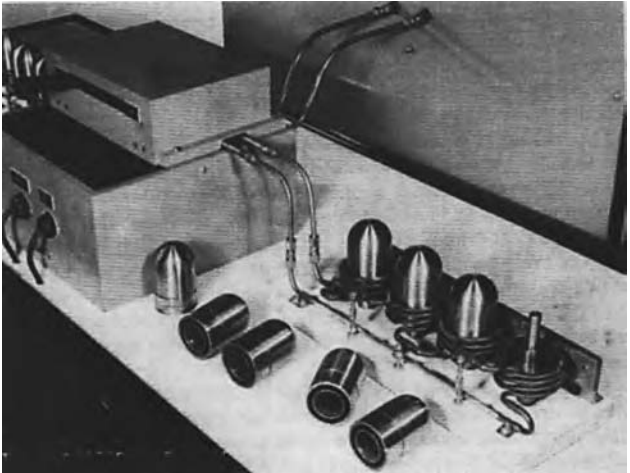
Fig. 6-4 Typical induction brazing operation.
