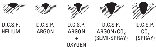
Fig. 5-5 Weld penetration changes for different shielding gases, polarity, and amount of current applied.
