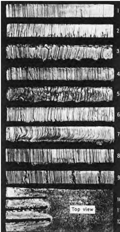
Fig. 3-19 View of the edges of metal cut properly and improperly by the oxyacetylene process
