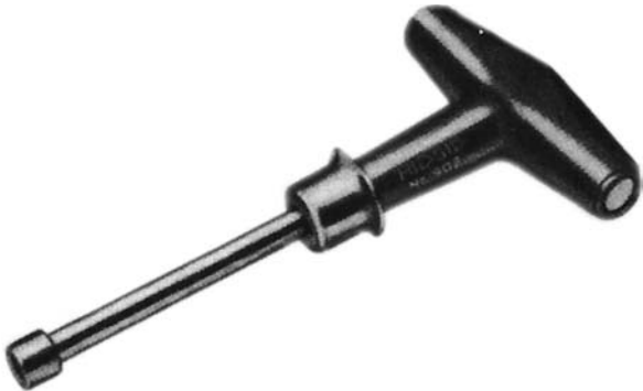
Fig. 3-17 Torque wrench for cast-iron and no-hub soil pipe. Pre-set for 60 inch-lbs (67.9 N-m) of torque. (Courtesy Ridge Tool Company)
