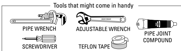
Fig. 6-28 Tools needed to install single-handle tub and shower set. (Courtesy Eljer Plumbingware Co.)
