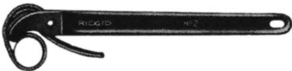
Fig. 3-12 Strap wrench— \frac{1}{8} inch through 2 inches (3 mm through 51 mm). (Courtesy Ridge Tool Company)
