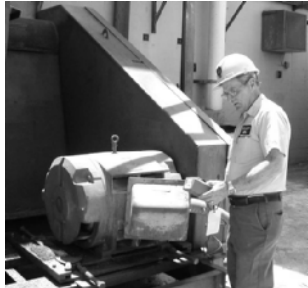
Fig. 21-2 Simple vibration meter in use. Copyright Balmac, Inc.
