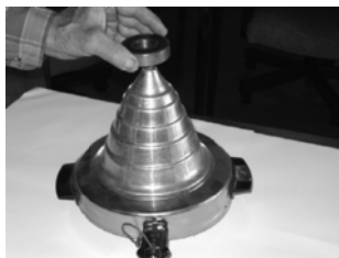
Fig. 20-3 Heating the inner race using a cone heater.
