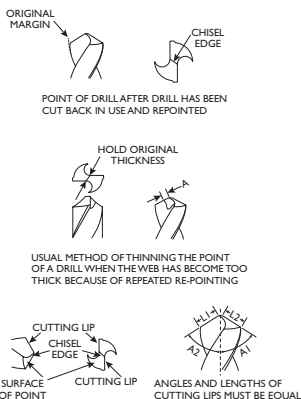
Fig. 5-5 Hold these dimensions when web-thinning.
