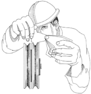
Fig. 38-1 Inspection using a sheave gauge. Courtesy of Maintenance Troubleshooting .
