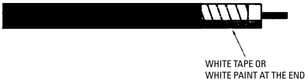
Figure 8-16 Identification of conductor cable No. 4 and larger.
