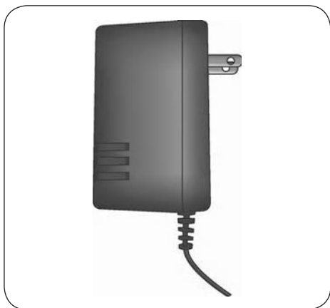
Figure 18-7 Typical Printer Transformer
