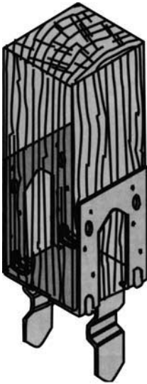
Typical WE44 Installation
