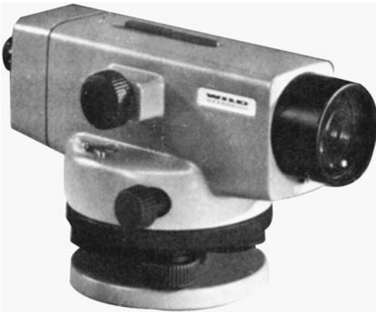
Figure 6-15 NA2 automatic level. (Courtesy of Wild-Heerbrugg)
