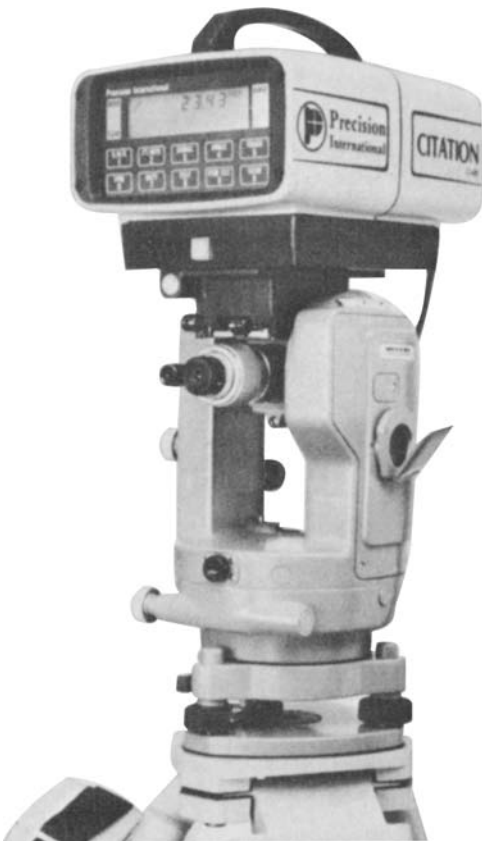
Figure 6-16 Typical EDM/Theodolite setup. (Courtesy of Wild Heerbrugg)
