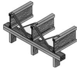
Typical N Bracing Installation
