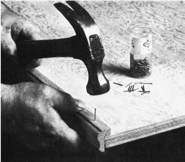
Figure I-3 Brads are small nails. They are used to attach thin strips of wood such as moldings. (Courtesy of The American Plywood Assn.)
