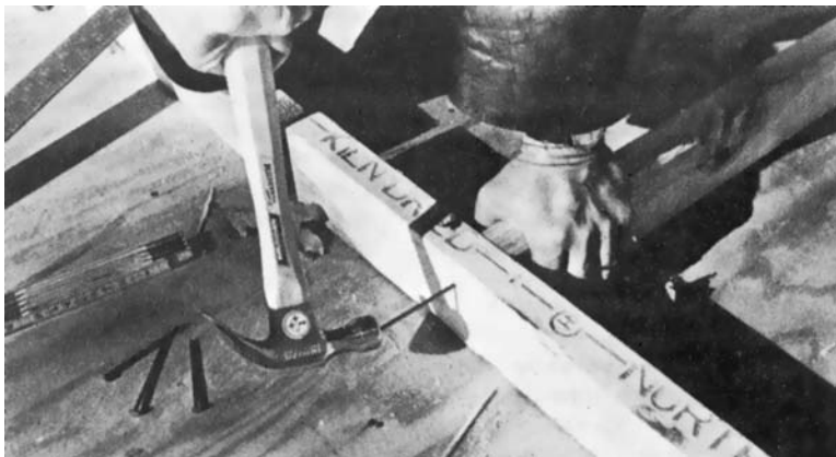
Figure 3-1 Construction lumber. Note the classification kiln-dried on one member. This stock will be used inside a structure.
