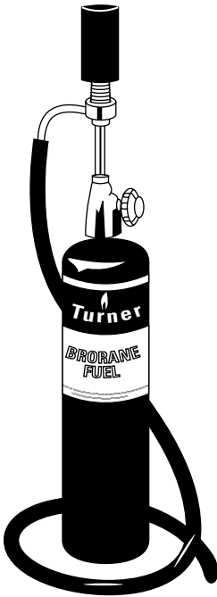
Figure 16-5 Gas leak detection is easy. This sensitive halide detector pinpoints Freon leaks in a short time. Used on all noncombustible refrigerant (Freon) leaks, the flame changes color when the exact location of the leak is determined. (Courtesy Turner Corporation.)
