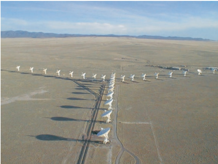
Fig. 5.3 The Very Large Array radio interferometer with a total of 27 active antennas. (Credit: NRAO/AUI/NSF)
