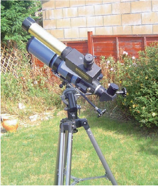
Figure 2.11. Mounting the PST on an equatorial mount, sequence 3.
