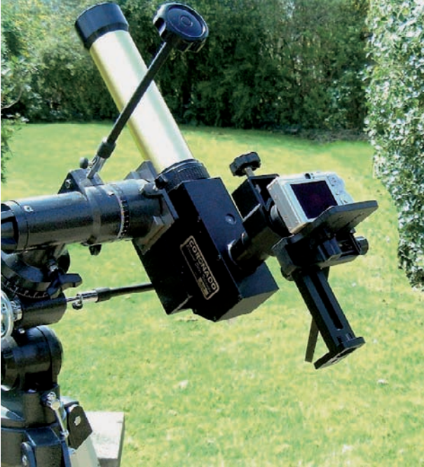
Figure 2.54. Canon Powershot SD450 mounted with the PST.
