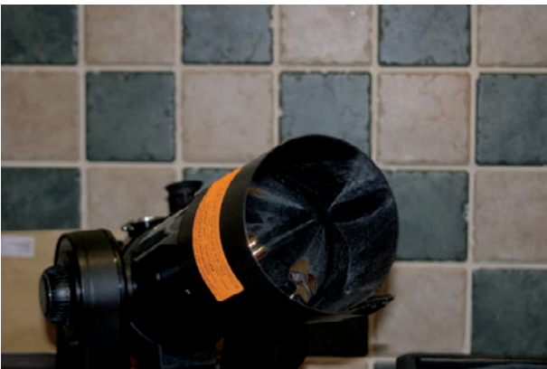
Figure 5.47. Baader filter fitted to a Meade ETX90.
