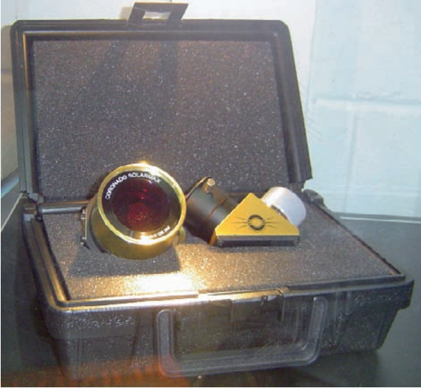
Figure 2.30. SolarMax filter with blocking filter (blocking filter not used with PST).
