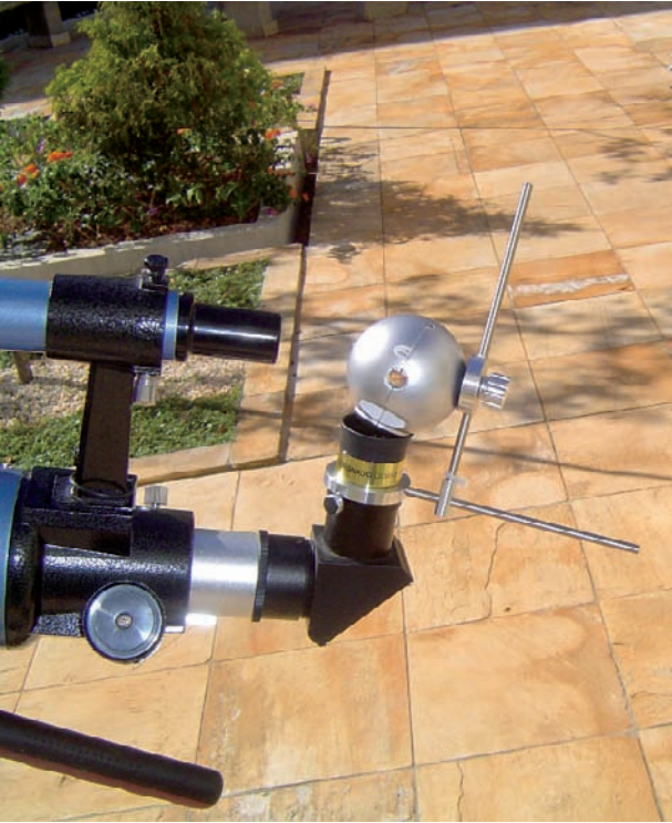
Figure 2.57. Afocal camera adaptor with Coronado CEMAX eyepiece.
