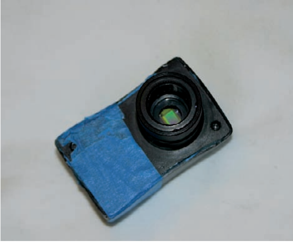
Figure 5.32. The Meade LPI modified with masking tape to reduce the eight levels.
