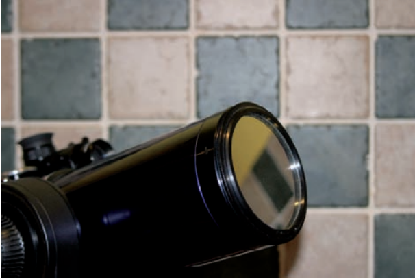
Figure 5.48. Astro Engineering solar filter fitted to Meade ETX90.
