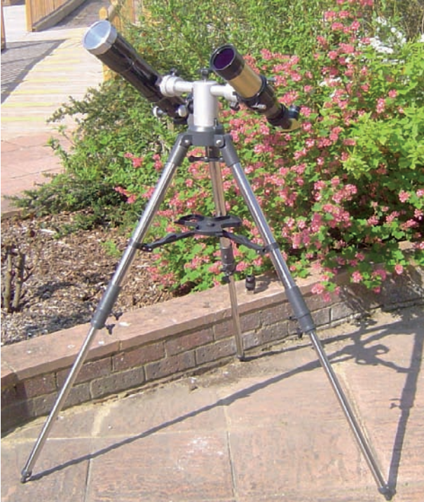
Figure 4.29. MaxScope 70 and Revelation 80 mounted on a Bresser GIRO.
