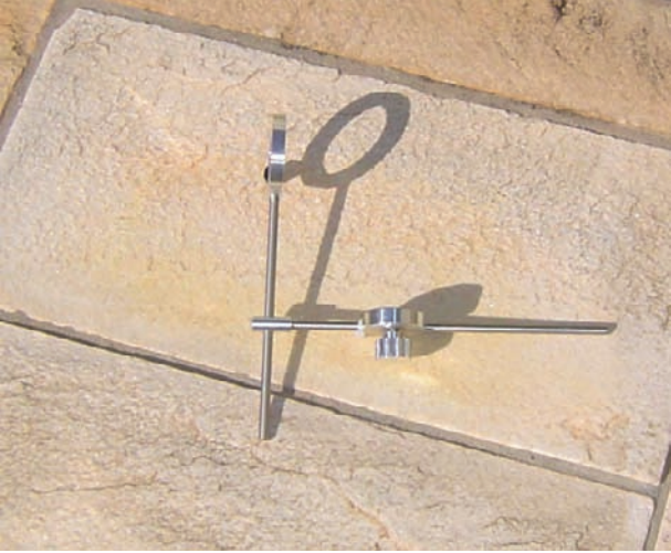
Figure 2.56. Afocal camera adaptor.
