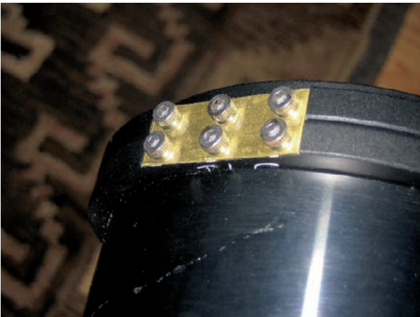
Figure 3.5. T-Max ring attached between the filter and the telescope. Photo by Larry Alvarez.
