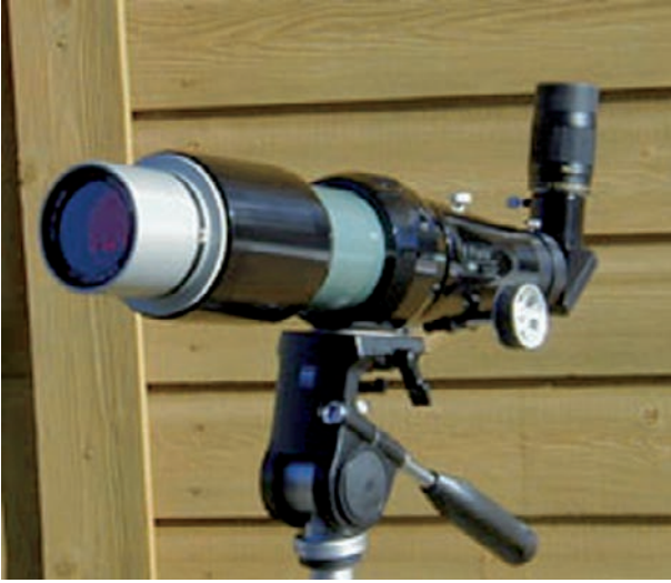
Figure 7.7. SolarScope 50-mm filter with Televue Pronto. Courtesy of SolarScope.
