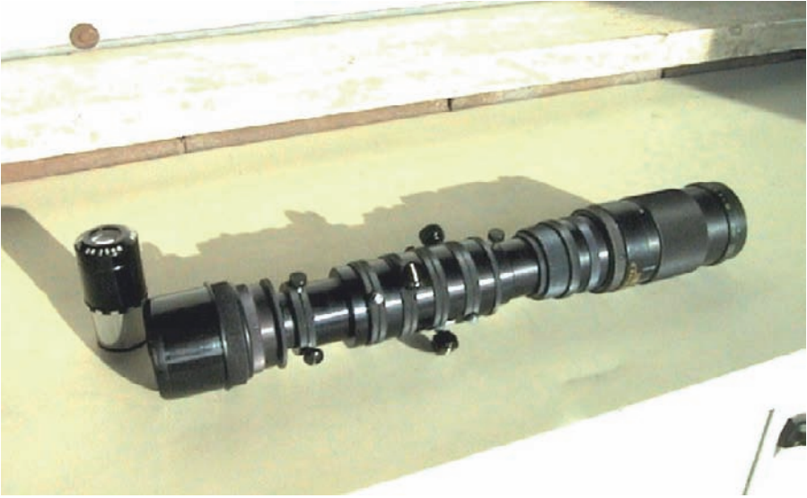
Figure 6.6. CromixSun with telecentric optic system.
