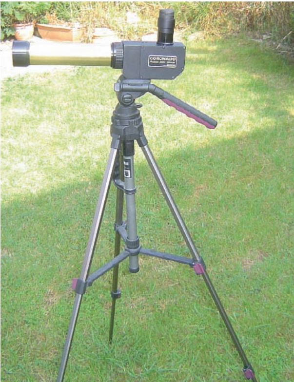
Figure 2.8. Mounting the PST on a camera tripod, sequence 4.
