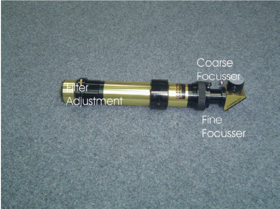
Figure 4.5. Topside view of the MaxScope 40.
