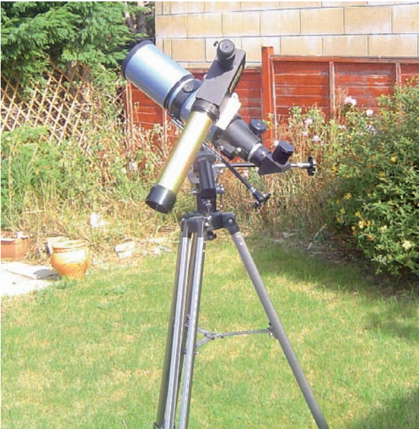
Figure 2.10. Mounting the PST on an equatorial mount, sequence 2.
