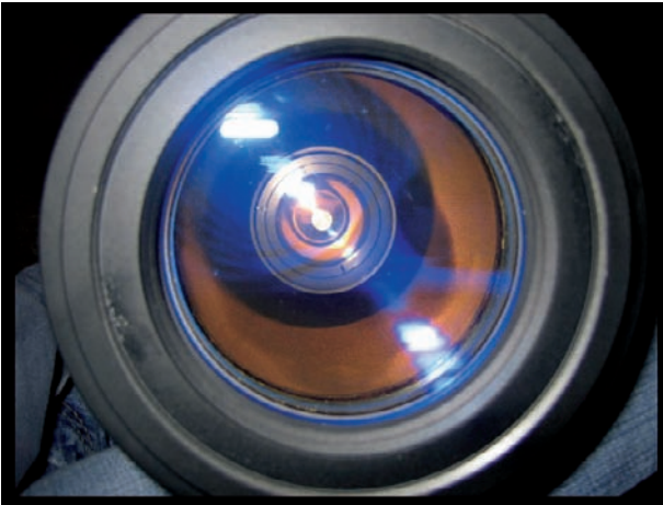
Figure 3.6. View through the objective showing the secondary (internal) filter. Photo by Larry Alvarez.
