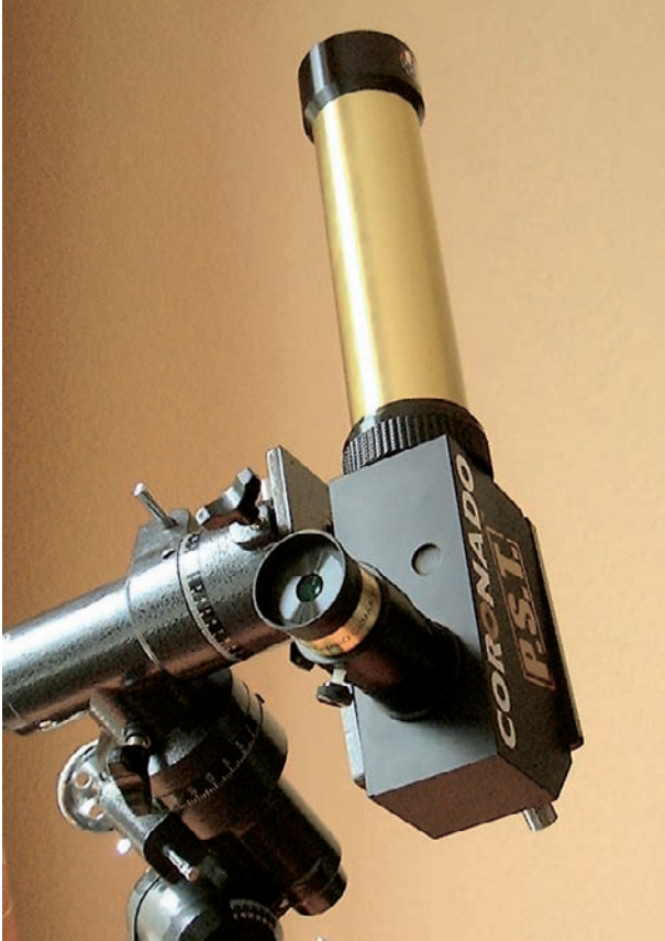
Figure 2.18. Mounting bracket for the PST Part 6. Courtesy of John Watson.
