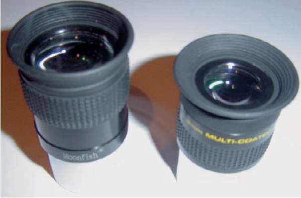
Figure 2.44. The eyepieces of 20- and 15-mm focal length from the Moonfish Group.
