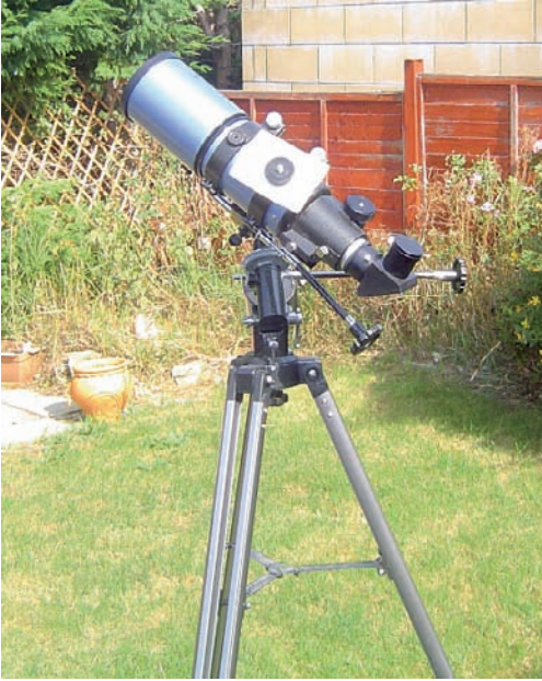
Figure 2.9. Mounting the PST on an equatorial mount, sequence 1.
