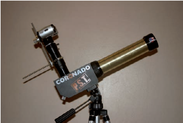
Figure 2.51. PST with afocal adaptor.
