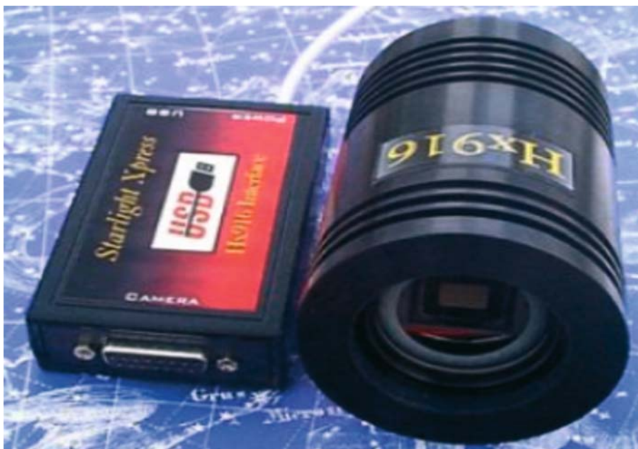
Figure 2.9. Starlight Xpress HX916 camera and USB control box. The USB control box is attached with Velcro to the west fork arm of the LX200. (Used with permission, Starlight Xpress™.)
