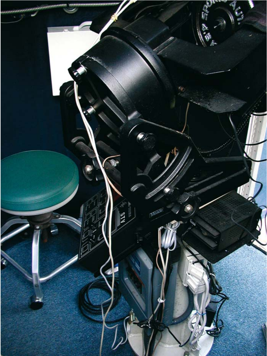
Figure 2.22. SBIG STV Deluxe camera control box mounted on pier shelf. Meade Superwedge is above, and three-breaker panel is below the STV display box. (Used with permission, Santa Barbara Instruments Group and Meade Instruments, respectively).
