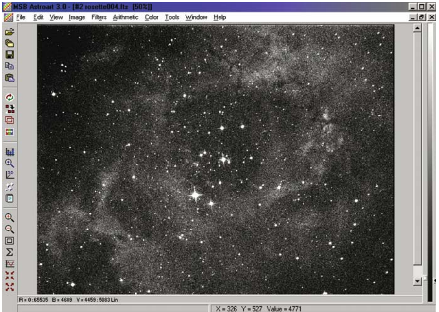
Figure 1.4. Astroait 3.0 screen capture. Single 300-s integration raw frame of the Rosette Nebula showing good nebulosity, captured with Astronomik 13-nm H \alpha filter. Diffraction spikes are artificial. Note the grainy background, indicative of noise, which can be removed with image processing. (Used with permission, MSB Software, Inc.)
