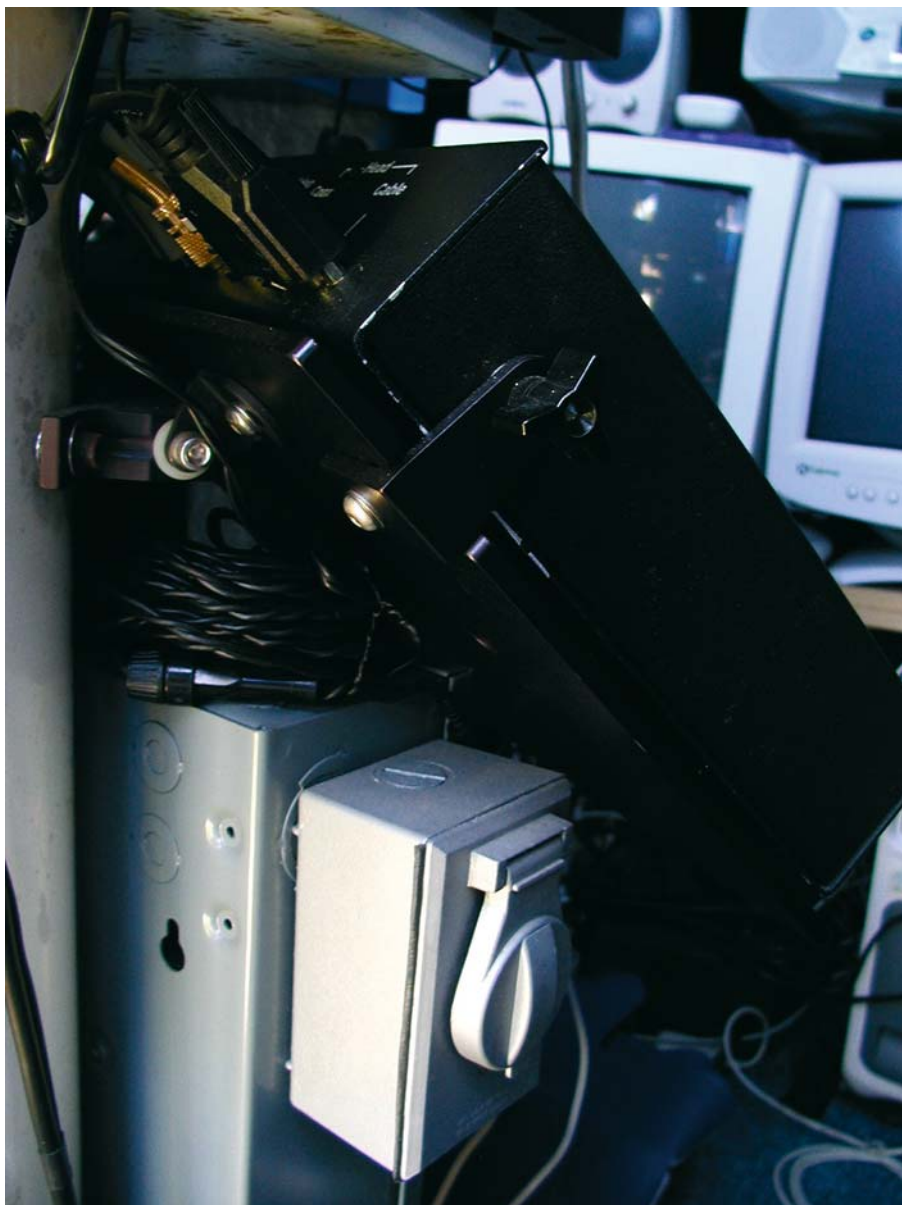
Figure 2.23. Greg Mueller (Mueller's Atomics) fabricated an SBIG STV control box bracket that allows the unit to fit nicely between the Meade Superwedge above and the circuit breaker panel below. White switch box controls a red bulb in the observatory, which preserves night vision.
