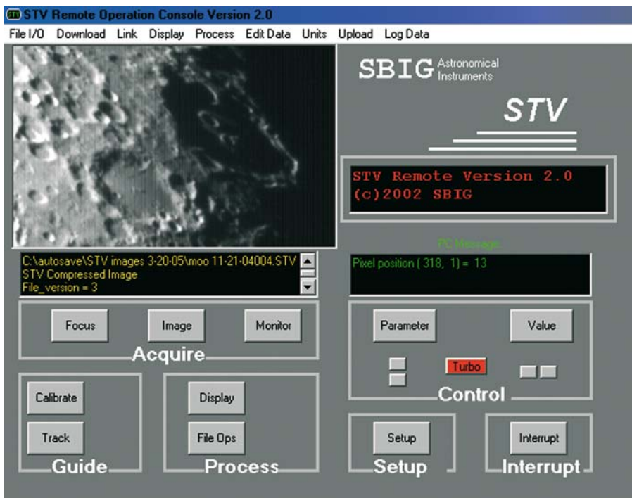
Figure 2.25. STV Deluxe screen capture. Using STV Remote version 2.0 software, an image of the moon has been captured and downloaded to the observatory computer, where it can be saved and further processed. (Used with permission, Santa Barbara Instruments Group).
