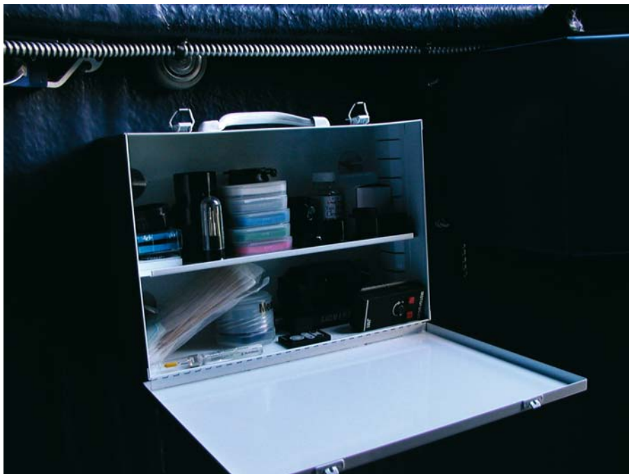
Figure 2.32. Accessory case mounted to observatory wall. Cover opens down and acts like a shelf.
