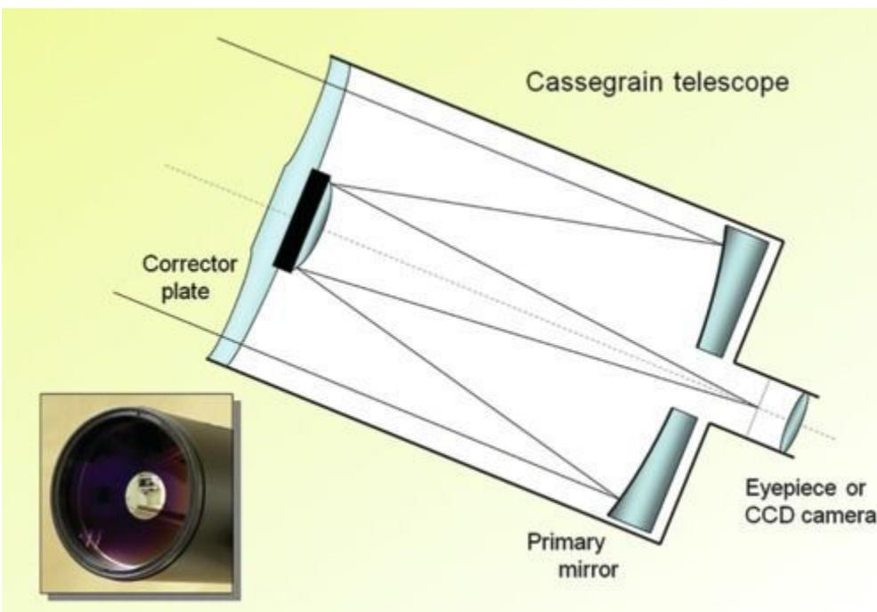
**Figure 5** The Schmidt-Cassegrain telescope. In this type of telescope there is a small secondary mirror in the centre of the front corrector plate. This secondary mirror reflects light back through a hole in the main primary mirror to the eyepiece or to a camera fitted at the rear of the telescope.
