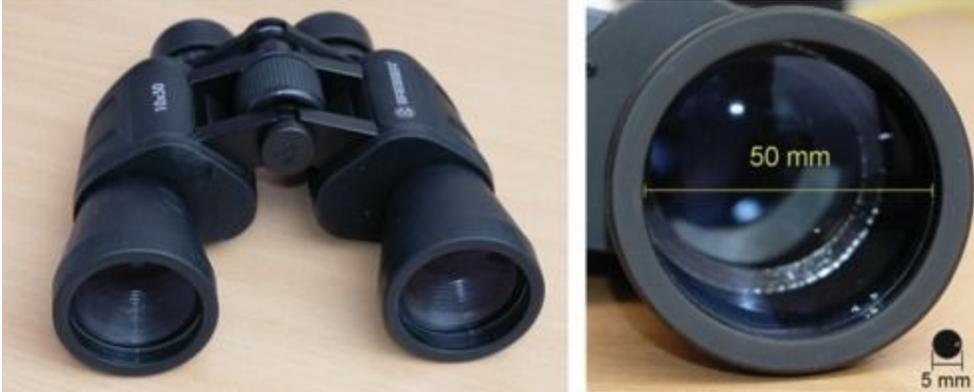
**Figure 3** Left: a typical pair of 10 × 50 binoculars. Right: comparison between the 50 mm objective lens of the binoculars and the 5 mm pupil of a typical eye. With ten times the diameter, the binocular lens has 100 times the area of the pupil, capturing 100 times as much light as the eye.
