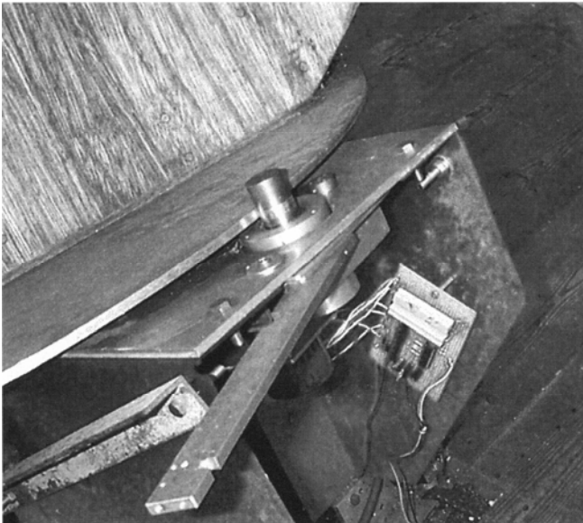
Figure 6.5 The friction RA drive
