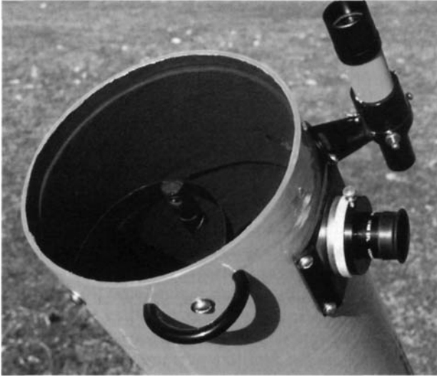
Figure 4.3 The open end of the telescope, showing the curved spider
