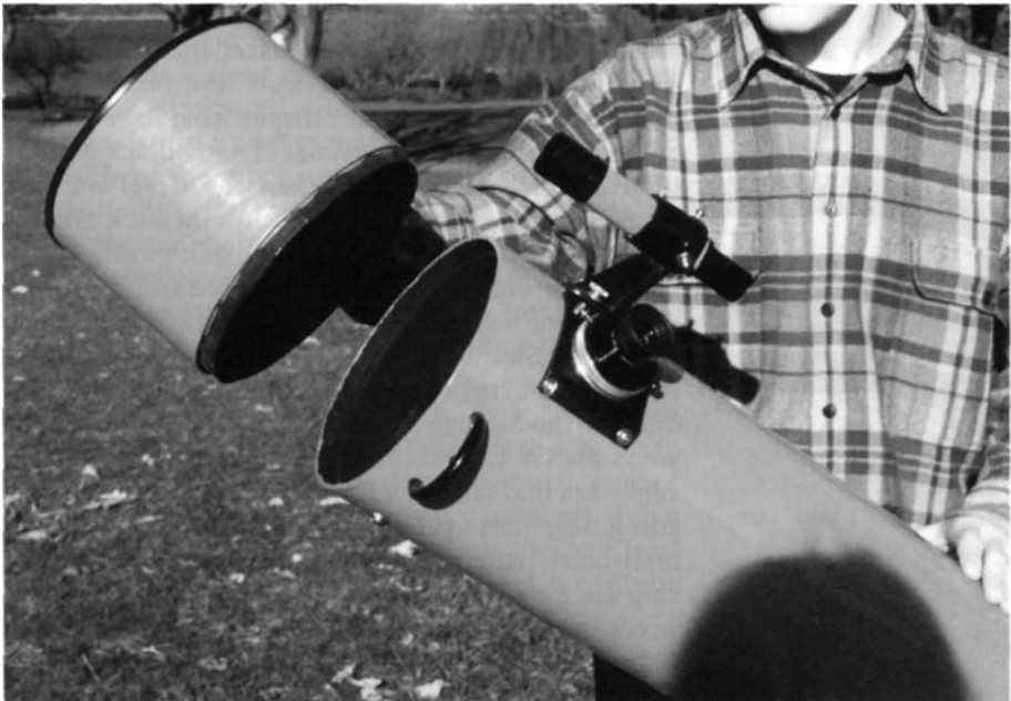
Figure 4.4 The removable tube extension
