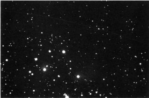
Figure 7.8 5× enlargement of a corner of an image of the Pleiades, showing off-axis performance of a Wright
