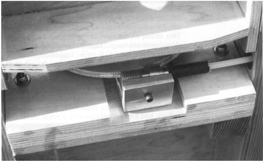
Figure 10.5 Altitude drive, viewed from underneath the baseboard.
