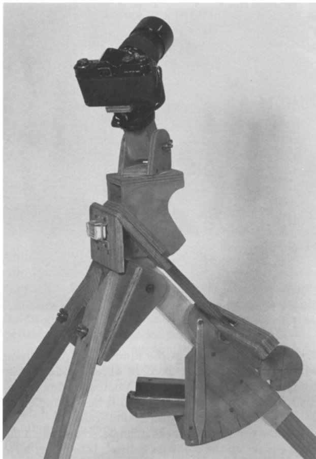
Figure 13.5 The latitude protractor ensures that skypod is at the right azimuth.
