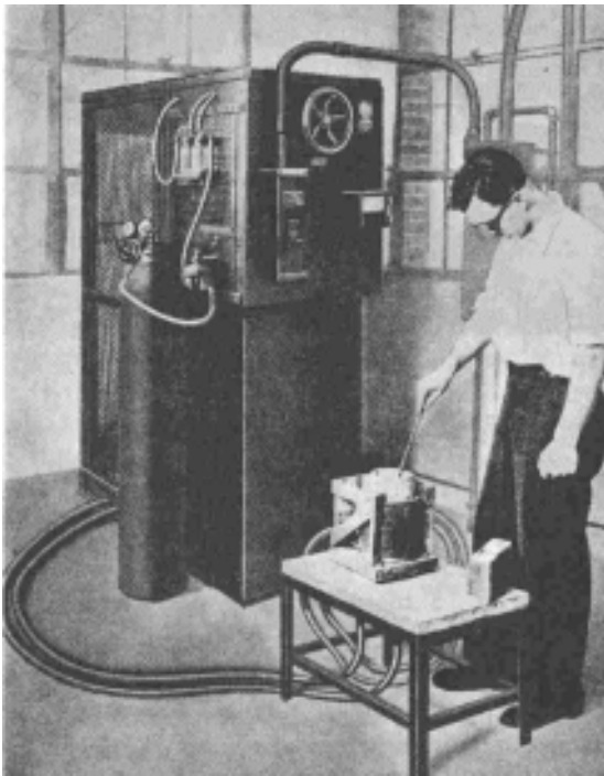
Ajax-Northrup High Frequency Induction Furnace. The converter is in the left background, the furnace proper in the foreground.
