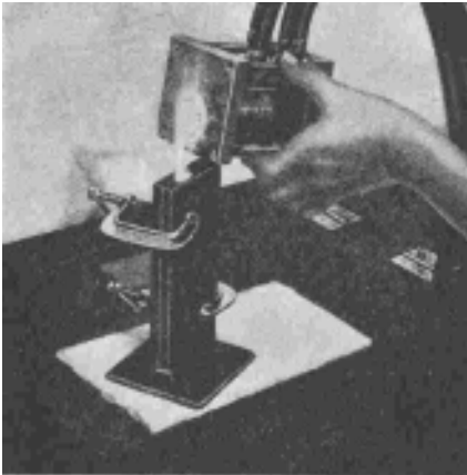
A very small Ajax-Northrup furnace. A type used in research work on the precious metals.
