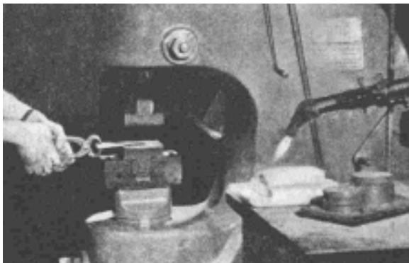
Hammering a block of hot platinum.
