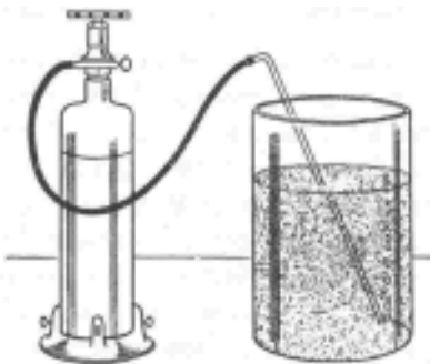
Precipitating gold with sulphur dioxide gas.
