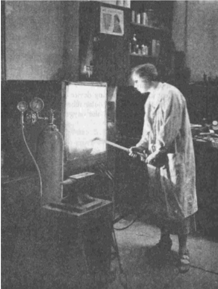
Melting platinum with the oxygen-gas torch.
