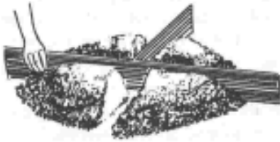
The dried material is piled in cones and quartered.
