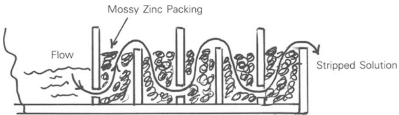
Figure 10-3 Basic zinc precipitation box
