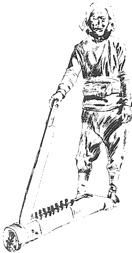
Chinese straw cutter (Shansi Province, Mainland China), with iron teeth to prevent straw slipping.
