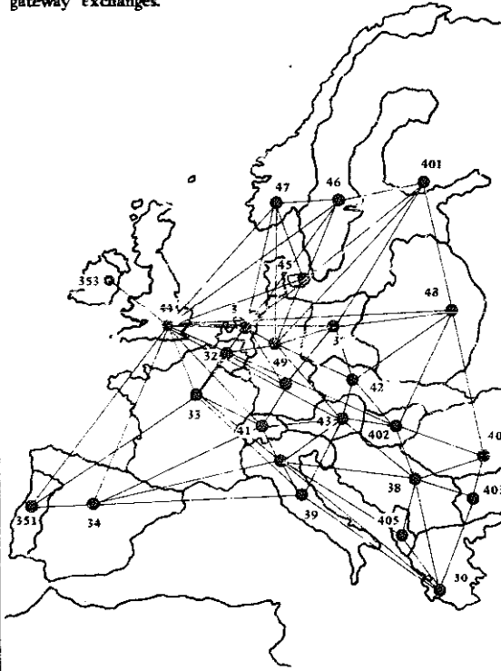
Fig 3. Interconnection pattern of West European 'gateway' exchanges.
