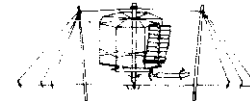
3b. Chinese clapper type windmill incorporating sail rig of Chinese junks. (From Science and Civilisation in China Vol. on Mechanical Engineering).
