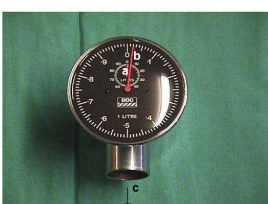
**3** Wright's respirometer. **a** Small pointer shows accumulated volume; **b** large pointer indicates tidal volume (it can be reset each breath); **c** to the breathing system.
