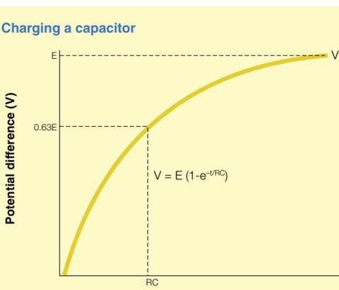
RC is the time constant, and is the time taken for the potential difference across the plates (V) to reach 63% ( $1 - e^{-1}$ ) of the value of the electromotive force of the power source (E)
