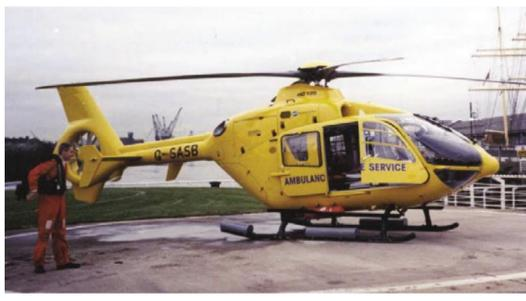
**5** The Scottish Ambulance Service EC 135 helicopter ambulance is unpressurized, which limits its altitude, affecting routing and fuel consumption and increasing the importance of weather conditions.
