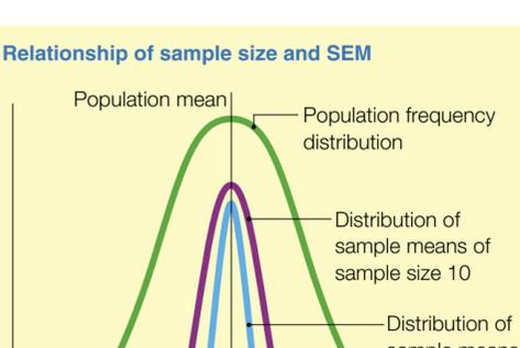
Standard error of the mean (SEM) =  $s/\sqrt{n}$ , where s is the standard deviation of the sample and n is the number of subjects in the sample
