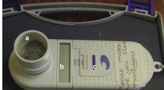
3 Hand-held electronic spirometer. a Mouthpiece, b display, c reset button.
