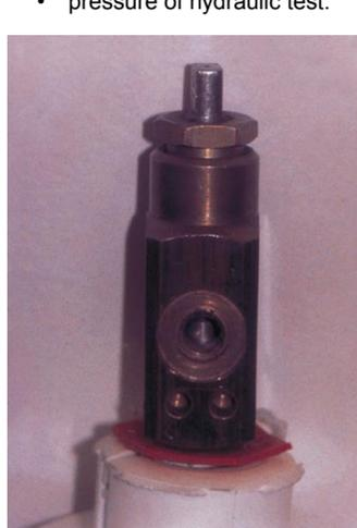
4 Pin-index valve holes on the cylinder.
