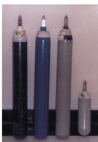
9 Cylinders. From left: oxygen, nitrous oxide, air, carbon dioxide.
