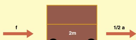
**c** If the force  $f$  is applied to an object of twice the mass ( $2m$ ) then it will accelerate at half the rate
