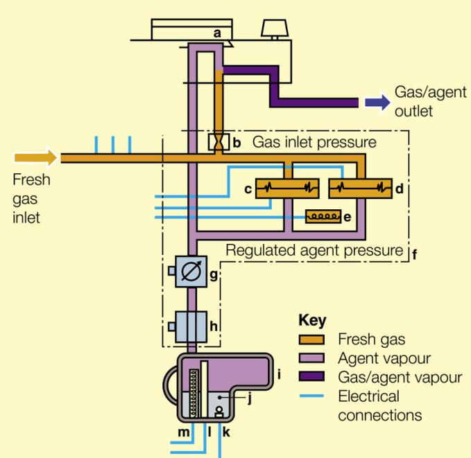
**a** Dial and rotary valve, **b** fixed restrictor, **c** pressure control transducer, **d** pressure monitor transducer, **e** heater in vapour control manifold, **f** vapour control manifold assembly, **g** pressure-regulating valve, **h** shut-off valve, **i** sump assembly, **j** agent, **k** level switch, **l** level sensor, **m** sump heaters
