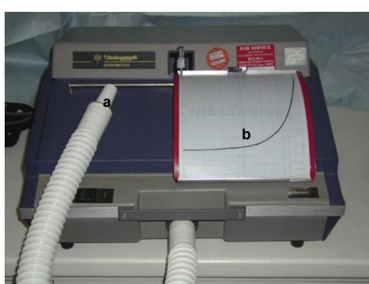
2 Vitalograph. a Mouthpiece, b spirometer trace.
