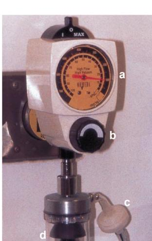
5 Vacuum control regulation unit. a vacuum gauge, b vacuum control, c filter, d float valve.
