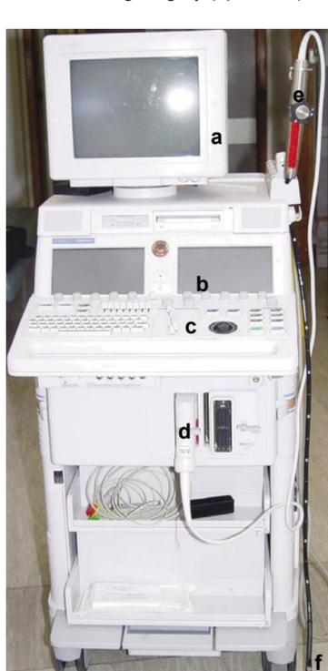
1 The echocardiography machine with a transoesophageal probe. **a** Echo display screen, **b** Touch screen control panel, **c** Data input track ball and control panel, **d** Transducer scan head, **e** Dial control for rotational probe, **f** Scan head.
