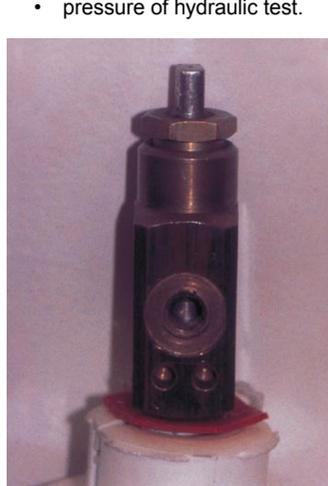
4 Pin-index valve holes on the cylinder.
