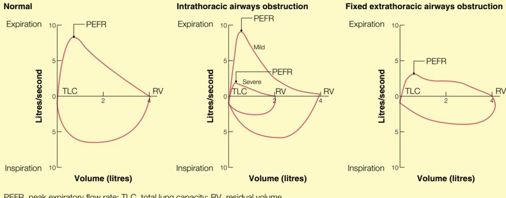
PEFR, peak expiratory flow rate; TLC, total lung capacity; RV, residual volume.
