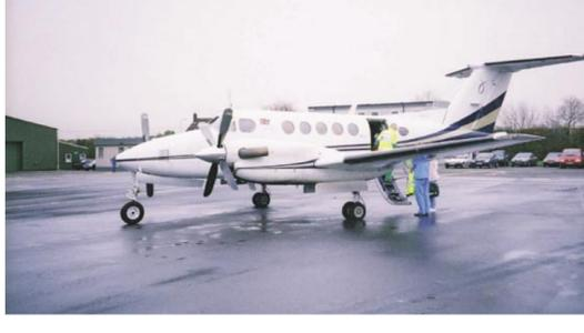
**6** The Scottish Ambulance Service Air King fixed wing air ambulance, which is pressurized and can therefore fly higher, above bad weather, faster and further than unpressurized air ambulances (e.g. the Islander).
