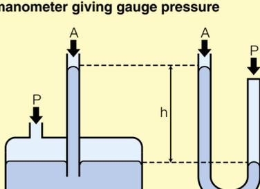
P, applied pressure; A, atmospheric pressure; h, measured pressure
