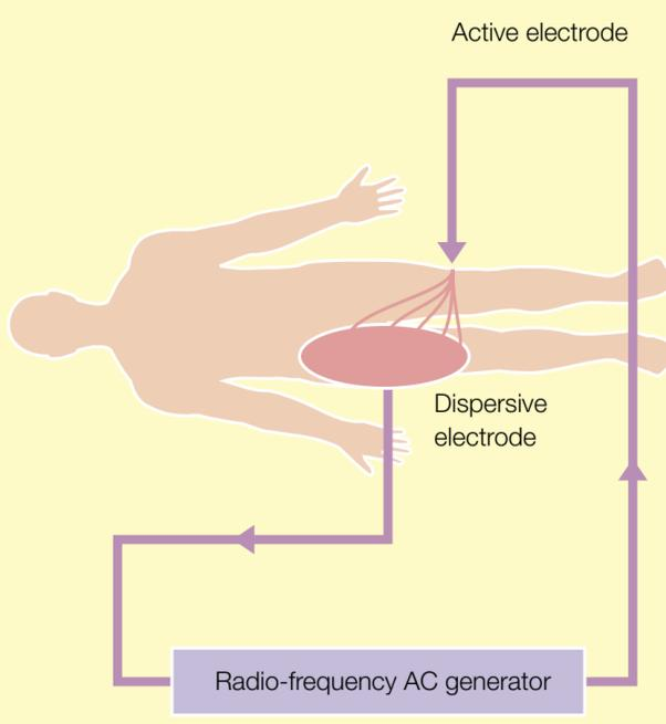
The tiny active electrode/tissue contact has a high resistance, therefore a high power is liberated ( $P = I^2 \times R$ ). Because this power is delivered to a small area, the power density, and ability to heat the tissue, is great. By contrast, the dispersive electrode, with its larger area of contact, has a low resistance and thus little power is liberated and it is distributed over a wide area, therefore the heating effect is negligible.
