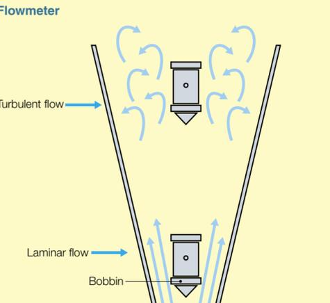
Laminar flow around the bobbin at the bottom of the tube, turbulent flow at the top. NB Pitch of the rotameter tube has been greatly exaggerated
