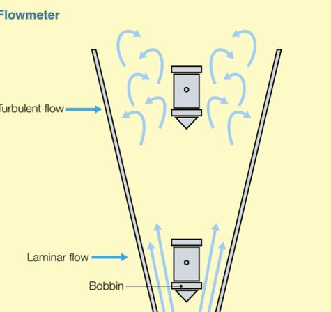
Laminar flow around the bobbin at the bottom of the tube, turbulent flow at the top. NB Pitch of the rotameter tube has been greatly exaggerated
