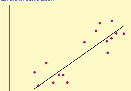
A statistically significant linear correlation in the whole sample can be calculated, but the data actually have a bimodal pattern, and within each subgroup there is no correlation of the two variables
