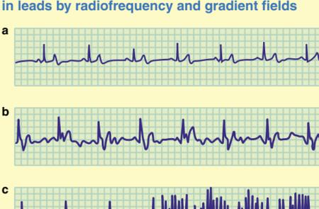
ECG with: **a** the subject outside the magnet bore; **b** the subject in the magnet bore (note the ST-T changes); and **c** the ECG trace during operation of the imaging sequence.
