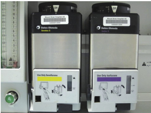
FIGURE 3-21 ■ Datex-Ohmeda Tec 5 vaporizers (GE Healthcare, Waukesha, WI) with a key-fill system.
