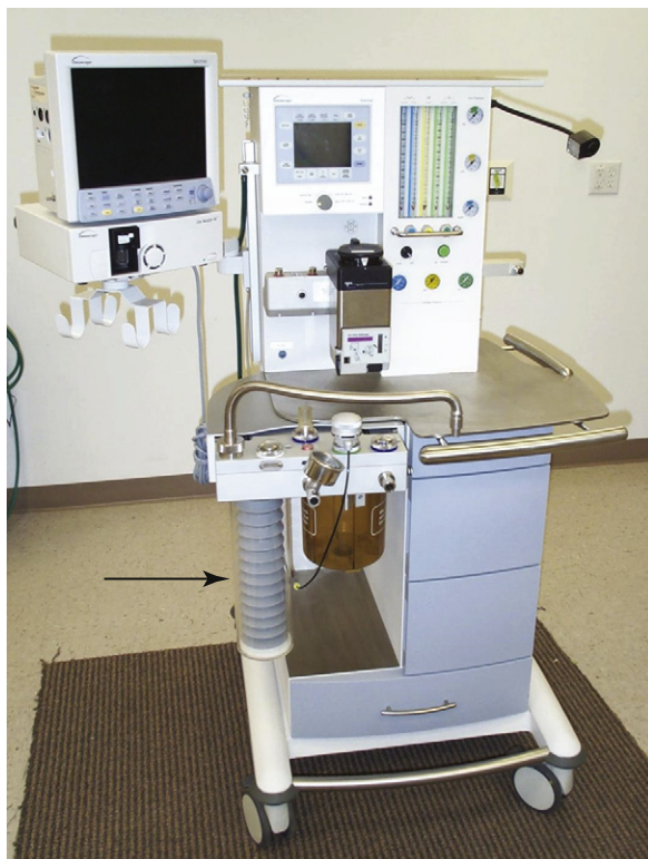
FIGURE 6-17 ■ Bag-in-a-bottle bellows design, descending bellows variety. Shown is the Datascope Patient Monitoring Anesthar anesthesia machine (Mindray North America, Mahwah, NJ) with descending bellows. The bellows ( arrow ) are in the inflated position.
