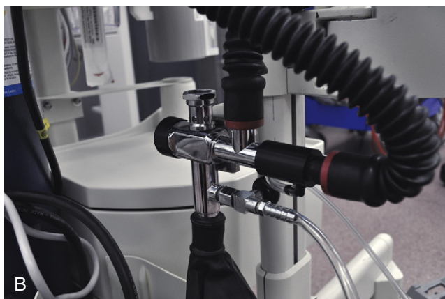
FIGURE 32-14 ■ Active “closed” scavenger assembly. Positive-pressure relief testing can be conducted as described for passive systems. Negative-pressure relief testing involves occluding the patient Y-piece after turning off all flow control valves and ensuring that circuit breathing pressure indicates only a negligible negative pressure (e.g., more than -1.0 cm H 2 O). Scavenger suction should be adjusted so the reservoir bag is neither overinflated or underinflated during routine use. (Modified from Operators instruction and setup manual: Narkomed M anesthesia system , Telford, PA, 2001, Dräger Medical.)
