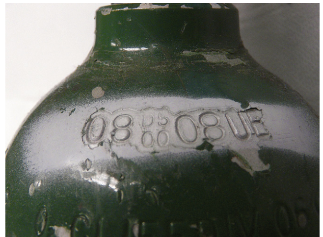
FIGURE 1-4 ■ An E-cylinder of oxygen. The inspection date, August 2008, has been painted white to indicate the cylinder was checked at the time it was delivered to the facility. All cylinders must be checked for leaks and structural integrity with an overpressure test at least once every 10 years.
