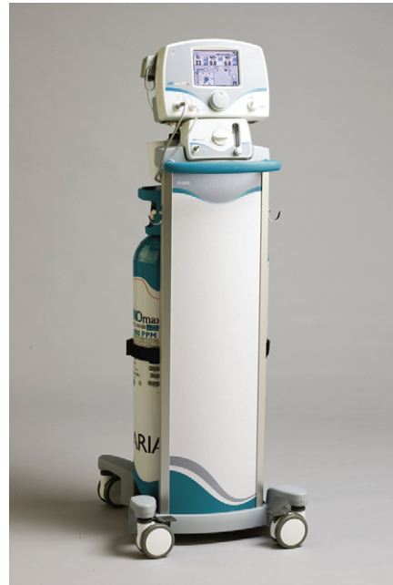
FIGURE 1-19 ■ Ikaria INOmax DS delivery system delivers a constant, operator-determined concentration of nitric oxide with sensors to detect oxygen, nitric oxide, and nitrogen dioxide. (Courtesy Ikaria, Hampton, NJ.)
