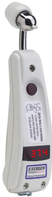
FIGURE 14-16 ■ Temporal Scanner (Exergen, Watertown, MA) infrared forehead temperature-measuring device, which scans the temporal artery.
