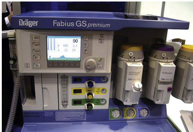
FIGURE 2-51 ■ The Fabius GS Premium workstation (Dräger Medical, Telford, PA). Note needle valve gas flow controls arranged vertically and the electronic display of virtual flowmeters. A total fresh gas rotameter flowmeter permits flow measurement in the event the electronic flow display fails.
