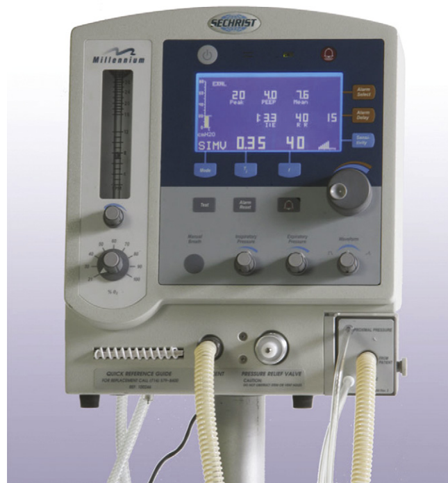
FIGURE 17-11 ■ The Sechrist Millennium neonatal/infant/pediatric ventilator. The ventilator can operate in the SIMV/IMV, Assist-Control, and back-up ventilation continuous positive airway pressure modes. IMV, intermittent mechanical ventilation; SIMV, synchronized intermittent mechanical ventilation. (Courtesy Sechrist Industries, Anaheim, CA.)
