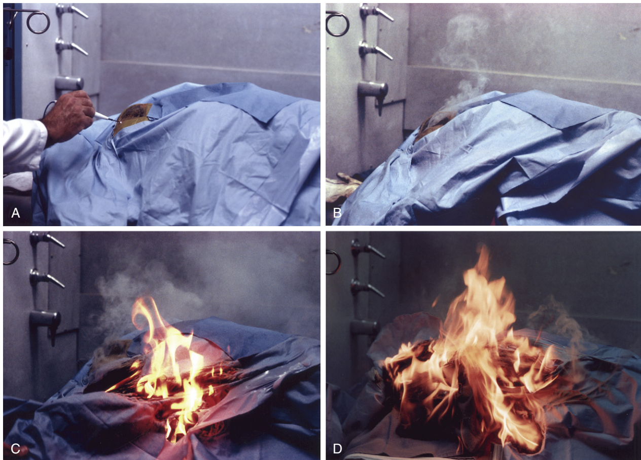
FIGURE 31-41 ■ Simulation of fire caused by electricosurgical unit (ESU) electrode during surgery. A, Mannequin prepared and draped for surgery. An ESU monopolar pencil electrode is applied to the operative site at the start of surgery. B, Six seconds after ESU application, smoke appears from under the drapes. C, Fourteen seconds after ESU application, flames burst through the drapes. D, Twenty-four seconds after ESU application, the patient’s head and drapes in flames. (From Barker SJ, Polson JS: Fire in the operating room: a case report and laboratory study. Anesth Analg 2001; 93:960. Used with permission.)
