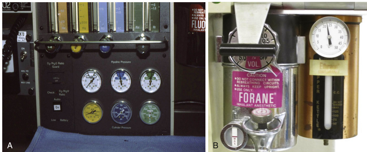
FIGURE 3-6 ■ Copper Kettle vaporizing system (Puritan-Bennett; Covidien, Mansfield, MA). A , The oxygen flowmeter knob on the extreme left is marked “C-K” to indicate that it controls oxygen flow to the Copper Kettle. B , Close-up of the Copper Kettle.
