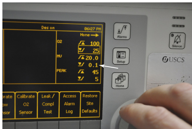
FIGURE 32-5 ■ Setting machine alarm limits. Alarm limit values are easy to adjust, although this task could be time consuming during routine preuse checkout. Safe default values can be established locally and set by trained technicians, which will help keep limits consistent. Note the inappropriately low minute ventilation threshold default on this machine (arrow).
