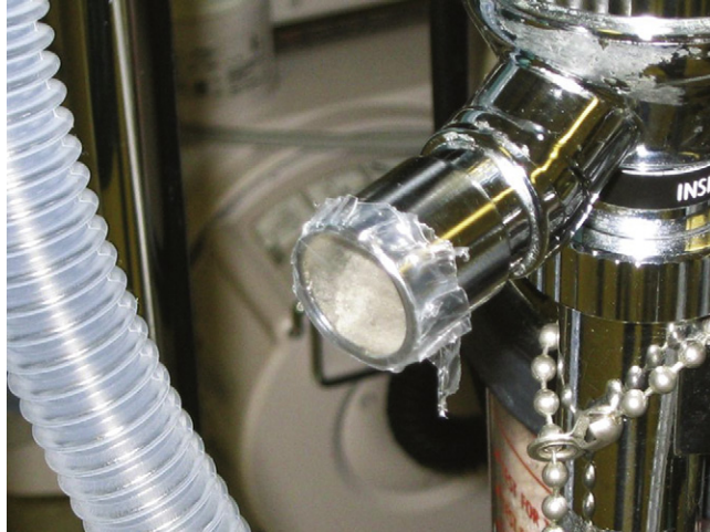
FIGURE 30-13 ■ Disposable circuit with plastic packaging intact. Plastic that is not removed before connecting the circuit to the inspiratory port on the absorber canister would cause complete obstruction to inspiration.
