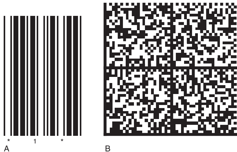
FIGURE 18-18 ■ Bar codes can be verified with many bar code scanning programs available on smart phones in addition to standard bar code scanners. A , The simpler bar code on the left contains the number “1.” B , The MaxiCode on the right contains the nursery rhyme “Mary Had A Little Lamb.”
