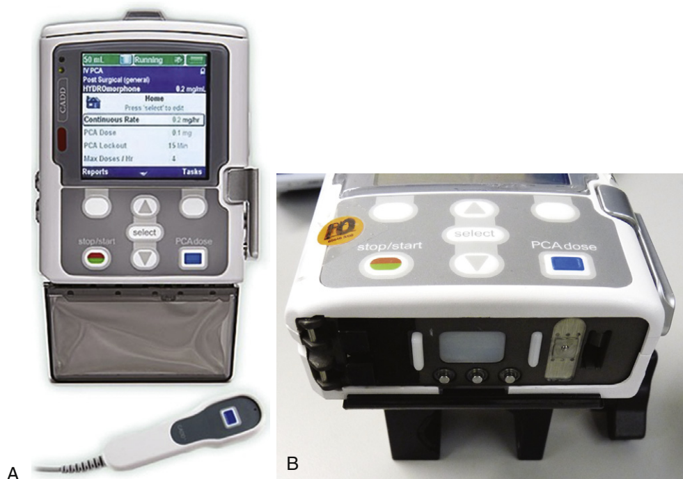
FIGURE 18-15 ■ A , CADD-Solis ambulatory infusion pump (Smiths Medical, St. Paul, MN) with external patient-controlled analgesia dose button. B , Pump showing the cartridge area.
