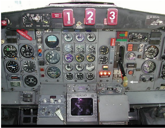
FIGURE 24-13 ■ Cockpit of a Boeing 727. The lever with a wheel on the end that controls the landing gear is shown (arrow). Note the three red switches labeled 1-2-3, which control the fire extinguishers for the three engines. (Photo copyright by Mike Olson, used with permission. Accessed at www.airliners.com .)
