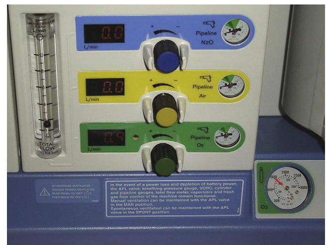
FIGURE 2-31 ■ Front view of a Dräger Fabius GS workstation (Dräger Medical, Telford, PA) showing a vertical arrangement of the flow control knobs. The knobs are less susceptible to accidental changes in flow by the protective half-sleeves on either side of each knob (compare with Fig. 2-30).
