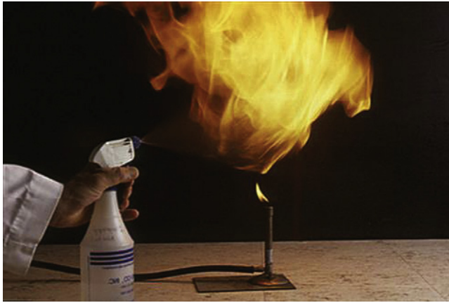
FIGURE 31-42 ■ A demonstration of the intense heat and flame present in an alcohol fire. (Photograph courtesy Marc Bruley, ECRI Institute. Reprinted with permission. Copyright 2009, ECRI Institute, www.ecri.org.)
