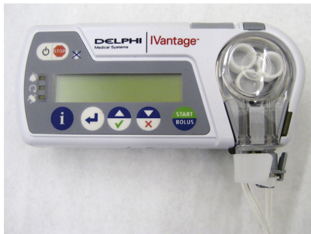
FIGURE 18-6 ■ The Delphi IVantage (Delphi Medical Systems, Longmont, CO) rotary peristaltic pump mechanism.
