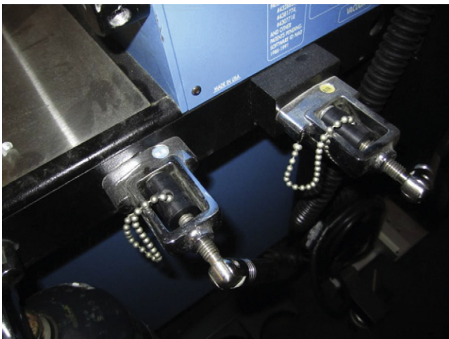
FIGURE 2-13 ■ Yoke plugs in unused tank hanger yokes.
