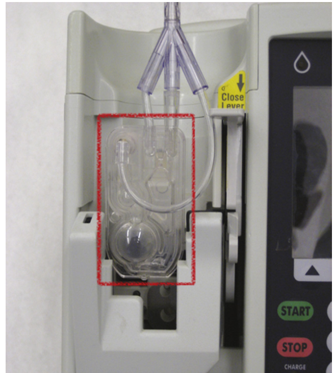
FIGURE 18-9 ■ The Abbot Plum A+ cassette (Hospira, Inc., Lake Forest, IL) removed from the pump.
