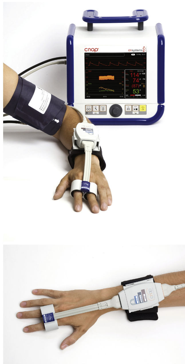
FIGURE 12-7 ■ A , The CNAP Monitor 500 with arm and finger blood pressure cuffs. B , The CNAP monitor double finger cuff and transducer. (Courtesy CNSystems Medizintechnik AG, Graz, Austria.)
