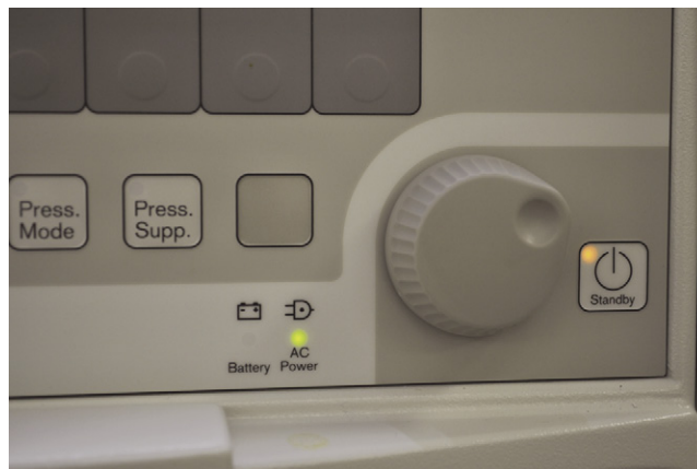
FIGURE 32-4 ■ Machine connection to alternating current (AC) power should be confirmed during preuse checkout procedures. Abrupt system failure could occur during battery-powered operations.
