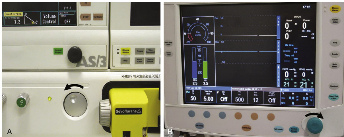
FIGURE 30-19 ■ A , Aladin vaporizer concentration dial on Datex ADU workstation (GE Healthcare, Waukesha, WI) is turned counterclockwise to increase agent concentration. B , Aladin vaporizer concentration dial on GE Aisys Carestation is turned clockwise to increase agent concentration.
