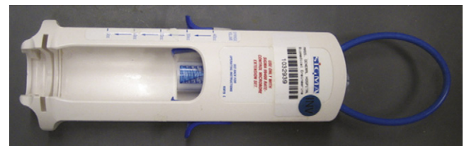
FIGURE 18-13 ■ Sigma Multidoser spring-powered syringe pump (Baxter, Deerfield, IL) without a syringe installed.
