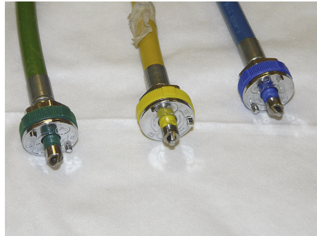
FIGURE 1-23 ■ Common types of quick couplers used in hospitals. Note that each has a specific pin configuration for the individual gas. The quick coupler and the attached hose should be color coded for the specific gas.
