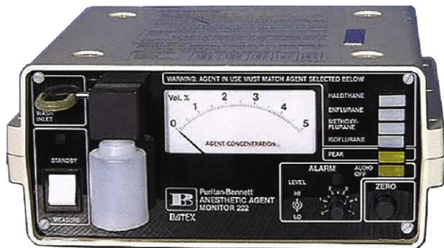
FIGURE 8-11 ■ Datex Puritan-Bennett anesthetic agent analyzer. This analyzer uses a single wavelength, so the agent being measured must be entered into the software by the user; failure to do this results in erroneous readings. Note the warning: “Agent in use must match agent selected below.” Keypads on the right are for selection of halothane, enflurane, methoxyflurane, or isoflurane.
