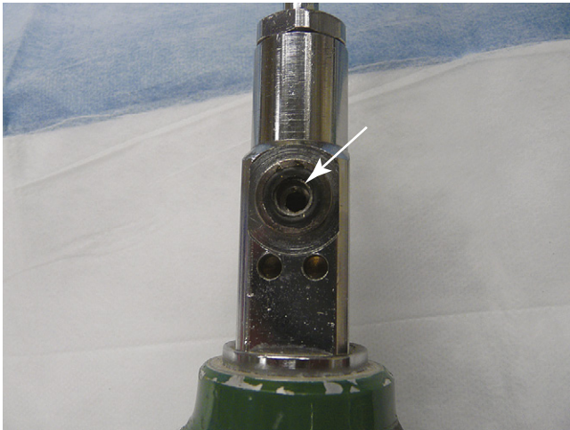
FIGURE 1-8 ■ Cylinder valve at the top of an E-cylinder shows the two holes for the pin index system and the outlet port with an attached washer (arrow).
