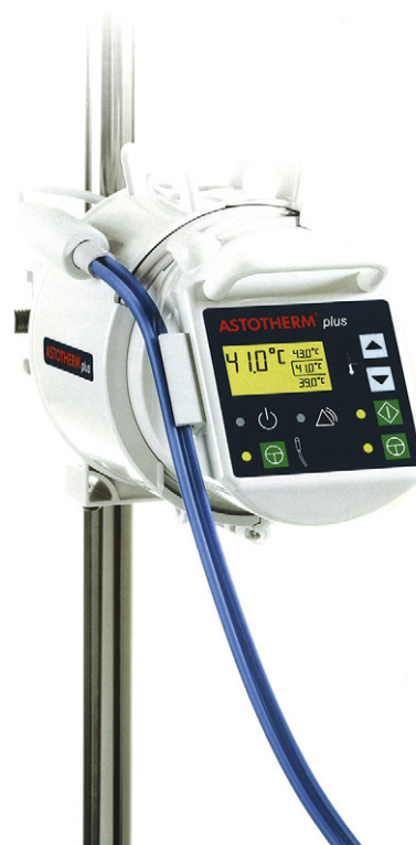
FIGURE 14-8 ■ The Astotherm device (Futuremed America, Granada Hills, CA). The fluid pathway is warmed by inserting the tubing in a series of grooves in a drumlike device that delivers heat to the fluid as it courses through the tubing.
