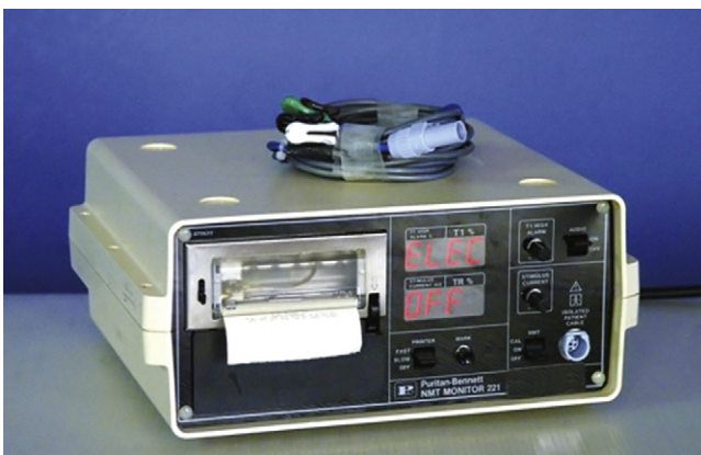
FIGURE 15-19 ■ Datex Relaxograph Neuromuscular Transmission electromyography monitor has an output that shows digital twitch height ( T_1\% ) and train-of-four ratio ( T_4\% ). A sample paper tracing is shown on the left side of the device.
