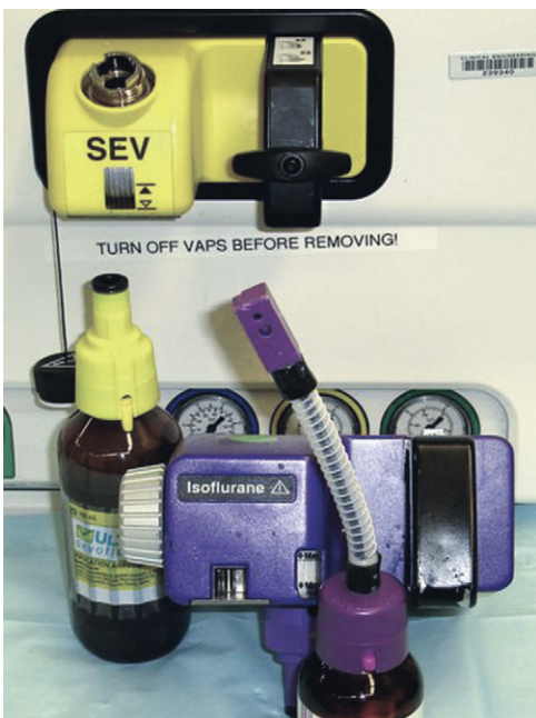
FIGURE 3-12 ■ Agent-specific filling devices for sevoflurane (yellow; Quik-Fil, Abbott Laboratories, Abbott Park, IL) and isoflurane (purple; Key-Fill, Harvard Apparatus, Holliston, MA).
