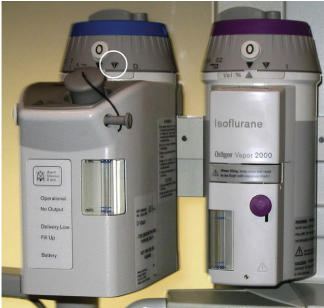
FIGURE 3-20 ■ Dräger Vapor 2000 vaporizers (Dräger Medical, Telford, PA). The white circle indicates transport mode (T) on the concentration dial.
