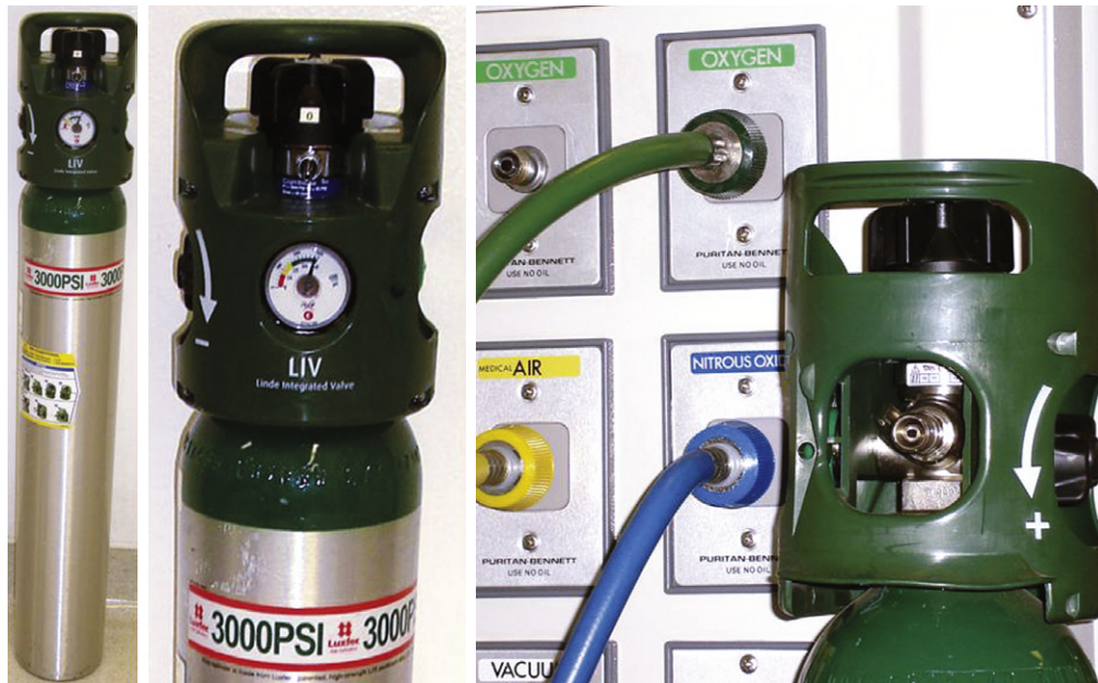
FIGURE 2-11 ■ Left , Oxygen tank pressurized to 3000 psig when filled. Right , The tank valve incorporates a regulator with a diameter index safety system (DISS) oxygen connector that supplies oxygen at 50 psig. The anesthesia machine oxygen hose is shown connected to a DISS wall outlet for oxygen.
