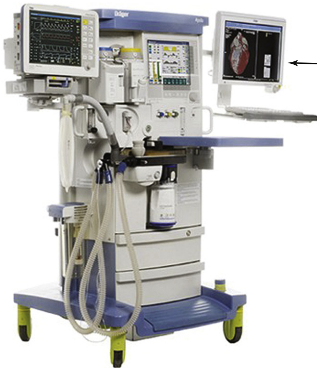
FIGURE 23-22 ■ Integrated anesthesia workstation displays. New technology will take advantage of powerful microprocessors and improved understanding of the human physiologic response to anesthesia to present clinical data in a more intuitive and relevant manner. Note the logical positioning of redundant information. Animation could be used (e.g., a beating heart, arrow ) to provide increased information content that would obviate the need for waveform displays. Trending of data (not shown) could also be readily incorporated into the display. (Courtesy Dräger Medical, Telford, PA.)
