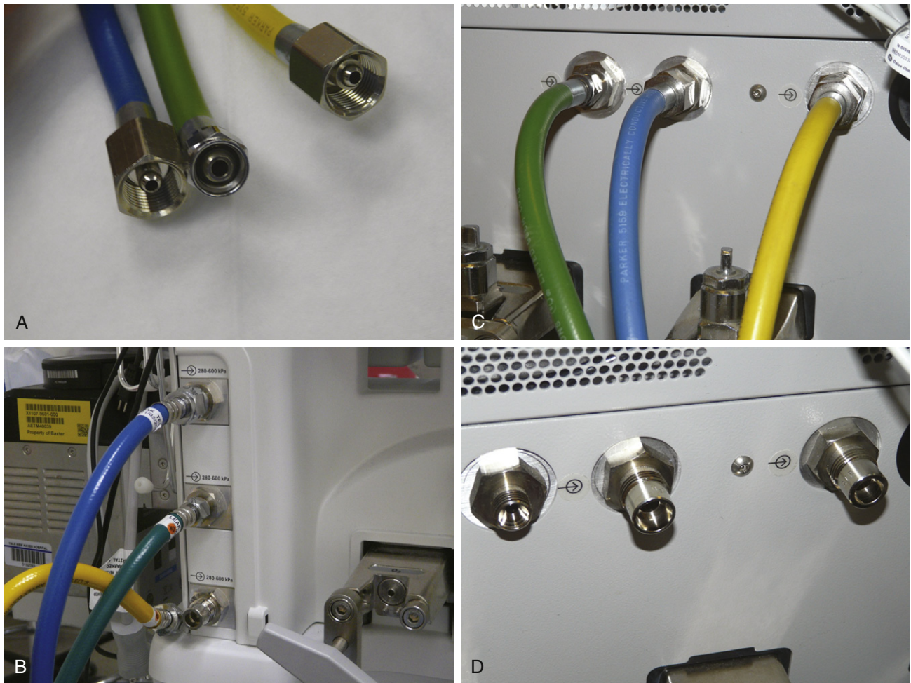
FIGURE 1-25 ■ A , Examples of hoses with the diameter index safety system (DISS). These are threaded connections in which the diameters of the threads are specific for each of the gases. B and C , Connections made to DISS fittings on the anesthesia machine. D , DISS fittings on an anesthesia machine.
