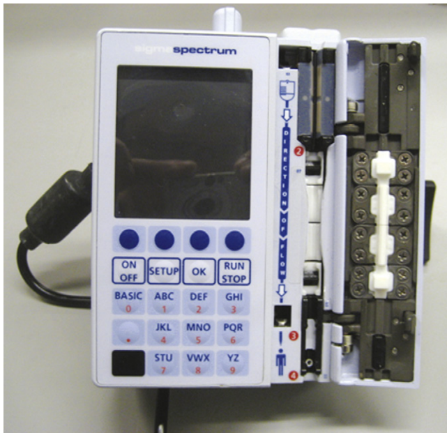
FIGURE 18-4 ■ The Sigma Spectrum (Baxter, Deerfield, IL) large volume, linear peristaltic infusion pump, shown with the mechanism door open.
