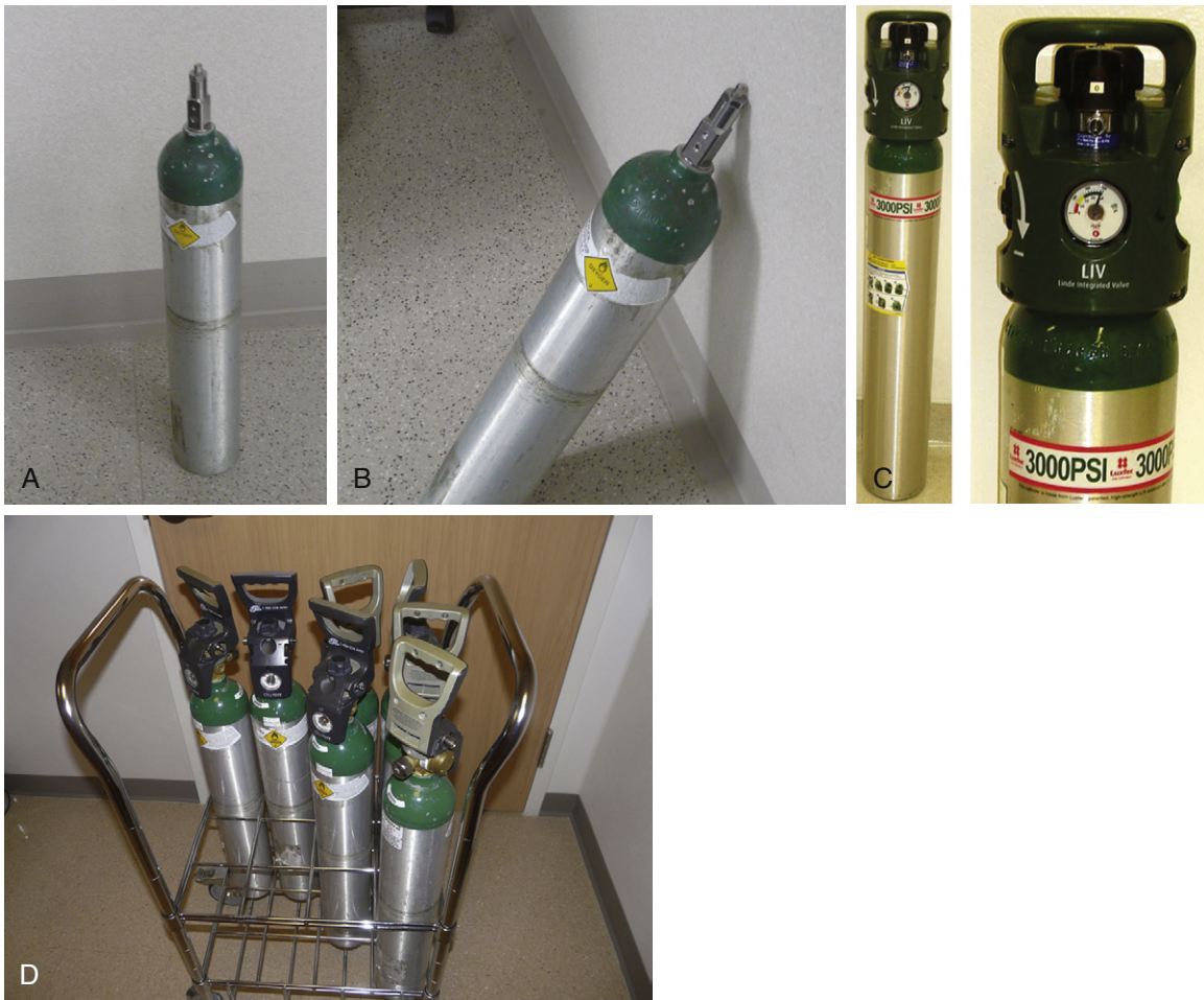
FIGURE 1-9 ■ A , Gas cylinders must never be left standing upright and unsecured. They are vulnerable to being knocked over easily, such as by opening a door. Cylinders that fall directly to the floor, and especially cylinders that fall so that the top hits a wall ( B ), are at great risk for breaking at the cylinder neck. This creates a dangerous “unguided missile,” in which the high-pressure gas escapes out the narrow neck and rockets the cylinder forward with enough force to penetrate a brick wall. C , Oxygen cylinders are now available with a maximum pressure of 300 psi and a capacity of 1000 L of oxygen. These would present an even greater hazard if ruptured. D , If upright, individual cylinders should be secured in some type of holder, such as a rolling stand for E-sized cylinders.
