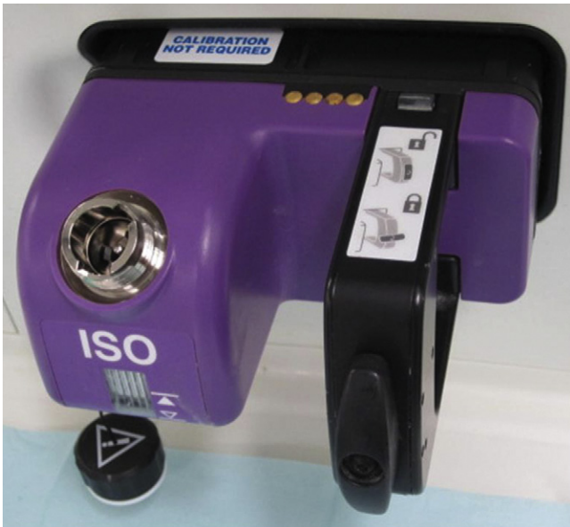
FIGURE 3-34 ■ Aladin vaporizer system (GE Healthcare, Waukesha, WI) isoflurane cassette. The workstation recognizes the agent-specific cassette by the arrangement of identification (signature) magnets (see Fig. 3-35).
