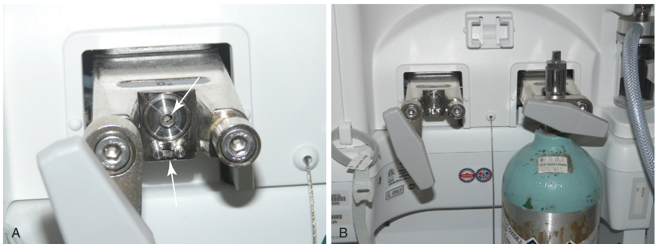
FIGURE 1-7 ■ A , Cylinder yoke on the anesthesia machine. Note the two pins for the pin index system at the bottom of the yoke ( bottom arrow ) and the hole ( top arrow ; not gas specific) that aligns with the outlet port of the tank. B , Oxygen yoke with the tank removed and the N 2 O tank in place.
