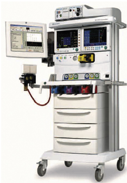
FIGURE 2-45 ■ GE Healthcare (Waukesha, WI) ADU workstation. The next step in evolution: electronic flow sensing, virtual flowmeters, and an electronically controlled vaporizing system.
