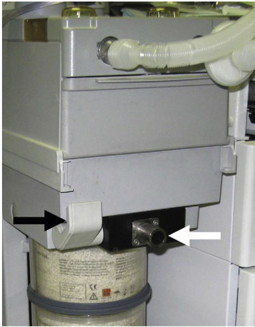
FIGURE 2-37 ■ Auxiliary common gas outlet ( white arrow ) on a Datex-Ohmeda Aestiva/5 machine (GE Healthcare, Waukesha, WI). This outlet is enabled and the connection to the circle system is disabled by pressing down the lever ( black arrow ) to the left of the outlet. This outlet is used to perform the low-pressure system leak check or to connect a noncircle system.
