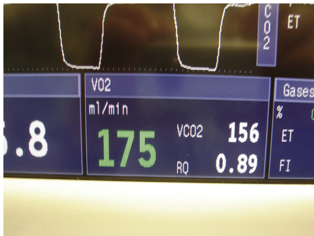
FIGURE 8-28 ■ Screen of Datex-Ohmeda S5 Compact Airway Module monitor (GE Healthcare, Waukesha, WI). Metabolic monitoring data ( \text{VO}_2 , \text{VCO}_2 , RQ) are shown from integrating concentration and flow signals.
