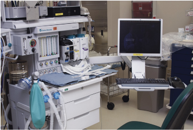
FIGURE 22-18 ■ Computer workstation mounted to an anesthesia machine. The mount allows flexibility in placement of the monitor and keyboard in relation to the machine. The computer's central processing unit is placed on the shelf adjacent to the anesthetic gas analyzer. Alternate configurations place the monitor and keyboard tray to the left of the anesthesia machine.
