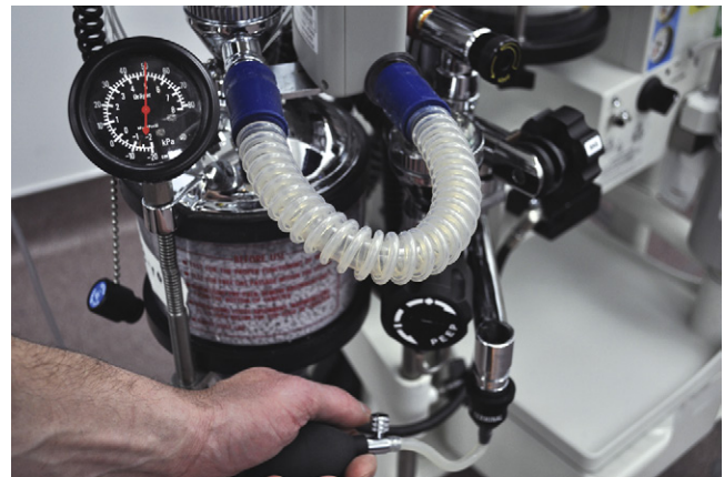
FIGURE 32-10 ■ Dräger (Telford, PA) positive-pressure breathing system leak test specified for the Narkomed 2, 3, 4, GS & M model anesthesia workstations. This particular procedure uses a sphygmomanometer bulb with bag-mount adapter and a length of tubing that short circuits inspiratory and expiratory ports. The test is negative if bulb-generated pressure decreases no more than 20 cm H 2 O from 50 cm H 2 O in 30 seconds.
