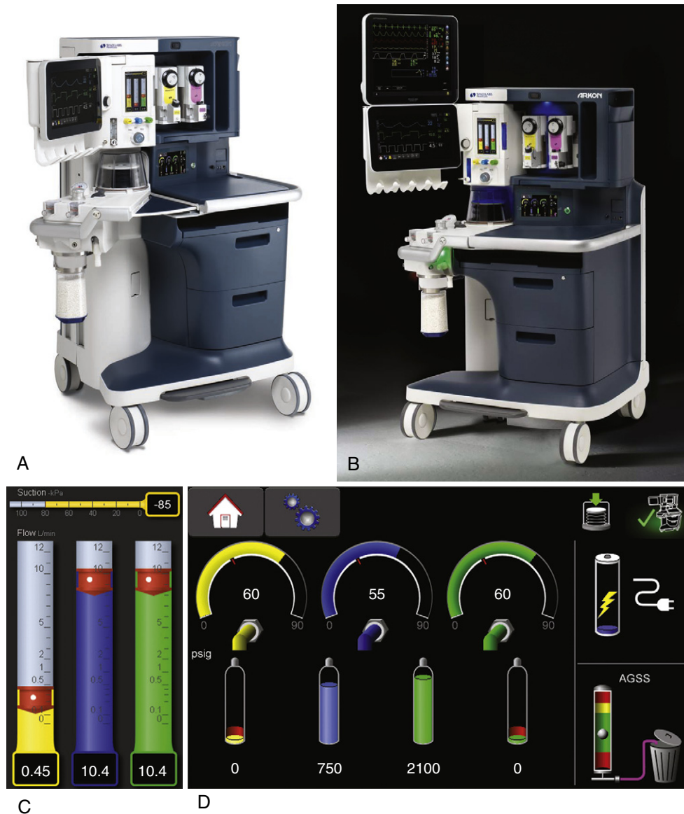
FIGURE 24-16 ■ A , The Arkon Anesthesia System (Spacelabs Healthcare, Issaquah, WA). B , Use of lighting for various functions; a red light is illuminated when the CO 2 absorber is out of the circuit. The green light next to the absorber indicates that the alternate fresh gas flow outlet is in use. The blue lights show that the ventilator is being used, the vaporizer has been turned on, or that the auxiliary oxygen flowmeter is in use. C , The gas flow controls have knobs that control a computer graphic display. Each gas has a red bobbin at the top that spins to simulate a traditional flowmeter. As the knob is turned counterclockwise, the flow increases, and a color-coded bar is filled in below the bobbin. D , The dashboard display. Wall supply pressures are clearly displayed. Below these are the reserve tank pressures and a graphic display of how much gas is in each tank. For example, the oxygen cylinder on the left is full, and the one on the right is empty. Other items displayed are whether the anesthesia gas scavenging system (AGGS) has sufficient vacuum, the charge of the backup battery and whether it is plugged in to charge, and whether a preuse check has been done (check mark next to the machine icon). The green arrow above the bellows icon shows that the ventilator driving gas is O 2 (the arrow would be yellow if air was being used as the driving gas).
