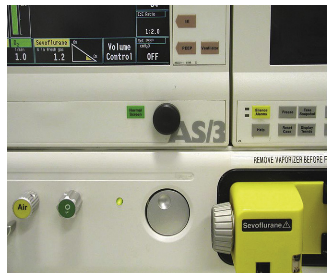
FIGURE 3-32 ■ Aladin vaporizer system (GE Healthcare, Waukesha, WI) used on the AS/3 Anesthesia Delivery Unit and Aisys workstations.
