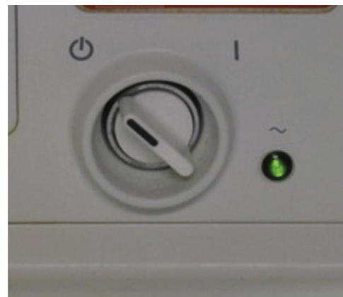
FIGURE 2-55 ■ Main ON/OFF switch. Care must be taken to not accidentally shut down the workstation.
