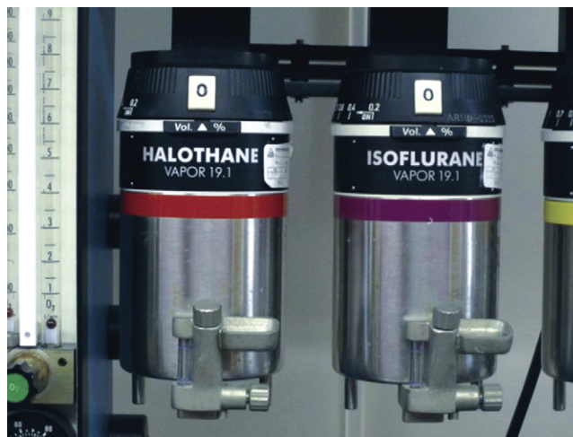
FIGURE 3-18 ■ Dräger Vapor 19.1 vaporizers (Dräger Medical, Telford, PA). Note the funnel-fill design, which has been superseded by an agent-specific key-fill design.
