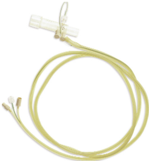
FIGURE 8-35 ■ Combined proximal flow sensor with sidestream gas sampling (D-Lite, GE Healthcare, Waukesha, WI). D-Lite and Pedi-Lite, a pediatric sensor, are available in both reusable (polyphenylsulfone) and disposable (polystyrene) versions. (Courtesy GE Healthcare, Waukesha, WI.)
