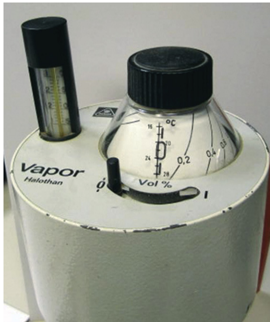
FIGURE 3-10 ■ In the Dräger Vapor vaporizer (Dräger Medical, Telford, PA), temperature compensation is achieved by reading the temperature from the thermometer and using the control dial to align the desired output concentration (slanting) line with the marking for ambient temperature.
