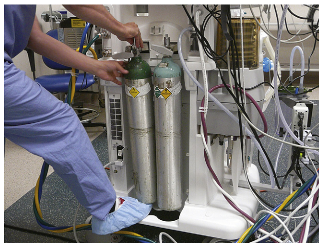
FIGURE 1-10 ■ Proper method for attaching an E-cylinder to the yoke of an anesthesia machine. The tank is first supported on the anesthesiologist’s foot while the holes on the tank are aligned with the pins in the yoke. The tank is then slid into place on the yoke, and the T-handle is tightened to make a gas-tight seal.
