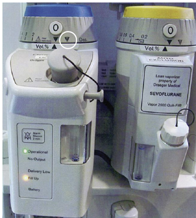
FIGURE 3-29 ■ Left, Dräger D-Vapor vaporizer for desflurane (Dräger Medical, Telford, PA). Right, Dräger Vapor 2000 sevoflurane vaporizer. The white circle indicates transport (T) setting.
