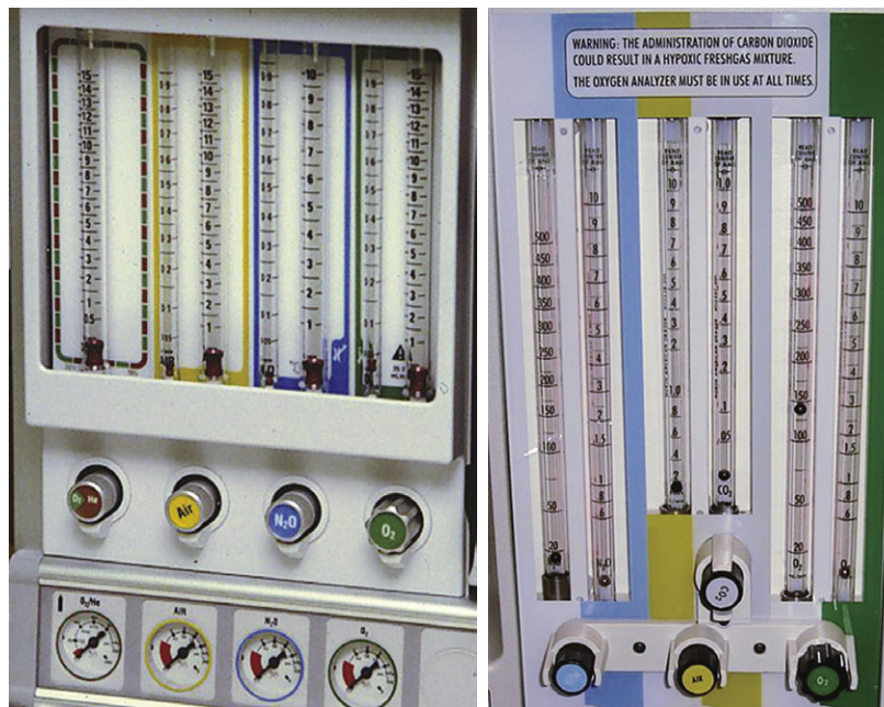
FIGURE 2-28 ■ Flowmeter banks on a four-gas Datex-Ohmeda (GE Healthcare, Waukesha, WI) anesthesia machine (left) and a four-gas Dräger Medical (Telford, PA) machine (right). Flowmeters for each gas are arranged in series. The oxygen flows first through a rotameter, where low flows (<1 L/min) are measured, and then through a rotameter, where high flows (<10 L/min) are measured. In the United States, the oxygen flowmeters are on the right side of the flowmeter bank when viewed from the front. One gas flow control knob is present for each gas, even if there are two (low and high) flowmeter tubes for that gas.
