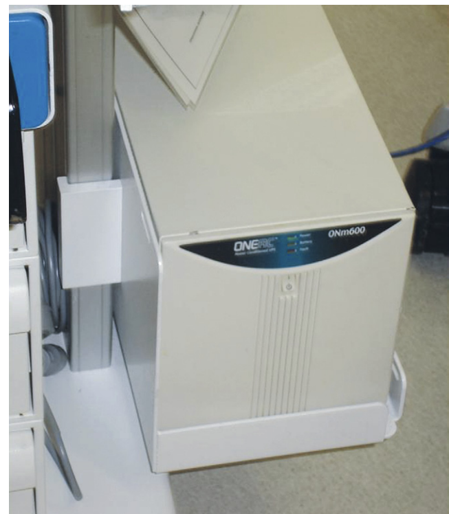
FIGURE 30-21 ■ Uninterruptible power supply unit.
