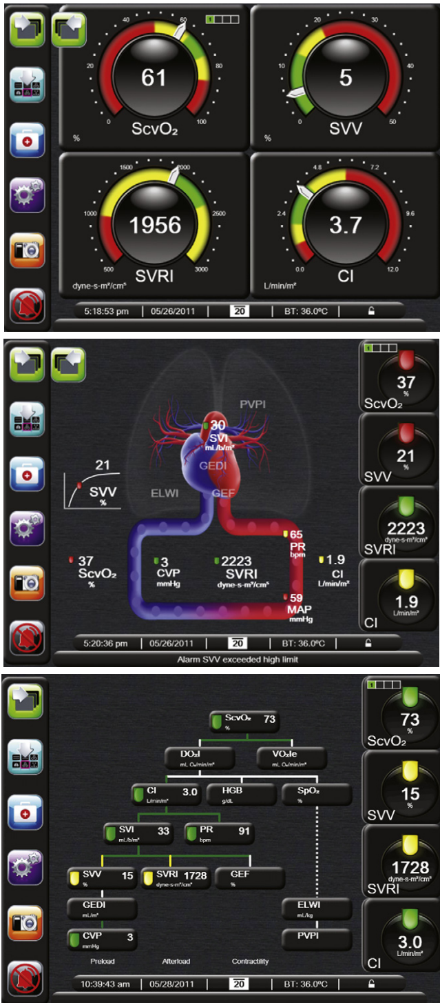
FIGURE 23-14 ■ More advanced displays of physiologic and hemodynamic data use color and shape to call attention to changes as well as to depict relationships among the displayed variables. (Courtesy Edwards Lifesciences, Irvine, CA.)
