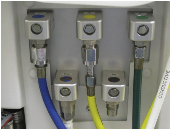
FIGURE 2-6 ■ Diameter index safety system hose connections to workstation pipeline supply connections.
