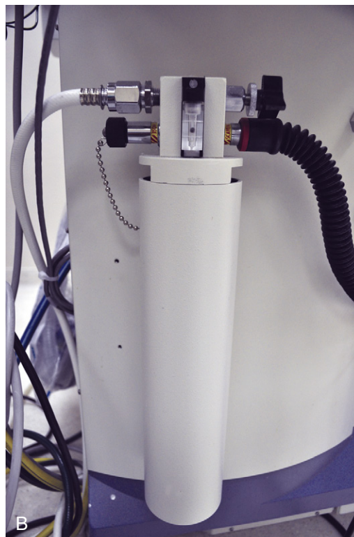
FIGURE 32-15 ■ “Open” scavenger assembly. The preuse check involves ensuring that gas flows freely from the patient breathing circuit into the scavenger and that the vacuum flow to the scavenger is adequate. (Modified with permission from Operating principles of Narcomed anesthesia systems , ed 2. Telford, PA, 1998, North American Dräger. Courtesy Dräger Medical.)
