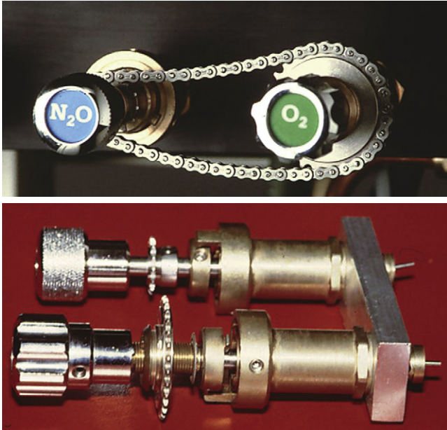
FIGURE 2-32 ■ Datex-Ohmeda Link-25 Proportion Limiting System (GE Healthcare, Waukesha, WI). Top: Front view of flow control knobs, sprockets (N 2 O, 14 teeth; O 2 , 29 teeth), and stainless-steel link chain. Bottom: Side view shows N 2 O sprocket fixed on the spindle, whereas the O 2 sprocket can move on the threaded O 2 spindle, like a nut turning on a bolt.
