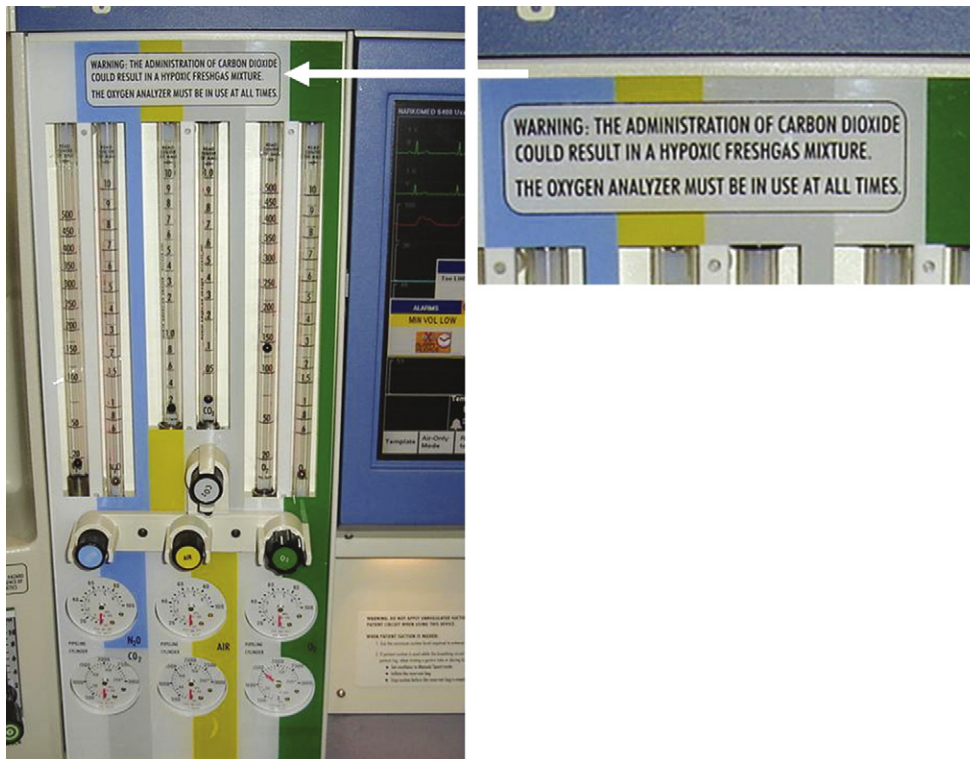
FIGURE 30-6 ■ Anesthesia workstation with CO 2 flowmeter. Note the warning label above the rotameter bank.
