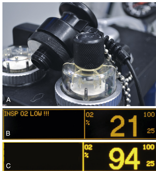
FIGURE 32-16 ■ Testing the low oxygen concentration alarm and calibrating the oxygen sensor. A , Removal of the oxygen-sensor housing exposes the sensor to ambient air. B , When the oxygen concentration decreases below the alarm threshold value, which in this case is set at 25%, the visual and auditory low inspired oxygen concentration alarms should activate. C , After replacing the oxygen sensor, the oxygen flush button should be used to bring the fraction of inspired oxygen to at least 90%.
