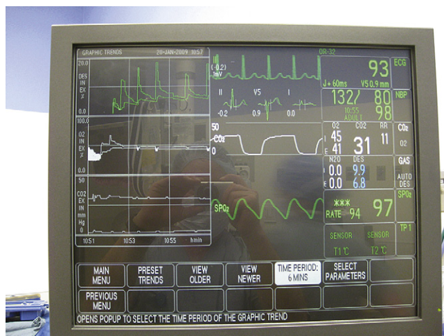
FIGURE 26-20 ■ Solar 8000i physiologic monitor (GE Healthcare, Waukesha, WI). Display of a 6-minute graph of inspired and expired desflurane (top left), oxygen (middle left), and carbon dioxide (bottom left). Injections of 1 mL desflurane are made in the inspired limb of the breathing circuit.
