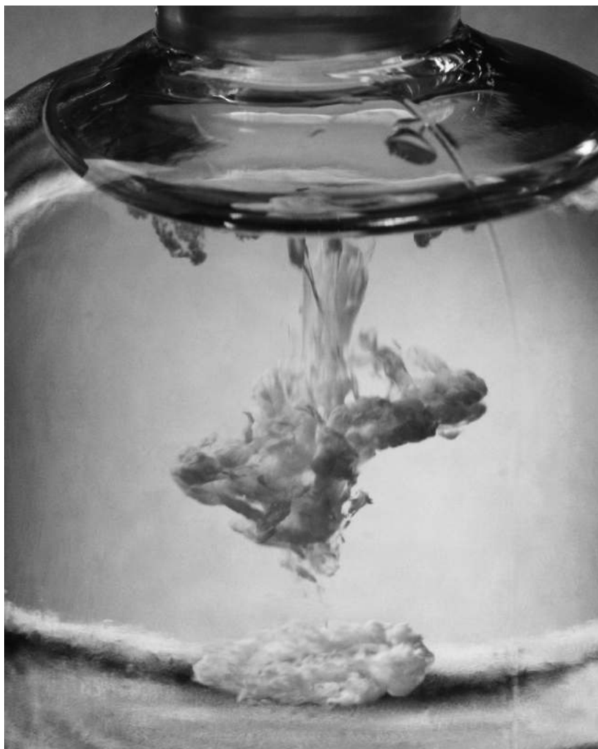
FIGURE 14.4. Distilled liquor of antimony dropped into a bottle of deionized water. The clear, colorless solution immediately precipitates an insoluble white cloud of mercurius vitae (antimony oxychloride) on meeting the water. Prepared by William R. Newman in the laboratory of Dr. Cathrine Reck in the Indiana University Chemistry Department. See color plate 4.
