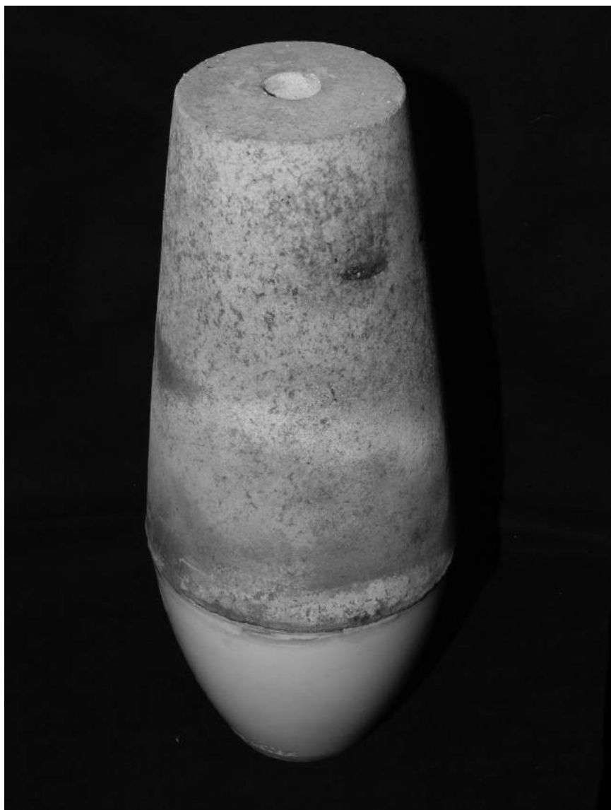
FIGURE 15.5. Modern subliming apparatus used to replicate Newton's experiments, consisting of an inverted, drilled-out fire-assay crucible set atop a porcelain, Coors crucible (in practice, the joint would be taped). The sublimate has permeated the fire-assay crucible, as shown by the variously colored horizontal bands at different heights. Prepared by the author in the laboratory of Dr. Cathrine Reck in the Indiana University Chemistry Department. See color plate 7.
