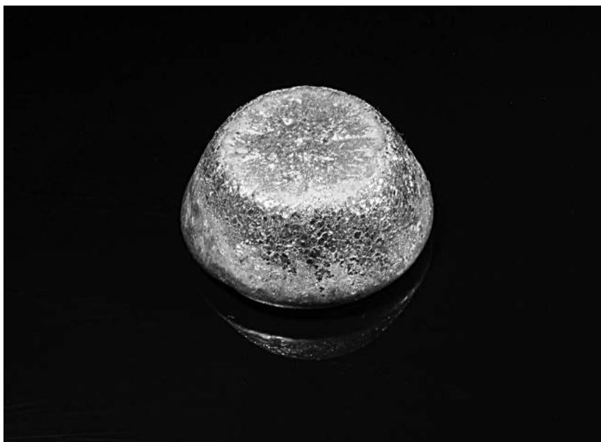
FIGURE 16.1. The “net,” or “Vulcan’s net,” is a purple alloy of copper and metallic antimony. The alloy seems to have been invented by the American alchemist George Starkey (who authored most of the texts attributed to Eirenaeus Philalethes). Starkey was impressed by its fine, crystalline surface, which reminded him of network. He based the name “net” on the mythical net of bronze that Vulcan used to ensnare Mars and Venus in bed together. The alloy played a major role in the preparation of the Philaethan sophic mercury, and Newton made great use of it in his own experimentation. Prepared by the author in the laboratory of Dr. Cathrine Reck in the Indiana University Chemistry Department. See color plate 8.
