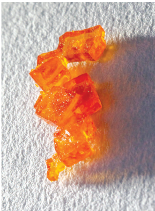
PLATE 6. Crystals deposited by slow evaporation of liquor of antimony. Prepared by the author in the laboratory of Dr. Cathrine Reck in the Indiana University Chemistry Department.
