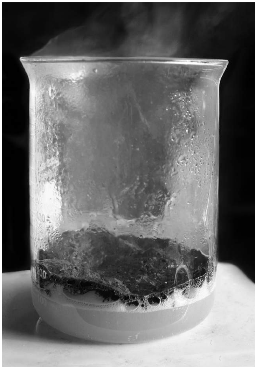
FIGURE 15.3. Newton's liquor of antimony being produced from aqua regia (nitric acid "sharpened" with sal ammoniac) and stibnite (antimony trisulfide). A vigorous reaction takes place, leaving behind a yellowish-white precipitate. Prepared by the author in the laboratory of Dr. Cathrine Reck in the Indiana University Chemistry Department. See color plate 5.
