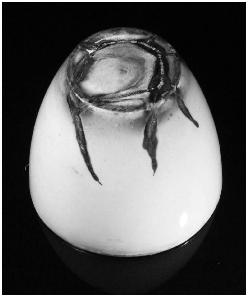
FIGURE 17.2. Cracked crucible used in subliming ceruse from Newton's succedaneum to "volatile Venus" as described in Fatio de Duillier's letter of August 1, 1693. The multiple colors on the bottom and sides of the crucible reveal the presence of lead and copper compounds as well as the partially reduced metals themselves. Prepared by the author in the laboratory of Dr. Cathrine Reck in the Indiana University Chemistry Department. See color plate 10.
