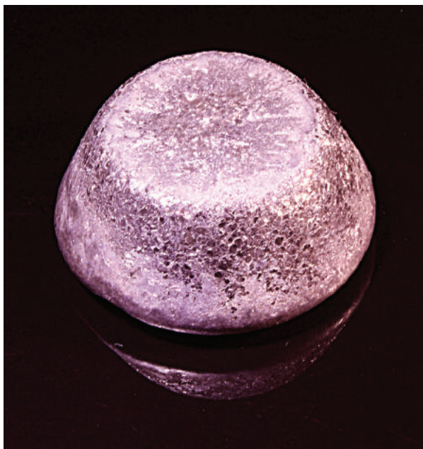
PLATE 8. The “net,” or “Vulcan’s net,” is a purple alloy of copper and metallic antimony. The alloy seems to have been invented by the American alchemist George Starkey (who authored most of the texts attributed to Eirenaeus Philalthes). Starkey was impressed by its fine, crystalline surface, which reminded him of network. He based the name “net” on the mythical net of bronze that Vulcan used to ensnare Mars and Venus in bed together. The alloy played a major role in the preparation of the Philalathan sophic mercury, and Newton made great use of it in his own experimentation. Prepared by the author in the laboratory of Dr. Cathrine Reck in the Indiana University Chemistry Department.
