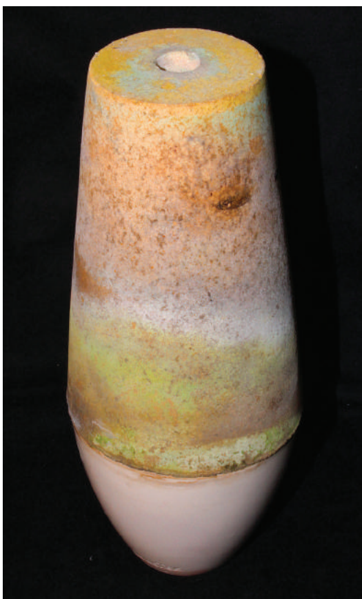
PLATE 7. Modern subliming apparatus used to replicate Newton's experiments, consisting of an inverted, drilled-out fire-assay crucible set atop a porcelain, Coors crucible (in practice, the joint would be taped). The sublimate has permeated the fire-assay crucible, as shown by the variously colored horizontal bands at different heights. Prepared by the author in the laboratory of Dr. Cathrine Reck in the Indiana University Chemistry Department.
