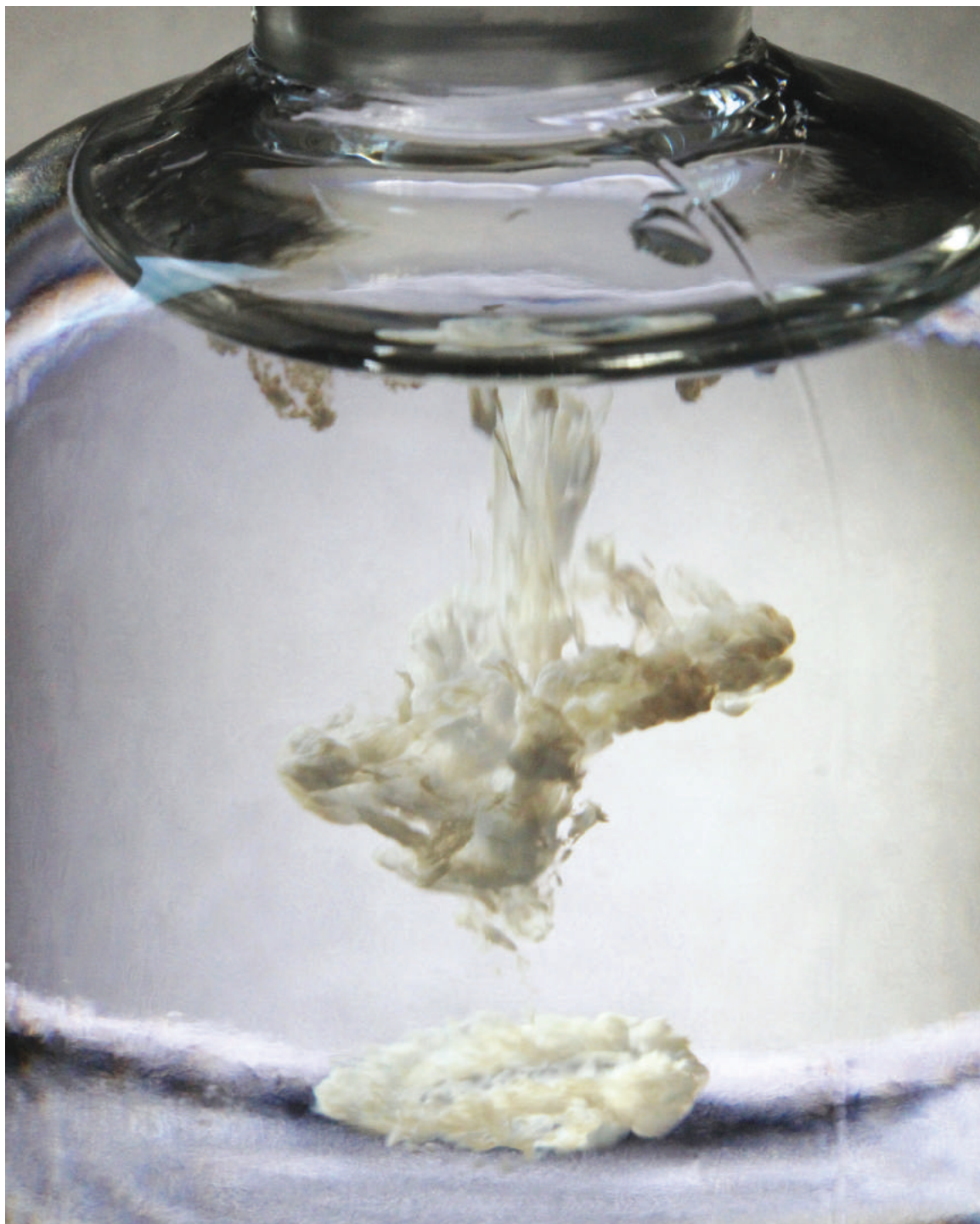
PLATE 4. Distilled liquor of antimony dropped into a bottle of deionized water. The clear, colorless solution immediately precipitates an insoluble white cloud of mercurius vitae (antimony oxychloride) on meeting the water. Prepared by William R. Newman in the laboratory of Dr. Cathrine Reck in the Indiana University Chemistry Department.
