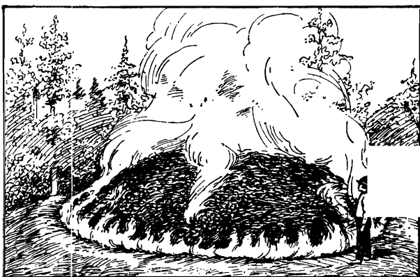
FIG. 7.—Sketch of a Meiler shortly after it has been lighted.
