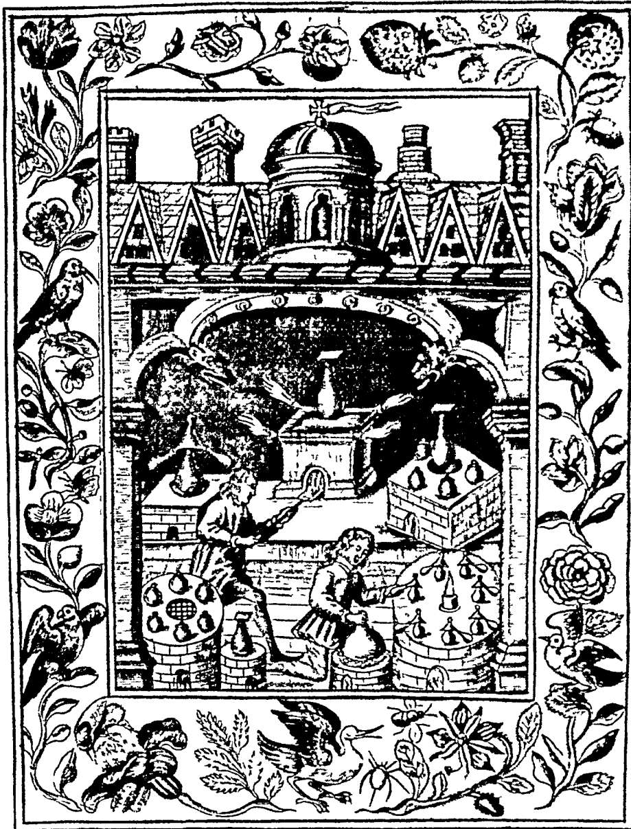
10 Alchemical furnaces in use for digestion and multiple distillation (From Thomas Norton, Ordinall of Alchimy , London, 1652)
